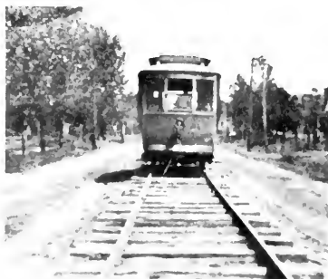
Pekin's first street car, shown on Derby St., ran from the industries to the Park. It was powered by batteries and had to be charged every night.
