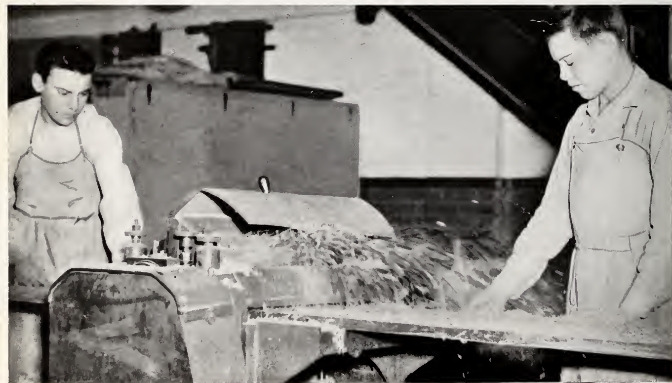
Horner and Cargal surface rough lumber as the starting point for their project.
