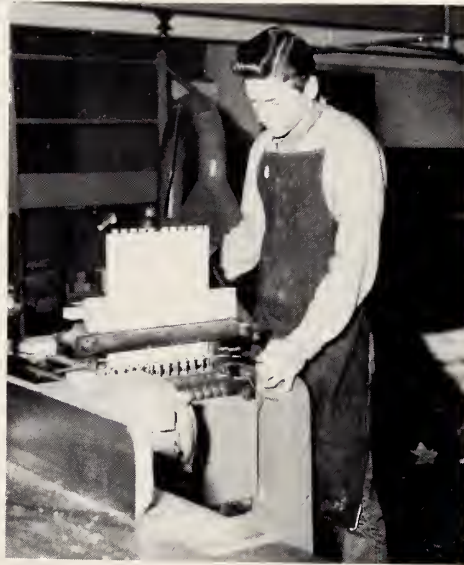
Marvin Richard keeps an eye on the dove-tail machine as he constructs drawer sides.
