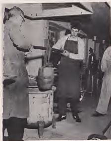
Mike Murphy and Mr. Holder lift a pot of molten metal before pouring it into the mold.
