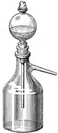
FIG. 33.—Kitasato filter for filtering hypodermic solutions, culture media, sera, water, etc. The material to be filtered is placed in the globose container and forced through the clay (infusorial earth) tube (Berkefeld filter bougie) by connecting the receiver with a vacuum pump. All parts of the filter must, of course, be sterilized by heat before and after using. (Williams.)
