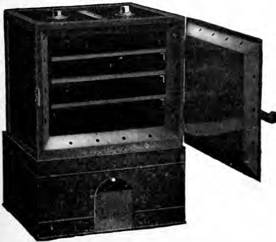
FIG. 14.—A hot air sterilizer. These sterilizers are double-walled, on stand, with perforations at top for thermometers. Ordinary baking ovens which can be secured from hardware dealers will serve the purpose.
