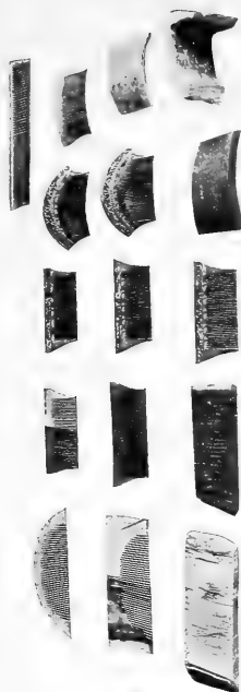
Fig. 3. Combs at different stages of manufacture.
