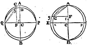
Quare si dicatur CQ sive CD, b, & AC sive CE, r, dicaturque abscissa QF, AF; in wraque figura, x; erit in prima figura  $\overline{FG}^2 = \frac{r^2}{h^2} \times \overline{2bx - xx}$ ;  $\overline{Fg}^2 = 2bx - xx$ ,
