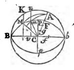
feu w distantia foci à centro in figura  $A \in M$ , sit L Logarithmus quantitatis  $a \vee \frac{a+x}{a-x}$ , & ultima ratio gravitatis particulæ A in frustum planis  $A \in M$ ,  $A \in M$ , terminatum ad gravitatem in frustum Spheræ centro C radio  $C \in A$  descriptæ iisdem planis contentum, exit ea  $3 \in M$   $\frac{1}{2} \times \frac{1}{2} \times$
