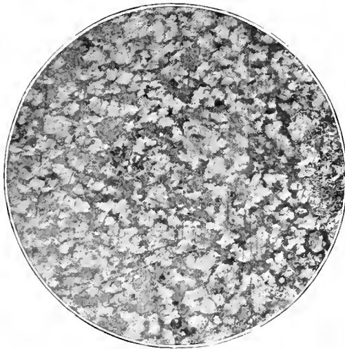
Fig. B— \frac{3}{8} " Steel annealed for a few minutes at 750^\circ\text{C} . \times 150 D. (Etched with \text{HNO}_3 .)
