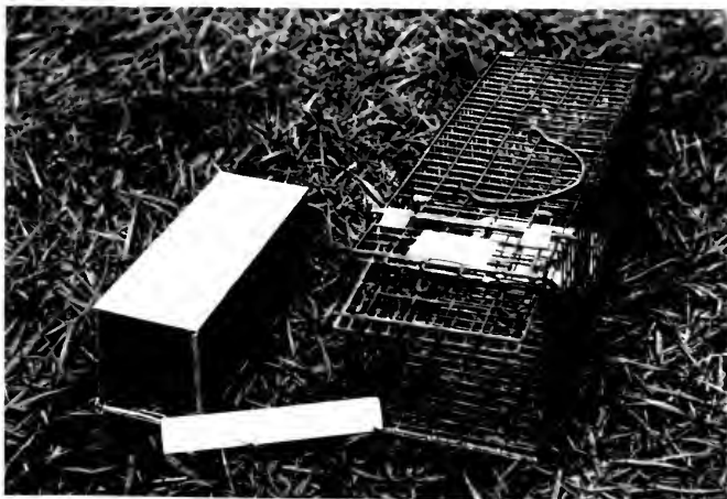
Figure 4-1. Sherman (on left) and Tomahawk live traps for small mammals.
