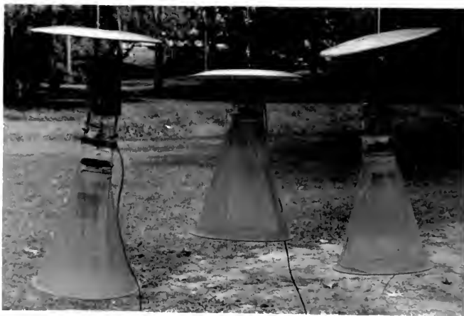
Figure 2-4. A CDC trap and modified traps (from left - CDC with UV light source, normal CDC, and hamster-baited trap).
