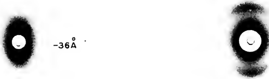
Plates 1 and 2. X-ray diagrams of oriented air-dried Antirrhinum chloroplasts. Kiessig camera. The little tubes are oriented horizontally. Distance sample - 20 and 40 cm.
