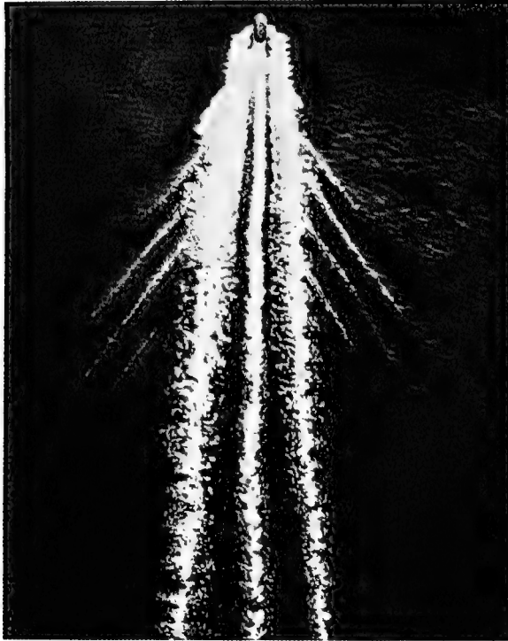
FIGURE 7. Wake of PT boat at 25 knots.
