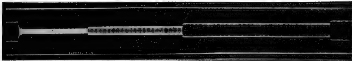
FIGURE 5. Oscillograph record showing negligible transients produced by receiver amplifier gain changes in equipment C (input signal maintained at steady value).
