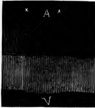
Fig. 64.—Simultaneous tracings from auricle and ventricle of turtle's heart. Between the crosses the vagus was stimulated, with the effect that the auricular beat diminished in force but not in frequency, while the ventricular beats were practically unaffected. (From Howell's Physiology .)
