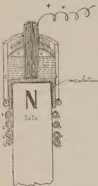
FIG. 50. Sectional diagram of electro-magnetic streaming. The small arrows show the direction of the electrical current and the large ones the movement of the mercury.
