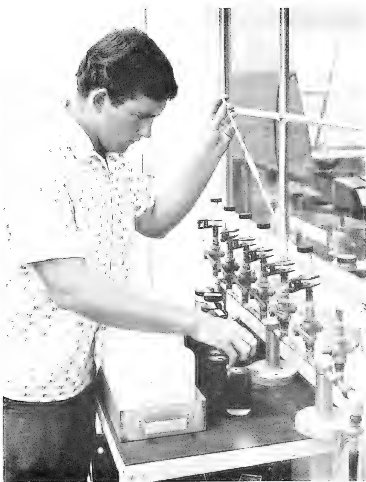
Figure 5. Manifold used in Millipore filtration to prepare slides of microorganisms.
