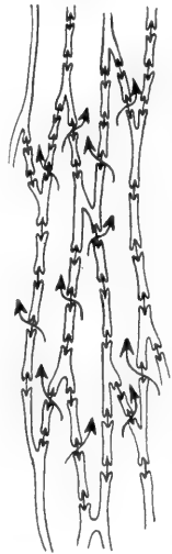
FIG. 56.—Diagram indicating by arrows how the water in the tracheids of pine passes longitudinally from one tracheid to another.
