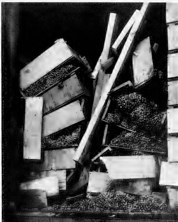
Fig. 31. California wine grapes in open lugs, showing loss from poor container, faulty stowing and bracing
