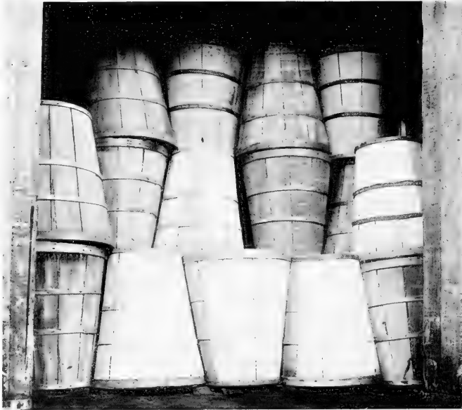
Fig. 30. Lettuce in hampers, loaded to top of car. Note absence of ventilation channels.
