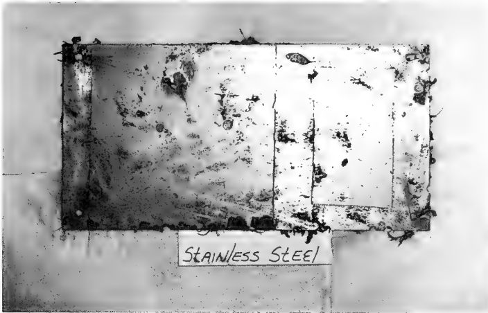
Figure 13. Stainless steel panel with saran film after biological growth had been removed with a spatula.
