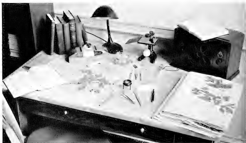
FIG. 4.—Equipment on a botanizer's work table. The articles on the table include dissecting needles, forceps, a scalpel, a ruler, watchglasses, test tubes and test tube holders, an alcohol lamp, a tripod magnifier and two dissecting microscopes.
