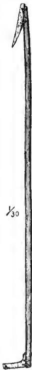
FIG. 311.—Long blubber hook. held on by two lashings of small seal thong, each passing through a large transverse hole in the prong and a corresponding one in the pole. The upper pair of holes do not exactly match. There are also two unused holes, one in the pole below the upper hole and one above the upper hole in the prong. These holes and the new appearance of the lashings indicate that the prong is part of another hook recently fitted to this pole. The two lashings are made by a single piece of thong.
