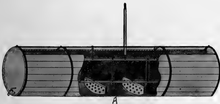
Figure 20. Tank for receiving lime after it has been slacked and is ready to mix with copper sulphate. The agitator is the special feature of this tank.
