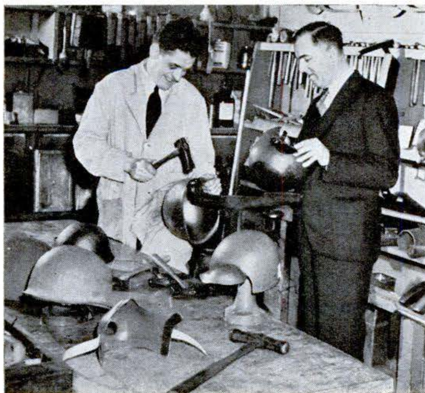
Frequent measurements are taken and recorded by the armorer to insure proper contours and sizes. Above, a workman is measuring a model to determine a place for earpieces
