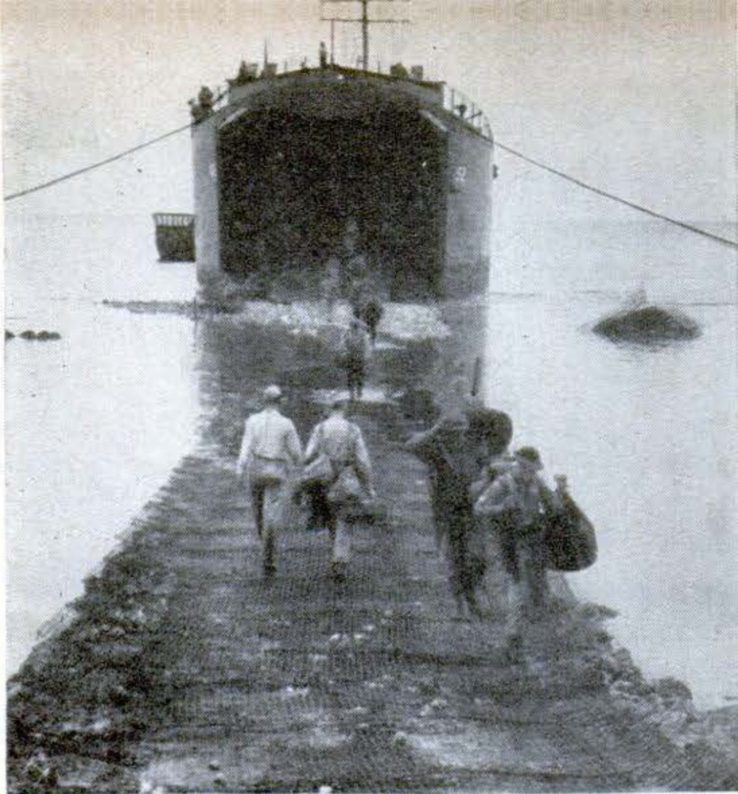
Grounded on the beach of a South Pacific island, a landing ship is connected with the shore by means of a mesh road that gives vehicles footing in sand
