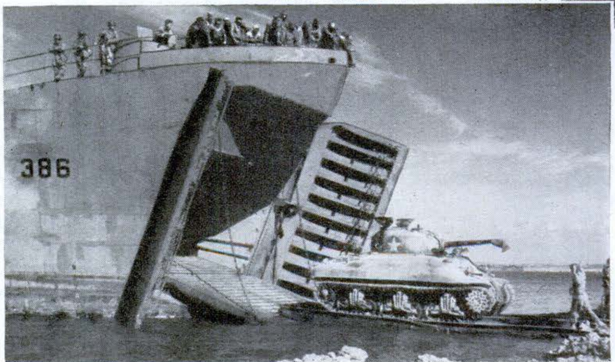
Grounded on the beach of a South Pacific island, a landing ship is connected with the shore by means of a mesh road that gives vehicles footing in sand
