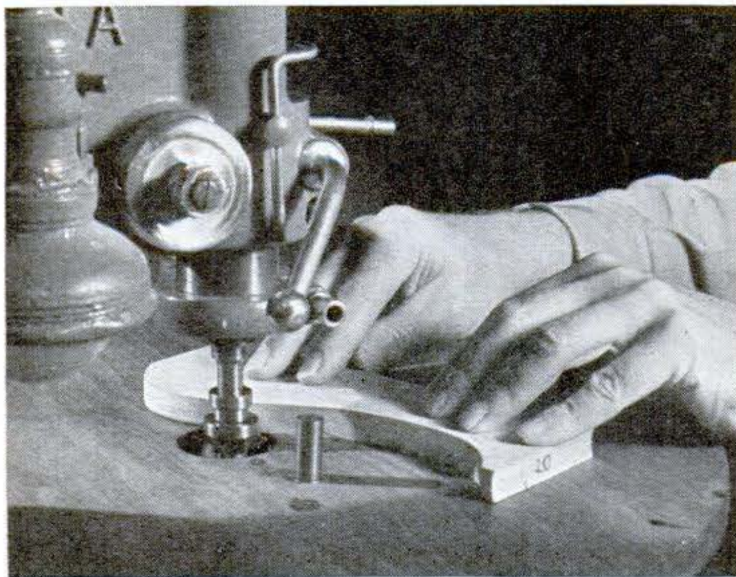
The shelves and slats may conveniently be rounded on a drill press which is equipped with a molding cutter. Rounding should be done on the underside
