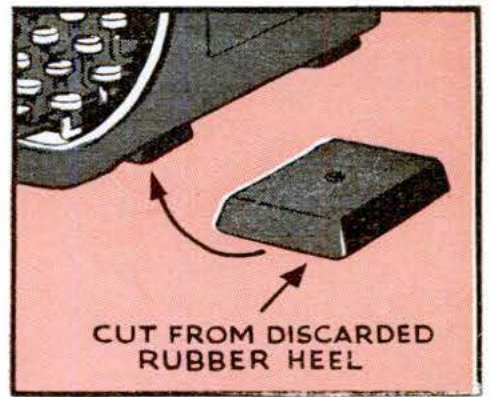
Most worn-out typewriter feet can be replaced satisfactorily with others cut from old rubber heels
