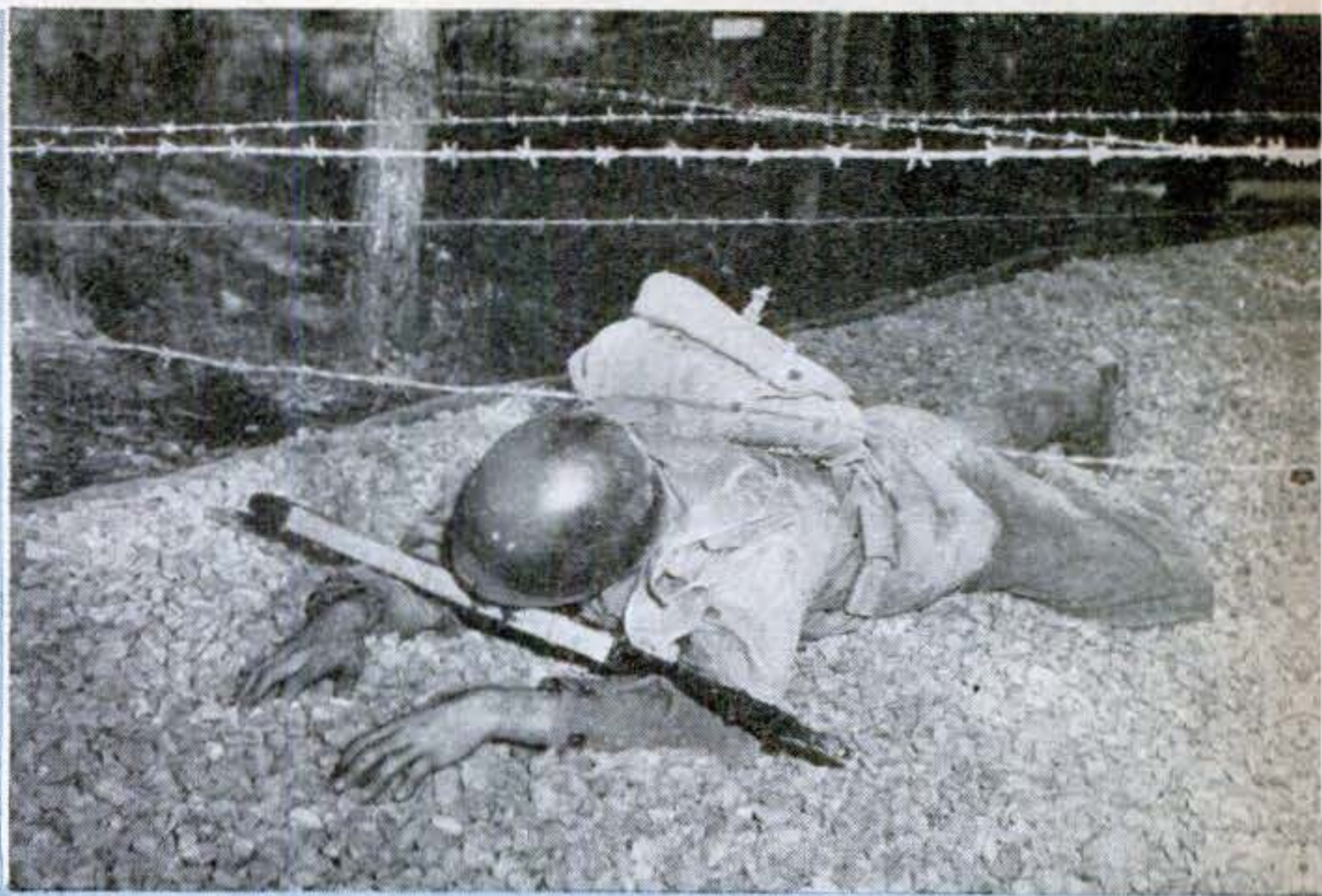
THE JACKET undergoes its acid test when a soldier, carrying his rifle in the crooks of his arms as he might in actual battle, and hugging the ground to avoid being caught on low-hanging barbed wire, crawls on his belly over needle-pointed chipped granite. Other tests include sliding into concrete tank traps and down steep revetments of sand and slag. The tear and ripped arm seam shown at the left was the result of only one trip around the course
