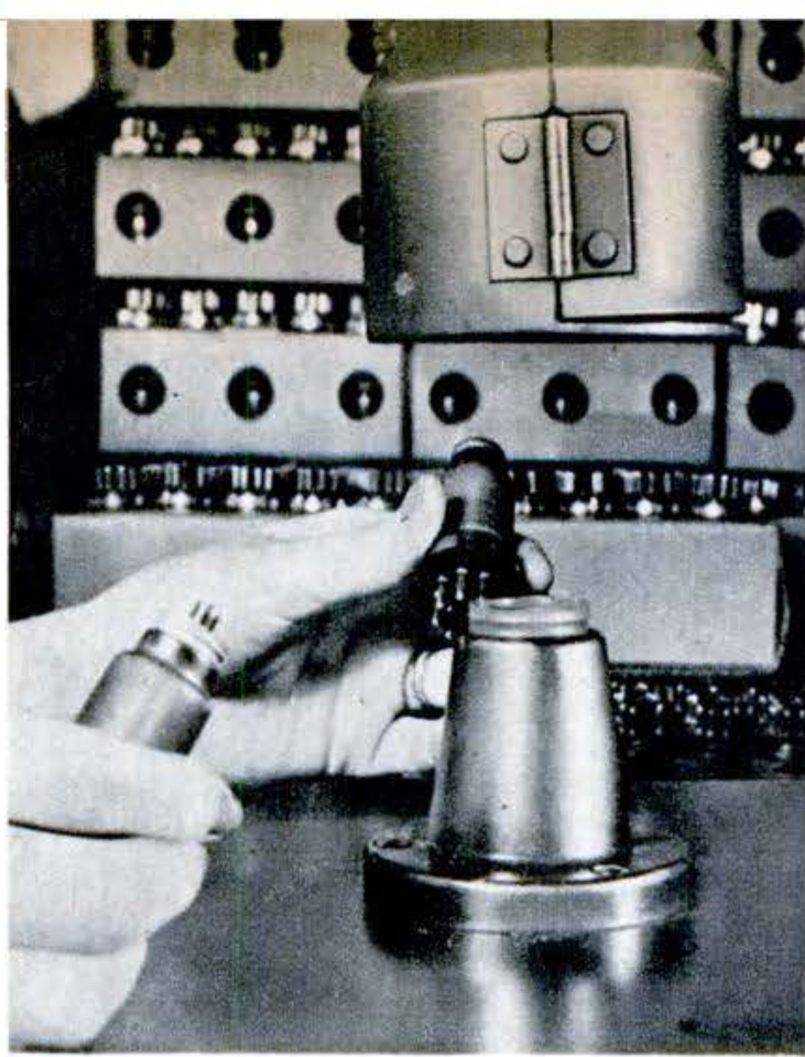
ALIGNING RINGS. Synthetic resin used in clinching tube parts lasts three weeks, where rubber was replaced often
