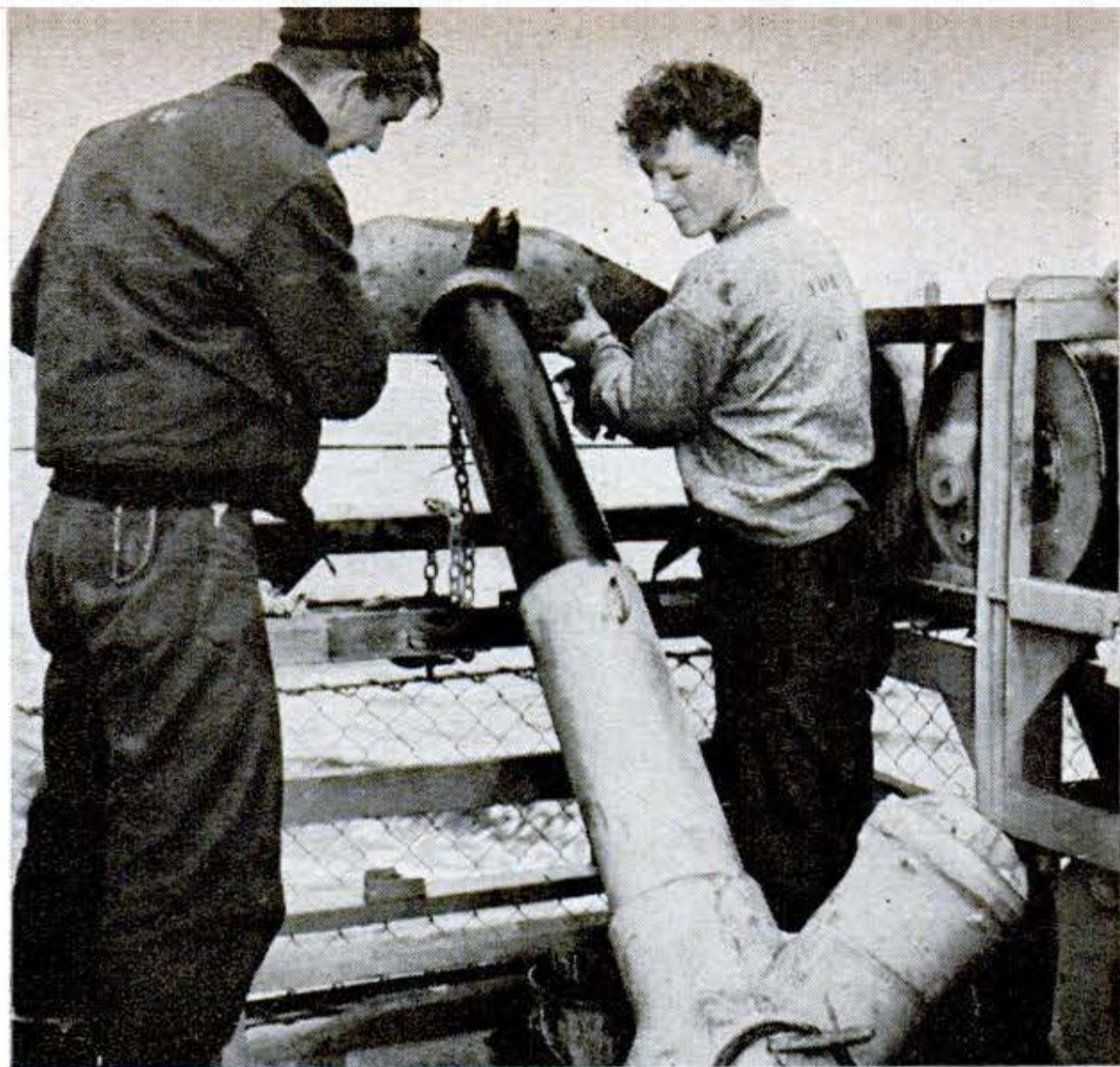
LOADING ARBOR. K-guns that hurl depth charges abeam the ship are loaded by means of arbors, which are kept racked along the side of the deckhouse. Here the shank of an arbor is being inserted in the barrel of the K-gun. The curved plate is made to hold the "can"
