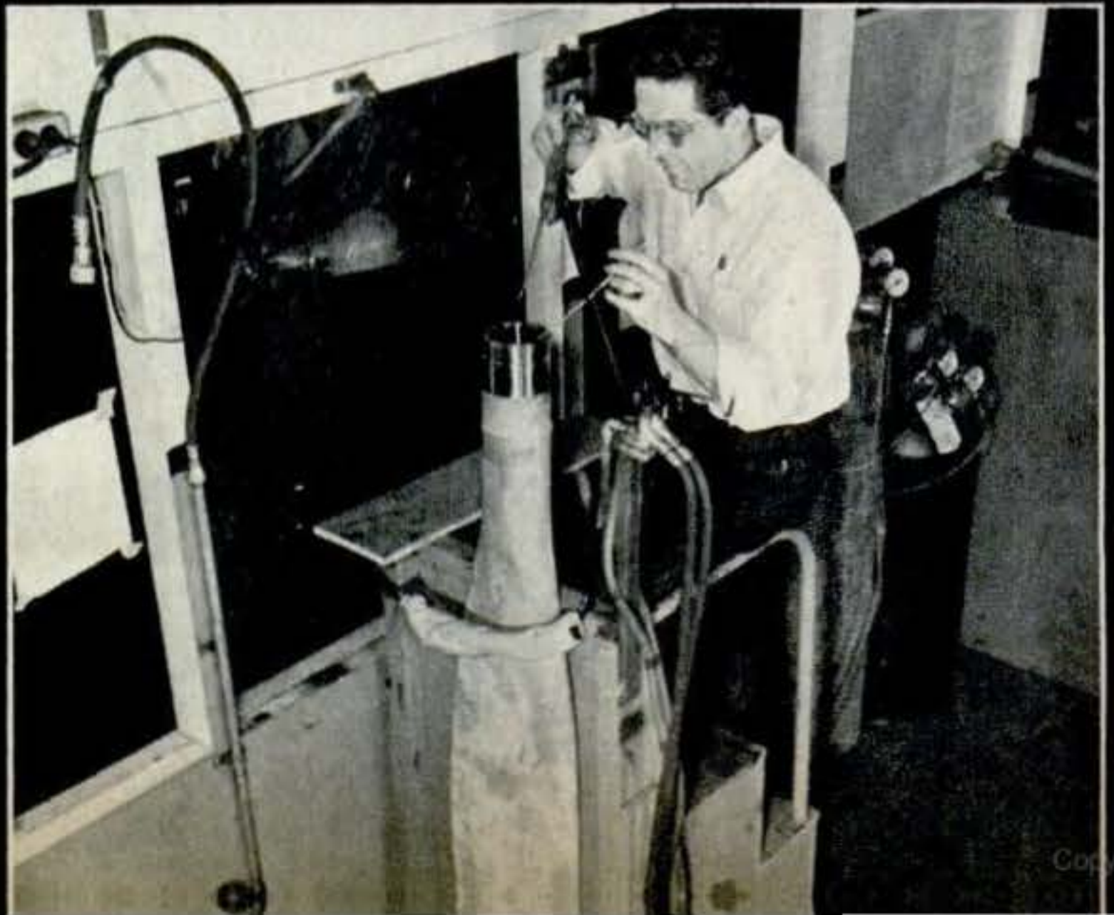
4 One of the last operations in making a blade is the pouring of melted lead into the balance cup in the base to give the propeller accurate balance
