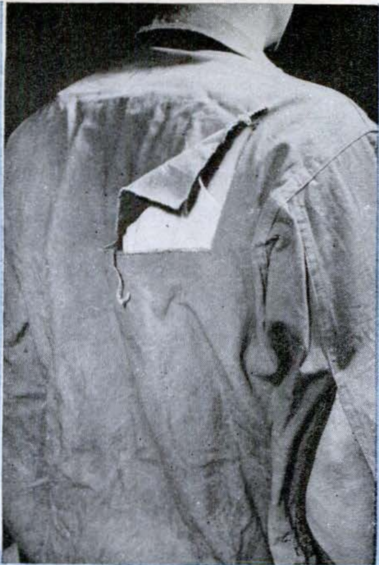
THE JACKET undergoes its acid test when a soldier, carrying his rifle in the crooks of his arms as he might in actual battle, and hugging the ground to avoid being caught on low-hanging barbed wire, crawls on his belly over needle-pointed chipped granite. Other tests include sliding into concrete tank traps and down steep revetments of sand and slag. The tear and ripped arm seam shown at the left was the result of only one trip around the course
