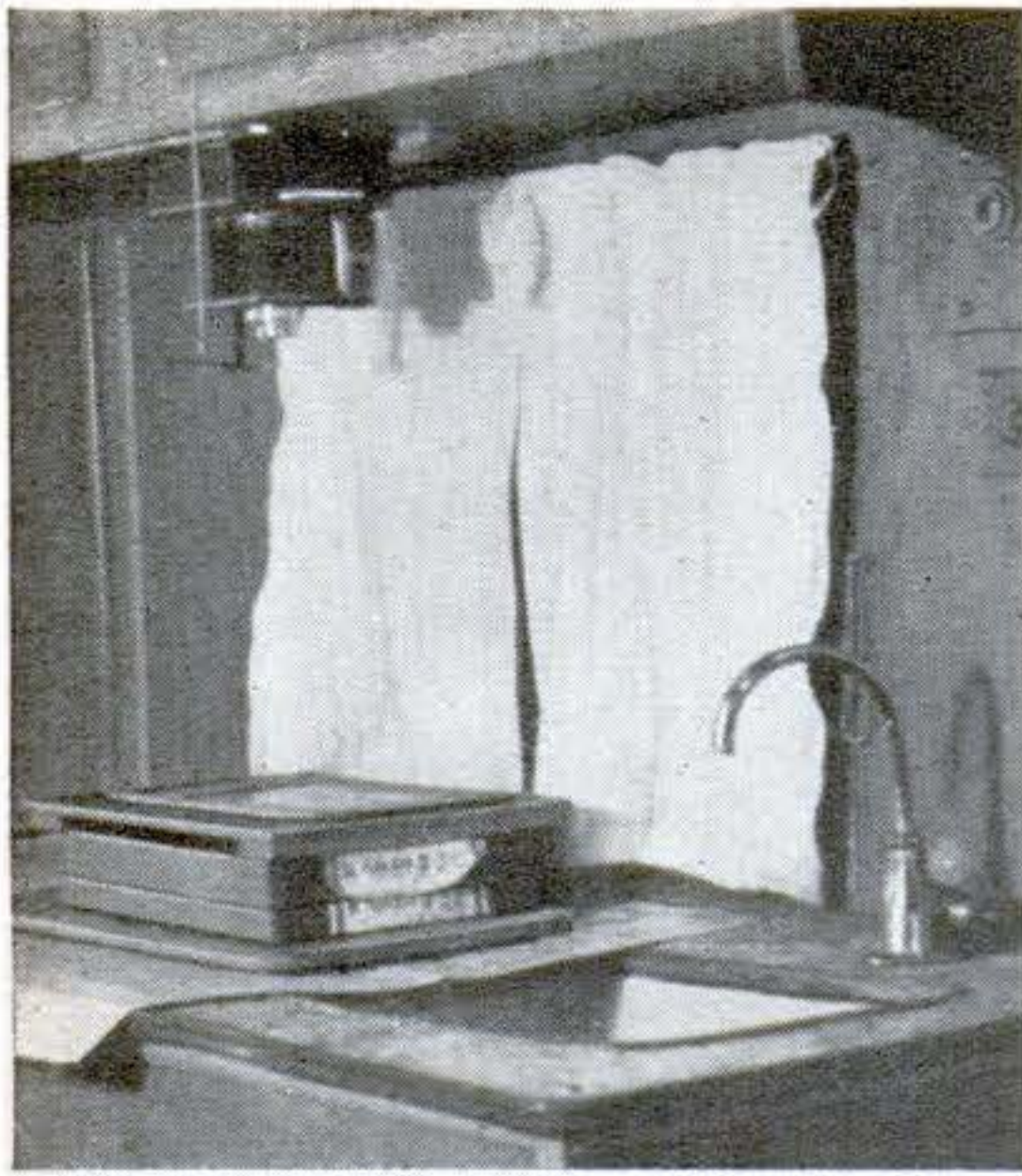
With space at a premium in a house trailer, this homemade enlarger is necessarily compact, though without sacrifice of efficiency. The string beside it at the left is connected to the light switch. Pictured above are the parts; at right, a close-up
