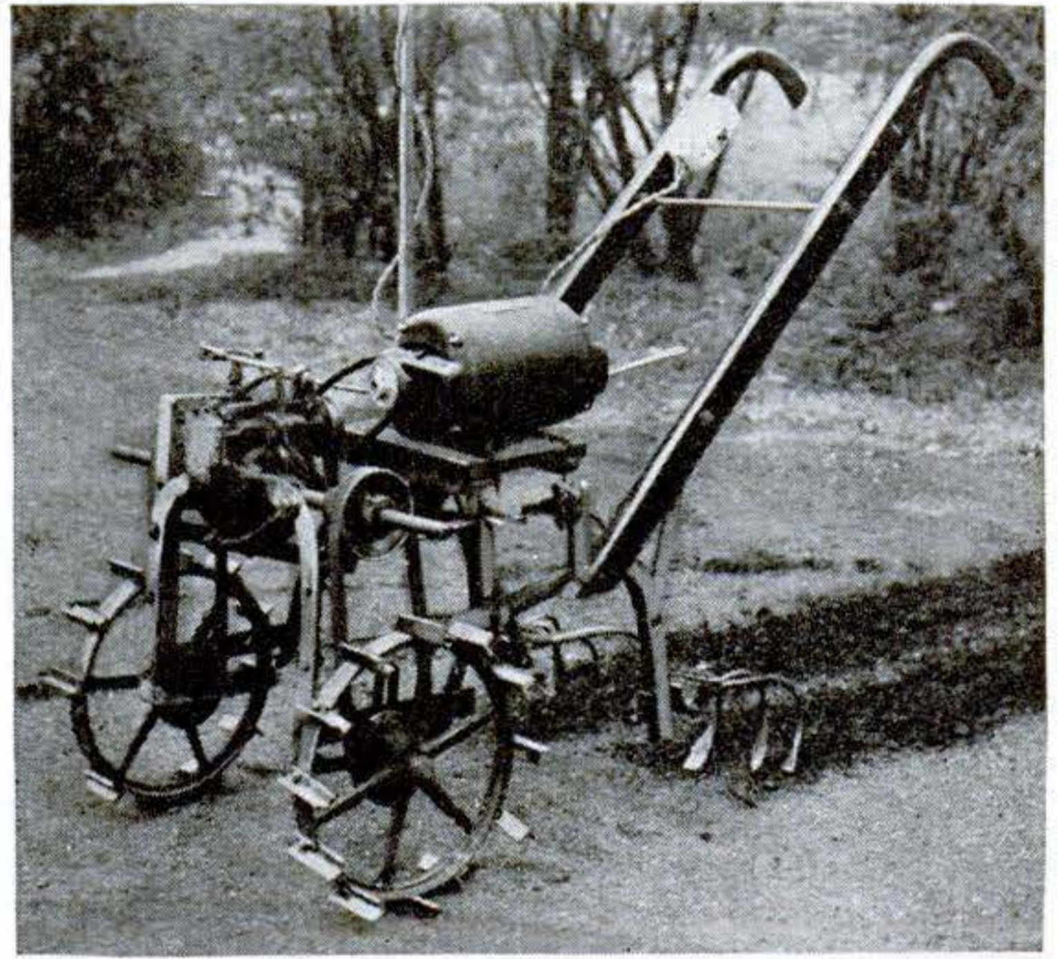
A small electric motor powers this cultivator assembled from odds and ends of scrap material
