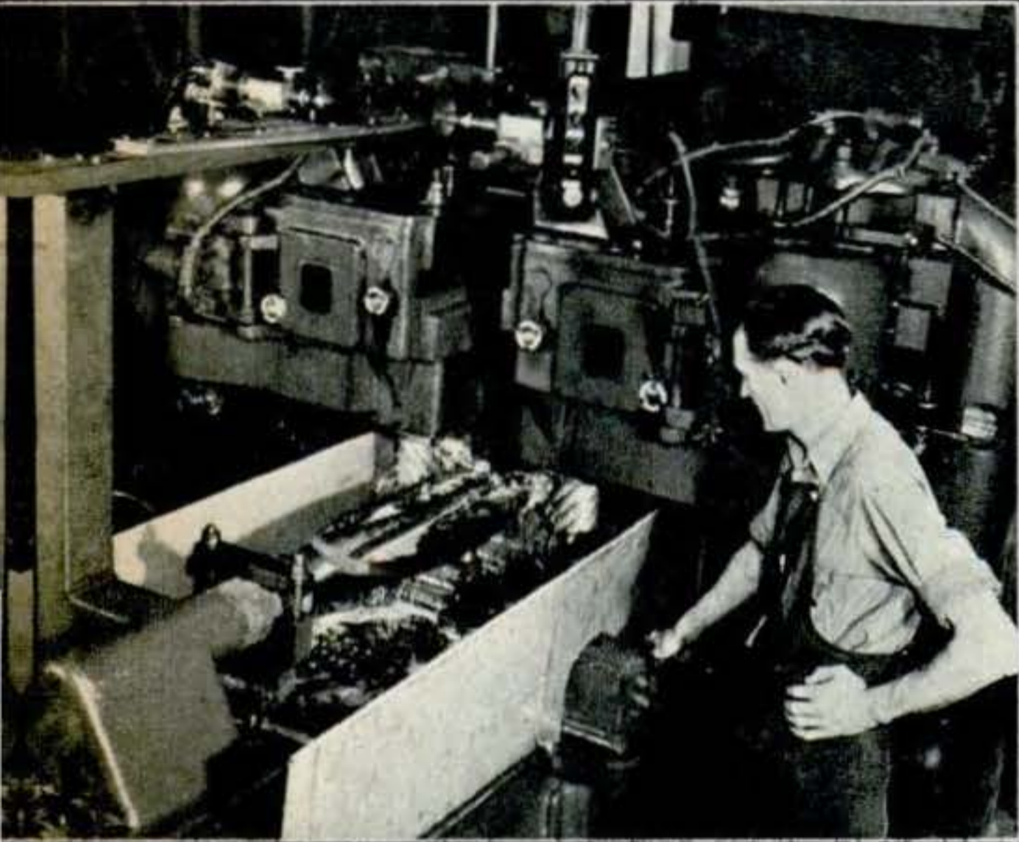
1 Guided by a master form and follower (on top of the upright), this shaper cuts extra width and weight from the original blade forging
