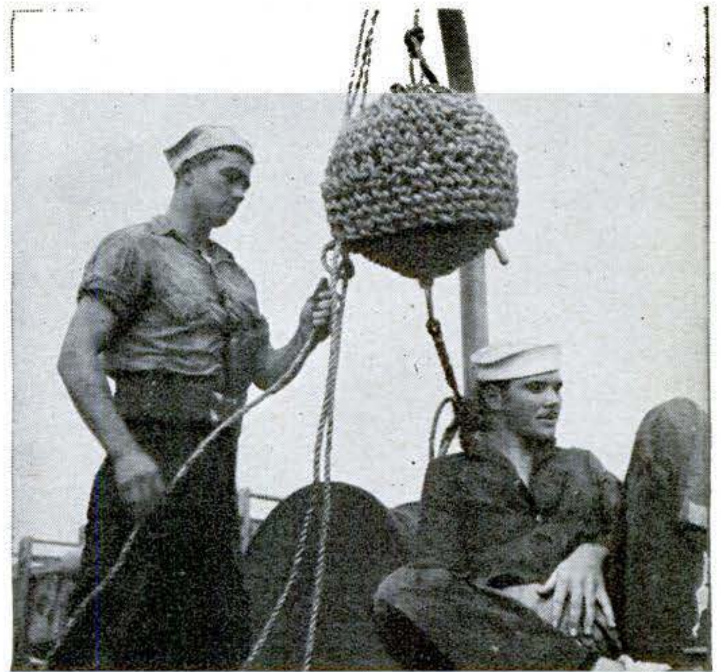
MARLINSPIKE SEAMANSHIP fills in odd hours at sea. This seaman is reinforcing a wicker fender with a series of half hitches. The fender is used as a bumper when the DE comes alongside other ships
