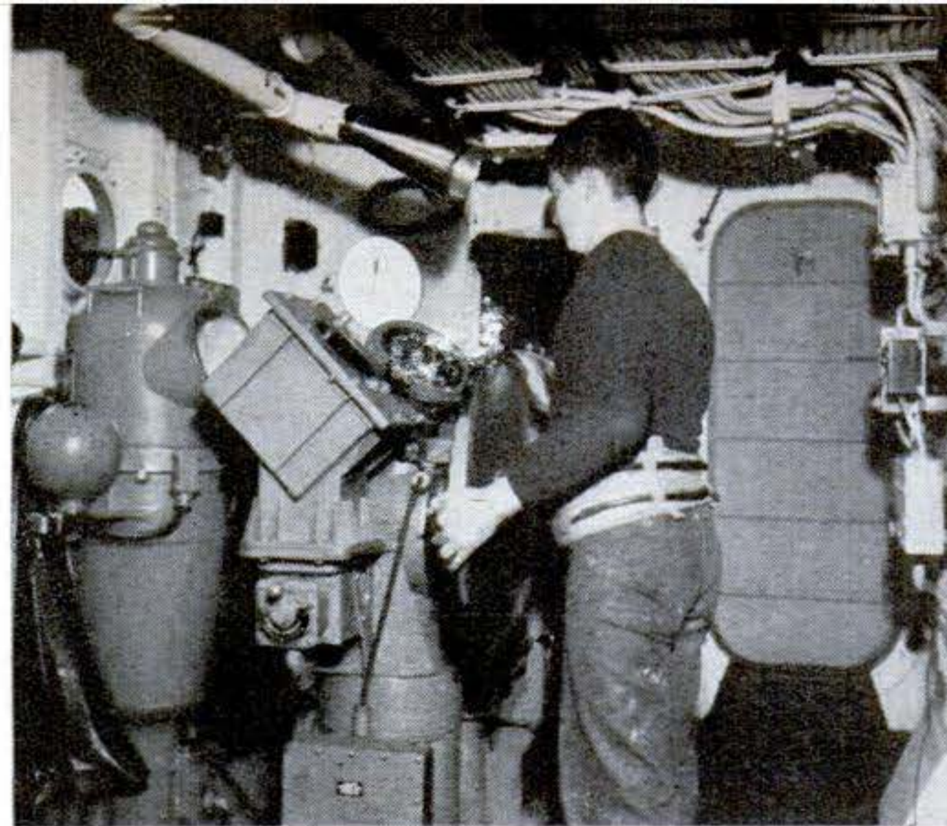
WHEELHOUSE. Gyrocompasses and other modern navigating aids help the helmsman to hold his course. Convoy work calls for close co-ordination
