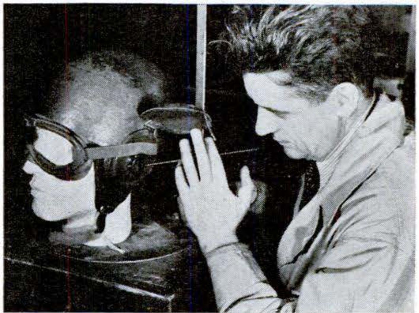
Frequent measurements are taken and recorded by the armorer to insure proper contours and sizes. Above, a workman is measuring a model to determine a place for earpieces
