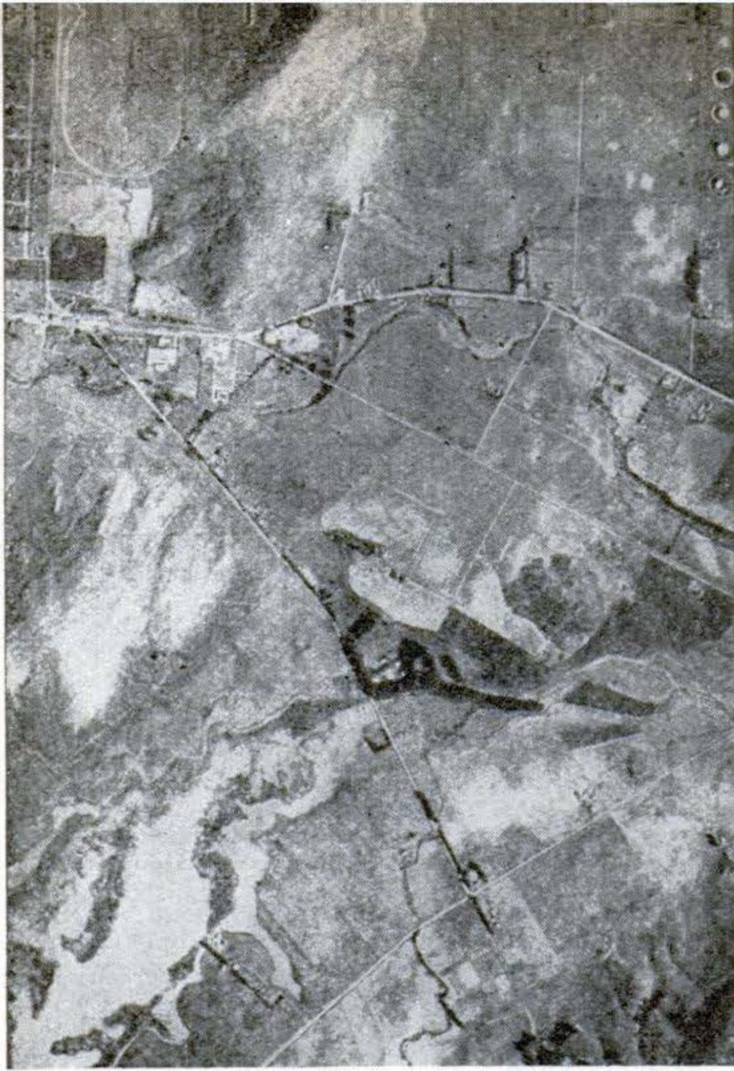
FROM PHOTO TO MAP. Interpretation of detail on an aerial photograph is illustrated above by the comparison of a vertical camera shot with a keyed map based upon it. Note how highways show up as white lines with angular turns; railways have gradual curves. Points of special interest to a bombardier are rail yards (3), oil tanks (9), airport (10). The curious oval in the upper left-hand corner (14) is the race track at the fair grounds
