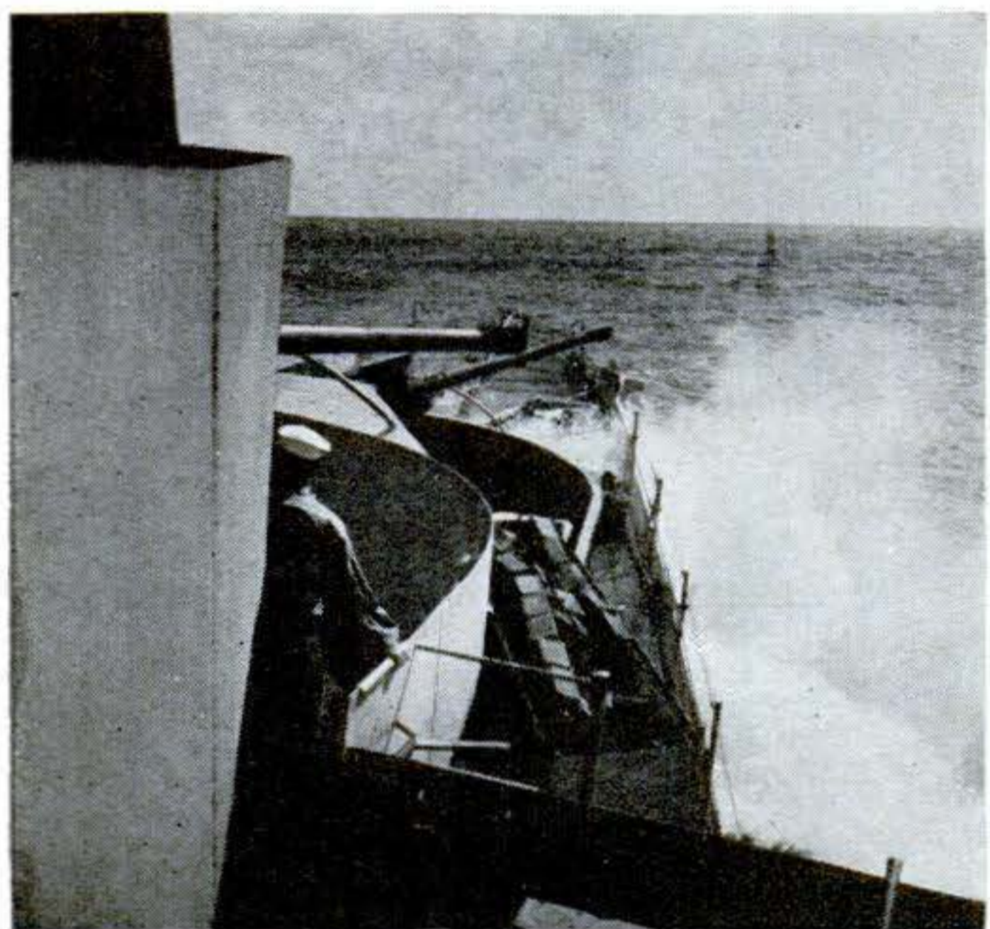
BOW of the DE has a flaring design that throws back the seas and keeps her from shipping too much water. Even so, there is plenty of flying spray, even on the exposed bridge, when waves run high
