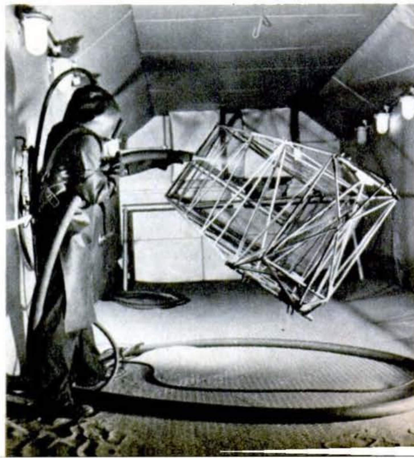
SANDBLASTING prepares finished framework for painting. The masked worker below is playing fine sand and compressed air on a tail section
