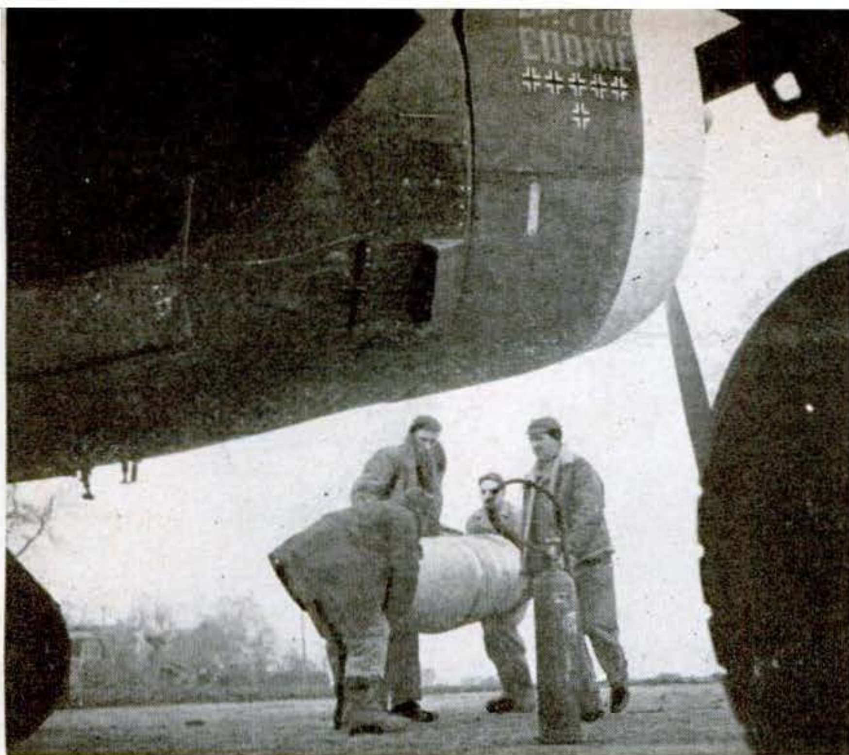
BELLY TANKS are reloaded and charged with pressure to make them work at high altitude. Notice the six black crosses on the nose of this plane; each stands for an enemy shot down. Some pilots prefer swastikas
