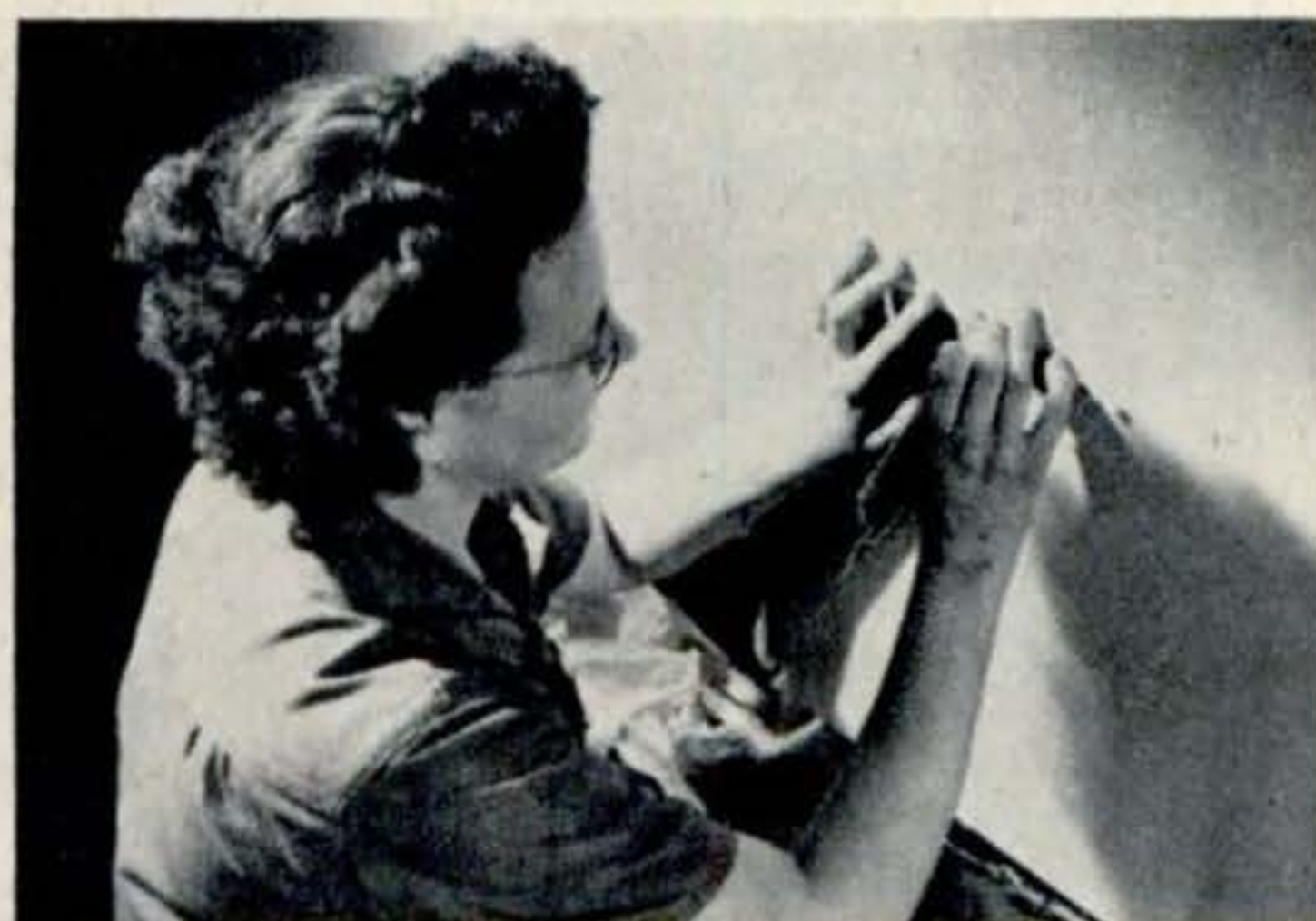
FABRIC is stitched and tied to fuselage and wing sections with heavy thread. One worker pushes the long needle through, while another sends it back
