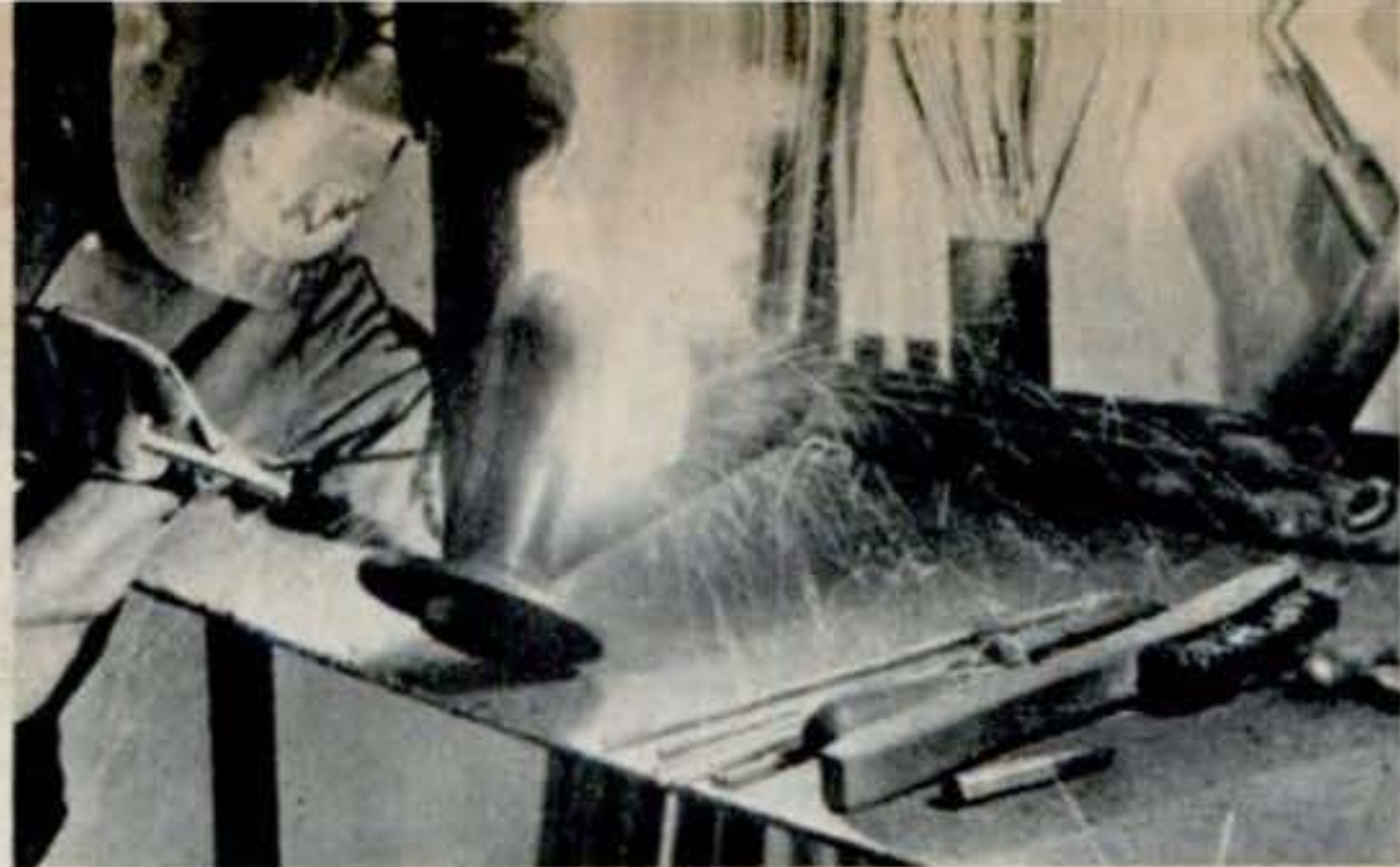
LANDING GEAR parts are assembled by welding members together into clusters. Arc-welding gives rugged strength needed for crash landings
