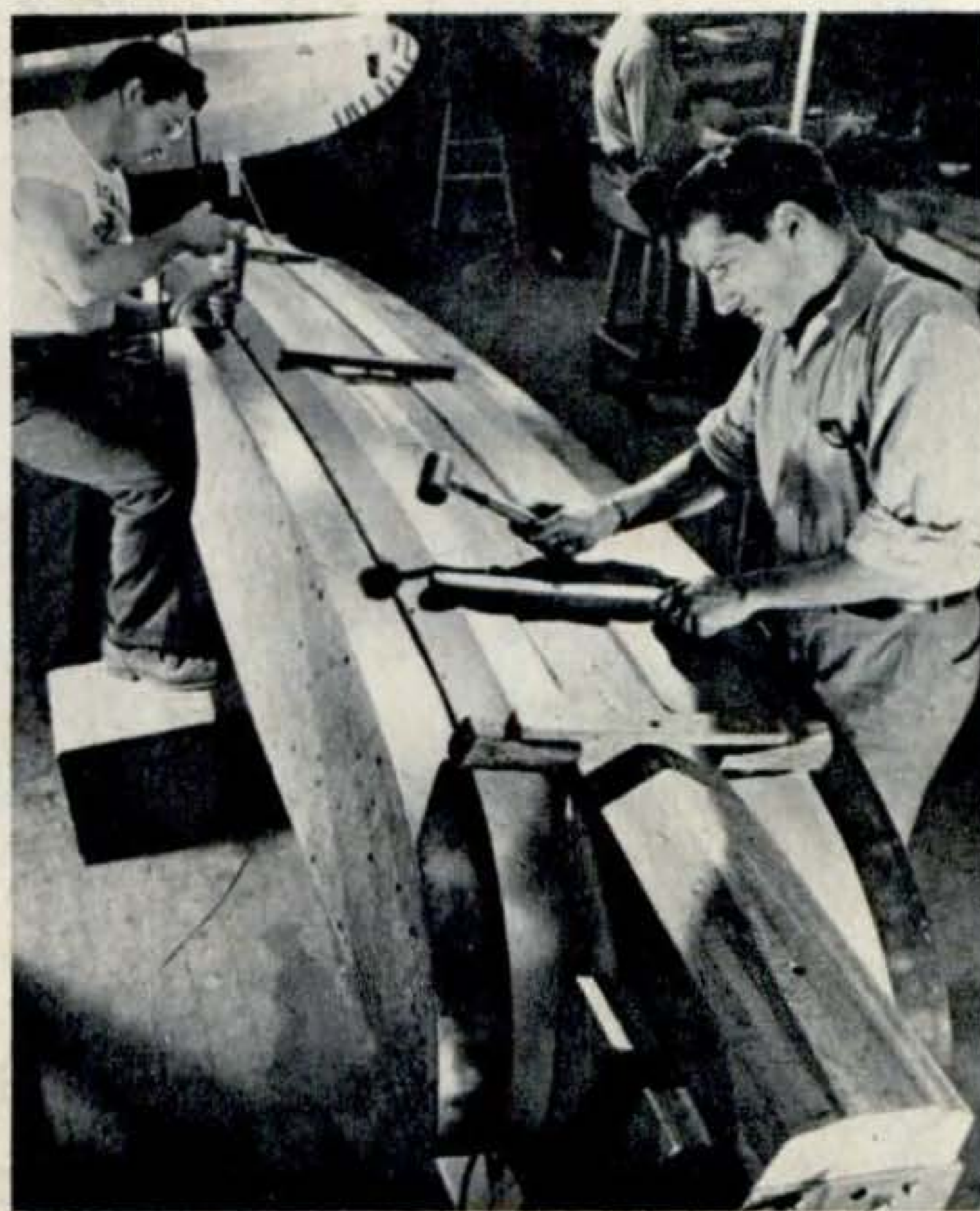
FAIRING STRIPS to cover the opening between wings and fuselage are shaped and drilled over a wooden form which is laminated to prevent warping
