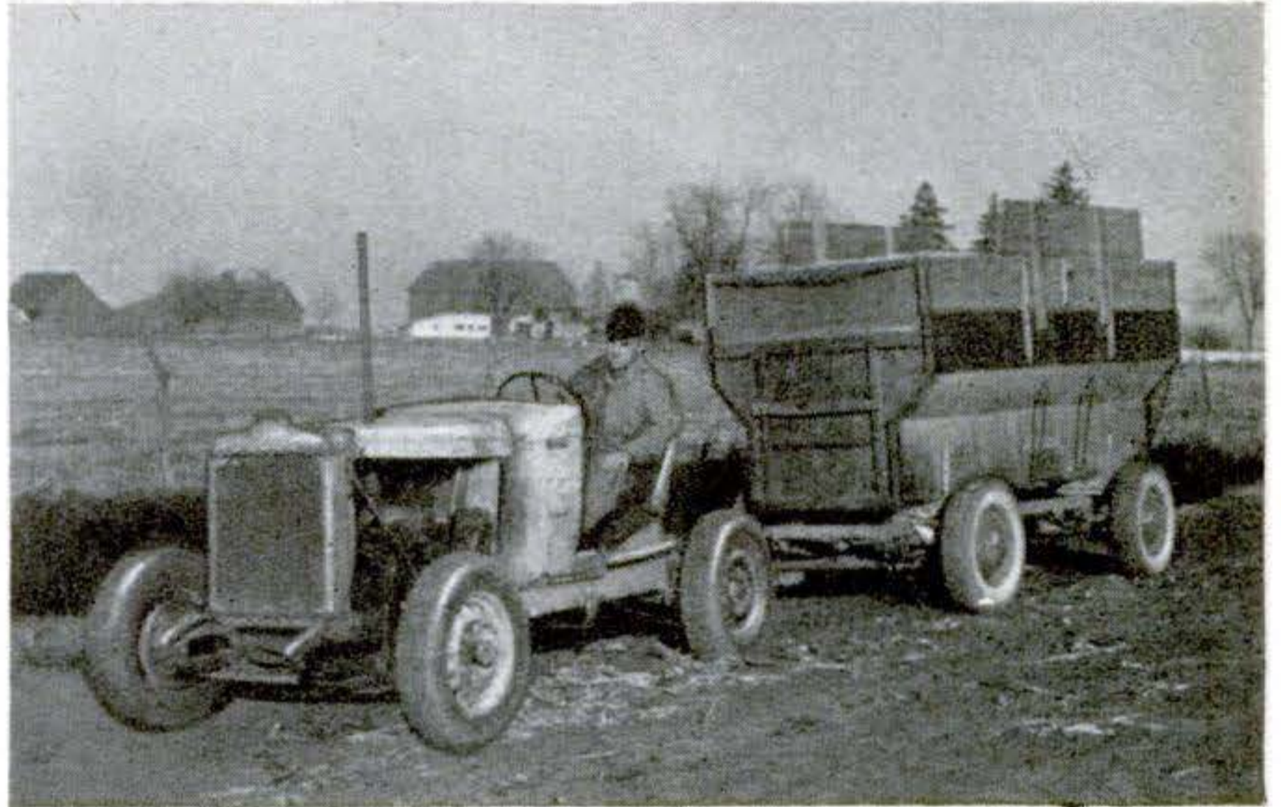
Enough drawbar pull to handle heavy loads is delivered through a second transmission and universal joint mounted back of the first
