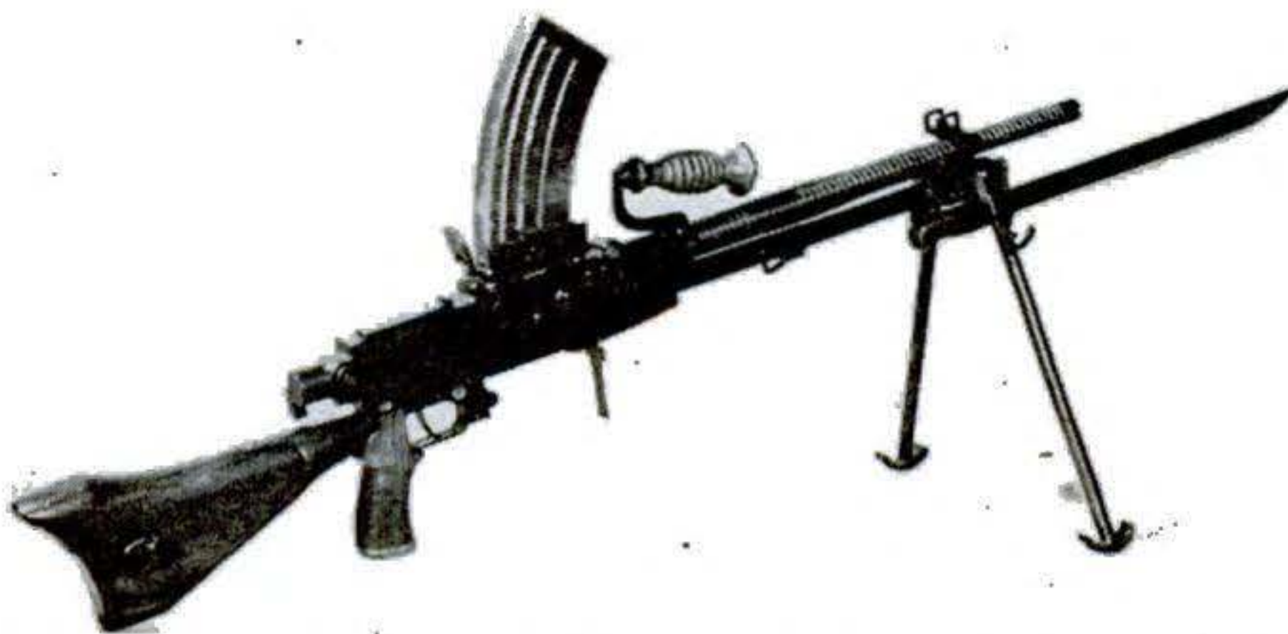
JAPANESE LIGHT MACHINE GUN, 6.5-mm., type 96 (1936). It is gas operated, magazine fed, air cooled; has bayonet for in-fighting
