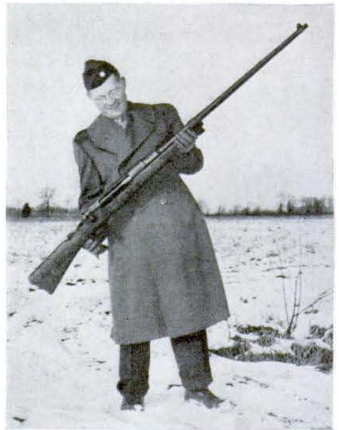
FIRST ANTITANK WEAPON. Lt. Col. George B. Jarrett (see page 57) displays a .50 caliber, single-shot rifle developed by the Germans in World War I. It weighs about 37 pounds.
