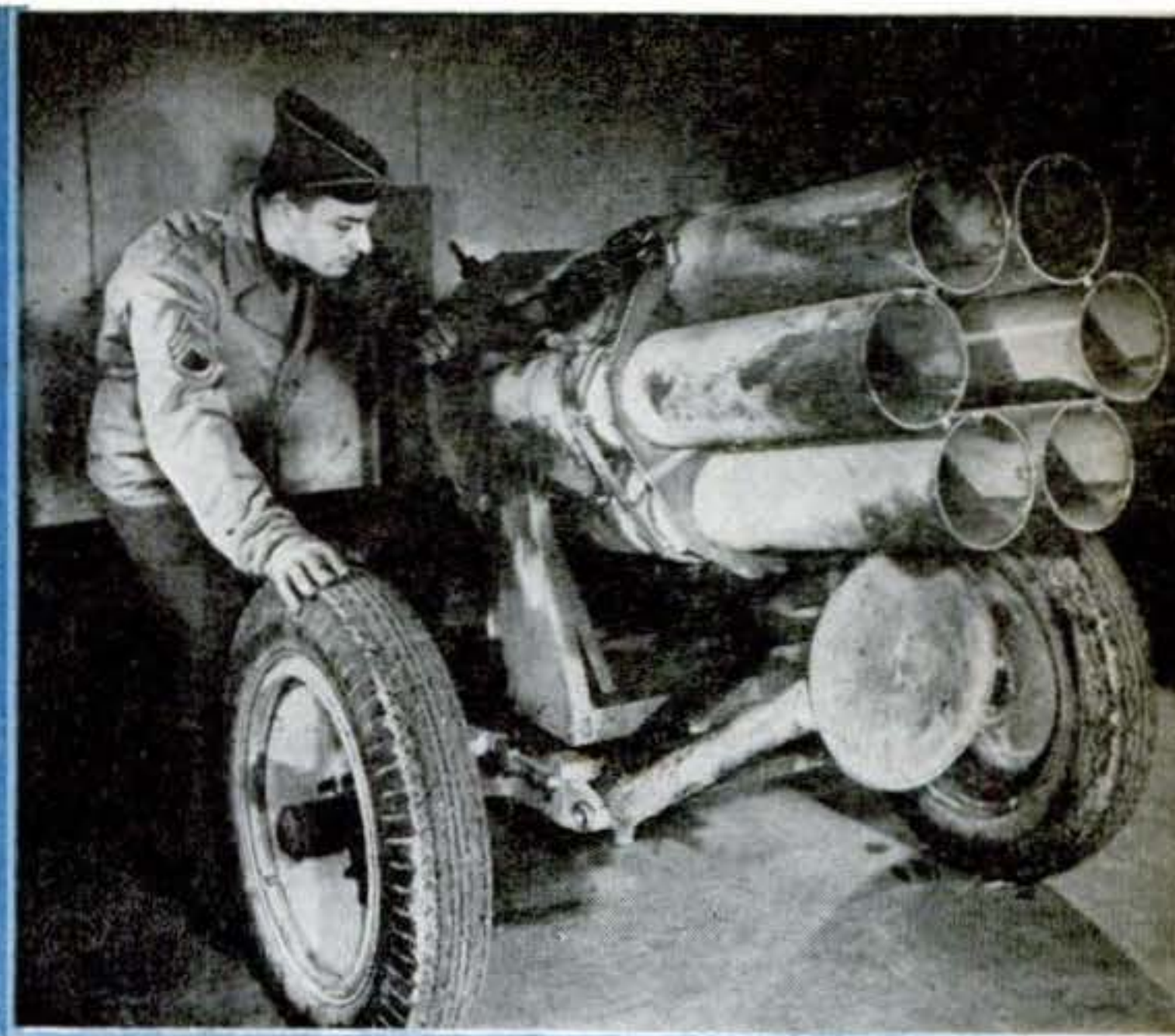
MULTIPLE ROCKET GUN as used by Germans. A 150-mm. mortar, it is electrically operated and fires explosive shells, smoke shells, and chemical rockets. Six rounds of 77-pound rockets are discharged in 90 seconds. Highly mobile, it's the "Nebelwerfer-41"
