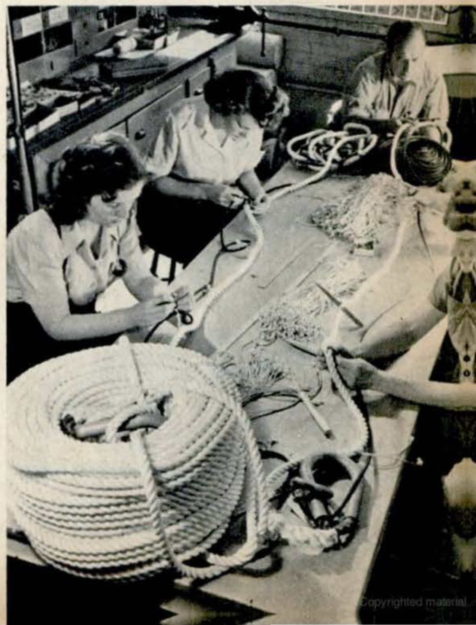
TOWROPE is fitted with a telephone cable through which the glider pilot can talk with the skipper of the towing plane. Cords bind the cable to towrope
