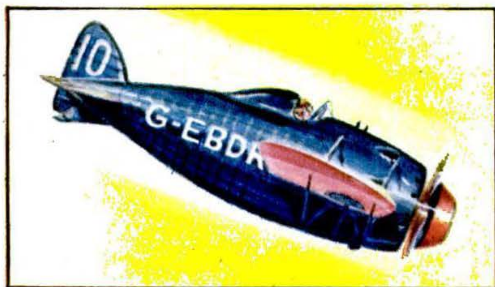
A midwing monoplane with retractable landing gear was conceived by the designer as far back as 20 years ago
