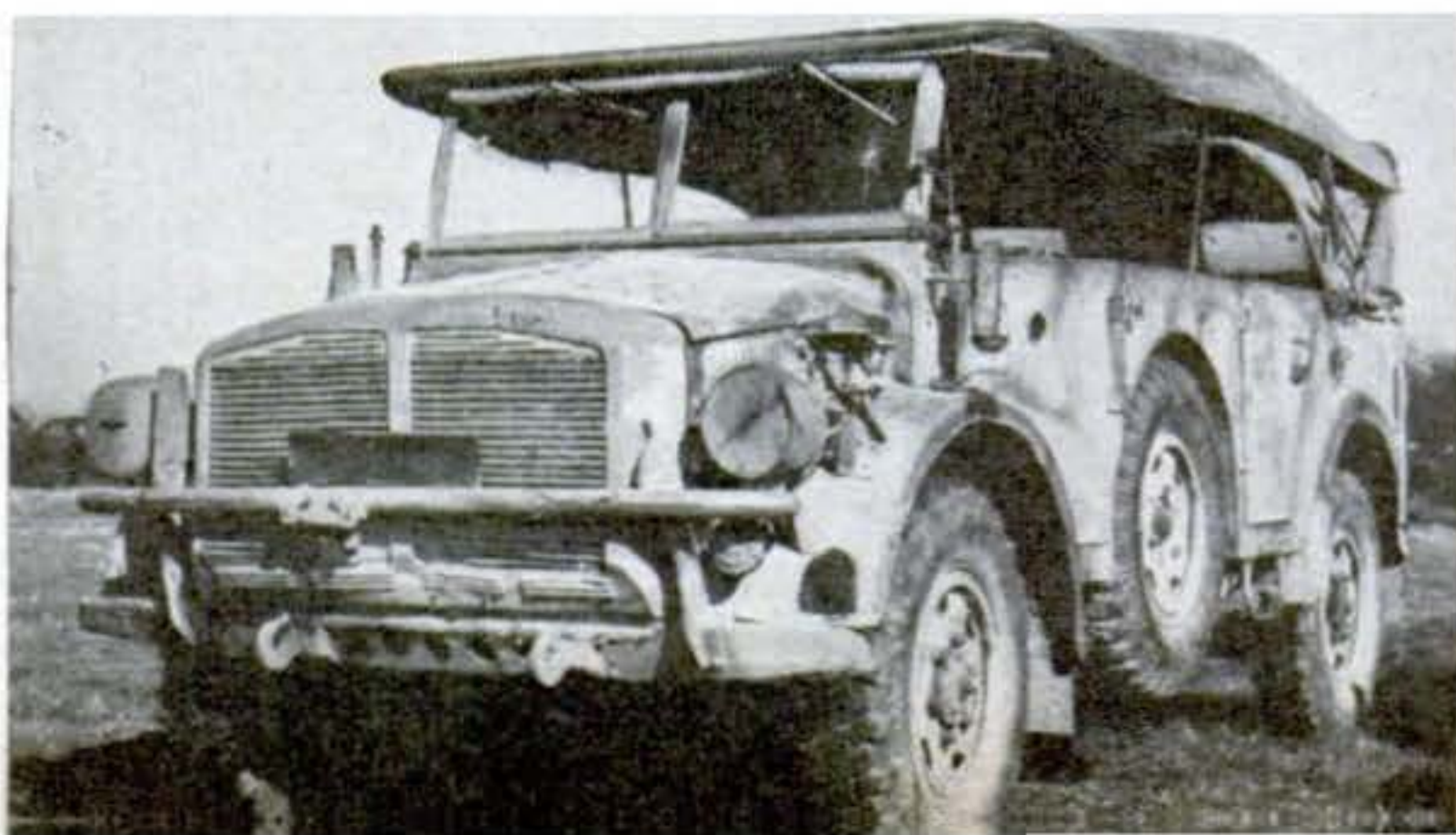
RECONNAISSANCE CAR —and it's not bad, either. This German vehicle, of 1½ tons, has speed, power, and low silhouette. Spare wheels, affixed to the center axle, give support on deep-rutted roads. Not armored
