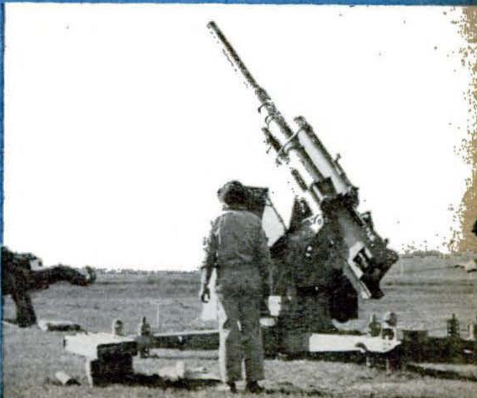
FIRING A GERMAN 88-MM. GUN at the Aberdeen Proving Ground. We don't use a three-piece barrel with enlarged chamber of this type because it is too dangerous for the gun crew. The Germans may be short of equipment for tooling full-length barrels
