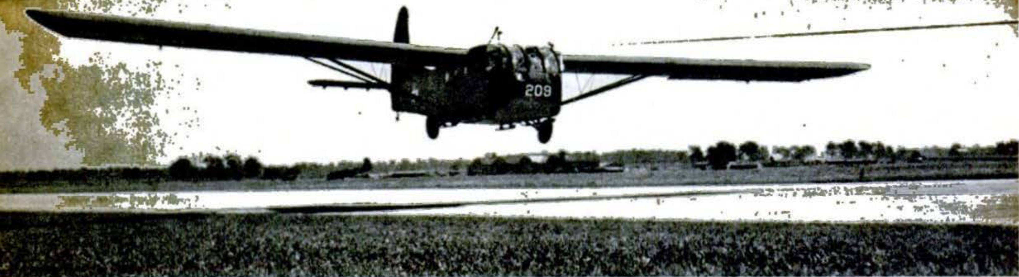
ARMY'S STANDARD troop and cargo-carrying glider is the CG-4A, seen here taking off behind its nylon towrope. Fifteen men, or an equivalent load in equipment, ammunition, and supplies, can ride it to a landing behind the enemy's lines. With its 84-foot wing span and 48-foot length, the CG-4A is not a simple craft to build, as the following photographs show
