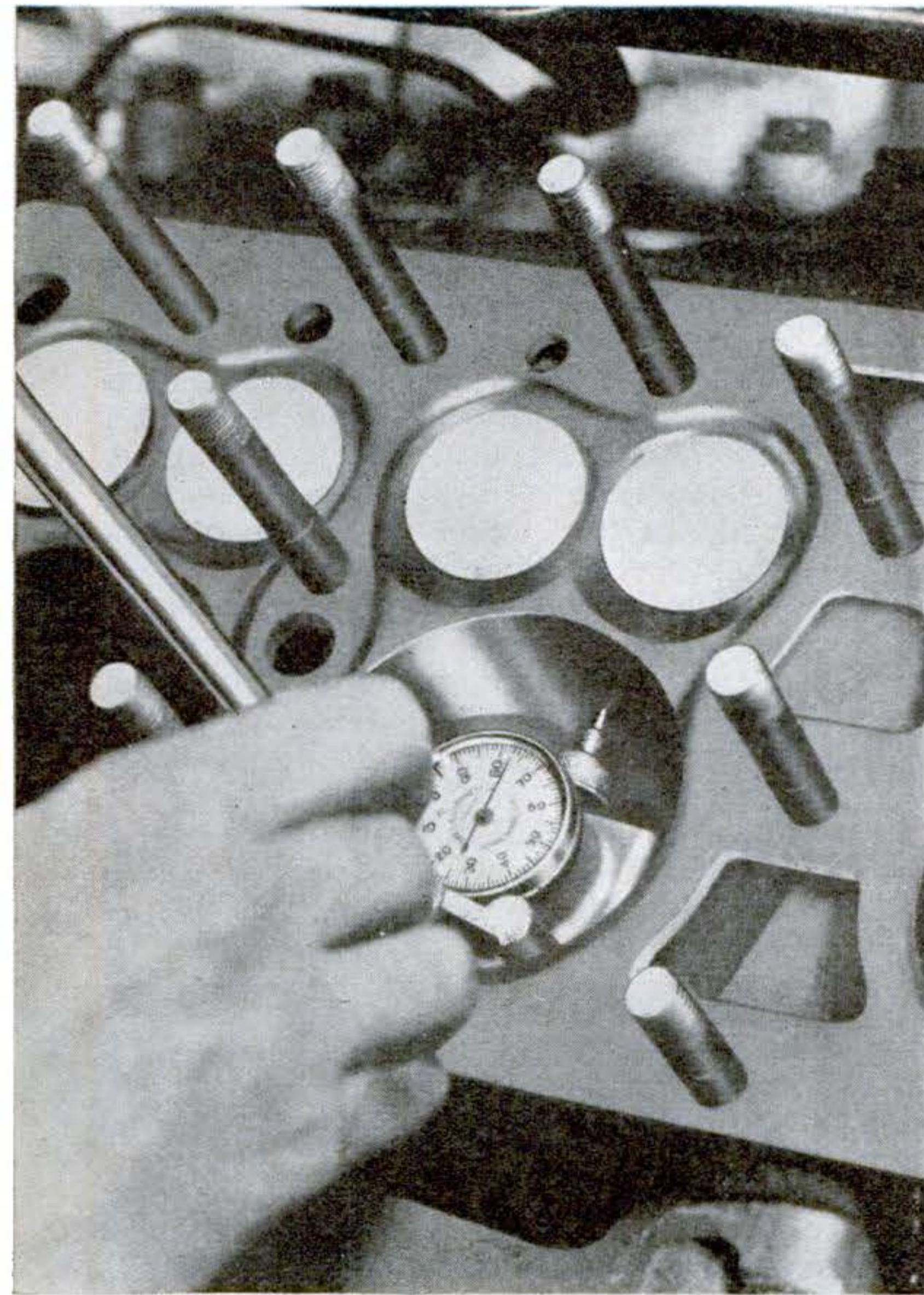
CHECKING THE CYLINDER BORE will show whether honing is advisable. Here a dial gauge is used. Right, a typical piston with its parts named
