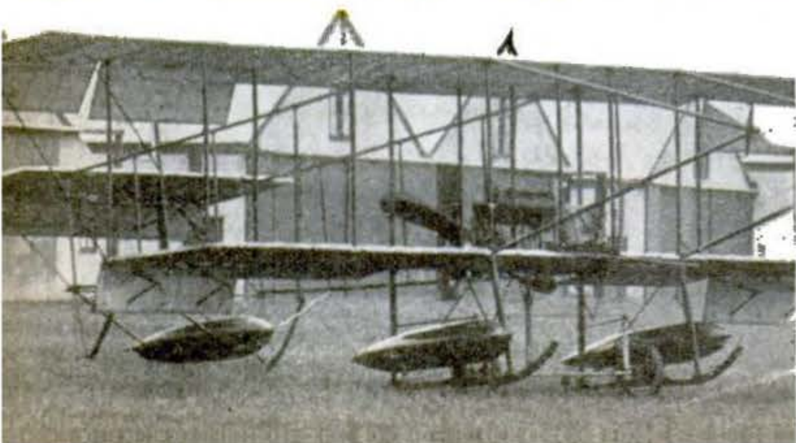
ALL-PURPOSE operation seemed to be the idea of the designer of this early plane—or else he just couldn't make up his mind. It had everything: wheels, pontoons, and skids
