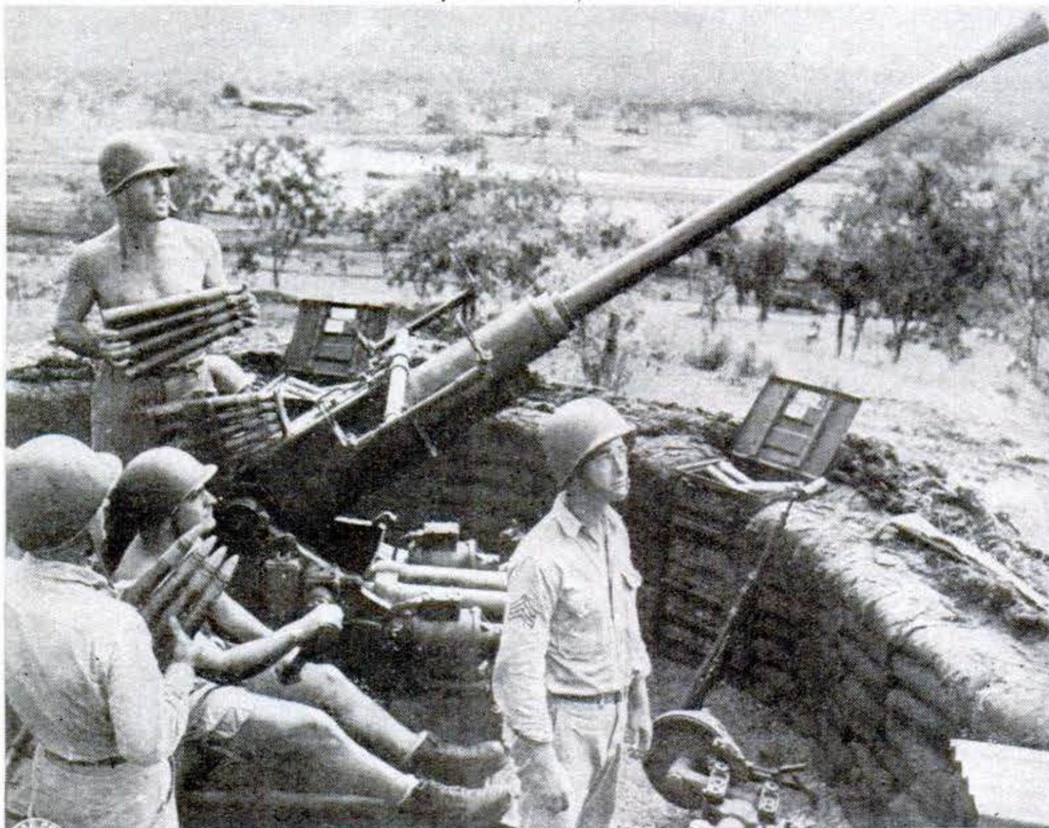
ARMY VERSION of the Bofors, seen here set for action in New Guinea, is different in a few details from the type used by the Navy. It has done a swell job in defending our land forces from aerial attack. Characteristic of the Bofors, on land or sea, is the flaring flash hider on the muzzle. This keeps gunners from being blinded
