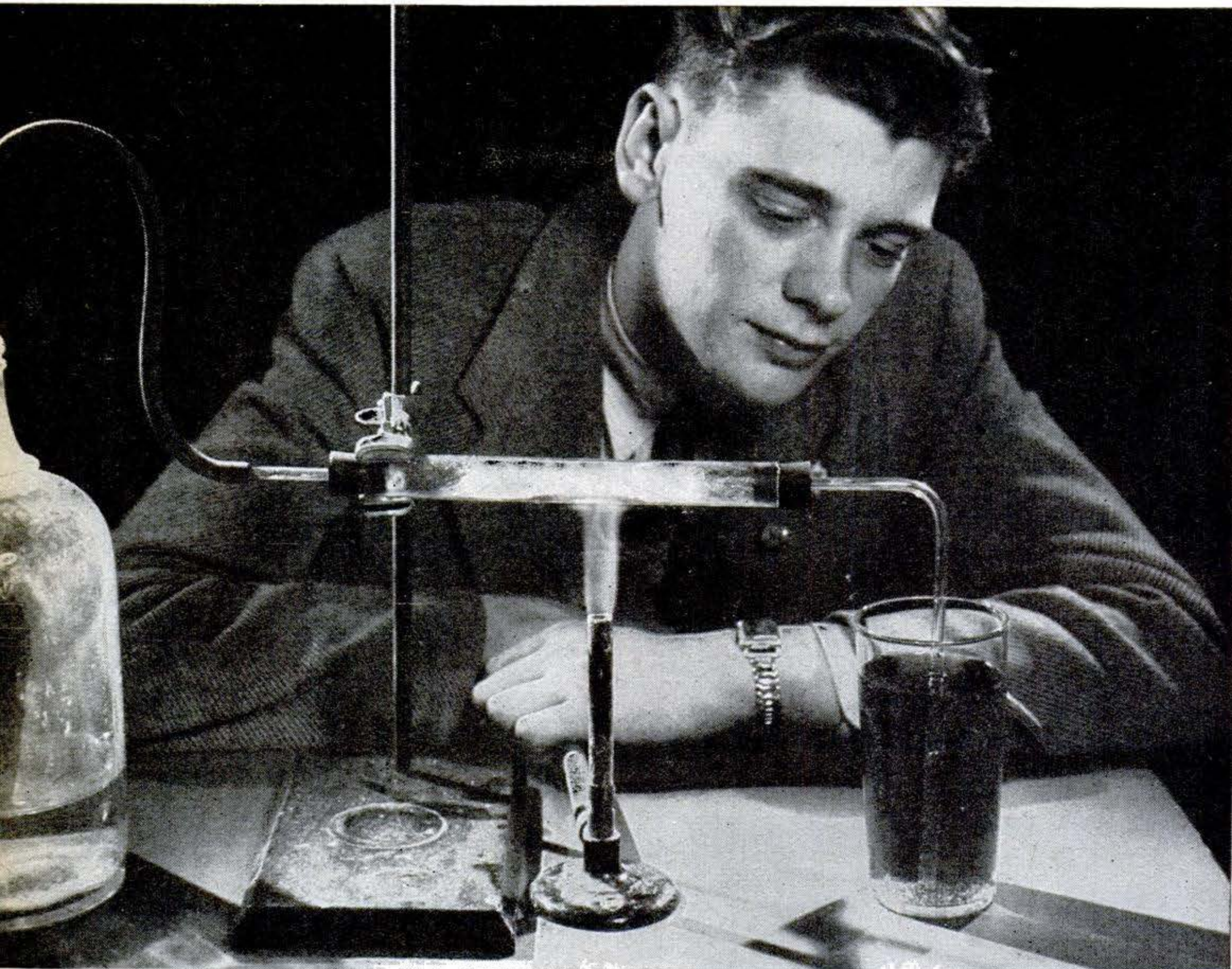
Cinnabar heated in the horizontal tube in this setup decomposes into metallic mercury and sulphur dioxide, the latter escaping as a gas
