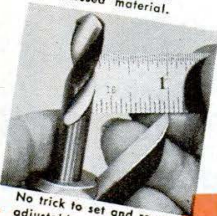
Cut deep holes in wood or compressed material.
