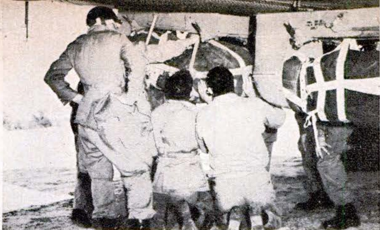
3 Here a bundle is being placed in its rack. There are six racks on the plane. The three remaining bundles are stacked at the door of the ship, ready to be thrown out just before the crew hits the silk
