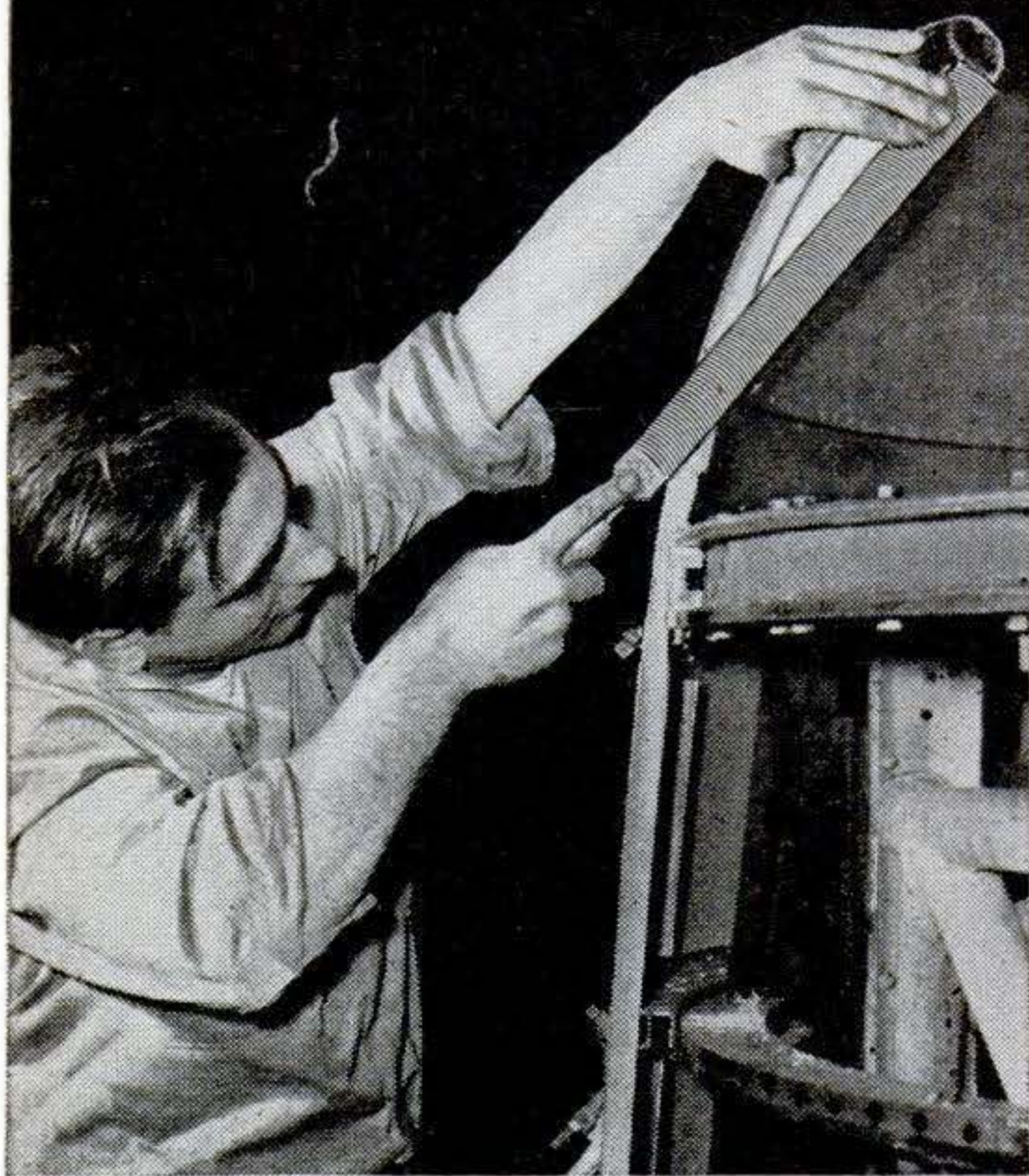
Photo courtesy Republic Aviation Corp.— Special-file operation on edge of cowling.
