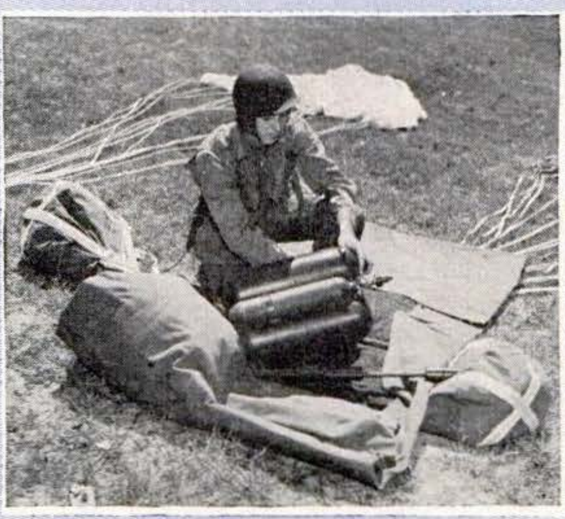
Here one flame thrower has been removed from the roll, while the other remains inside. Note the felt padding on the inside of the parapack. This protects the equipment from being damaged in landing
