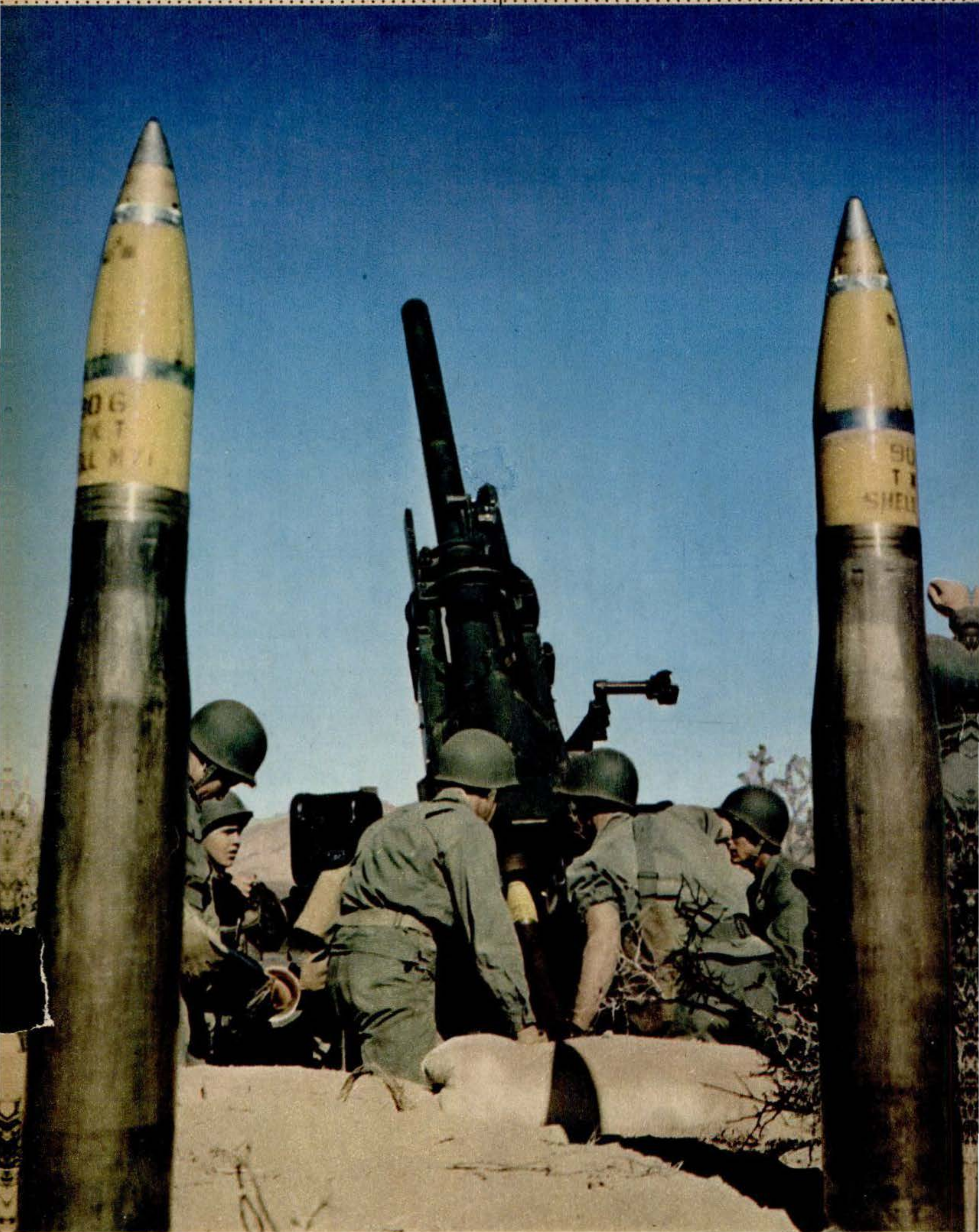
As nearly automatic, in spite of its weight and caliber, as human ingenuity and electrical research can make it, this 90-millimeter plane-killer stands framed between two of its own shells. Standard equipment for the armed forces, this weapon has attained an almost incredible effectiveness. Its 15-foot barrel can be wound down to five degrees below the horizontal for use against armor
