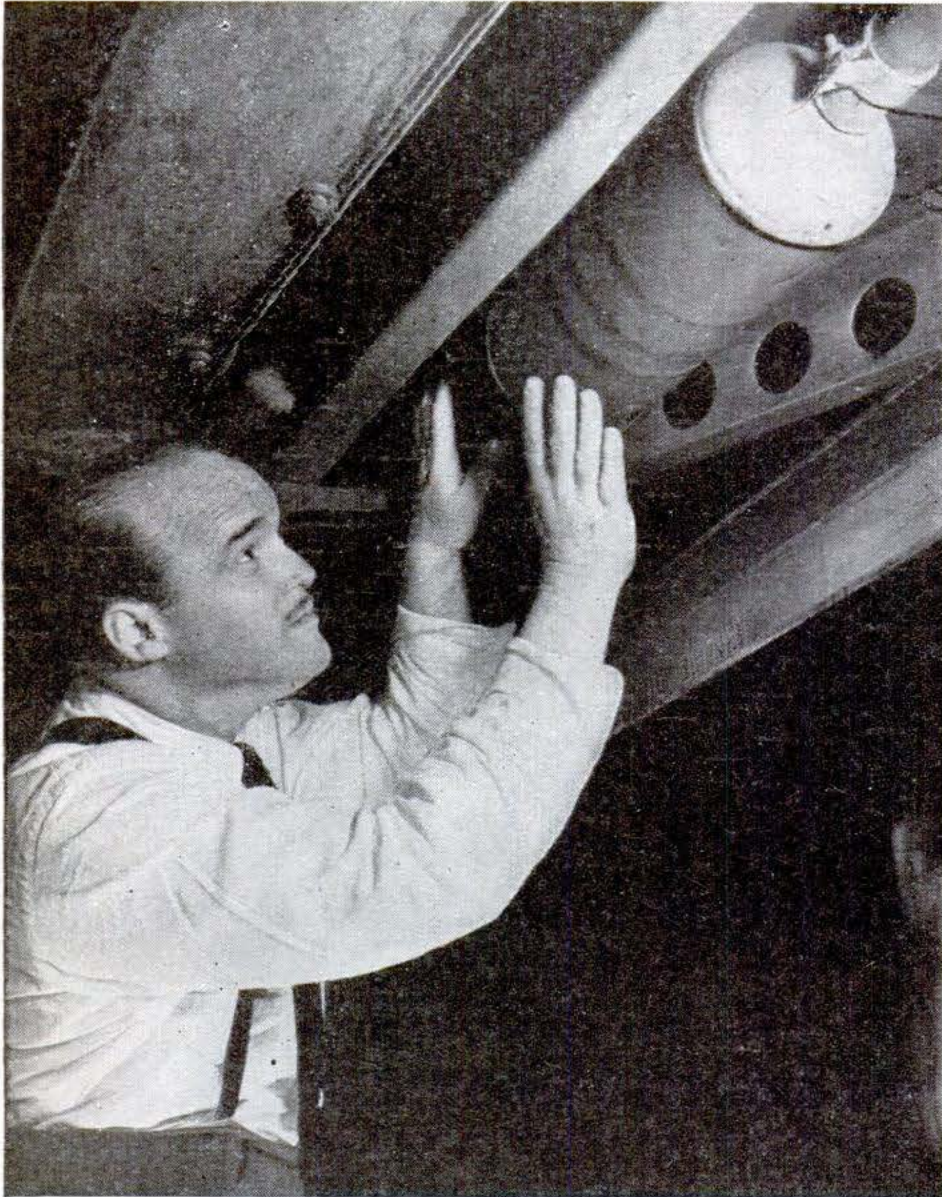
When your car is next on a grease rack, inspect the exhaust system carefully—its failure can ruin your engine or even take your life
