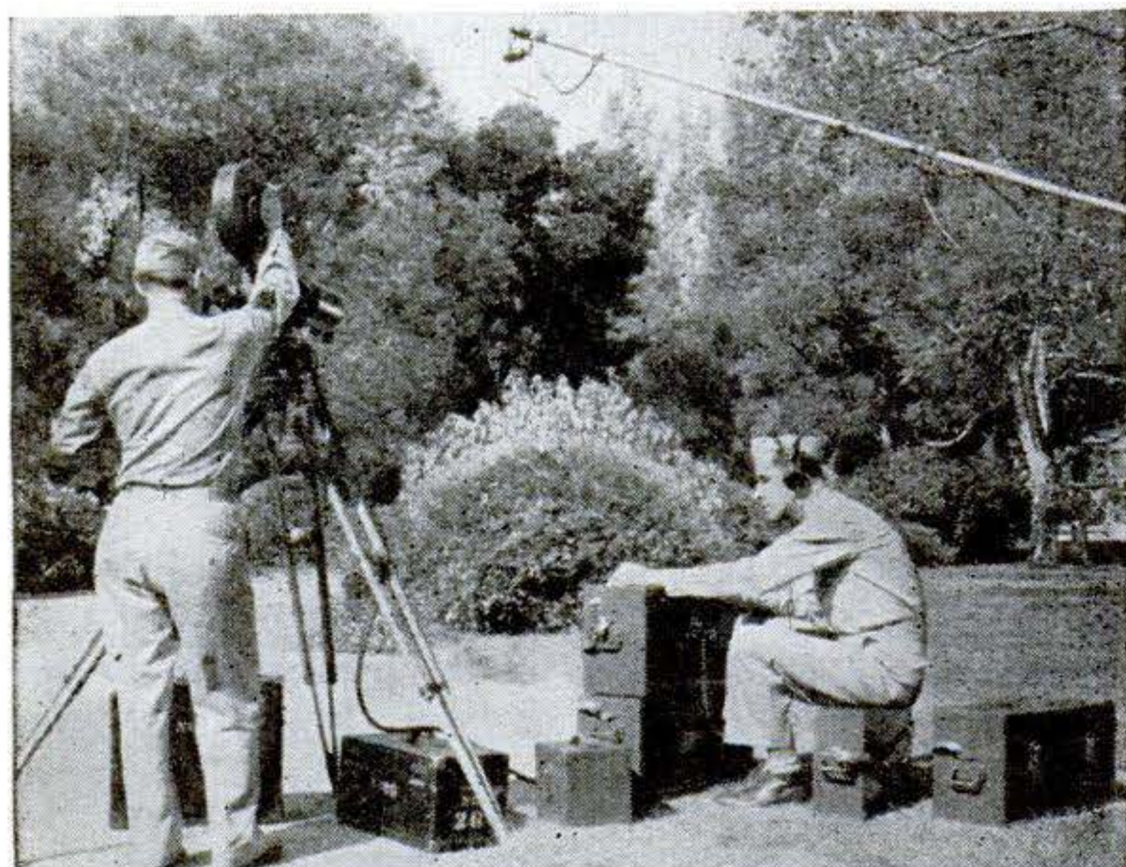
With portable equipment in half a dozen cases, Army cameramen can record battle and other sounds in synchronization with their front-line movies
