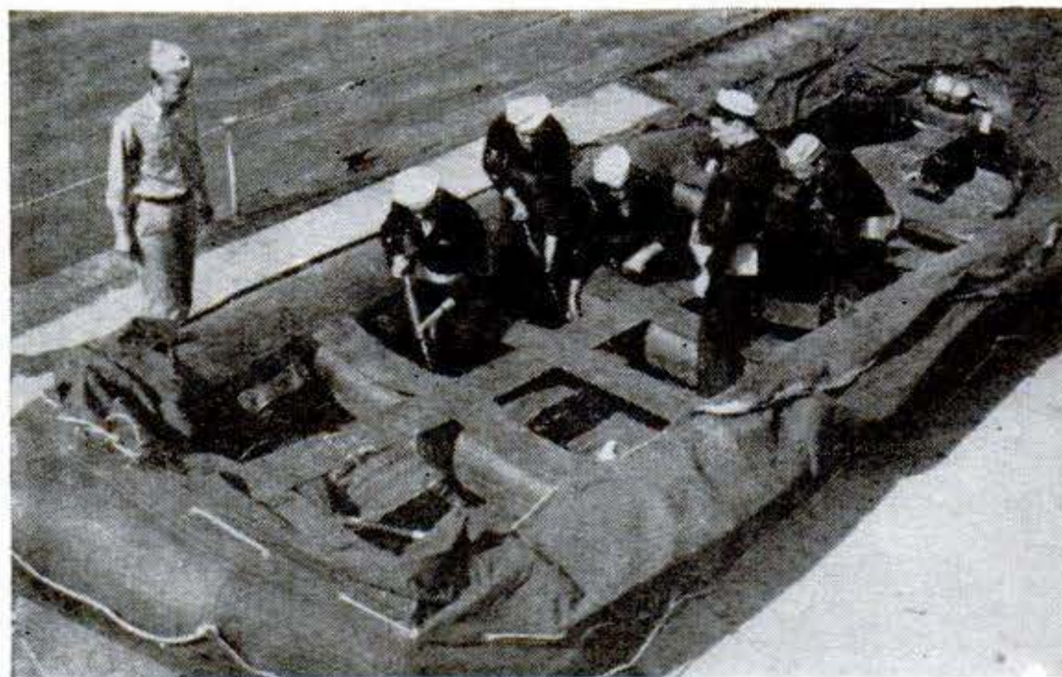
The cross tubes shown provide lateral stability, and bulkheads in the buoyancy tubes insure safety
