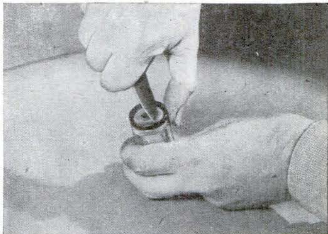
When lens elements are being taken out of their mount, the rim may need spreading to release them
