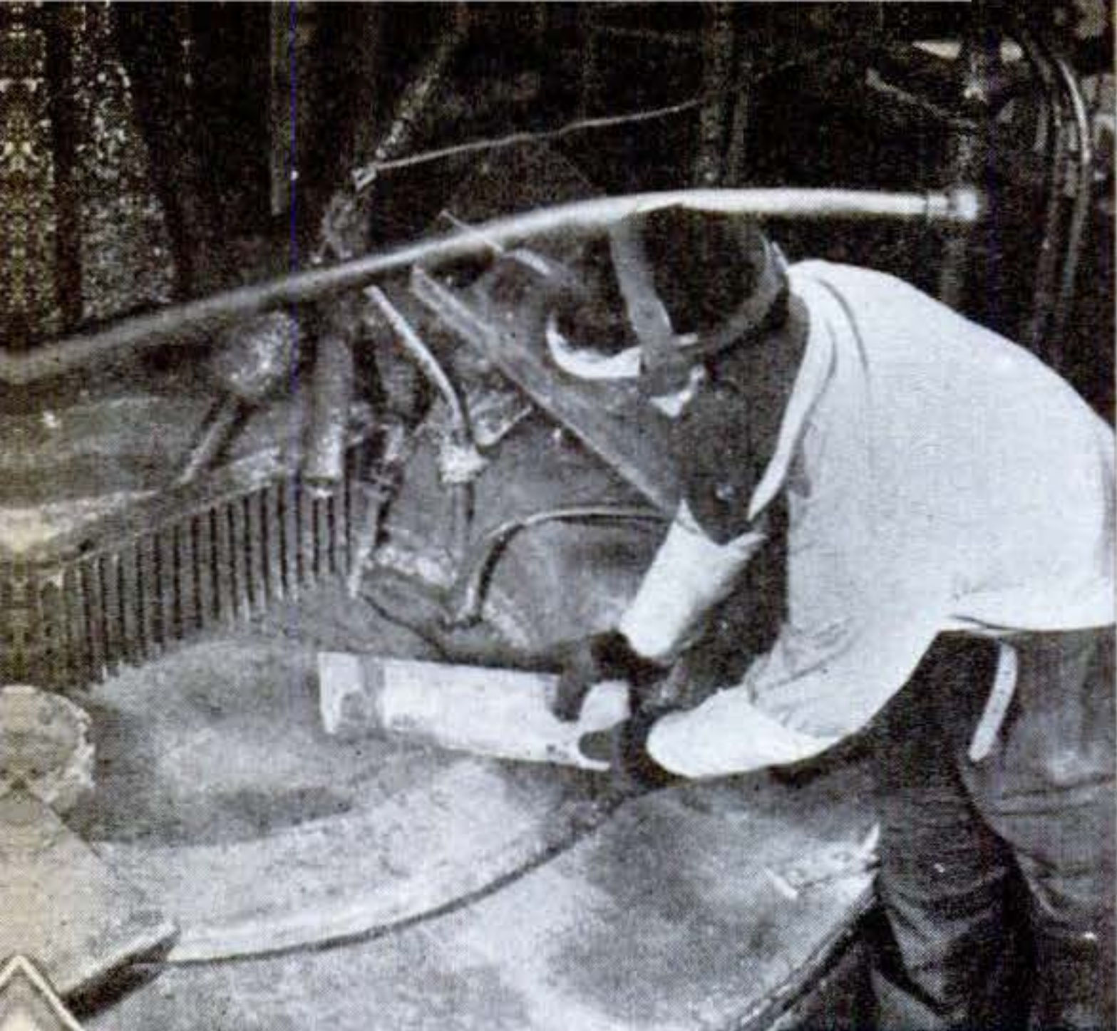
MELTING POT on ninth floor of the shot tower receives 98-pound pig of lead as one of the preliminary operations in the making of shot for shotguns
