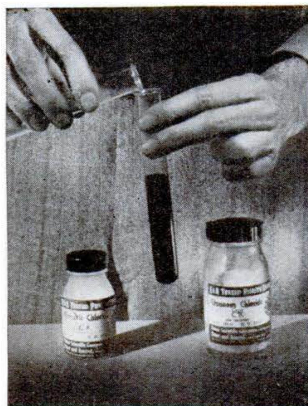
When stannous chloride is poured into a solution of mercuric chloride, first white mercurous chloride (calomel) is precipitated, as at left, since the tin chloride steals chlorine from mercuric chloride
