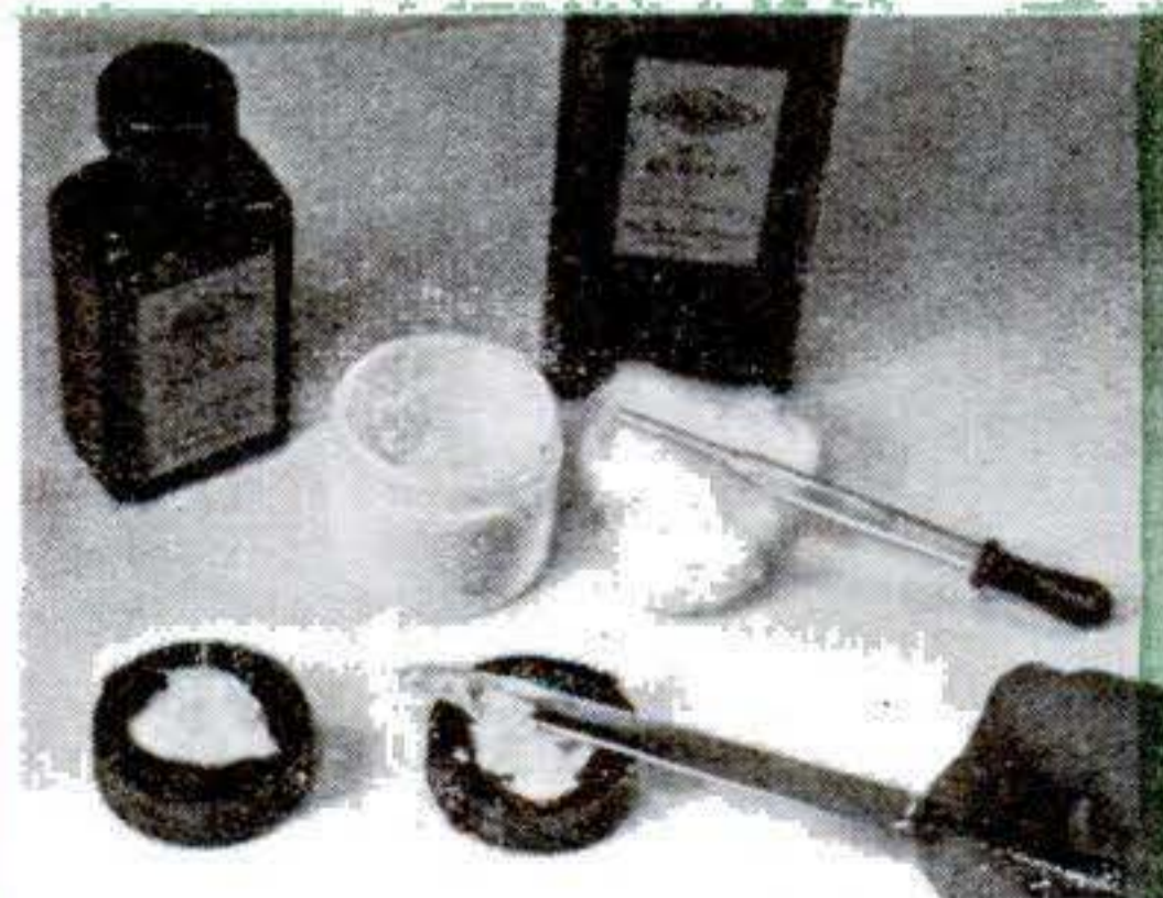
Freshly mixed plastic packed in both halves of the mold should be more than enough to fill them
