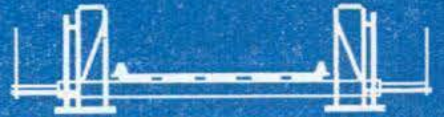
TRIPLE TRUSS—SINGLE STORY
