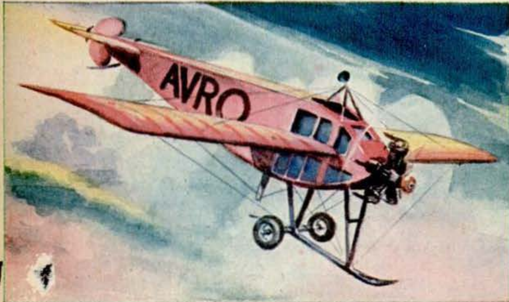
1912 Three years later, this test cabin monoplane was powered by a radial engine and had new wing mounting
