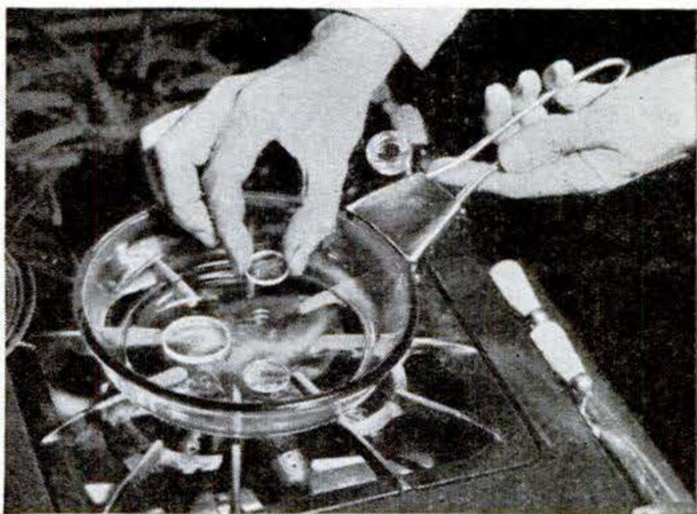
Old cement is removed with xylol or some other solvent (above), and the elements are cleaned, matched, and heated, with balsam melted on the concave lens, shown held in the fingers below
