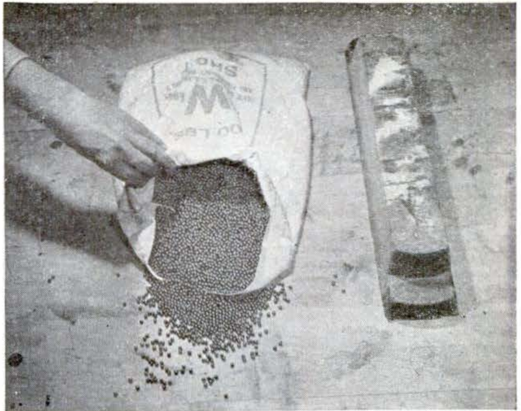
FINISHED SHOT are packed in comparatively small bags of 100 pounds' capacity. Compare the size with that of 98-pound pig of lead shown at right. Such a bag will hold somewhat more than 350,000 individual No. 6 shotgun pellets
