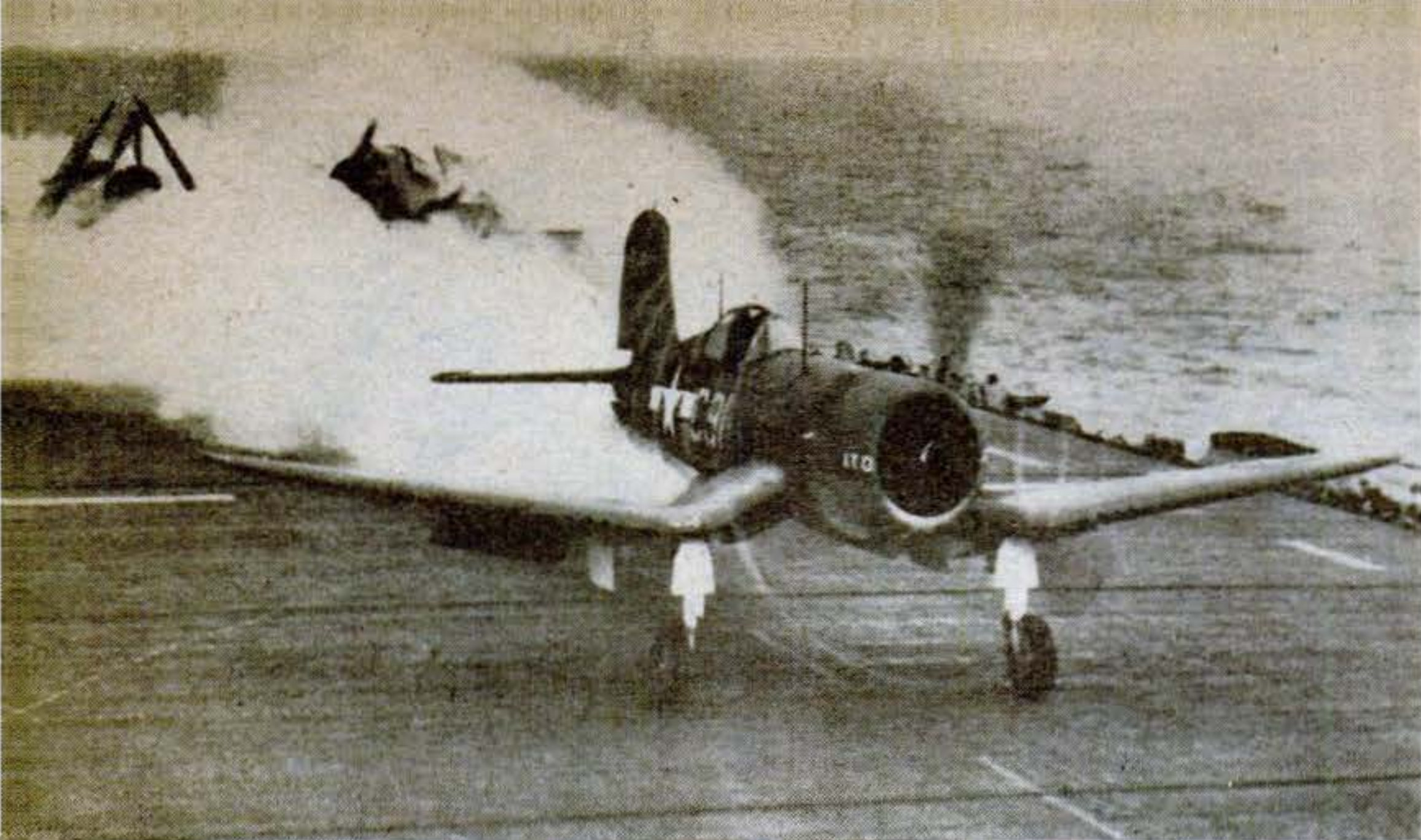
Navy Corsair, extra-powered with two rockets, hot-foots it down the deck of a plane carrier for a take-off. Each rocket gives an extra 330 horsepower
