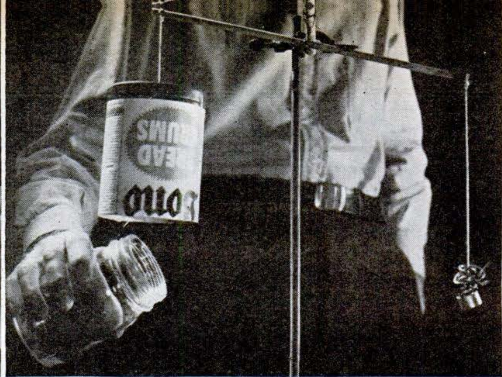
Poured upward from a jar into a container balanced on a beam, hydrogen demonstrates its buoyance by lifting that side of the balance. It is the lightest of gases
