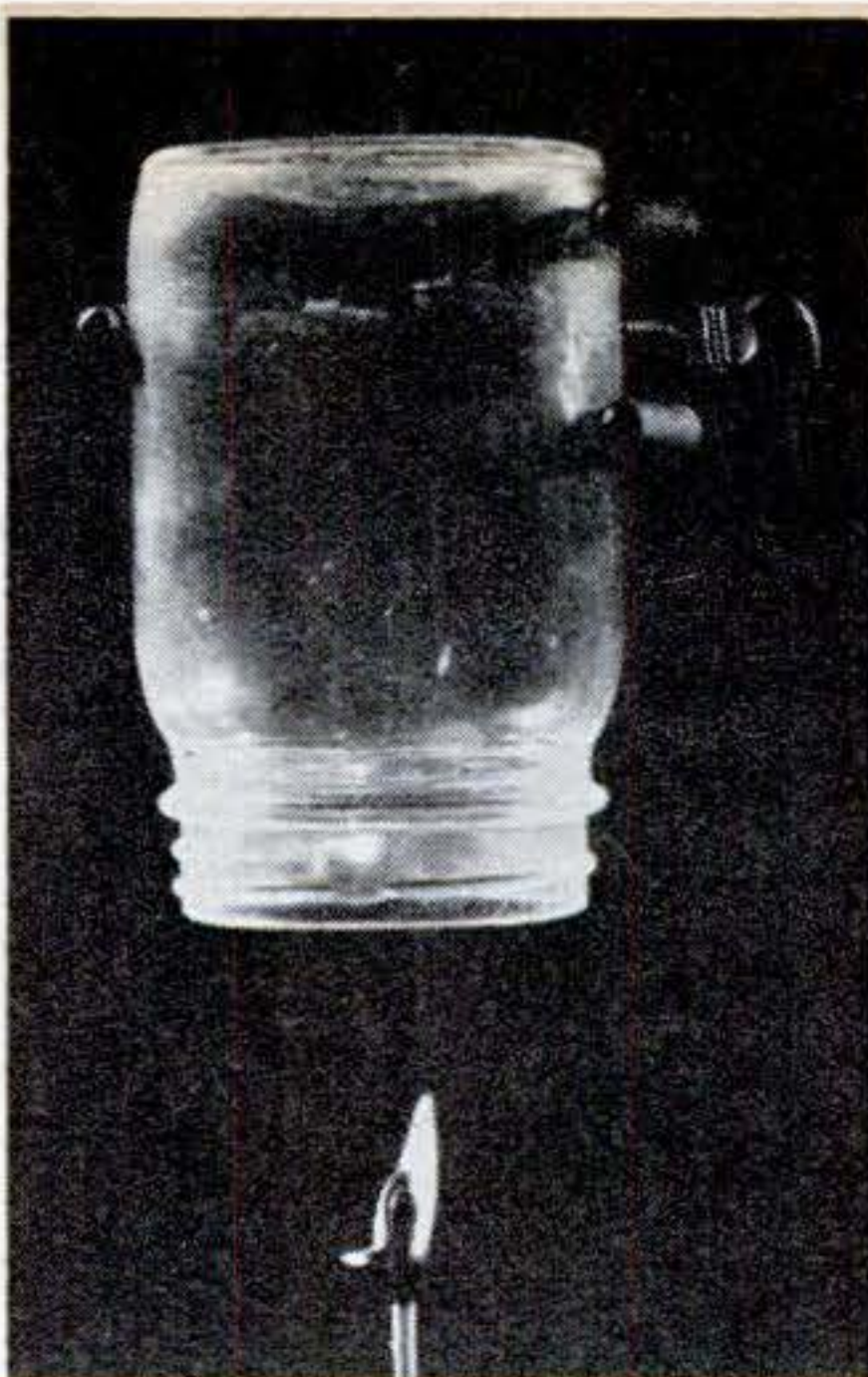
Bring a lighted match up to a jar containing hydrogen, and the gas will ignite . . .
