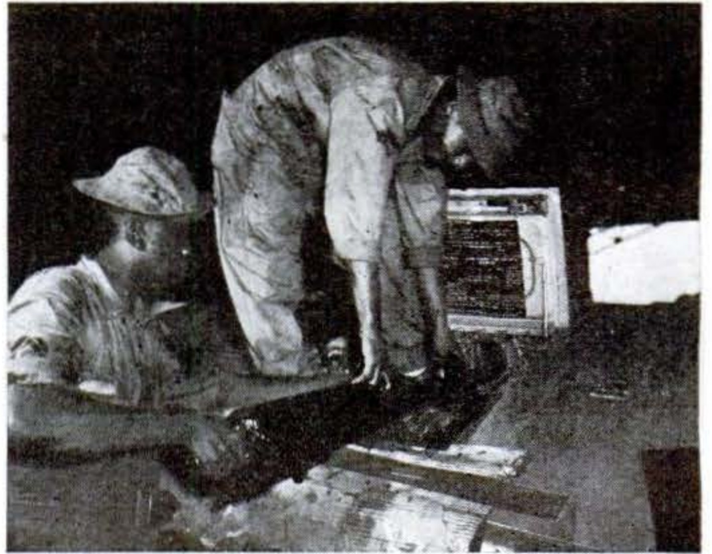
4 Guns come out of the wings, are given a heavy coat of rust-preventing oil, then reinstalled. Eight different oils are used to protect the ship
