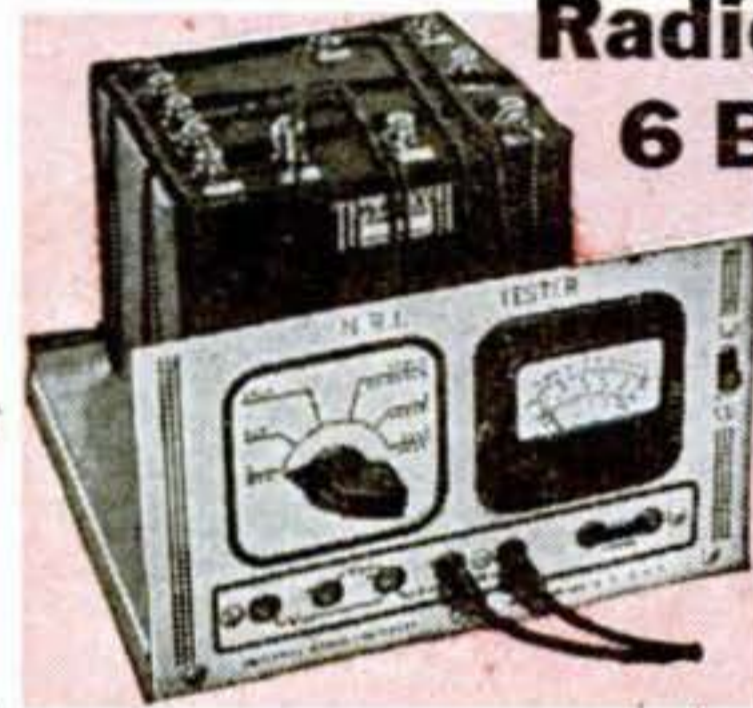
MEASURING INSTRUMENT (above) you build early in Course. Use it in practical Radio work to make EXTRA money. Vacuum tube multimeter, measures A.C., D.C. and R.F. volts, D.C. currents, resistance, receiver output.
