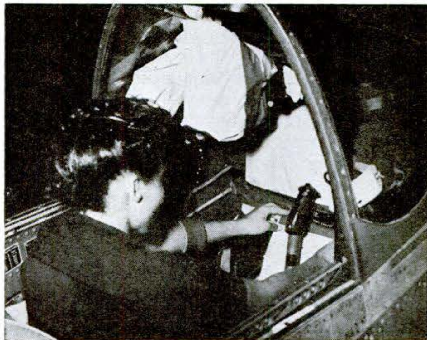
6 Instruments are not removed from the ship but are wrapped in oilcloth; tightly taped. Silica-gel bag is hung in cockpit, which is then sealed
