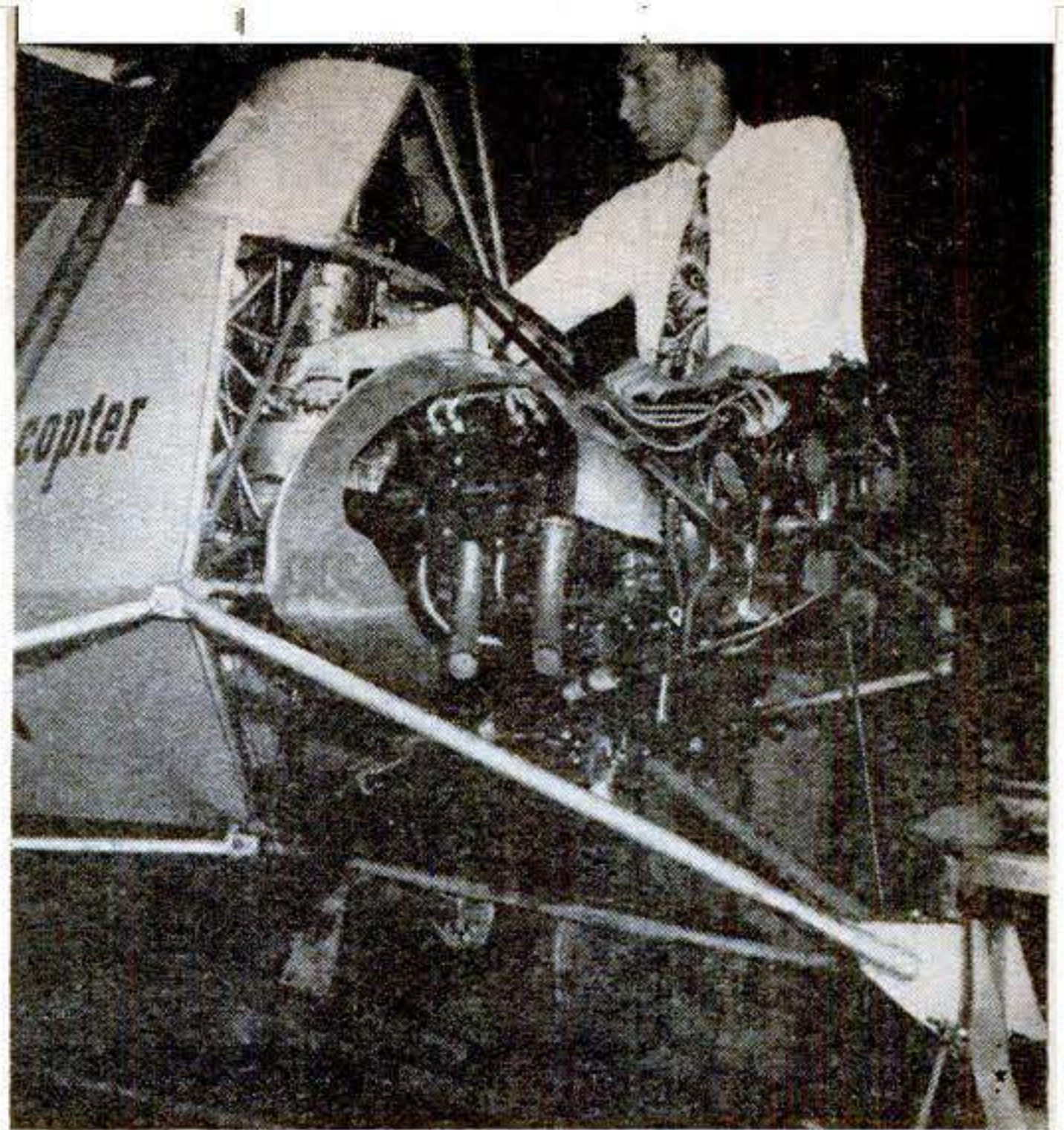
Schematic drawing of the "heart" of the ship. The 90-hp. engine spins the rotors at an almost constant r.p.m. of 240, to produce speeds (controlled by blade pitch) up to 90 m.p.h. At right, Hiller inspects engine, which is mounted in the tail instead of under rotor mast, as in more familiar 'copters
