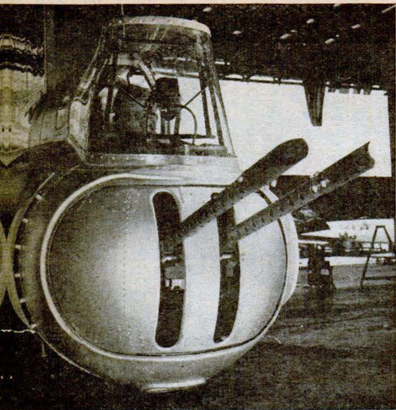
STING IN THE TAIL end of the Boeing B-17 has been stepped up by this new swivel turret, which allows the twin .50 caliber machine guns to swing through a 90-degree arc, or 30 degrees more than formerly. New turret allows 50 percent more firepower than the old. An all-around flak curtain and bulletproof glass protect the gunner.
