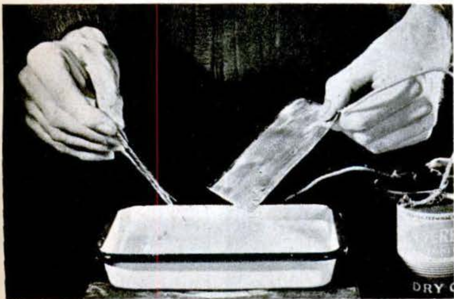
"Rainbow" coated with molybdenum, this copper plate shows only one of the unlimited number of brilliant color patterns that can be produced by moving the positive anode over the plate
