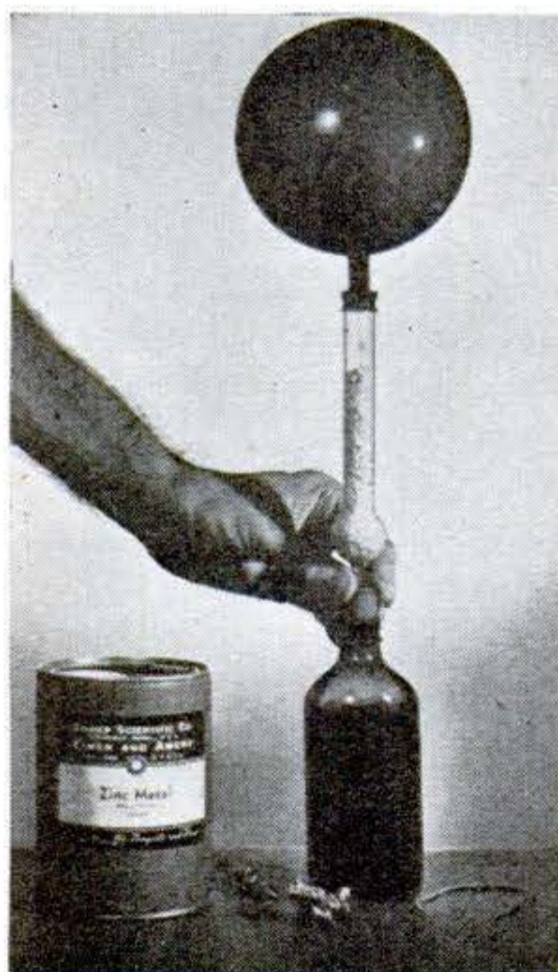
Toy balloons can be inflated from a bottle of dilute acid and zinc. Hydrogen is here passed through a drying tube
