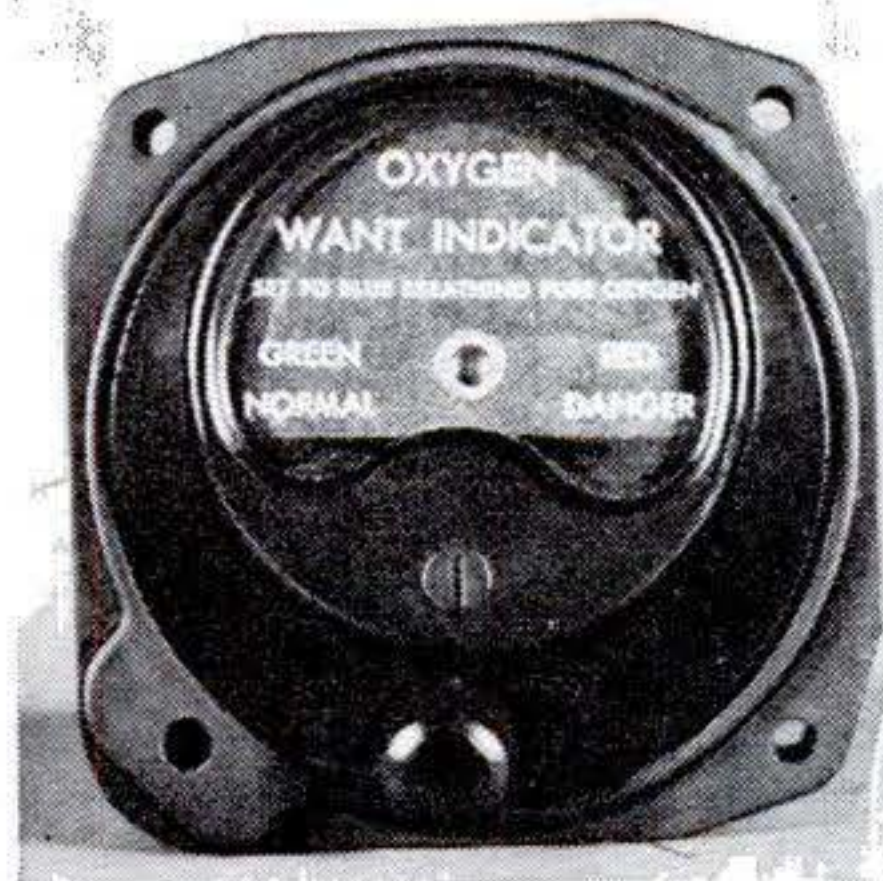
High-altitude flyers check oxygen need by this indicator connected with photoelectric earpiece signaling color of blood Photos from Air Force.
