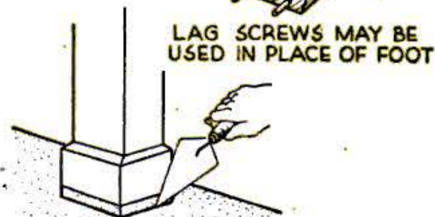
TROWEL CONCRETE MIX FLUSH WITH BASEBOARDS
