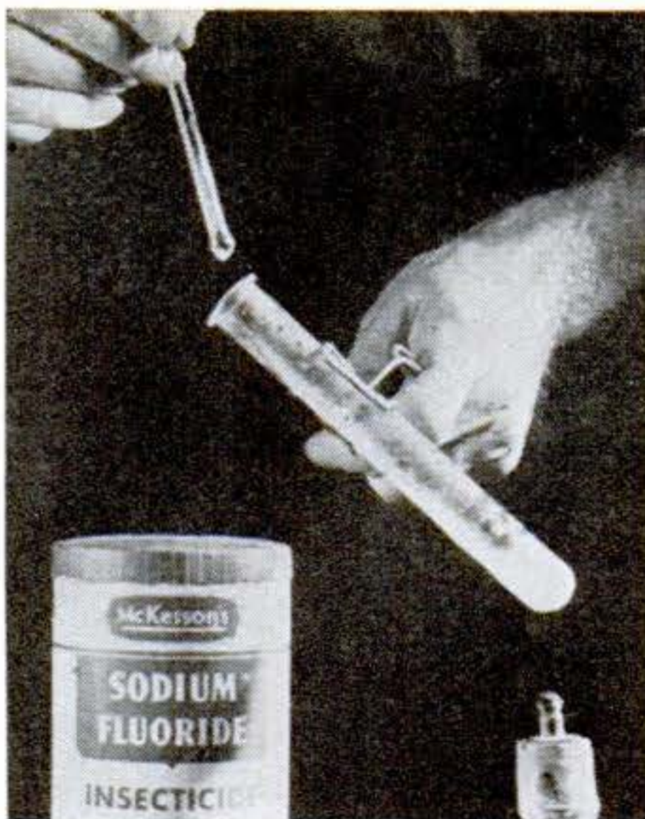
Fluorides heated with sulphuric acid and common sand give off a gas that turns a drop of water white by formation of silicic acid
