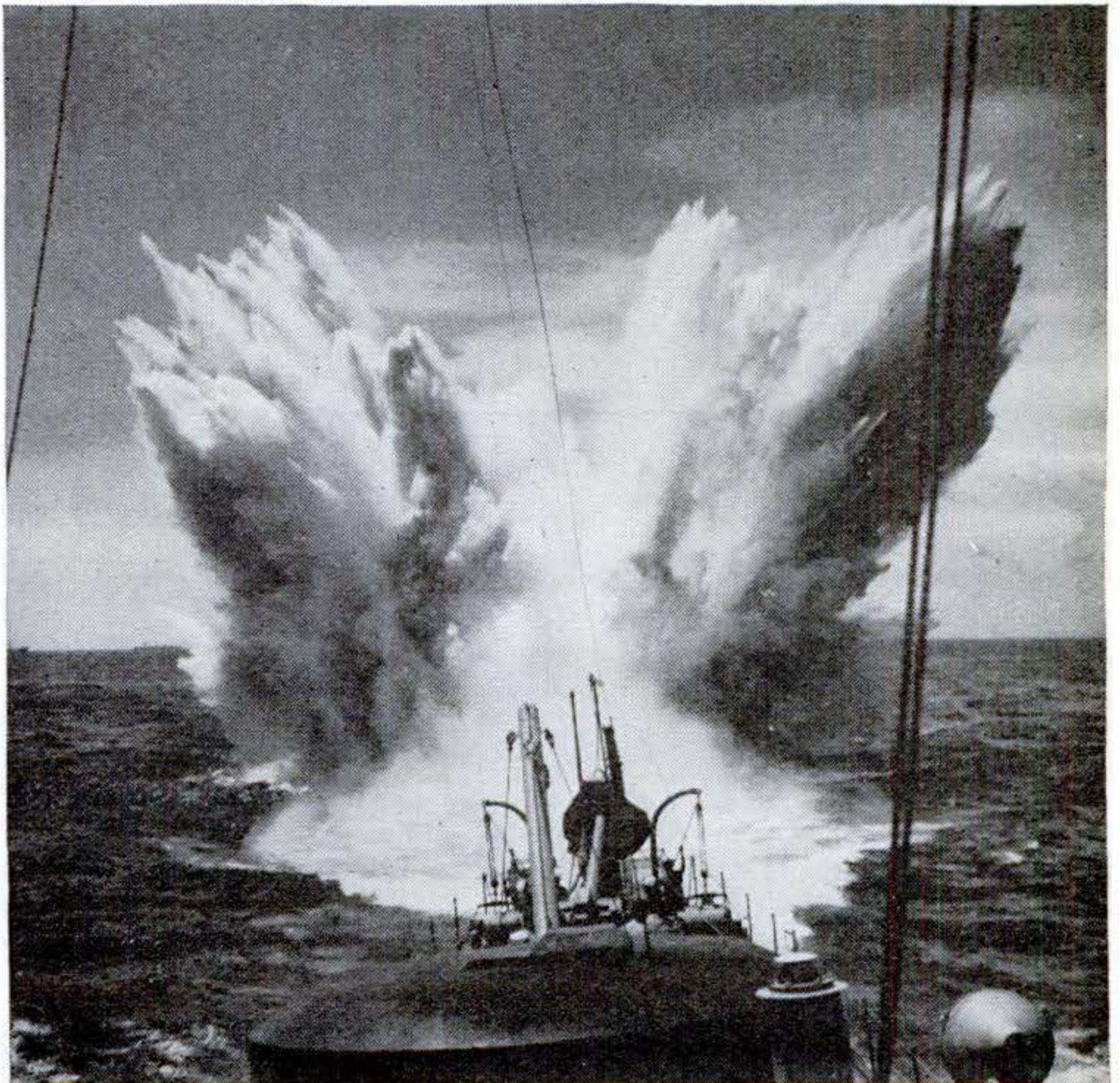
U. S. depth bombs have a bursting charge of TNT, come in 325- and 650-pound sizes, and have a fuse that can be set to detonate at any desired depth
