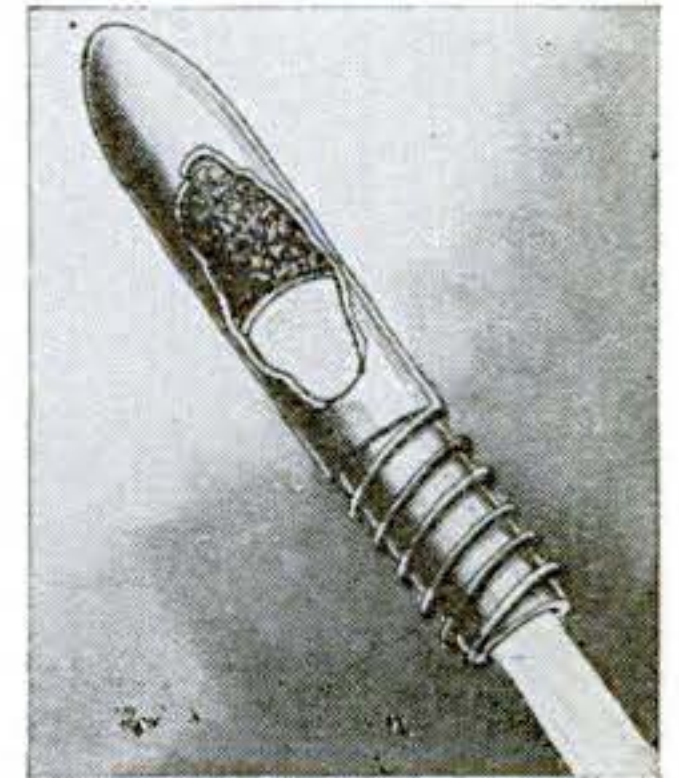
CONGREVE ROCKET, developed in early 19th century, had an explosive in its head, was fired from a tripod-mounted tube fitted with tangent sights. It was only moderately successful
