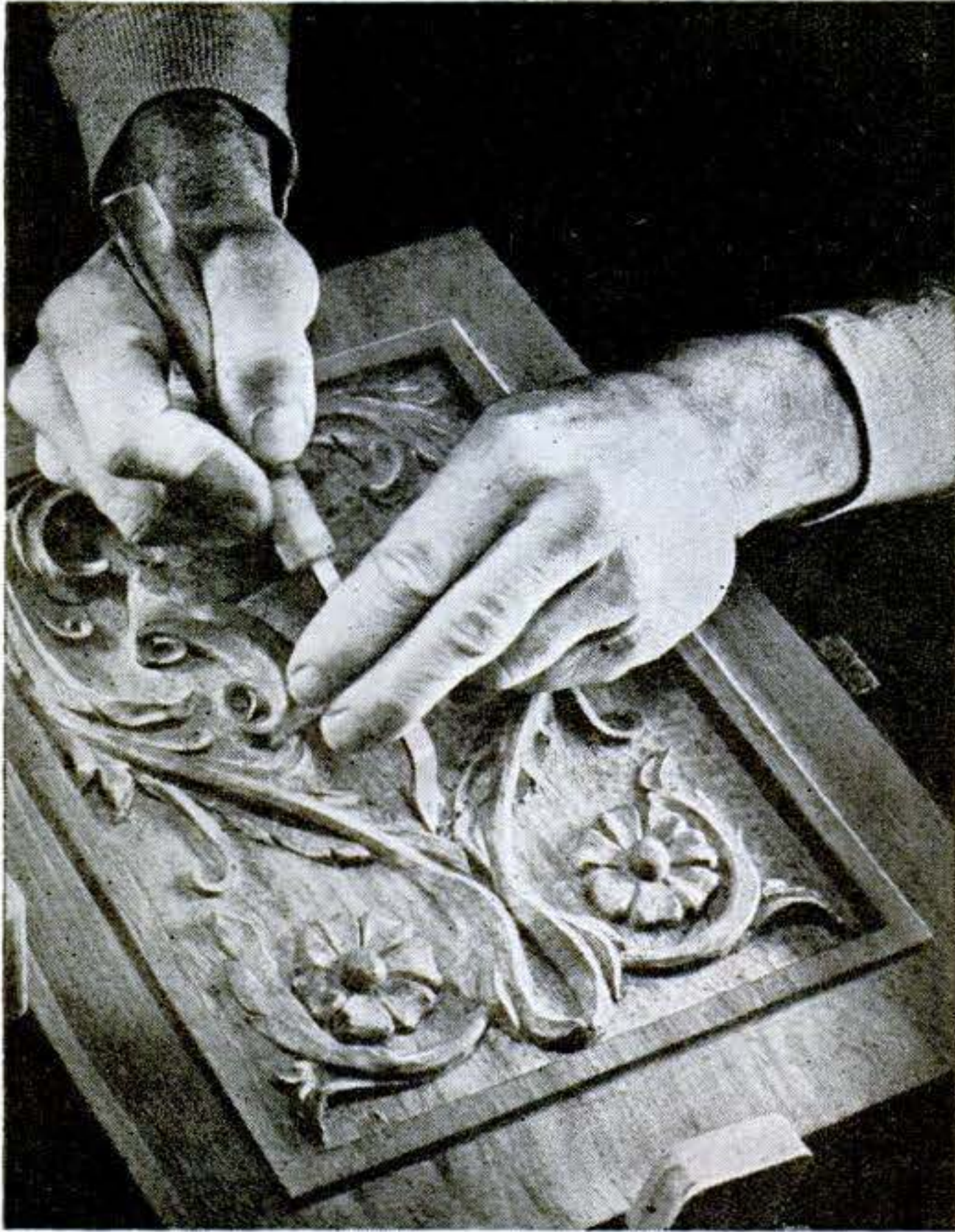
Above, a spoon skew is found handy for working in the corners while touching up the ground. Below, a wide butt chisel is used for straightening the border. The edge is rocked down from one corner.
