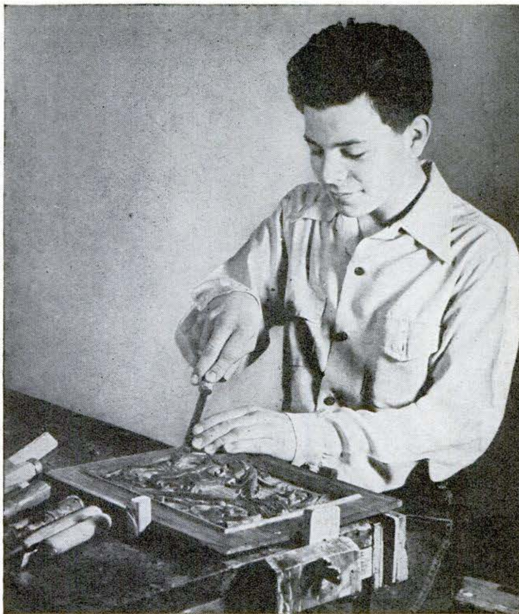
Shearing cuts with a flat chisel bevel the border of the panel, reducing apparent height so leaves may roll over it slightly.
