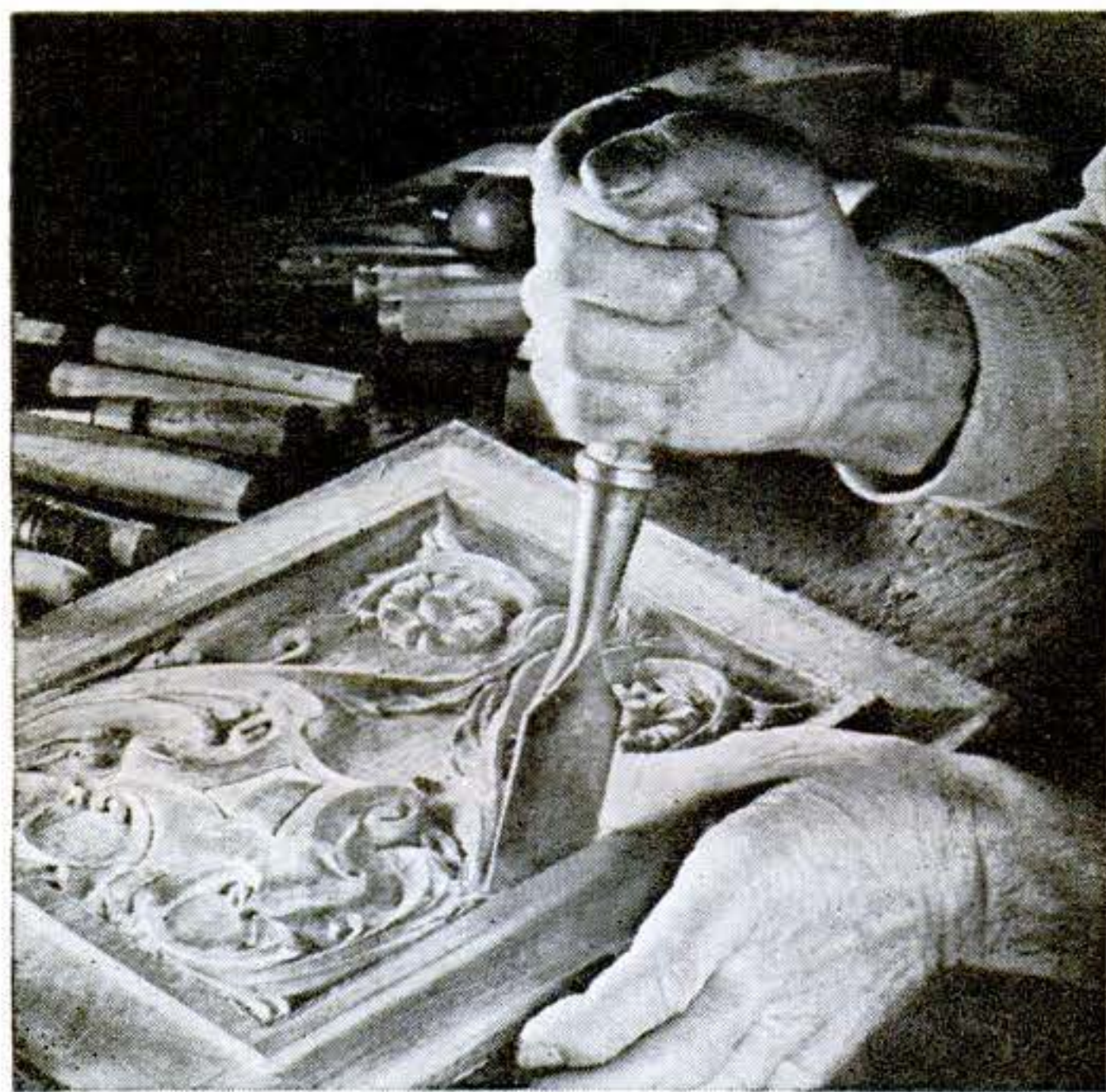
Above, a spoon skew is found handy for working in the corners while touching up the ground. Below, a wide butt chisel is used for straightening the border. The edge is rocked down from one corner.
