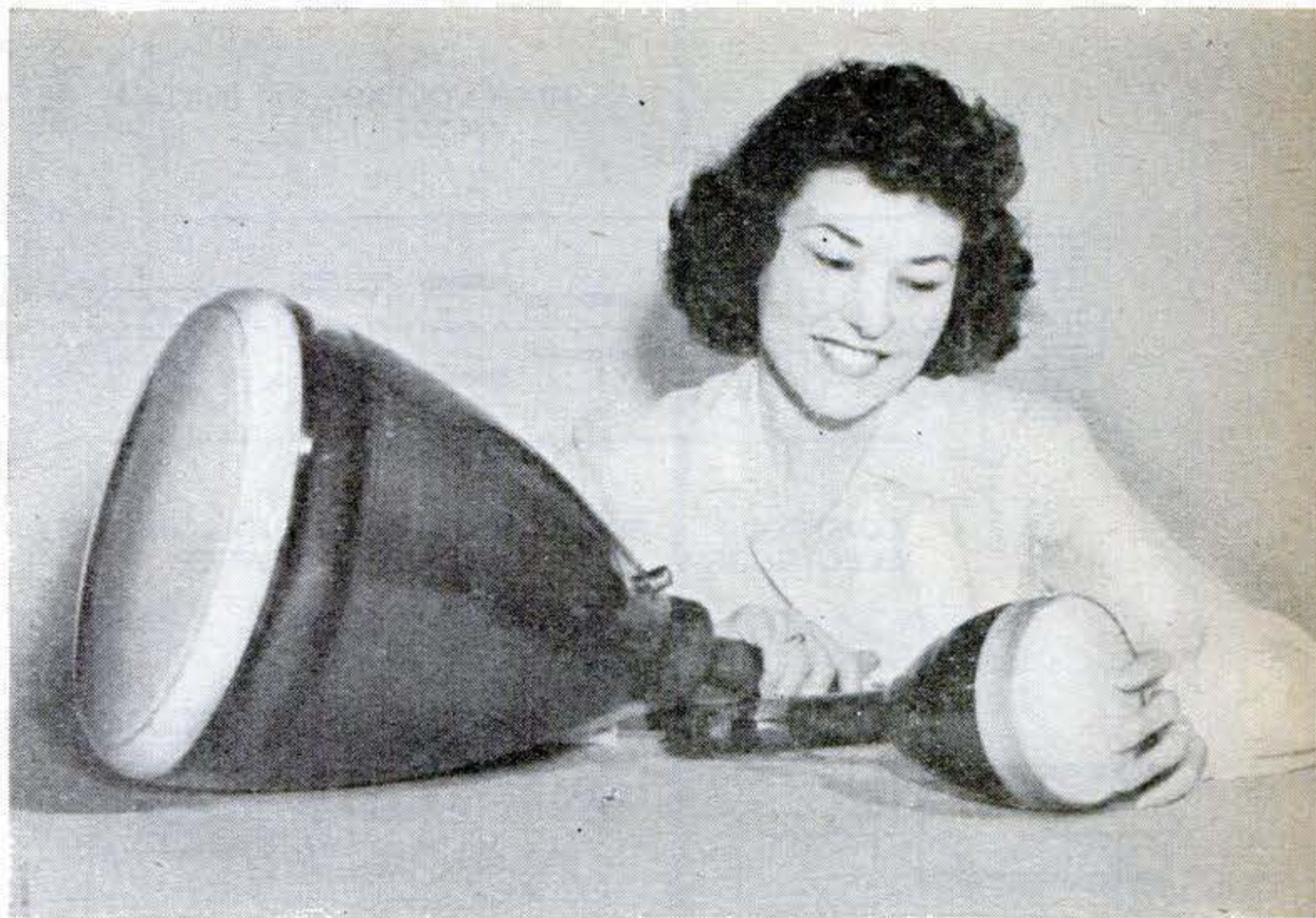
Size isn't everything in cathode-ray television tubes. RCA's postwar tube (right) is far brighter and more powerful than the prewar tube.
