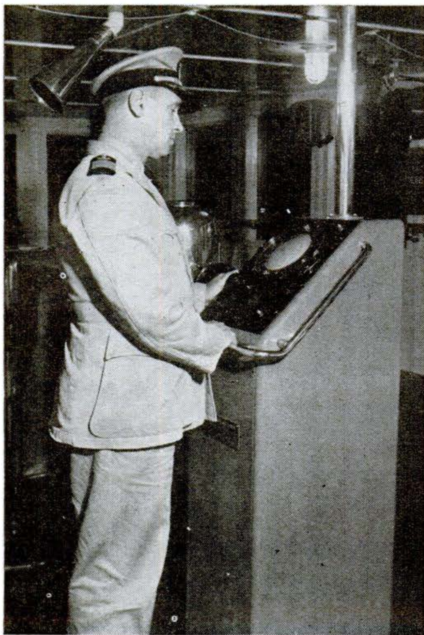
On ships, the "electronic navigator" will detect obstacles at distances up to 30 miles in any weather.
