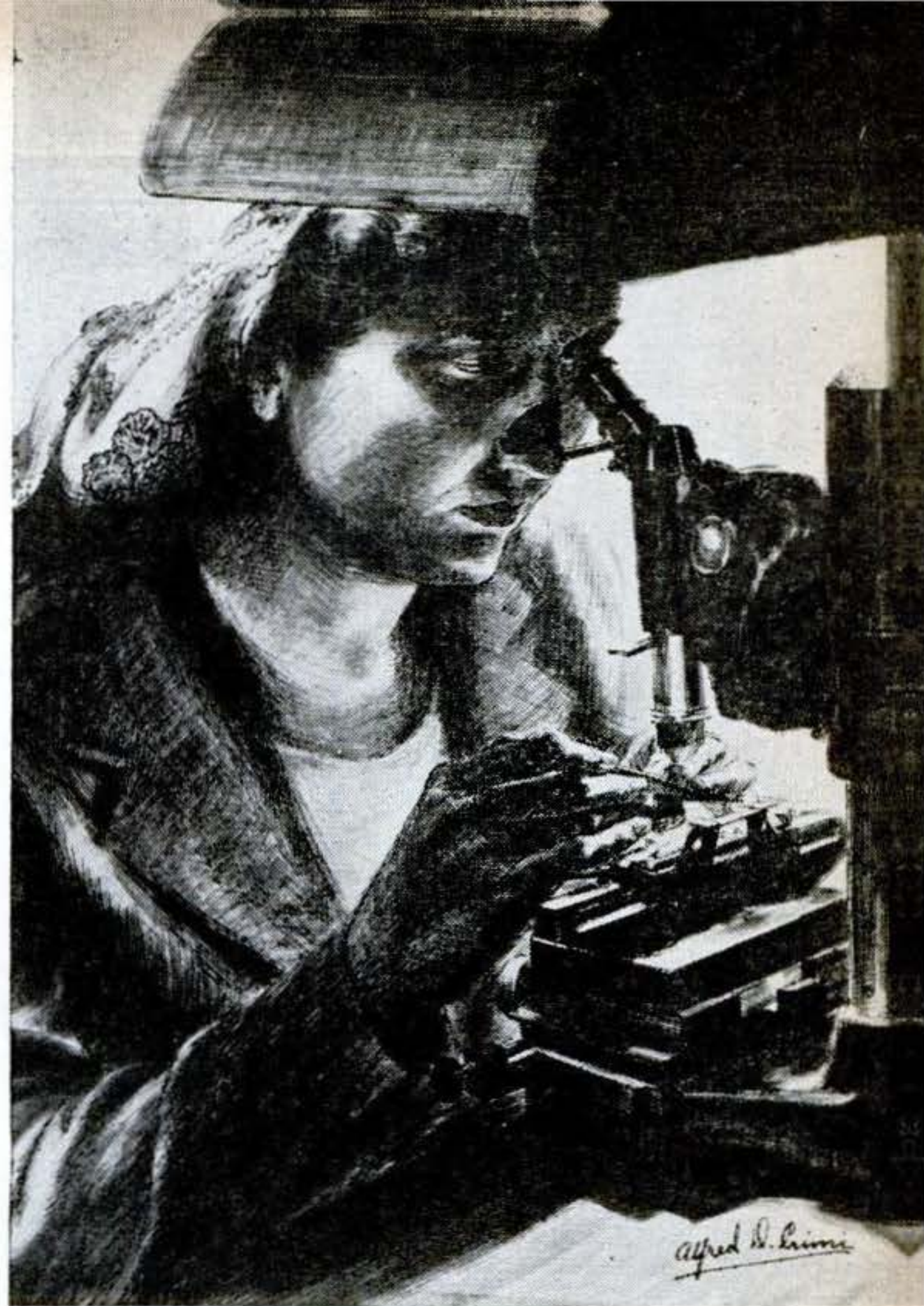
RANGE SPRINGS for the sight are set under a microscope. A study in patience and concentration.
