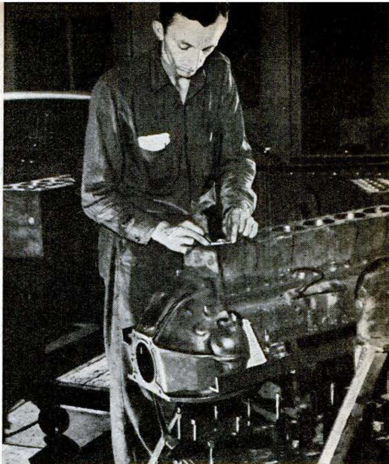
IN THE SHOP. Harrison checks a cylinder block that has been reground. Despite his artificial leg, he is able to oversee and help with the shop's work.
