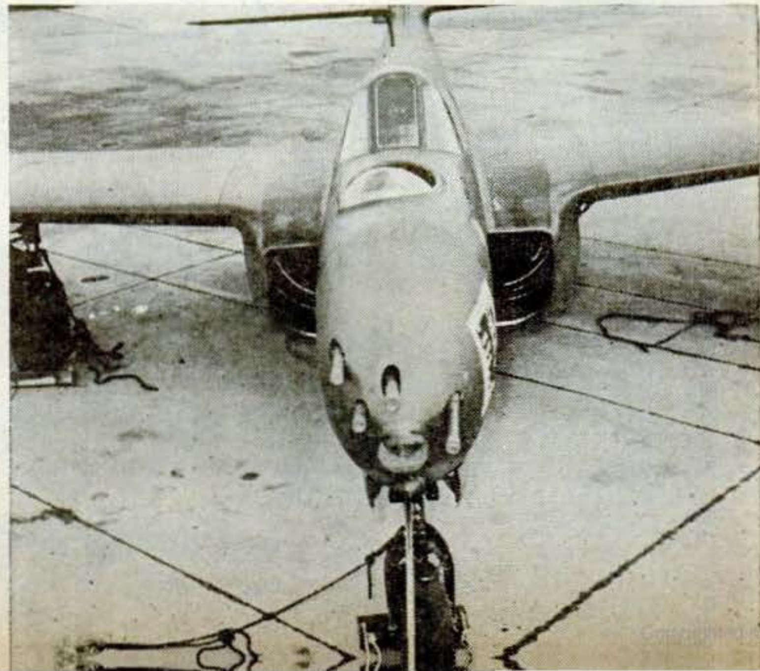
"MYSTIC MISTRESS" is mother plane for "Reluctant Robot." Extra cockpit is for observer. Radio controls are on pilot's throttle and stick.
