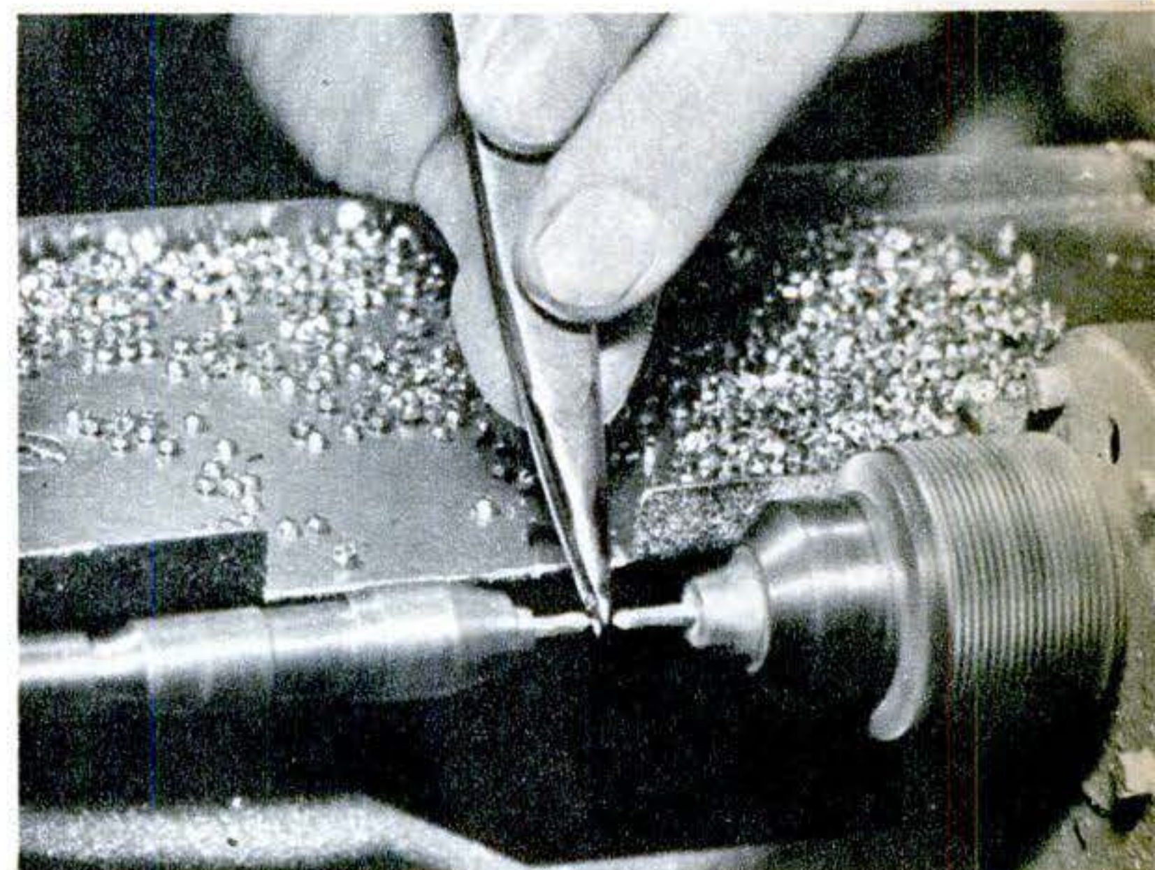
A shank threaded only about a half inch from the end taps the nuts and they build up until the shank is full.
