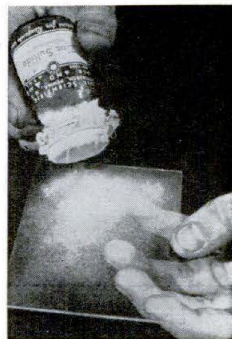
Tiny fluorescent flashes are given off when alpha rays bombard zinc sulphide in a darkened room. It is the same principle as that employed in treating watch dials with luminous paint.
