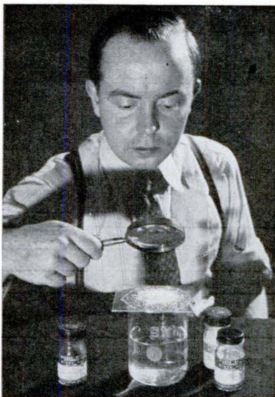
Tiny fluorescent flashes are given off when alpha rays bombard zinc sulphide in a darkened room. It is the same principle as that employed in treating watch dials with luminous paint.
