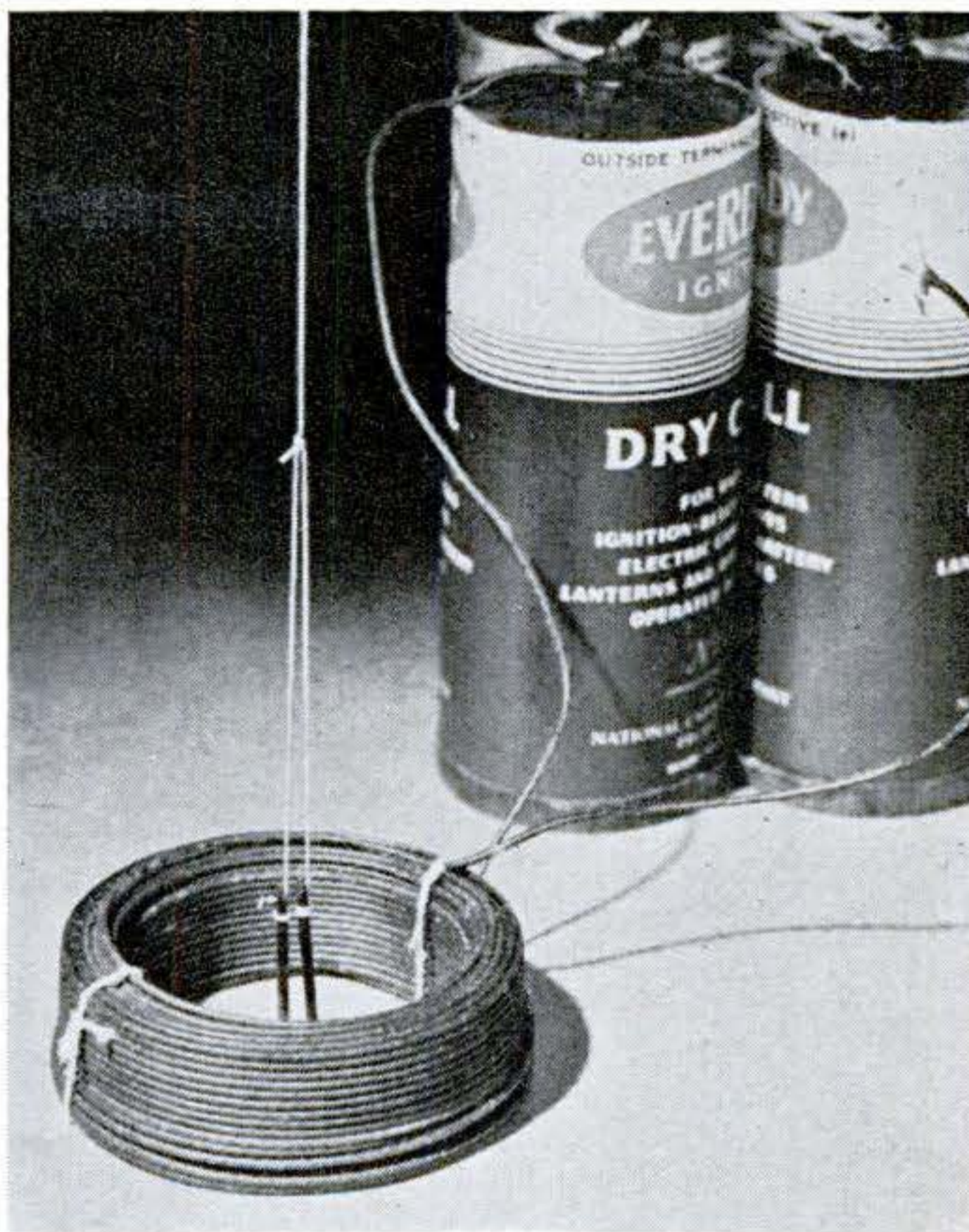
Two nails hang side by side when no current flows in the coil, but when a magnetic field is set up, they acquire like poles and fly apart as at left.
