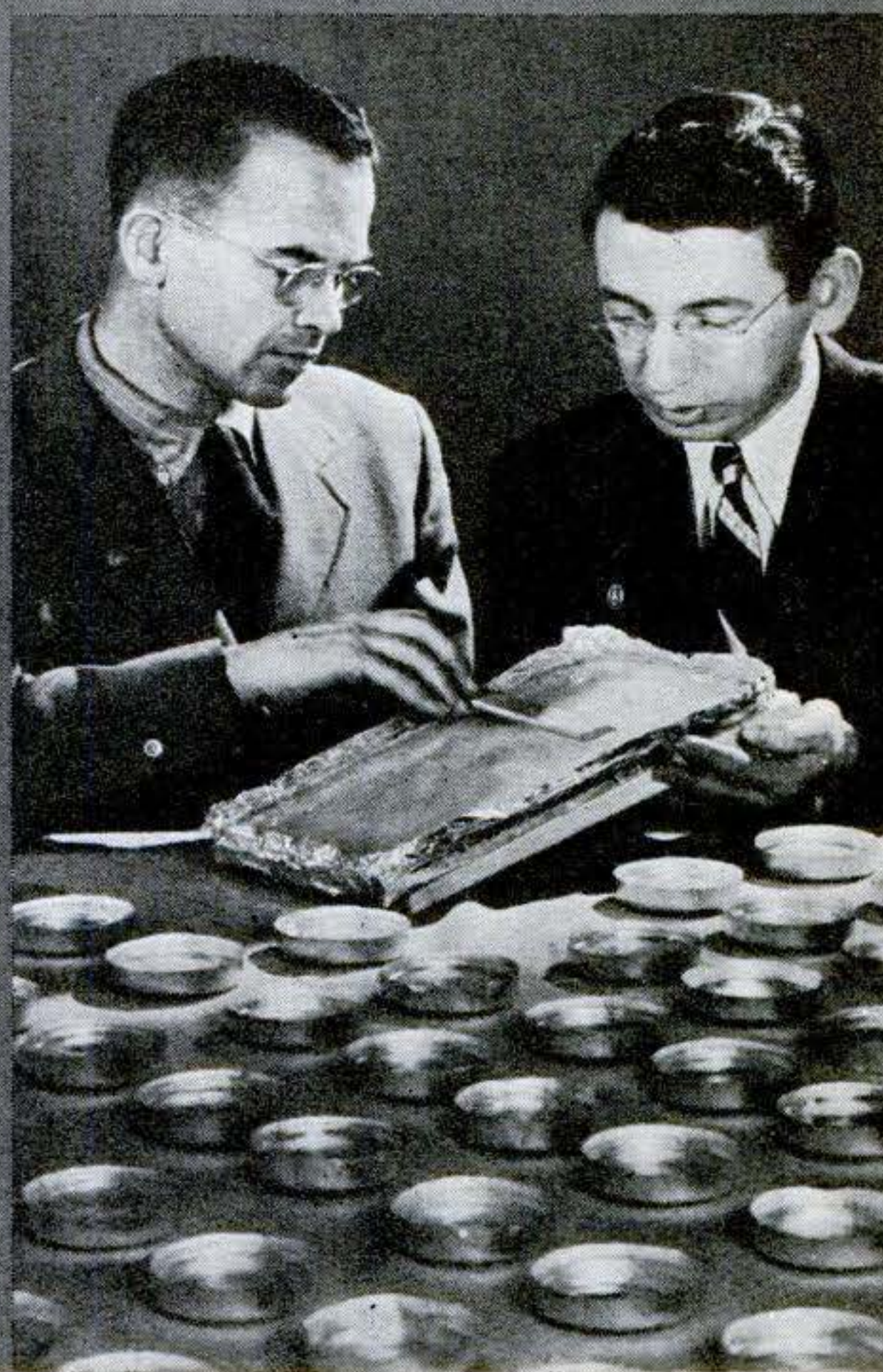
6 The synthetic crystal, optically superior and much larger than calcite produced by nature, is ground on a piece of sandpaper to eliminate minute surface bubbles.
