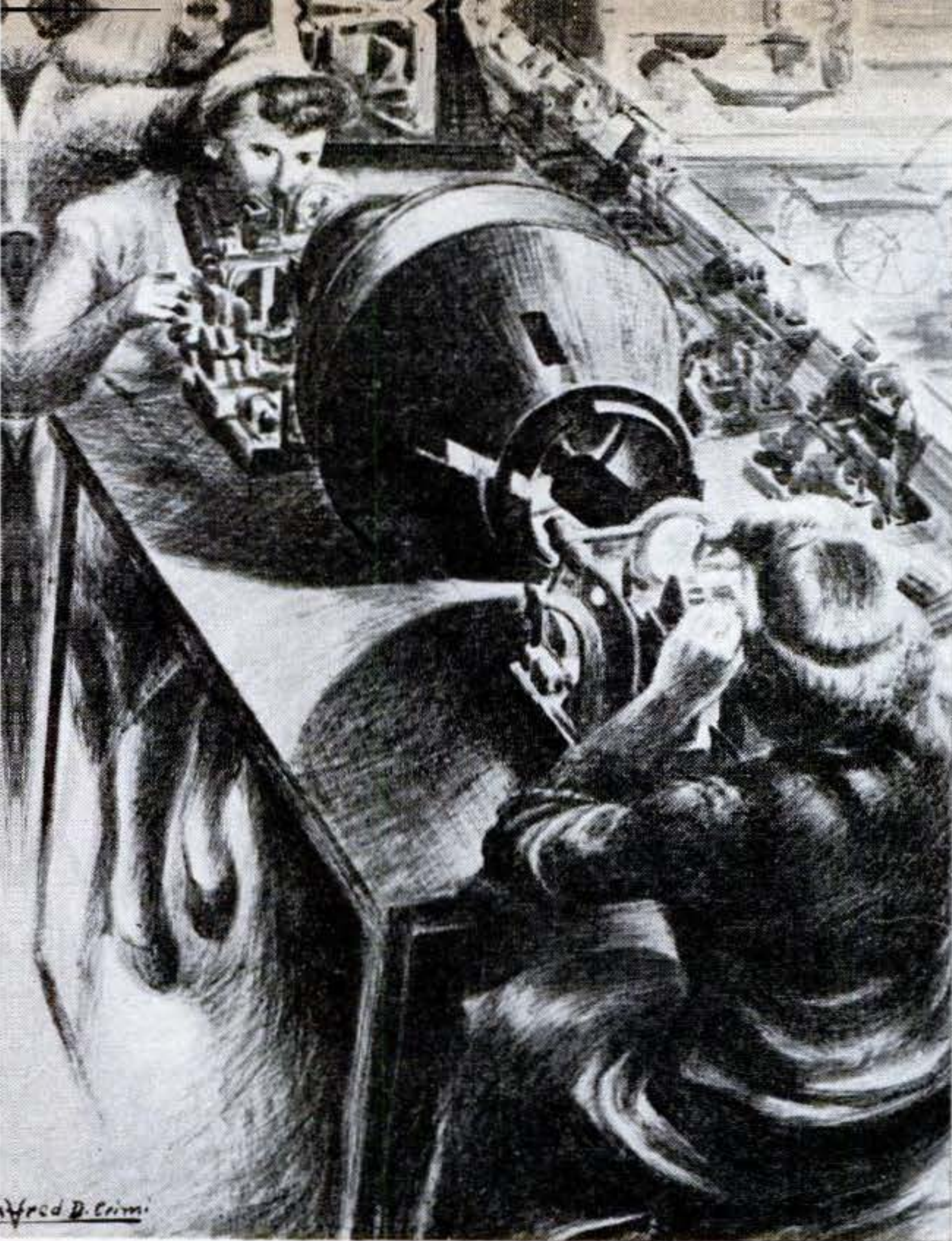
ASSEMBLY LINE of a Navy gunsight, where rigid adjustment is made on the sight's optical alignment.
