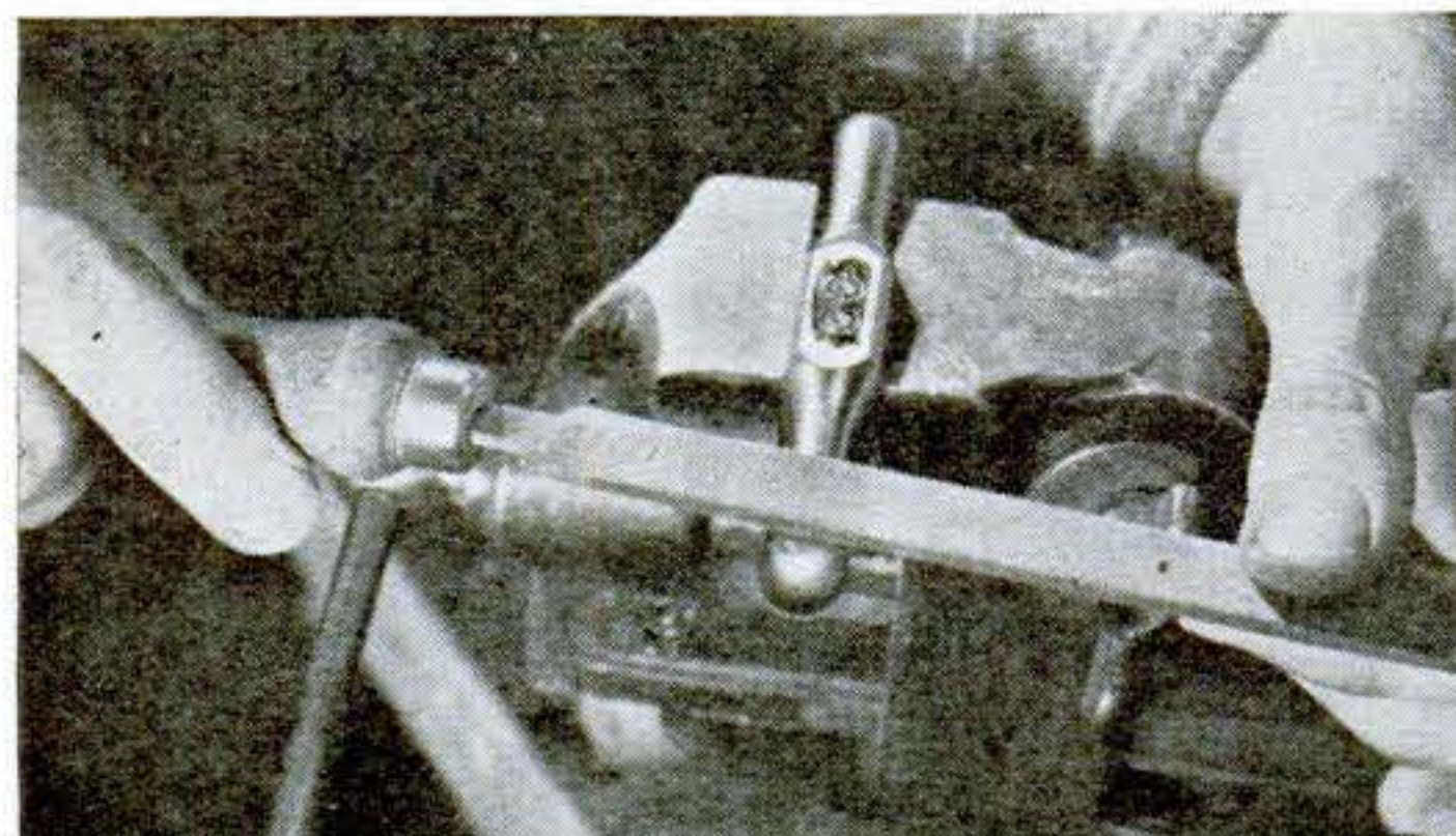
Filing brings the ends to oval shape. Note that two holes are laid out on the flat for the eye.
