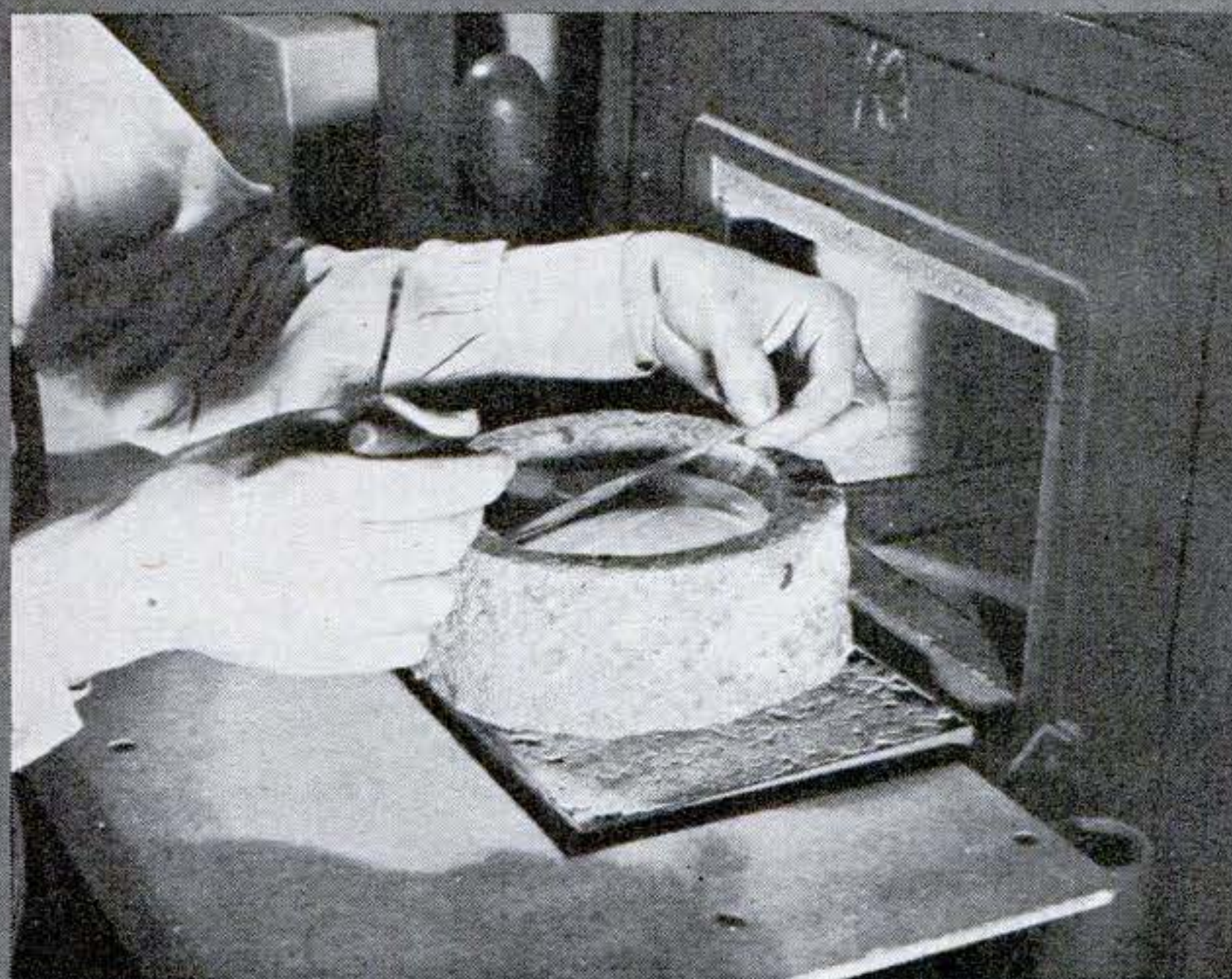
3 Molten crystal is withdrawn from the oven, and the mica floated on it. This piece of mica controls the arrangement of the atoms in the molten mass as it hardens.
