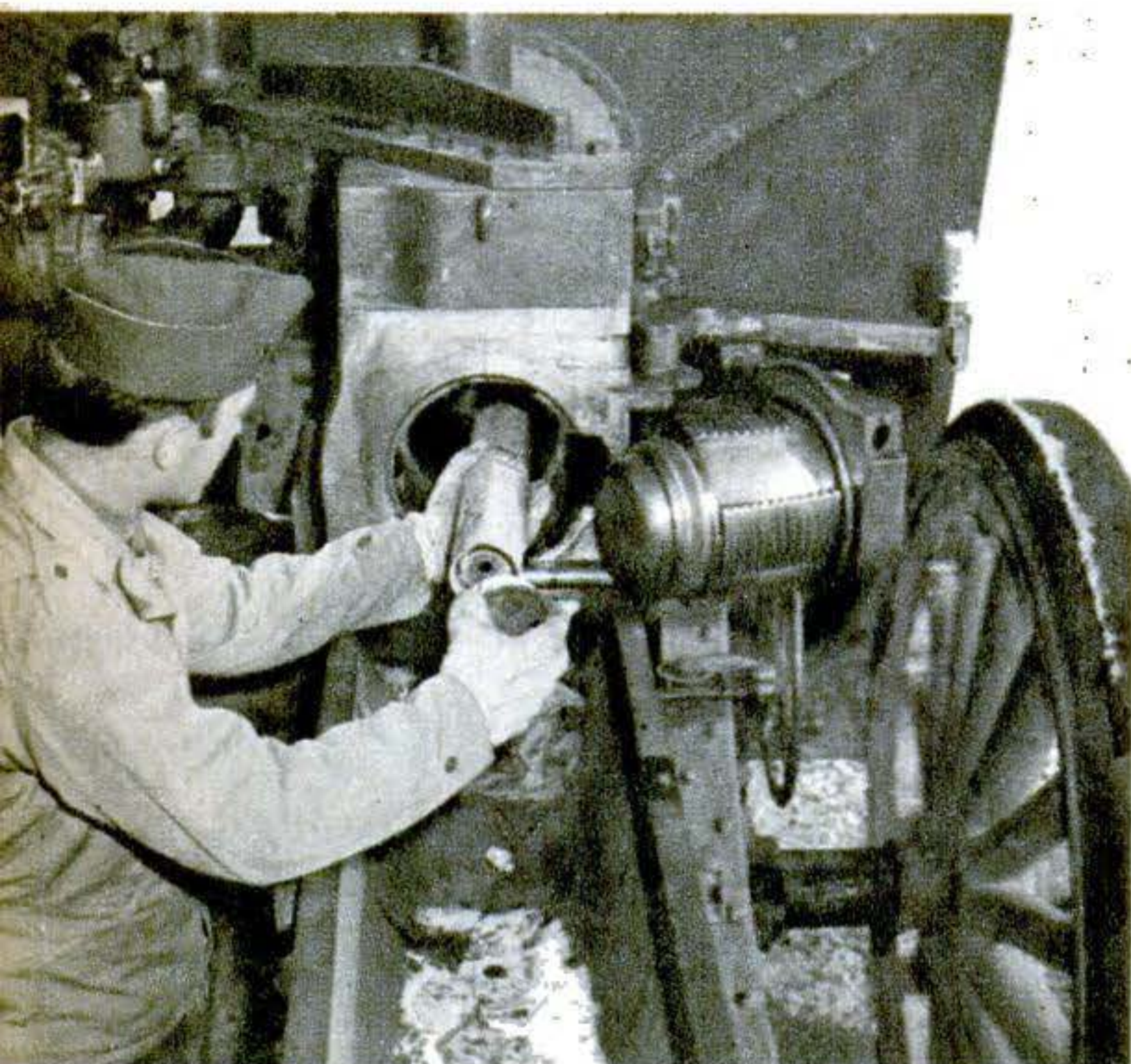
LOADING. A small block of wood with a leather washer is placed in the rear end of the bomb when it is to be fired from the air gun. Fitting the barrel snugly, the washer keeps air from escaping around the projectile. At left, an M-74 incendiary is being loaded into the opened breech of the gun.
