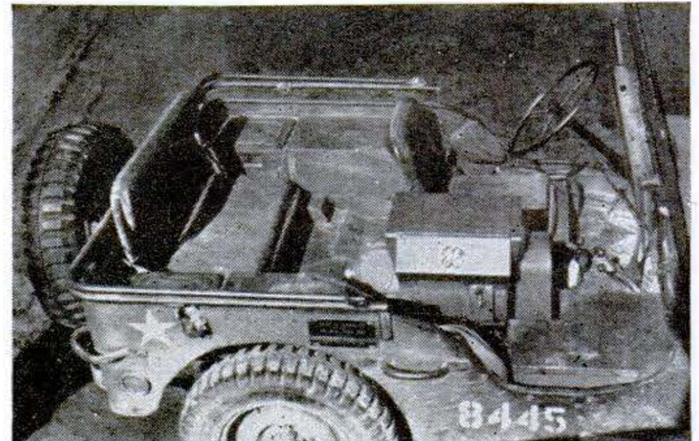
Above, gas welding equipment in a special rack on a jeep. Below, the versatile electric welder jeep.
