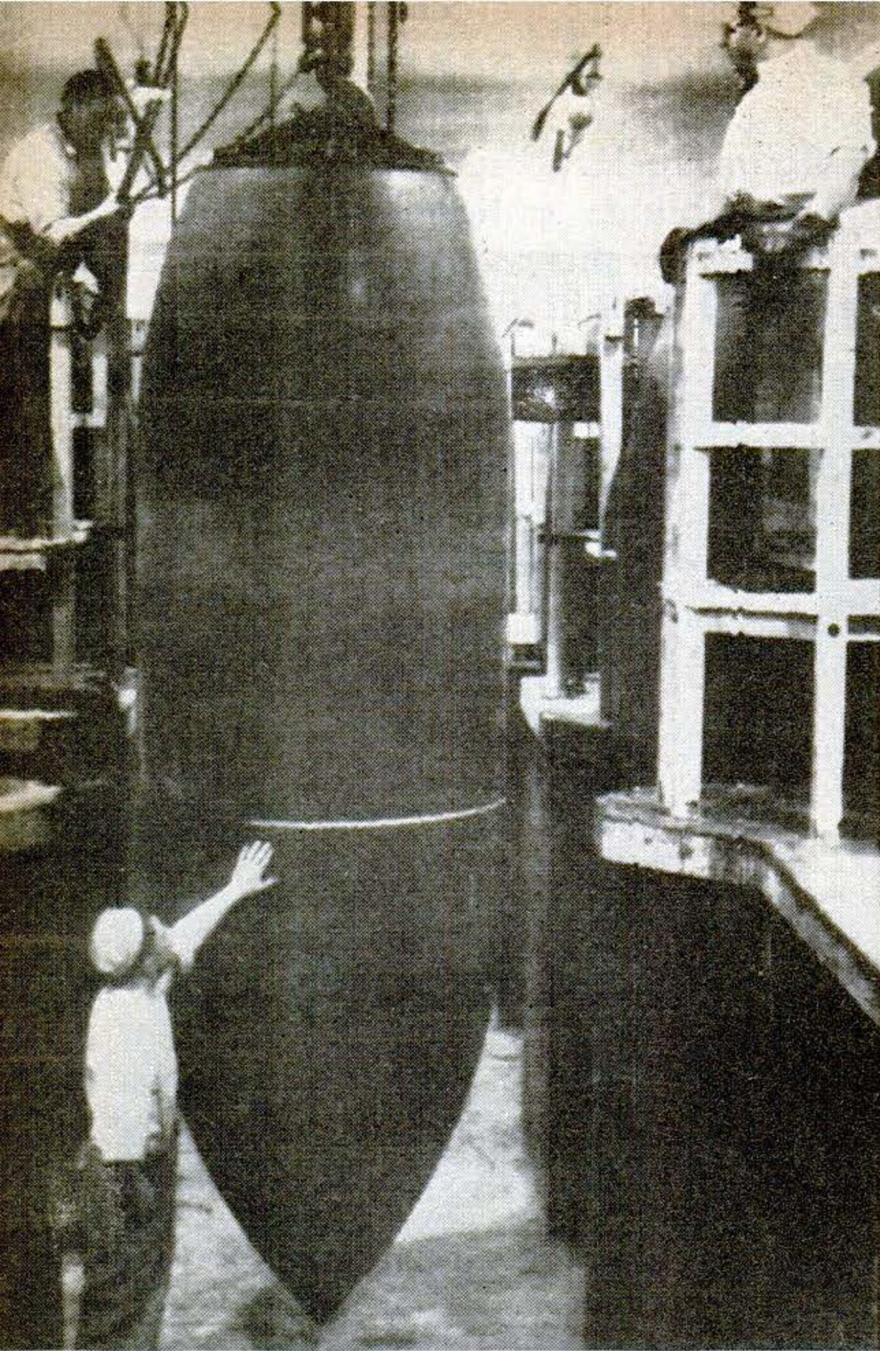
"VOLCANO" BOMB , biggest ever used, is 10 times as destructive as the German V-2 rocket. Only one plane—the British Lancaster—can lift this giant missile, which is 25 feet, 5 inches long and weighs 11 tons.
