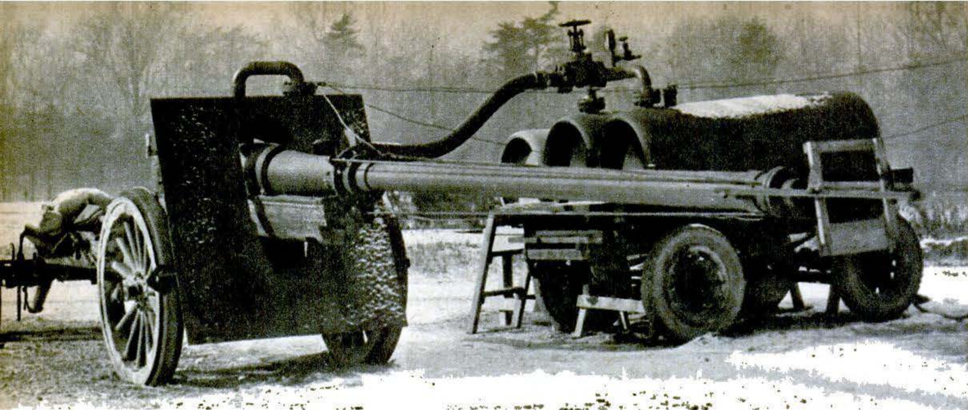
"AIR GUN" TESTS INCENDIARIES at Edgewood Arsenal. Compressed air piped from tanks into the breech of this World War I 155-mm. gun hurls bombs to simulate their falling speeds on targets.
