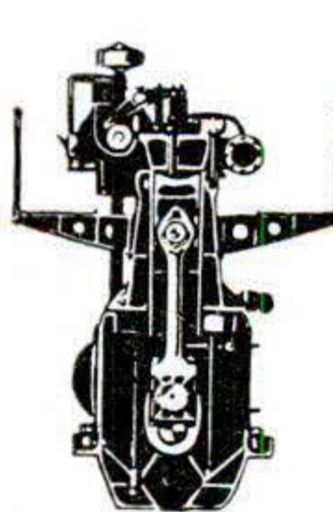
Section through power cylinder — Worthington Diesel Engine.
