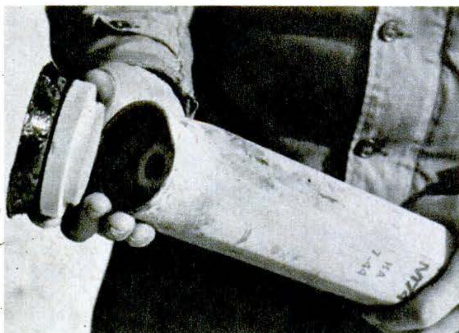
LOADING. A small block of wood with a leather washer is placed in the rear end of the bomb when it is to be fired from the air gun. Fitting the barrel snugly, the washer keeps air from escaping around the projectile. At left, an M-74 incendiary is being loaded into the opened breech of the gun.
