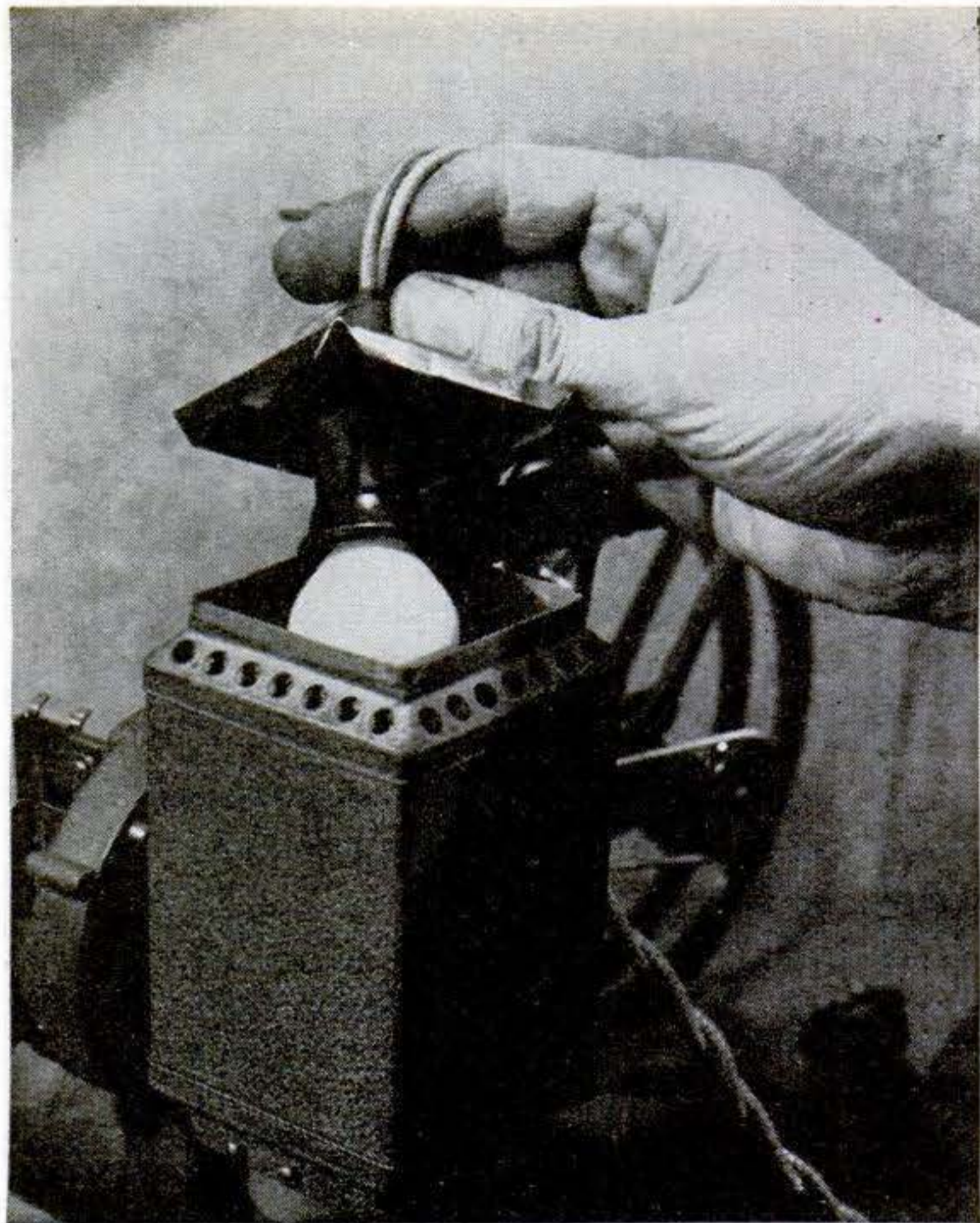
This small opal-glass lamp gives light for printing. The metal cap supports it in the projector lamp house.
