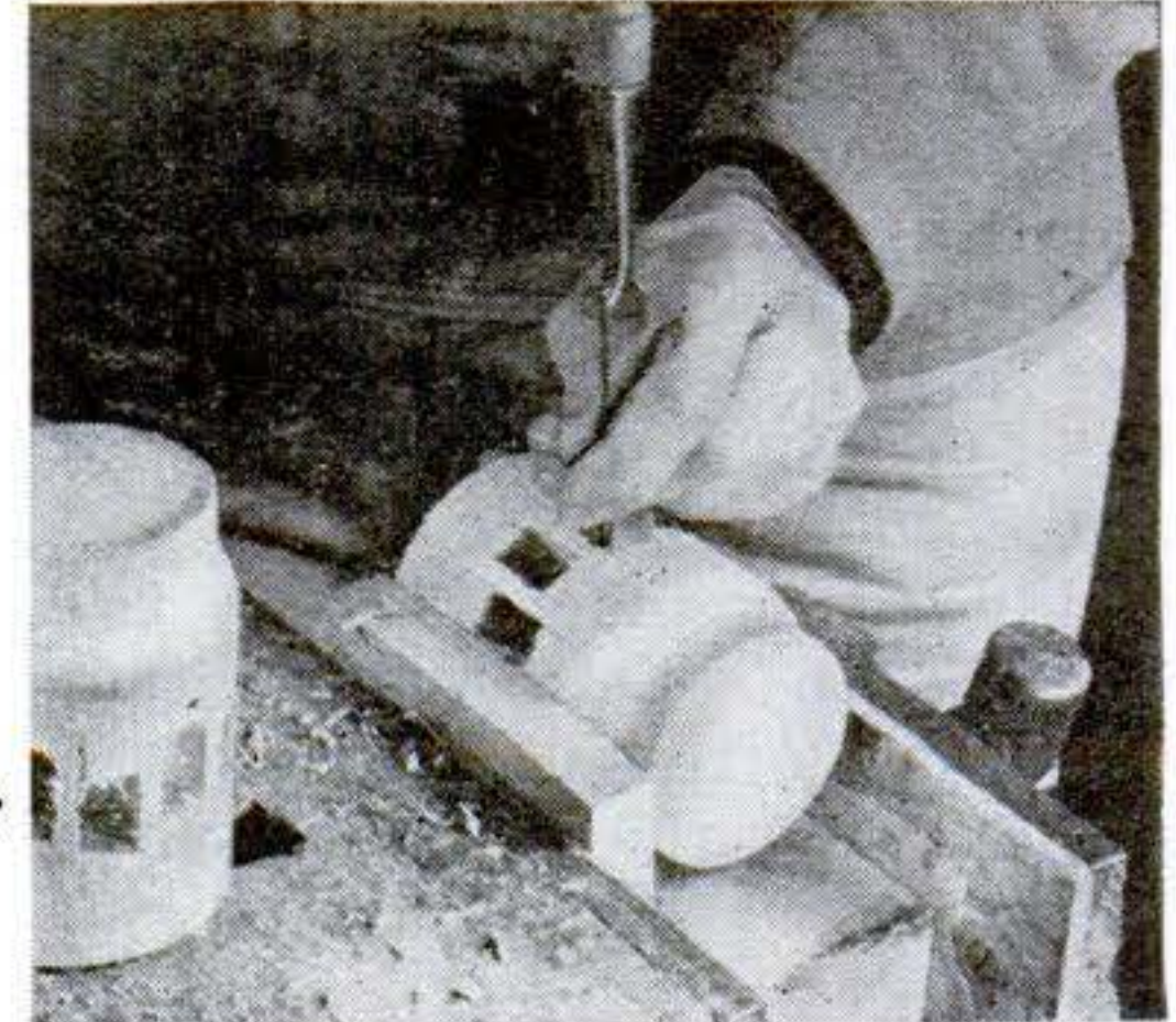
This jig is also of use when the drilled mortises are chiseled to shape, as shown at the right. Note the slight staggering of alternate mortises.
