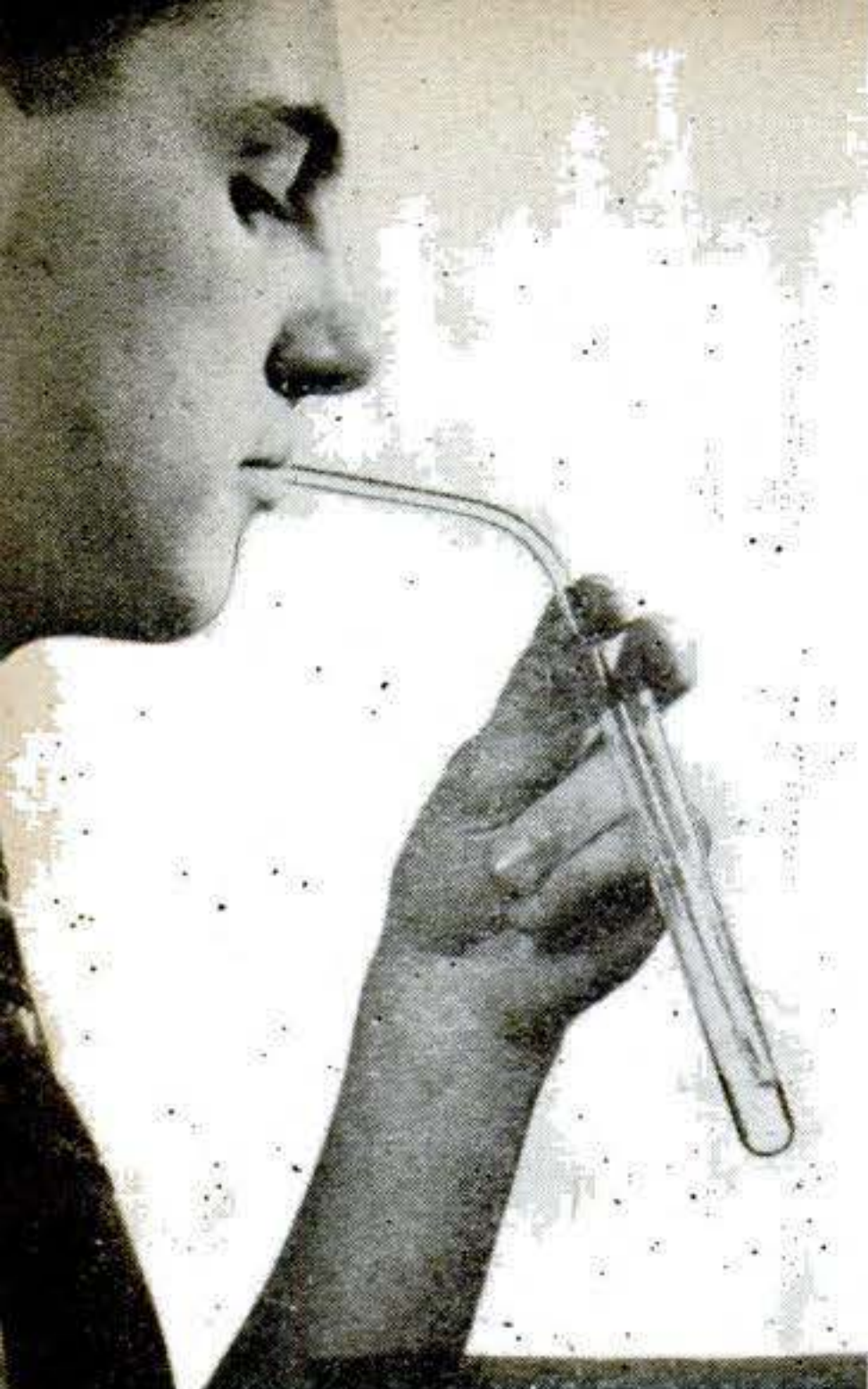
Blow into a weak alkaline solution and carbon dioxide from your breath joins the water, forming carbonic acid that neutralizes the solution. Drive out the CO 2 , and the alkalinity is restored.
