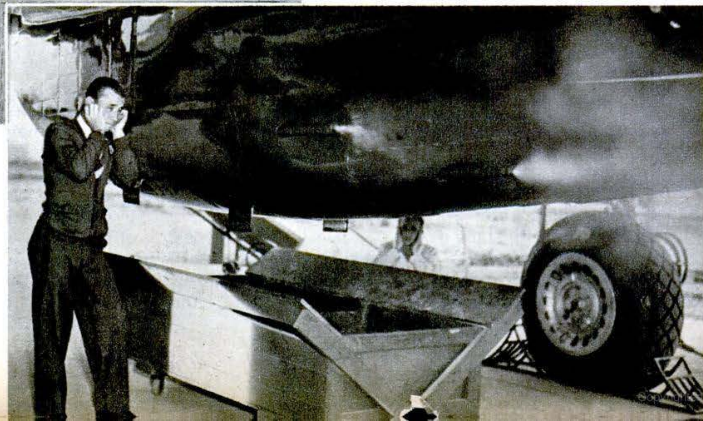
BIG NOISE is the result when ordnance men test the 20's on the ground. The box is placed under the fuselage to catch the empty shells.
