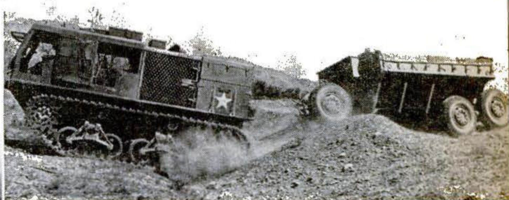
Rough-riding trailers bear the shells to feed the huge M-1. Each carrier hauls 32 rounds, enough for about half an hour.
