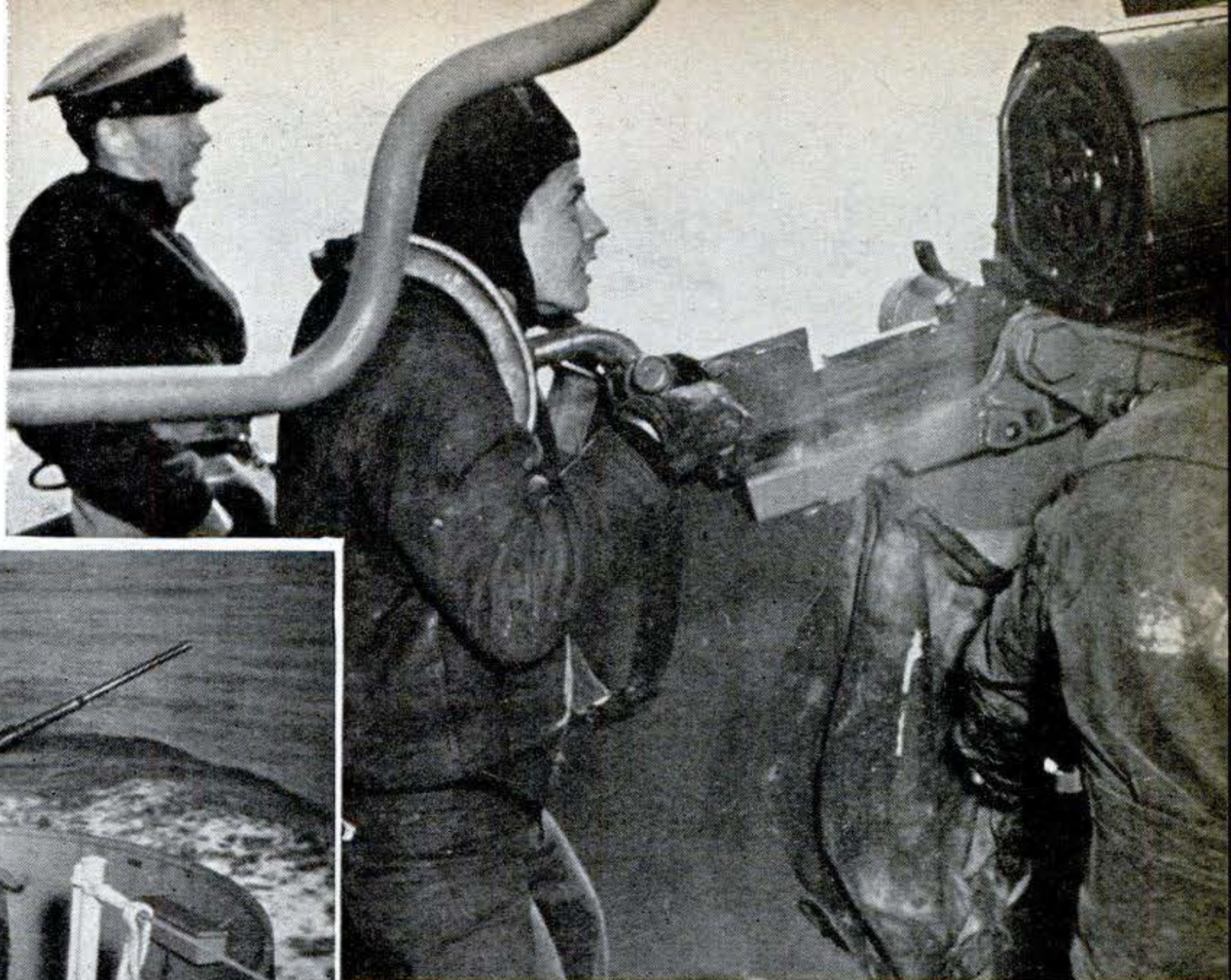
20-MM. OERLIKONS guard the destroyer against low-flying enemy planes. Independently controlled, they fire tracer shells at intervals for correcting the aim.
