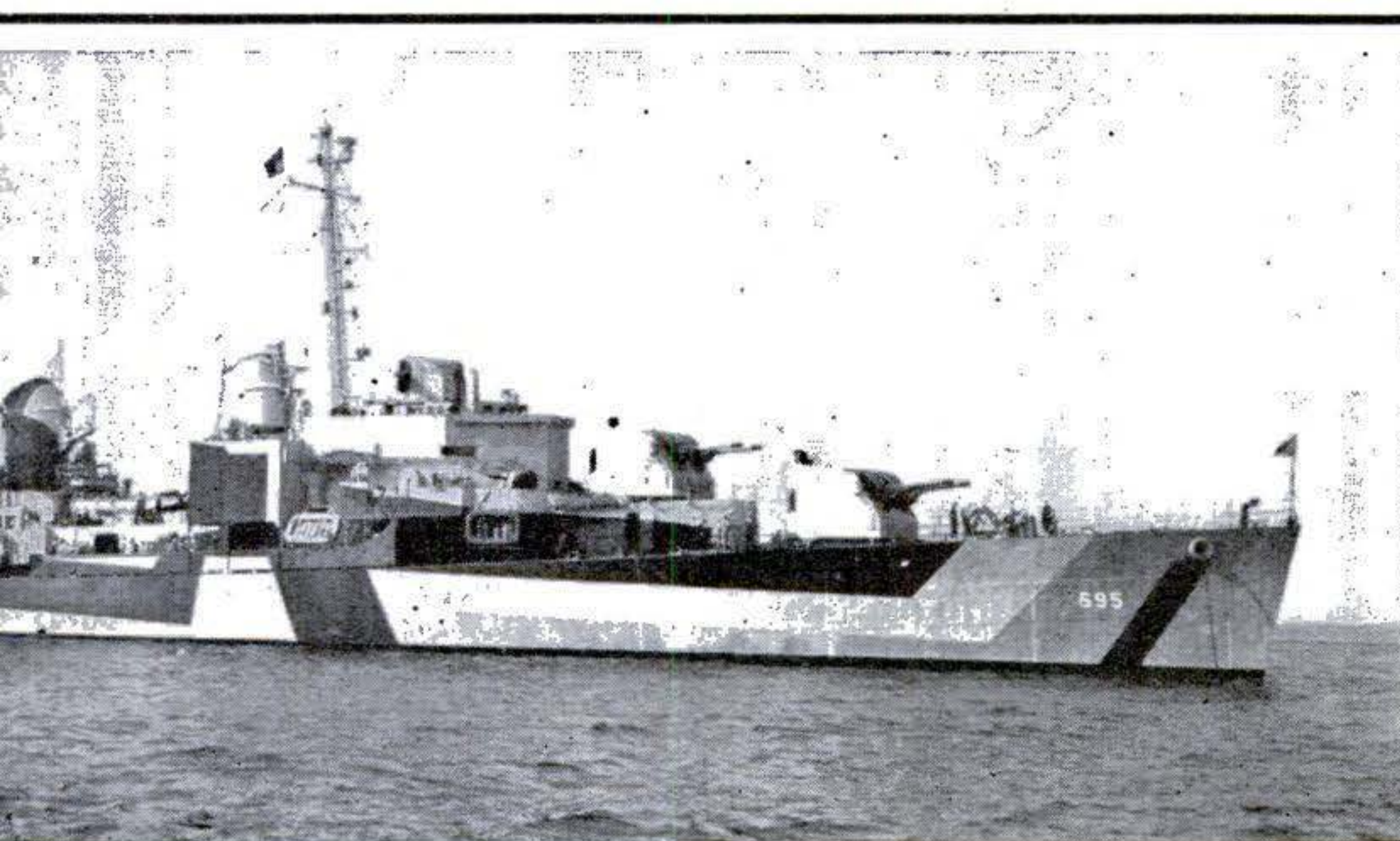
SUPER-DESTROYER. Ships of our Allen M. Sumner class, such as the Cooper (left), are so big and powerful that in the last war they would have been classed as cruisers. Much of the great weight (2,200 tons) went into increased armament. The guns can throw over a ton of steel in 15 minutes.
