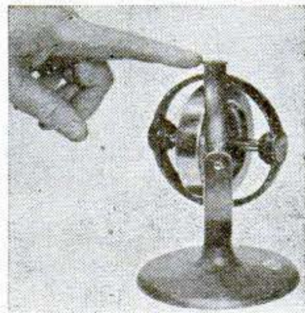
Try to push the rotor out of its spinning plane. Instead of tipping, it turns to side.
