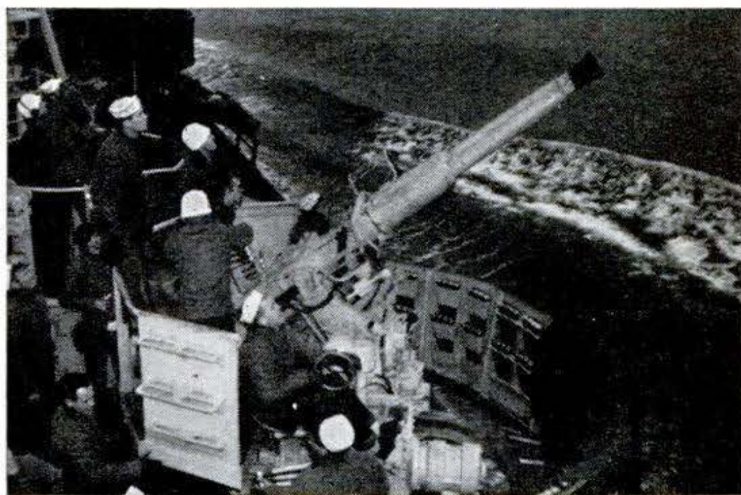
40-MM. BOFORS guns in twin mounts are dual-purpose weapons, used against planes and warships.
