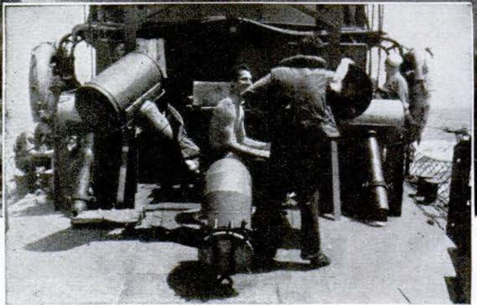
Y GUNS (right) toss depth charges far out on both sides to crush lurking submarines. Above, an "ash can" hurls up a geyser of water as it explodes.
