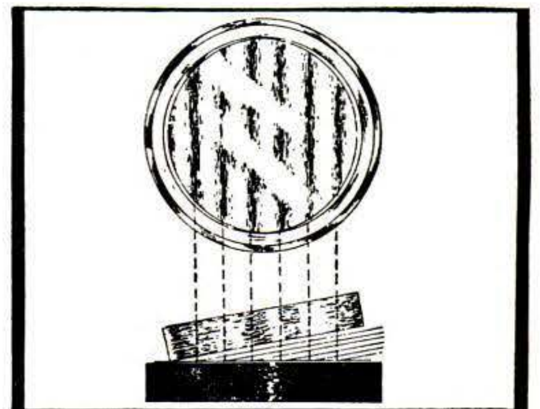
Optical Flat. Surface of Work. Interpretation of bands on truly flat surfaces.
