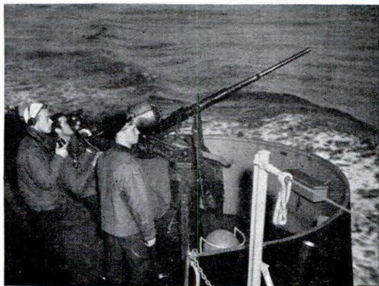
20-MM. OERLIKONS guard the destroyer against low-flying enemy planes. Independently controlled, they fire tracer shells at intervals for correcting the aim.
