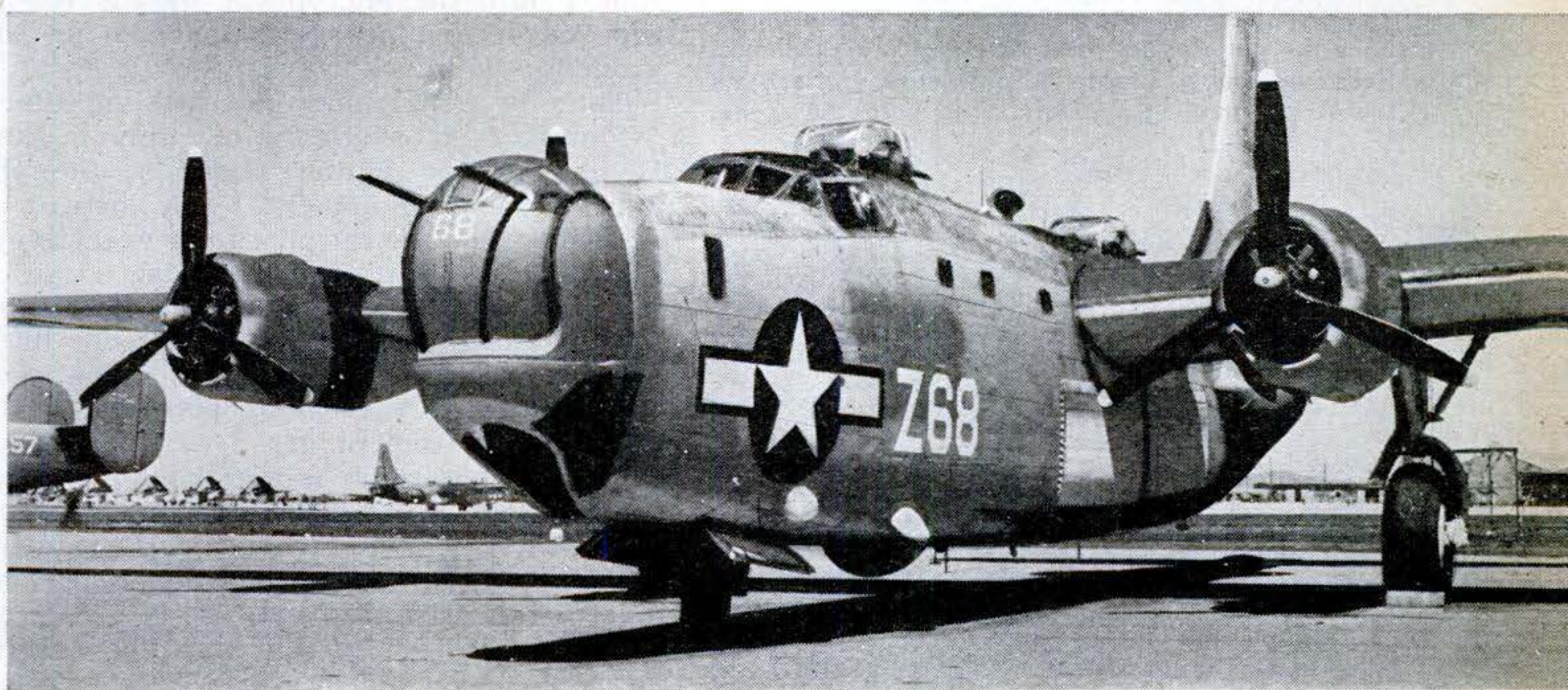
A Privateer (Navy patrol-bomber version of the B-24 Liberator) displays a load of radar gadgets. On top of the fuselage, back of the gun turret, is the IFF antenna. Under the belly, the second white "radome" is the "potato masher" for jamming enemy radar. The rounded bowl is the retractable "dish" antenna of the ASV (Air to Surface Vessel) search set. Rods behind this are antennas of the radar altimeter.
