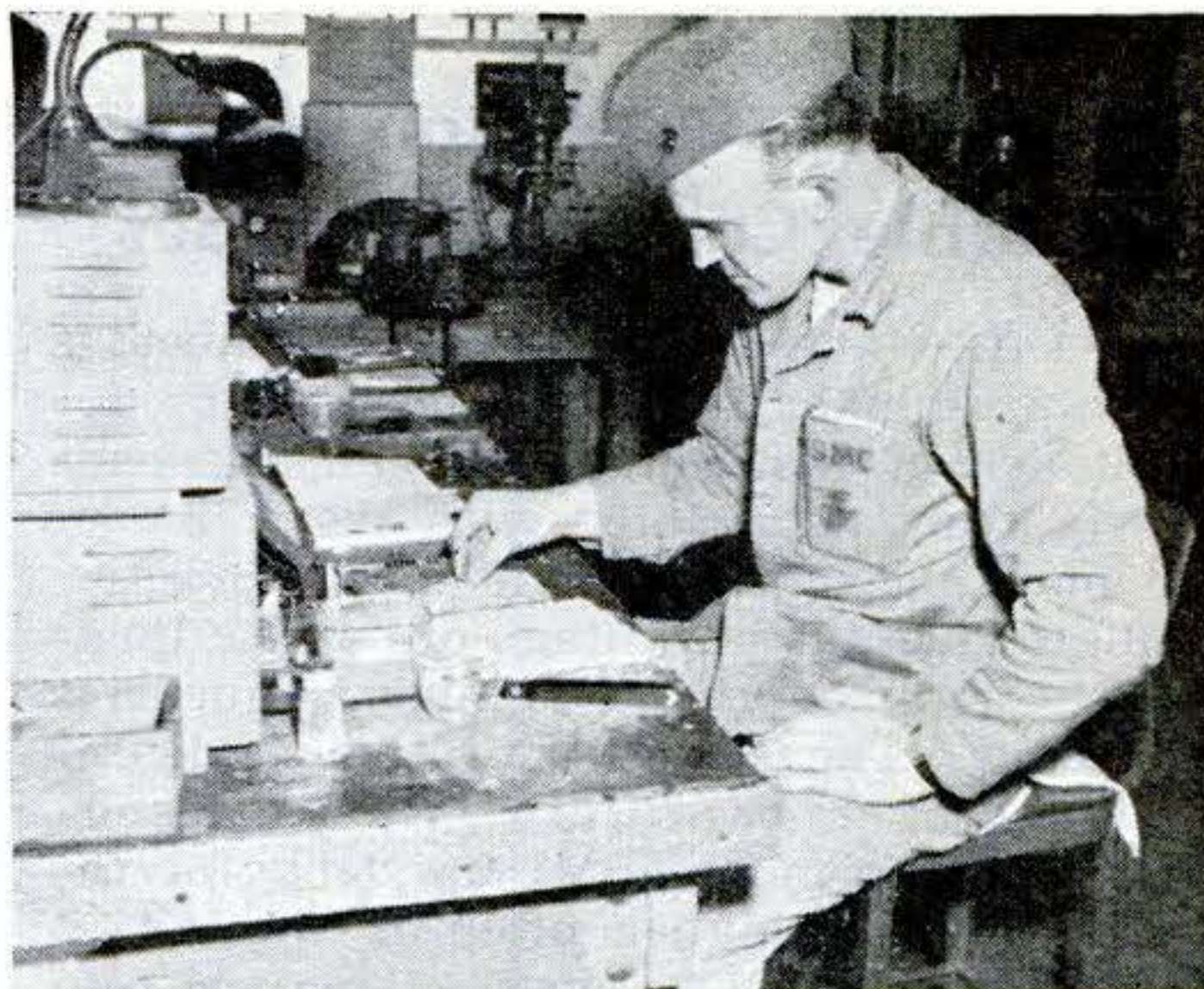
To obtain accurate frequency control, every crystal must be finished by hand (above), and tested on an oscillator (below). If it can then pass heat, shock, and vibration tests, the crystal is ready for use.
