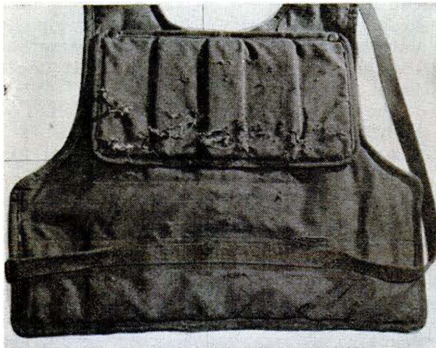
This back piece took a lot of punishment. Our body armor can't stop all shell fragments, but it protects against the kinds that cause most casualties.
