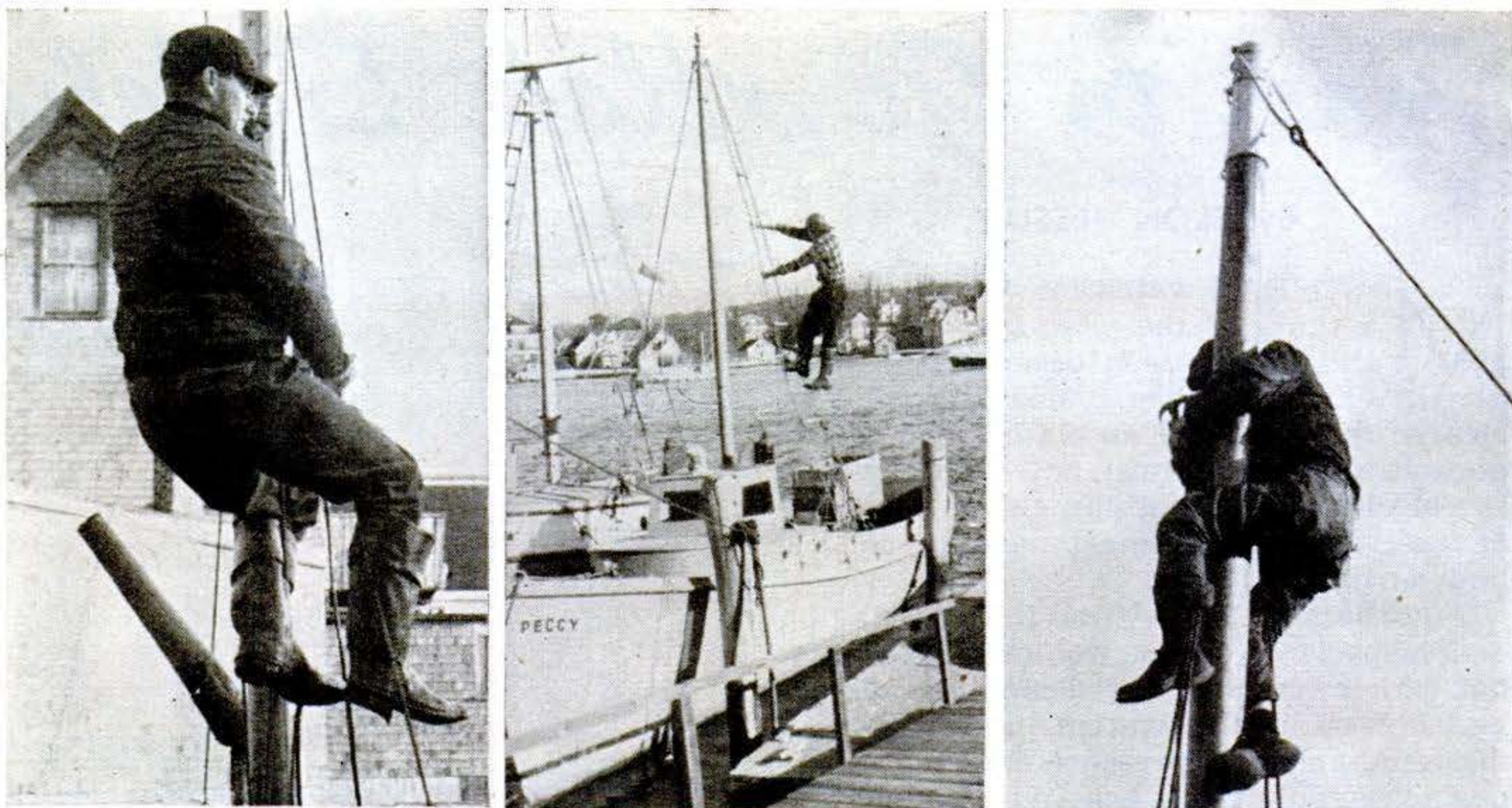
Taking it easy on a pair of shrouds. The Down East fisherman at left, up for observation, wears sea boots to help his legs grip the shrouds. Ratlines on the powerboat at center are solely for reaching the light. At right, the sailor uses the narrowed ends of shrouds for holding on while engaged in a task on the masthead.
