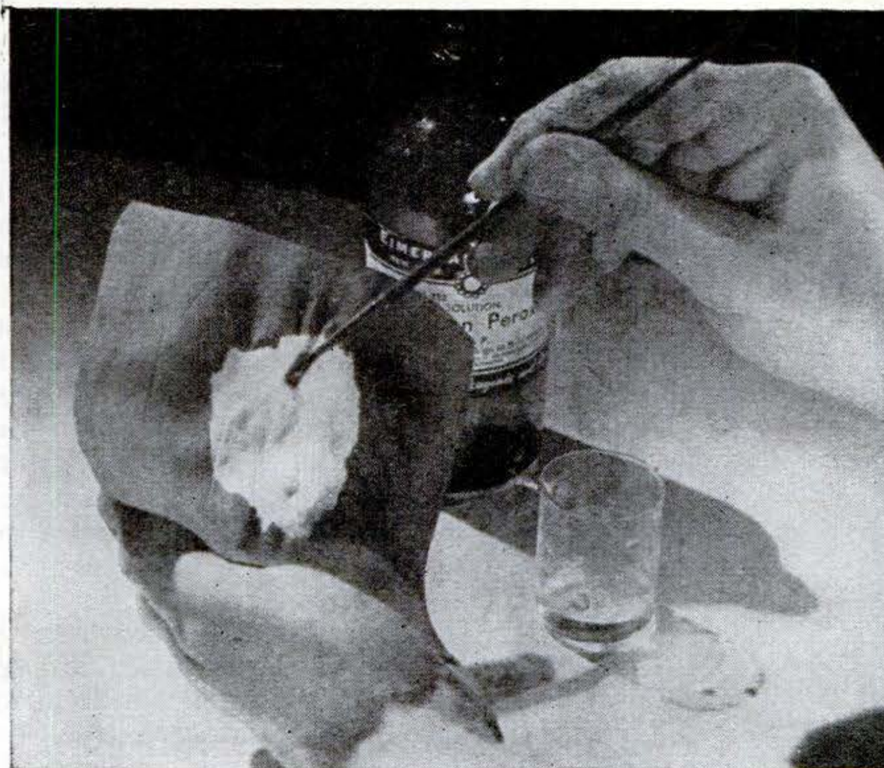
Hydrogen peroxide brushed over lead acetate darkened by hydrogen sulphide restores the original white color, left, as it will when applied to white lead paint. It also functions as a reducing agent. If a few drops are added to a solution of potassium permanganate and sulphuric acid, right, molecular oxygen evolves.
