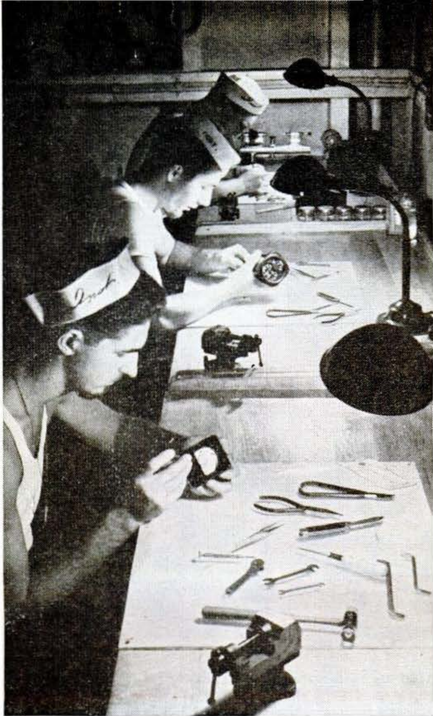
Finest precision work is done in this instrument shop, where compasses, bombsights, gyros, gauges, and other vital parts are completely overhauled. Many of these men were watchmakers in civilian life.
