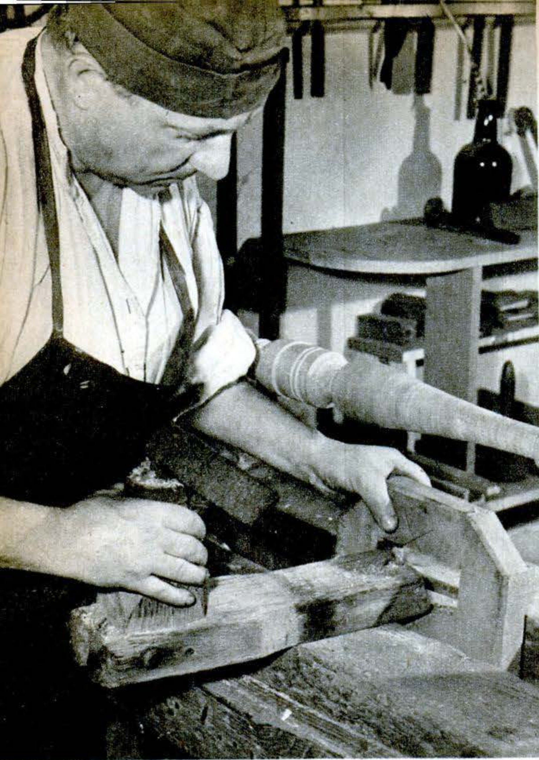
THE OLD-TIME LATHE , used for turning, grinding, polishing, etc., was made of heavy timbers and other pieces, and was a difficult device to adjust. The tool rest, a strip of iron fastened to sturdy wooden pieces, could be moved only by loosening a wooden wedge, then sliding the assembly into the desired position and tightening the wedge again. Above, the cabinetmaker adjusts the piece on which the tool rest is fixed. Below, he inserts the wedge to secure the piece.
