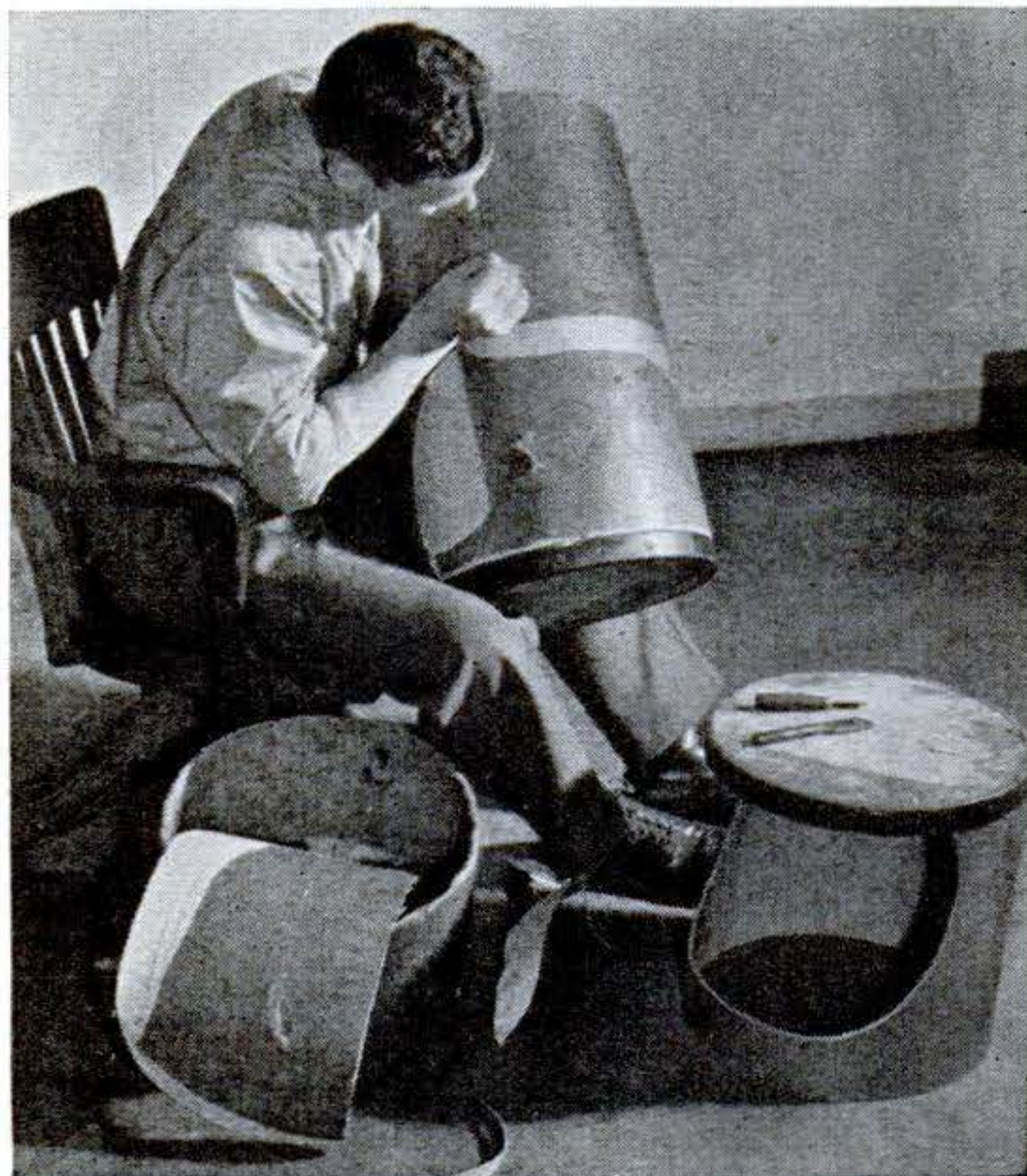
Photo-chemical containers with wooden bottoms are provided with openings and cut to a height of 15".
