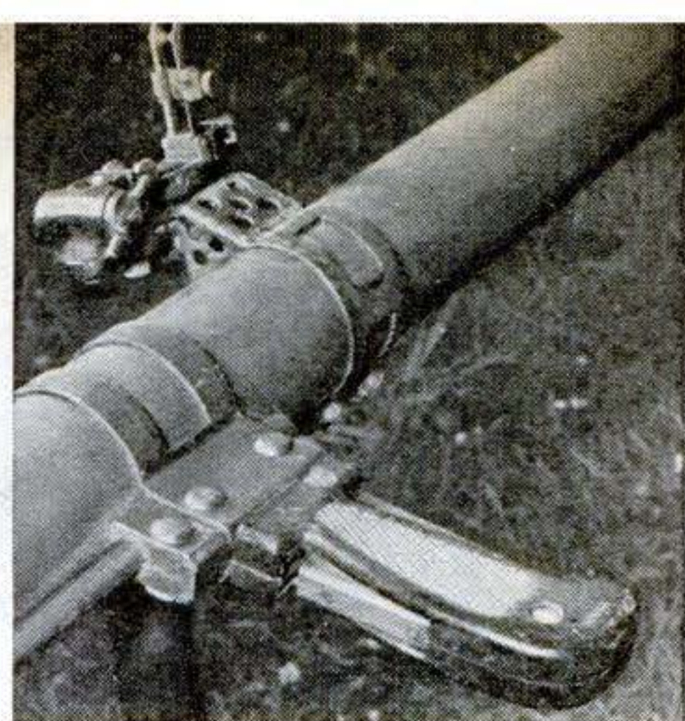
Here's the trigger assembly and the leaf sight on the gun's barrel. The trigger is at the forward side of pistol grip; safety grip is at rear.
