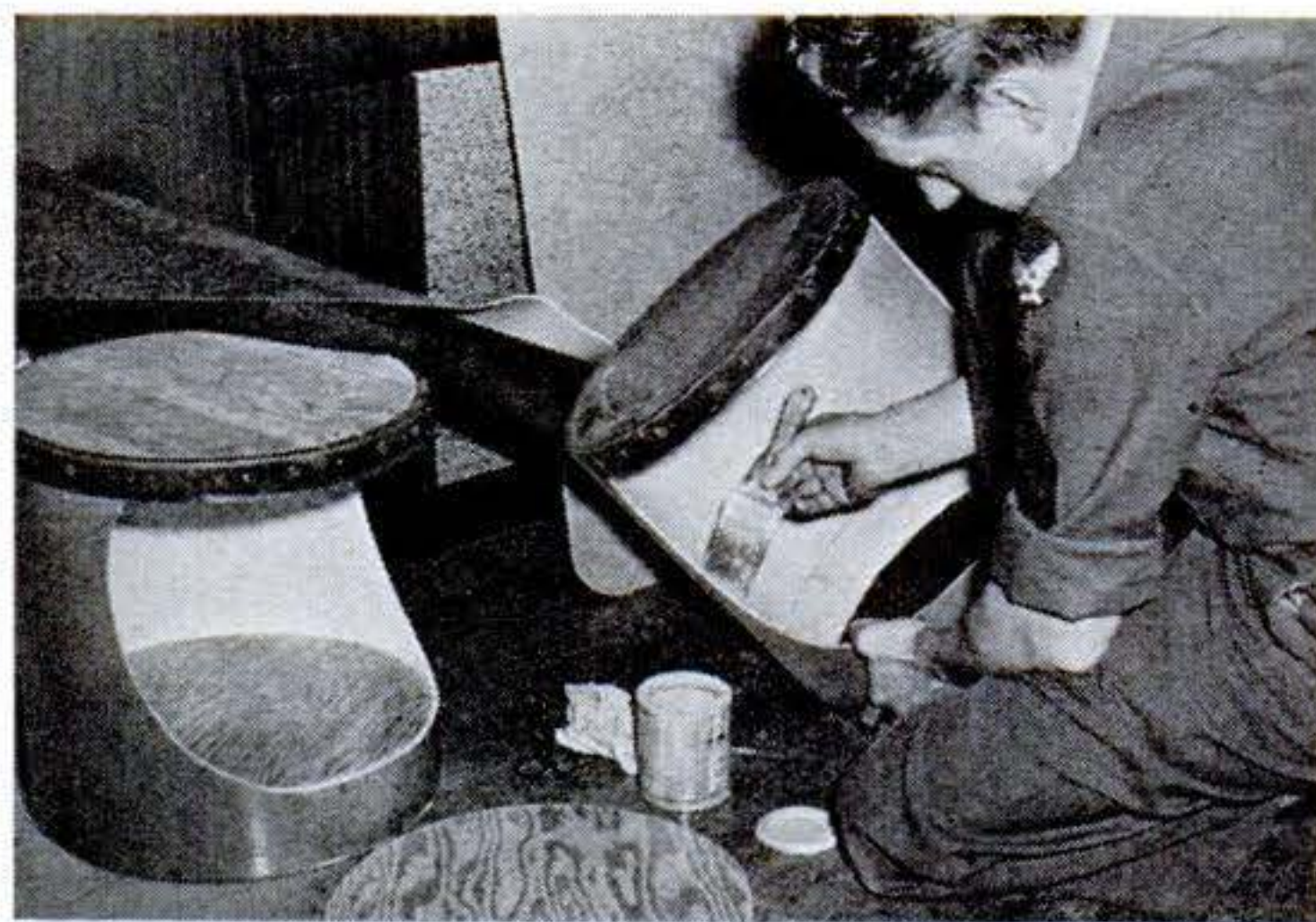
Disks are cut from ¼" plywood for a shelf in each container, and the insides are then painted ivory.
