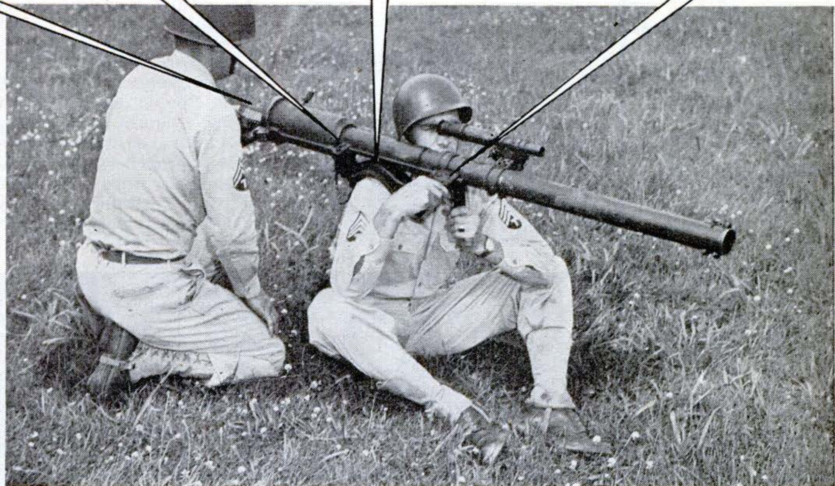
The recoilless cannon looks much like the bazooka from a distance, but, unlike the bazooka, it throws regular high-explosive ammunition or smoke shells which are propelled by a powder charge. Because of the comparatively low muzzle velocity, specially shaped projectiles are used which will penetrate most tank armor. Above, the gunner spots his target in the telescope sight of the infantry's artillery weapon.
