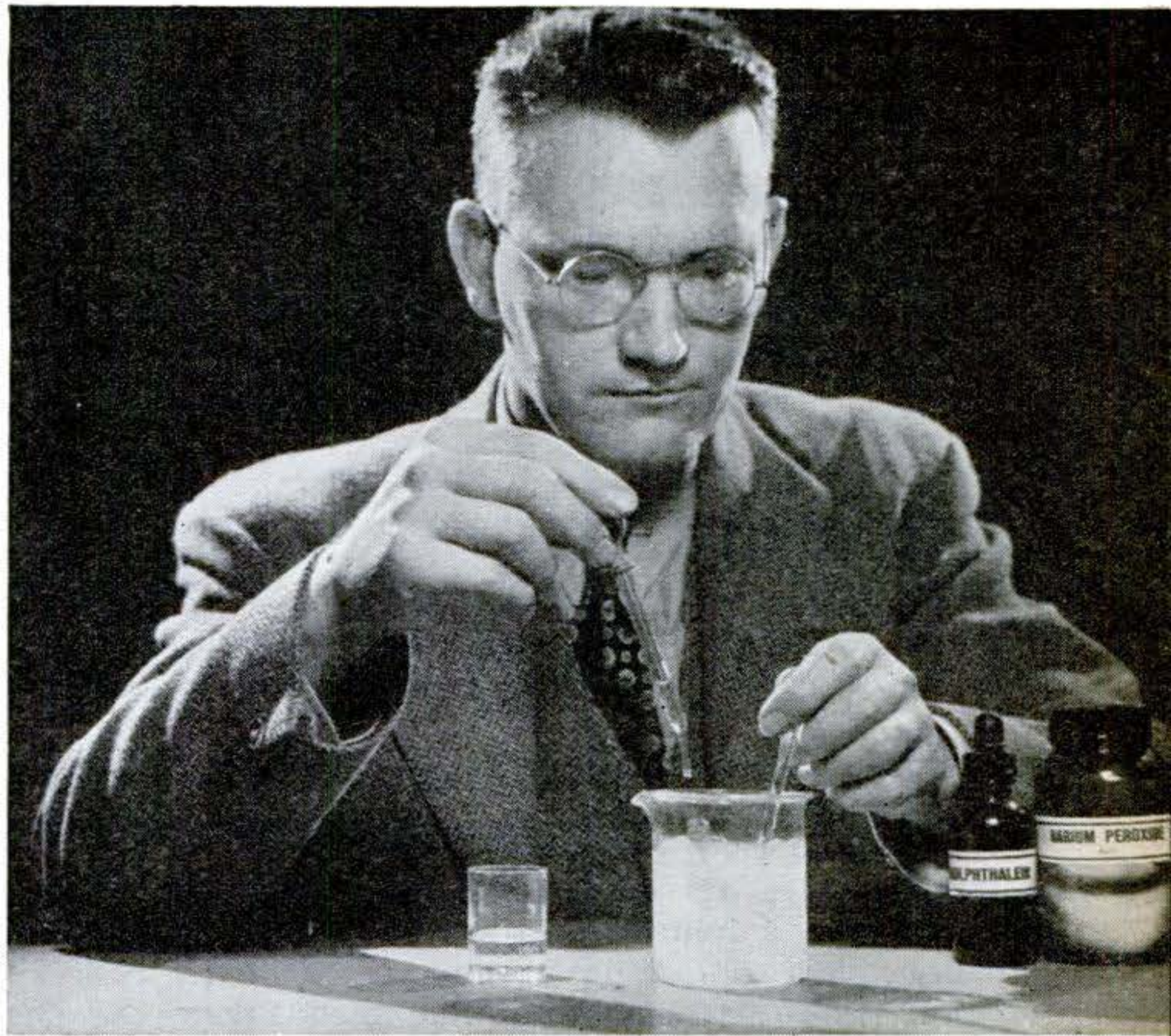
Drop sulphuric acid into an ice-cold barium peroxide solution until it has been neutralized. This reaction produces hydrogen peroxide.
