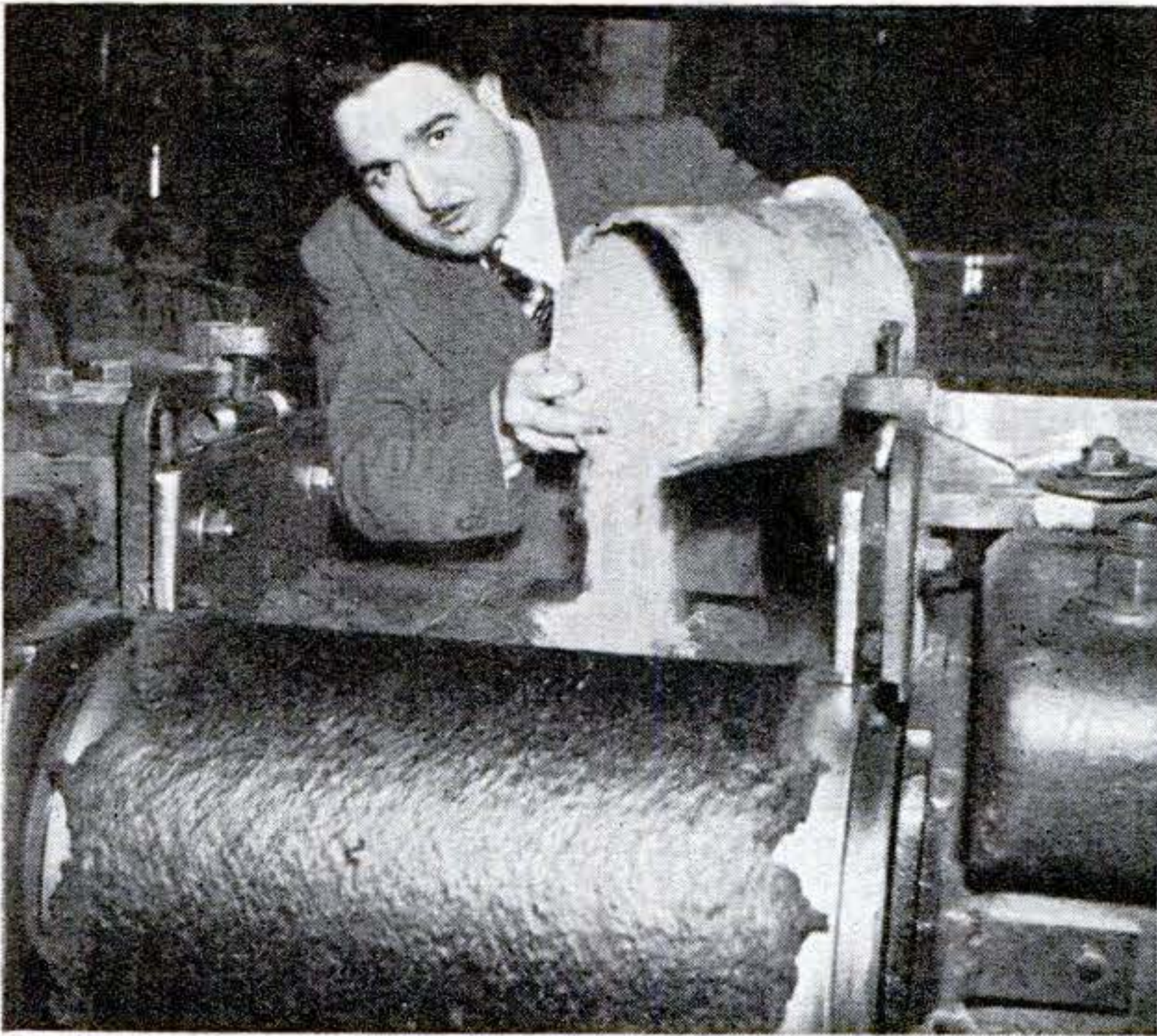
Sawdust spread over soft rubber in the process of retreading gives the tire greater traction.
