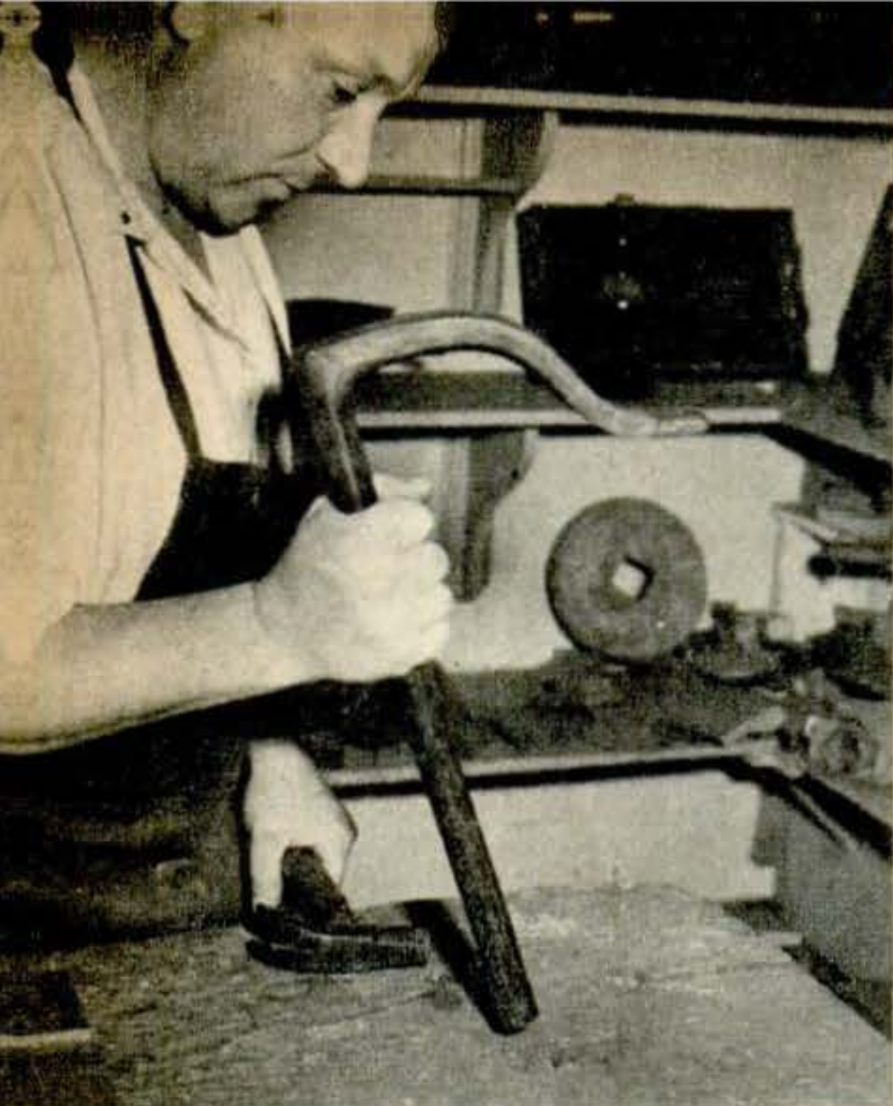
"HOLDFAST." The efficiency of the old-time bench clamp, also called the "holdfast," is demonstrated at The Ayscough Shop in Williamsburg. Inserted in a hole in the bench, it is driven down with a hammer, its clamping end holding the work firmly. The hammer also is of the eighteenth-century period.
