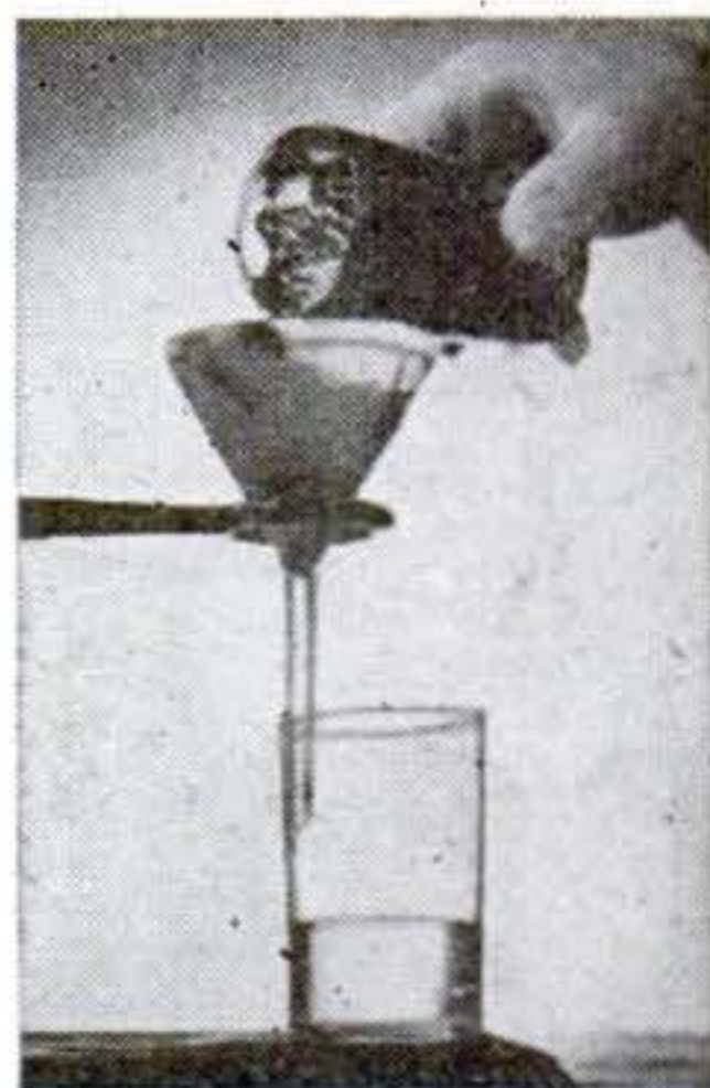
Charcoal takes iodine out of solution, and the liquid will come through a filter amazingly clear.
