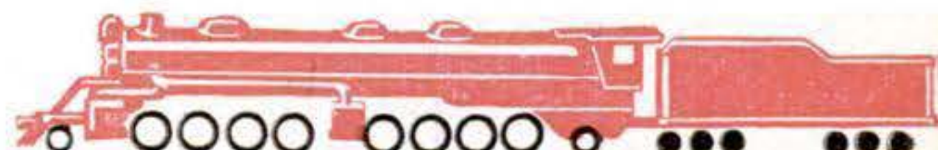
2-8-8-2 type wins its greatest popularity in hauling heavy-tonnage trains in mountainous territory.
