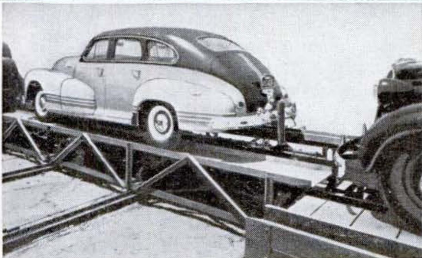
Arms automatically roll car onto the transfer table, which will carry it to empty stall.
