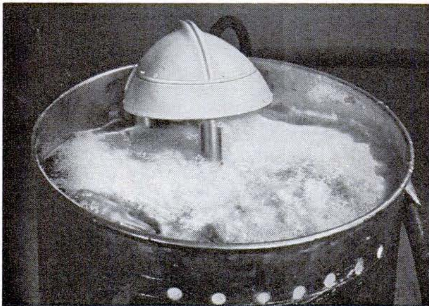
As shown above, the shaft and diaphragm extend down into the water. The picture below reveals how 240 vibrations a second whip the soapy water into spray, forcing it through the dirty clothes.
