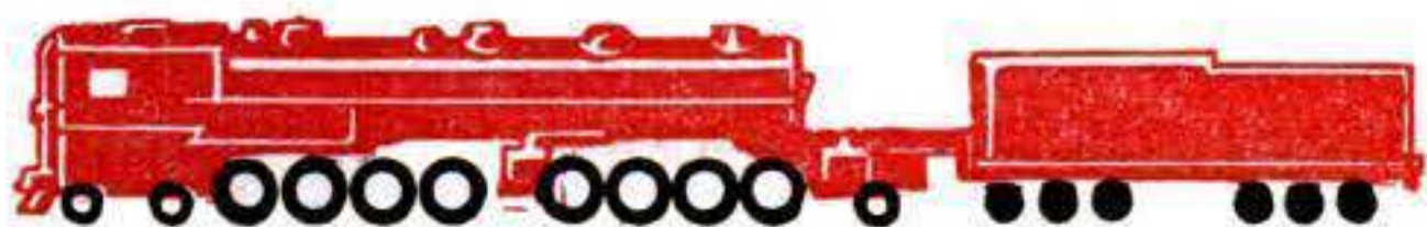
4-8-8-2 oil-burner, used only by Southern Pacific, seems to go backward. Cab is ahead of boiler.
