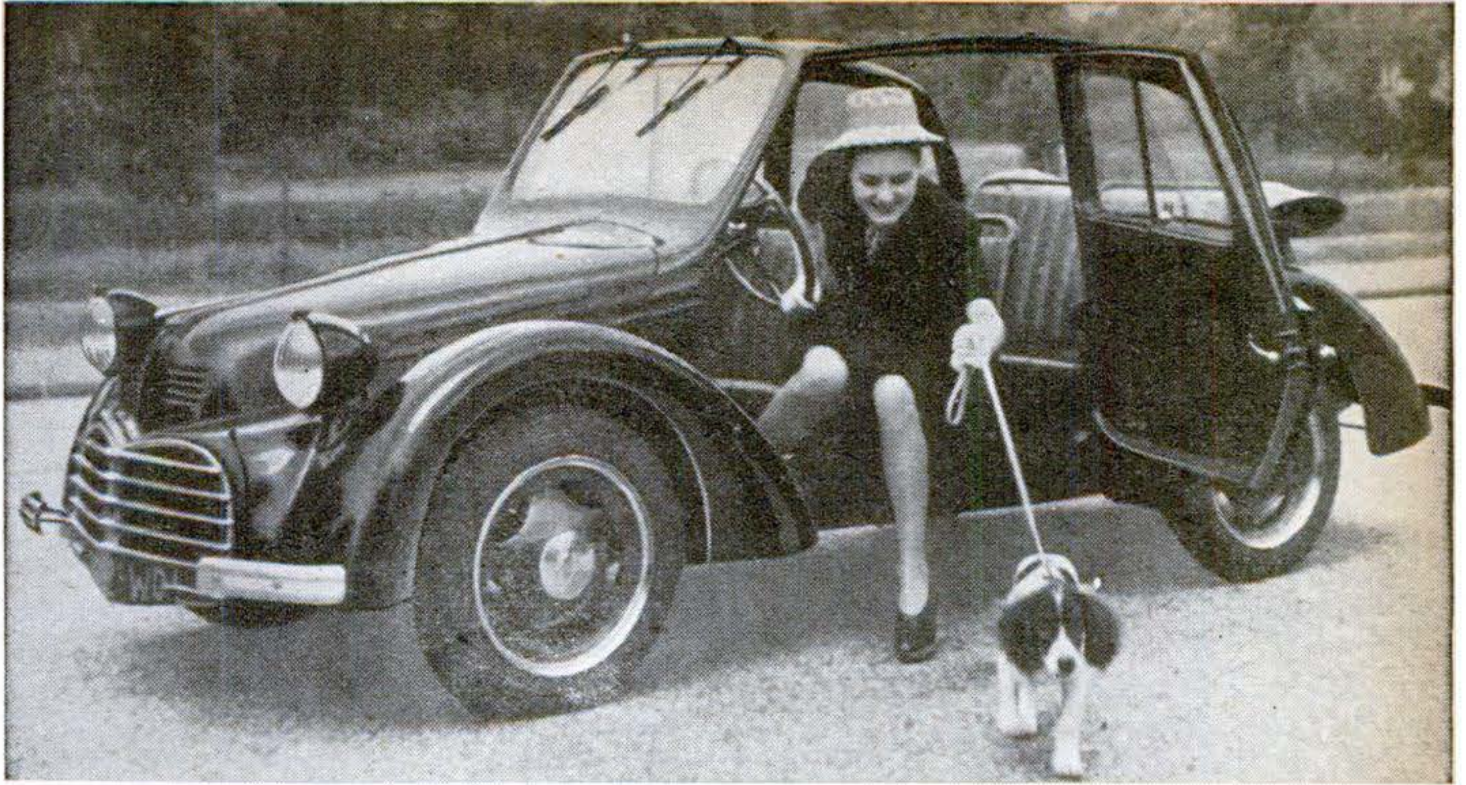
Roomy for its size, the 800-lb. French "Gregoire" is a two-door convertible sedan. Top speed is 60 m.p.h.
