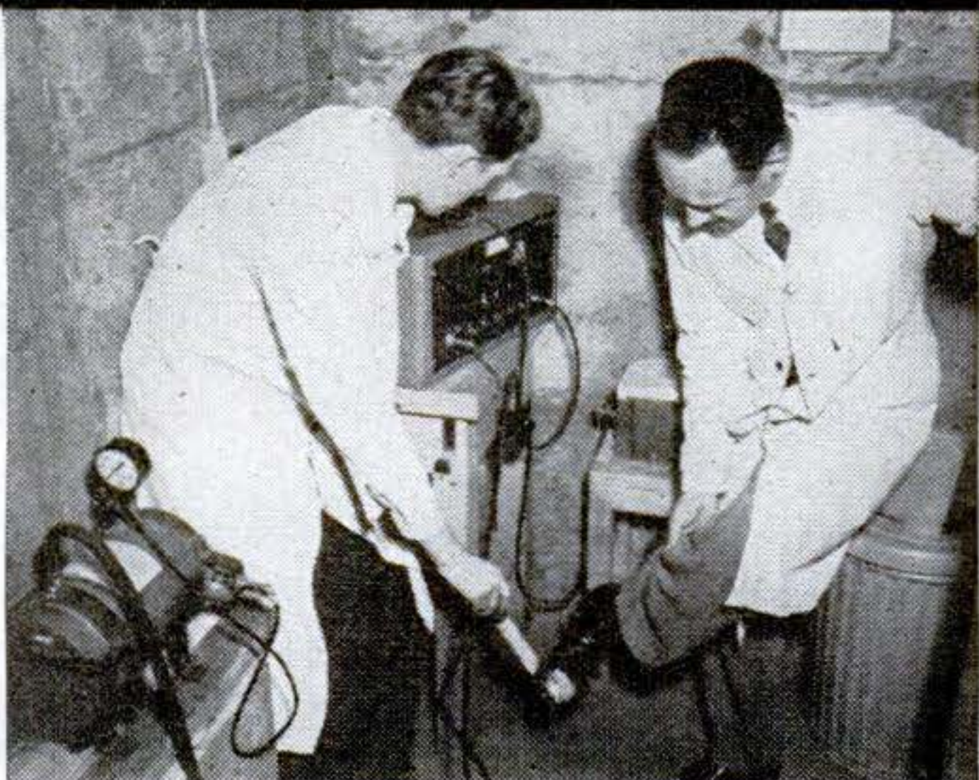
All lab workers undergo frequent checks for possible radioactive contamination. They wear washable clothing and special shoes marked by painted toes.
