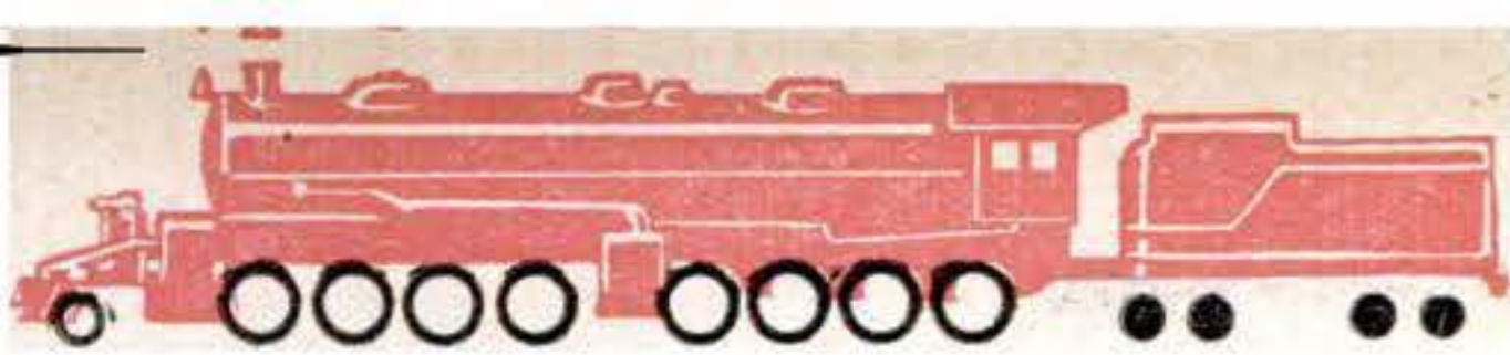
2-8-8-0 type (16 drivers), generally used to haul heavy coal and ore trains where grades are steep.
