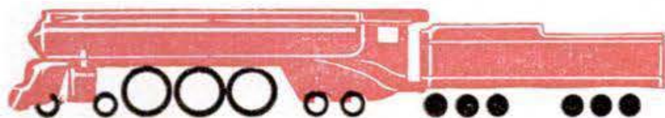
4-6-4 Hudson type, today's most popular high-speed passenger engine where hills are moderate.
