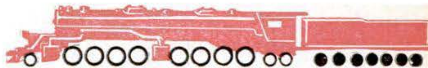
2-8-8-4 type is the "Yellowstone," so named because it was first put in use by Northern Pacific.
