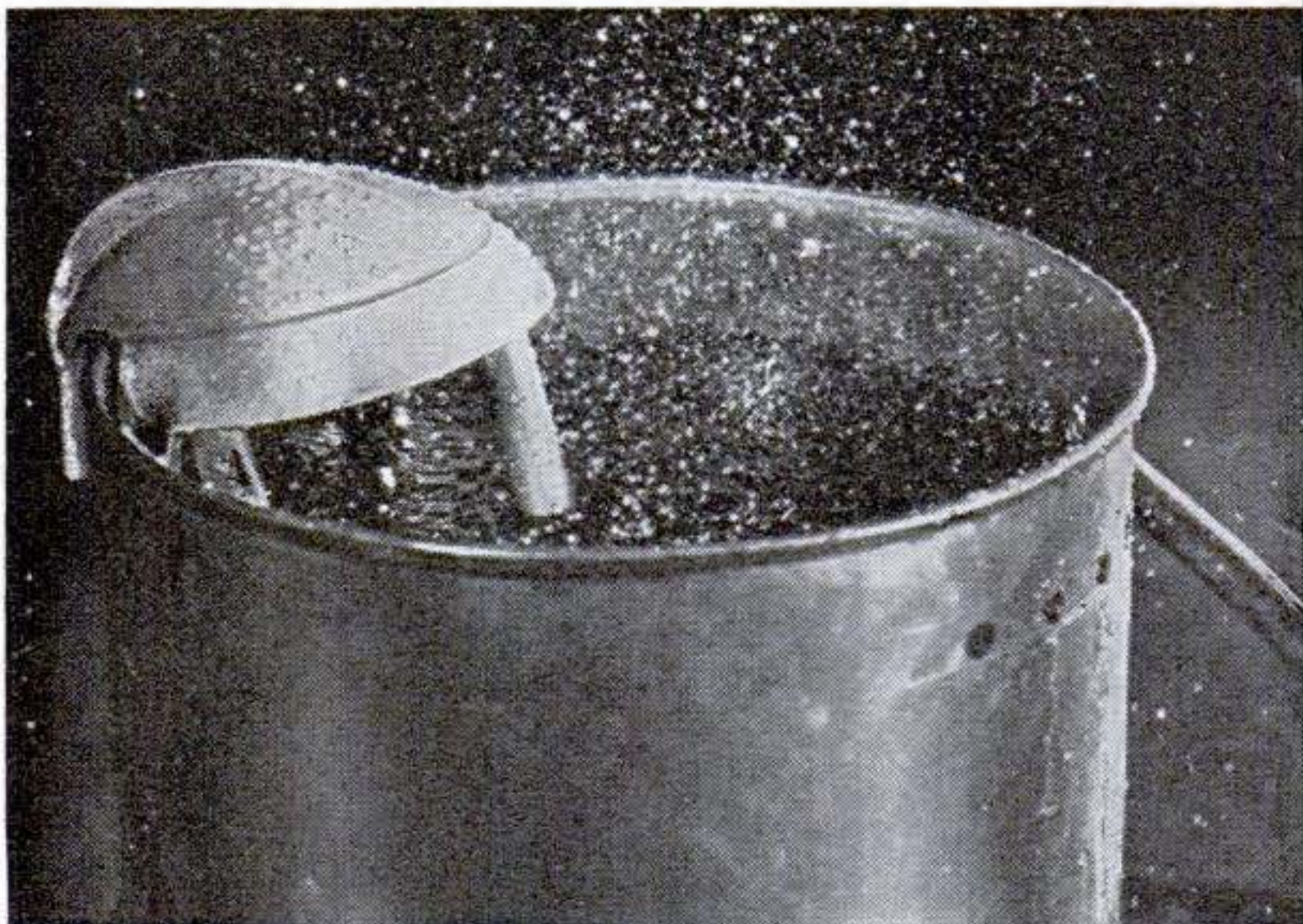
As shown above, the shaft and diaphragm extend down into the water. The picture below reveals how 240 vibrations a second whip the soapy water into spray, forcing it through the dirty clothes.
