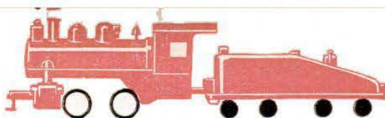
0-4-0 type switcher is used for light switching on industrial tracks where clearances are restricted.
