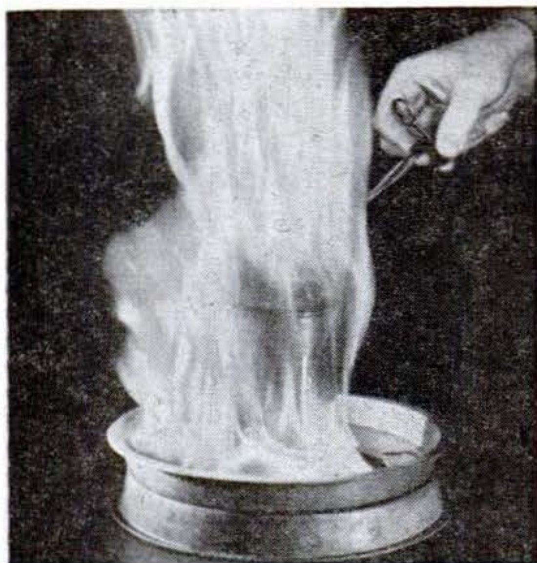
Oil and gasoline fires must be smothered by cutting off the oxygen supply. At the left above is a fire made by lighting a little gasoline floating on water. This fire is easily extinguished by covering the can with cardboard, center. Never use water, for it only spreads the flames, as demonstrated at right.
