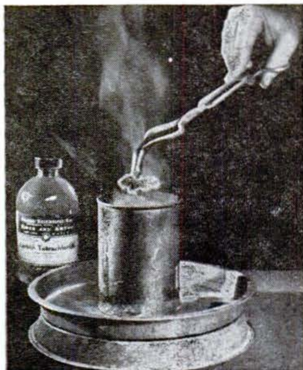
Oil and gasoline fires must be smothered by cutting off the oxygen supply. At the left above is a fire made by lighting a little gasoline floating on water. This fire is easily extinguished by covering the can with cardboard, center. Never use water, for it only spreads the flames, as demonstrated at right.
