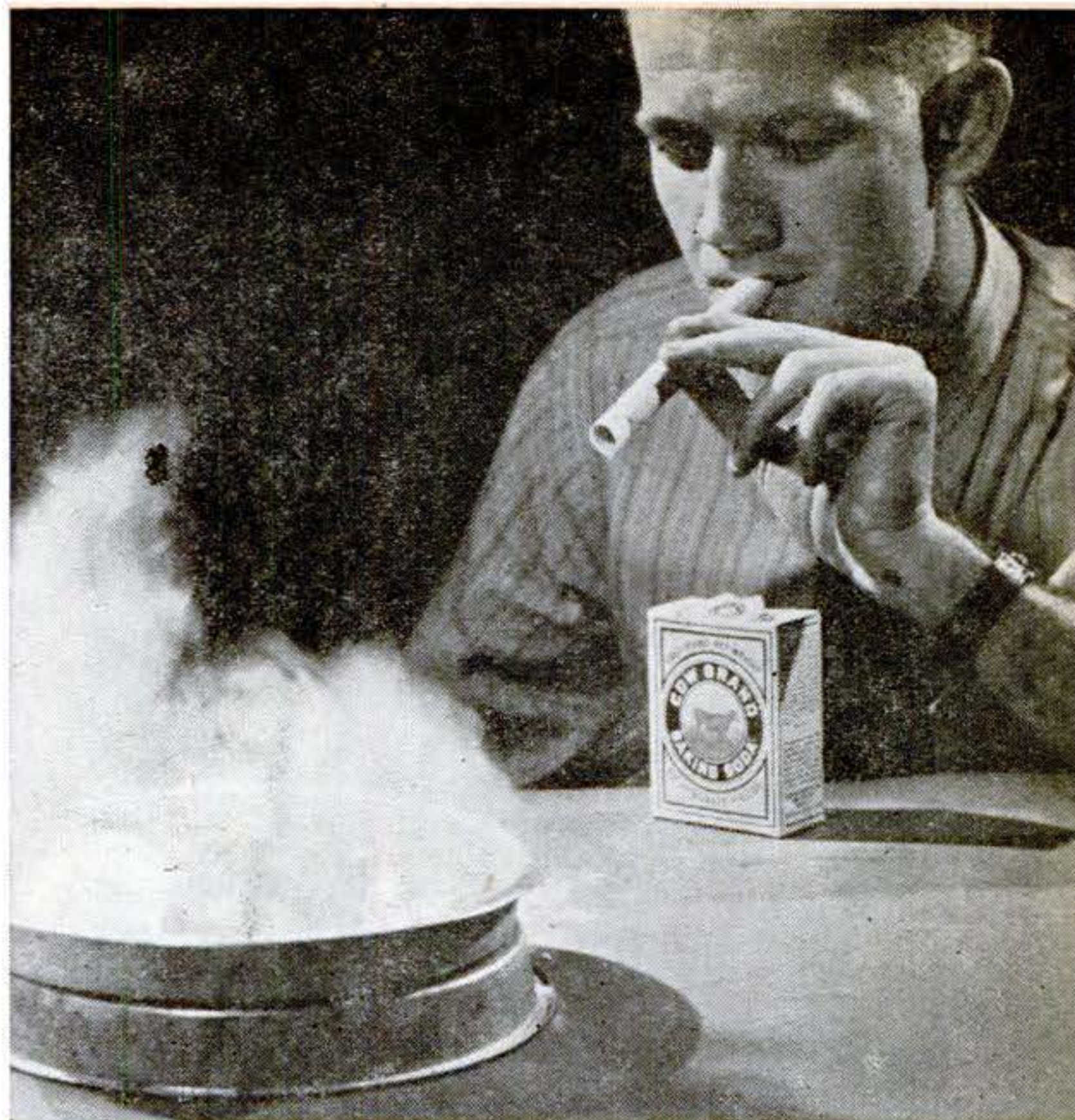
If blown as dust, bicarbonate of soda will put out a fire.
