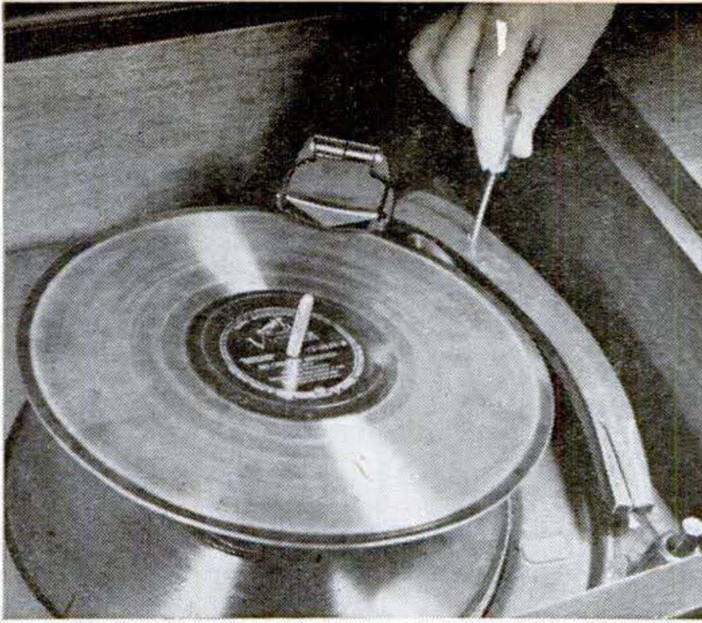
Adjusting the pickup so that the needle will engage the first groove of the record. The position of the screw varies on different models.
