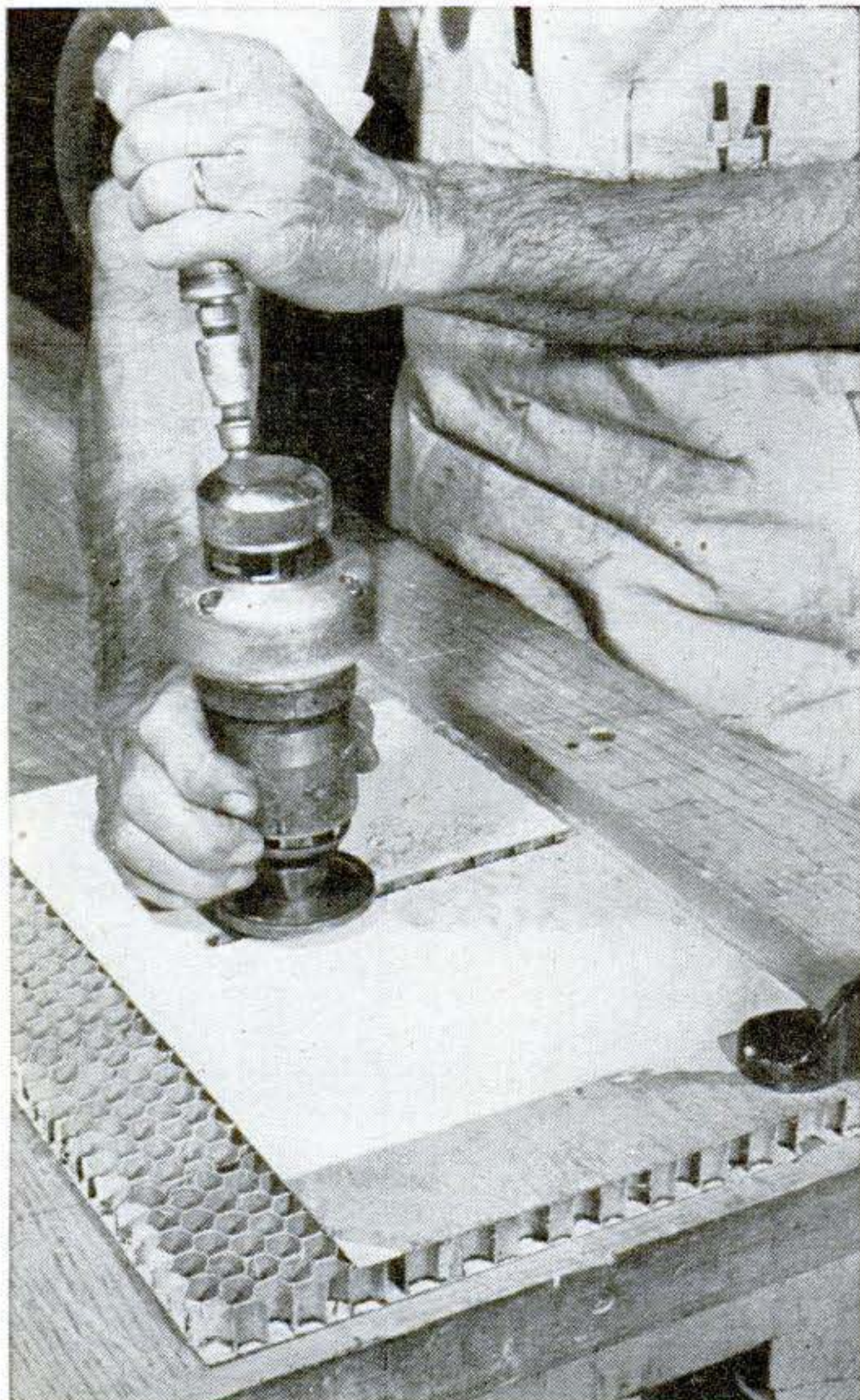
Newest lightweight plywood has mahogany surfaces and a plastic honeycomb core, called micarta. At left, a hand-guided electric router cuts channel through a panel of the material, which is used to form such models as the stairwell and bannister, below, of Lockheed's huge Constitution. The mahogany surface of the new plywood provides an extremely smooth finish that takes lacquer well.
