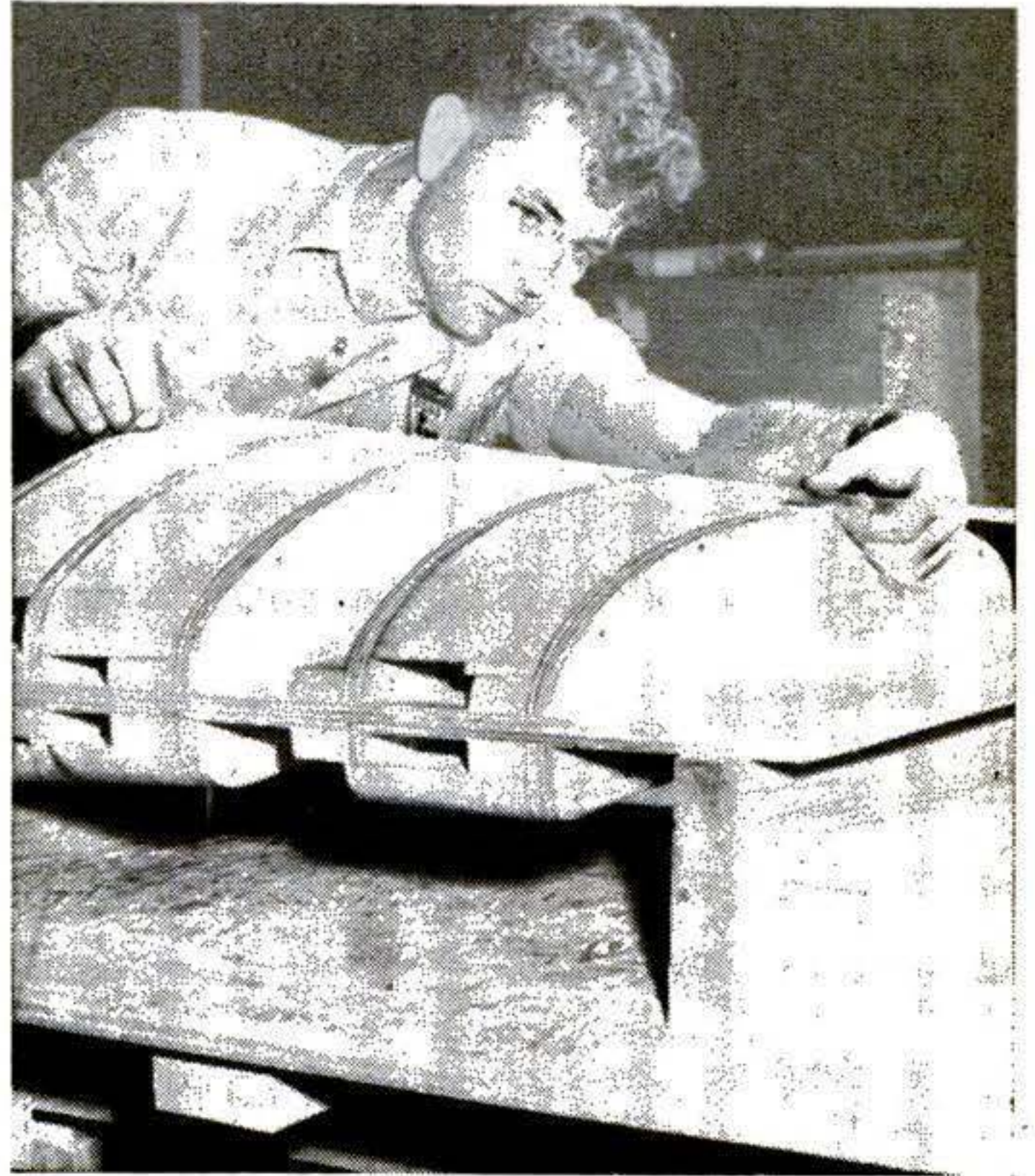
Gladwell checks a mahogany model of large air duct with metal template to insure accuracy. Mahogany holds its shape well, with little shrinkage, and is easier to work than pine despite its toughness.
