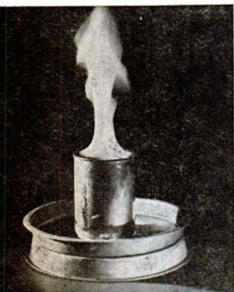
Oil and gasoline fires must be smothered by cutting off the oxygen supply. At the left above is a fire made by lighting a little gasoline floating on water. This fire is easily extinguished by covering the can with cardboard, center. Never use water, for it only spreads the flames, as demonstrated at right.
