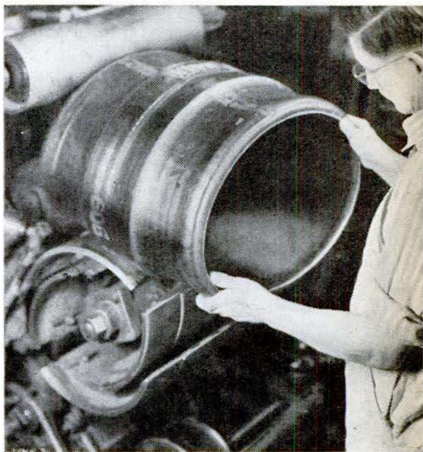
6. Looking like a barrel with both ends removed, tire is taken off the collapsed drum. Operator gives it a quick check before placing it on conveyor to go to inspection station. (Goodyear photos.)
