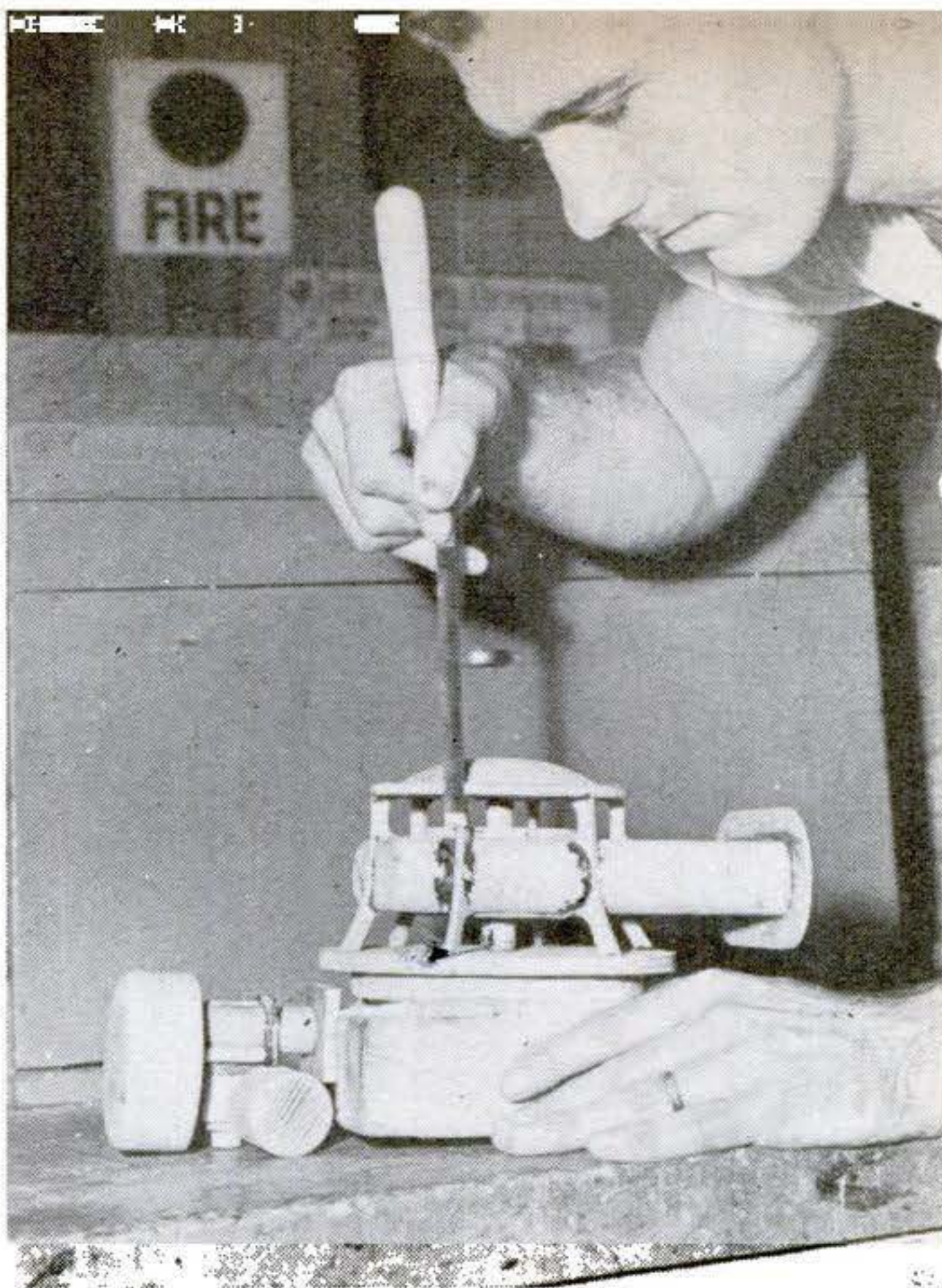
Using a 1/2-inch bent-shank carving chisel, Northrop's Stanley Ton smooths plywood bracket on a reproduction of oxygen pressure regulator. Other parts of the complex assembly are made of white pine.
