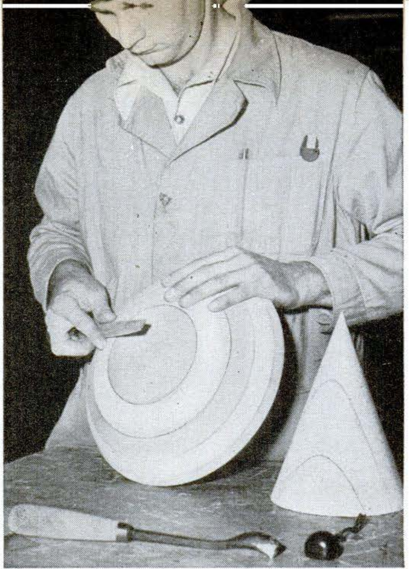
Art Russo, of Northrop, wields a fine-toothed rasp to smooth white-pine tail section of a droppable gas tank. The maple cone at right is a copy of the nose of an air-duct diffuser.
