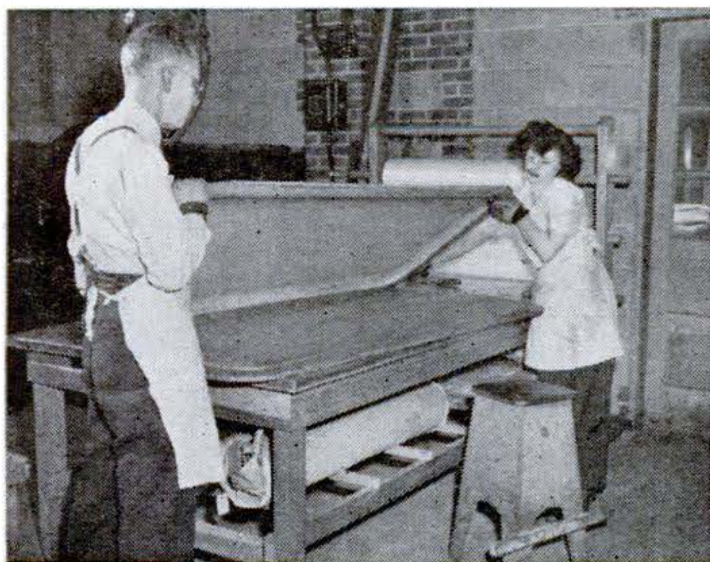
4. After curing, the glass-cloth mold is removed from the autoclave, taken off its wooden form, and finished with a coat of thermosetting varnish.
