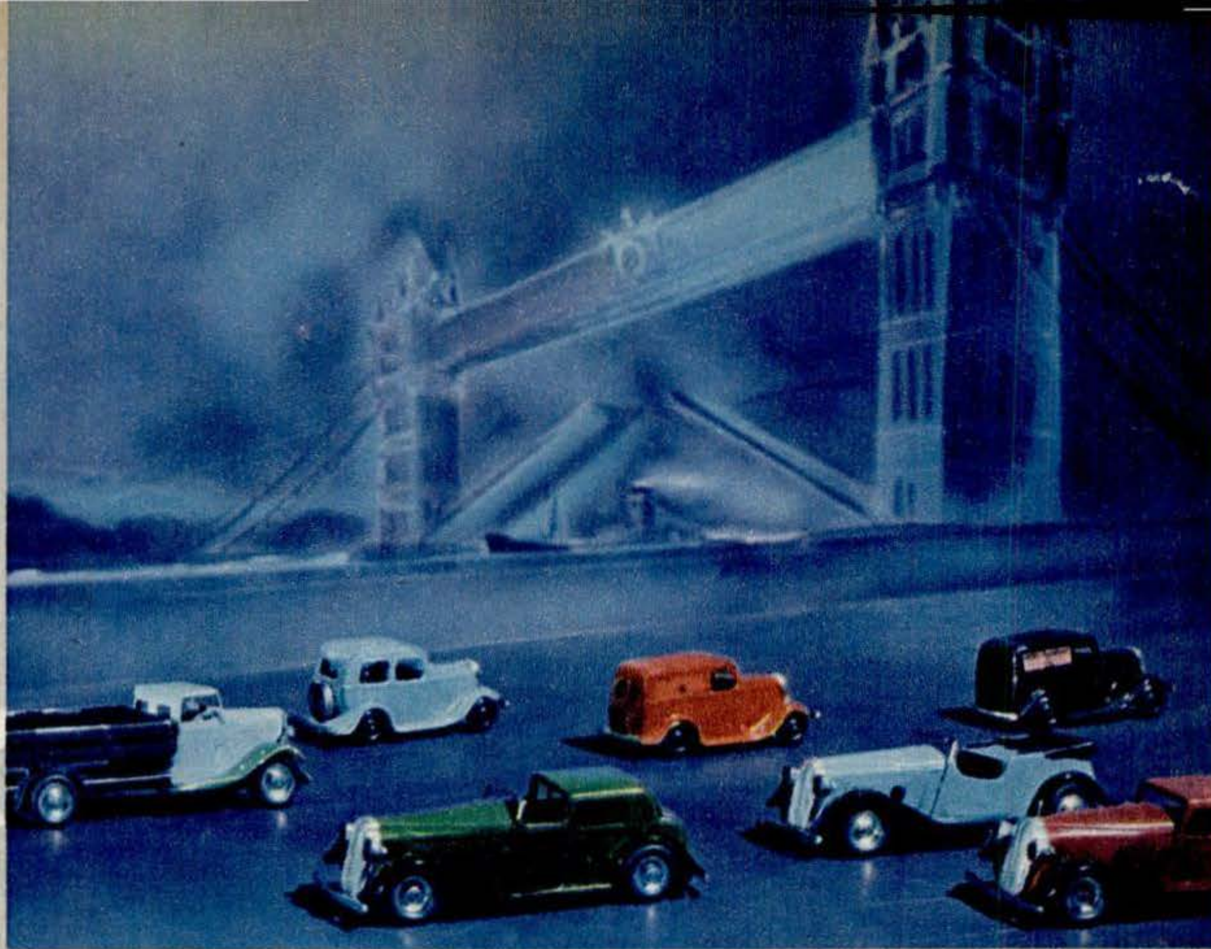
Below: The scale-model American Flyer cars are plastic and weigh only one-third as much as metal cars, permitting longer, more realistic trains.
