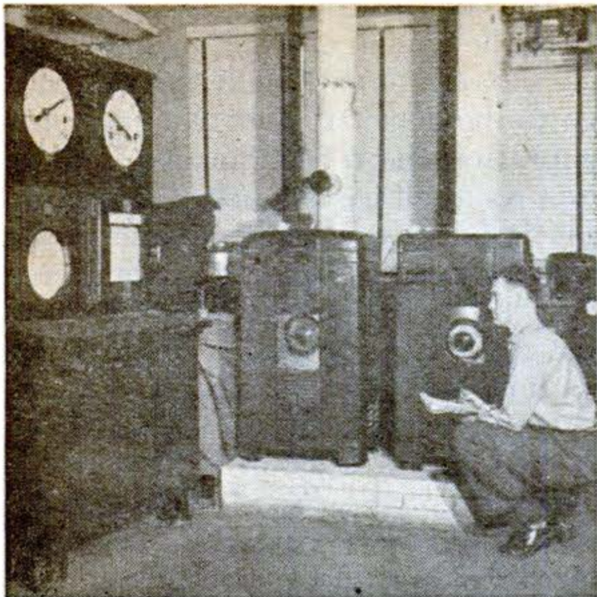
Ordinarily, pot burners require high grade oil because heat from the flame cracks a cheaper grade while it is vaporizing. Socony-Vacuum engineers now have developed a pot-type heater which prevents cracking, making it possible to use the more economical fuel. It is shown above under test and in a cutaway view.
