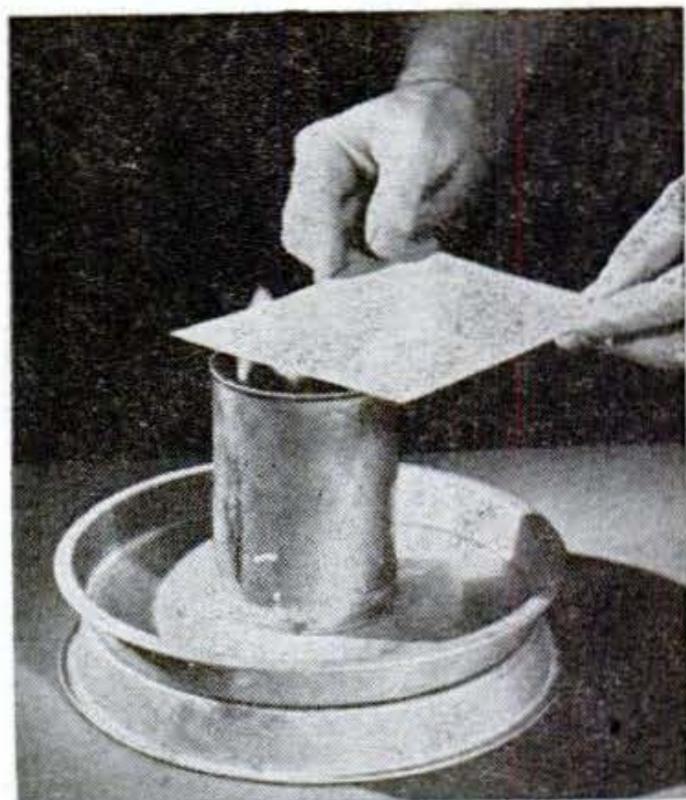
Oil and gasoline fires must be smothered by cutting off the oxygen supply. At the left above is a fire made by lighting a little gasoline floating on water. This fire is easily extinguished by covering the can with cardboard, center. Never use water, for it only spreads the flames, as demonstrated at right.
