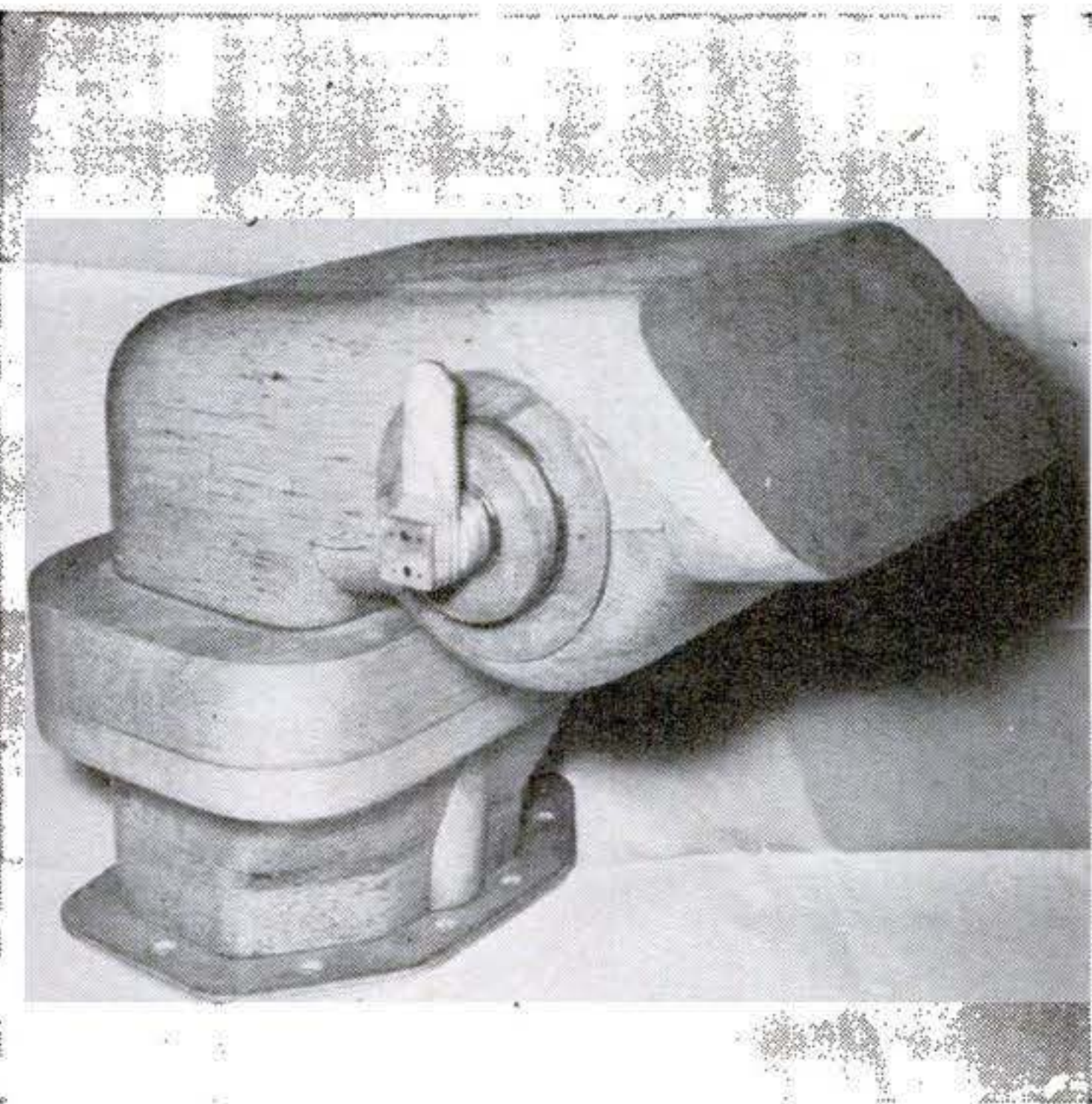
A dozen pieces of sugar pine were put together with waterproof glue to form this model of the Lockheed Saturn's carburetor intake valve. Engineers use the model in making clearance studies of accessories.
