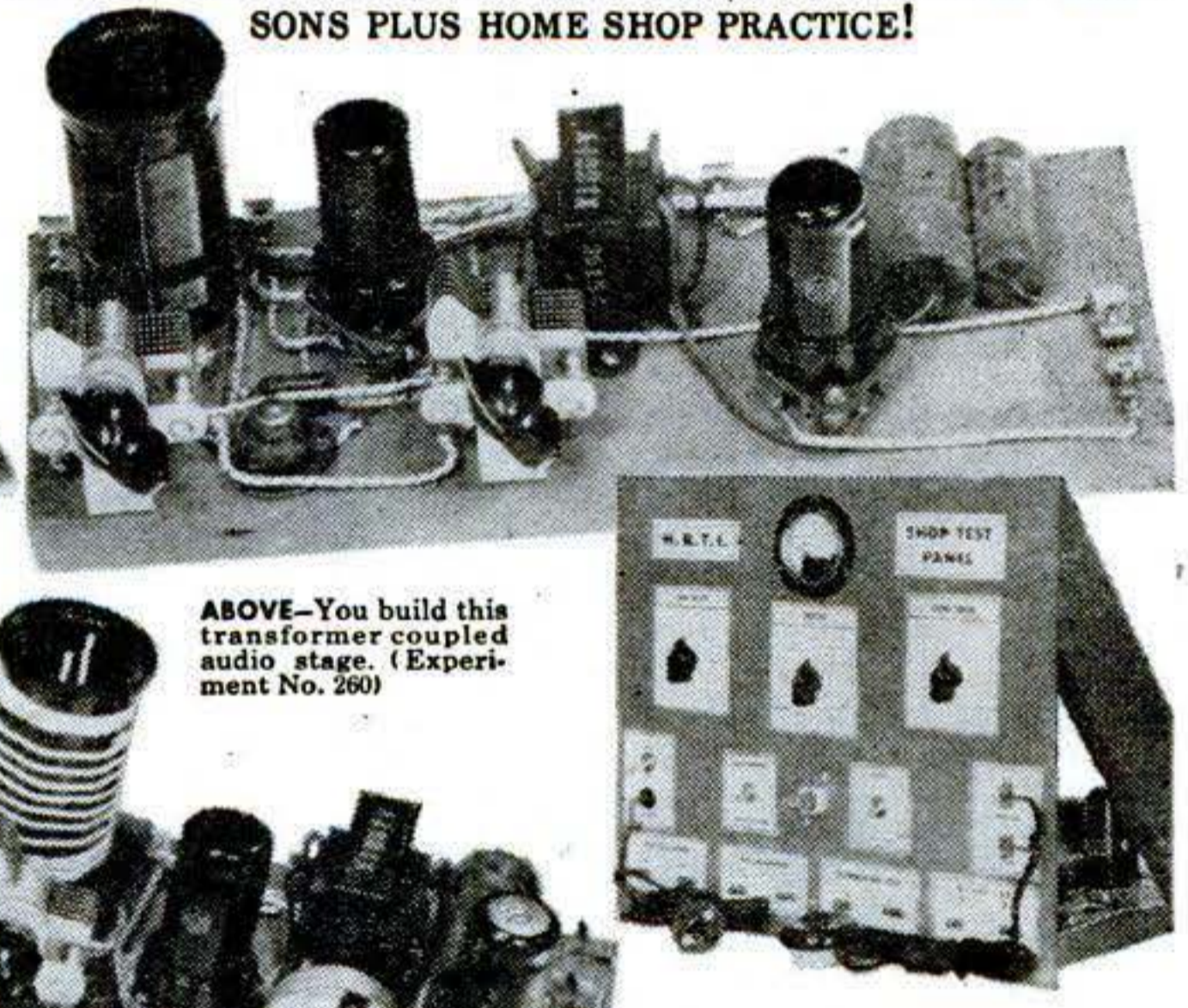
ABOVE- You build this Multi-purpose Shop Test Panel. 5 Test instruments in one. LEFT- You build this tuned radio stage, regenerative detector and audio amplifier. (Experiment No. 329)
