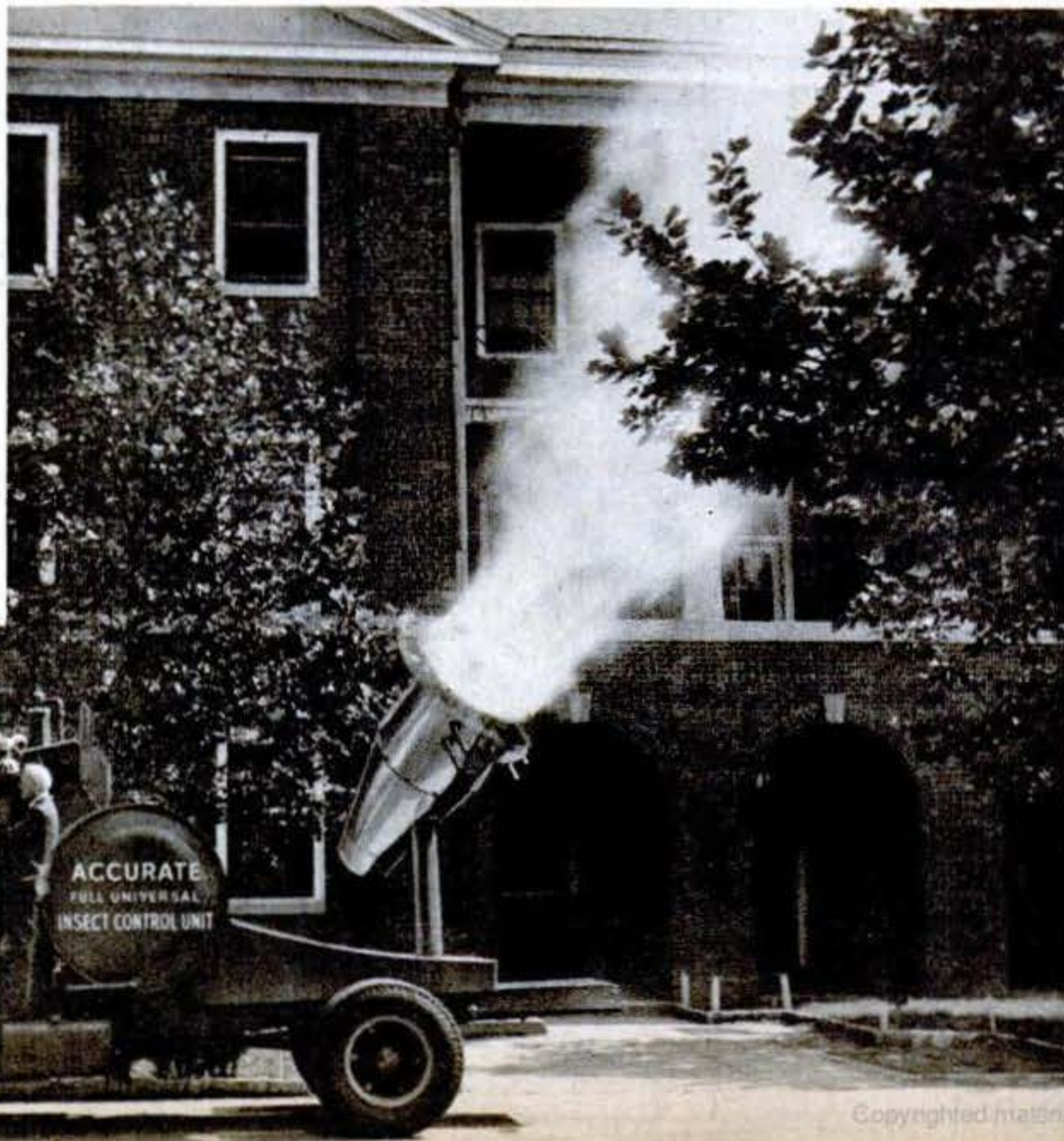
Motorized Spray Gun. For insect control in large areas, the truck shown below carries a swivel-mounted aircraft engine and propeller. Insecticide fed into the propeller's blast is spread hundreds of feet in any direction.
