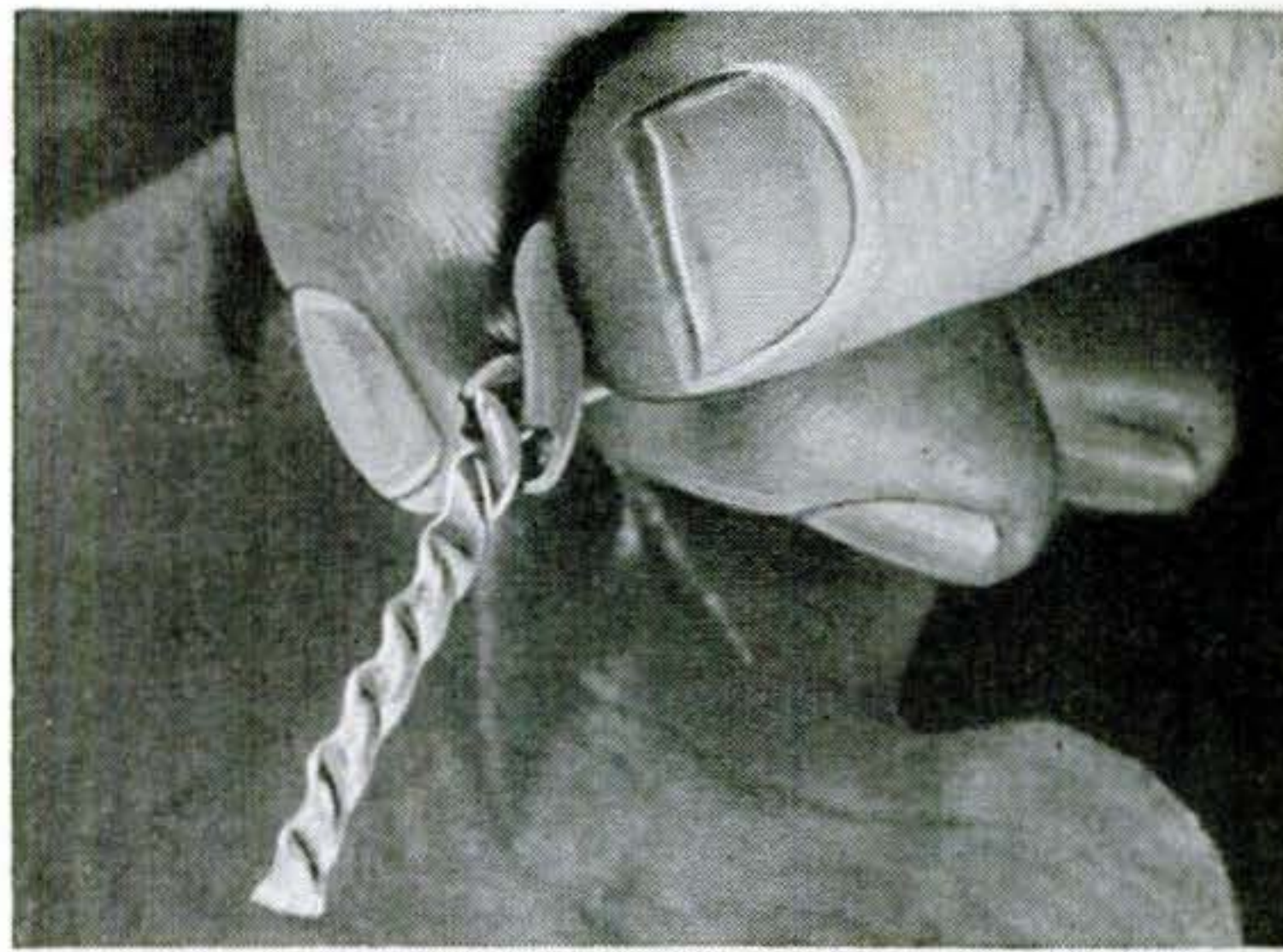
The surplus of melted solder is wiped off, and the soldered connection is left clean.
