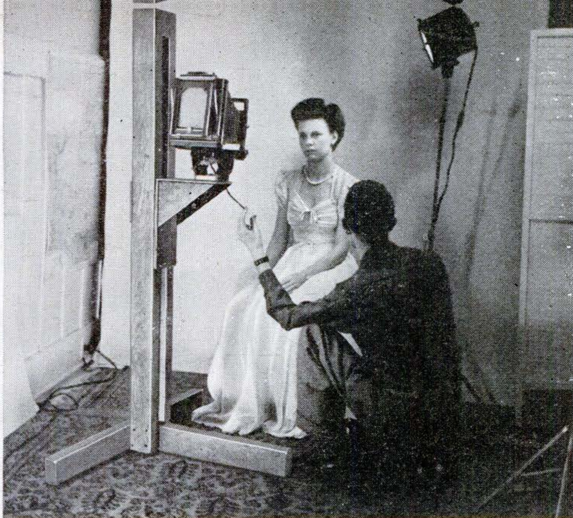
Despite its cumbersome appearance, this studio stand is readily maneuverable. One wing nut loosens the camera shelf for quick adjustment to any level. The base slides on dome gliders.
