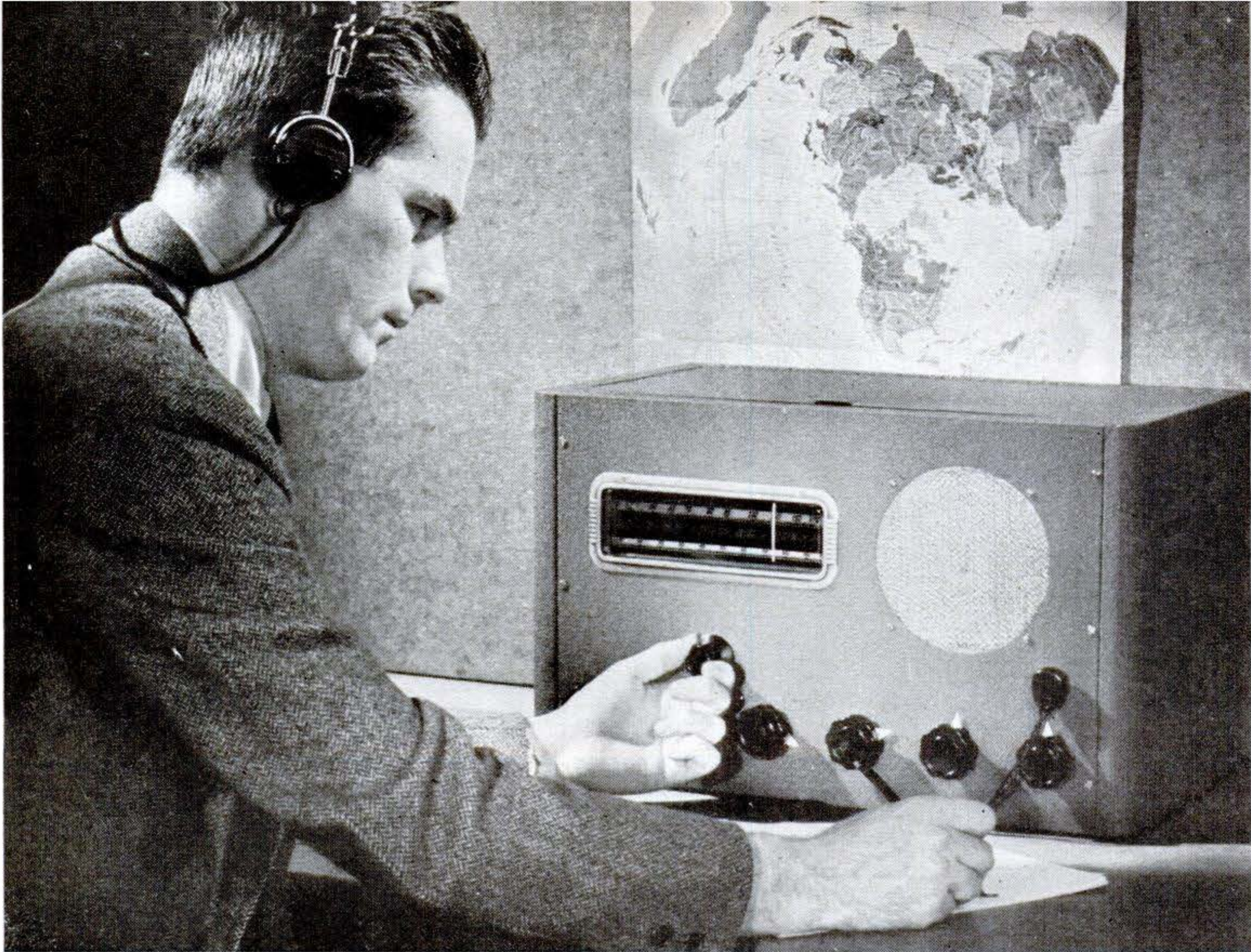
Elusive short-wave signals often come in best at night, so headphones are built into this two-band superheterodyne for midnight DX listening. Flicking a couple of switches, however, brings in the full broadcast band at loudspeaker volume.
