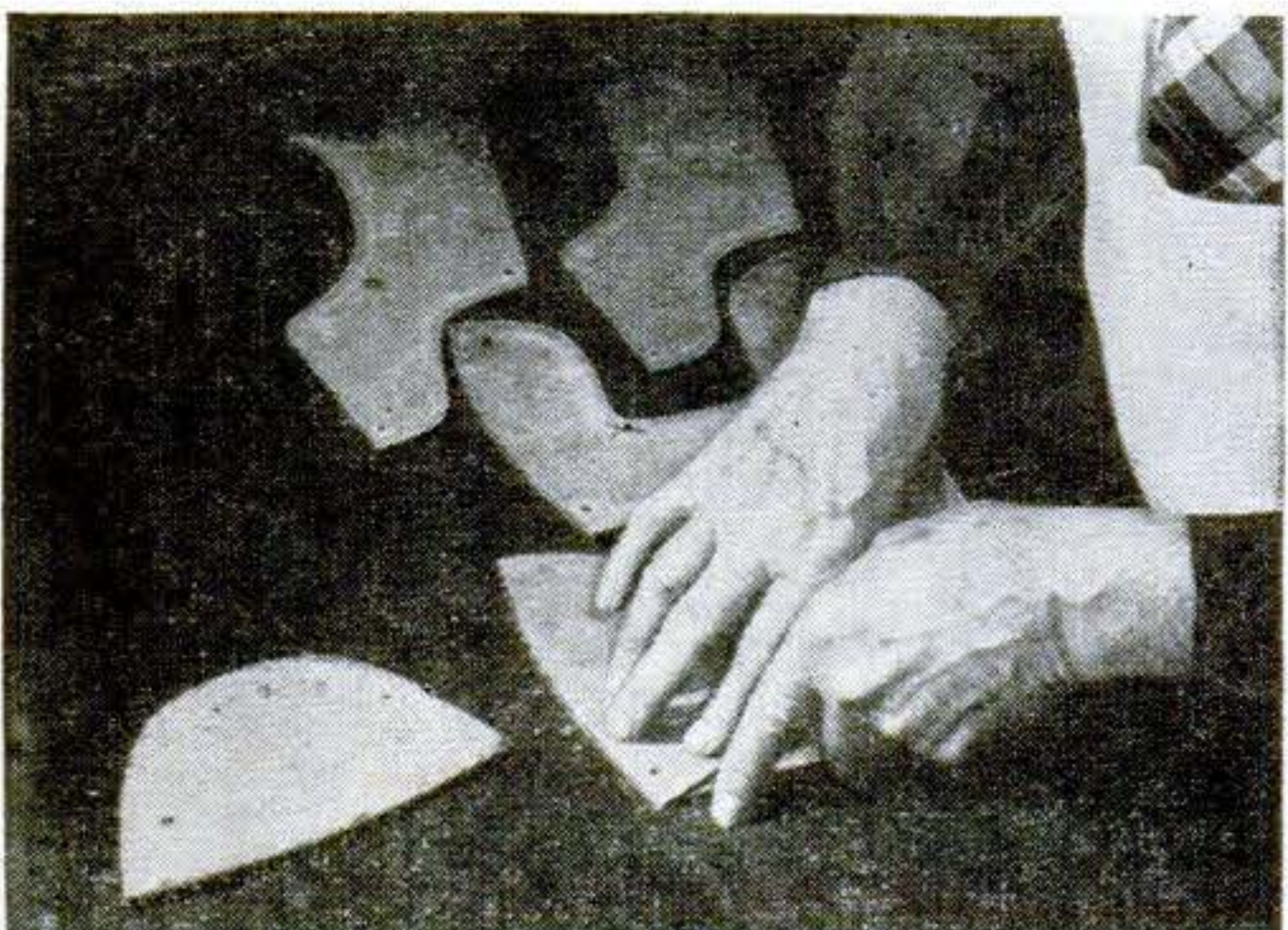
3. Meanwhile, the vamp, tip and two side pieces, forming the upper body of the shoe, are cut out by hand along brass-rimmed patterns, making possible a more careful selection of cuts and matching of parts.
