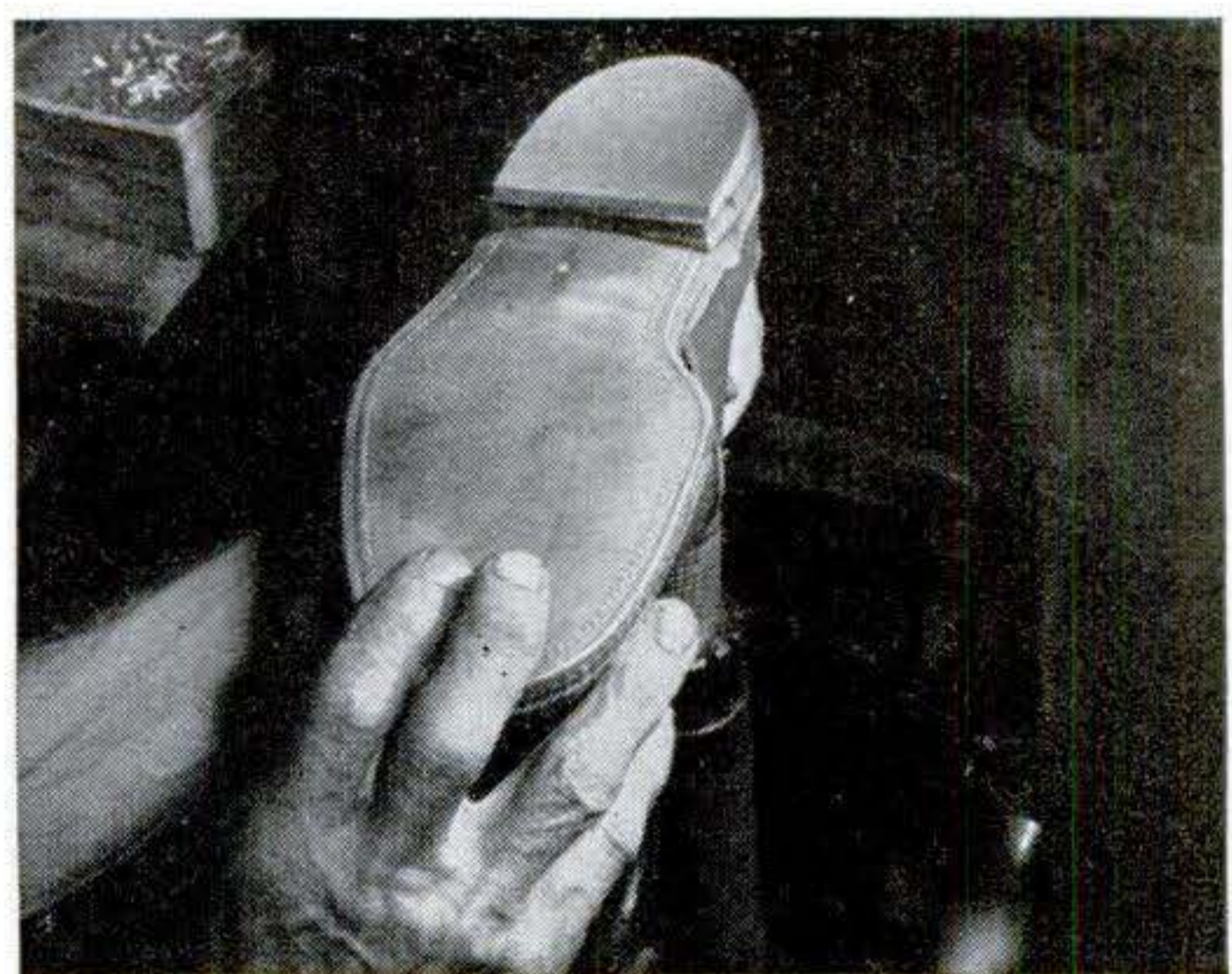
12. On the heeling machine, final step in the process, an automatic nailing mechanism fastens on the heel. Waxed, washed, and polished, the finished shoes, with laces added, are now ready for boxing.
