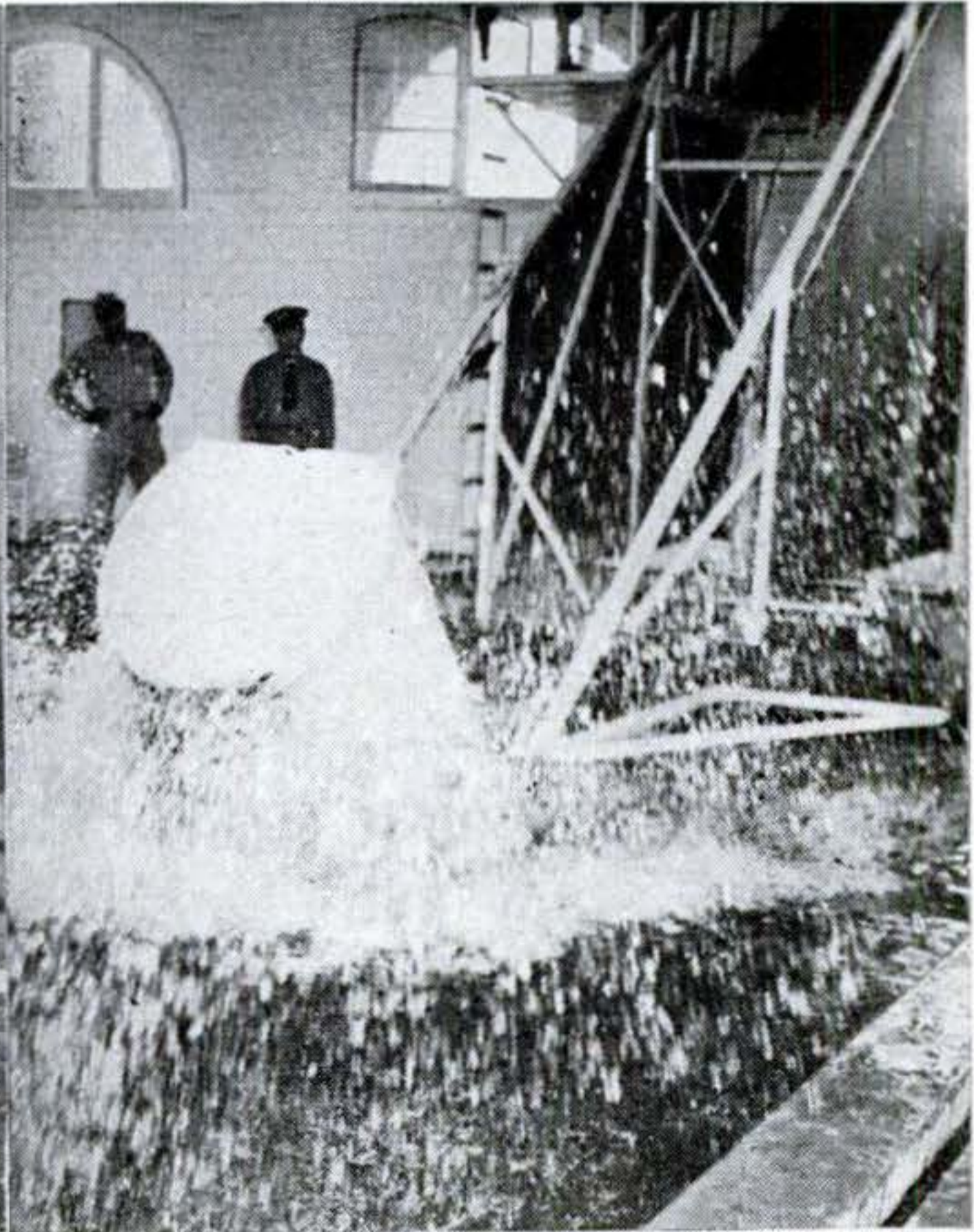
pilot and gunner, about to hit the skids. At right the "Dilbert Dunker" crashes into the water. The men must now get out of their safety harness and free their emergency equipment—all in a few seconds while the cockpit is still in motion.
