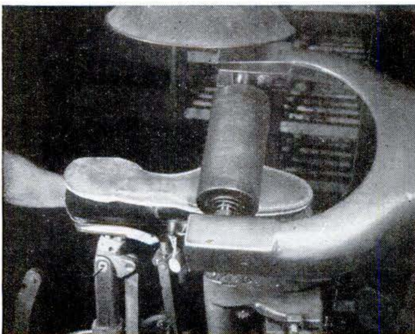
11. A leveling machine, exerting 450 pounds of pressure, smooths the sole into position and insures a proper fit on the bottom of the shoe. It takes a month to six weeks to complete a pair of shoes.
