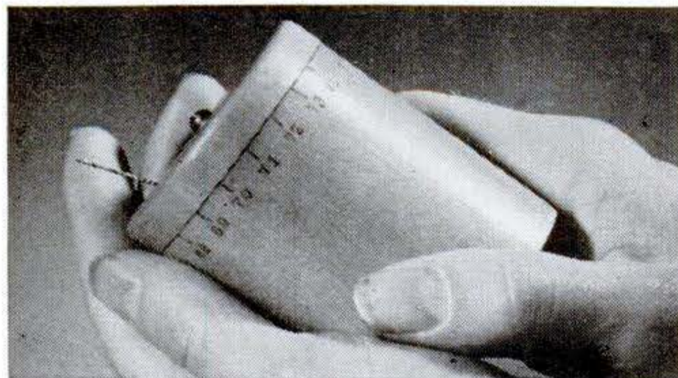
The 3/16" holes let you store several drills of each size in this container. To get a particular drill, turn the cover hole to the size you want.
