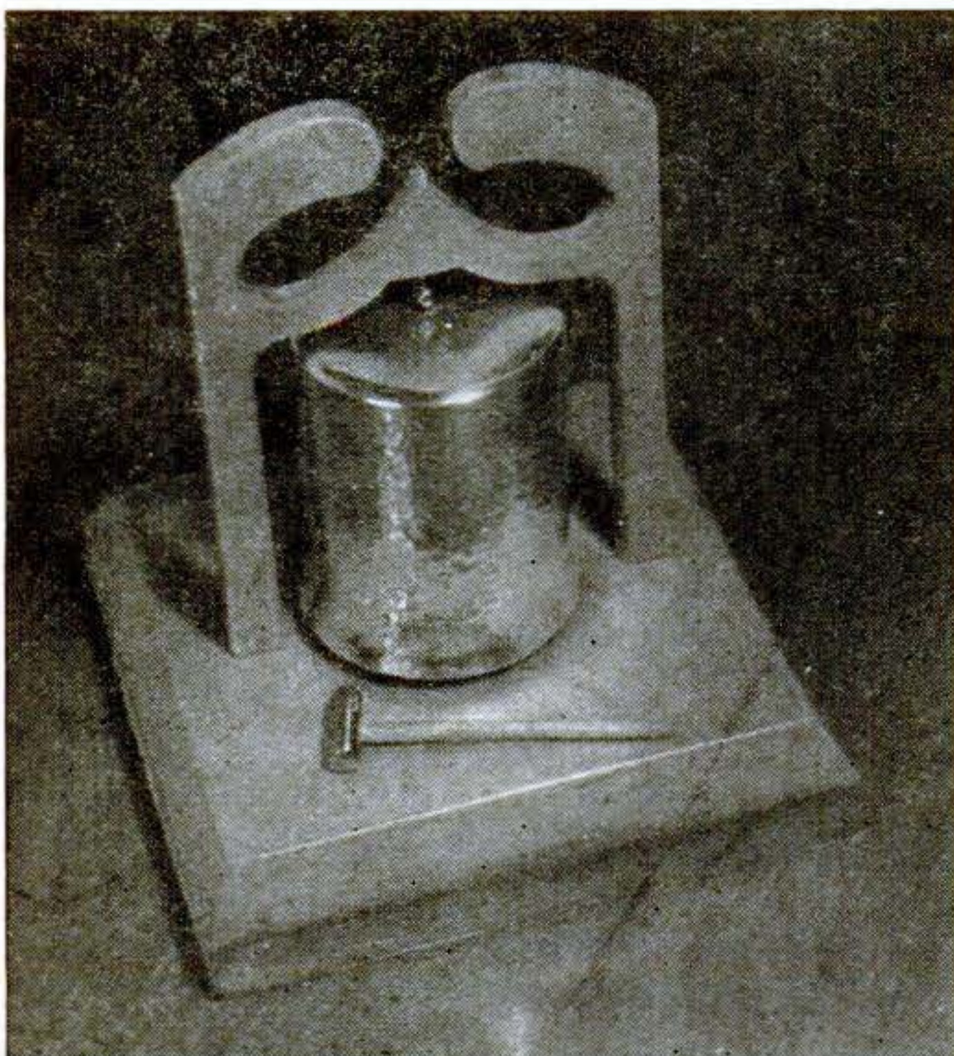
Flanging is done with the edge of a mallet while the tubing is revolved on a round bar. The hammer head and handle shown were turned on a lathe.
