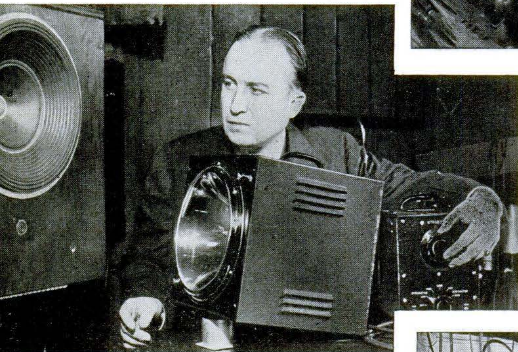
ACOUSTICS ENGINEERS tackle the problems that arise in radio design and development. At left, an RCA expert uses a stop-motion stroboscope to check on the performance of a loudspeaker.
