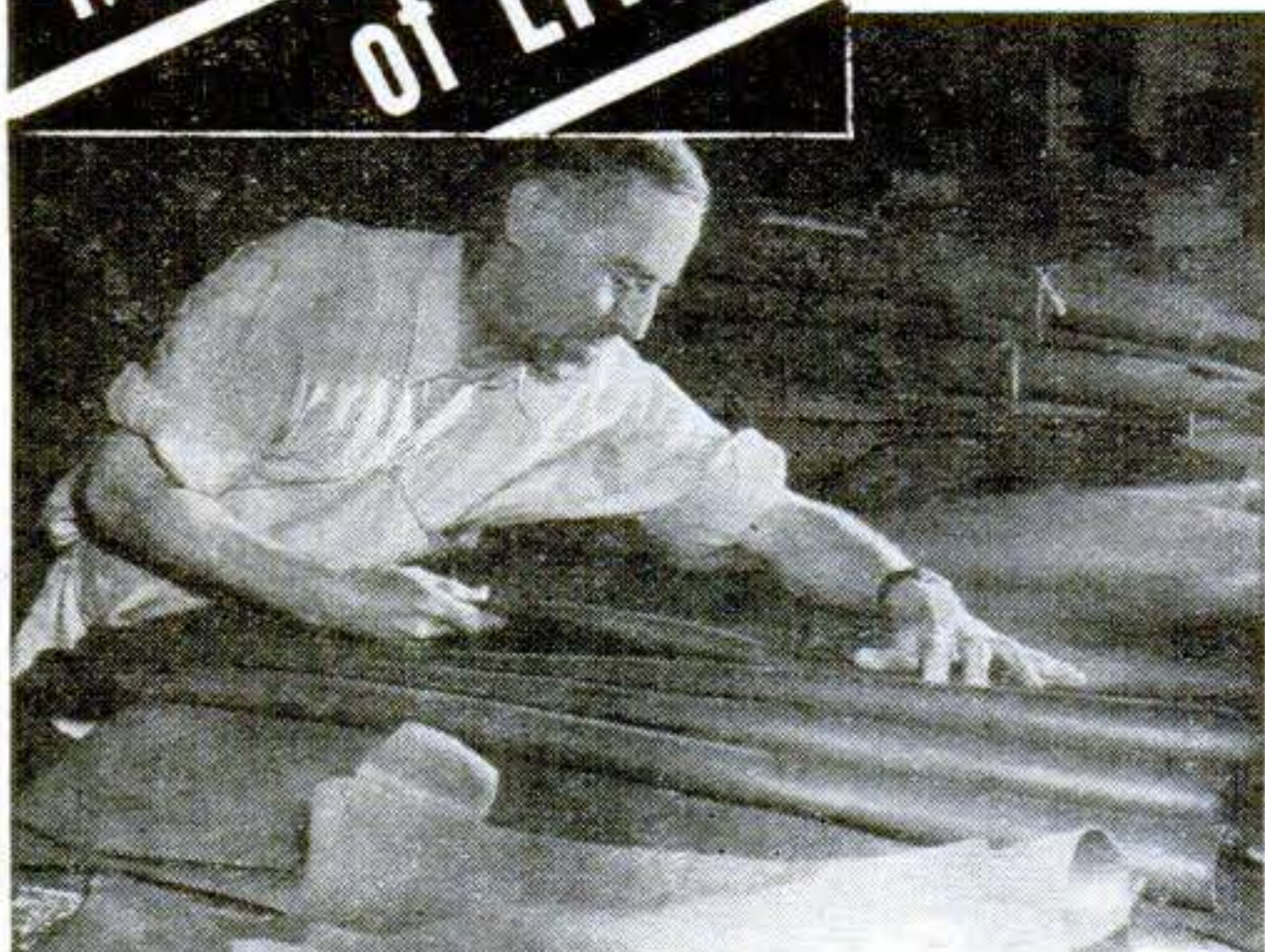
1. First step in the manufacture of shoes is the testing, sorting and selection of skins arriving from the tannery. (These pictures were taken at the Johnston and Murphy shoe factory in Newark, N. J.)
