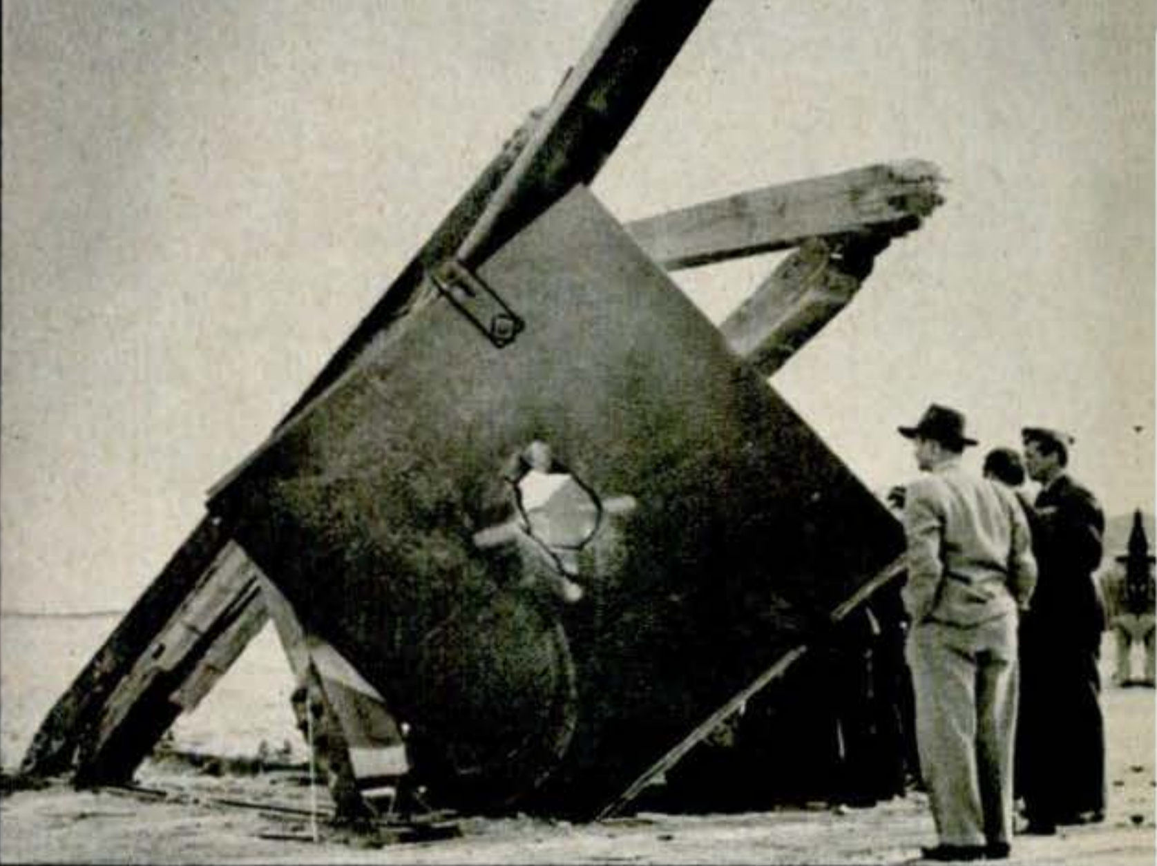
4. The four top photographs, taken at intervals of about 2/1,000 second, show the rocket approaching the target, penetrating it, passing beyond it (with war head broken off and dangling vertically from rocket's body), and exploding. The bottom picture shows what the impact of such a projectile, traveling 1,500 feet a second, can do to the target even without an explosion. The target, pierced and virtually demolished, is 2\frac{1}{2} -inch steel armor plate.
