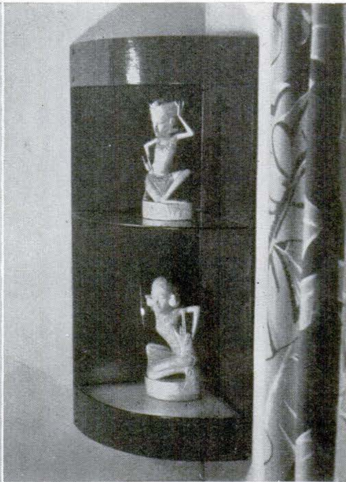
Light from the base of the cabinet illuminates the objects displayed on its glass shelves, while that from the top provides a soft glow for the room.
