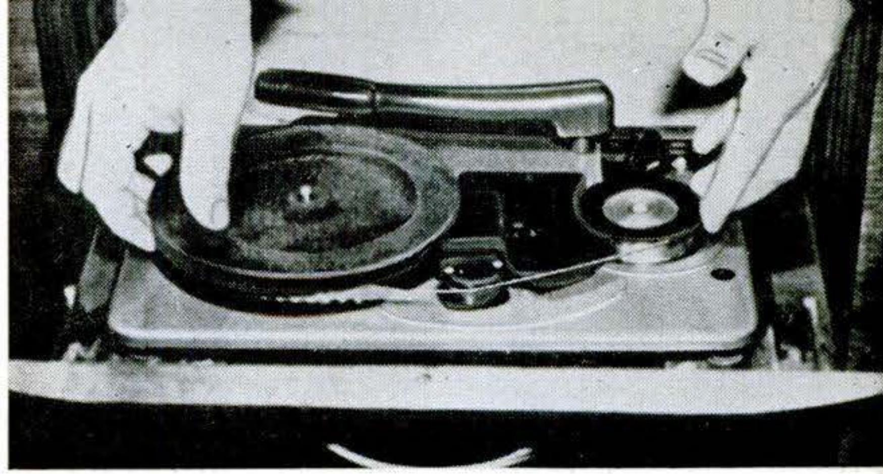
First wire recorder to reach the home market, the St. George unit has a combined erase-record-playback head; uses the windup reel as a turntable.
