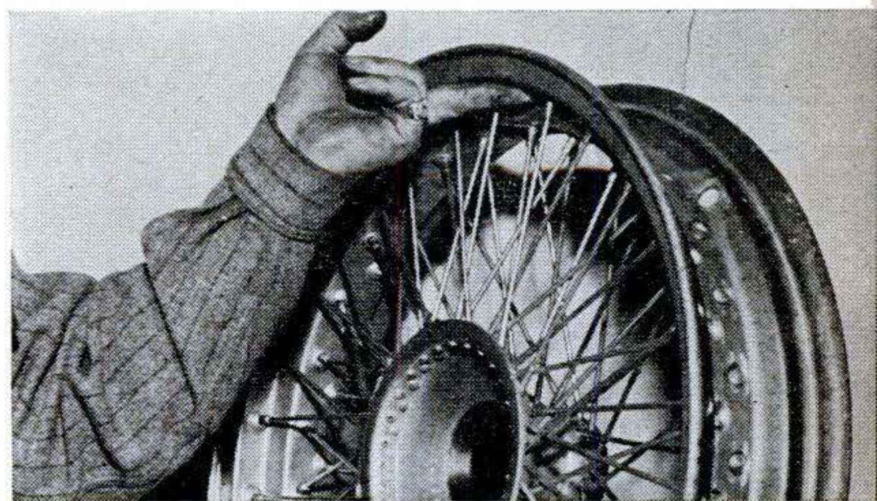
Duraluminum wheels weigh only 16 to 18 pounds without tires, about half as much as steel wheels. The 5\frac{1}{2} -inch-wide rim would support a 4,000-lb. car.
