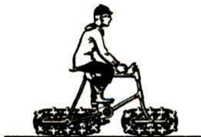
A crawl tread installed on his son's bicycle tested the traction wheel patented by Henry Stith in 1880.
