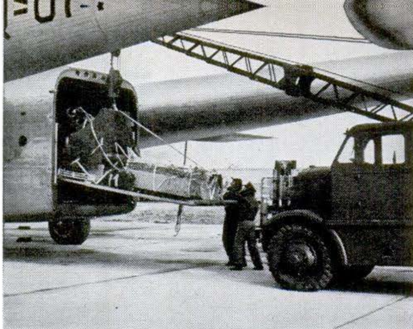
The 2,240-lb. howitzer is loaded into the rear door of a C-82 Fairchild cargo plane. Packed on skids beforehand, it can be put aboard in 15 minutes.
