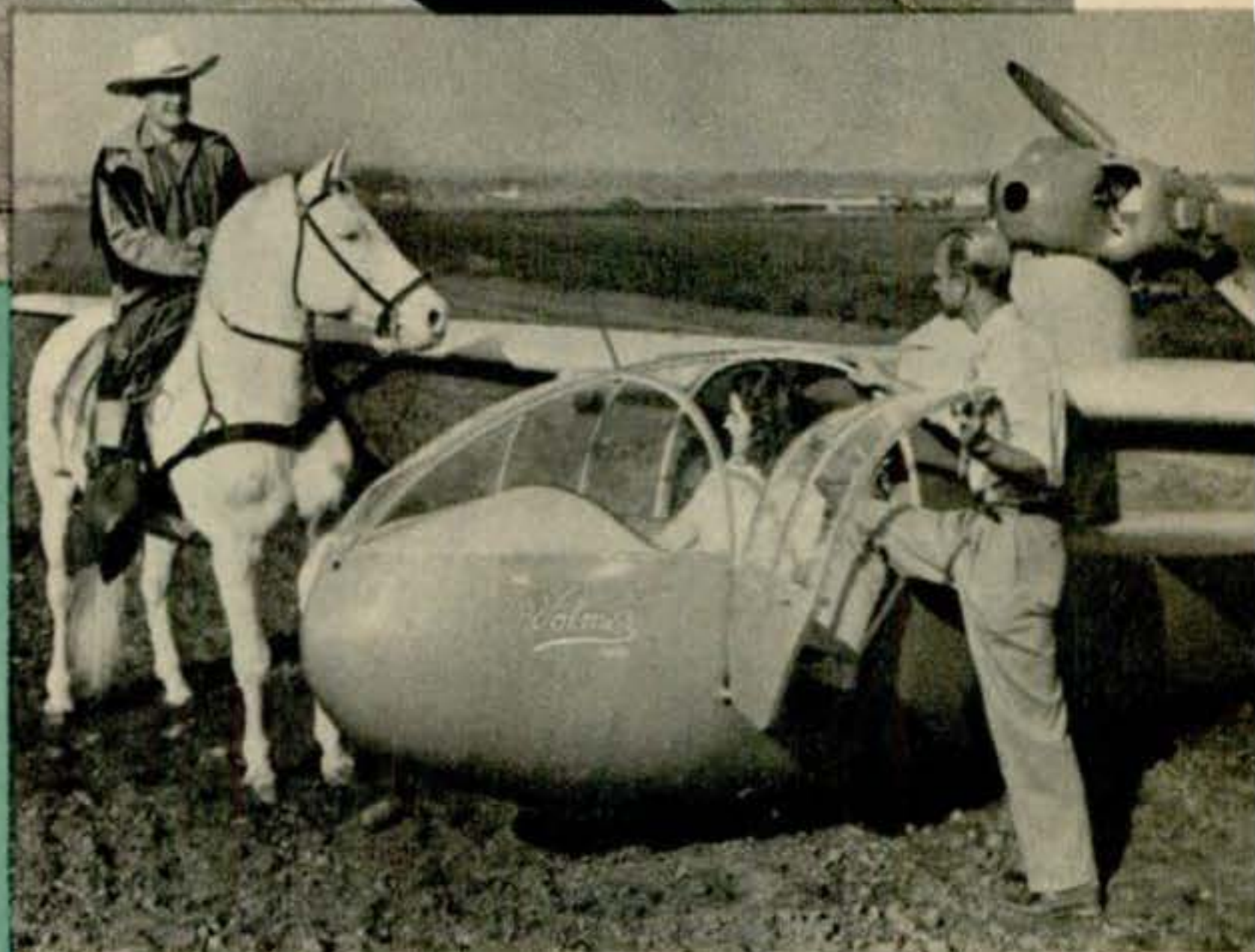
VJ-21 MAKES ITS BOW. With a 75-hp. engine atop its wing, the Volmer Aircraft Company's new three-place personal plane has a cruising speed of 110 m.p.h. and a 500-mile range. Prototype has a single main wheel and small retractable wing wheels (one of which is visible in top photo), but production models will have fixed tricycle gear. Lower photo shows the designer, Volmer Jensen, entering cockpit of the 1,350-pound craft.
