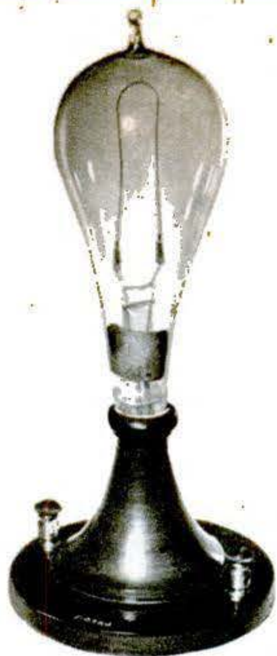
Edison bamboo-filament lamp: 1880.
