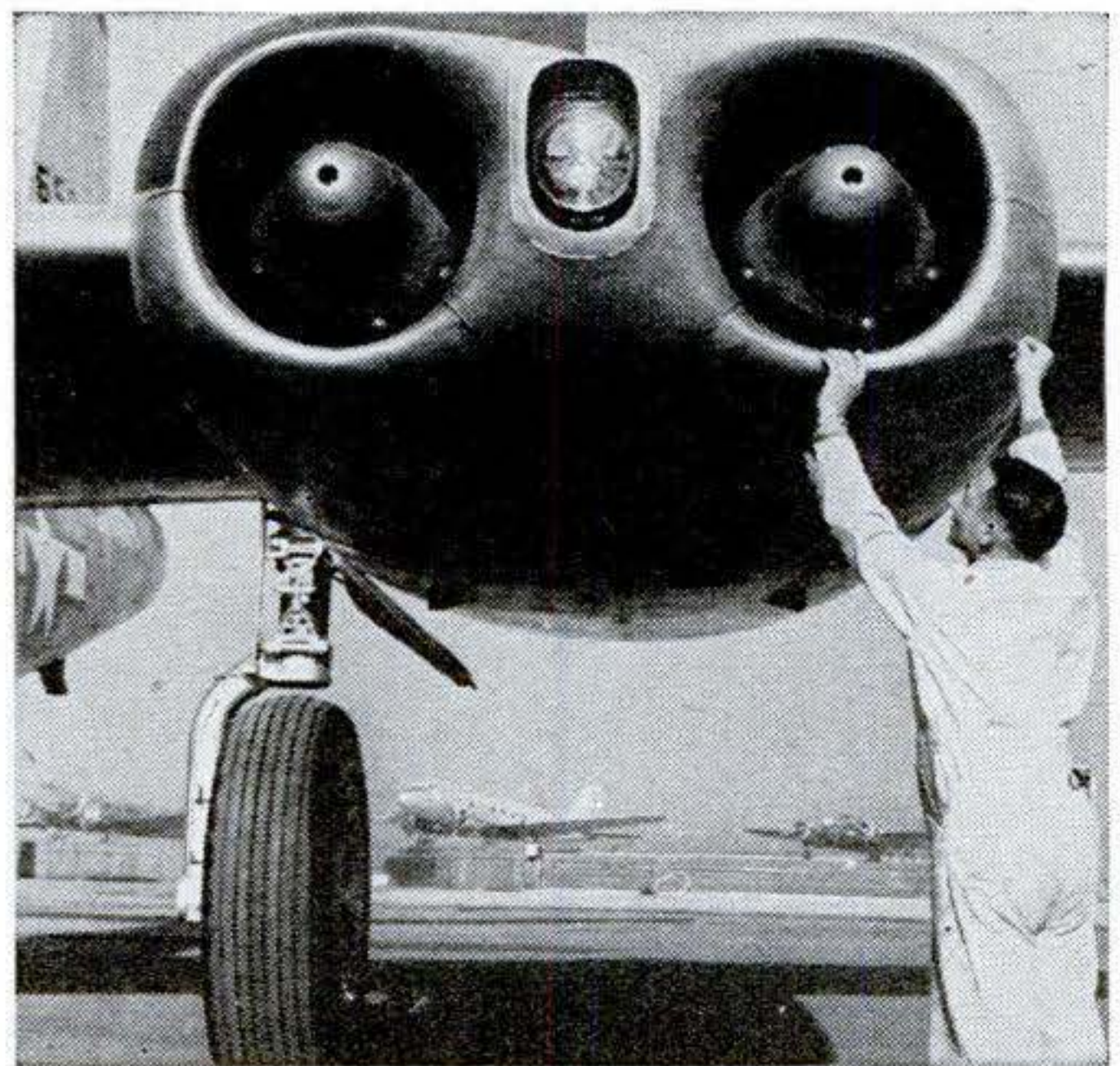
Twin-jet nacelles are ahead of wing's leading edge for easy accessibility. The new high-pressure tire was specially developed to fit into the thin wing.
