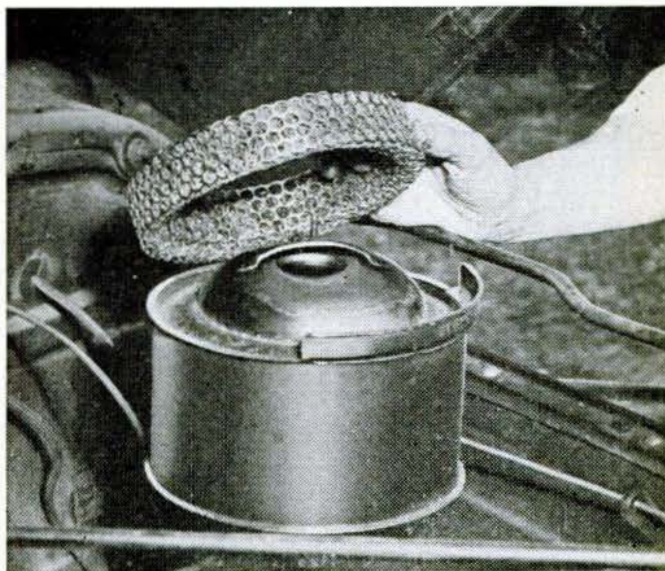
Remove the mesh filter from the air cleaner and wash the dirt from the filter with gasoline. Then dip it into a container of light oil and allow to drain for some time before returning to its place.
