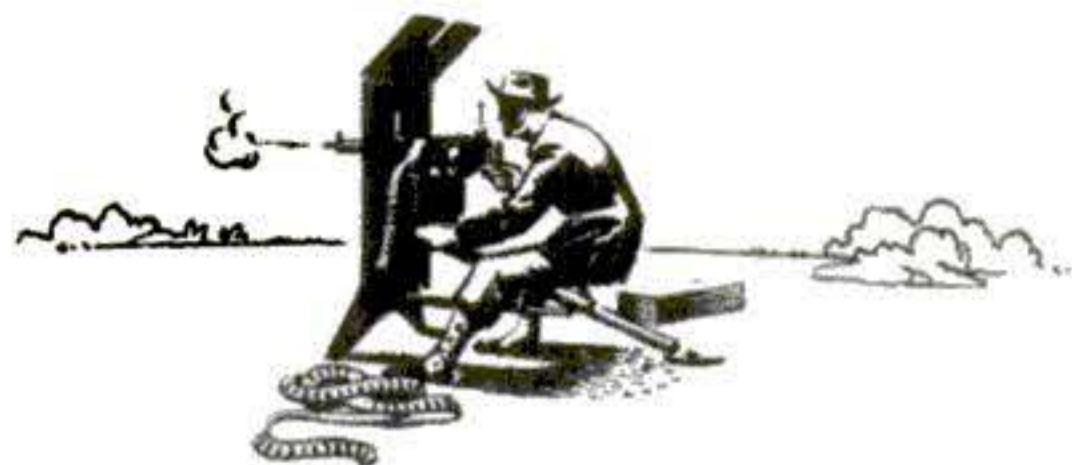
The Maxim, invented about 1885, was the first true machine gun. Firing and ejection were automatic.
