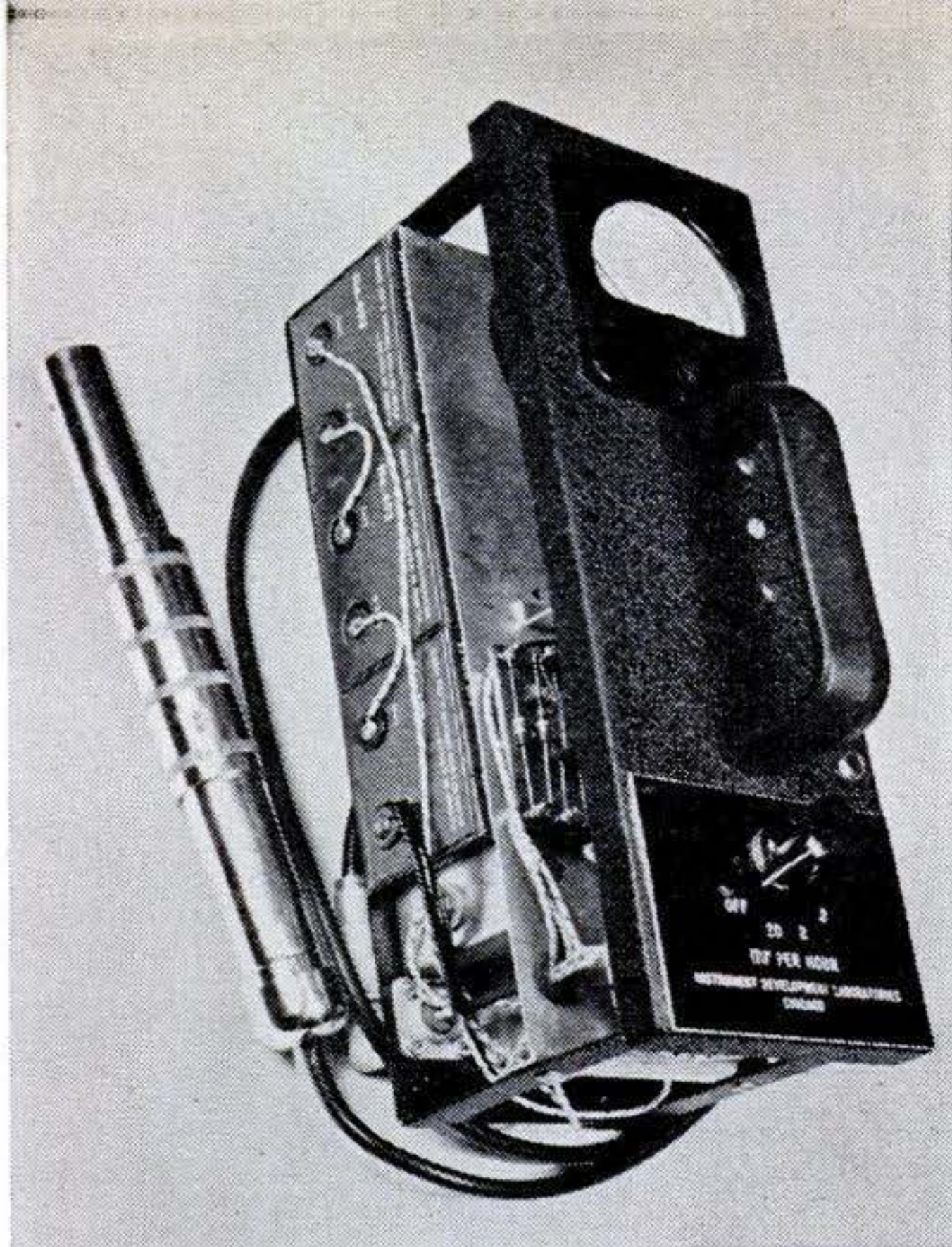
This Geiger counter, made by Instrument Development Laboratories, Chicago, weighs only 10 lb. complete with case, probe and batteries.
