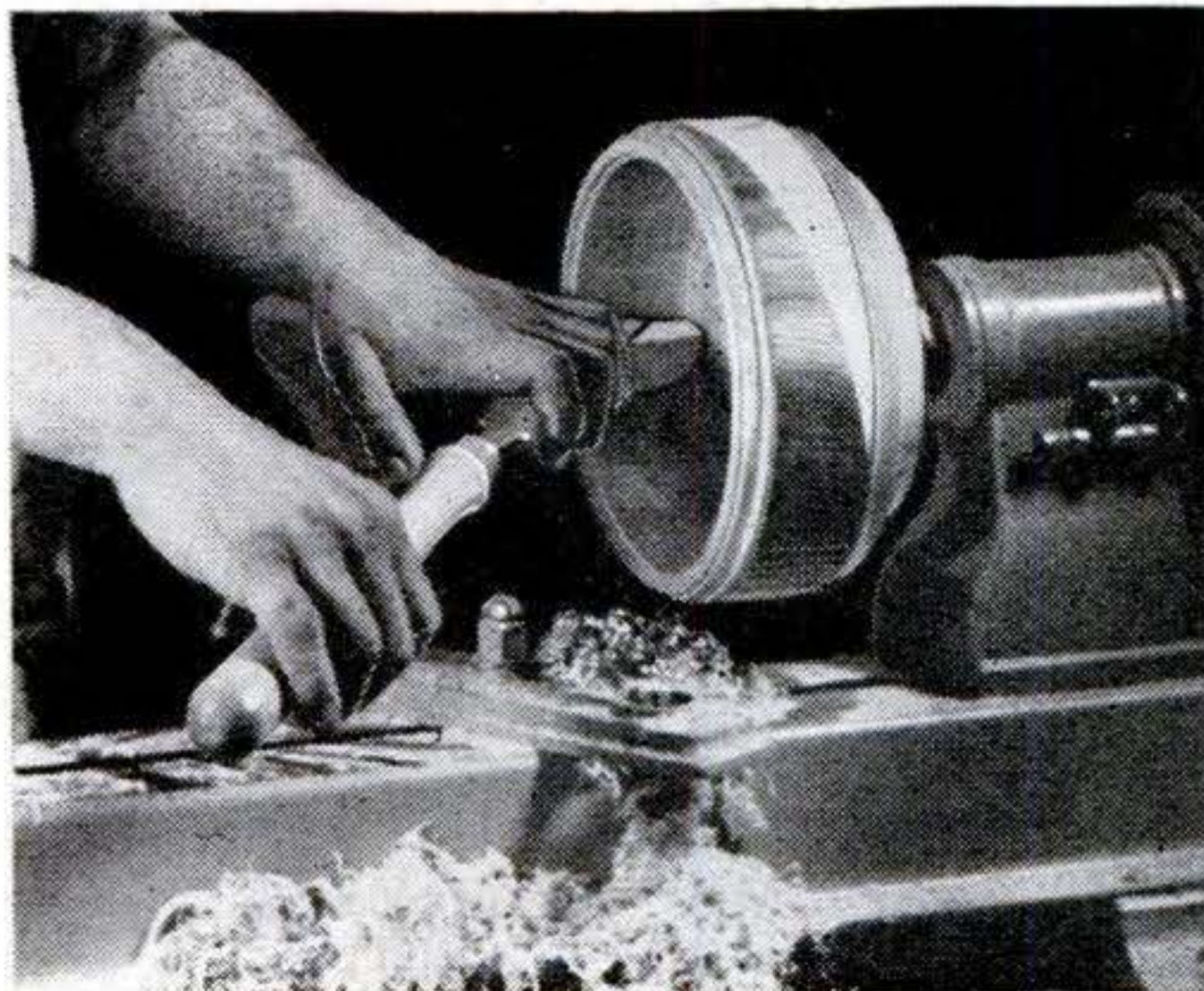
In finishing the bowl inside, projection of the tool rest into the hollow shortens tool overhang.
