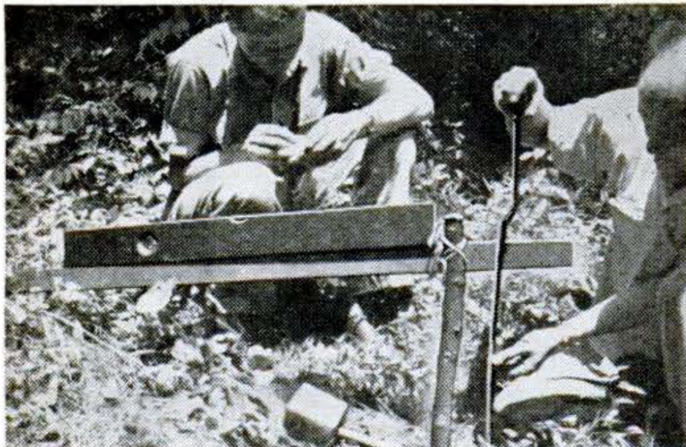
With the straightedge held level, vertical height between a pair of pegs is read off and noted down.
