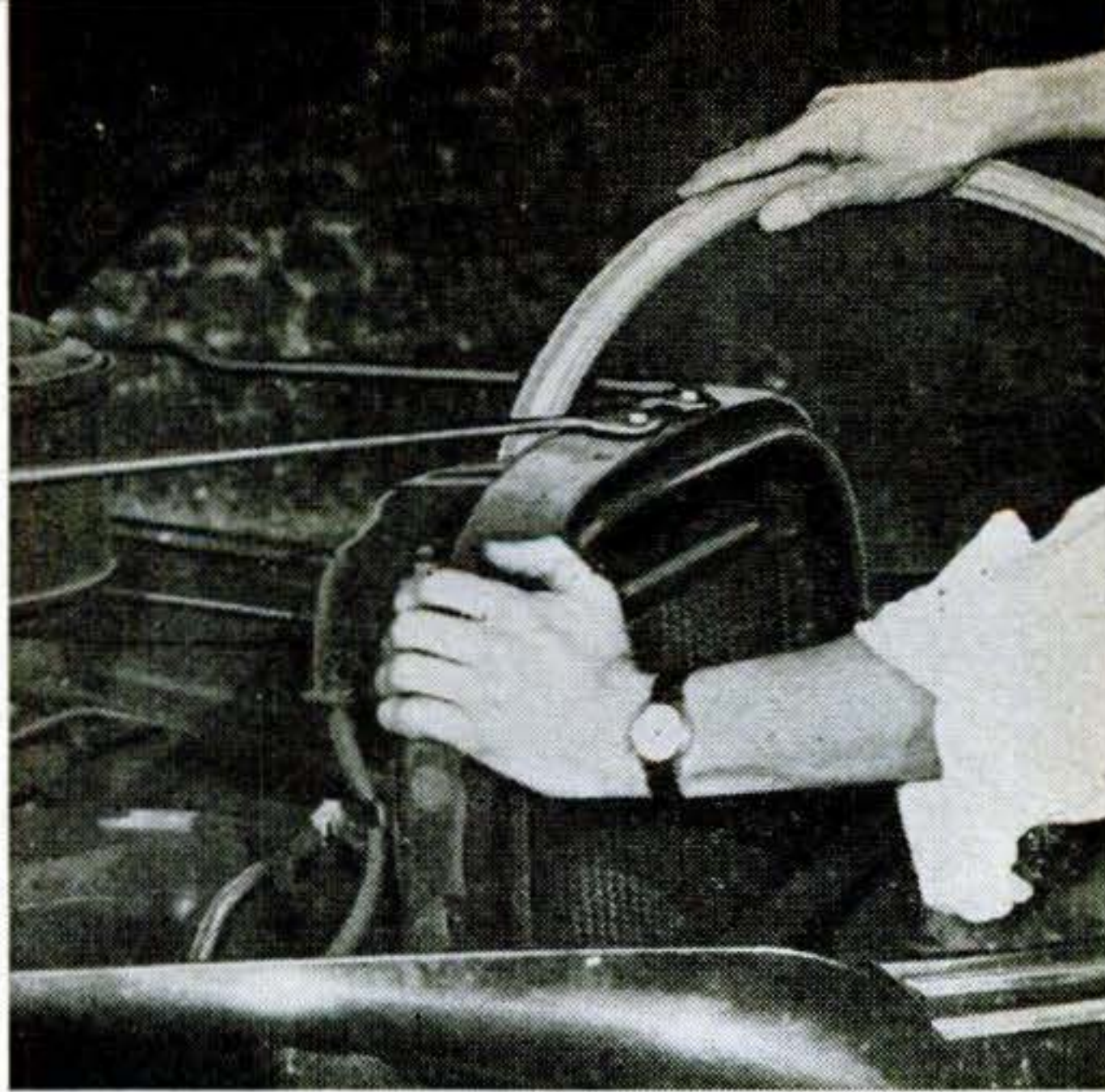
Also flush out the cooling system. Reverse flushing is more effective in cleaning out the corrosion, but a hose used in the old way will help a great deal.
