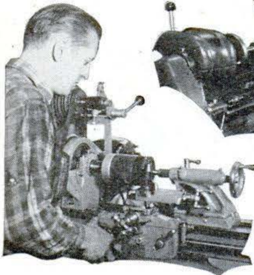
MACHINING STOCK PISTON
