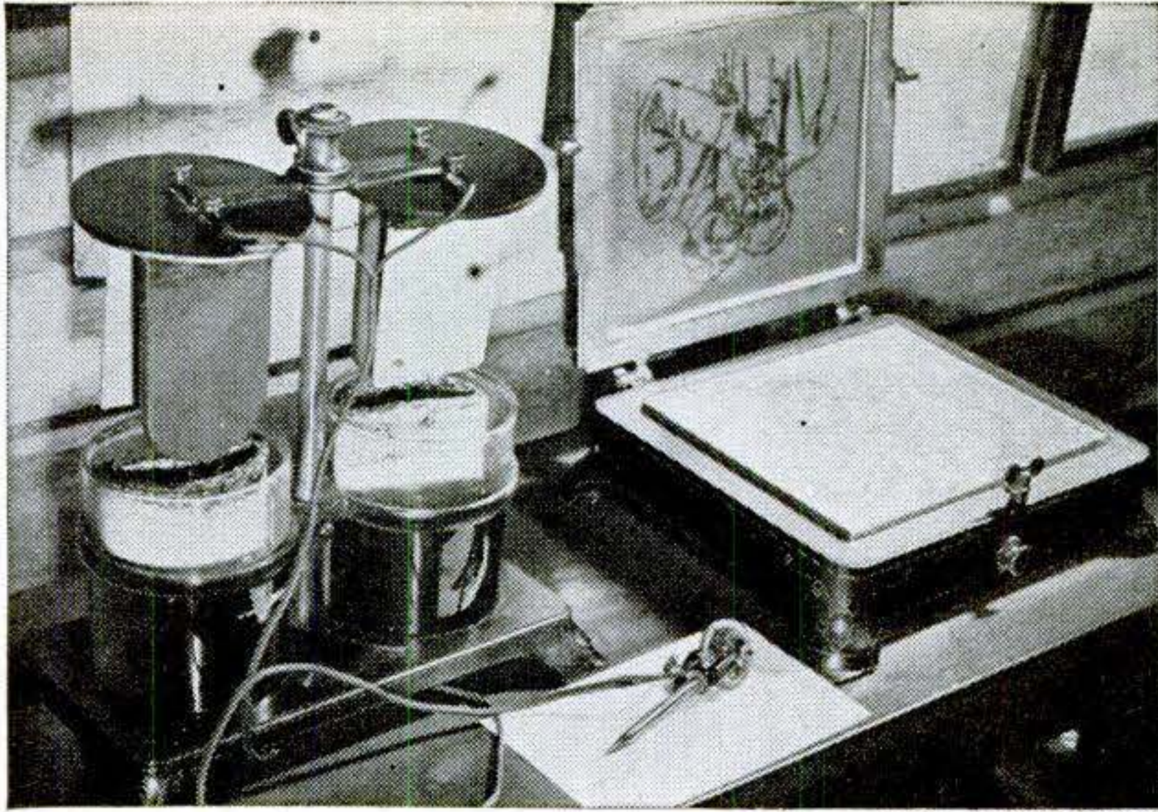
The Edison Electric Pen, shown at left, was a forerunner of the mimeograph. The inventor first manufactured it at Menlo Park. The pen is powered by a small electric motor that draws current from the wet-battery cells at the left of the picture. The stencil made with the pen is placed in the frame at right and ink forced through the perforations with a roller, making copies. Popular in big business offices, more than 60,000 of the pens were once in use.
