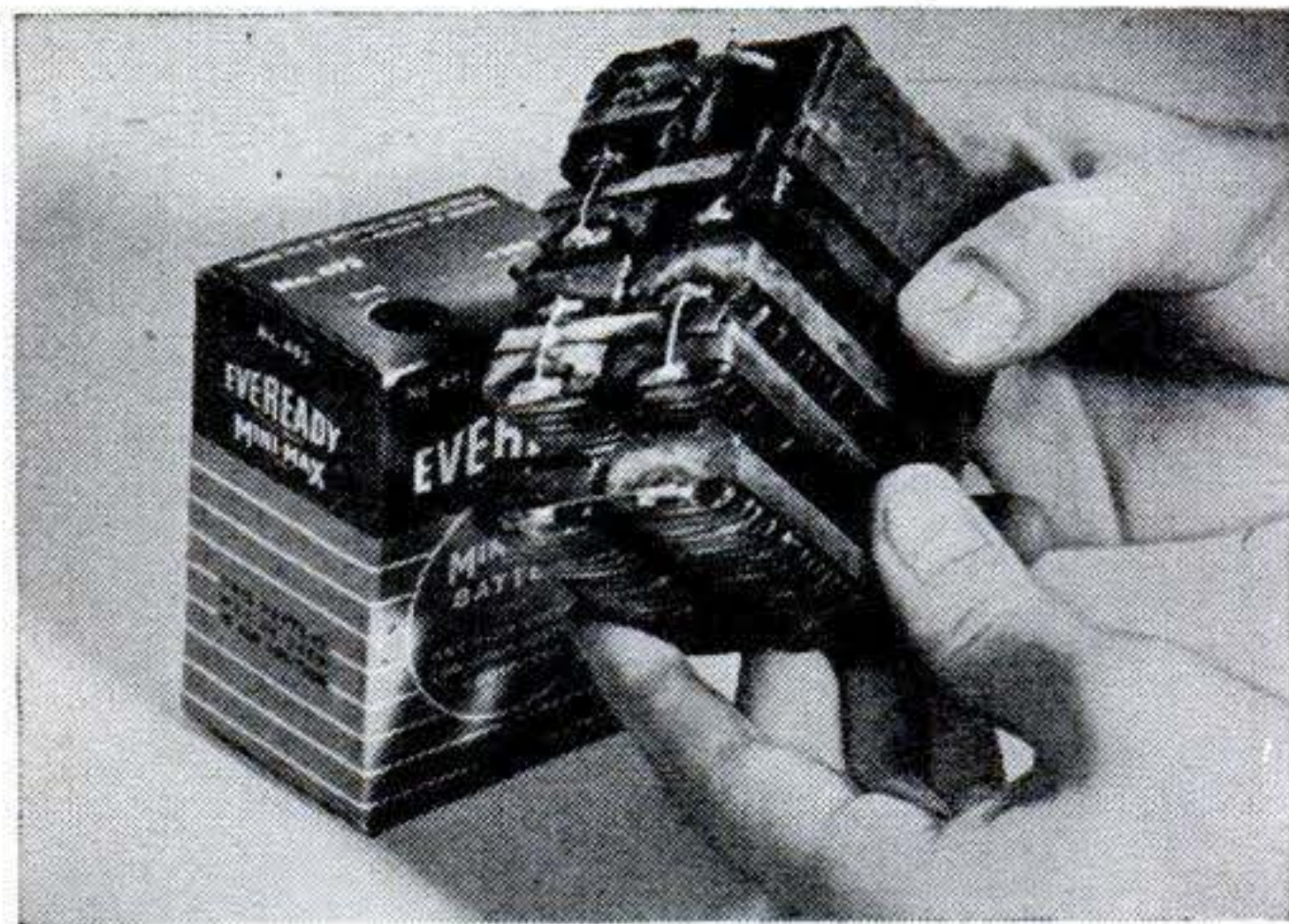
Close-up shows compactness of 300-volt battery made of 10 stacks of flat cells. It is slightly less than three inches square, just under four inches high.
