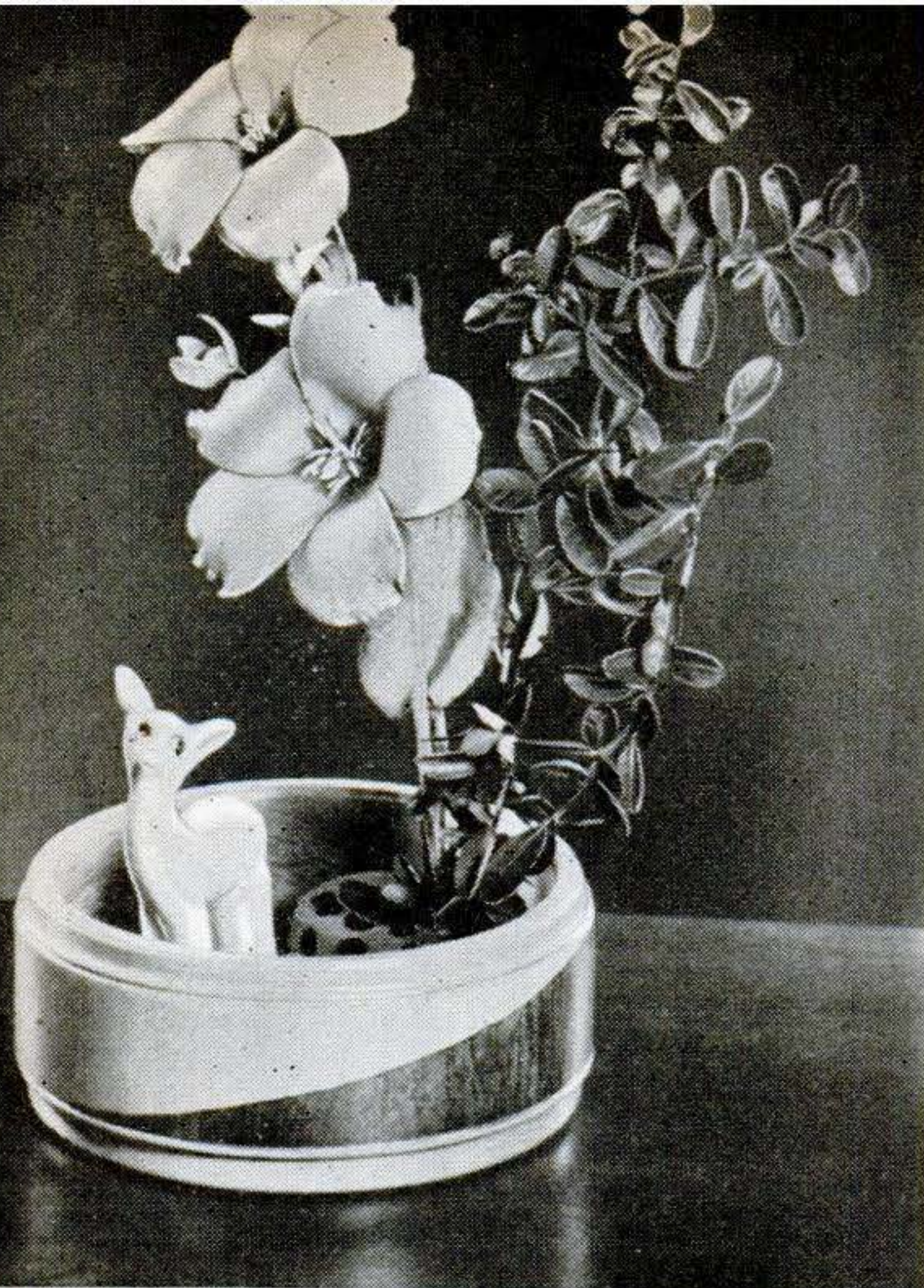
For flowers or rock plants, the bowl can be fitted with a glass container. The veneer is put on as a ribbon joined to give a spiral effect.
