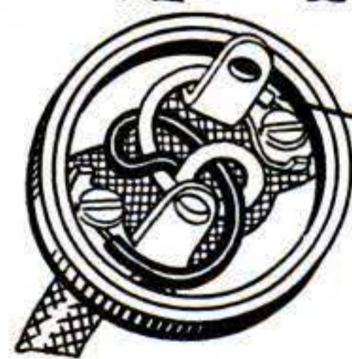
INSULATION RIGHT UP TO SCREW HEAD
