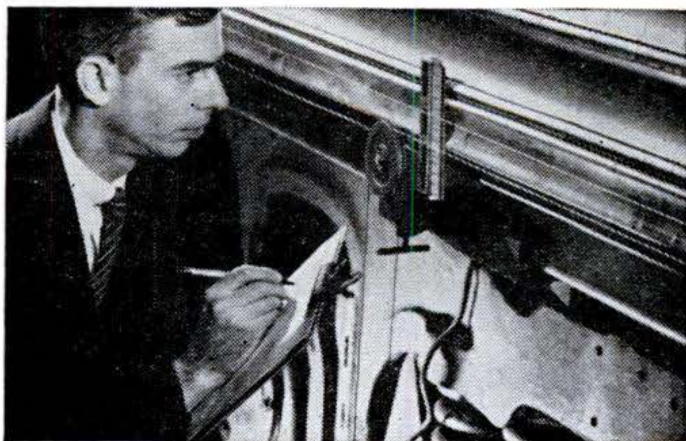
Taking readings of vertical deflection during the test of Budd's new Vista-Dome car. Gauge measures the car's contraction under a compressive load.
