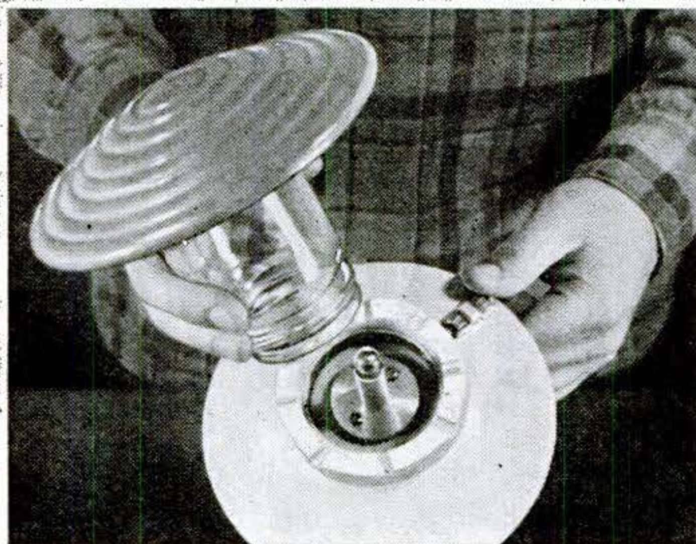
One end of the glass jar is cemented to the wooden shade; the other end screws into the metal lid which is fastened into a recess in the cover.
