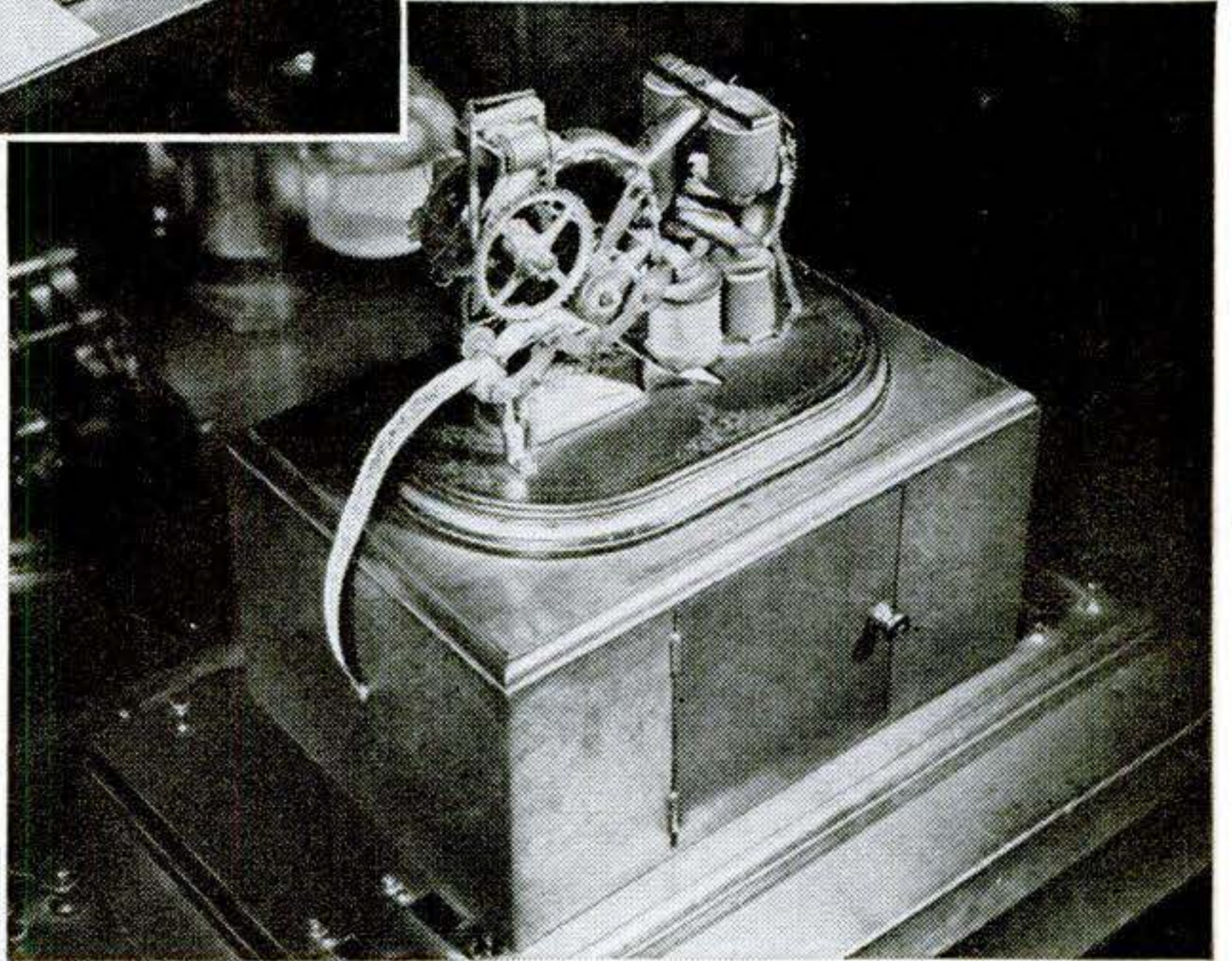
Edison devised the Motograph Telephone Receiver, left, to get around patents on the Bell magnetic type. The transmitting current is fed into a revolving chalk drum. This pushes against a spring with pressure varying according to the intensity of the current. The spring activates a sound-producing diaphragm.
