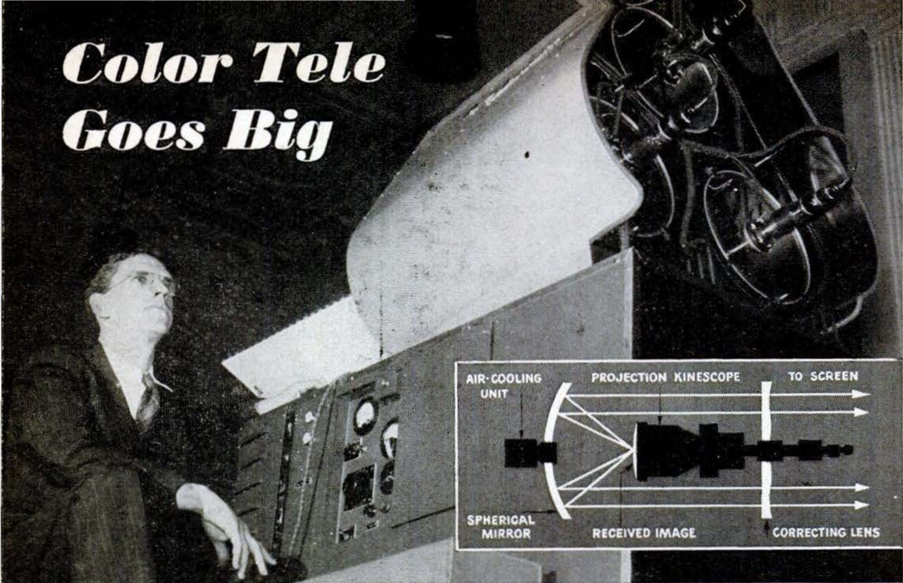
Color projector contains three monochrome kinescopes. Inset shows one with its associated optical system.
