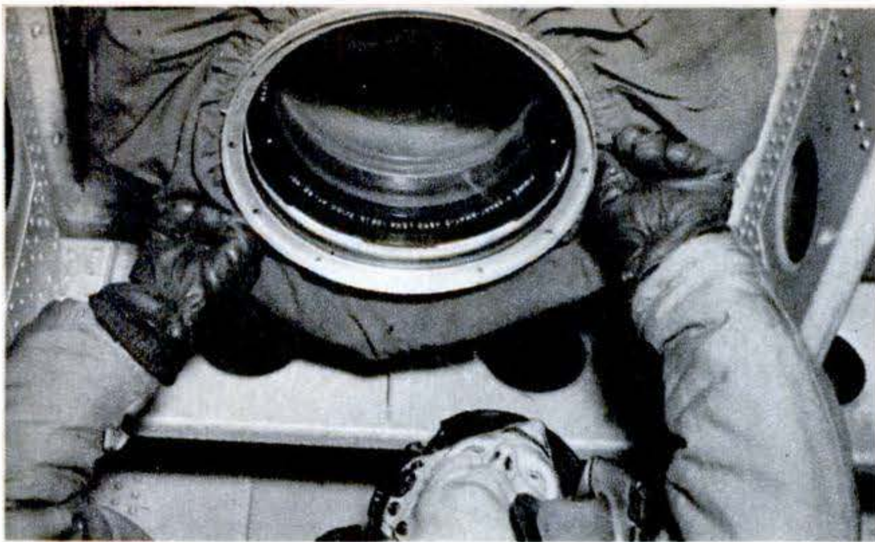
Its draft seal pushed back for a test run, the big lens looks down out of a B-29's forward bomb bay.
