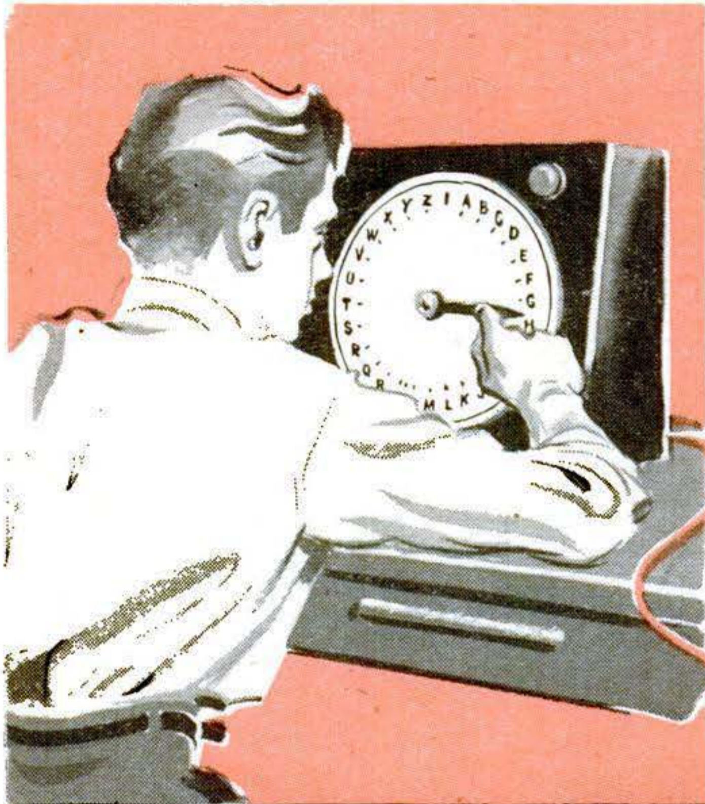
Words spelled by the pointer on one of the selsyn dials will be transmitted to the other since the shafts of the pair follow each other accurately.
