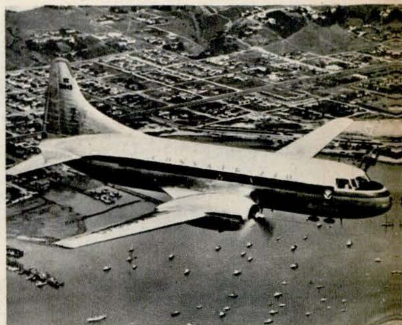
The finished product. Equipped with two 2,400-hp. engines, the Convair-240 supplements conventional power with jet exhaust for additional speed.
