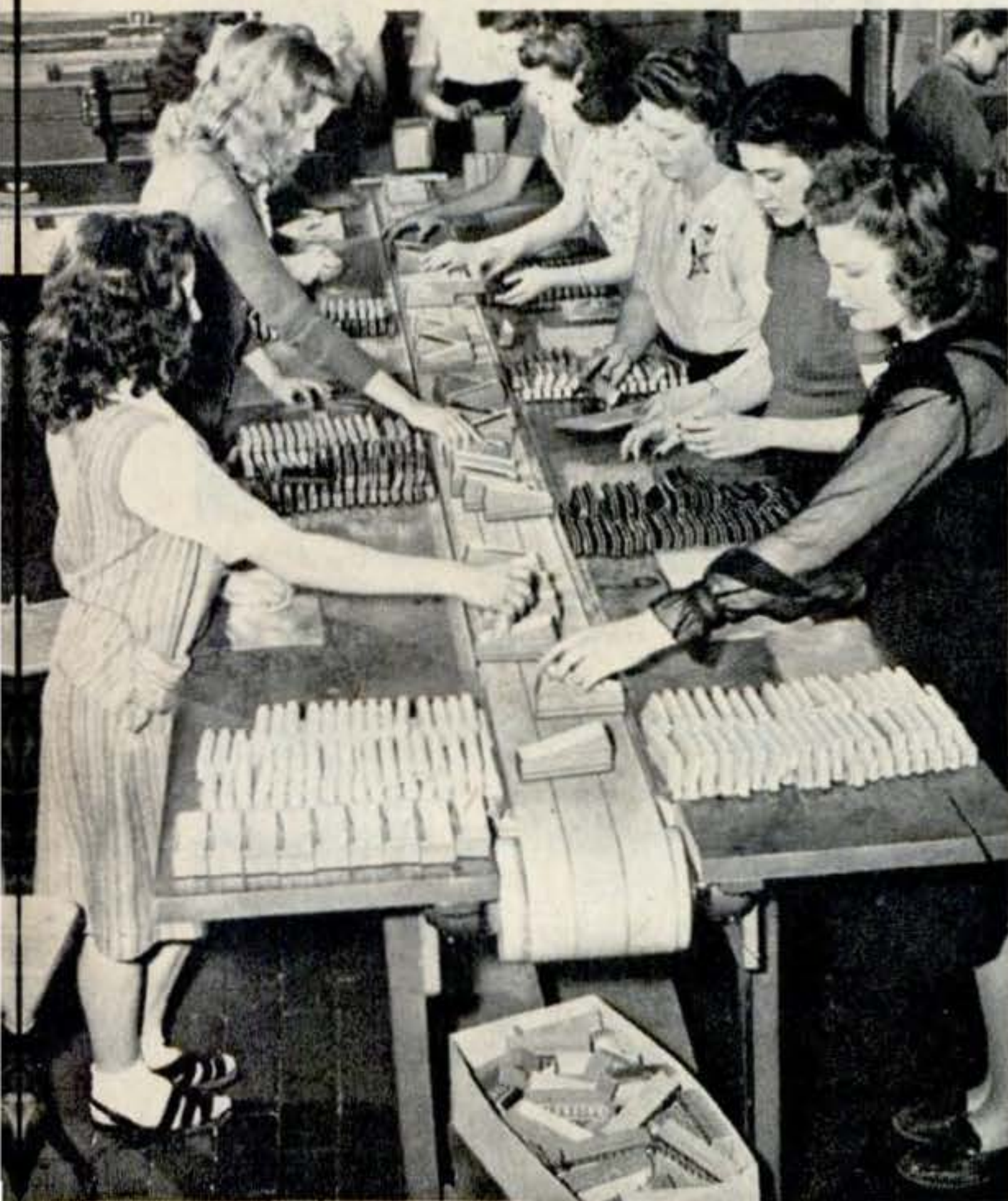
6. Finished harmonicas move rapidly along a conveyor belt, assembly-line style, where they are individually boxed for shipment after first receiving a careful inspection.
