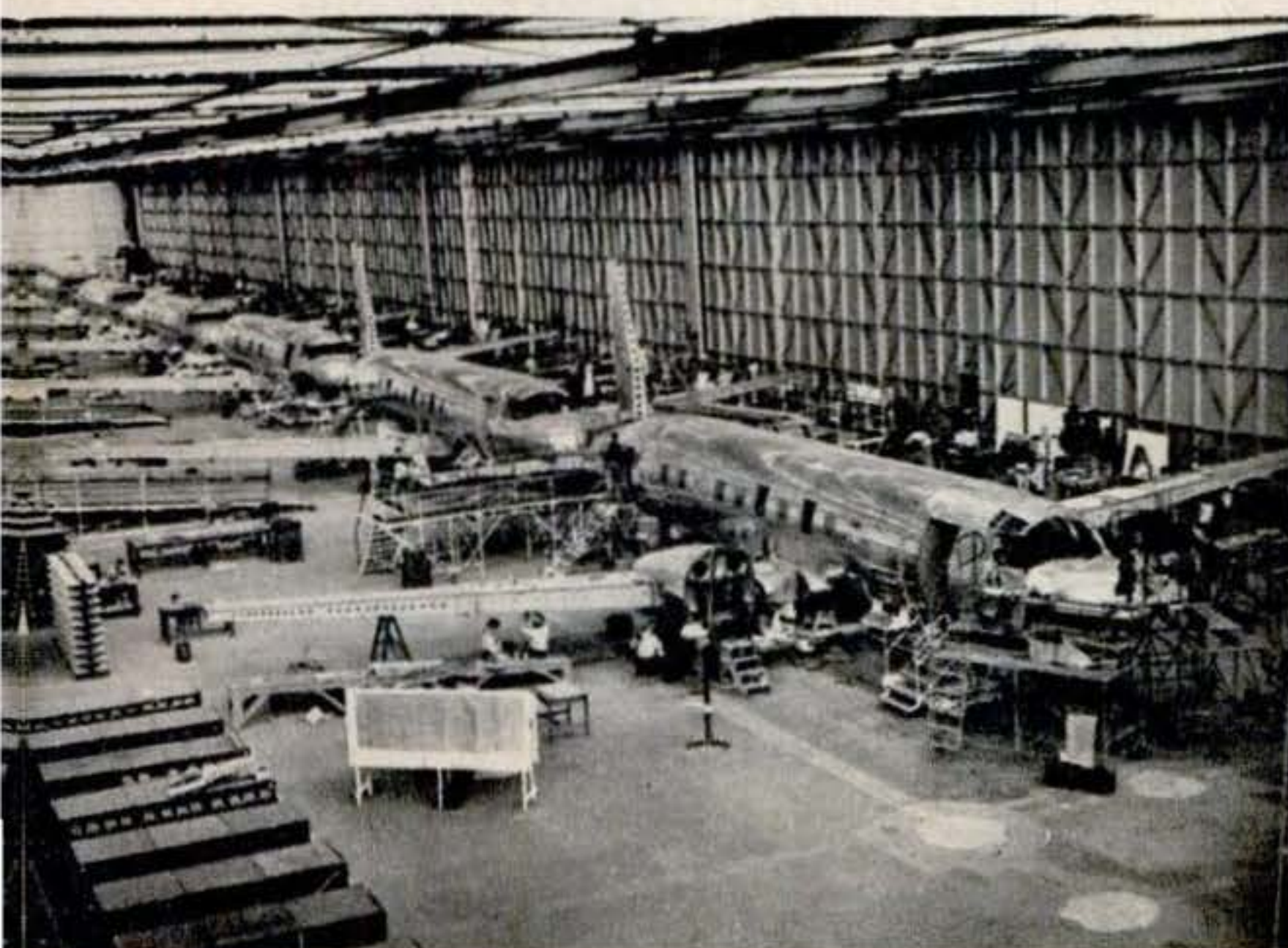
Wing sections, tail surfaces, nacelles and other parts, already built and awaiting installation, are quickly added as planes move down the line.
