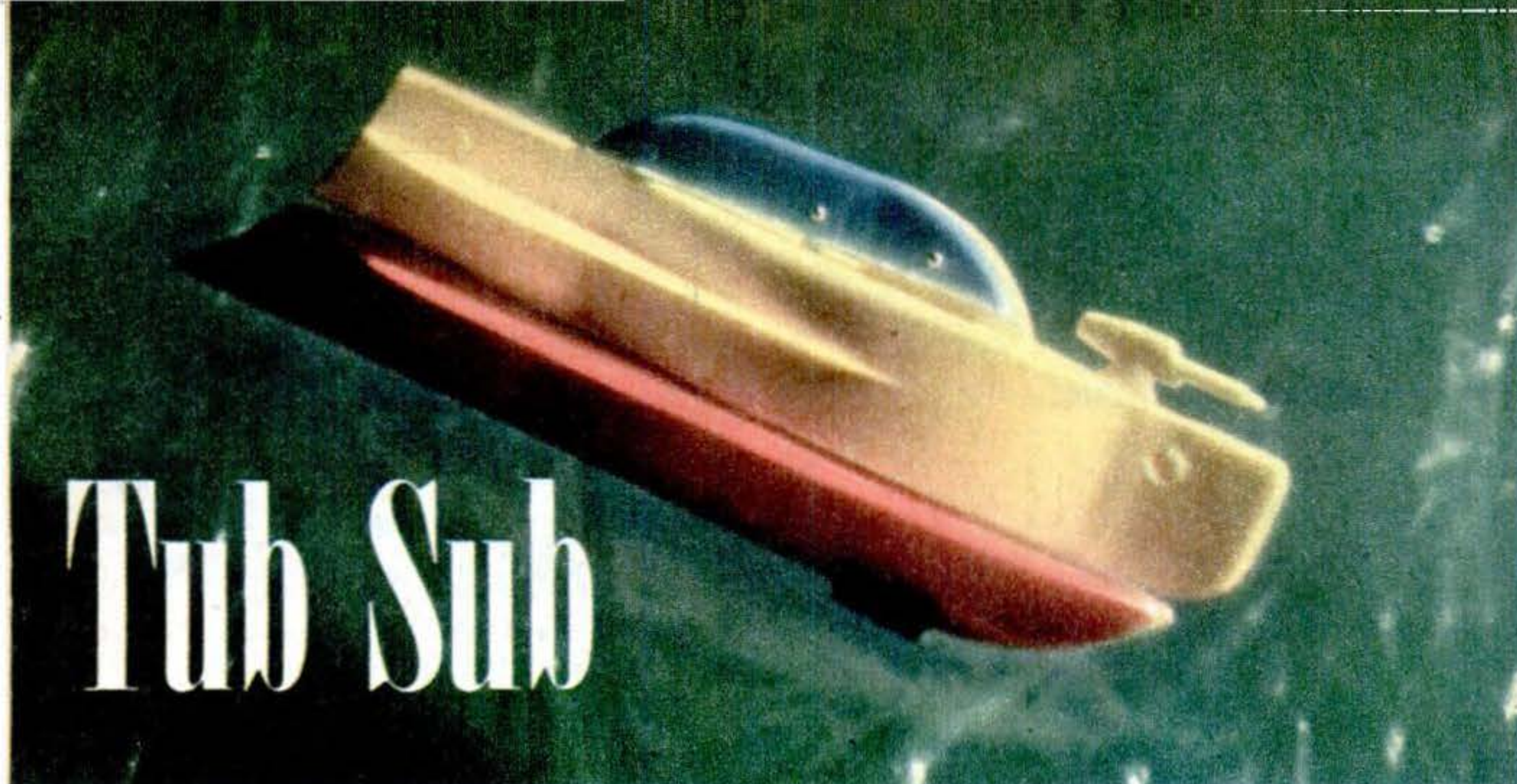
The toy sub in action, downward bound. Moving the ballast weight on the keel regulates depth of dives.
