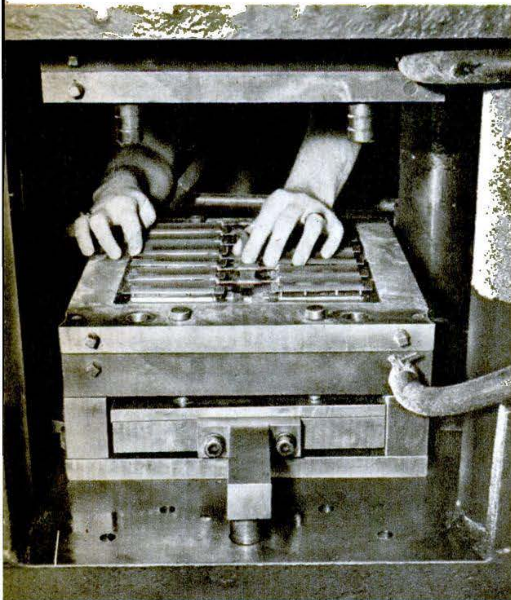
4. Plastic cover plates, of polystyrene, are molded under a pressure of 1,500 lb. at 400° to 500°F. Some harmonicas are made entirely of plastic, even to their reeds.
