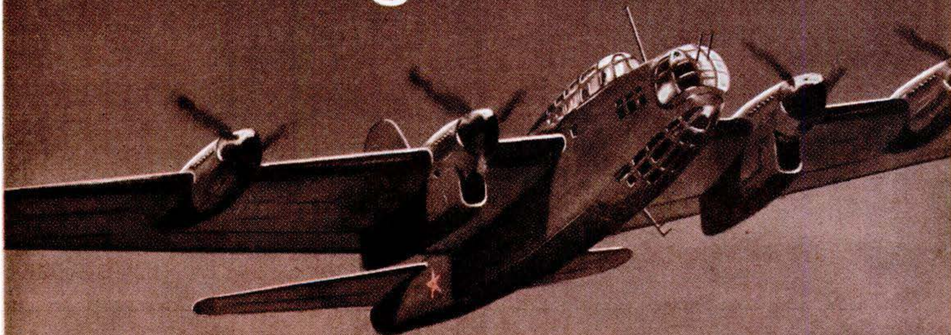
TB-7: Four liquid-cooled, 1,350-hp. engines give it a cruising speed of about 200 m.p.h. carrying bomb loads up to 11,000 lbs.
