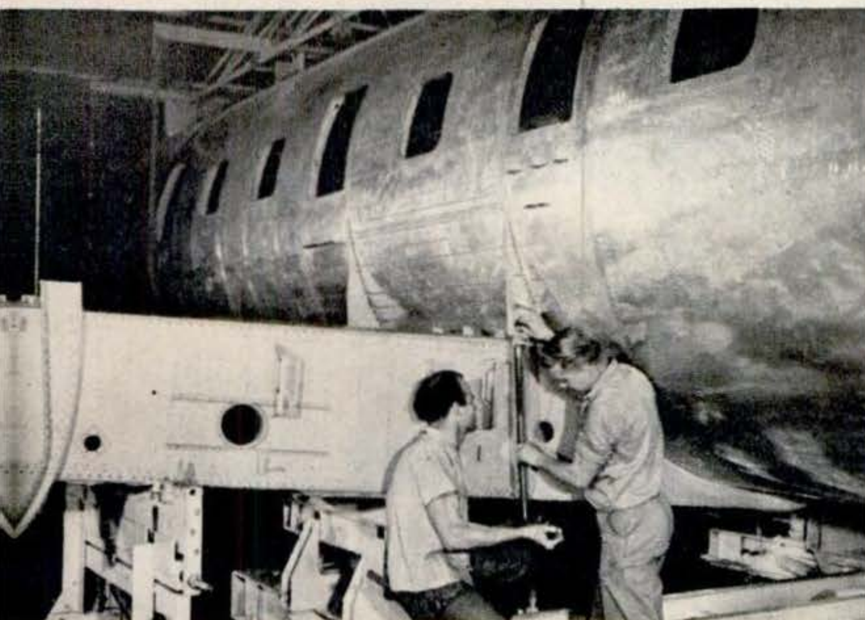
A torque wrench, providing exact degree of tightness, is used in bolting wing center section to fuselage. Over-all wing span is 91 feet nine inches.
