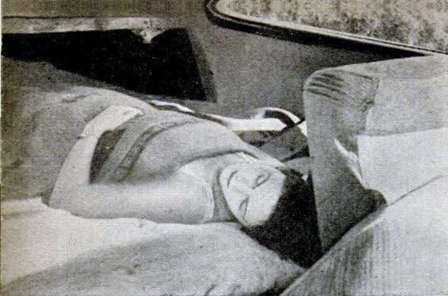
Full-length sleeping comfort on vacation trips is provided by this modification of a two-door sedan. The foot of the bed is in the trunk.
