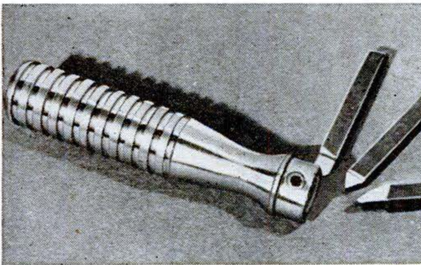
Grooves turned on the handle improve the grip. The same result can be obtained with a knurling tool.
