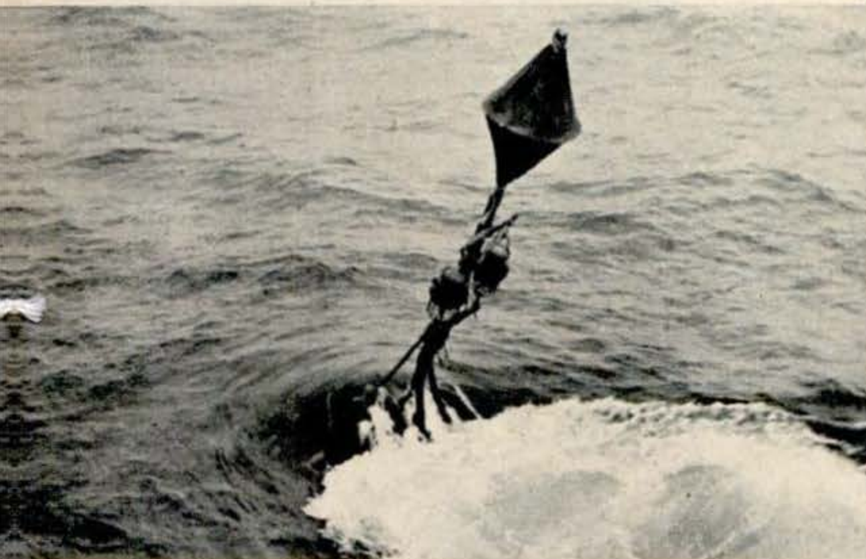
5. Swift current swirls a wake around a marker buoy during operations in the Gulf Stream. Bracket on the staff holds two lamps that are visible for nine miles. Buoy is hauled back on ship after repairs.
