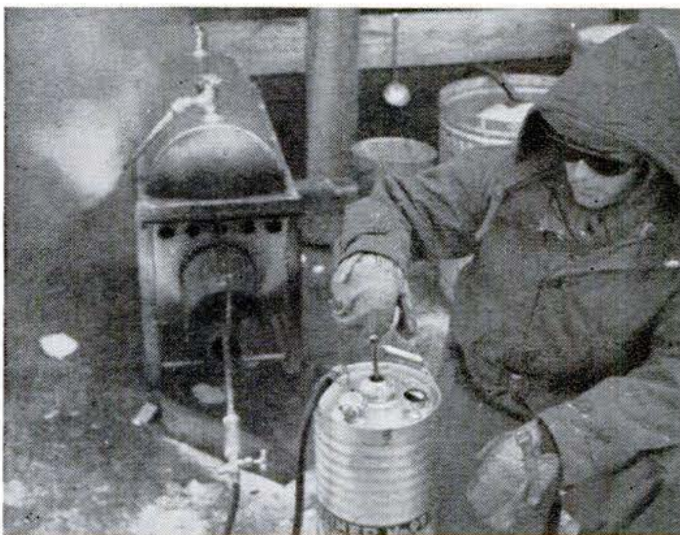
Next, start the automatic steam-making machine, operating on Diesel oil. Expedition found need for more than the one steam-maker taken along.
