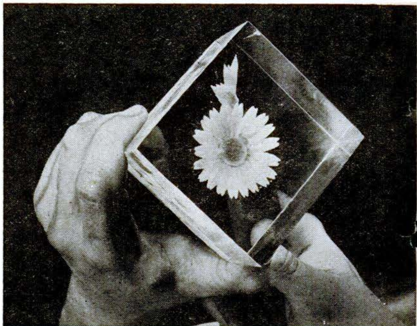
6 Leaves are made with the drill angle somewhat greater than for the petals. Forward thrusts cut the points. Starting at the centerline, one side is completed first and then the other.
