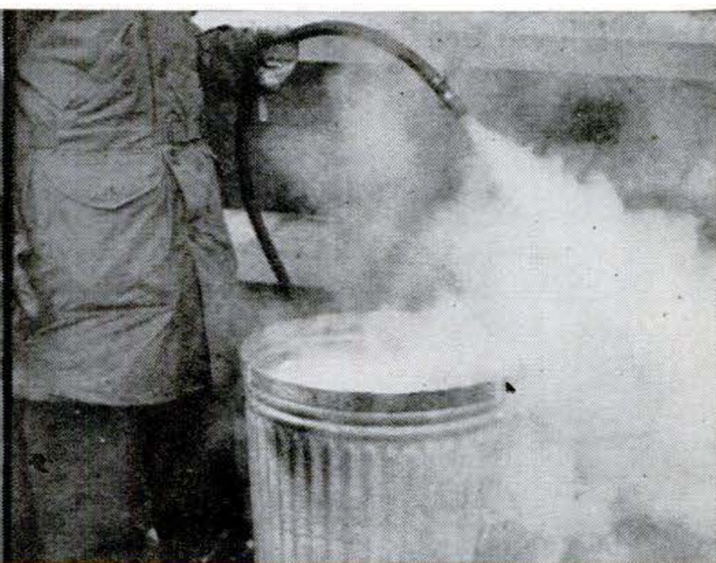
Finally, you turn the live-steam hose into the can. Soon you will have pure drinking water. All polar barracks need hot-water machines.
