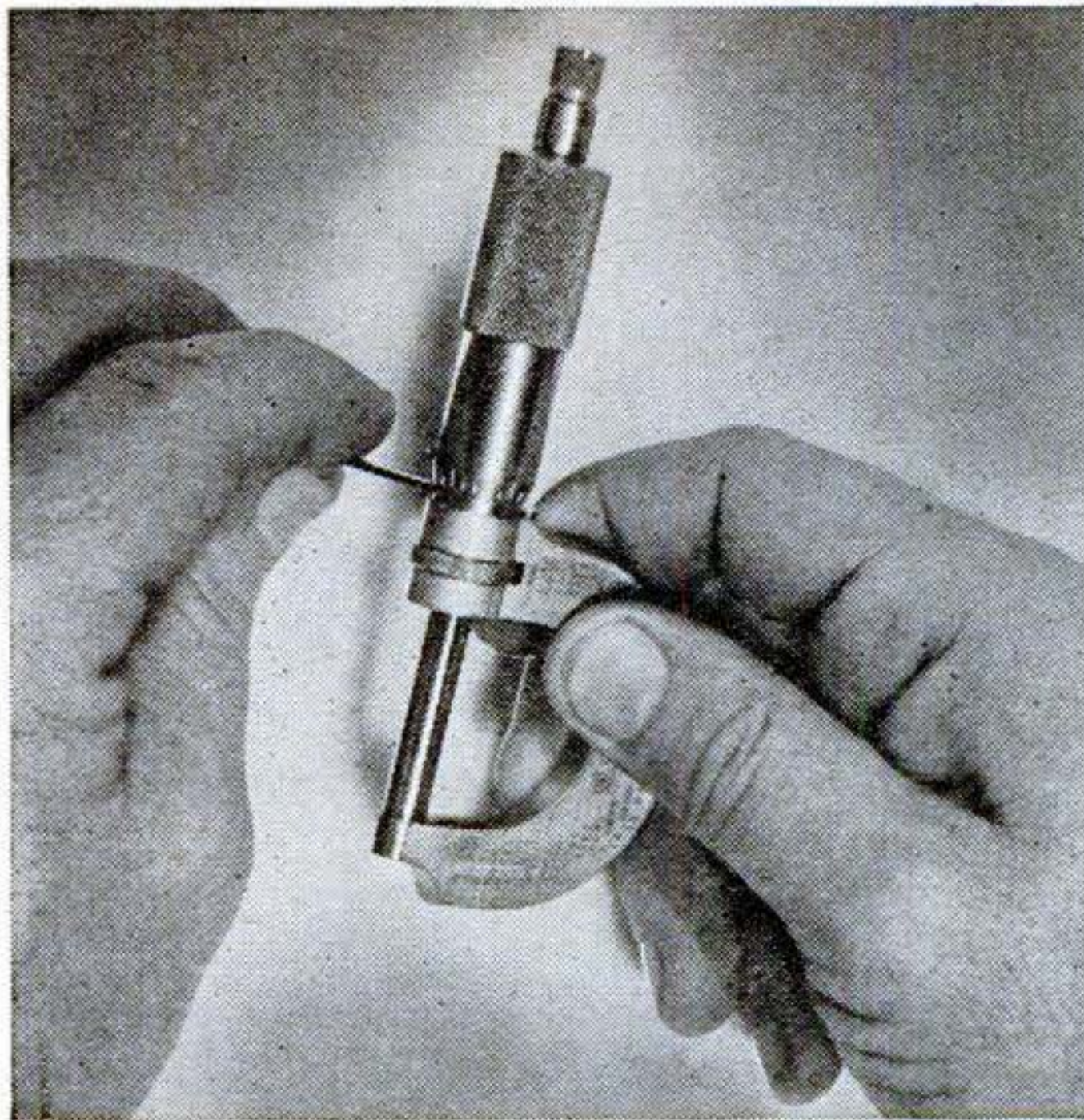
To adjust for accurate readings, the spindle is touched to the anvil and the sleeve turned by a spanner wrench until the zero lines match.
