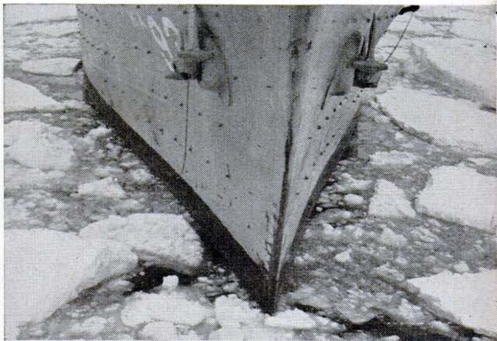
A thin-skinned cargo ship feels its way through the ice pack. Sharp chunks like these punched holes in all the ships. For pack travel, ships should have several inches of steel armor.
