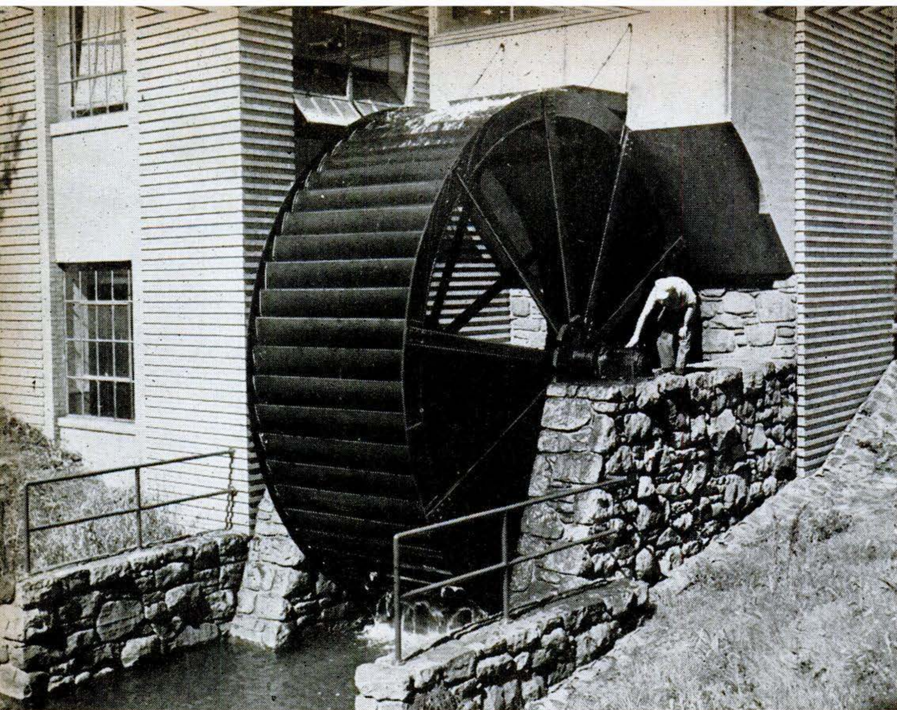
Gravity turns the overshoot wheel. Water-carrying buckets on one side overbalance the empty ones opposite.
