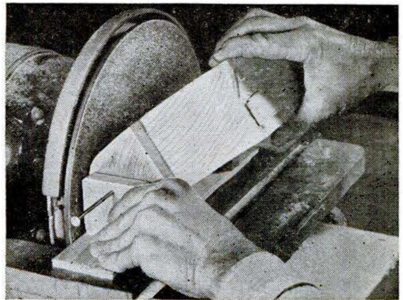
Rounding the back on a pivot jig. The lid blank is swung on two nails. Shape the front freehand.
