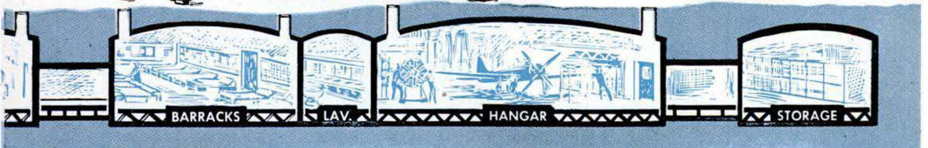
Buildings will be connected by tunnels, with exits at central hatches. Elbowroom helps morale.
