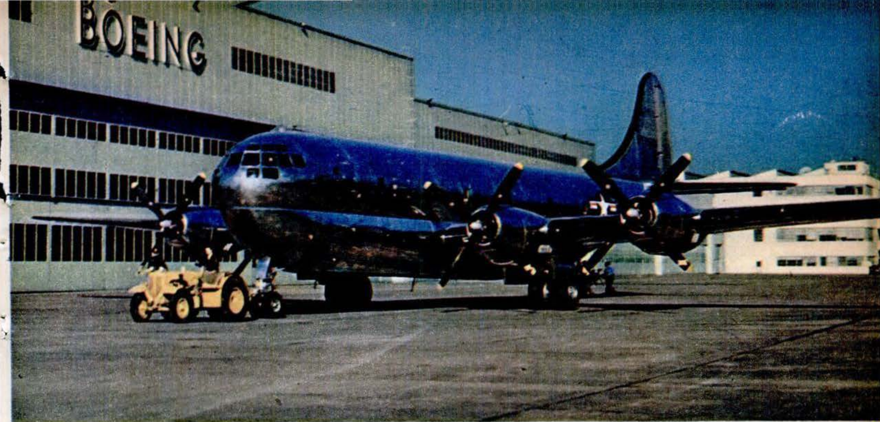
The towering tail of this AAF C-97 Stratofreighter illustrates the problem of getting it to fit inside the hangar.
