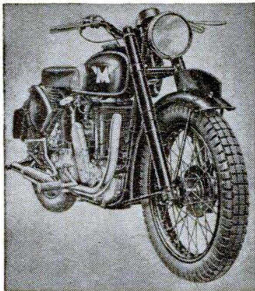
Enclosing the springs in telescopic forks gives a neat appearance in front. This is a Matchless.
