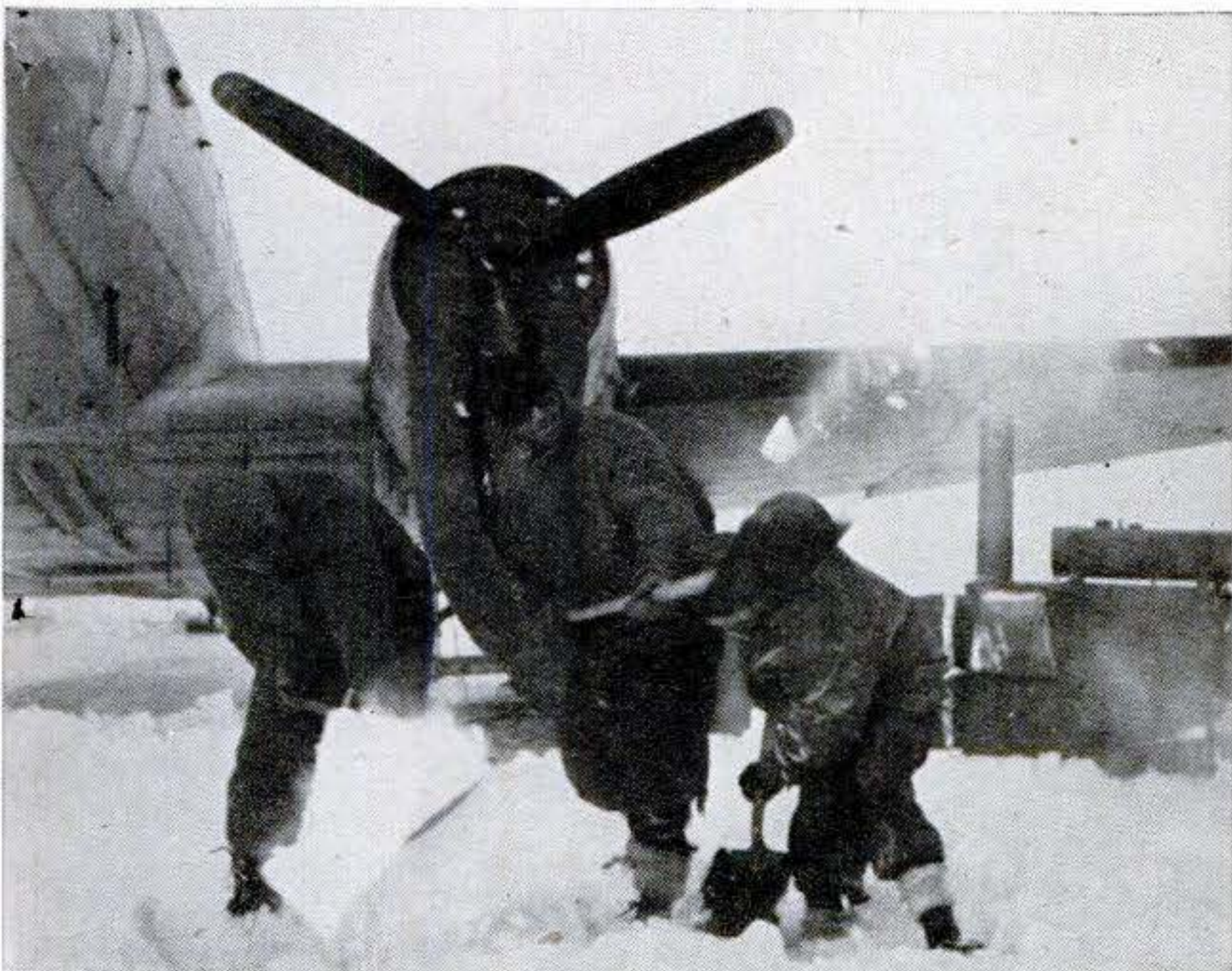
Planes must be kept clear of snow, for the tiniest opening lets it drift in. Hours must also be spent preheating planes before they take off.
