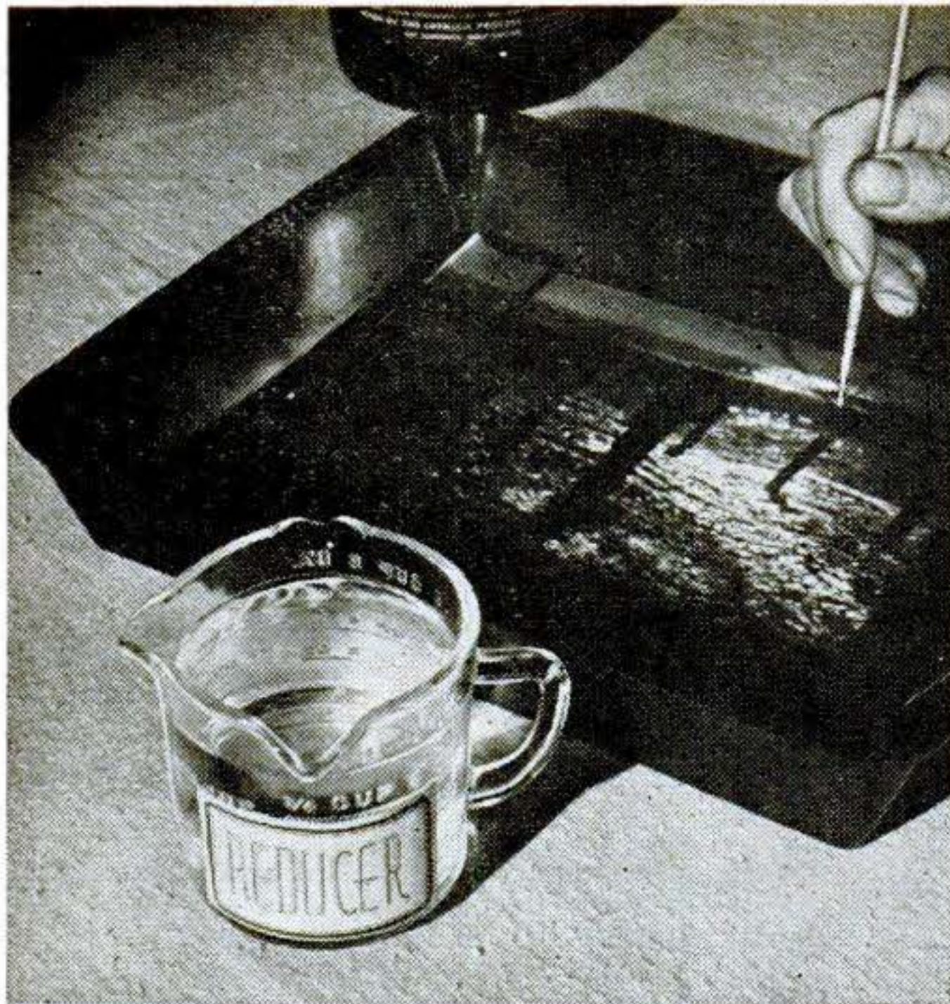
A brush gives you better control when very small areas are to be reduced. Reducing solutions may be made from such household bleaches as Clorox.
