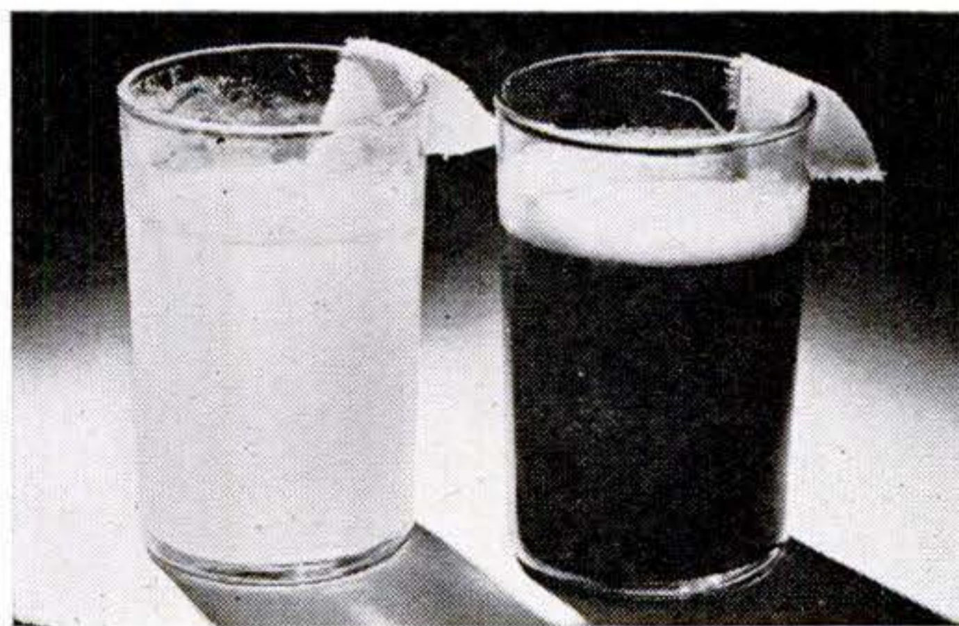
In water containing a little iron, soap produces a pale precipitate. If washing soda is added, this looks even worse. That it actually is not may be shown by placing a strip of white cloth in each.
