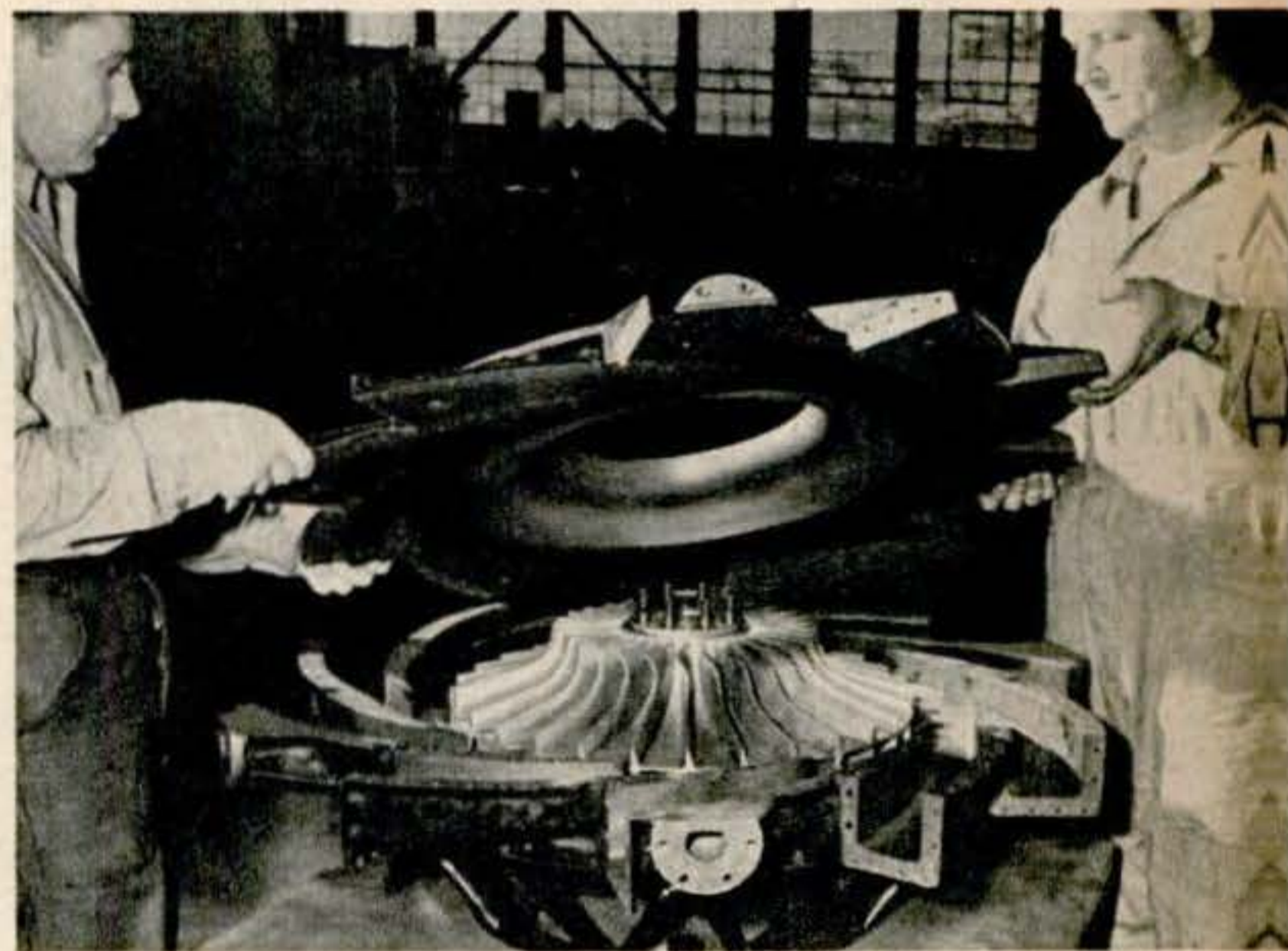
6. Compressor chamber is split and compressor removed. This is final step in tear-down; components are now ready for testing.
