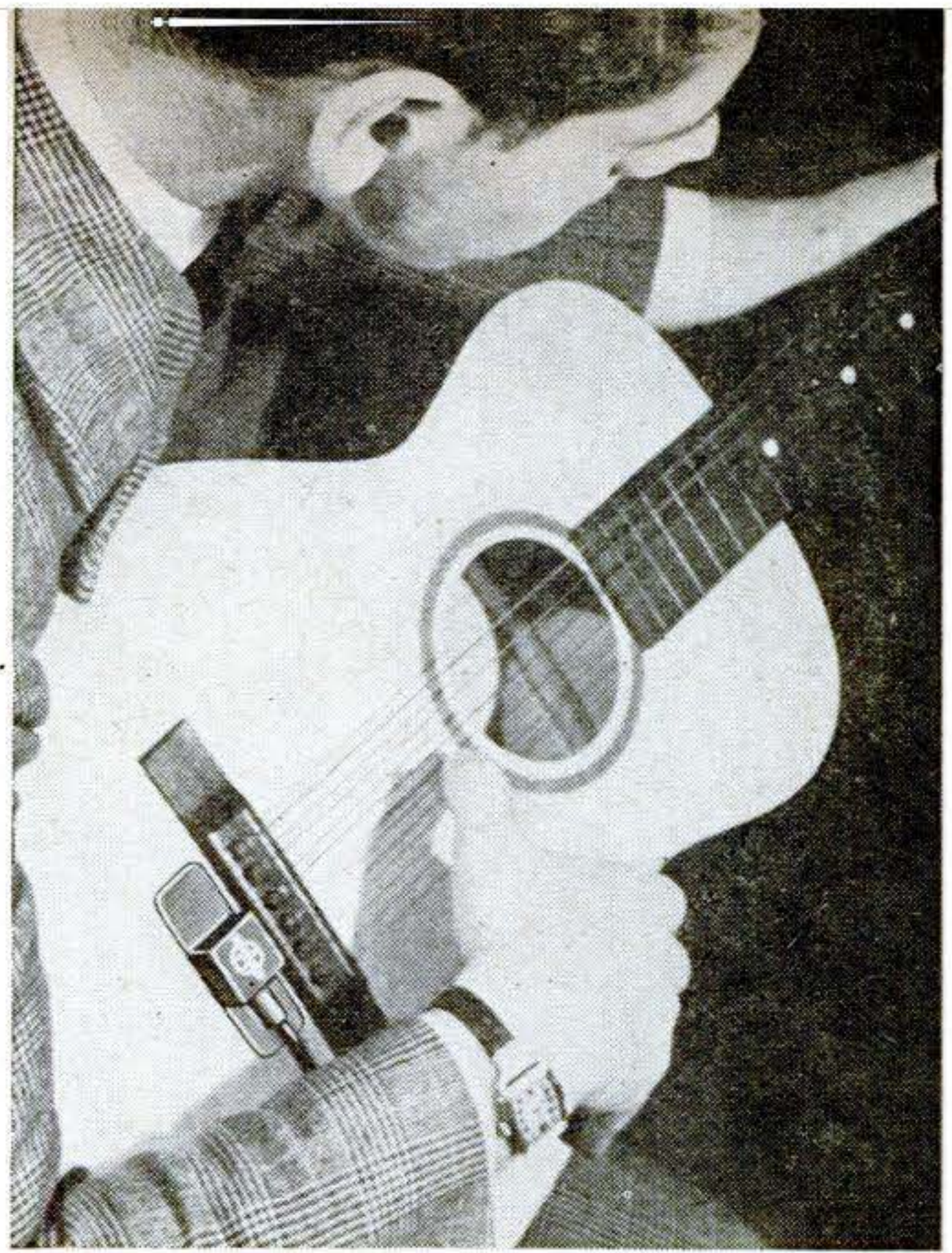
A little rubber cement was used to attach the contact microphone to this flat-top guitar. You can find the best place for the mike by actual trial.
