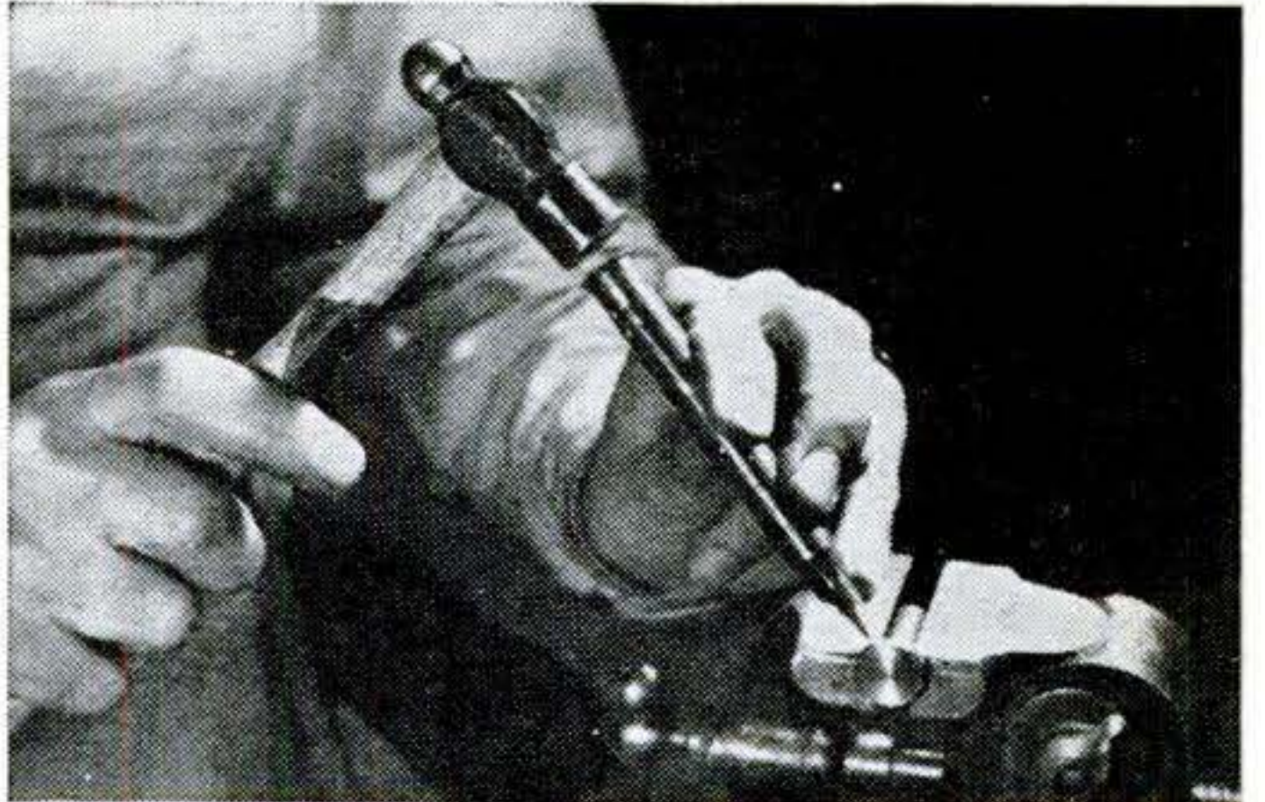
Cutting teeth enlarges the blank. If some sizes must be exact, experiment by making others first.
