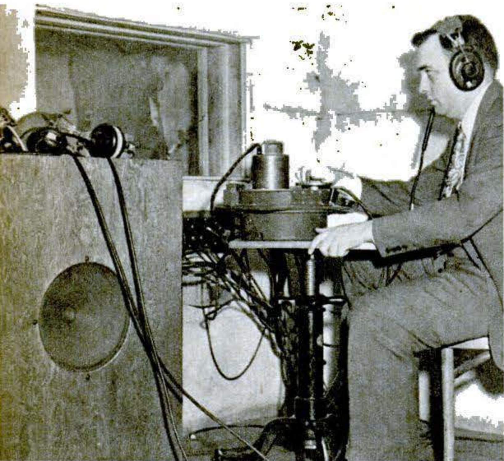
Inside the "padded cell," a specially built soundproof room, Dr. W. R. Garner shows how ear response is tested in research aimed at a blind-flying system using sound signals.
