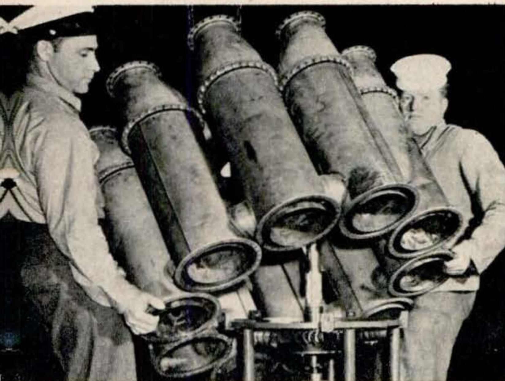
5. Assembly line in reverse moves along as the combustion chamber, ring, and elbow casing are removed from the turbine wheel.
