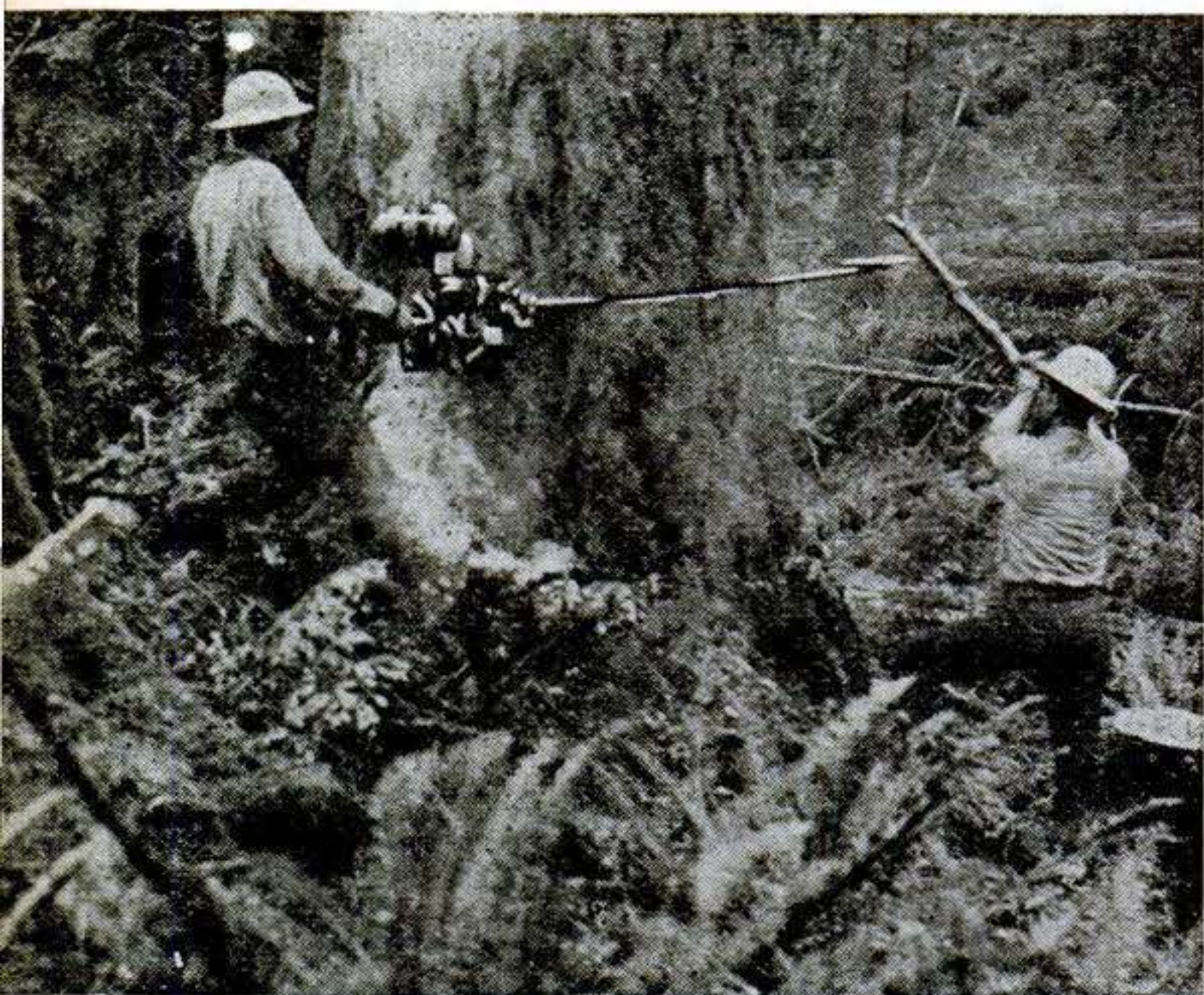
Cutting the niche to direct the fall of Douglas fir, power saws have replaced the crosscut and ax. Note how man at right pushes with stick.
