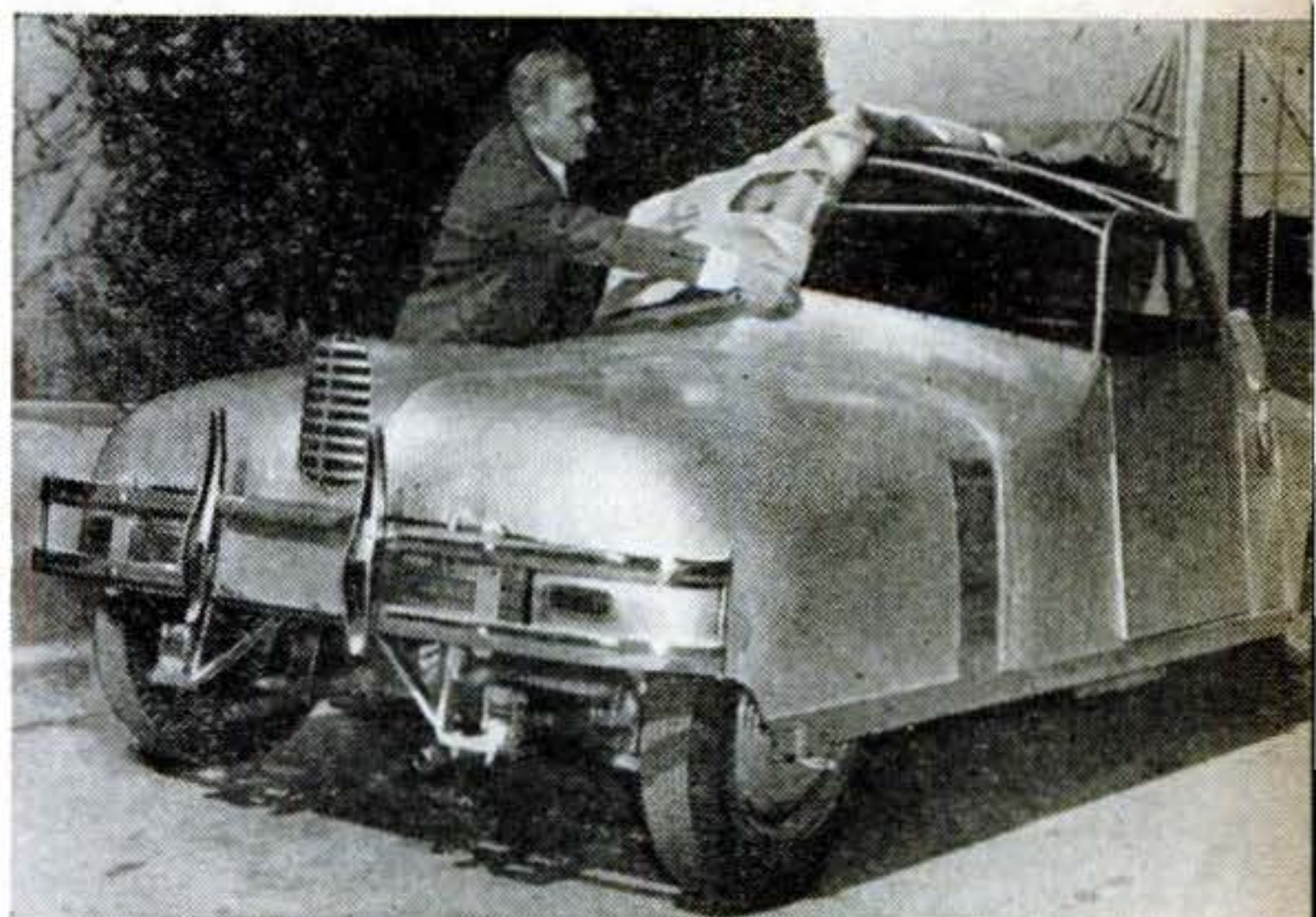
Roy Hunt, the builder, stretches the canvas top over the frame. Vents are provided at the sides and back of the rear-engine compartment.
