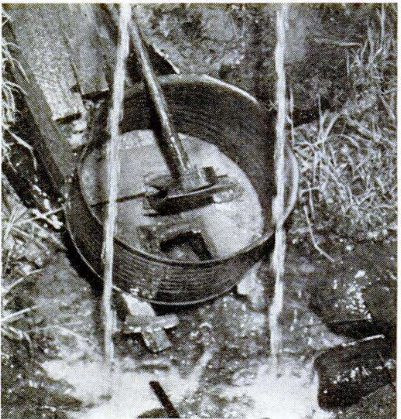
Washtub's dump valve is tripped at bottom of its fall. Runoff isn't wasted—it goes on to operate a waterwheel-powered machine shop.
