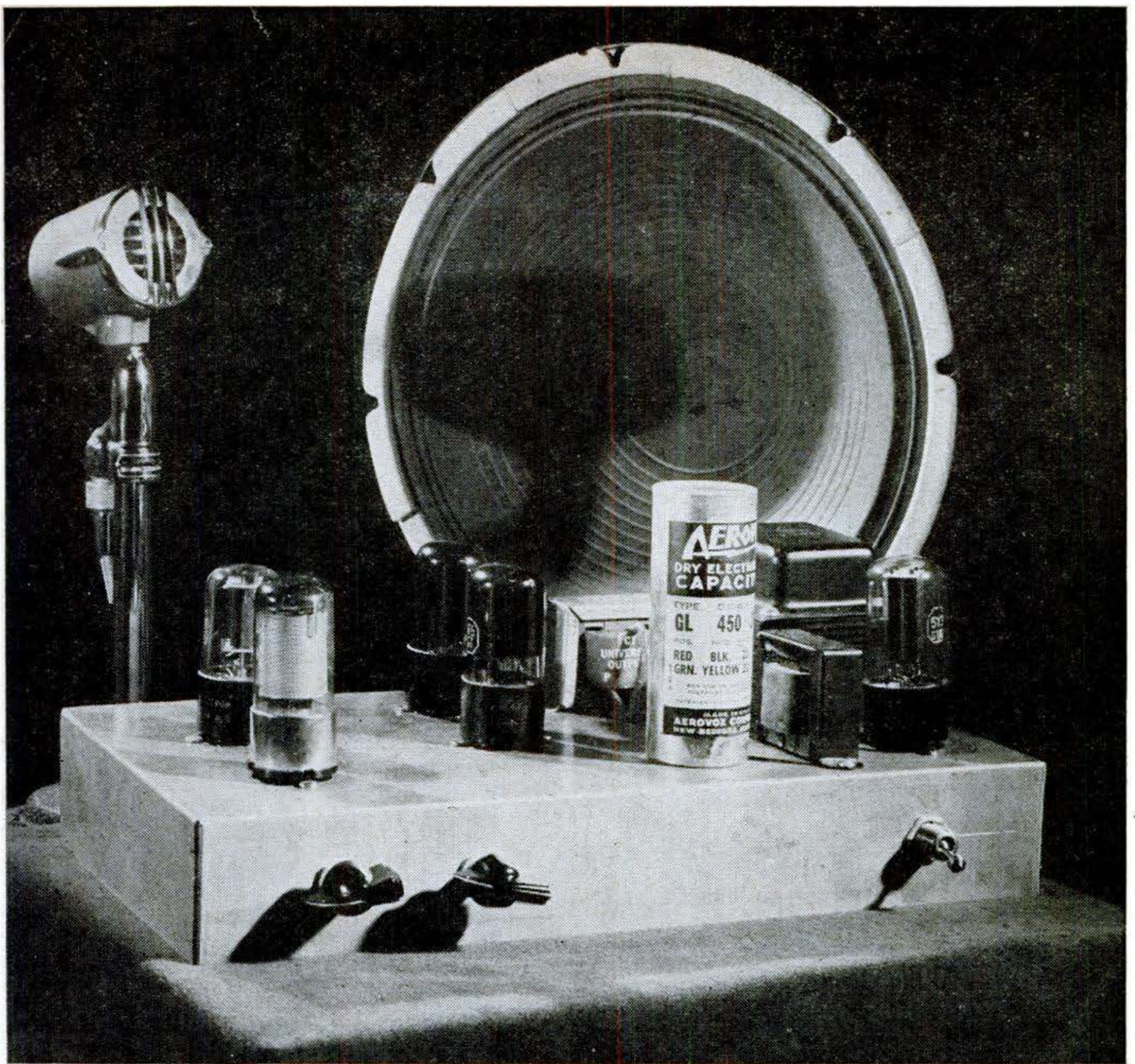
These three units and a carrying case in which the speaker is baffled make a complete portable PA system.
