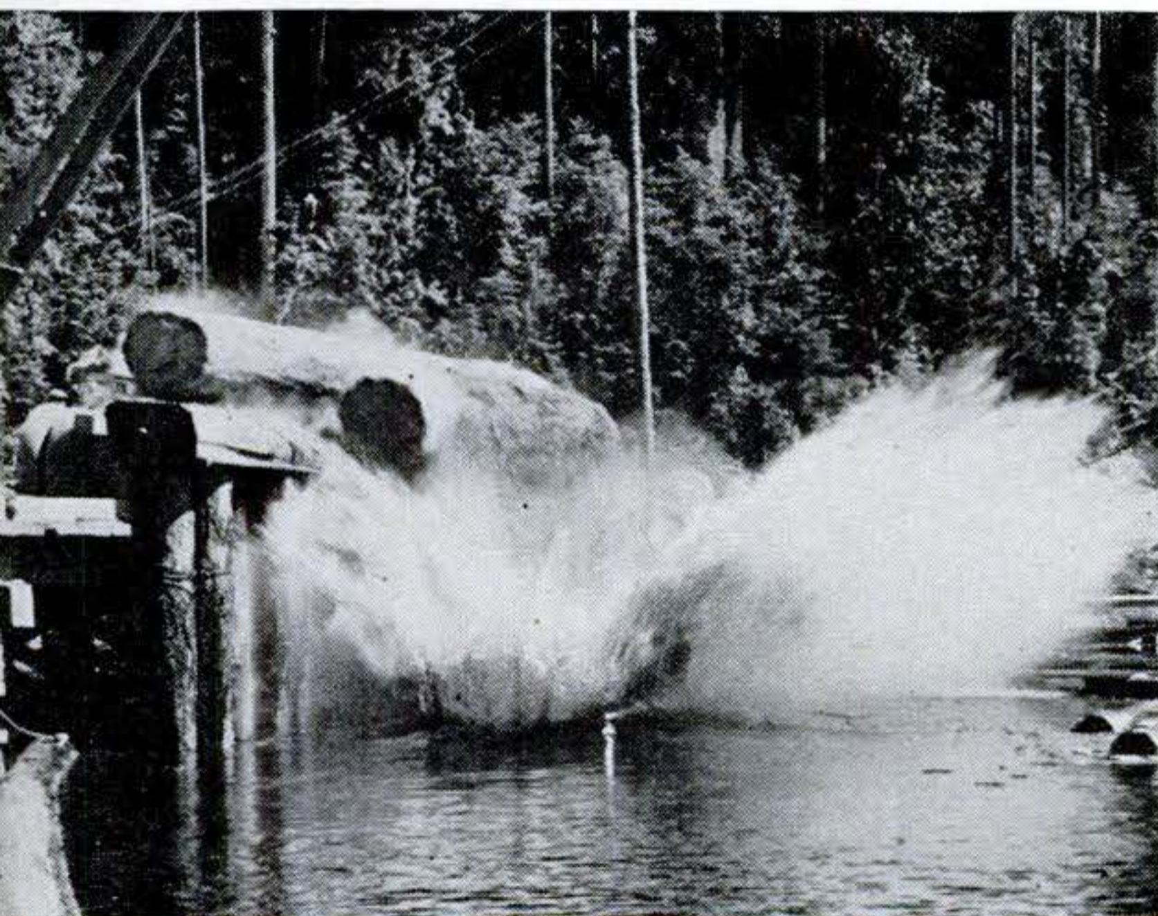
The river, 17 miles farther on, is the end of the trail. The dumper, powered by a gas winch, rolls logs into water, ready for the mill.
