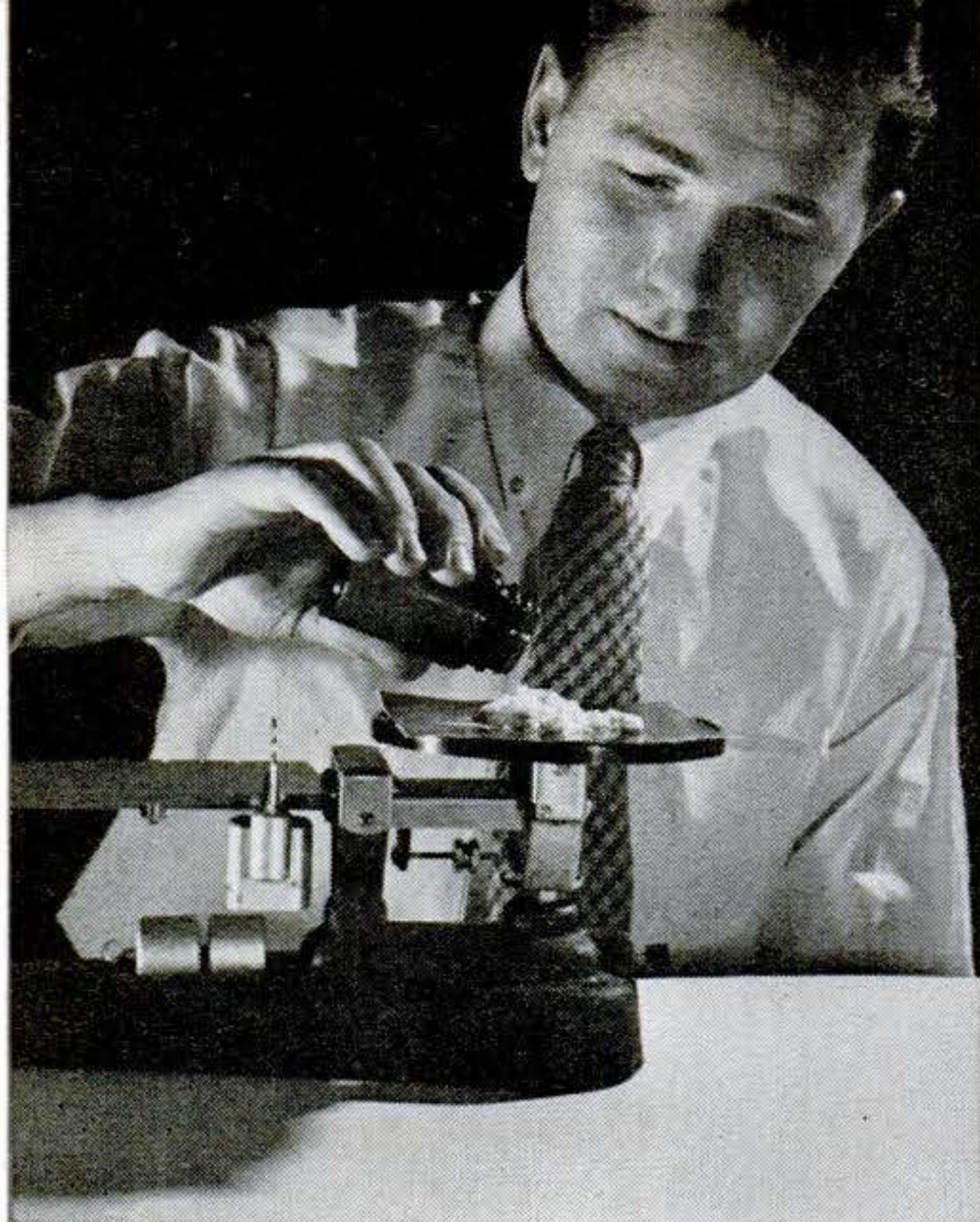
Schramm demonstrates for PSM's camera the method that may lead to artificial fur, meat, textiles and other proteins. Here he weighs one of starting compounds, an amino-acid anhydride.
