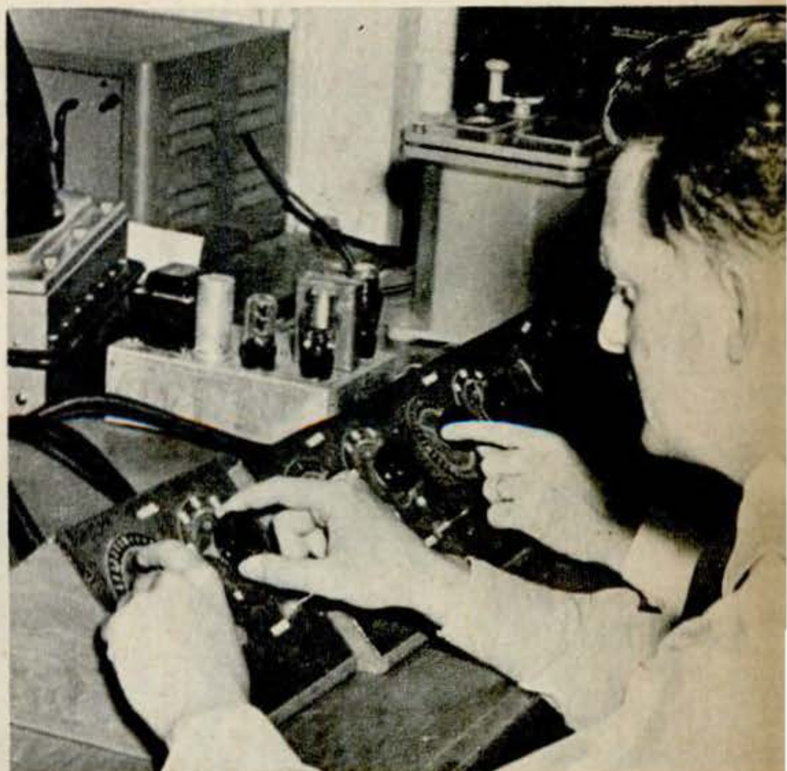
Technicians operate manual equipment also used to control radar images. Real planes are not used as targets, since pilots could not fly same course again to repeat tests.
