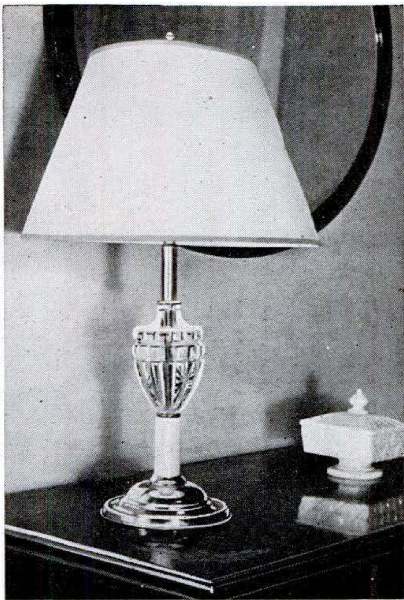
The canopy is the base, plastic tubing raises the glass body, and a brass tube carries the socket.
