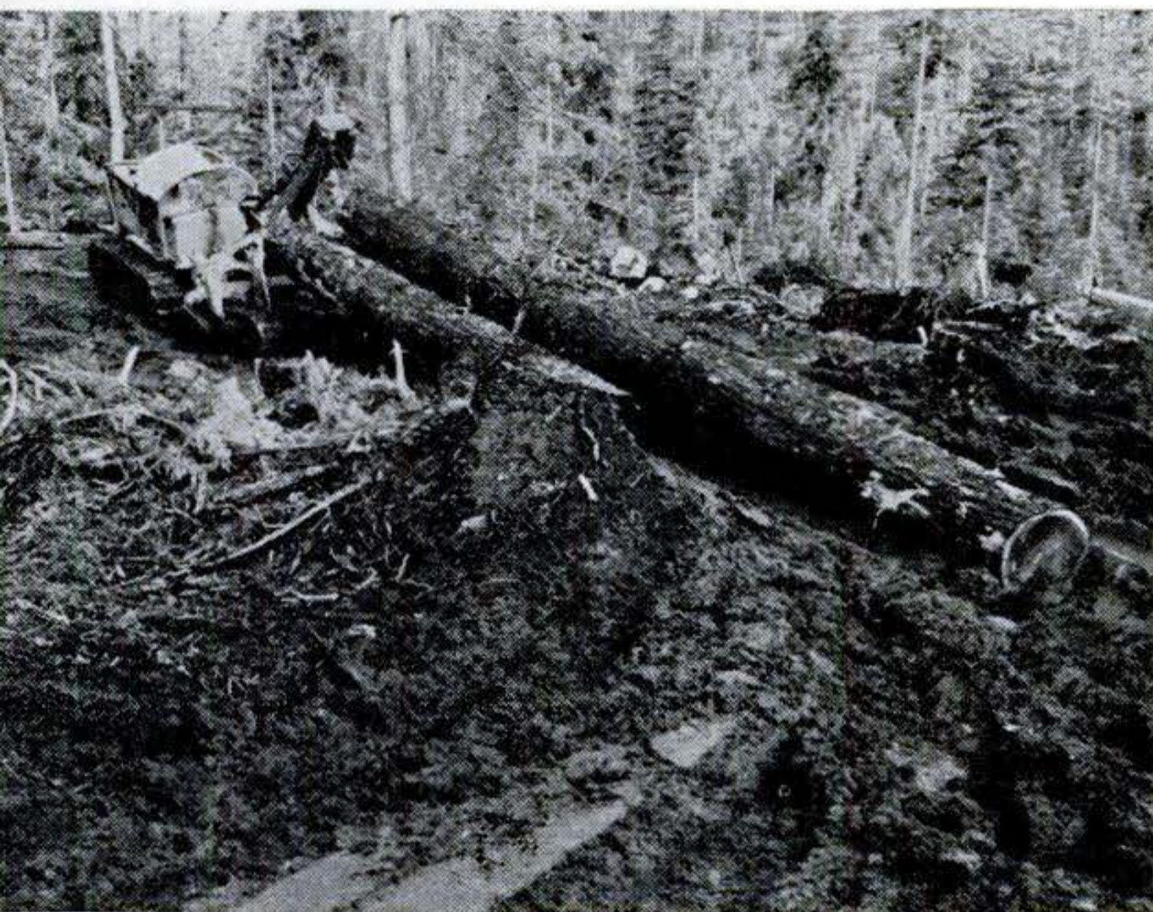
An archeat drags logs to loading point. Arch, on rear of tractor, handles a separate line to each log; it replaces the dangerous high line.
