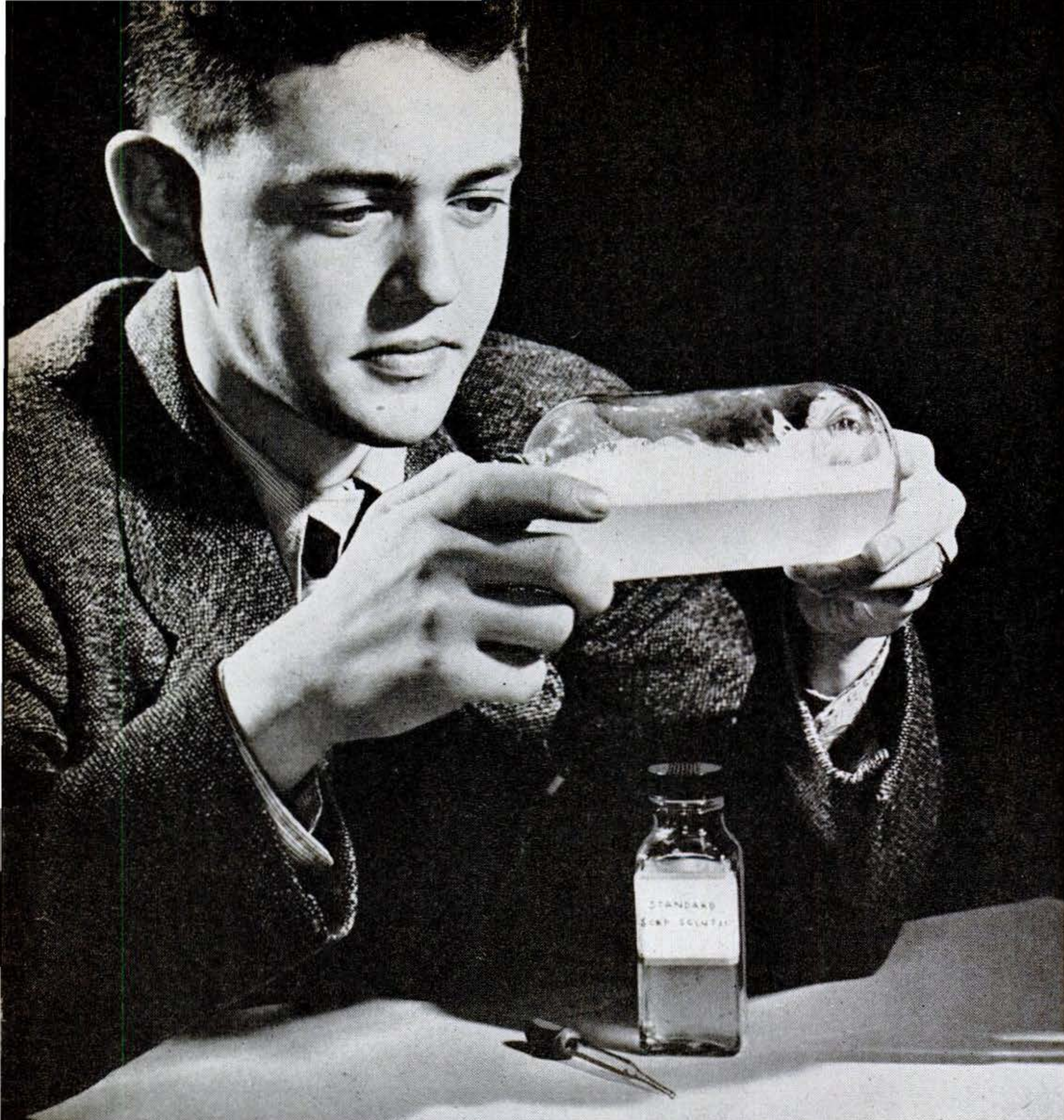
Count the drops of soap solution needed to produce stable suds on the surface of distilled water and on an equal amount of hard water. You then will have an indication of the relative hardness of the latter.
