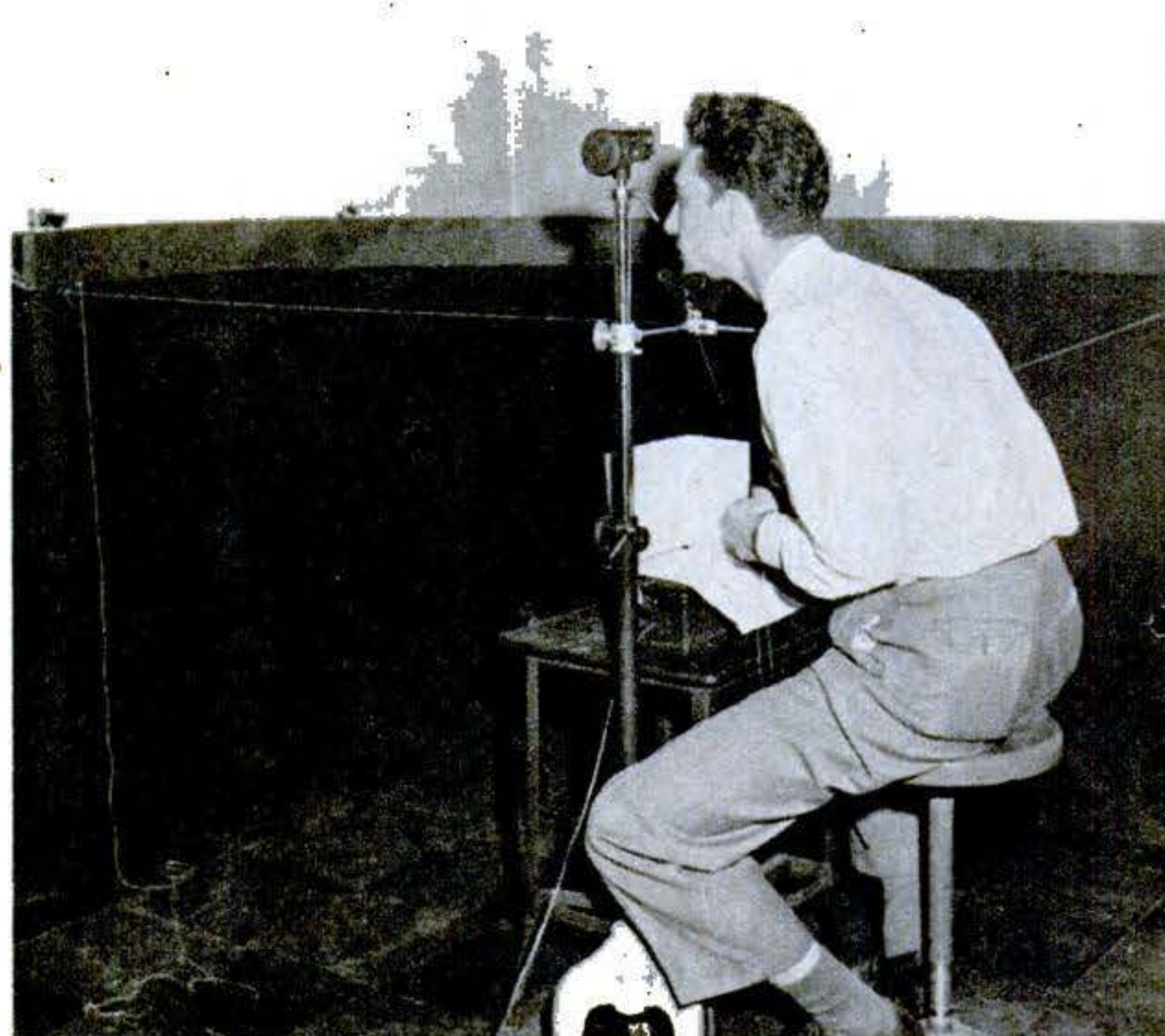
Curved toy train track (hidden behind black paper) and cars bearing tiny lights measure ability to estimate angles—important for operators of complex control panels.
