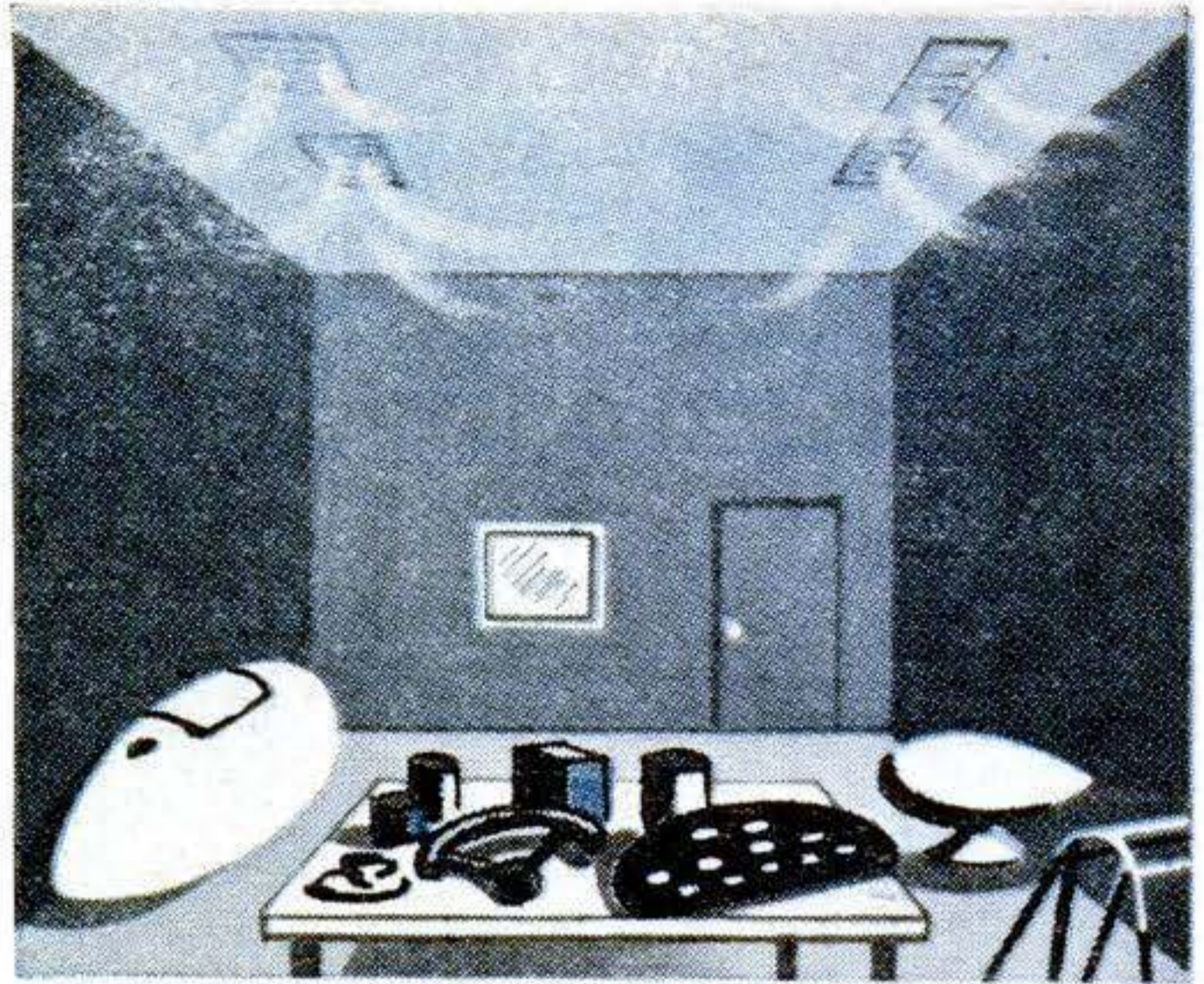
Hot test room provides temperature up to 165° and humidity as high as 95 percent for small-scale trials, as of plastic aircraft parts and food packaging for torrid climes.
