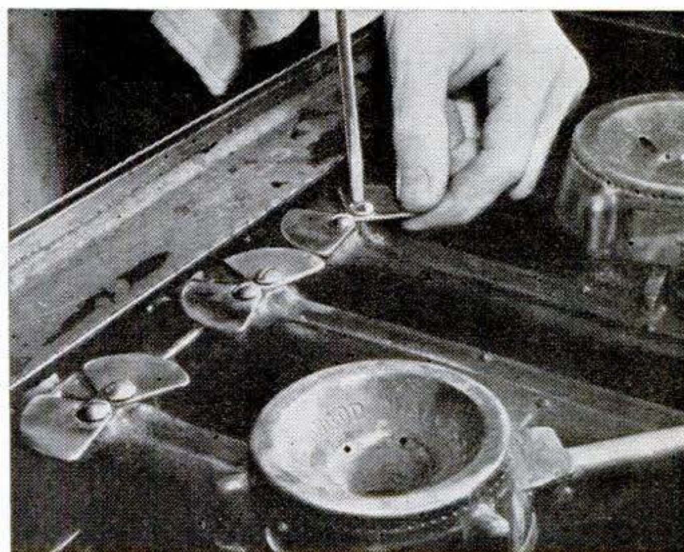
Another type of burner has an air adjustment in the form of a shutter on the end of the base and also requires loosening a screw. The one shown has a high- and low-flame valve for each burner.
