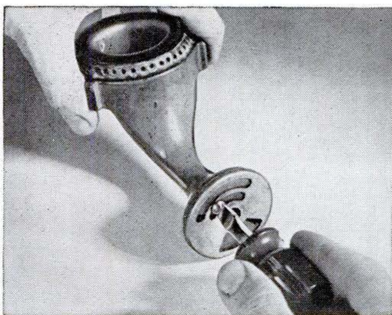
One simple, common type of burner has a rotating shutter to admit air. It can be adjusted when a screw is loosened. After the correct setting has been made, retighten the screw carefully.
