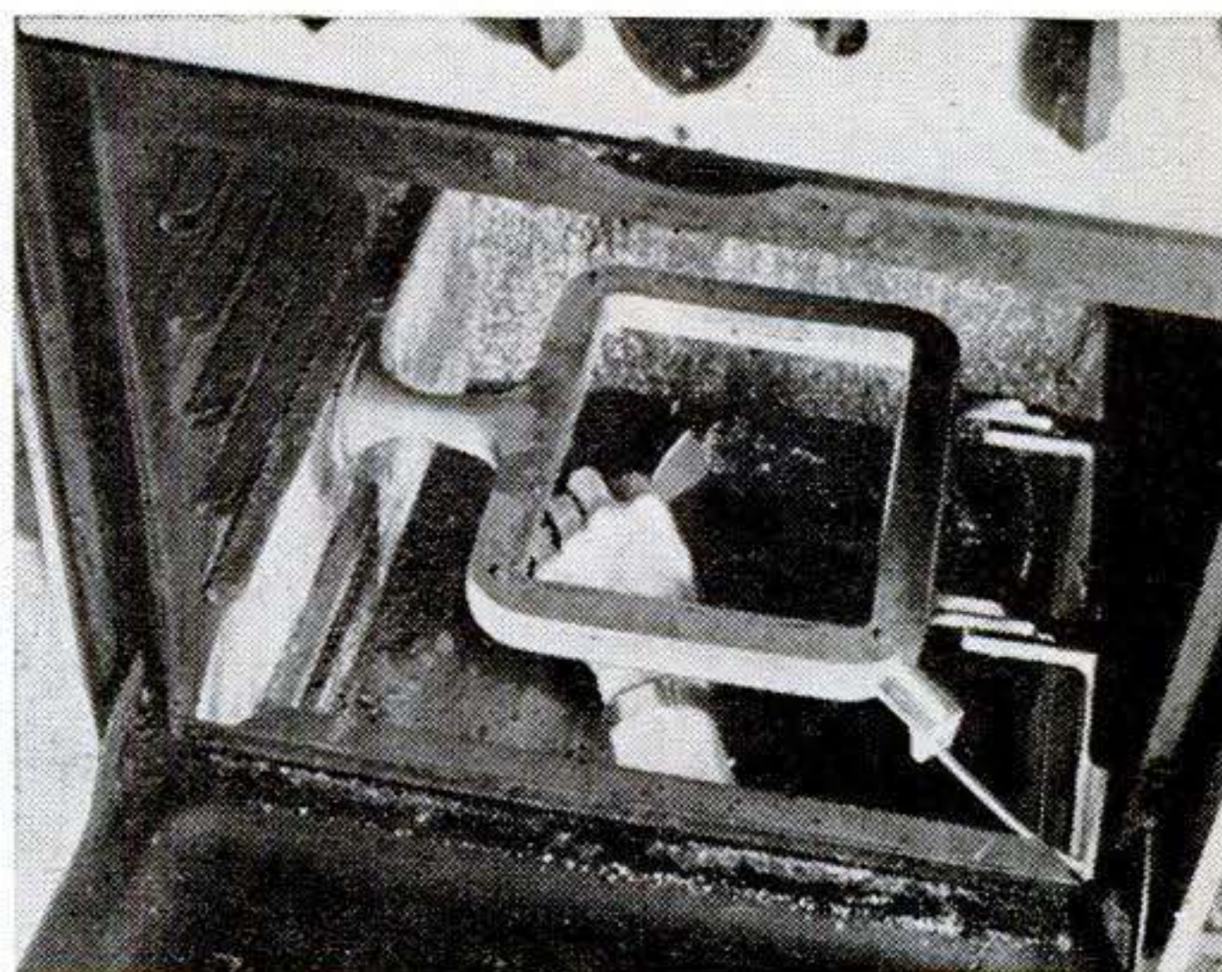
With the bottom, broiler pan, and racks removed, an oven can be scraped of batter and grease. The burner, being inverted, rarely requires cleaning. Adjust it like the top burners. [Turn the page.]
