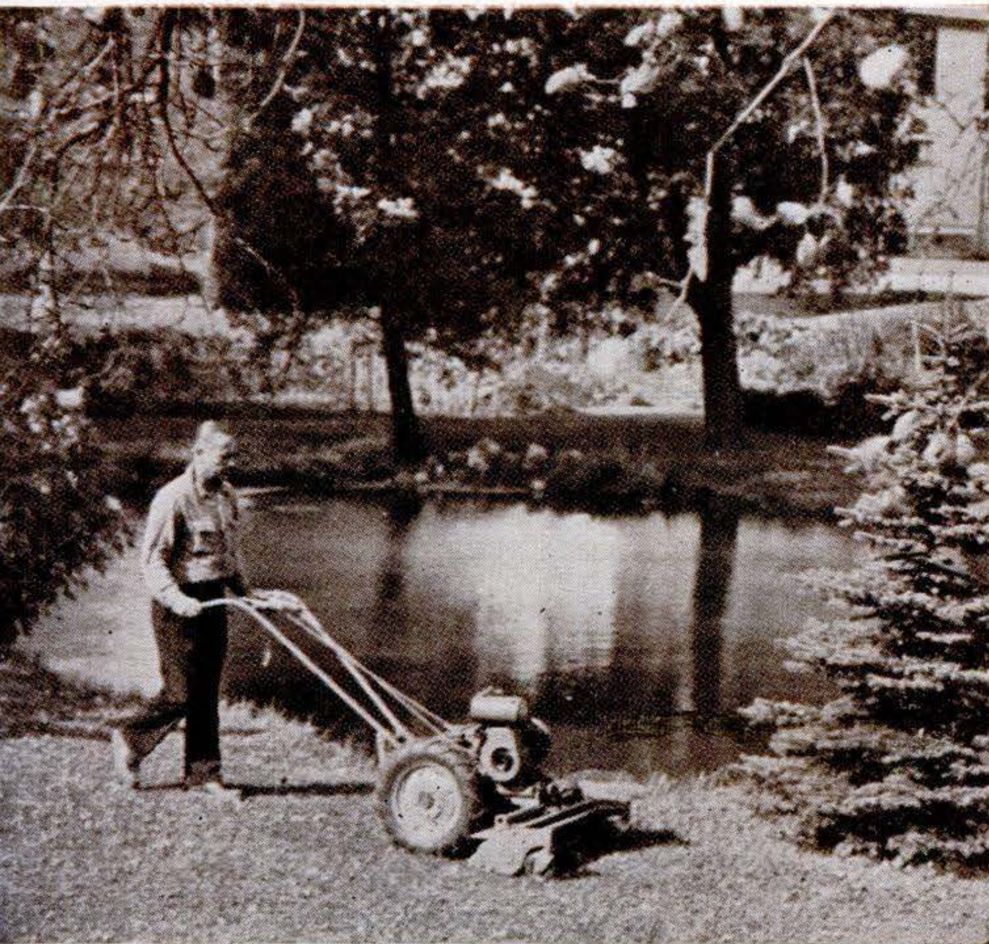
For easy grass cutting, a simple conversion job turns a Bolens garden tractor into a reel-type power mower.
