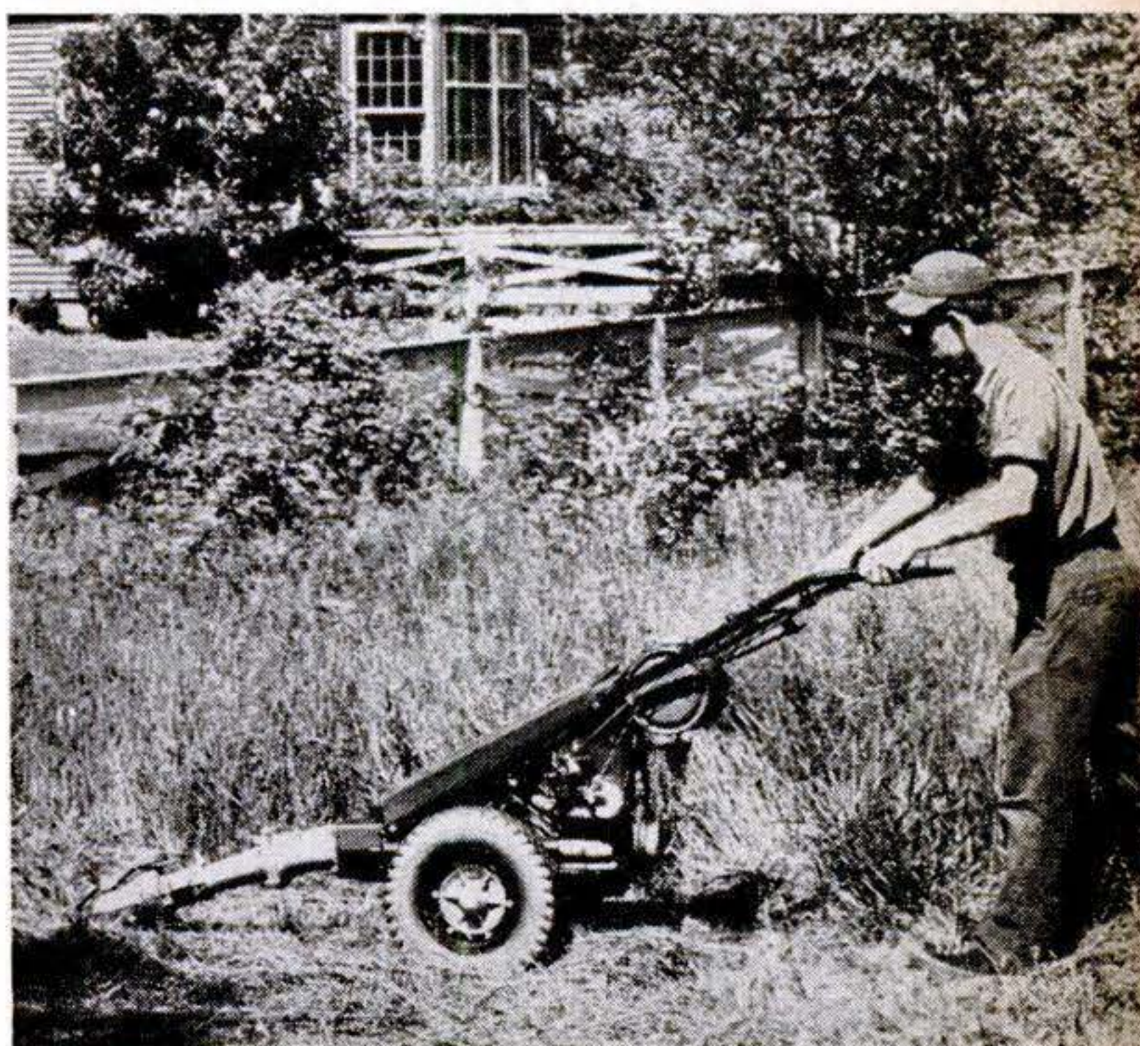
With 42-inch sickle-bar mower attachment, the Gravely 5-hp. tractor works in heavy growth. This machine has plenty of power in terrain where a smaller 1½-hp. job would have trouble.
