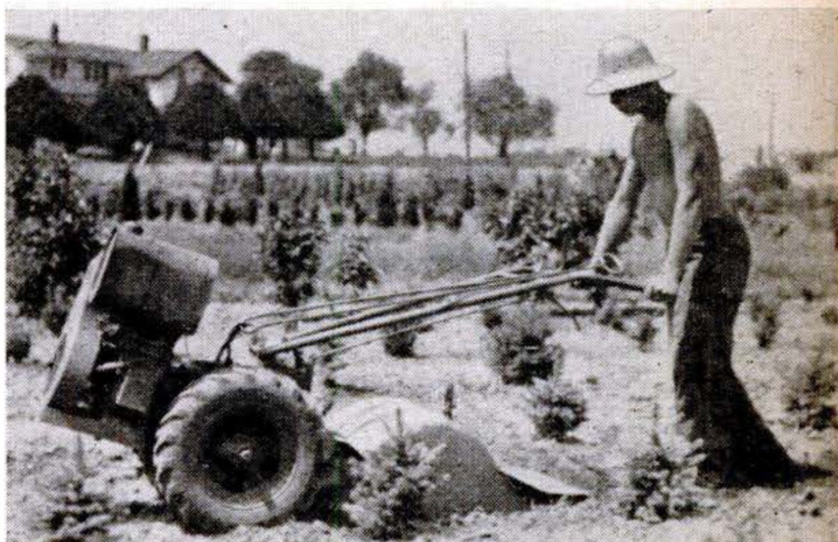
Ariens rotary garden tractor (above) is a competitor of the Roto-ette ® , shown on opposite page. It uses spinning rotor and hooked teeth to plow, disk, and harrow in one operation.
