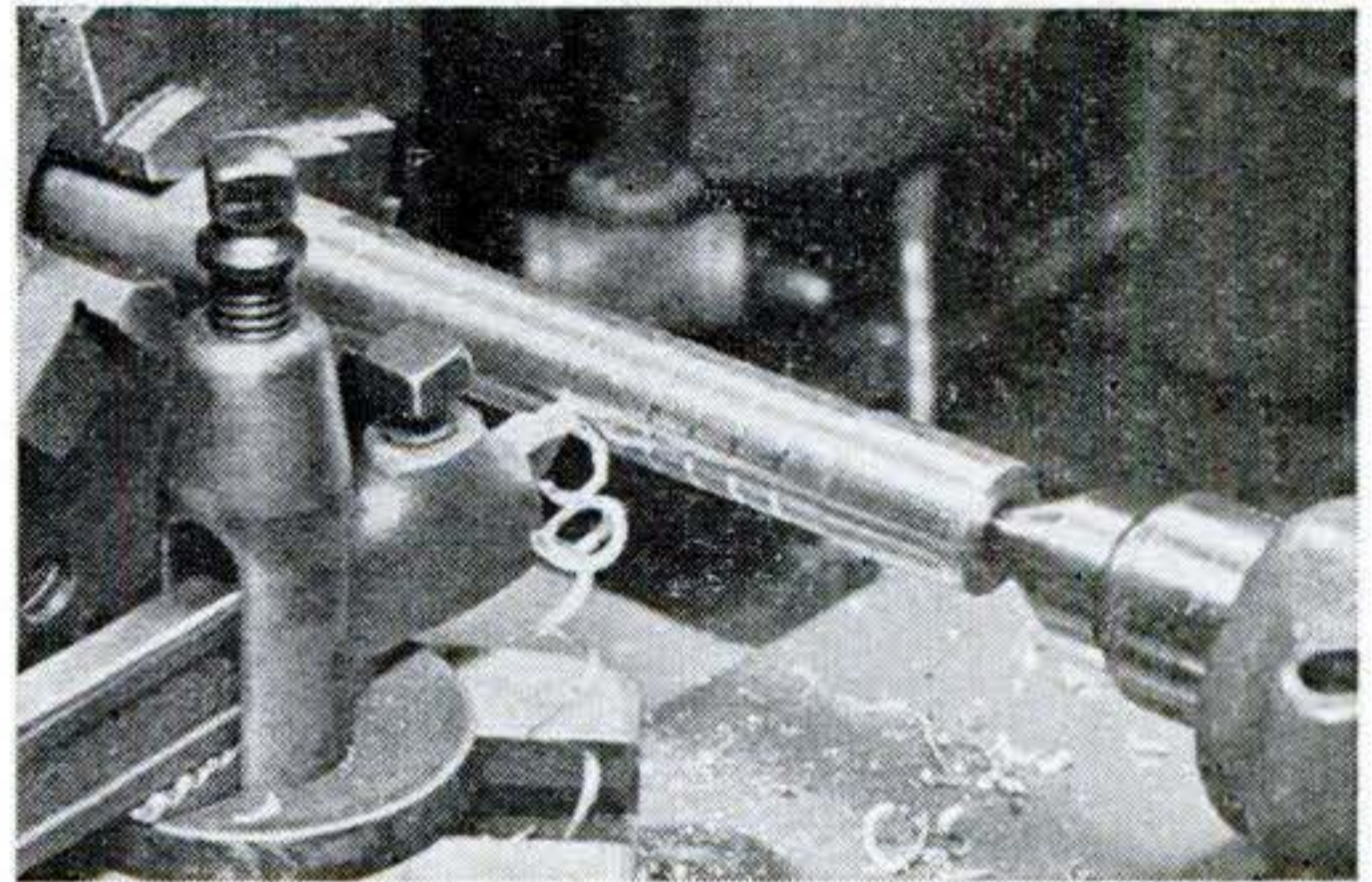
This handle was turned from aluminum rod, but plastic, wood, or other materials can be used.
