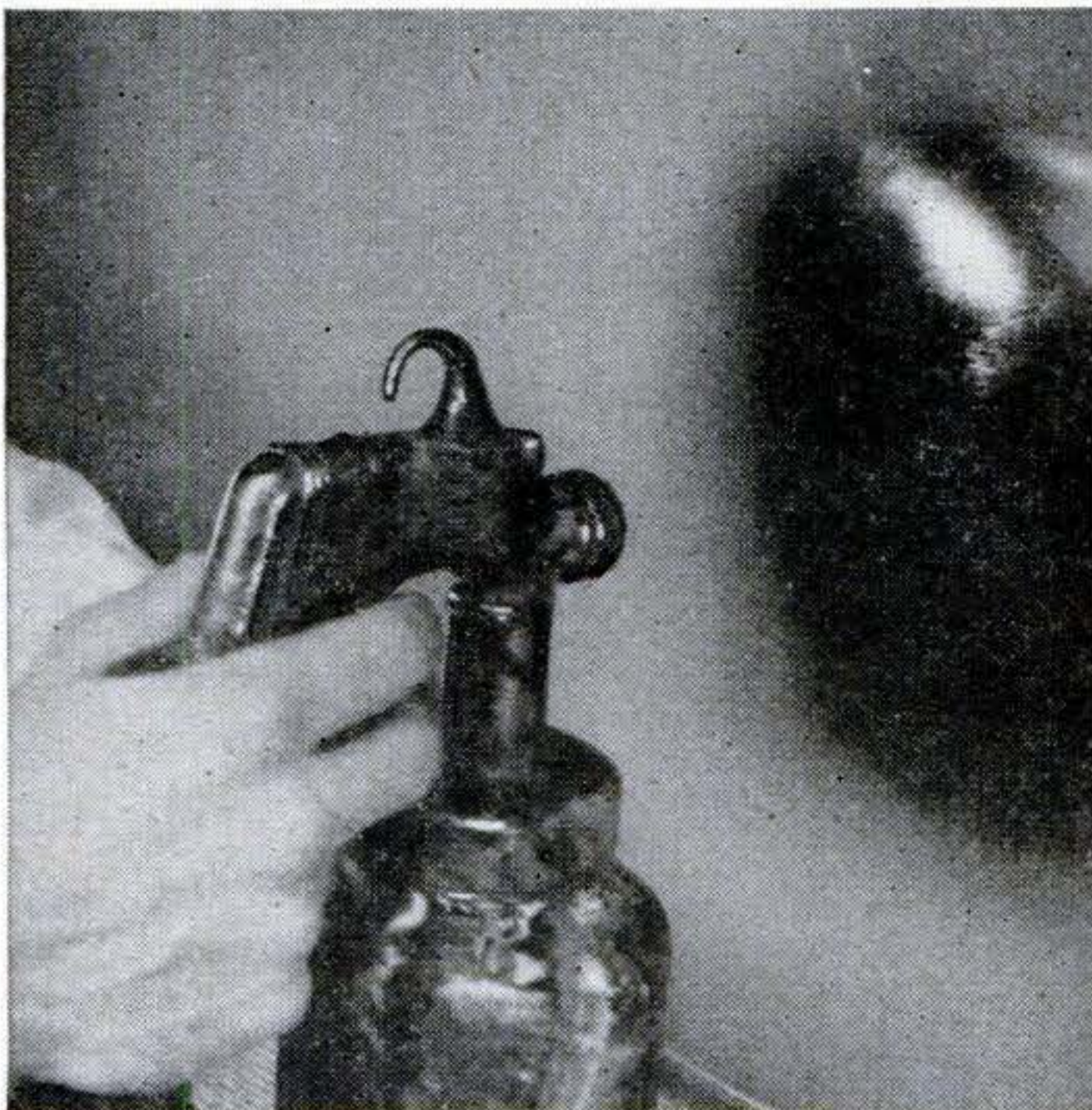
Lay a smooth surface for the finish coat by applying the primer with a spray gun. Follow the priming coat with wet sanding. You'll get a better job by refinishing the entire fender.
