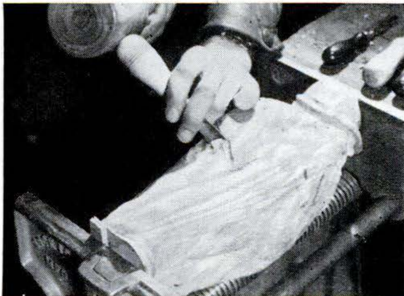
Rough the figure with a gouge; then work in the full details with a flat chisel or carving tools.
