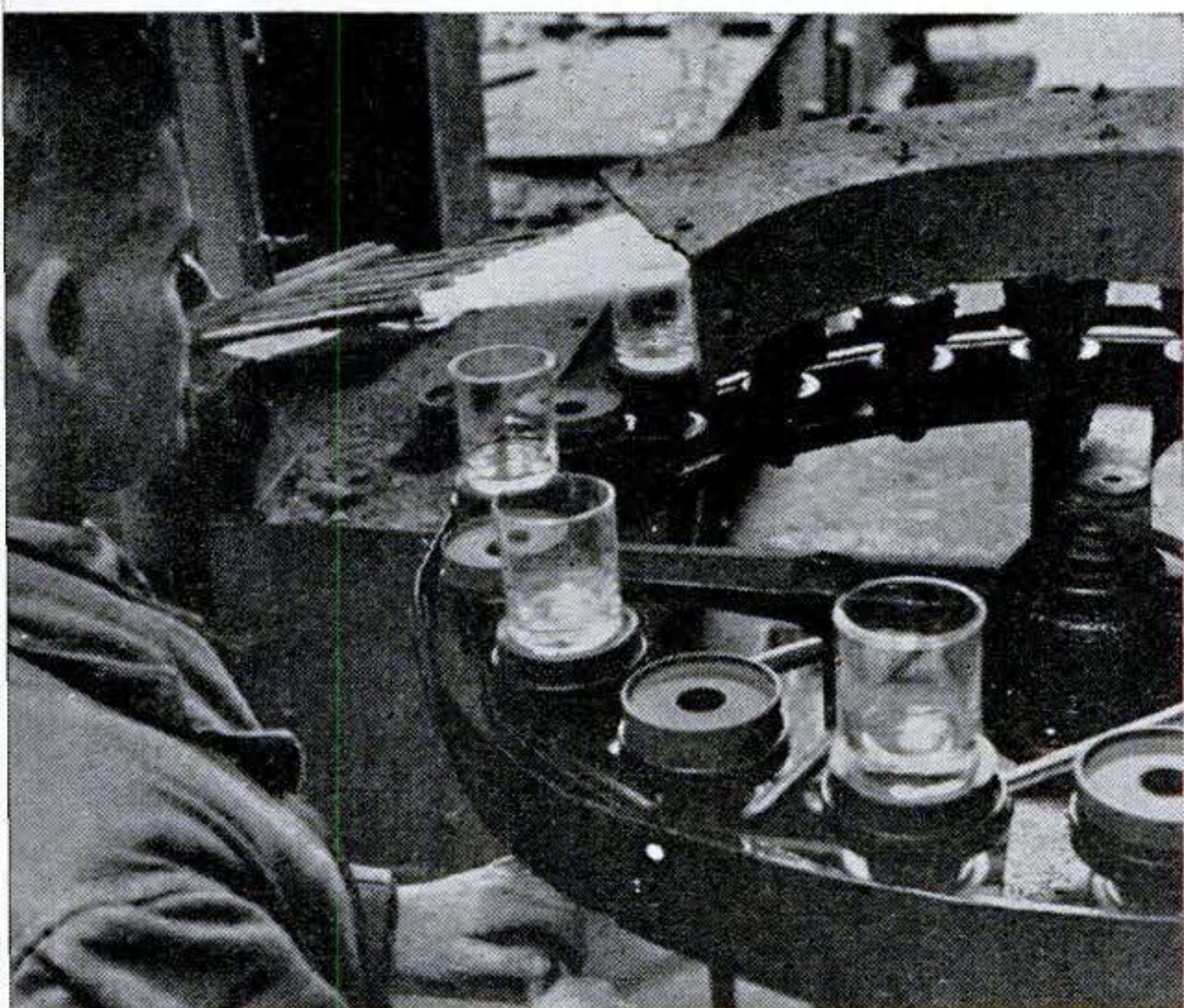
A battery of flame guns , left background, glaze the ground tops of tumblers. While faster than the "off-hand" or handmade method, this newer process produces a less perfect finish.
