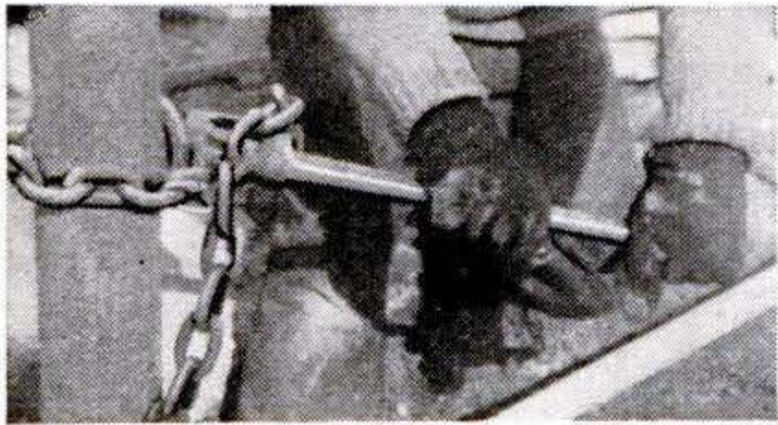
Loop a sturdy chain around the pipe and fasten it as shown at the right.
