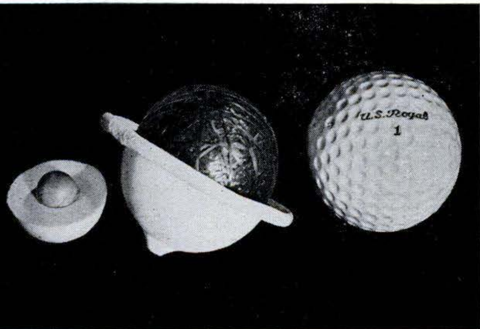
Lively golf ball uses pea-sized pellet of bouncing putty in rubber core (left). Wrapped in rubber thread, core rests in half of balata cover (center). Cover is then vulcanized (right).
