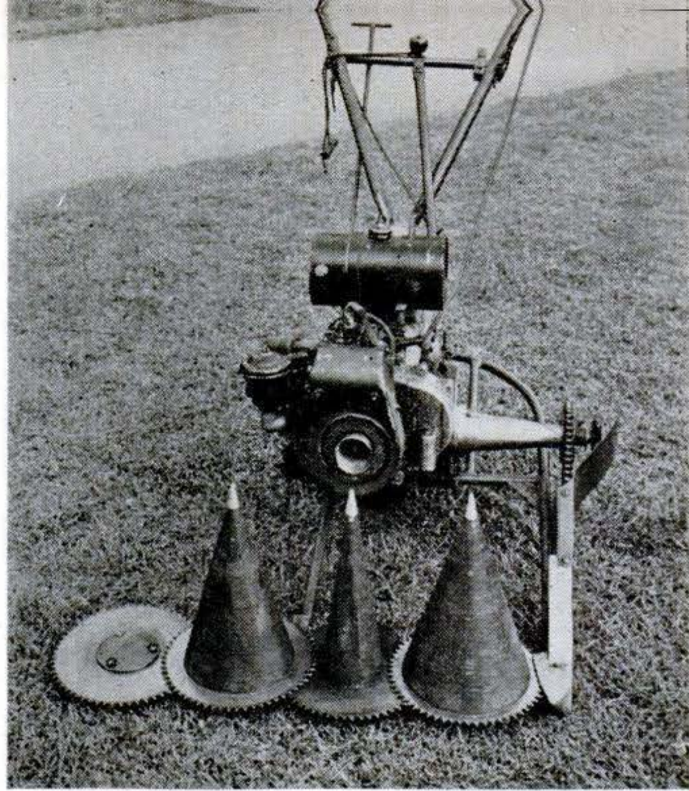
Spinning saws of Roto-ette ® field mower, shown in foreground above, cut weeds and small trees; the revolving dunce caps throw the cut material out at side. Mower attachment: $160.
