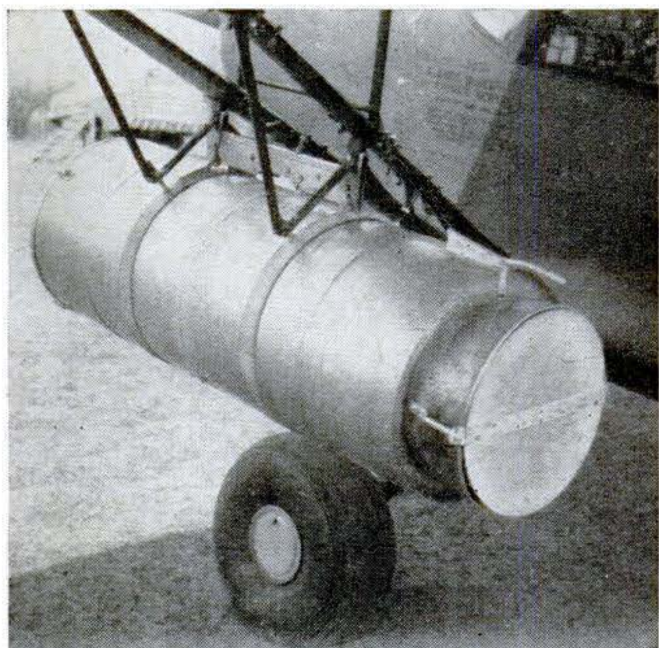
Signal Corps' new wire dispenser lays telephone lines from speeding airplanes, trucks, and even rockets. It is shown above mounted under the wing of an L-5 liaison plane.
