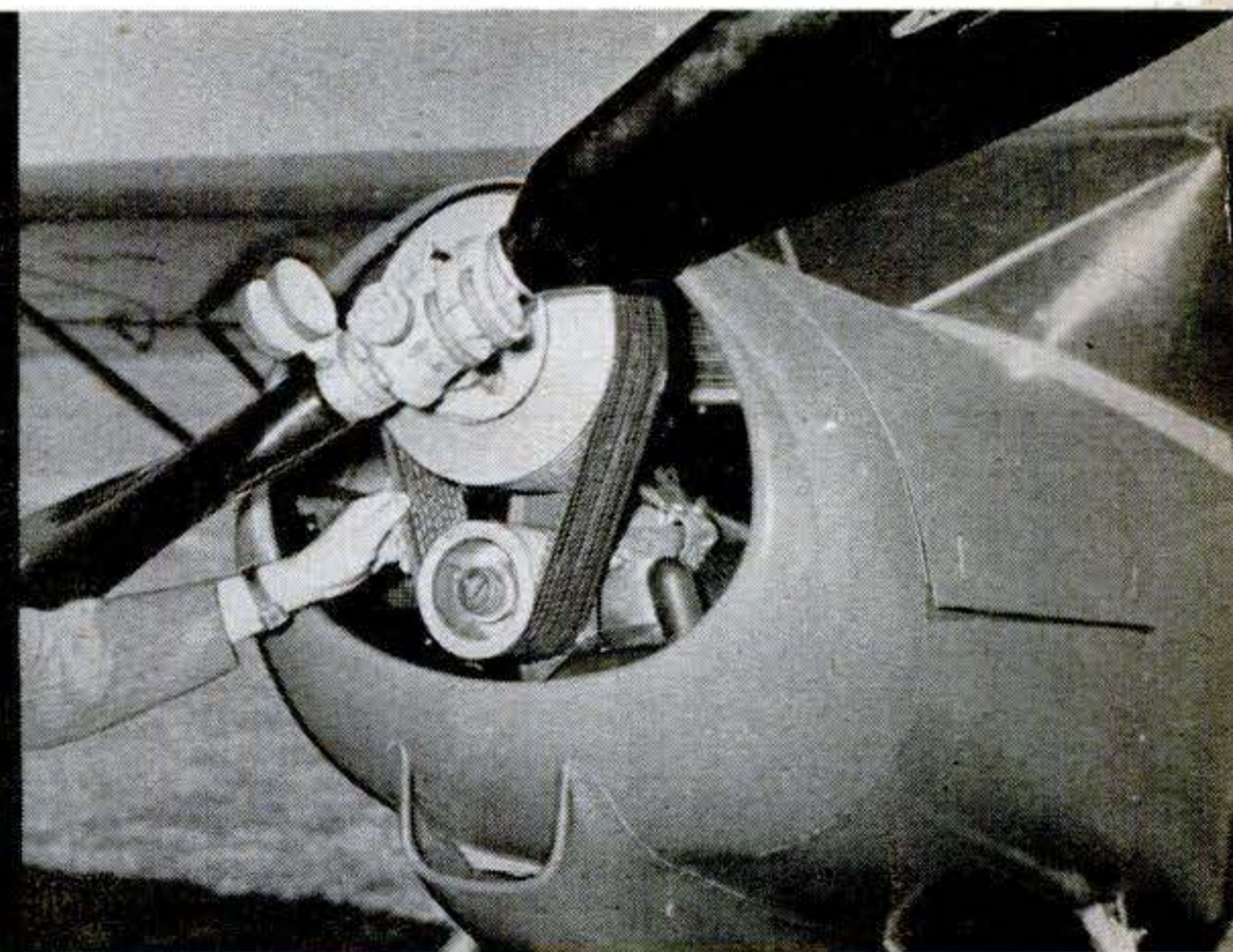
Reduction gear lets engine turn 2.3 to 1. Prop turns 1,200 revs maximum and 1,080 at cruise. Inventors stress that the minimum speed, unlike most planes', is above wing's stall point.
