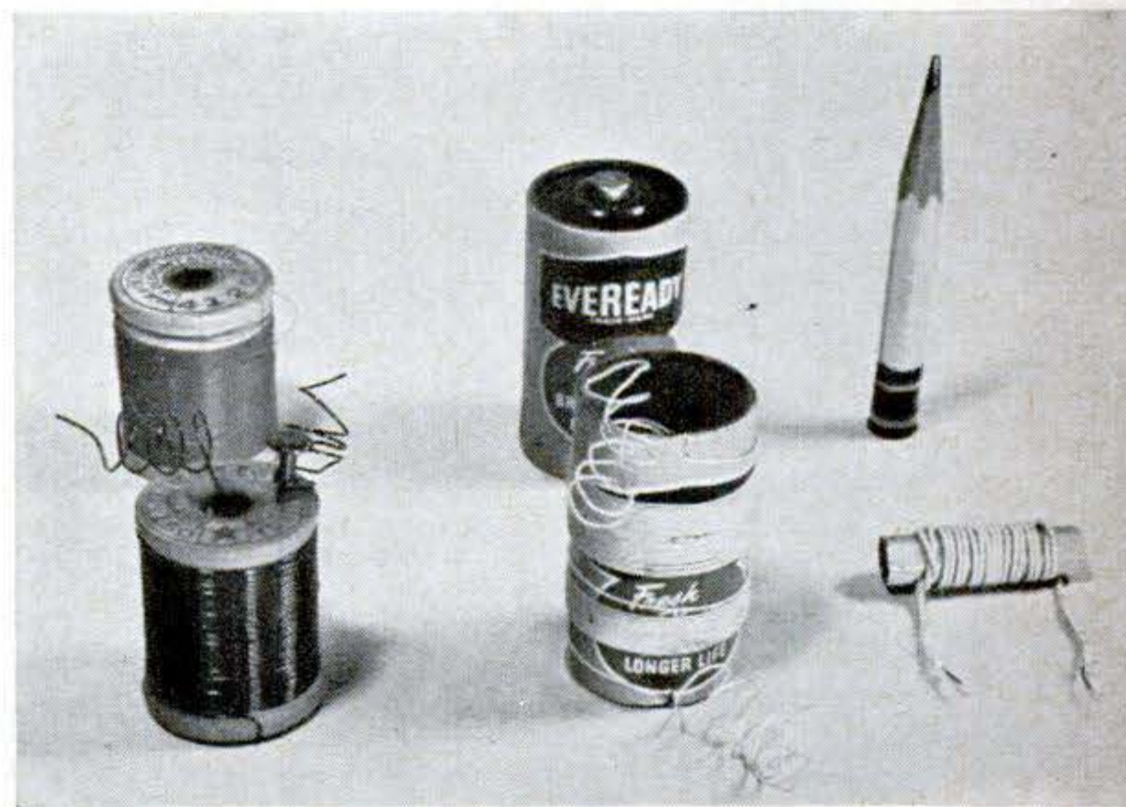
4. Coil forms can be improvised from many common objects. Windings must, of course, be figured in relation to diameter of the form. ➔
