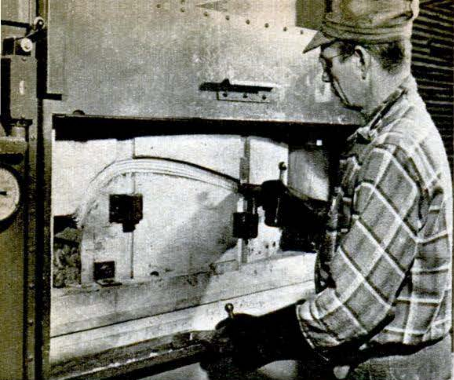
Here workman removes guides around mold before applying current. He will then pull down copper shield, enclosing mold, to prevent harmful radiation. Molds are made of wood to provide good insulation against loss of heat and energy.
