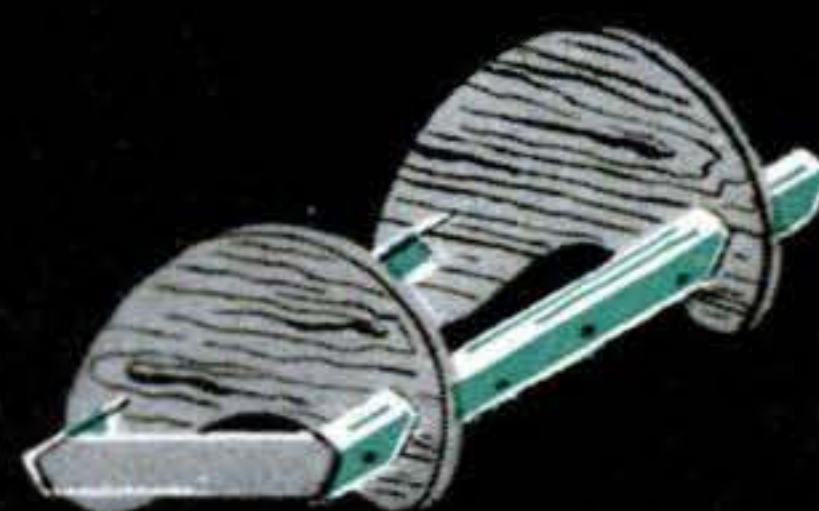
Telescoping book ends are made with stair nosing sliding in slots in plywood ends.
