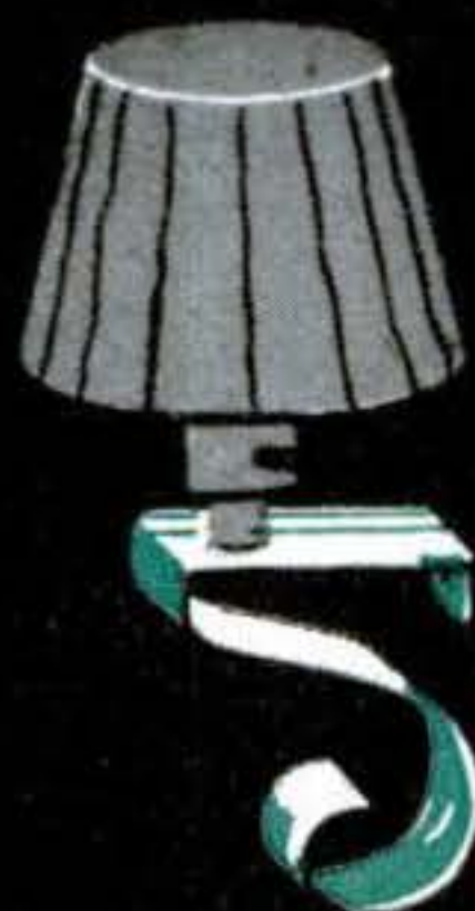
Bracket for wall lamp is bent from length of flat molding and screwed to wall.
