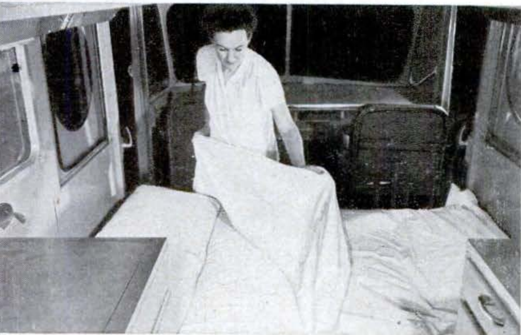
Seat backs bridge aisle to make a comfortable double bed. Rear aisle is big enough to sleep a third adult on an air mattress. A bunk for a child can be fitted at front of the vehicle.
