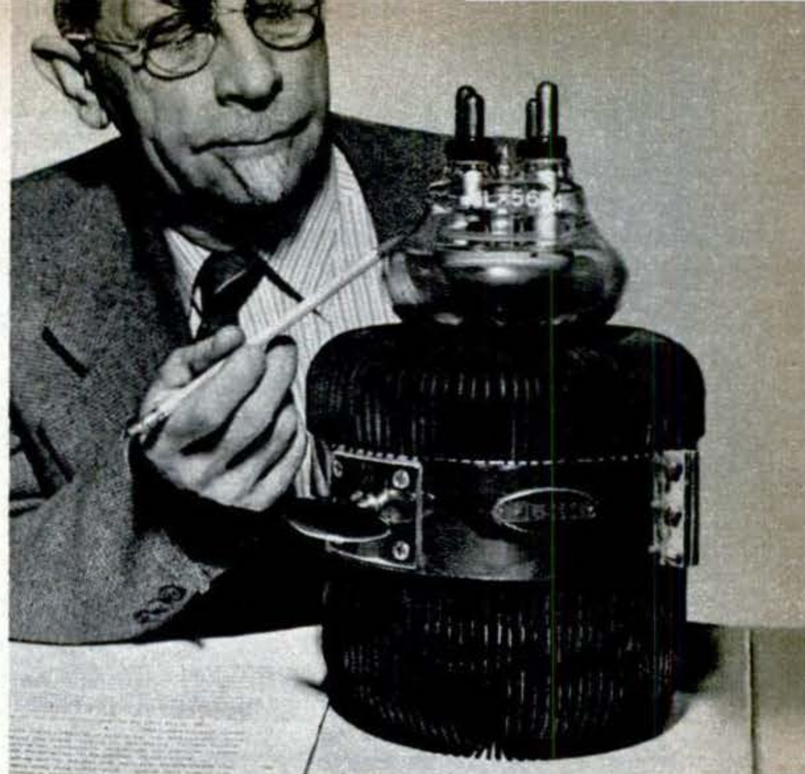
Radio waves for heat bonding are produced by this high-frequency generator, an oscillator tube with a tuned circuit consisting of coil and condenser. Fins around edge are for air-cooling.
