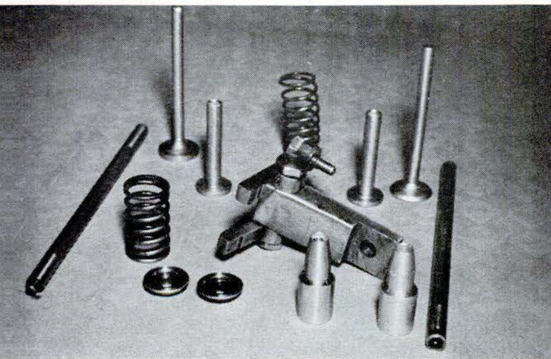
18 Pushrods, guides, and rockers are all straightforward machining jobs, starting from bar or flat cold-rolled stock. Springs are wound from .062" and .080" music wire.
