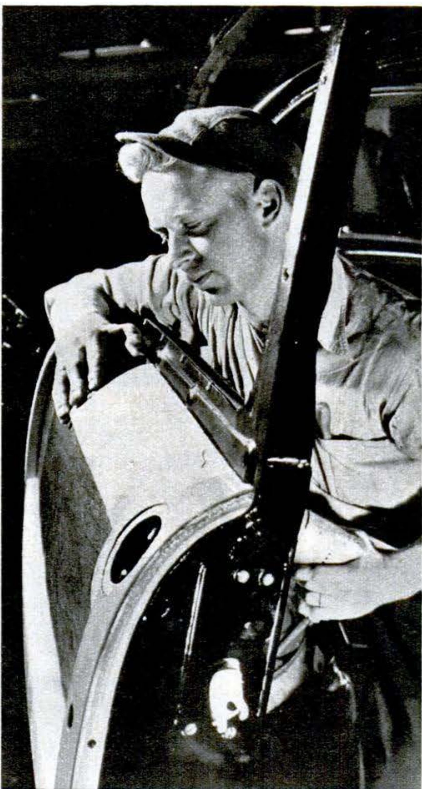
Plywood panels are bolted directly onto outside of all-steel underframe to form station-wagon body. Panels are so attached that individual sections can be removed and replaced if damaged. Phenolic-resin glue in panels makes moisture-resistant bond that's stronger than wood itself.
