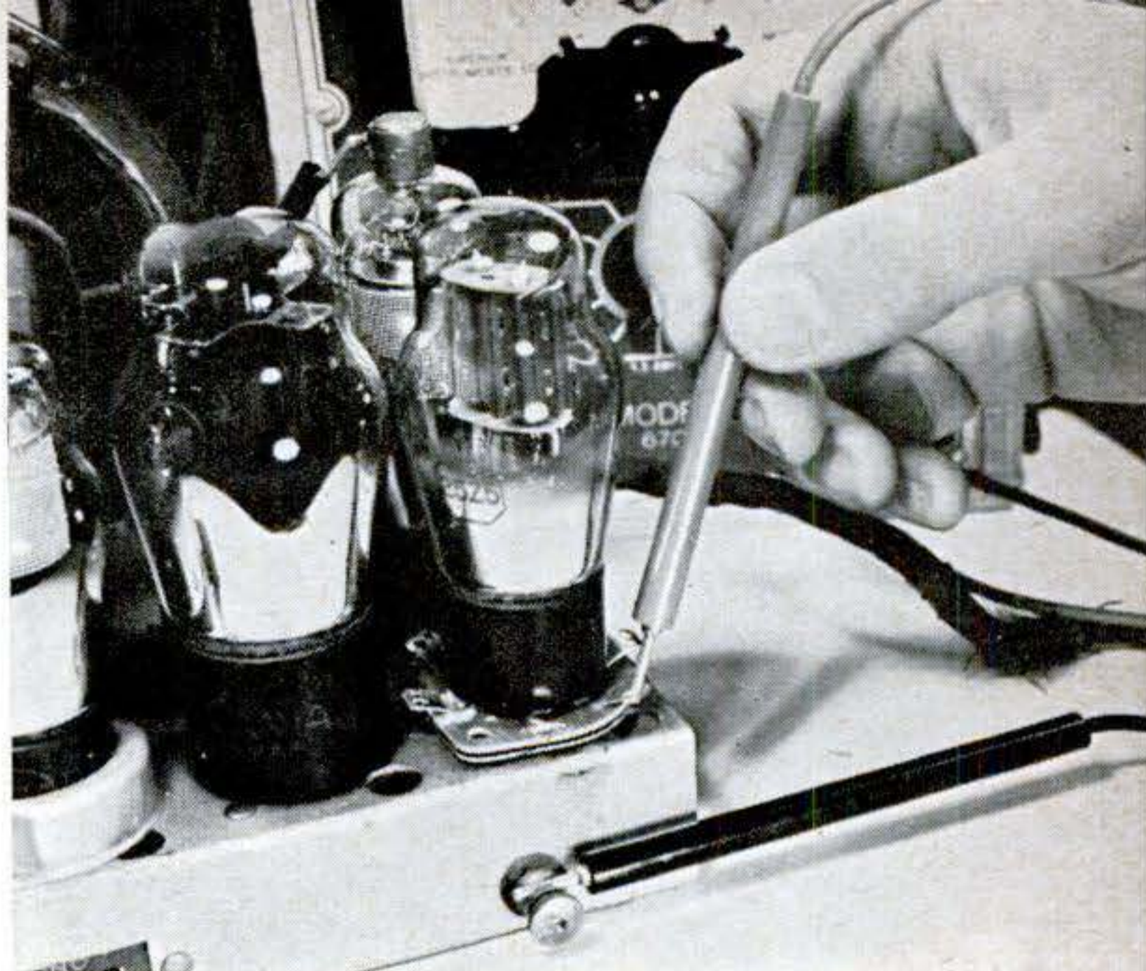
2. Test-point adapter, easily made from wafer tube socket, allows you to check voltages at the tube instead of turning chassis over.
