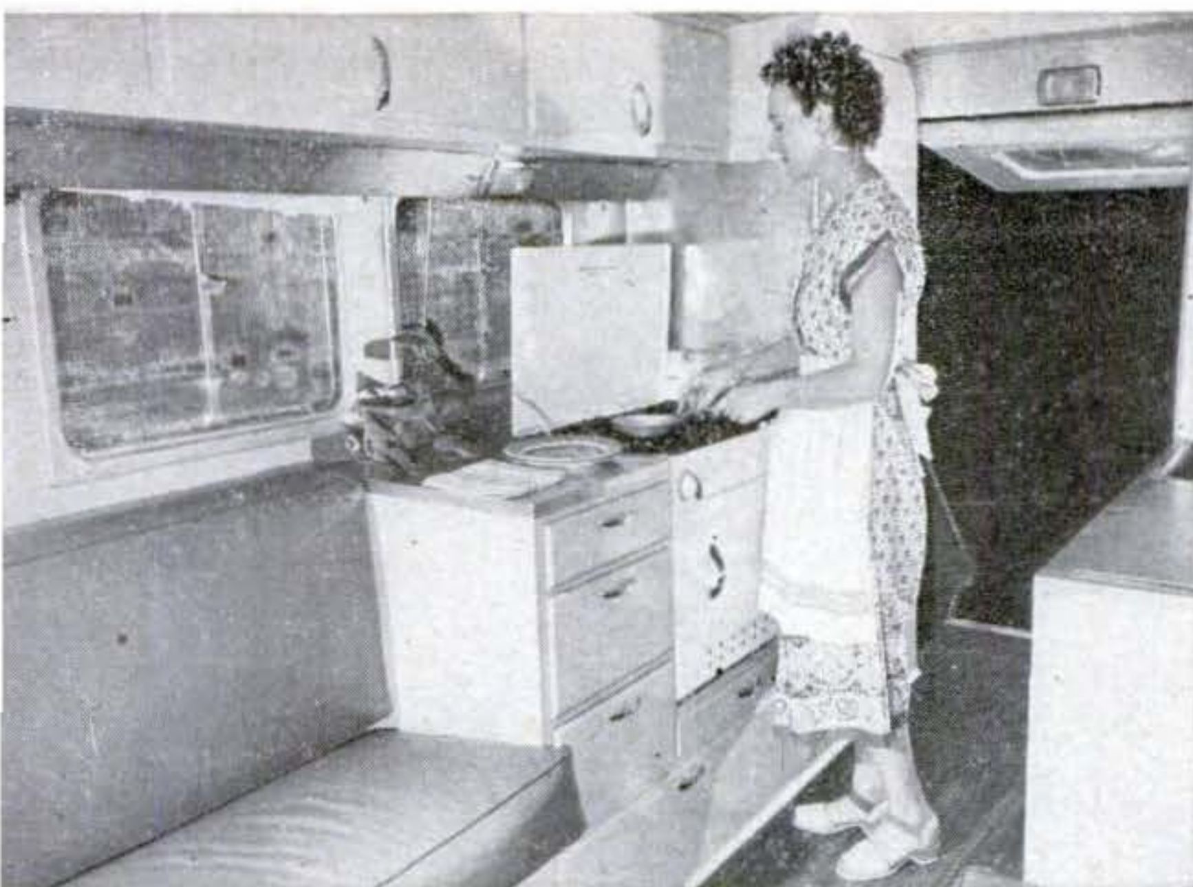
Good meals can be cooked on the three-burner gas range with temperature-controlled oven. Exhaust fan is in locker overhead. Icebox, sink, and more storage space are in counter at right.
