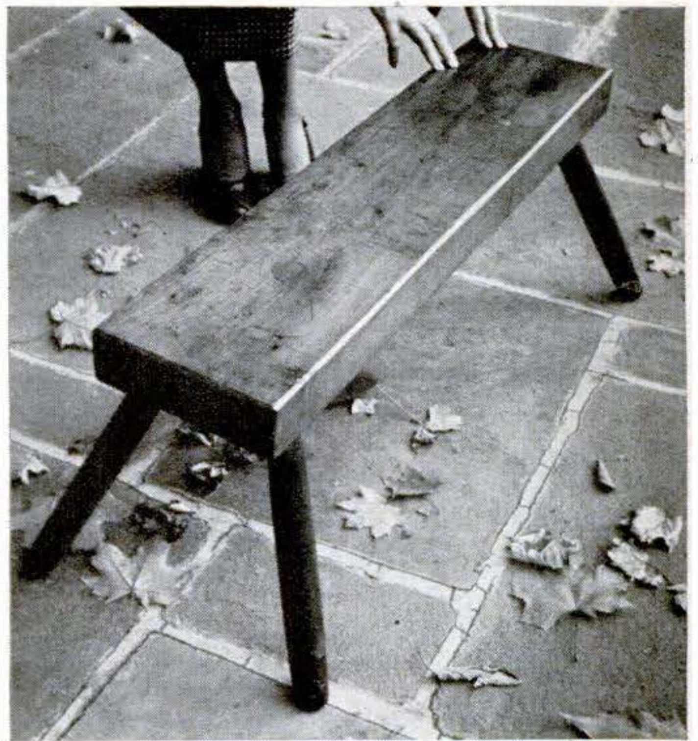
Long enough to seat two, this sturdy bench was made from a billet of used lumber. Note that previous holes in the plank were filled.
