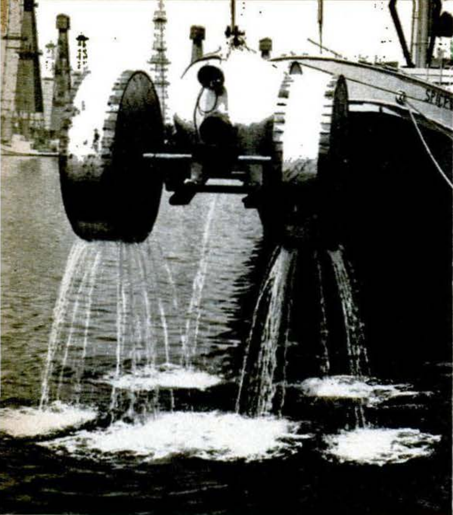
Barton's bathysphere is hauled up by cable after 340-ft. test dive at Long Beach, Calif. Two powerful, externally mounted searchlights give illumination within a radius of 10 feet.
