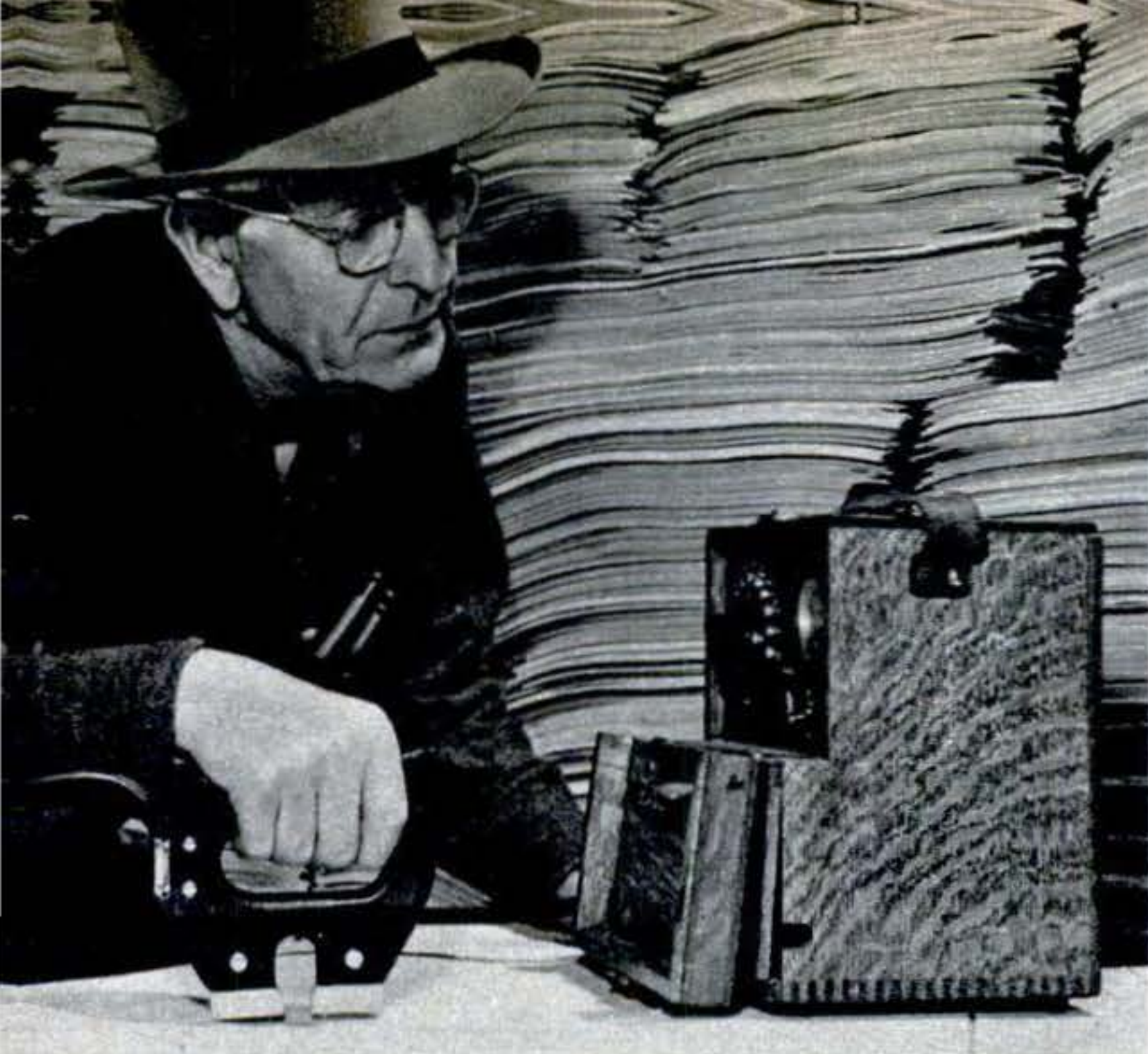
Raw plywood veneer is first checked for moisture content, which must be just right, by instrument that pricks wood, measures electrical conductivity, records amount on sensitive meter.
