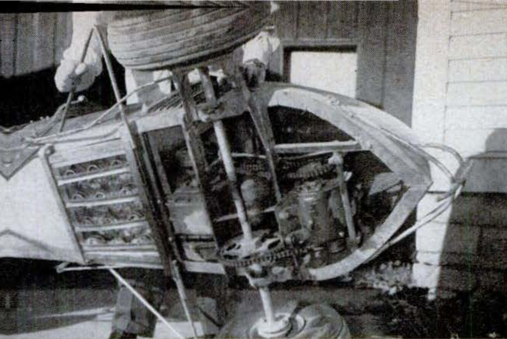
Underview of the same car shows how the frame was curved by notching, bending, and welding the flanges of steel angle stock. Note the coil seat springs and the steel wheel guards.
