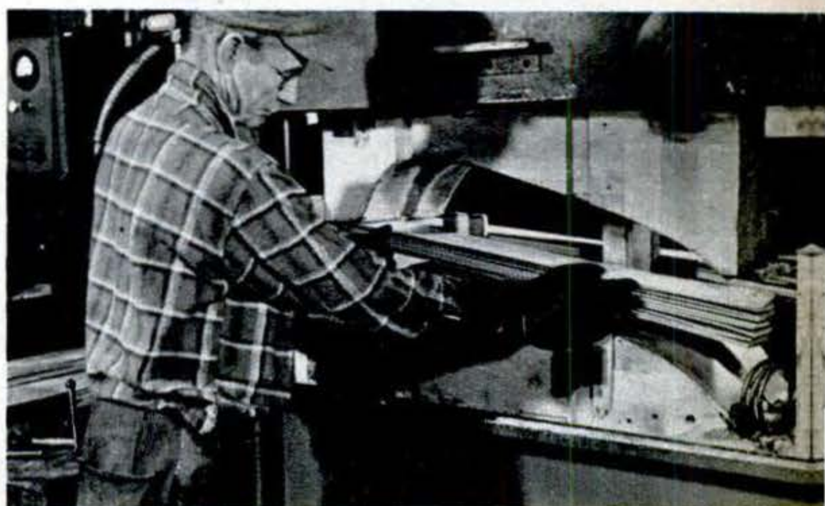
Loosely stacked, glued "sandwich" of veneer sheets for door-frame pillar now goes to forming mold. Pressure of 350 to 375 lb. per sq. in. will be applied hydraulically from above and below.
