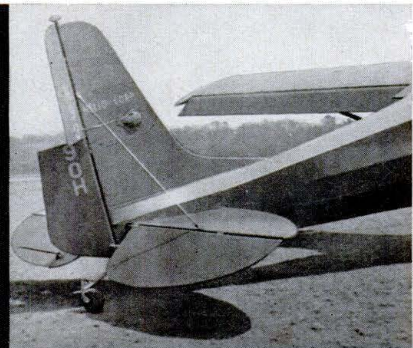
One of plane's neat problems was yaw at low speed—tendency to turn opposite to bank. This was remedied by splitting rudder. Bottom half is linked to ailerons, top half to rudder pedals.
