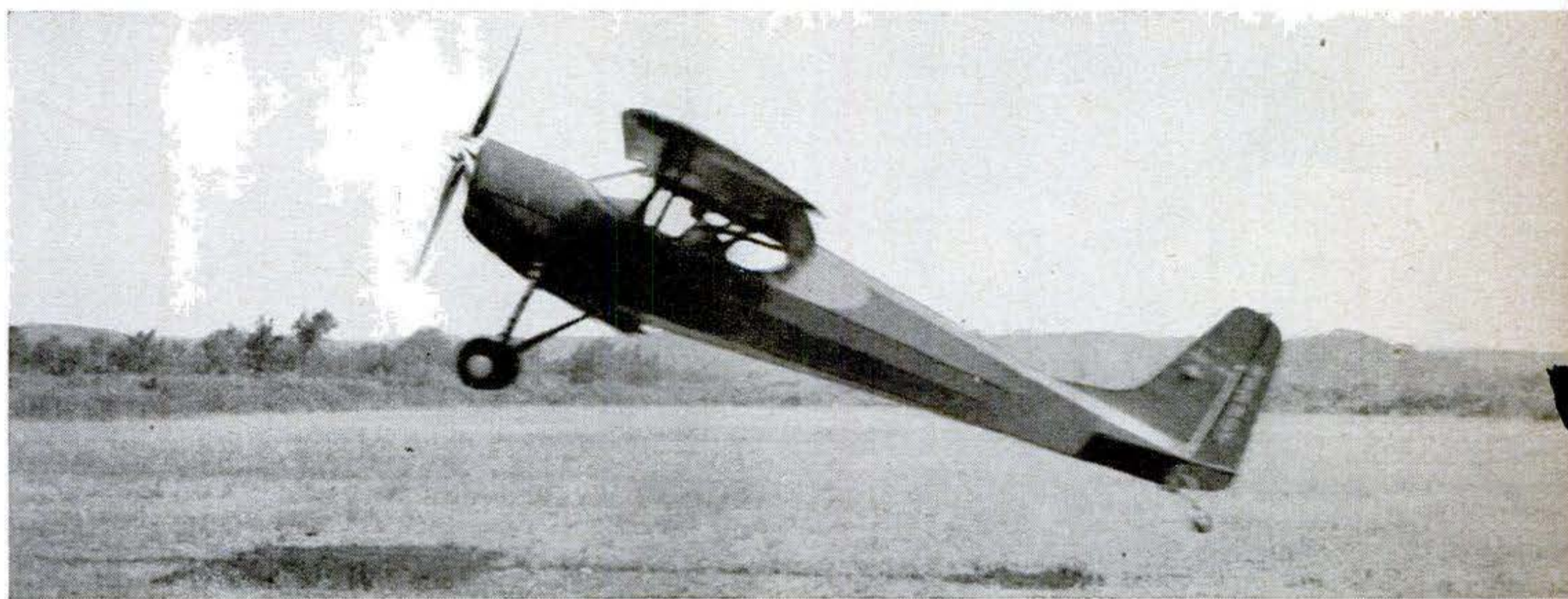
Second high-performance ship, Heliplane, takes off at spectacular climb angle without danger of stalling. Plane's 29-foot span is normal, but length is 4 ft. greater as aid to stability.
