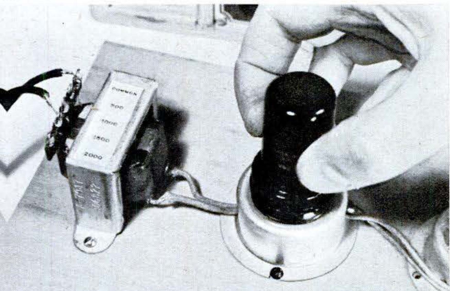
7. Old transformers for 2.5 and 5-volt tubes can be used in modern circuits with 6.3-volt heaters. This arrangement gives 6.25 volts.
