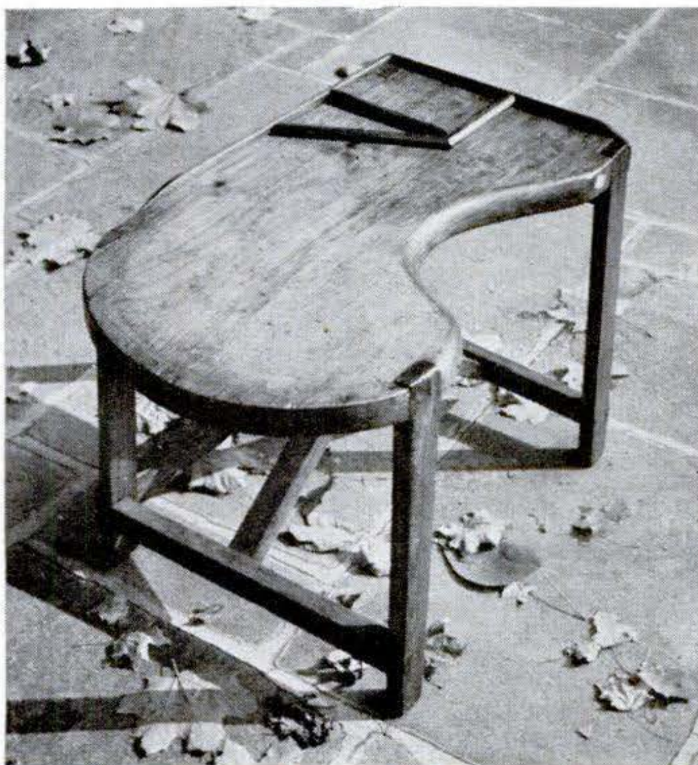
A cobbler's bench inspired this coffee table. Notice the diagonal bracing. The short piece, at the near end, butts against the longer one.
