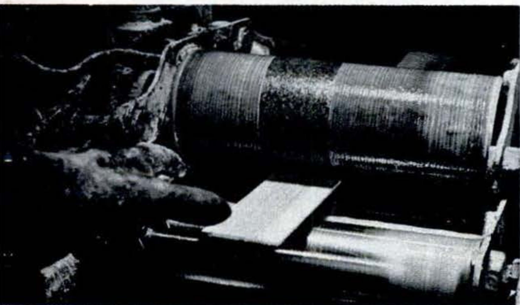
Double-roller spreaders apply glue, a special phenolic-resin type, to veneer sheets after they have been cut to size by rotary cutter. Narrow strip above will form part of door-frame pillar.
