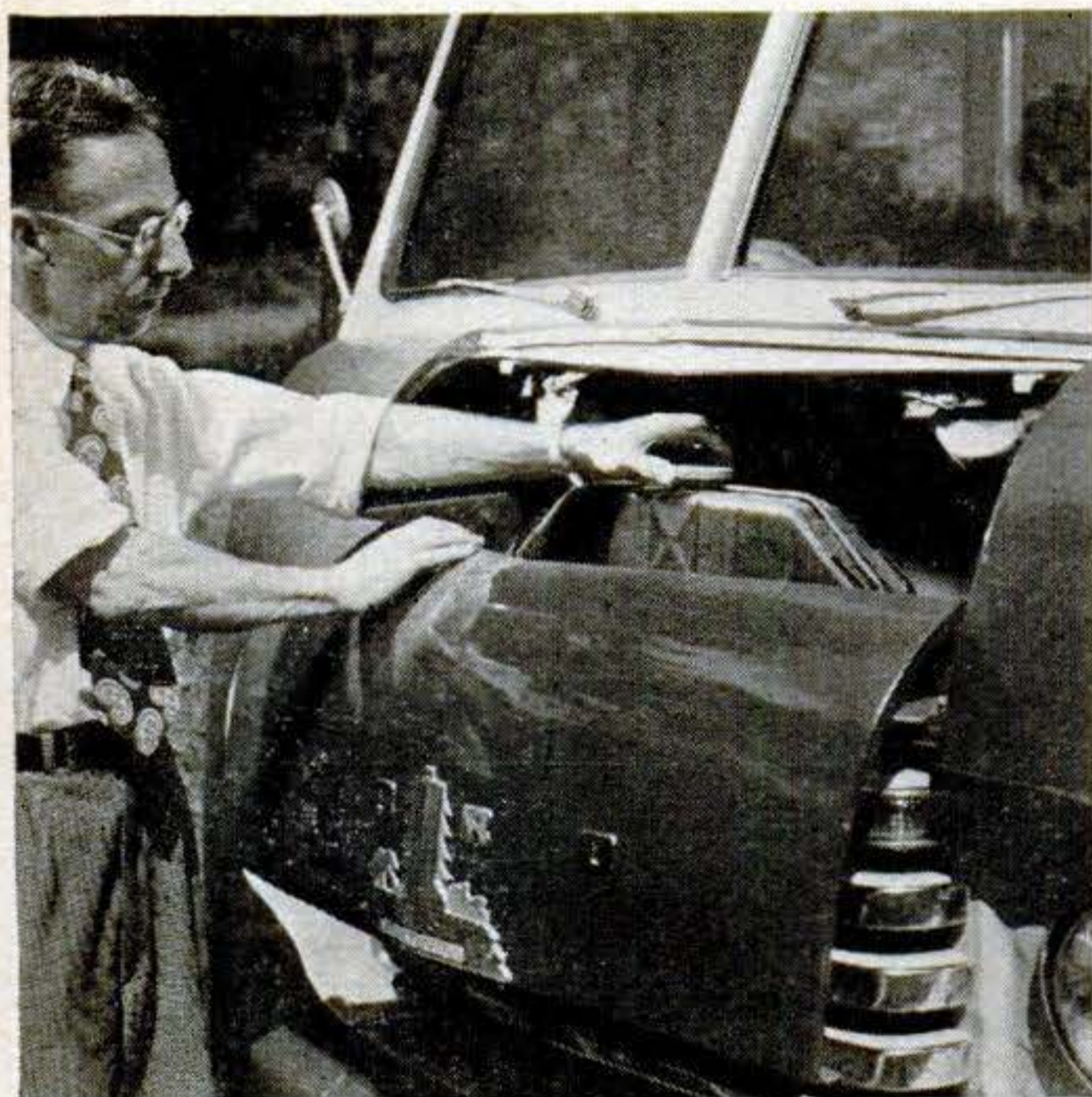
Oversize radiator is reached by sliding front panel out and down over grille. Twin vacuum motors swing big wipers. The insigne in the center reads "Ford-Boyertown Touring Coach."
