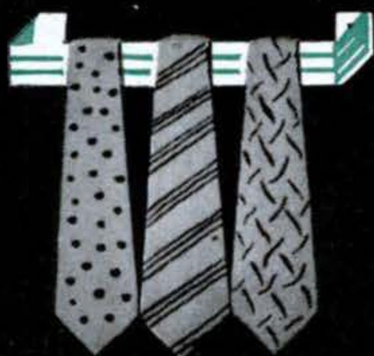
Tie rack is made by bending flat molding and screwing or nailing it to a door.
