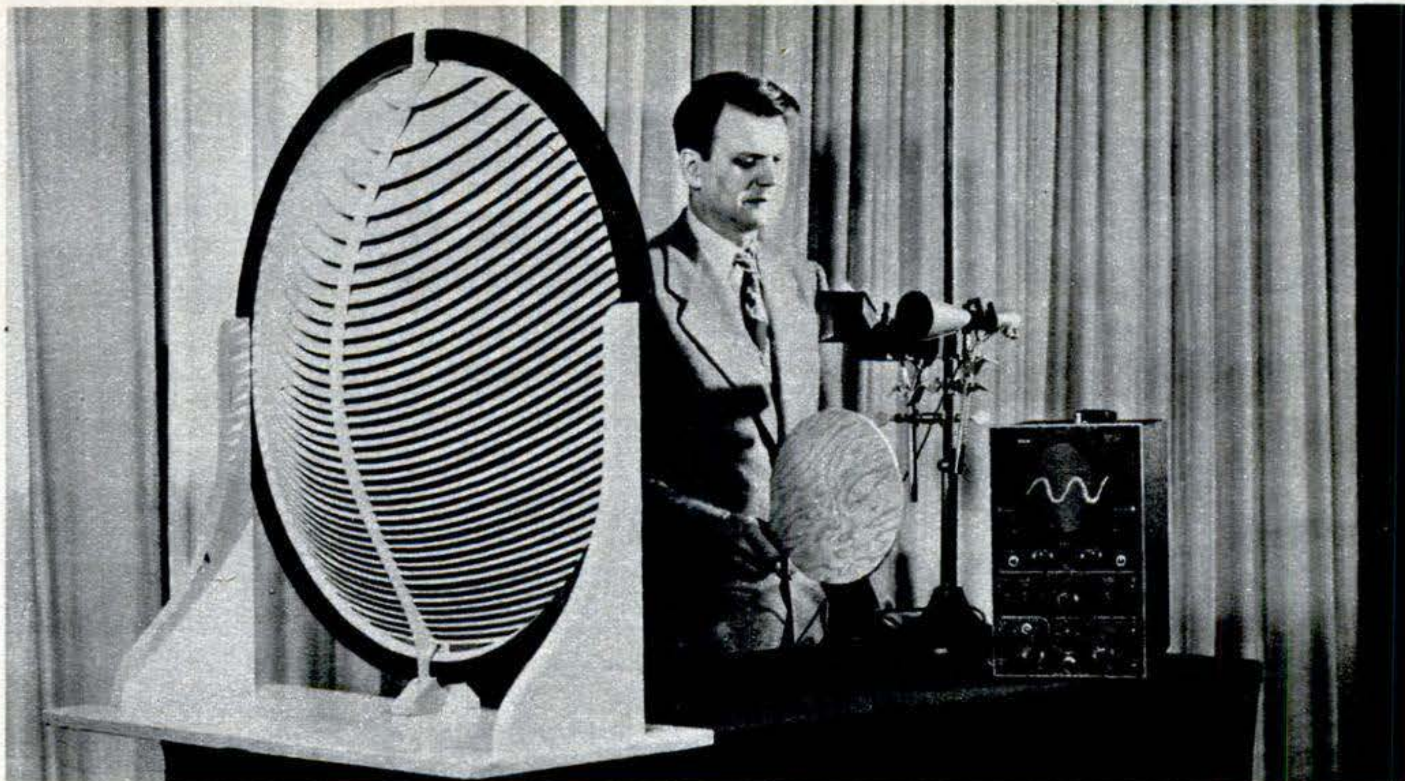
Microwave ancestry of sound lenses is shown by using one lens to focus both types of waves.
