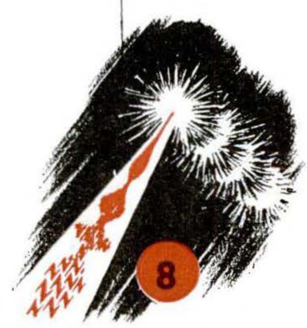
8 Tube face is coated on inside with fluorescent phosphor. Phosphor lights up as electrons strike it. Amount of light is governed by the intensity of the beam.
