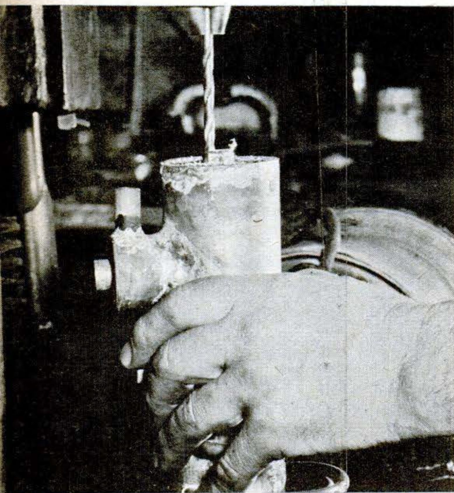
After second test, in which boiler held 300 lb. pressure for an hour, fittings were taken off and holes drilled for steam gauge and try cocks. Next, washing in hot water removed flux.
