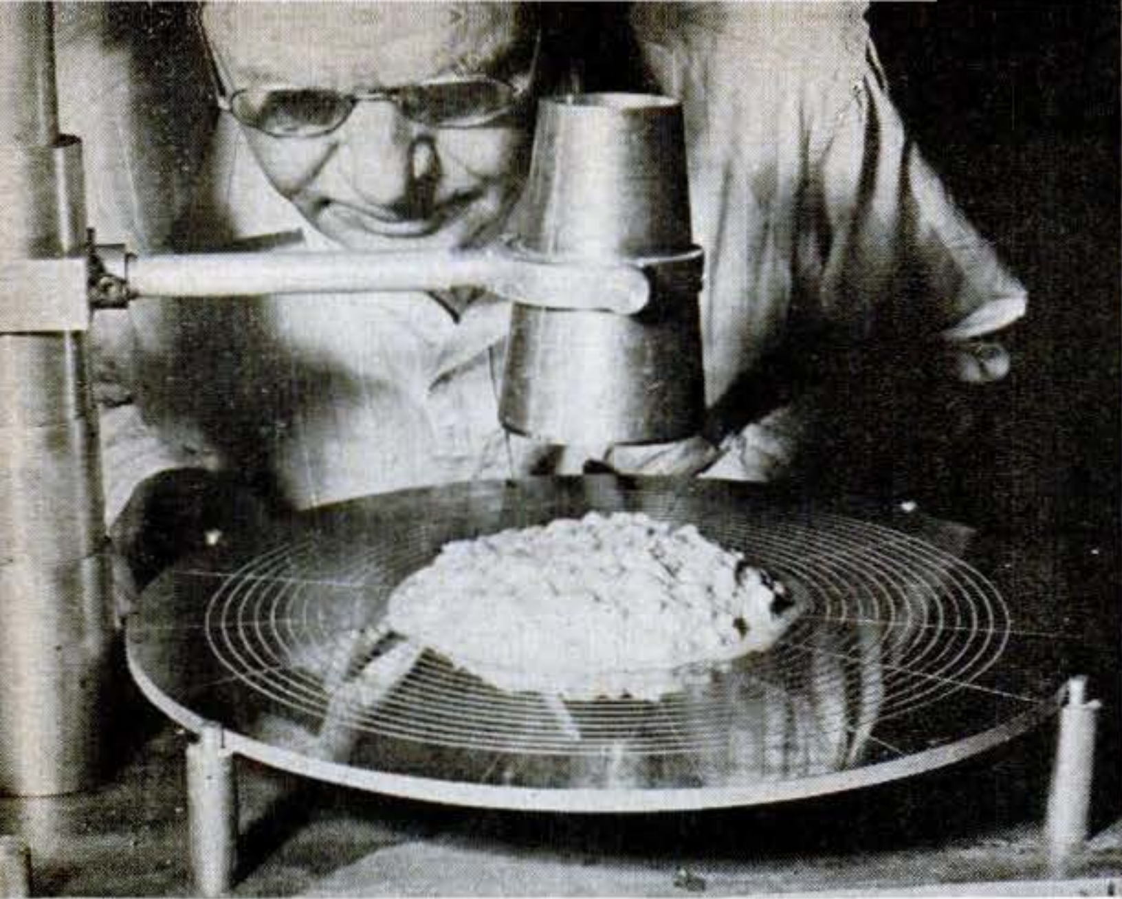
Consistometer measures stickiness of creamed corn by showing how far a can of it spreads when dumped on plate ruled off in circles.
