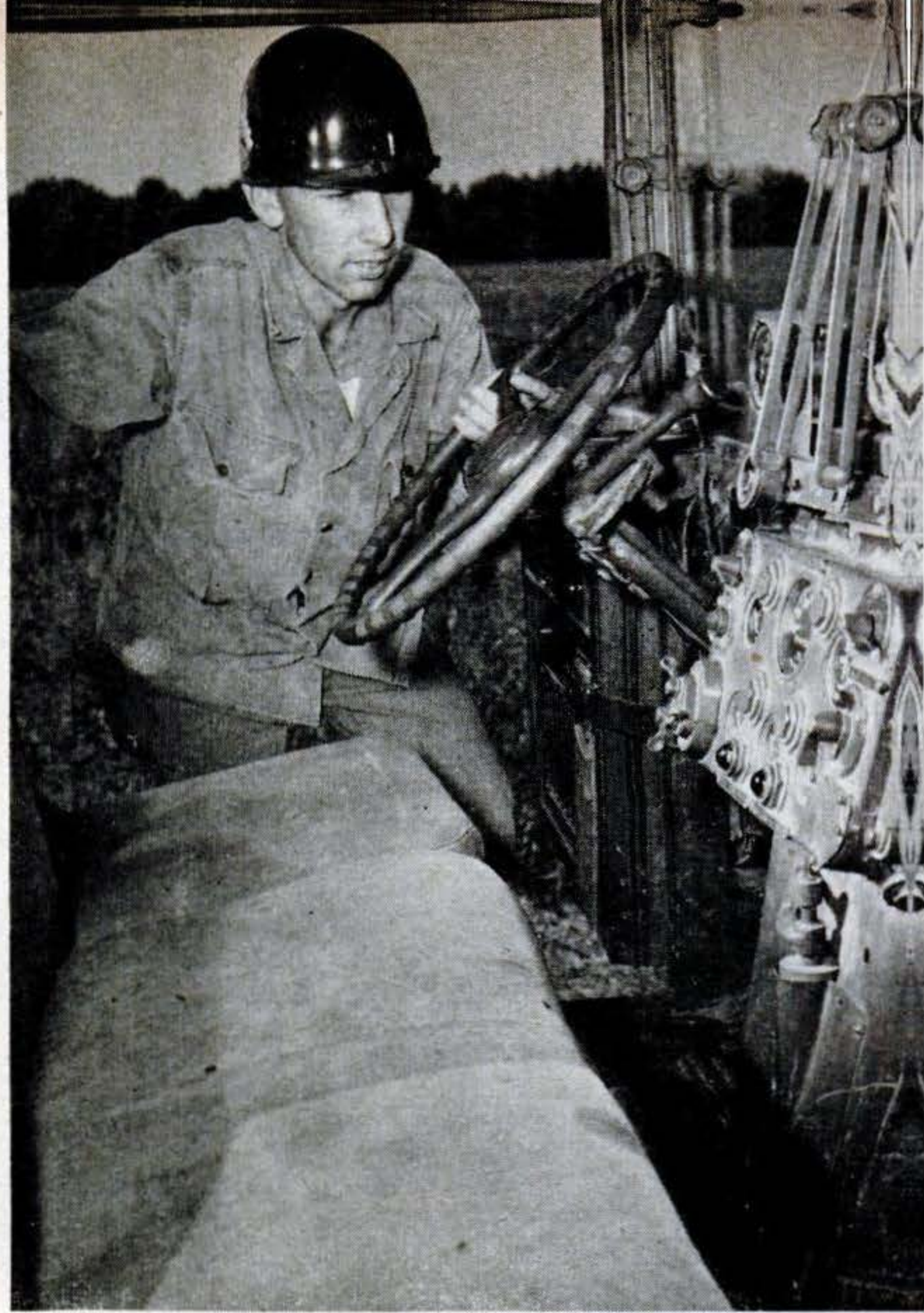
Wide doors and plenty of clearance under steering wheel make new trucks easy to get into. More important, as combat drivers will testify, they're easy to get out of in a hurry.
