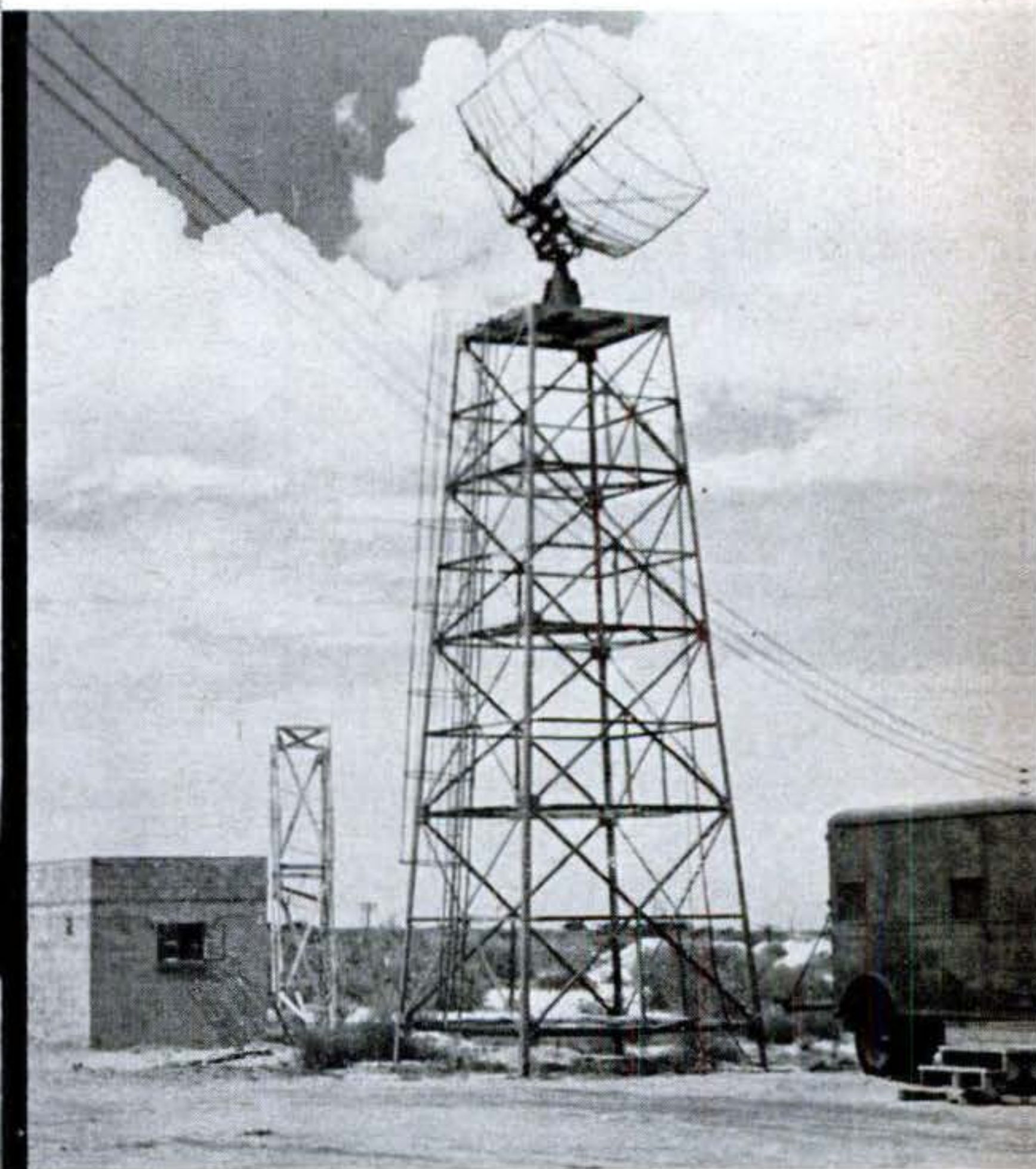
13 Station Viking broadcasting. This telemetering antenna picks up the rocket's messages on conditions aloft, automatically sent out over 30 channels during flight.
