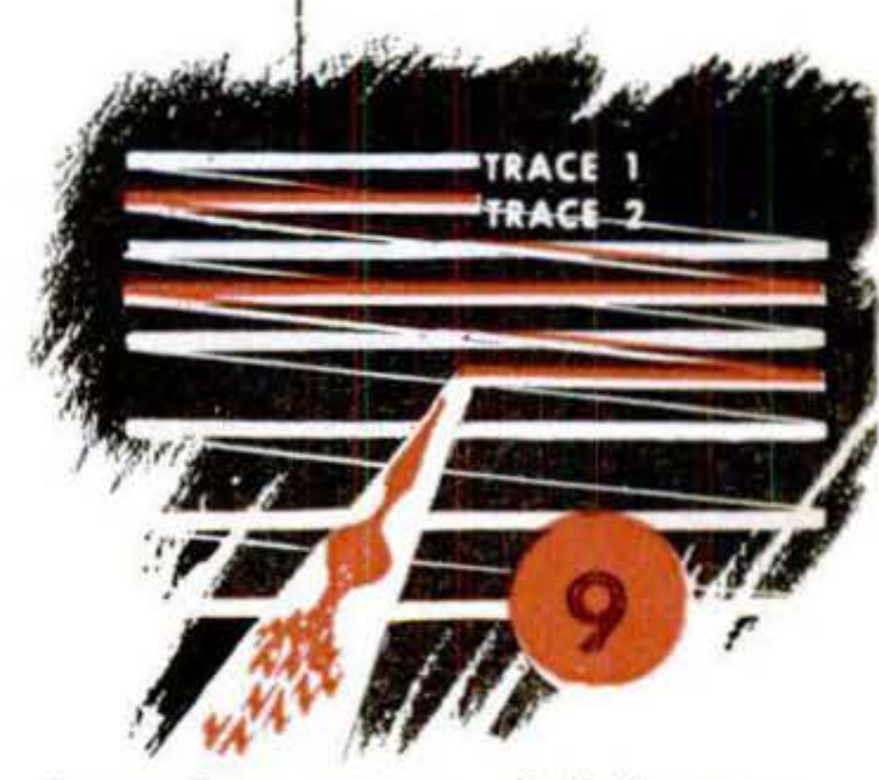
9 Scanning action of deflection yoke moves beam across face in 1/15,750 sec. Beam makes two interlaced half pictures. Trace 1 (white) draws 262\frac{1}{2} lines in 1/60 sec. Trace 2 (red) then does the same in the spaces between trace 1. Resulting picture consists of 525 lines drawn and erased 30 times a second.
