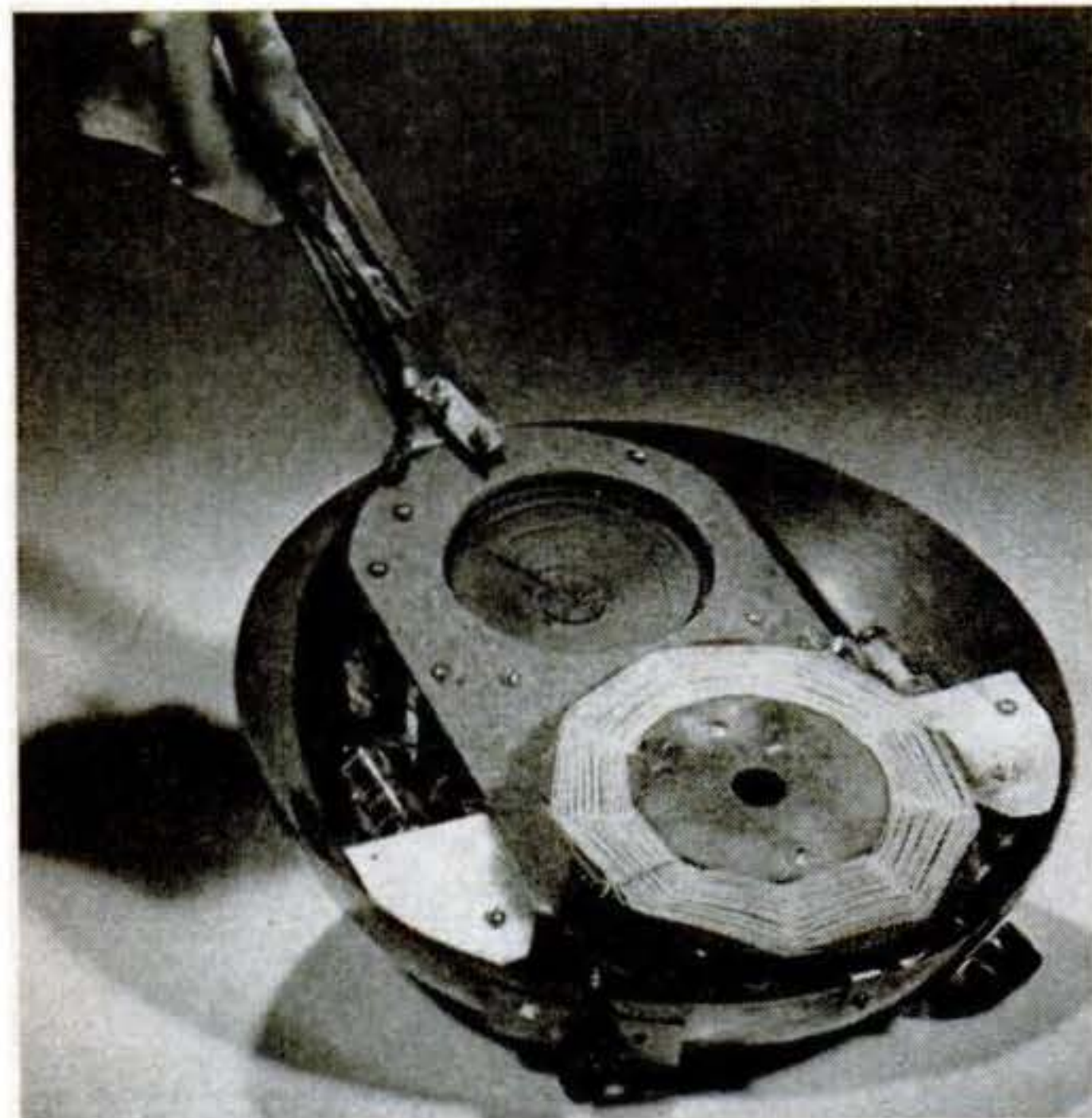
To hold the set in the pan, use a flat bracket at top and a right-angle bracket at bottom. Chassis should not touch the pan.
