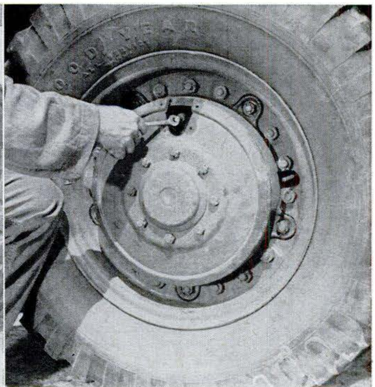
New sealed brakes are mounted in drum on outside of wheel for easy access. Brakes can be relined and adjusted without pulling wheel. Minor repairs can be made through opening.
