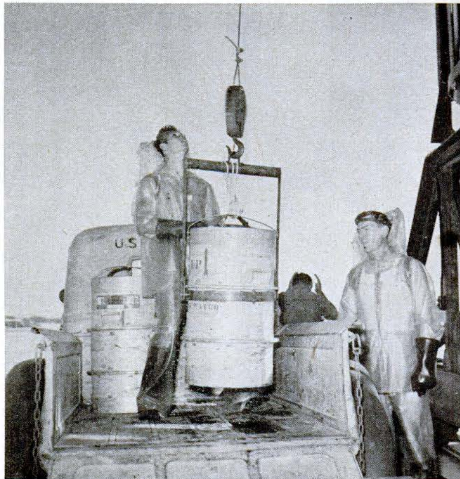
4 Delivering the 270-pound charge of 90-percent pure peroxide is a dangerous job. Workers transferring the drums to gantry crane wear protective suits and double rubber gloves.
