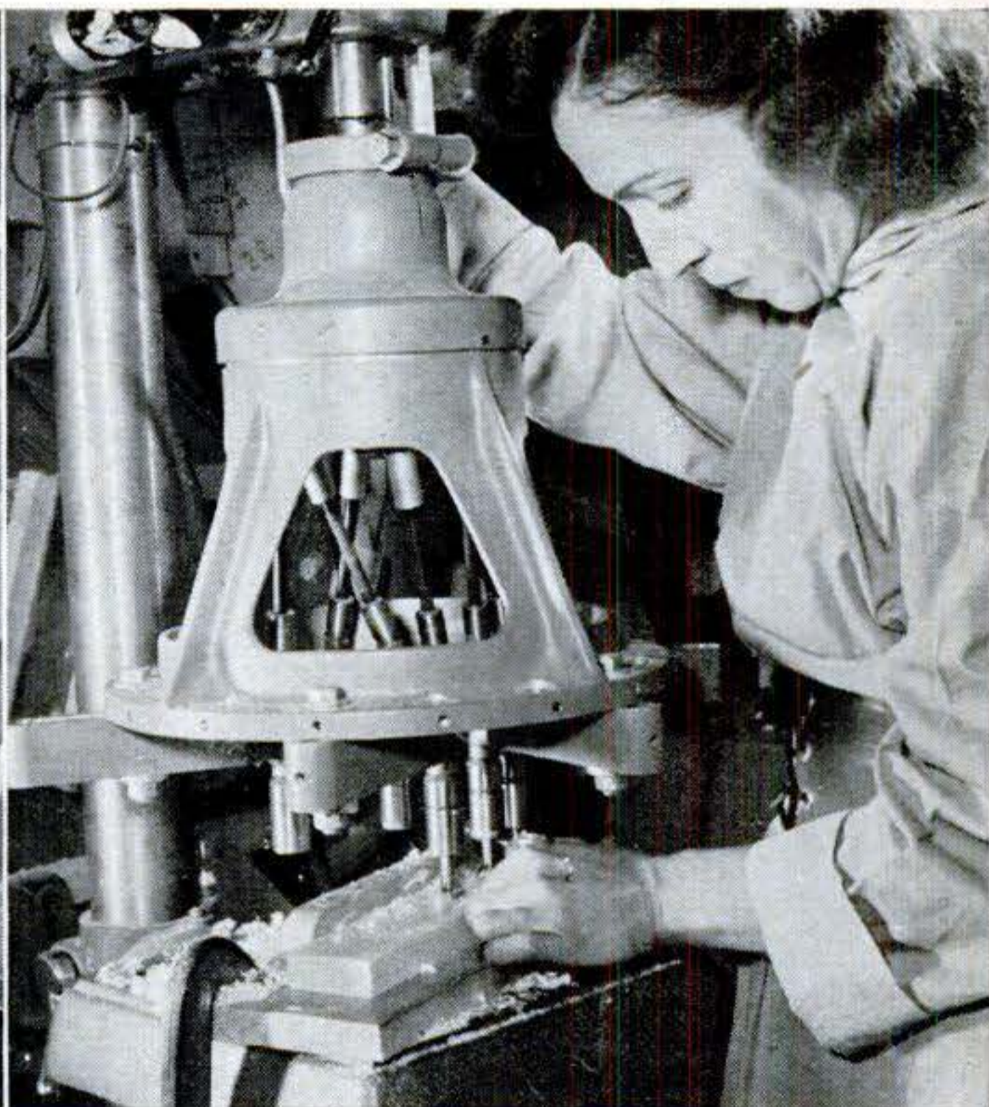
Holes for pegs are sunk with multiple drill. Depth, diameter are the same— \frac{5}{8} in. Standard pegs are 1½ in. long; smokestack's, 2 in. Designer Monaco's father helped establish shop. ▶
