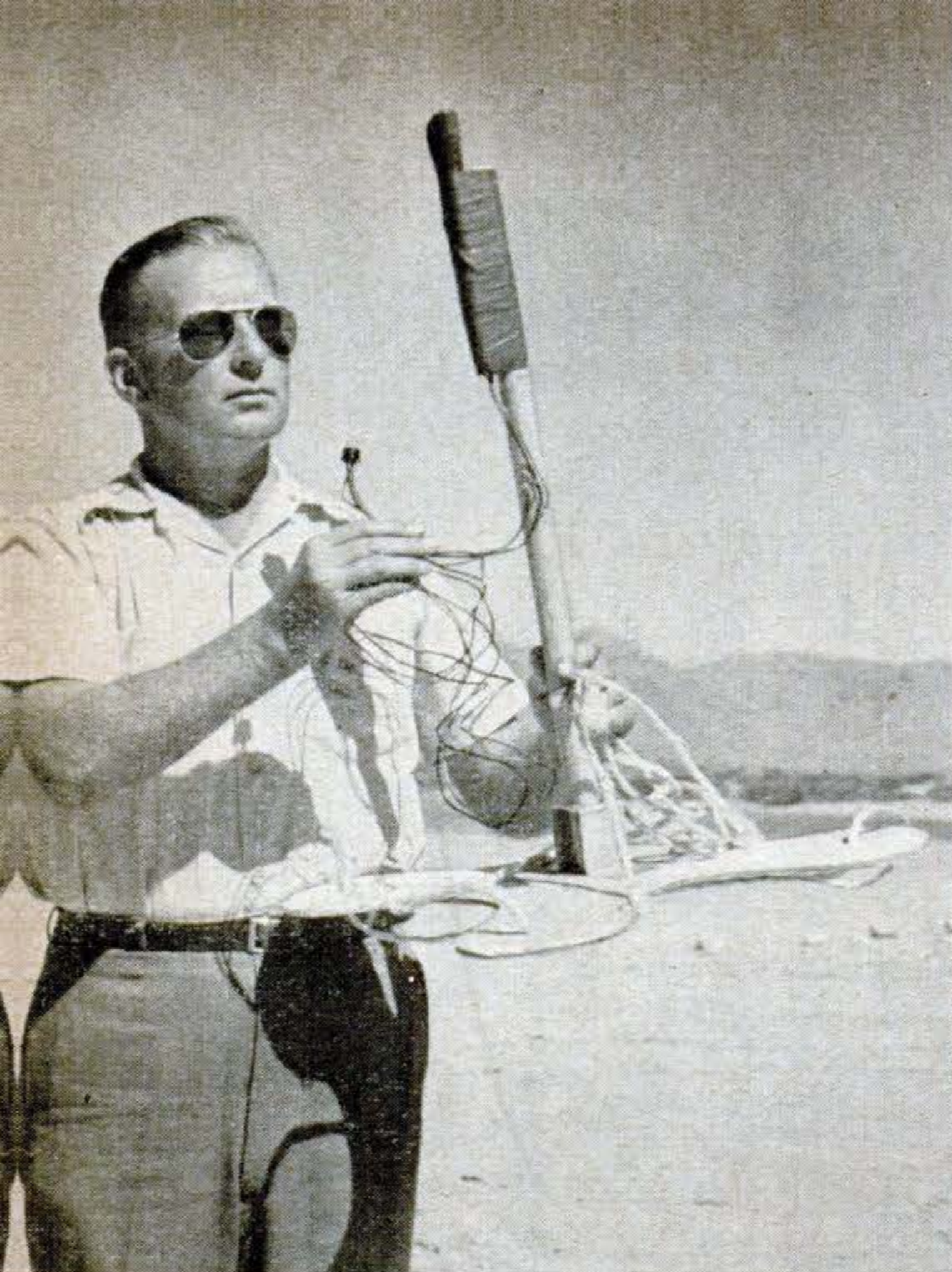
7 Electrically operated "firecrackers" on a stick will ignite Viking's gas mixture. In less than a second rocket takes off. Cords lash assembly's plywood base to rocket understructure.
