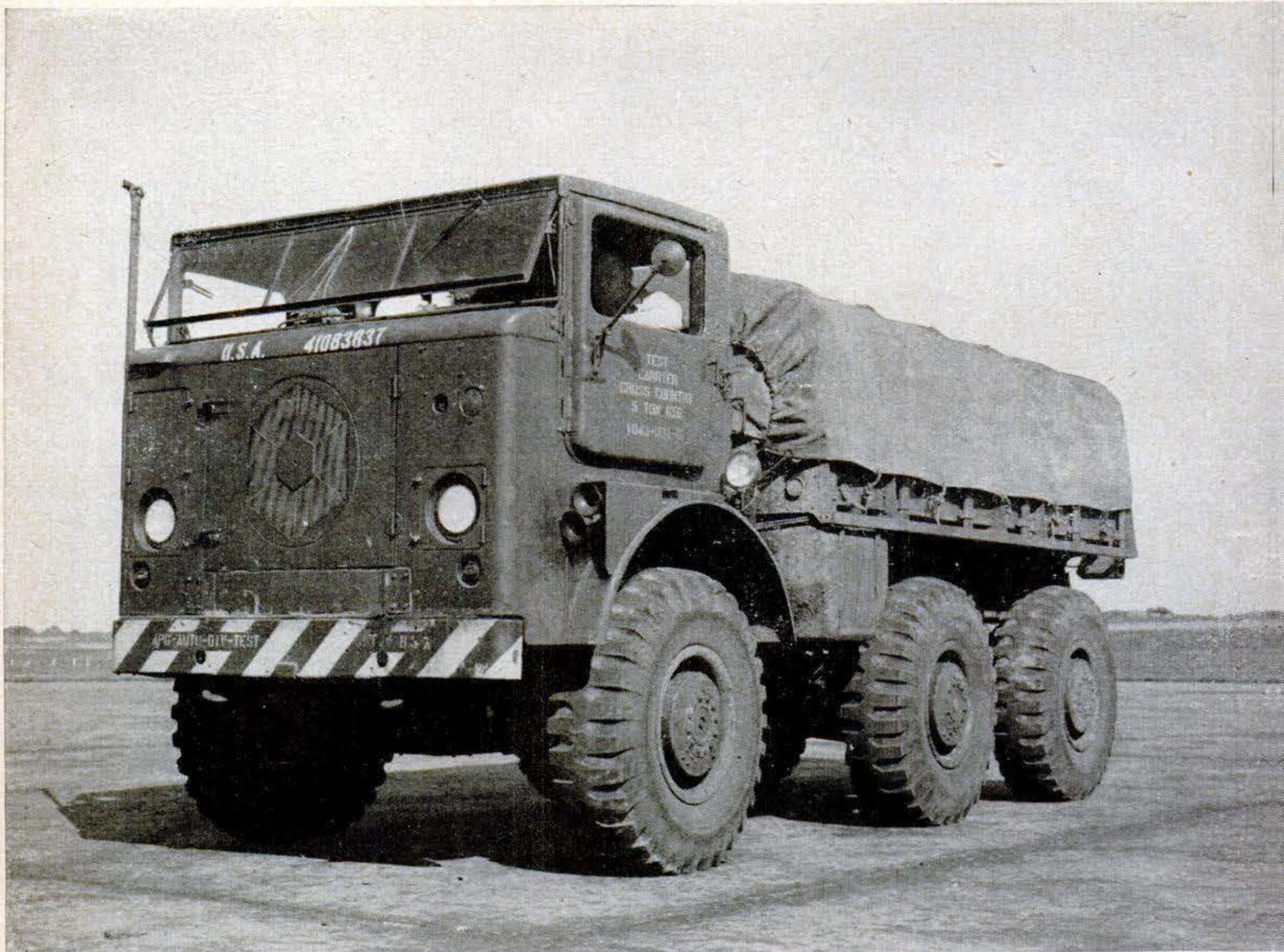
This 5-ton 6x6 has air-cooled engine, torque-converter transmission. Middle set of wheels
