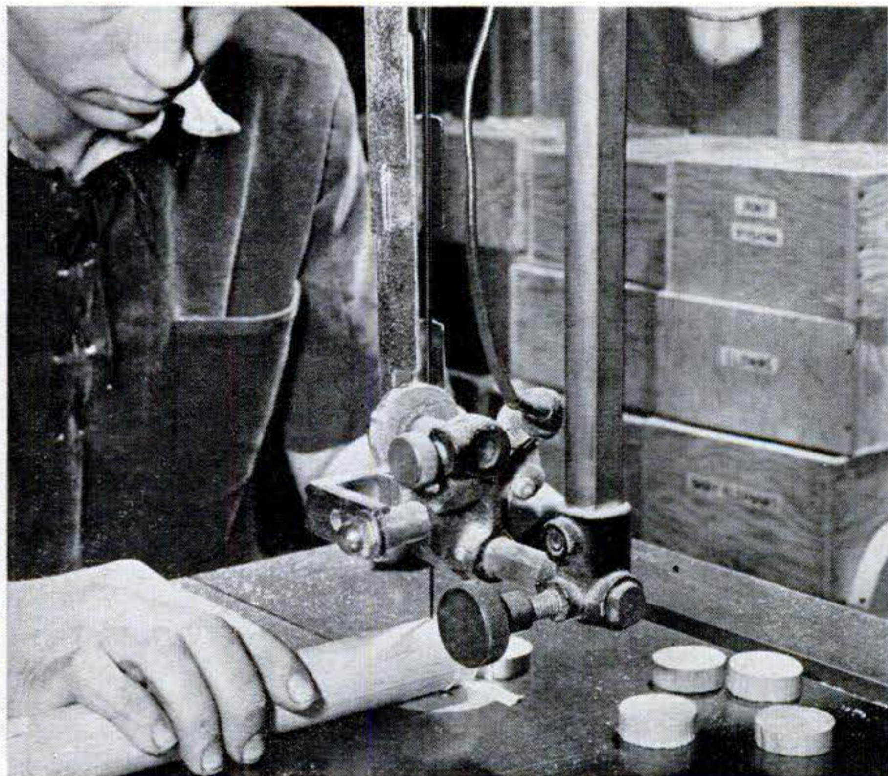
Wheels can be cut from dowel on bandsaw, but factory can get them cheaper from toy factory specializing in wheels. They are 1½ in. in diameter. Rims are sanded to make "tires."
