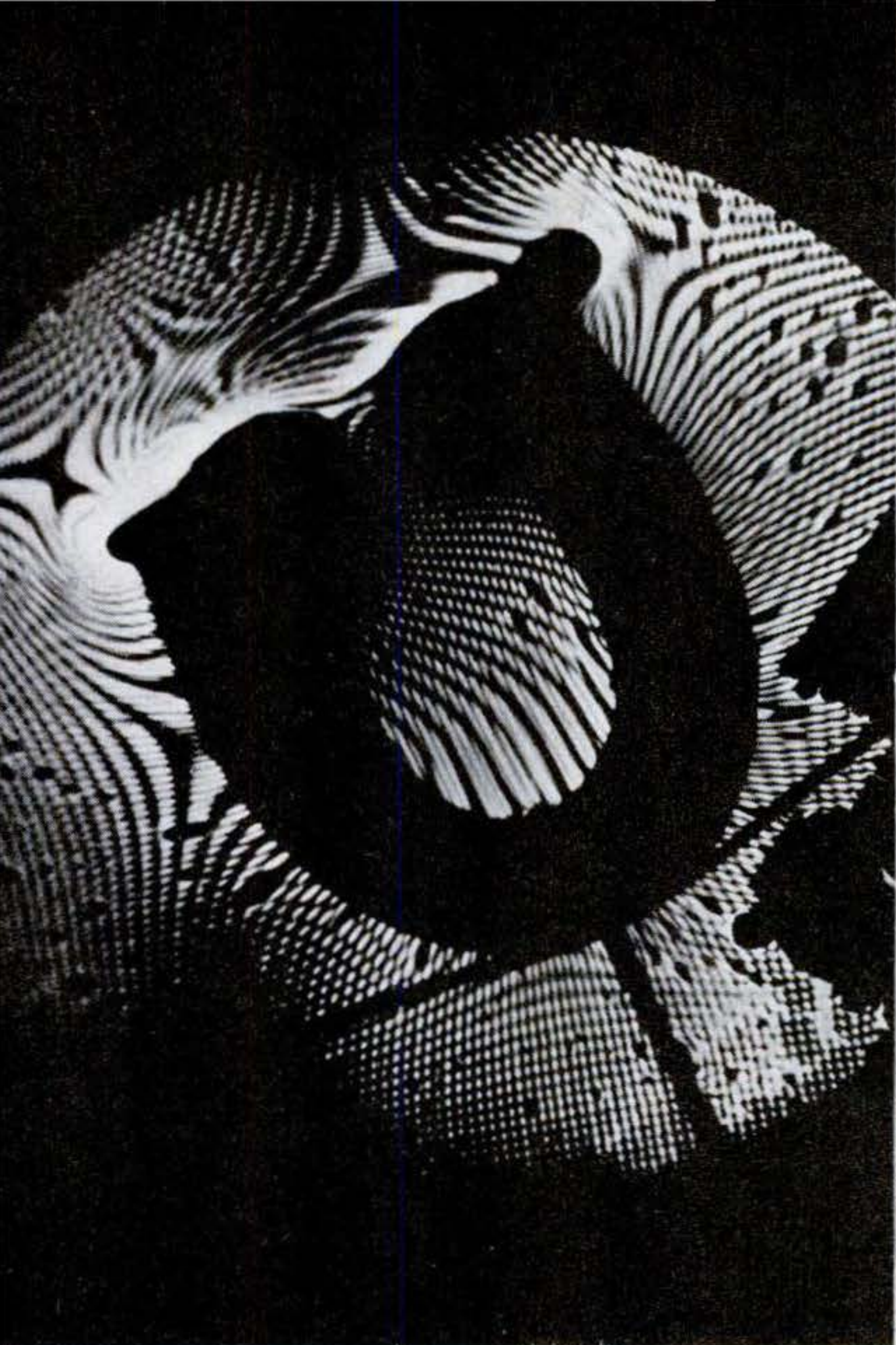
Magnetic field around horseshoe magnet is traced in distorted shadow lines of fine screen photographed through electron microscope.
