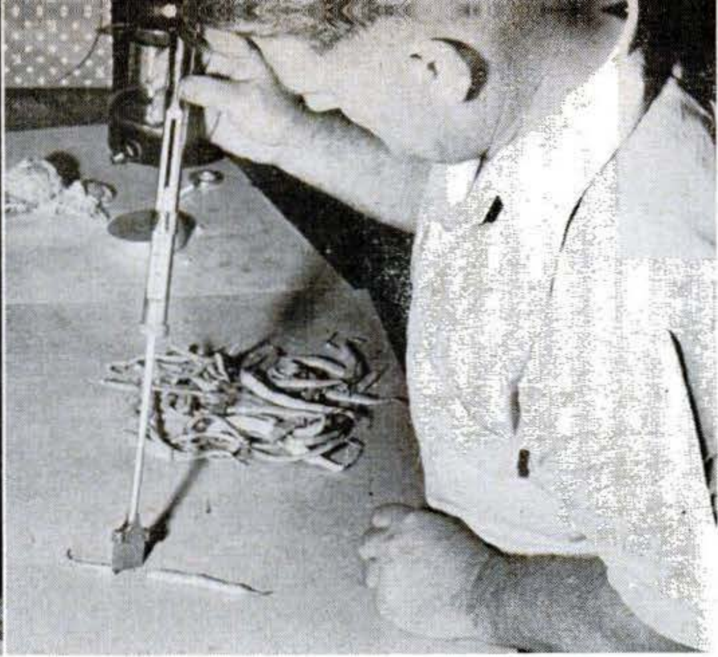
Stringiness gauge records how much pressure is needed to cut through a string bean. That helps to tell how long canner should cook it.
