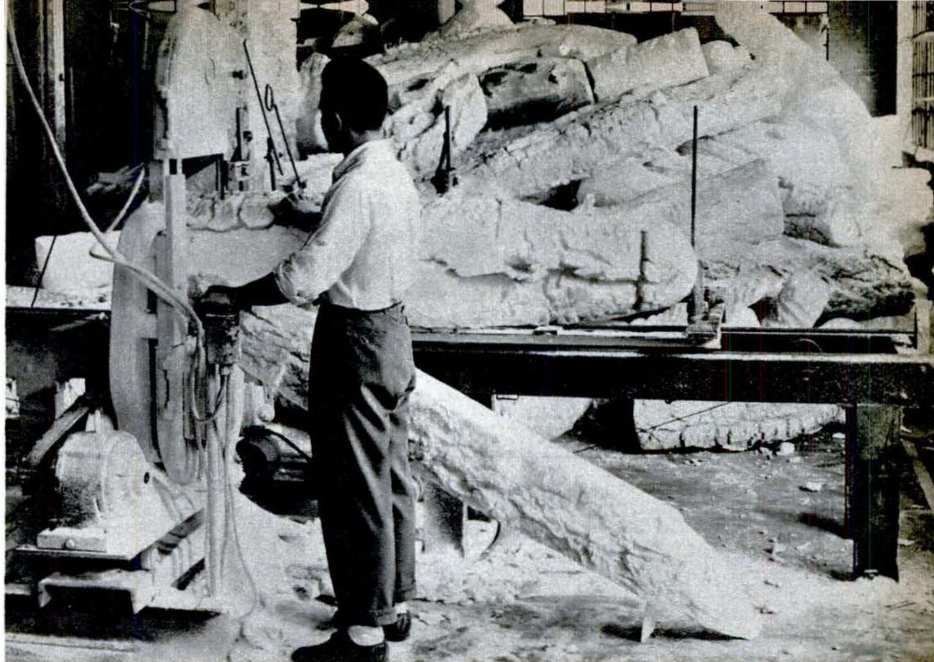
Polystyrene comes to manufacturing firm in big "logs" that have a rough, barklike exterior.
