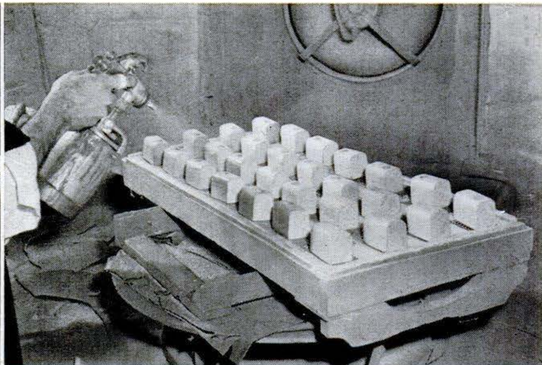
In lacquering shop, boilers are put on screen rack and sprayed under 15-lb. pressure. Higher pressure would blow blocks off rack. Next step is stacking for a 6-hour drying period.
