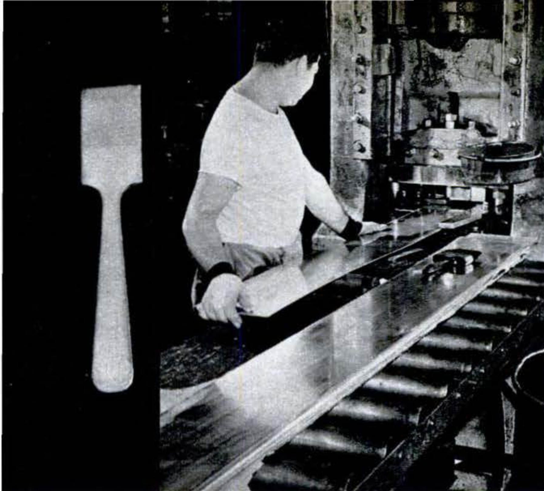
Forks and spoons start down production line in this blanking machine. By cutting two interlocking blanks with each stroke, machine keeps waste scrap to minimum. Metal is nickel silver.
