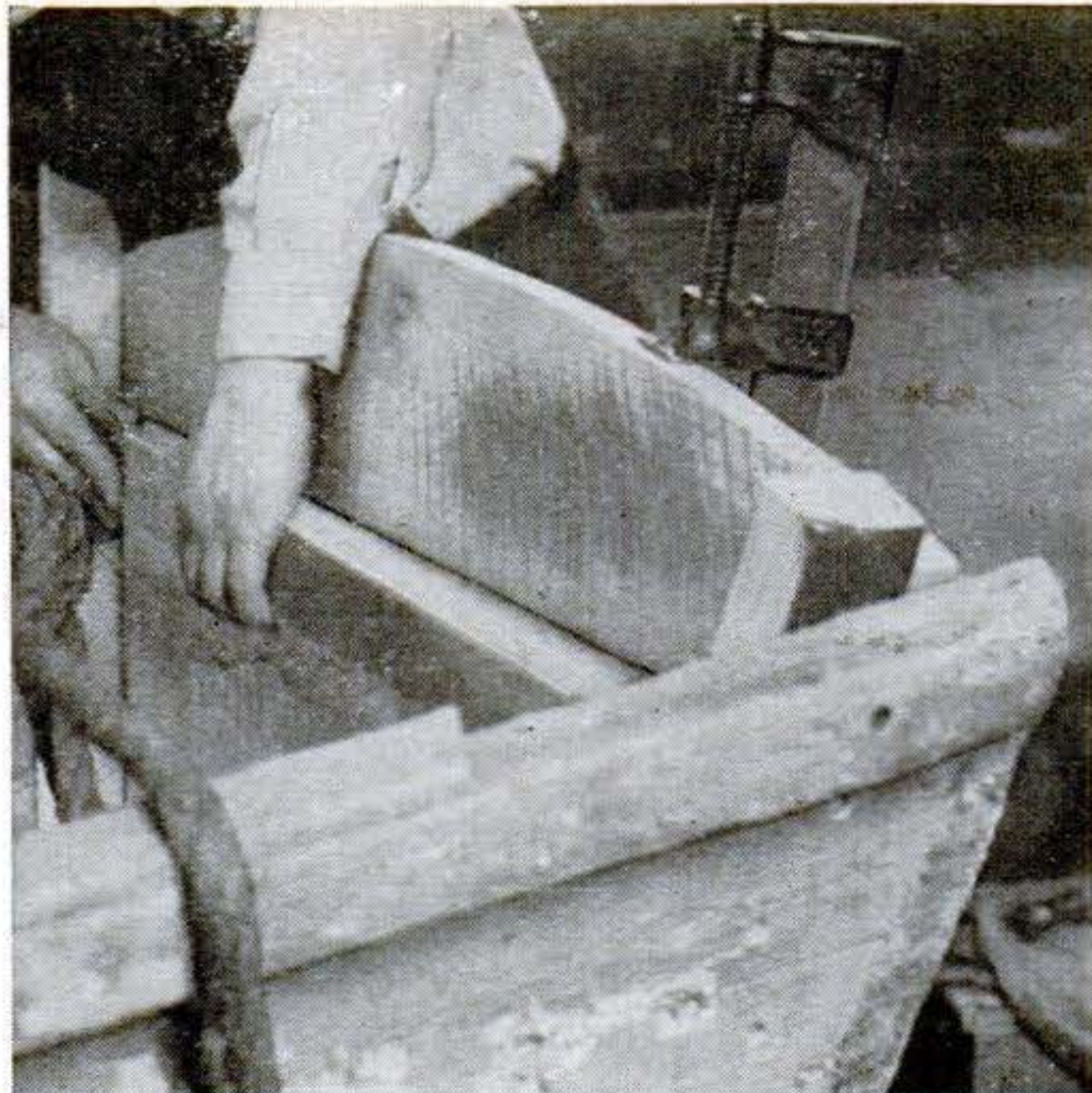
Here the new transom has been cut and screwed in place. It's made up of two planks, calked at the joint. Seat support is being fitted.
