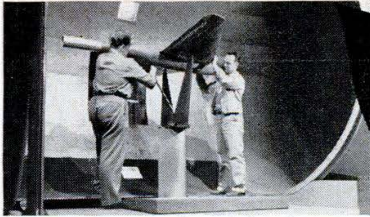
Aeronautical Engineering offers a wide choice of interesting duties. Here two engineers install a guided missile model in the Northrop Aircraft, Inc. wind tunnel.
