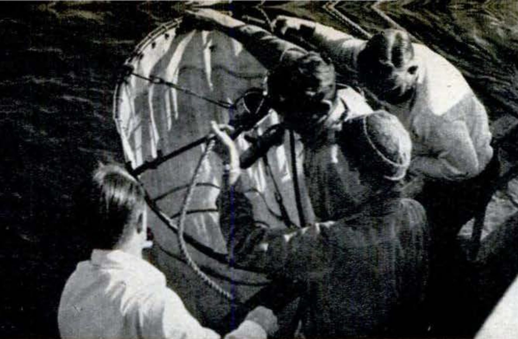
At the start of a run, scientists lower a dragnet that will gather samples of sardine eggs and other minute forms of sea plants and animal life. An instrument registers depth of catch.
