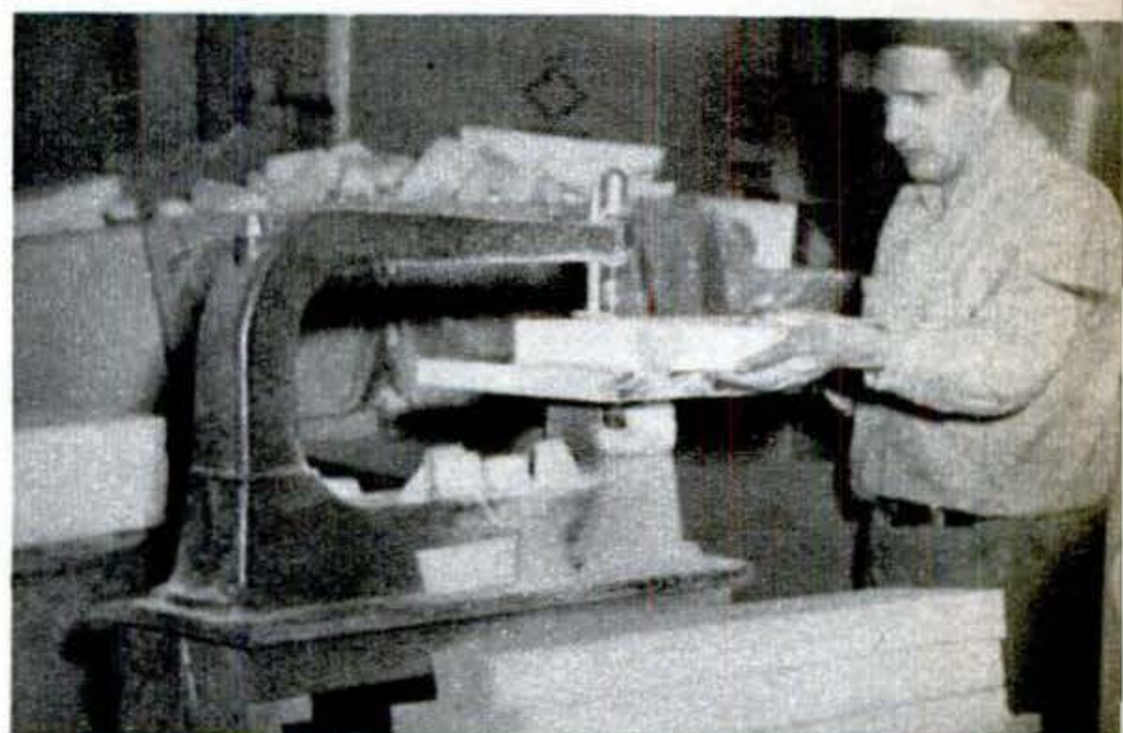
Shaping machine trims off rough surface and creates flat slabs from plastic sections. These are cut into smaller pieces with power saws. Ornaments are made with series of special tools.
