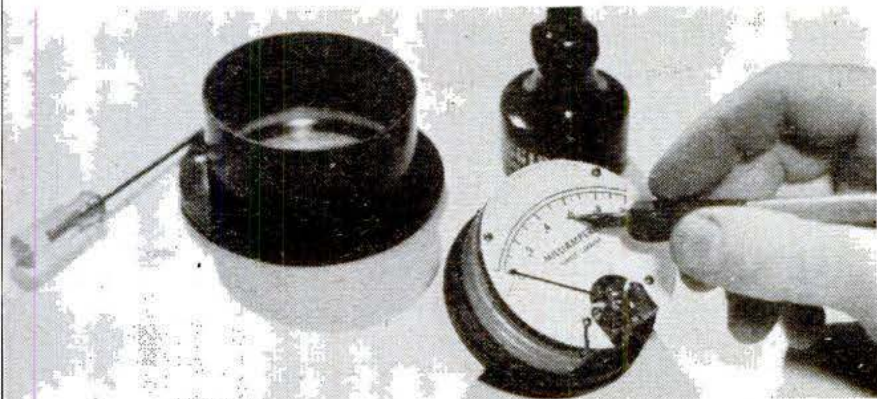
4. If a meter is altered to read 0-1 ma. by removing a shunt, the scale must be re-marked.
