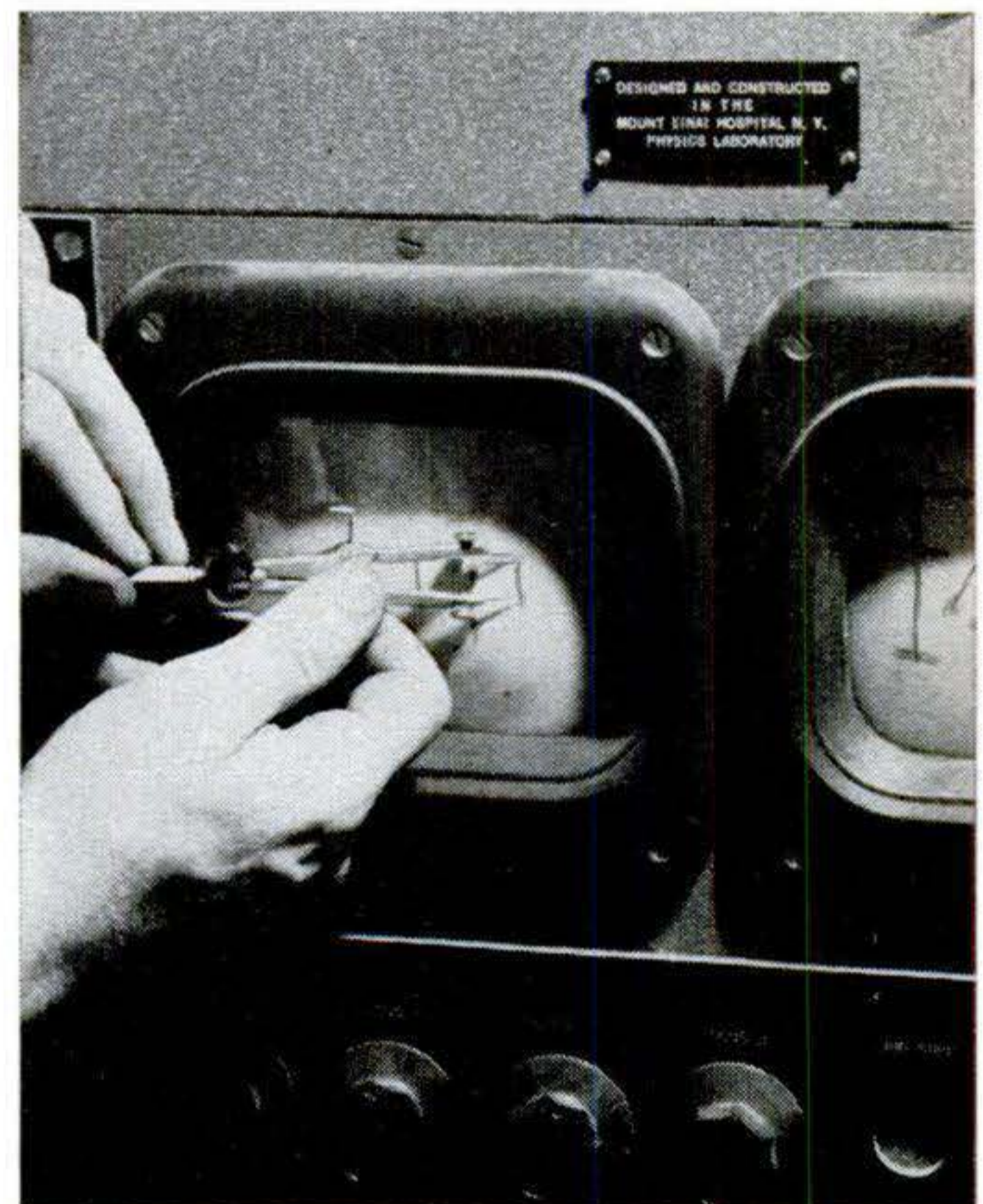
Impulses from the Geiger counter that detects radioactive tracers in the human body can be fed to a cathode-ray oscilloscope to aid record-keeping. This is another piece of apparatus constructed by Dr. Feitelberg and his collaborators in his hospital workshop. With such devices, he can solve problems that previously stumped doctors. Many instruments used in this work can now be purchased, but Dr. Feitelberg finds it helpful to be able to build his own.
