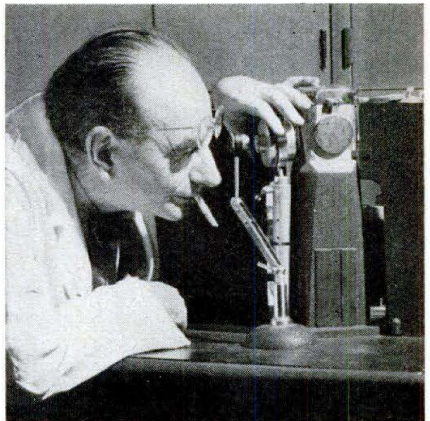
X-ray diffraction patterns obtained with this instrument enable physicians to investigate molecular details of human tissues that are beyond the reach of their most powerful microscopes. This apparatus is used now to analyze kidney stones for data on which special diets can be prescribed for patients from whom the stones have been removed. It is also being used in the study of rheumatic skin nodules and in many other medical research programs.
