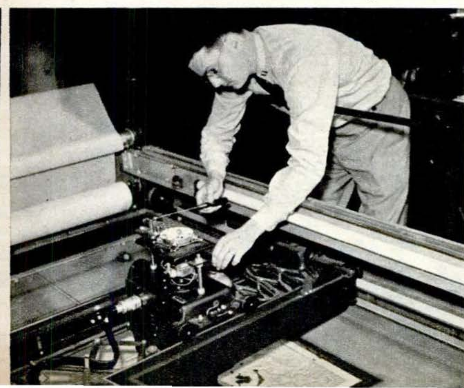
Naval officer below is making adjustment to the airplane simulator, or carriage, that moves in any direction over the tank. Suspended from it and submerged in water is the quartz crystal.
