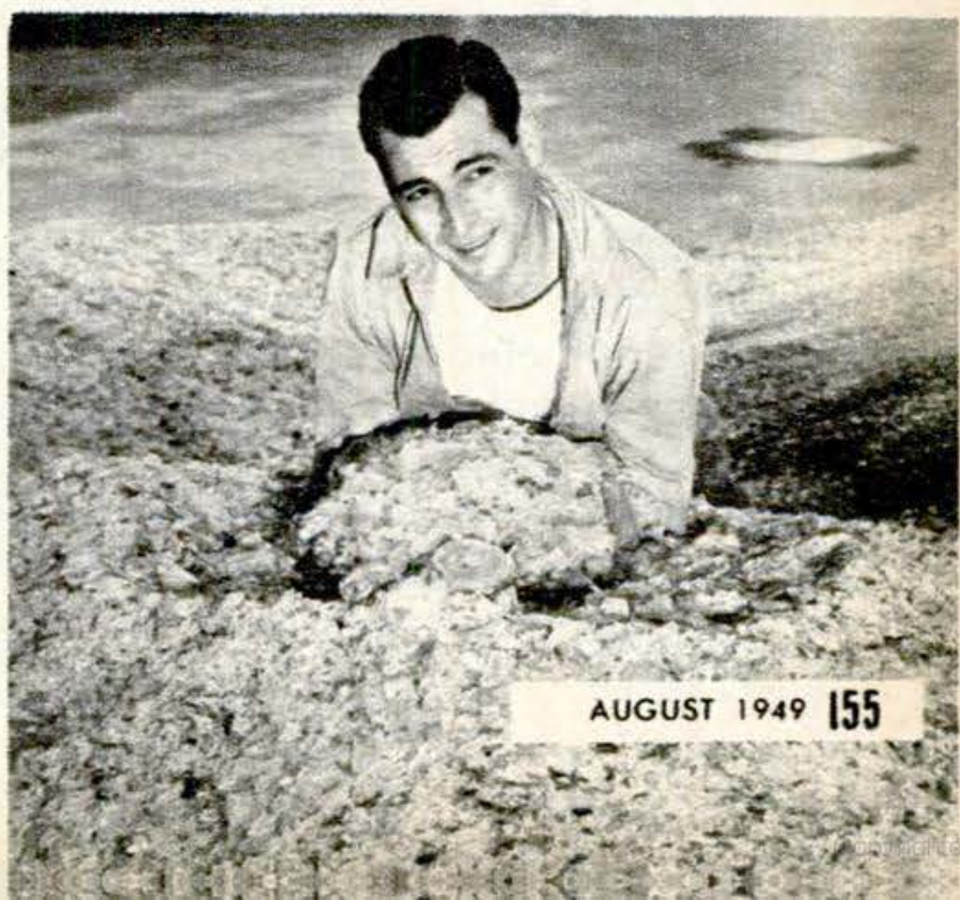
This is cullet after final, two-step washing, and inspection, ready for shipment to bottle maker. The cleaning process rubs off sharp edges so that it can be handled without danger of cuts.
