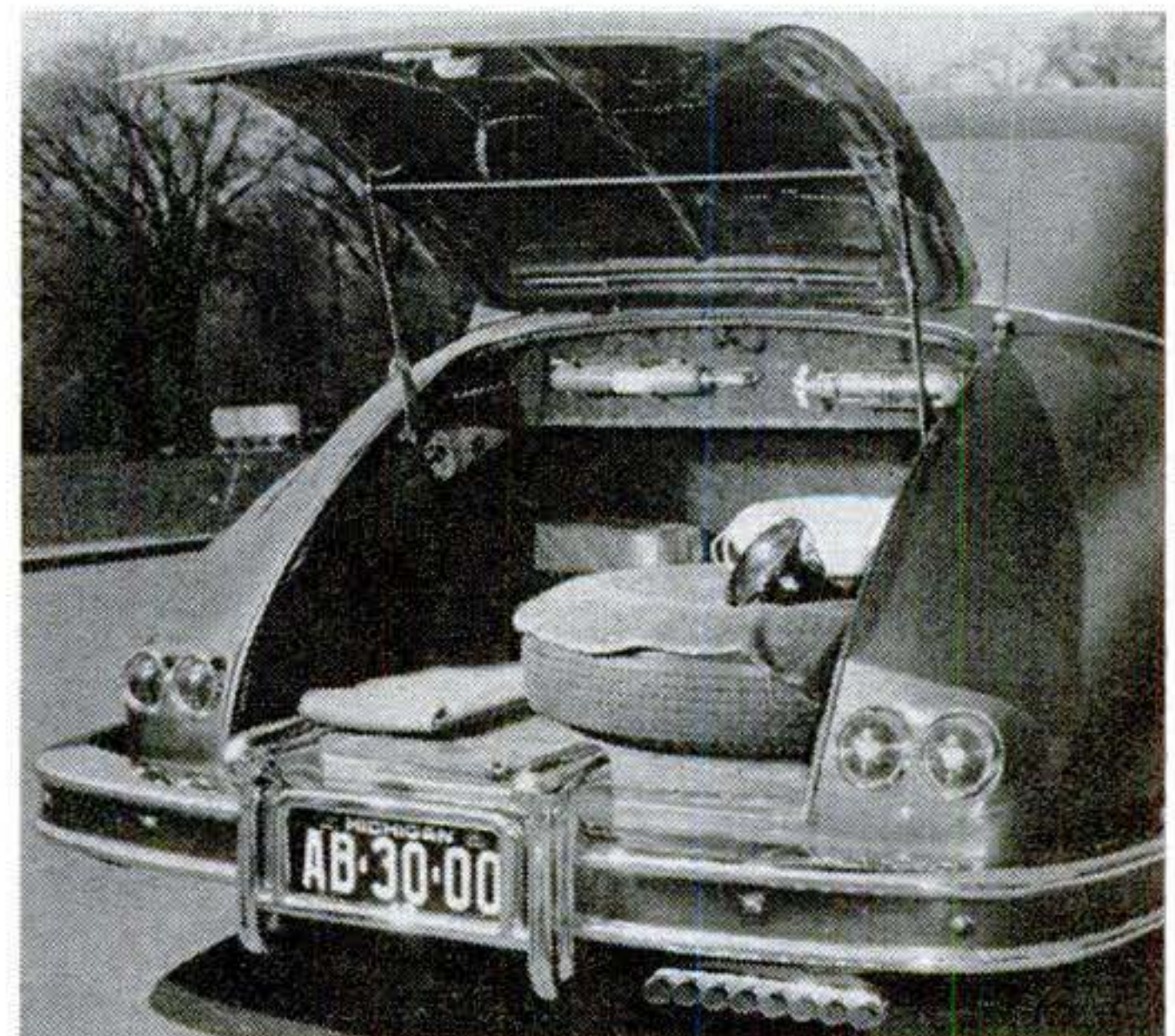
Trunk lid raises hydraulically; so does radio aerial to its right. Inside are fire extinguisher and compressed-air cylinder for filling flat tires. The eight-stack exhaust pipe is just for looks.
