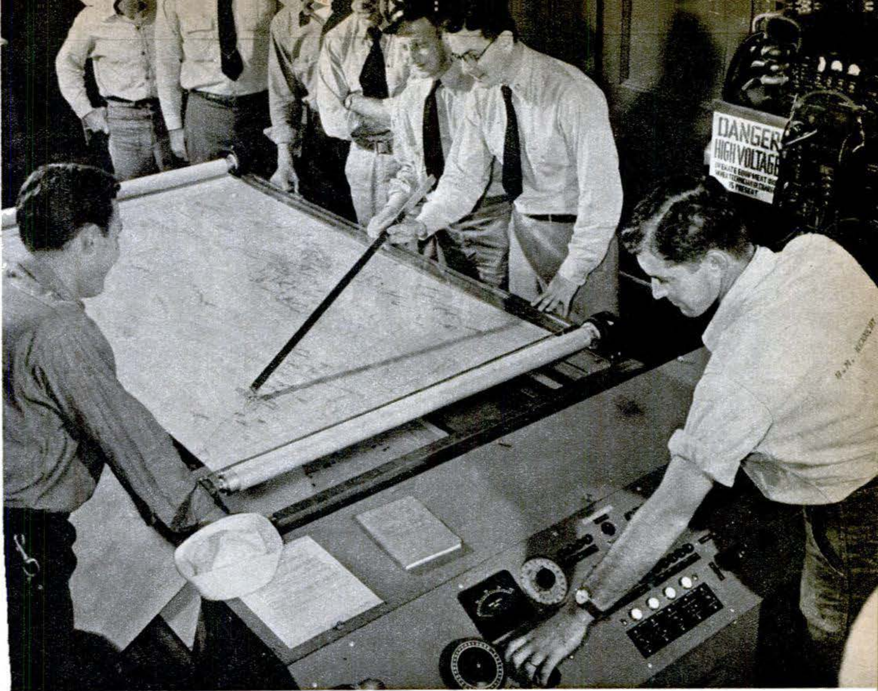
An ultrasonic radar flight simulator in operation at Naval Air Station, Los Alamitos, Calif.
