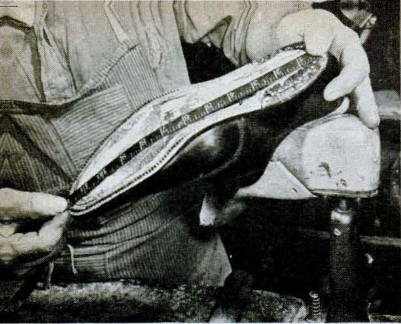
1 Tape measure shows that size-11 shoe above, which is to be lengthened half a size to 11½, measures 12 inches from tip to tip before the rebuilding process begins.
