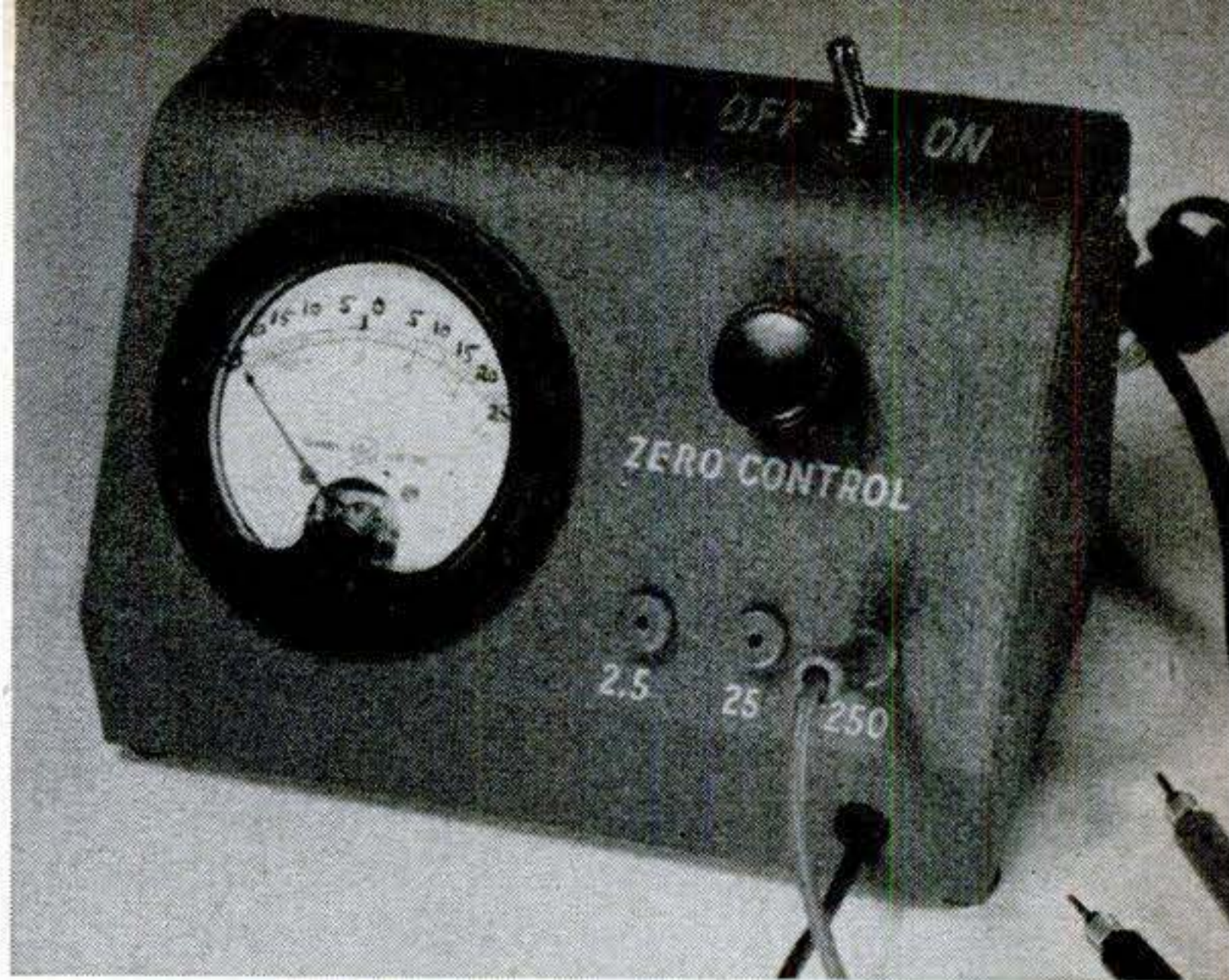
10. This simplified VTVM uses one tube. Scale divisions, from 0 to 25, are marked on glass.
