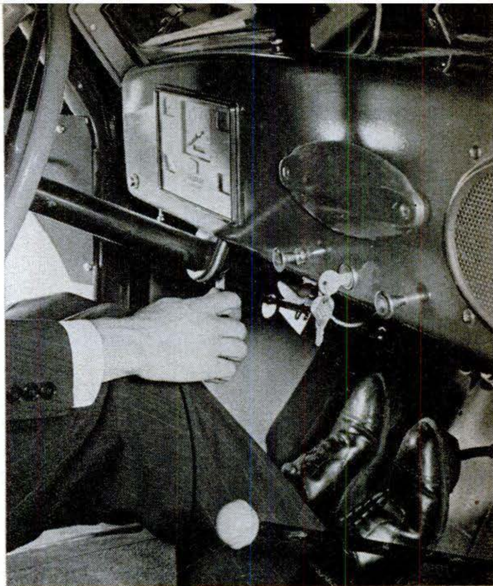
Hand-brake lever in the newer Crosleys is located just under the dash. It sets the new disk brakes on the rear wheels by mechanical linkage. Hand brake was previously on the floor.
