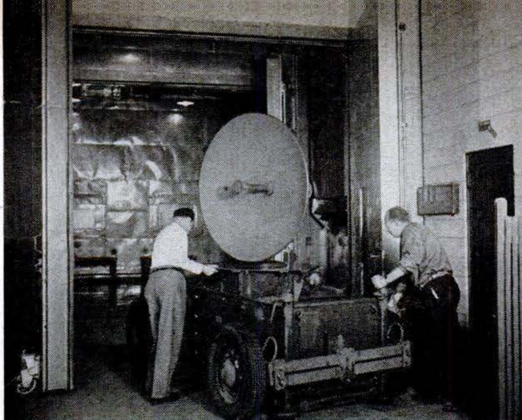
Mobile radar tracking set is rolled into the main tropical test chamber. Door behind the cone can be closed to make two test rooms. Note observation windows in the rear wall.
