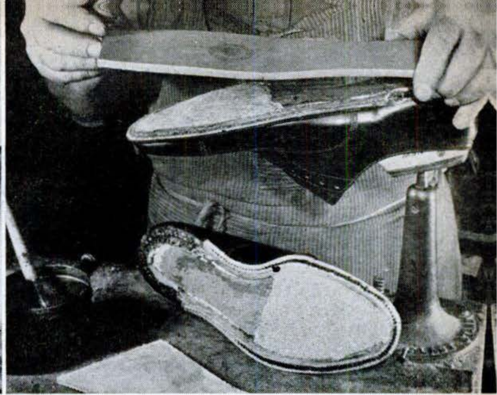
4 After sandpapering the cork cushion (shoe in foreground) to give it a smooth finish, a leather sole is temporarily attached (shoe on the stand) with some rubber cement.
