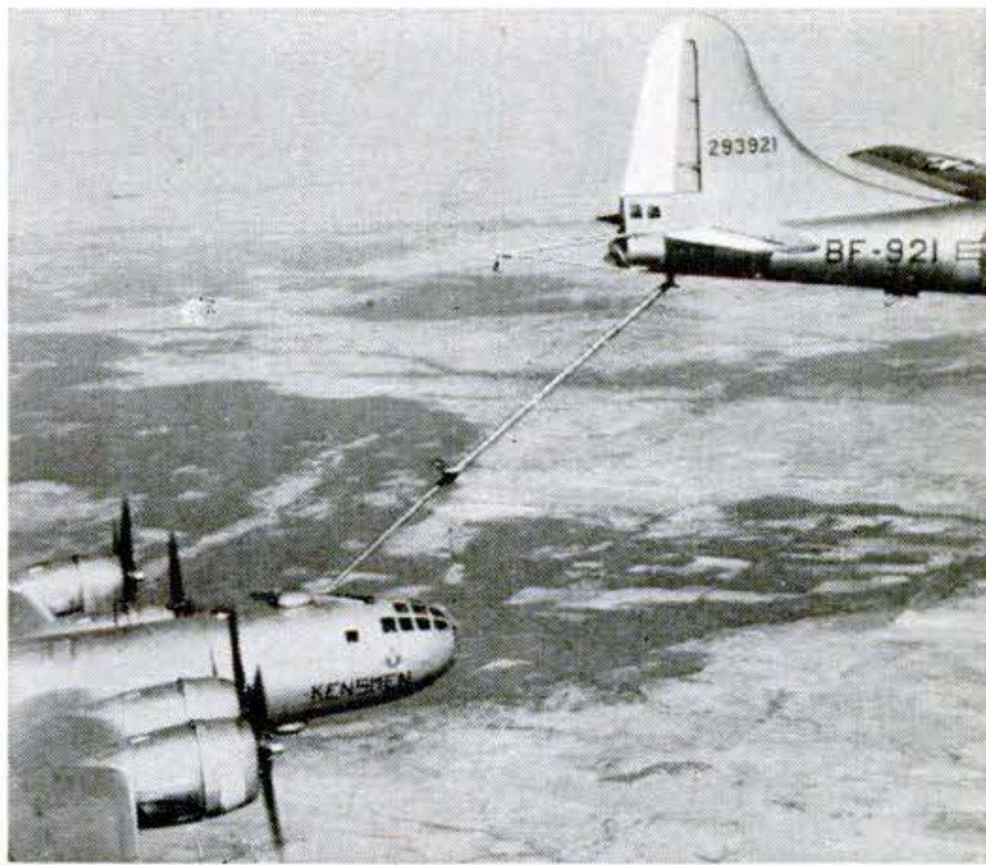
In Boeing system for refueling bombers, telescoping pipe or boom is “flown” by controls called rudder-deviators to tanker plane. It requires, however, a trained crew in bomber.
