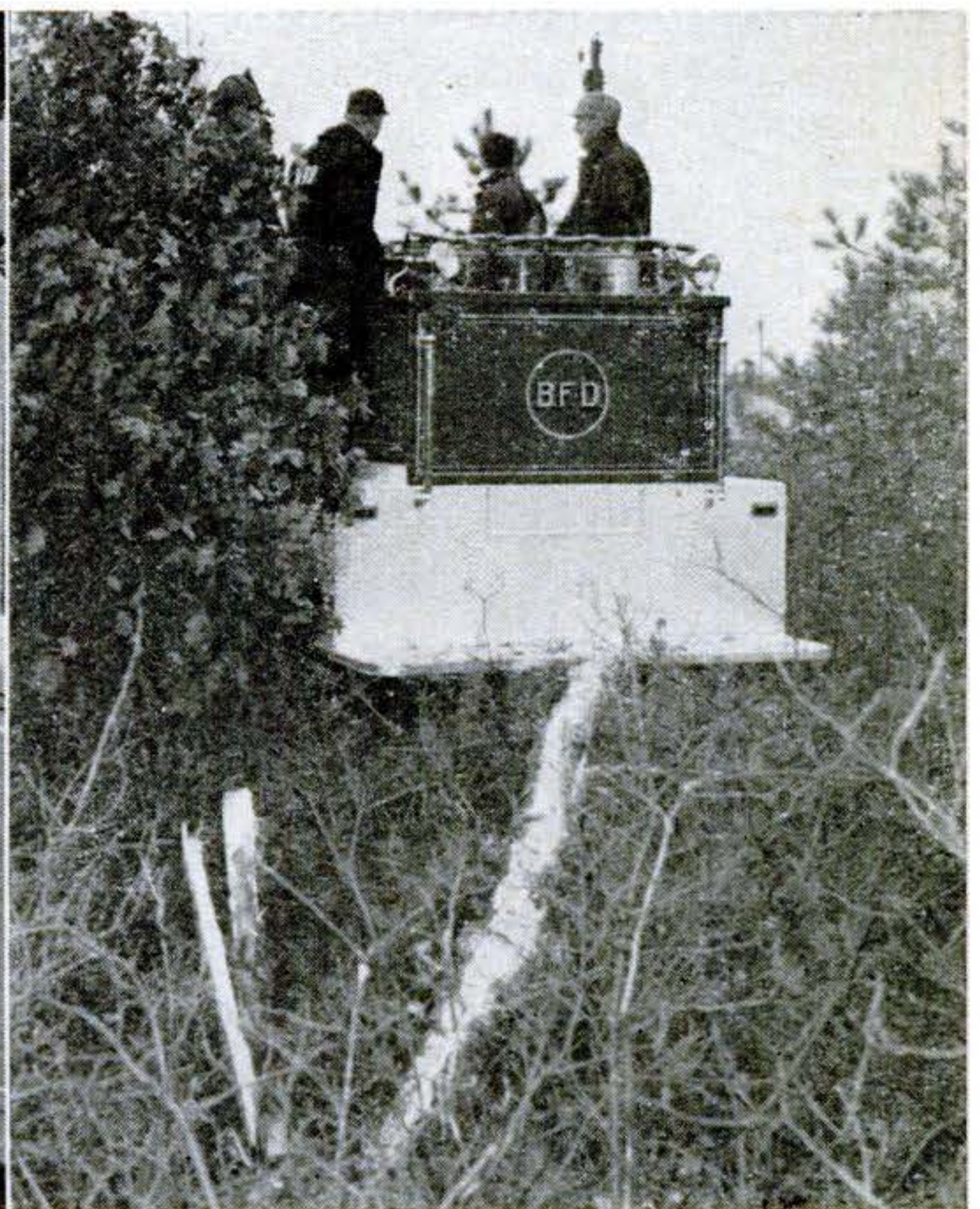
Truck's heavy bumper pushed down this 5-inch tree in demonstration. Truck's ten speeds forward and two in reverse let it traverse practically any terrain. Slowest speed is about 2 m.p.h.
