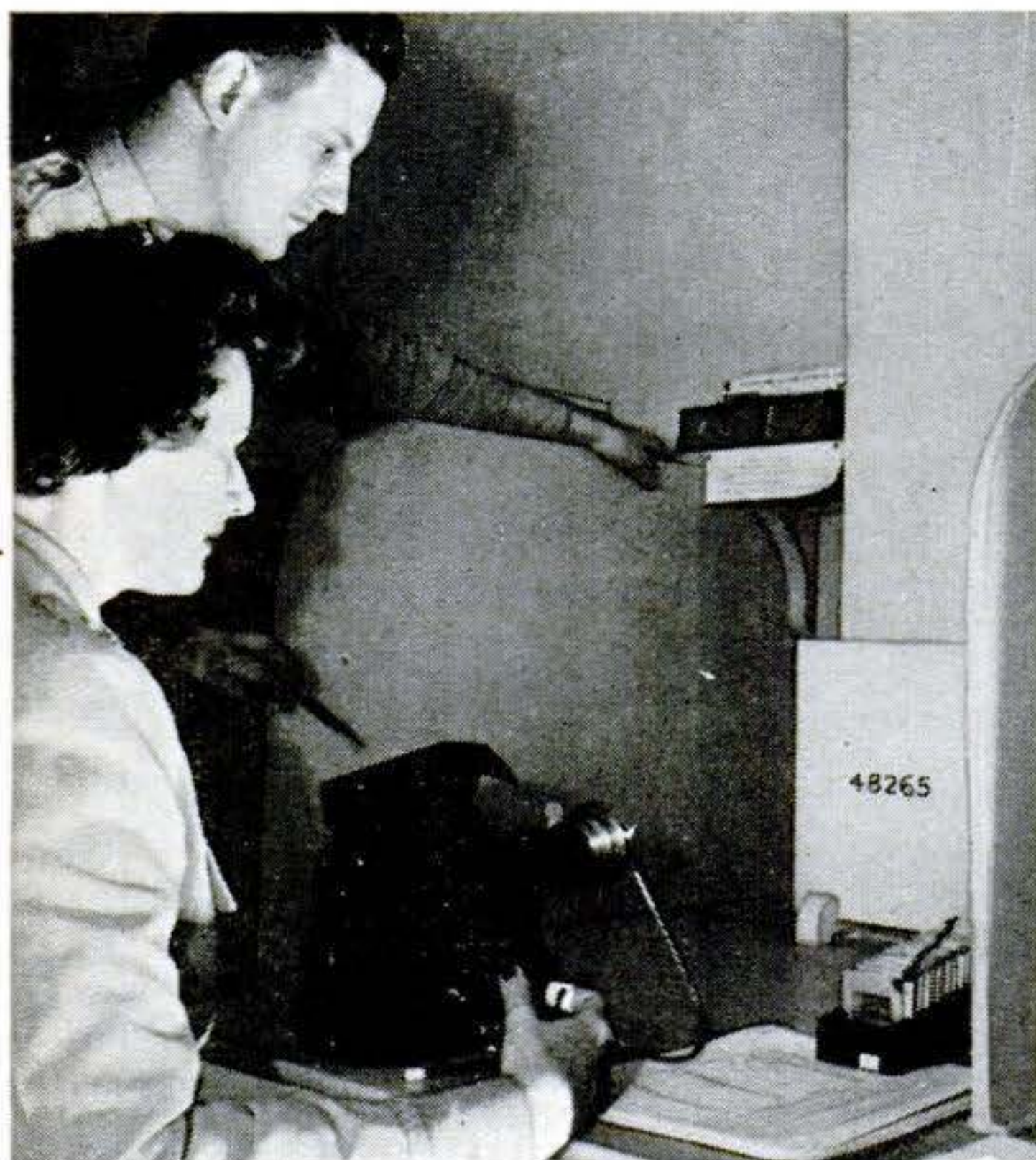
Tachistoscope is short-range projector with camera-type shutter. It flashes numbers on screen at varying speeds. Idea is to learn to recognize longer series of digits in shorter time.
