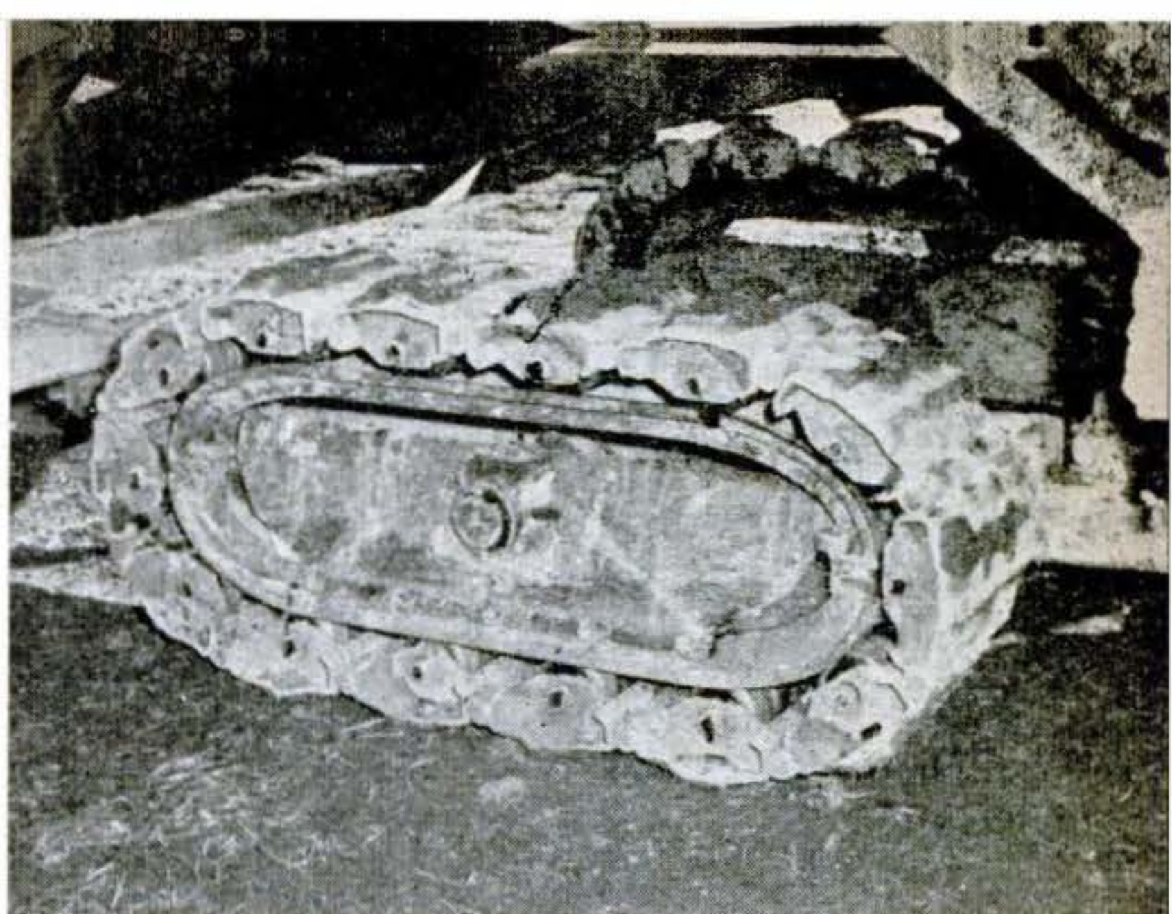
Rear end of loader rides on crawler tracks having individual rollers on each shoe. Tracks spread weight over large area, providing good flotation and stability on soft or uneven ground.
