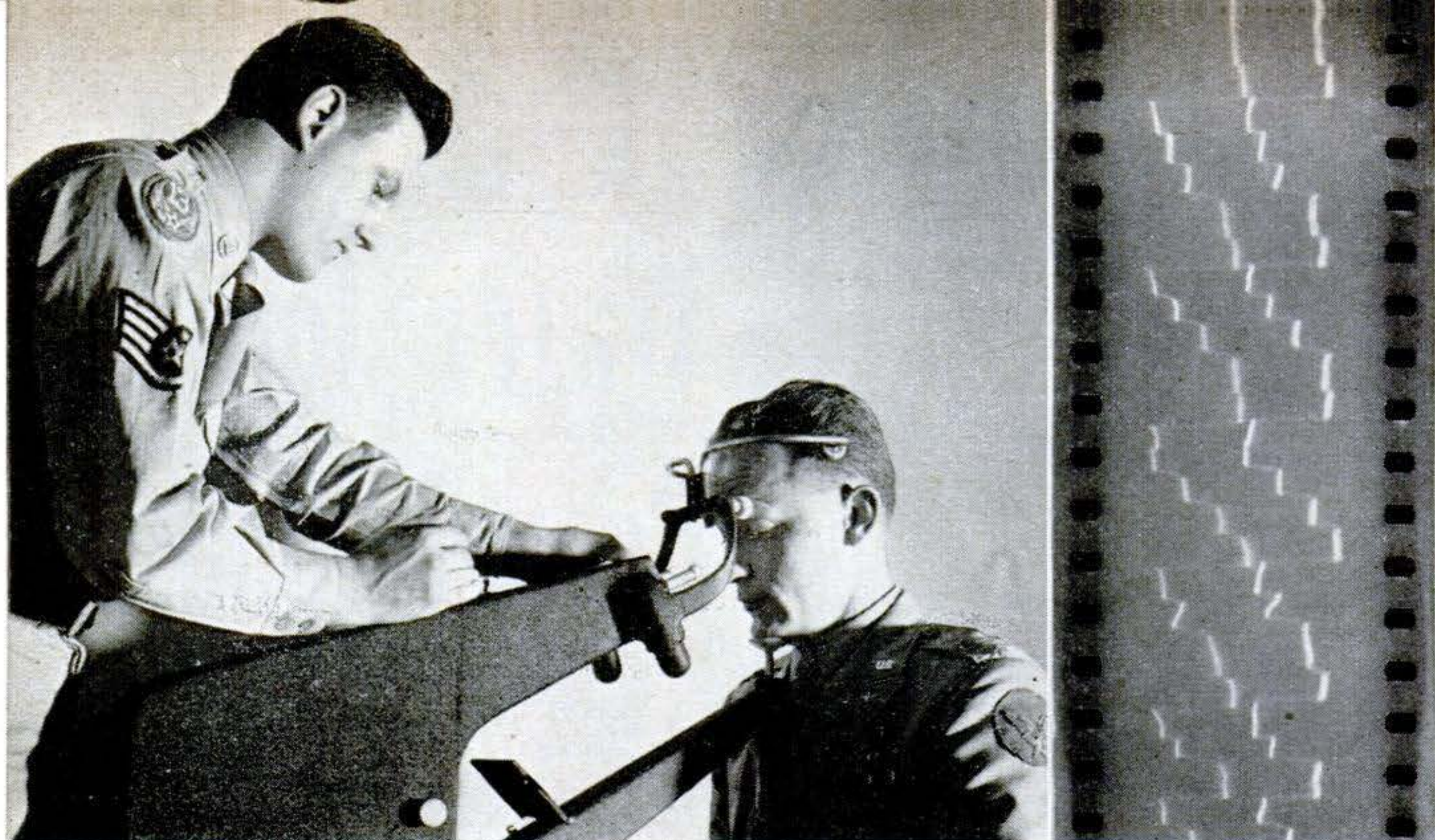
Movement of eyes while reading test passage is photographed in ophthalmograph. Film at
