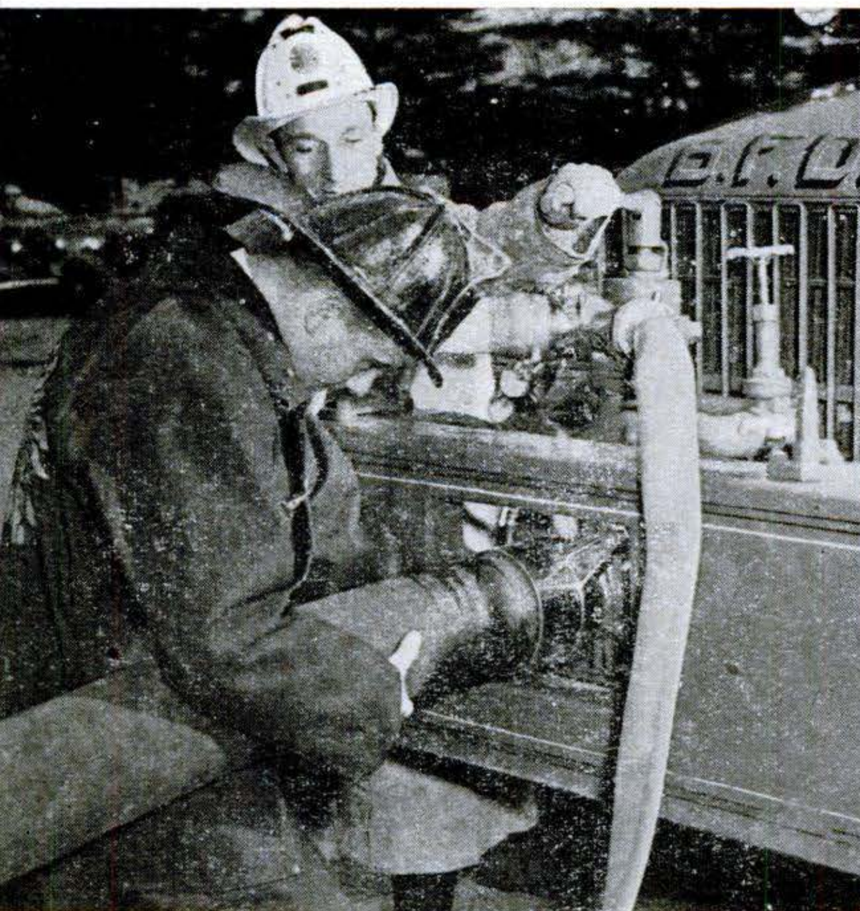
Where hydrant is available, hose coupling in bumper aperture takes standard 4-inch intake hose. Water can be discharged at 200-lb. pressure through one 1½-inch and one 2½-inch nozzles.
