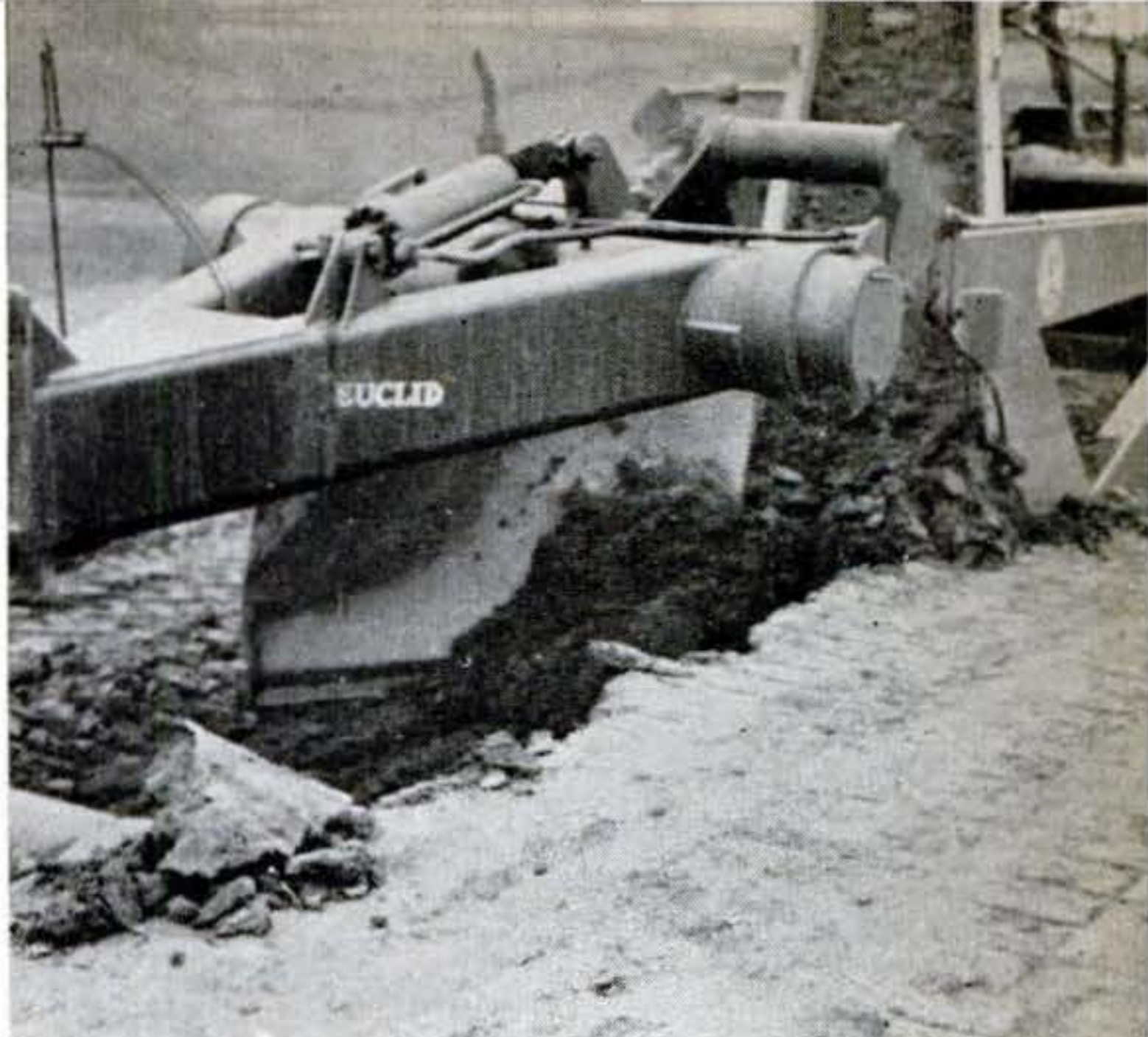
Close-up of big mouth in action shows how dirt sheared off by large, plowlike blade and edge-cutting blade at side is funneled into 35-foot-long rubber conveyer that feeds it to trucks.
