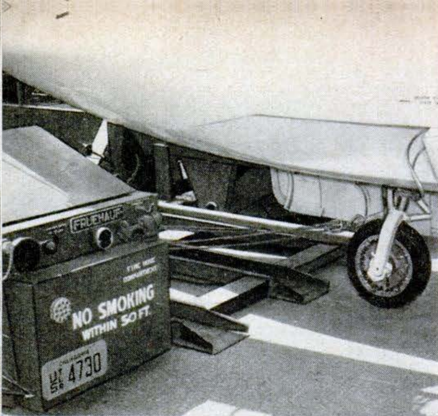
When the aircraft is aboard, electric motors return loading gear to place. The plane can be fueled while it is traveling. A portable pump supplies pressure to a pair of fire hoses.
