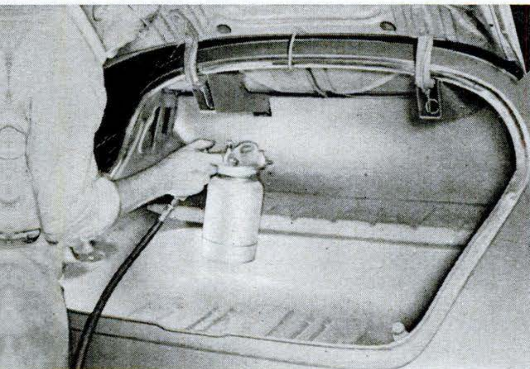
A contribution to quietness as well as protection of luggage is hair flocking of rear compartment with spray gun. This simulated-cloth covering is good for lifetime of the automobile.
