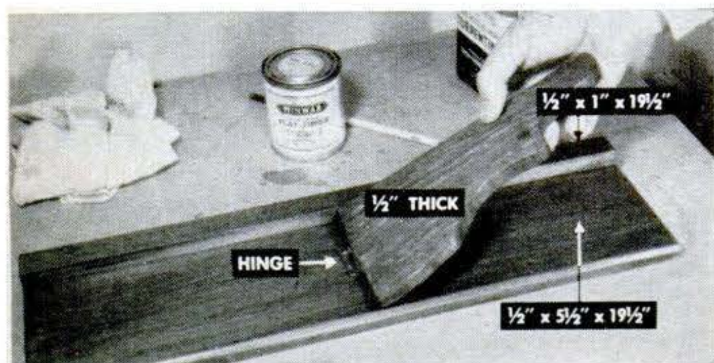
Bracket that supports wall table is hinged in exact center of piece that is screwed to wall.
