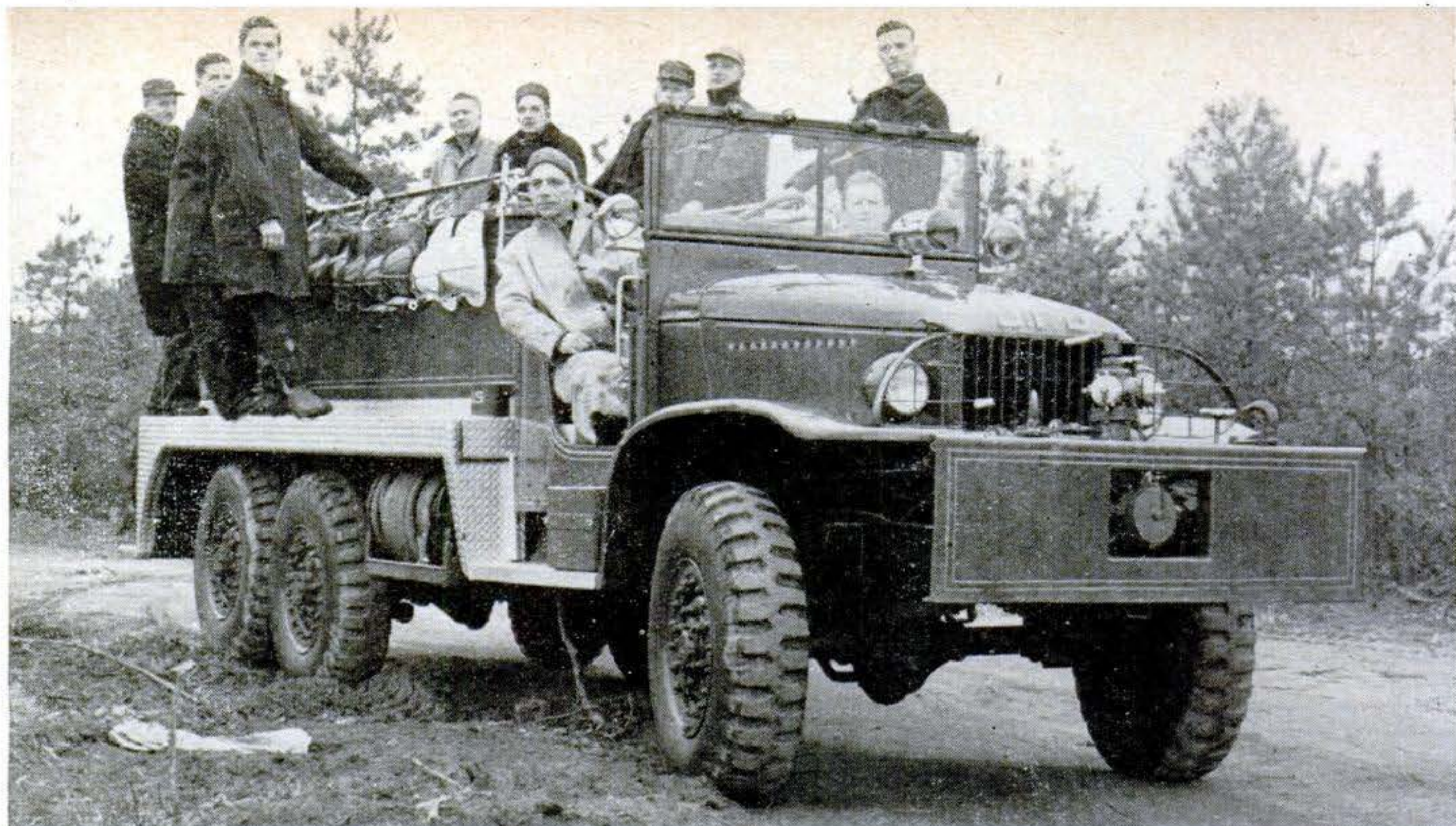
Fog-dispensing truck has 12 nozzles, six to a side under catwalks, that can produce either spray or straight streams. In addition, men on catwalks can fight fire with hand fog guns.
