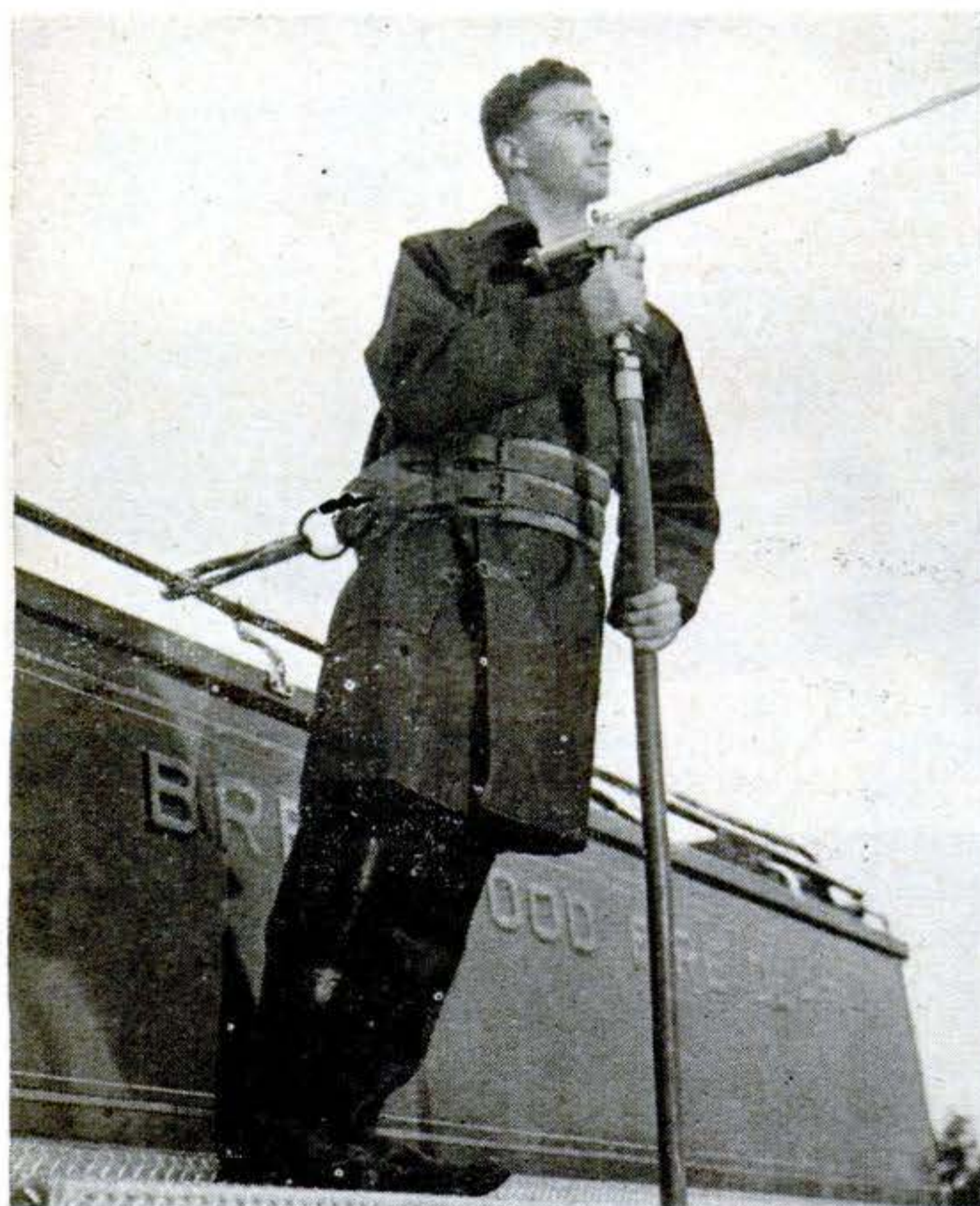
Safety belt connected to sturdy rail on top of truck frees fireman's hands so he can use fog gun while truck moves rapidly through fire. Truck's 817-gal. tank can be filled from pond or stream.
