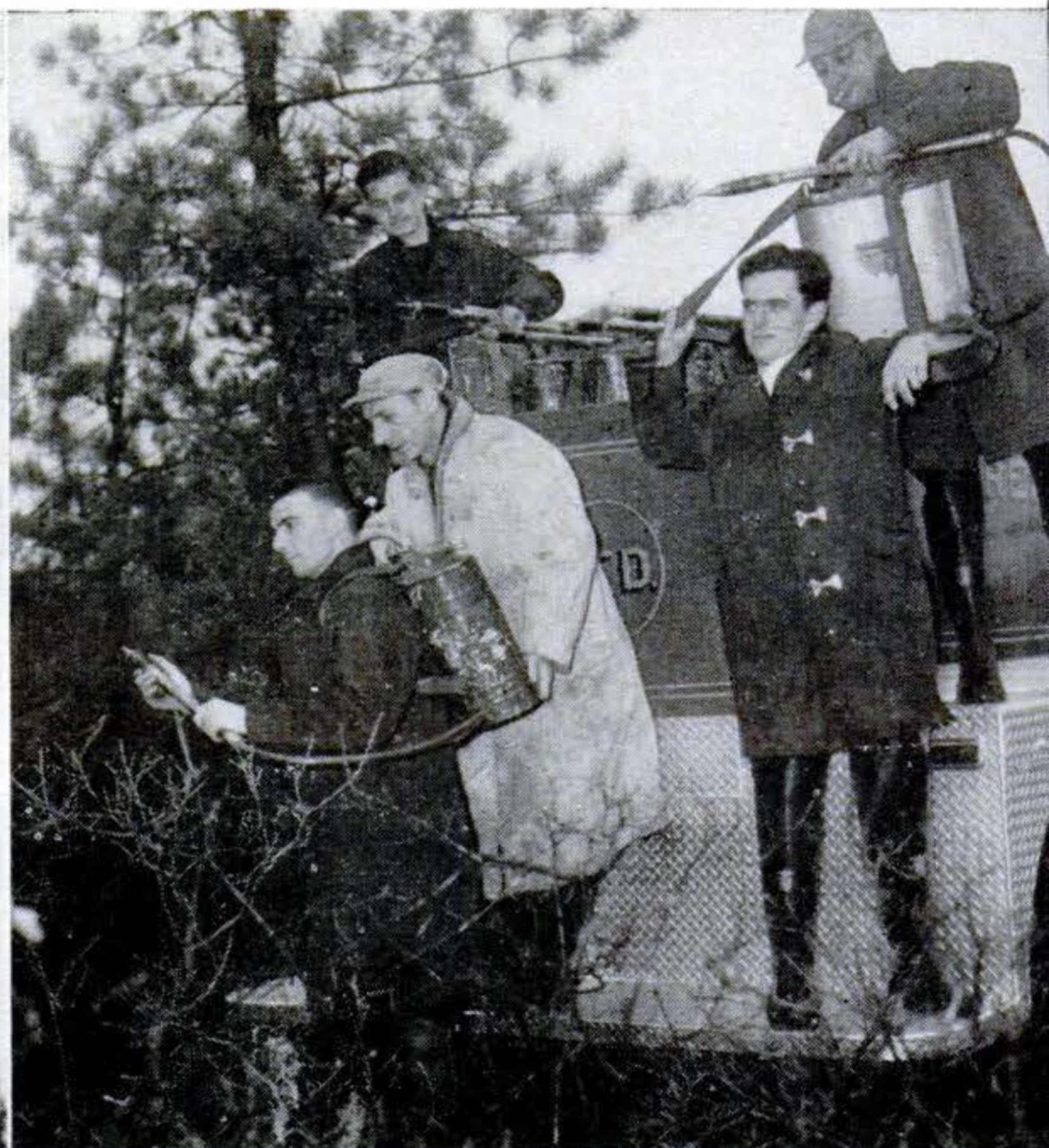
Dozen 5-gallon cans equipped with hand pumps are carried on top. These are dispensed to firemen who are dropped off to fight fringe of fire as truck proceeds to fog out head of it.
