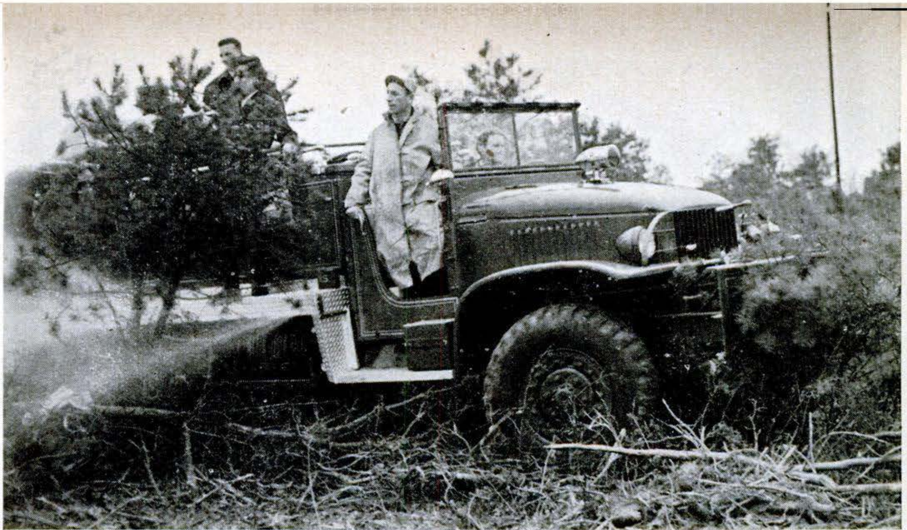
Fog streams shown above protect crew and equipment if truck becomes encircled by fire—
