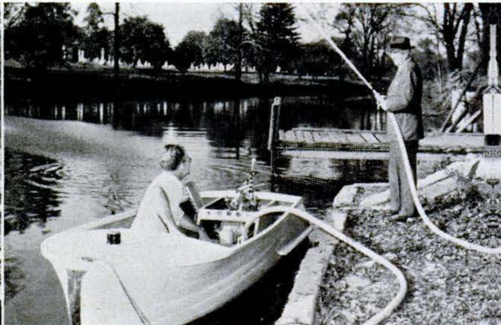
Attach a hose to the pump unit, and you have a one-man fire department. With the motor going at full speed, a stream of water can be shot 60 feet into the air under 85 pounds pressure.
