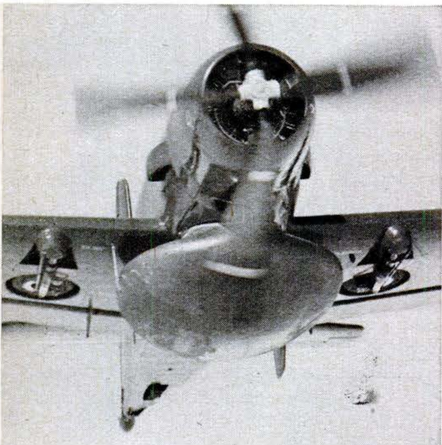
Douglas Skyraider (AD3W) is carrier-based search plane. The huge plastic radome underneath houses the radar antenna. Possibly teamed up with specialized killer plane with emphasis on weapons.
