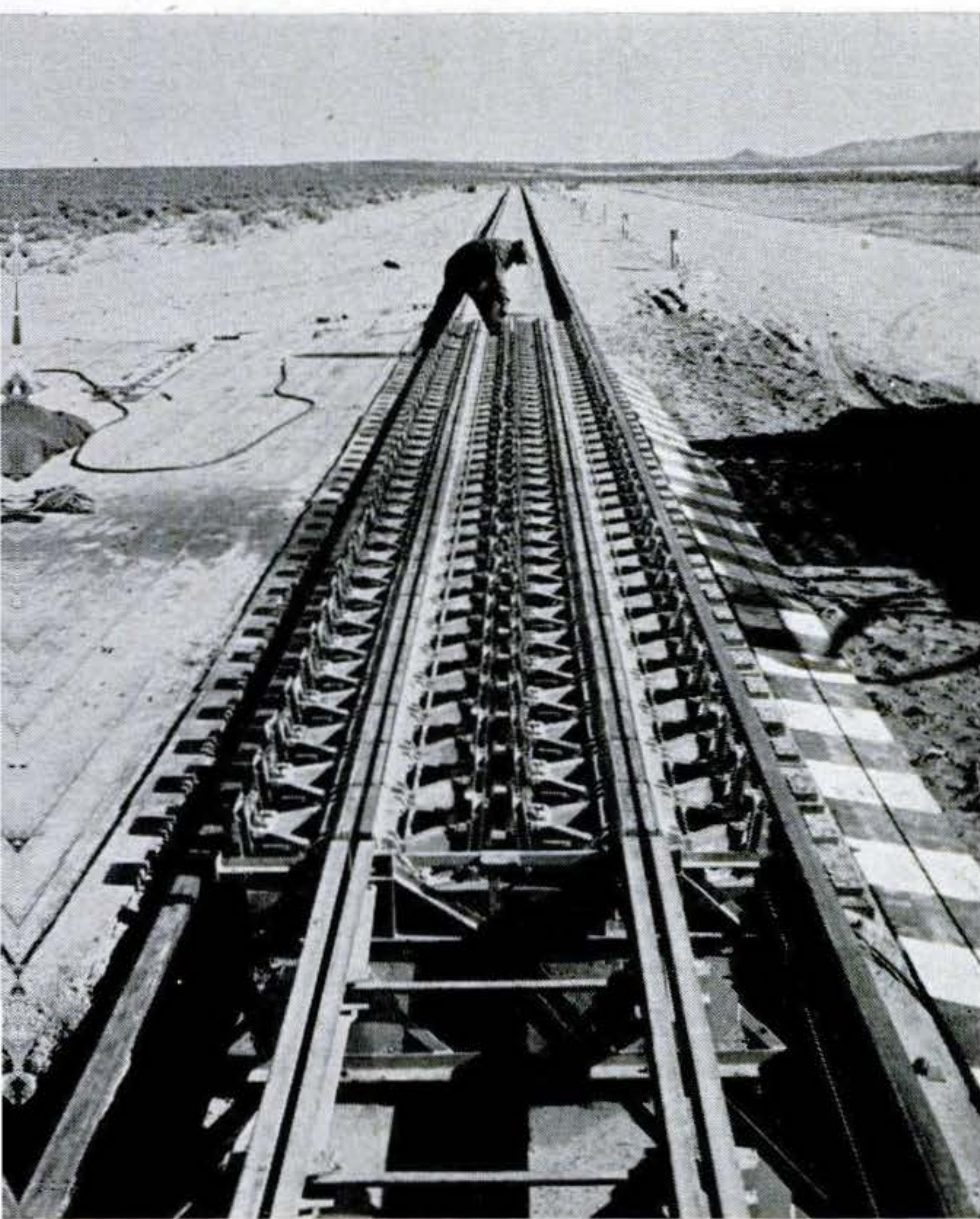
Braking section of track begins 1,250 feet from starting point of sled's run and is about 50 feet long. Slots of inner rails guide sled's braking runners between pairs of brakes.
