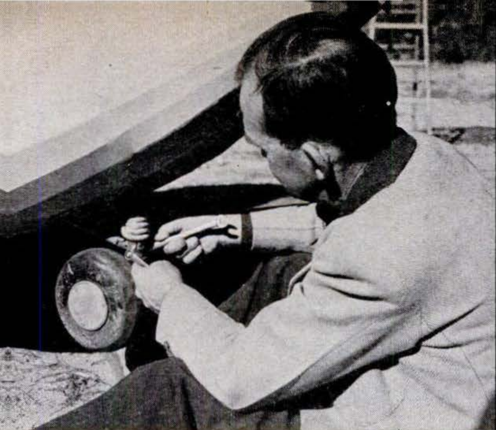
Steerable nose wheel can be retracted manually after take-off. Five-inch tires are normally used on airplane tail wheels. Mabel's pilot performs with air show called Hollywood Hawks.
