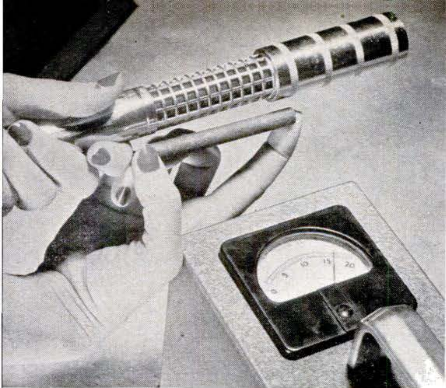
Needle of ray-detecting Geiger counter swings across dial when probe connected to counter is held beside uranium metal. Meter is set for low sensitivity, or needle would go off dial.
