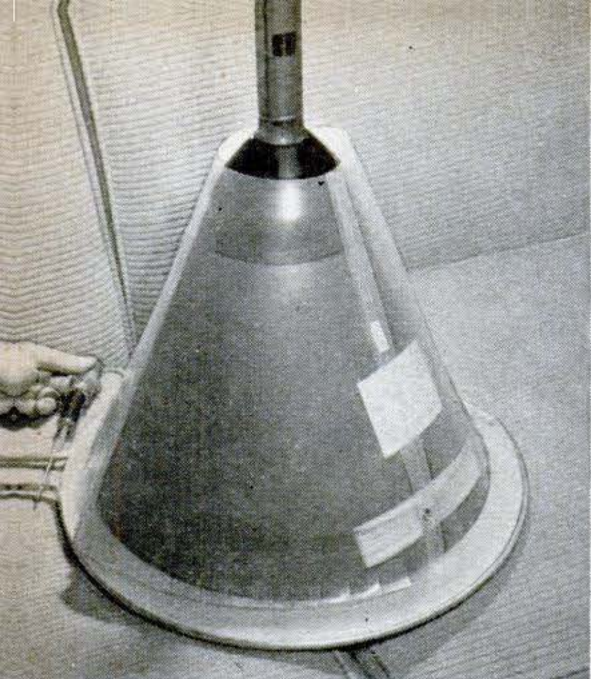
13 The entire metal shell of the 16AP4 is "hot," so it's wise to cover it with a plastic insulating hood and ring. The brackets I bought had a metal ring support.
