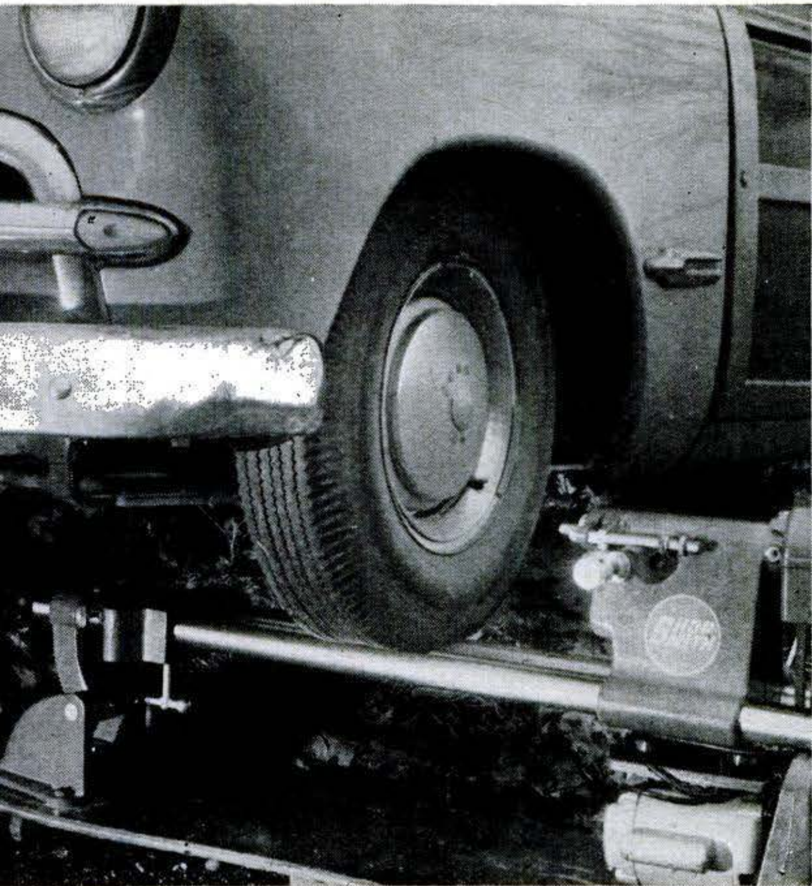
Tubular ways are rugged and rigidly parallel. They went through this strength test unharmed.
