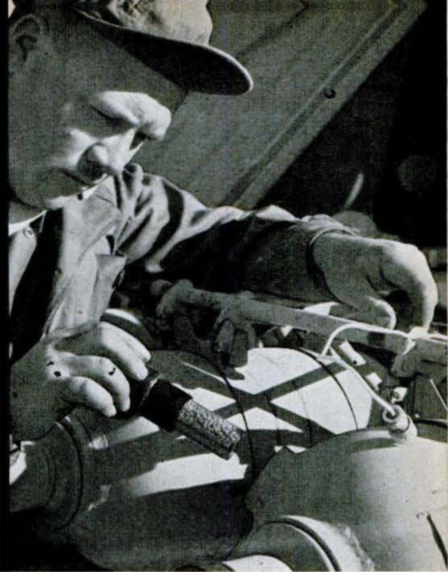
Last step before run is arming rockets. Electric igniter resembling spark plug fires rocket by touching off highly active pelleted powder. Its flames ignite solid-fuel propellant.
