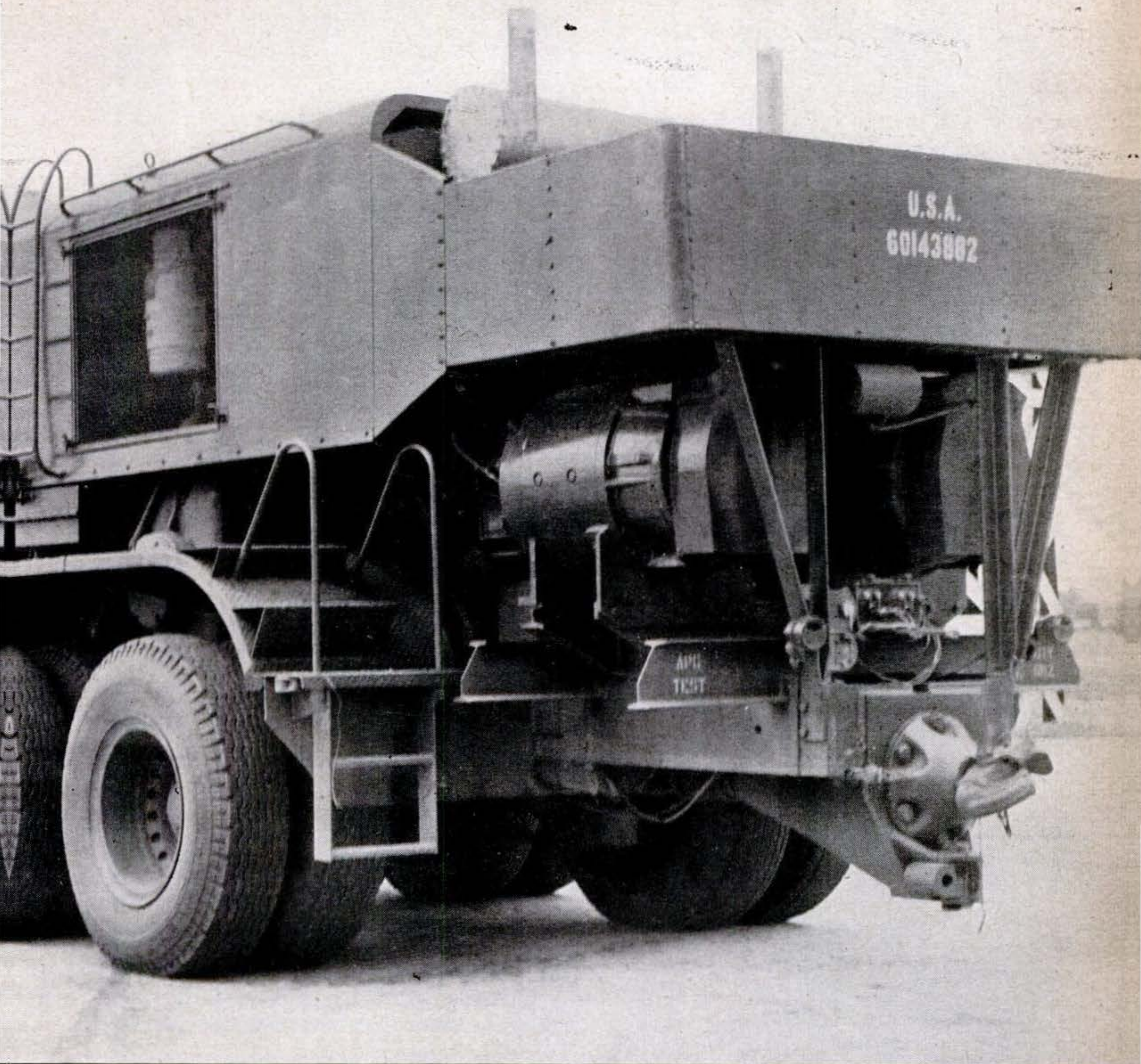
train has two 500-hp. engines driving generators that run four motors that drive wheels.
