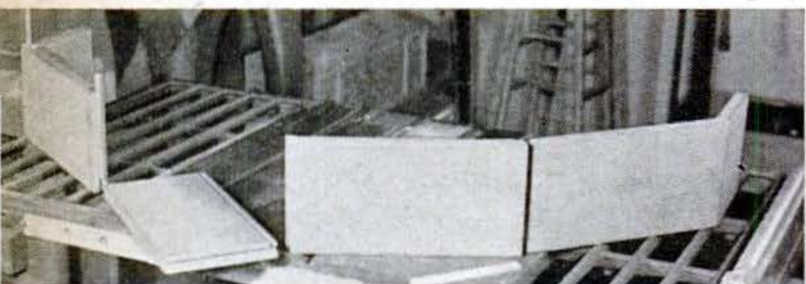
After the segments of the outer box are cut to shape and the ends grooved for splines, the pieces are checked for correct joint fit.
