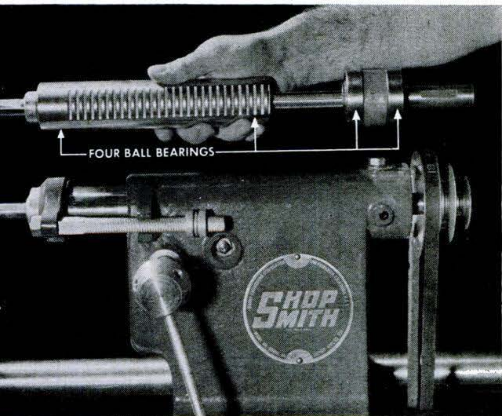
Four ball bearings in arbor give tool unusually smooth, quiet operation. Using quill to position saw blade allows fine adjustments, permits dado cutting without special blade or washers.
