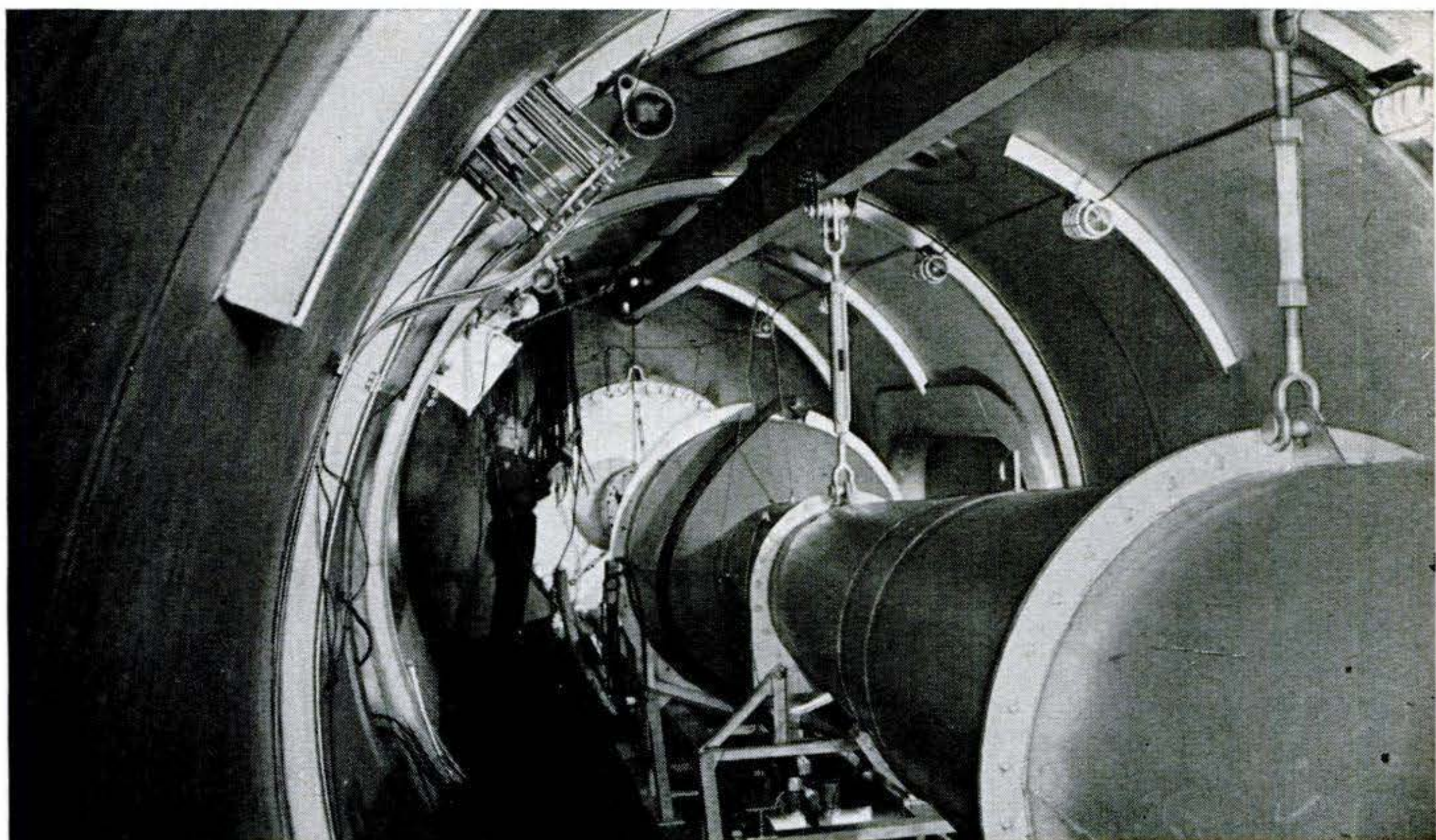
Engine under test is mounted just beyond flaring section of exhaust pipe (center) in big tank.
