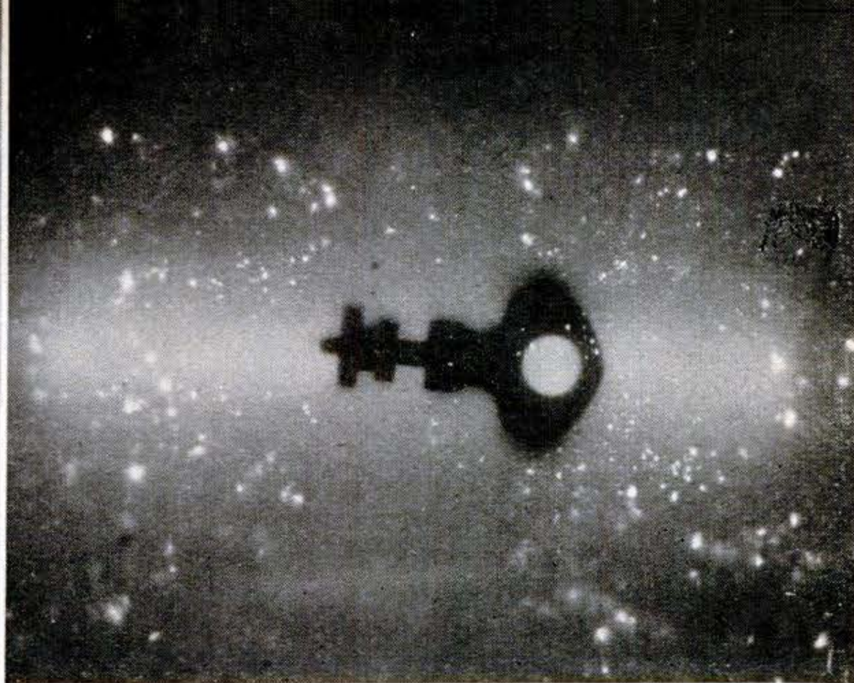
Rays from uranium rod, laid over key on photo film in darkroom, took this picture of key. Rod itself made the glow extending across picture. This is a print from developed negative.
