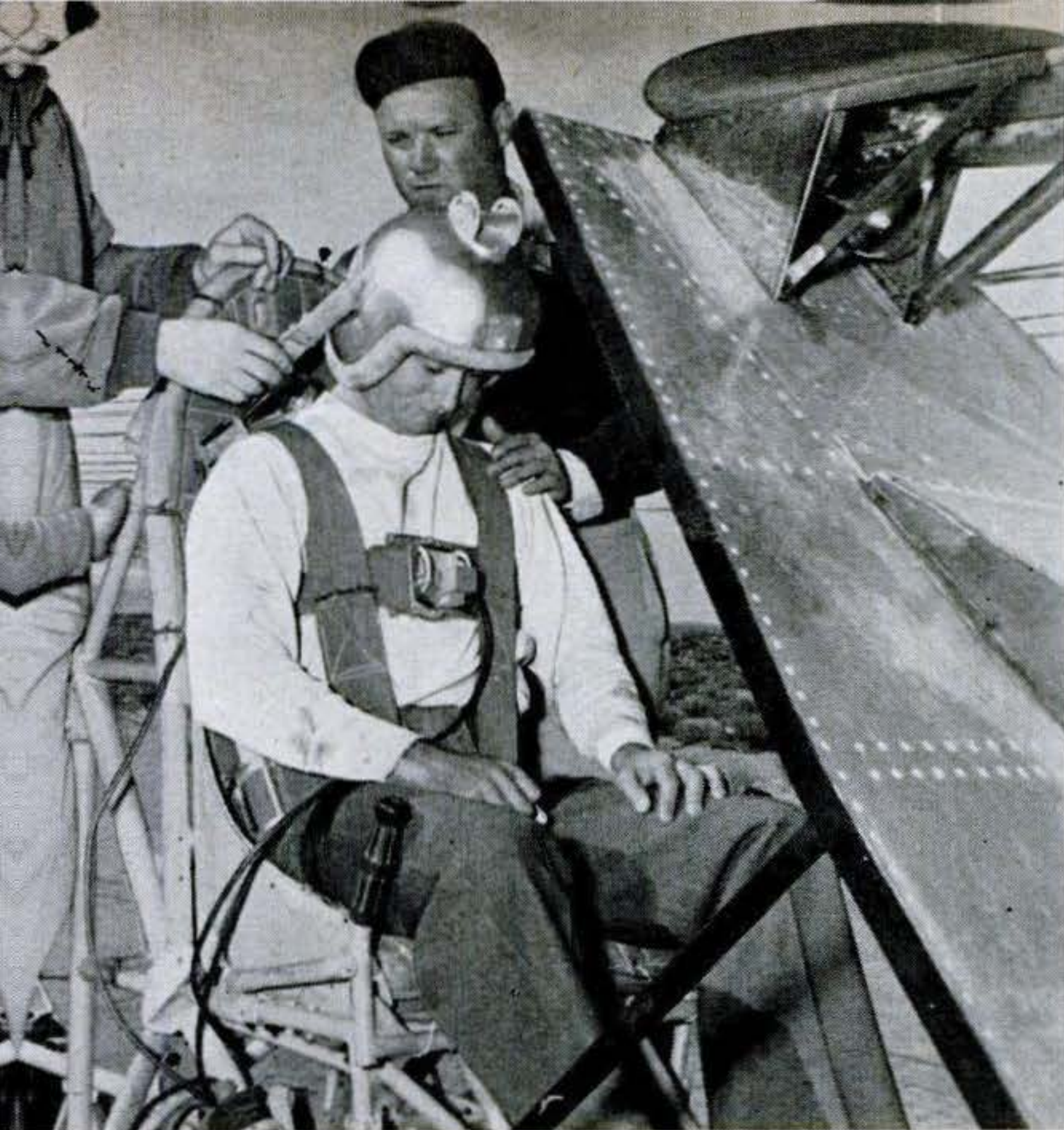
Helpers strap rider in seat and adjust his crash helmet in preparation for a run. Gauges attached to his chest strap and helmet register the G-forces to which his body is subjected.
