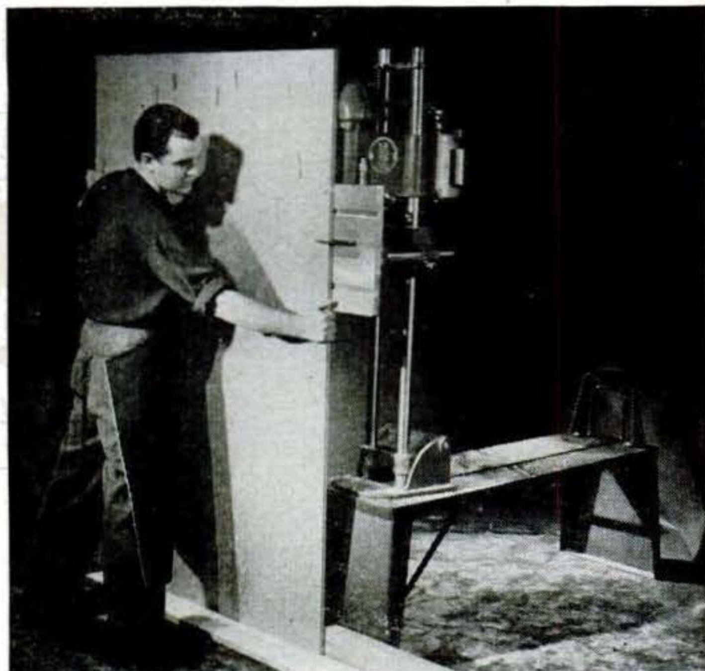
Need to saw large, heavy pieces? Just up-end saw and feed work vertically. Guide for bottom edge is plank on floor. Pressing work against table keeps it flat and the cut straight.
