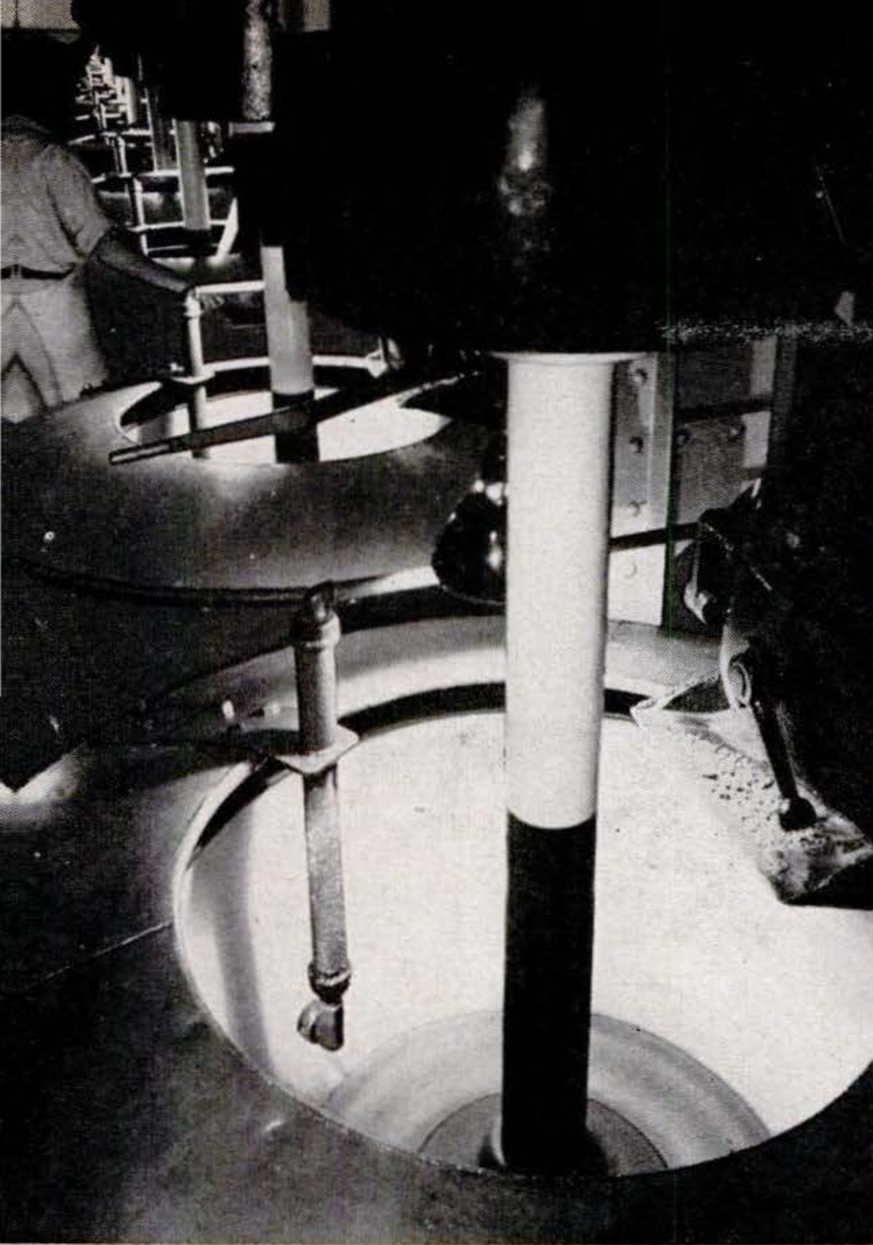
2 After molasses coating on raw sugar is softened with a heavy sugar-and-water syrup, mixture is washed and whirled in centrifugal machine above to remove some impurities.
