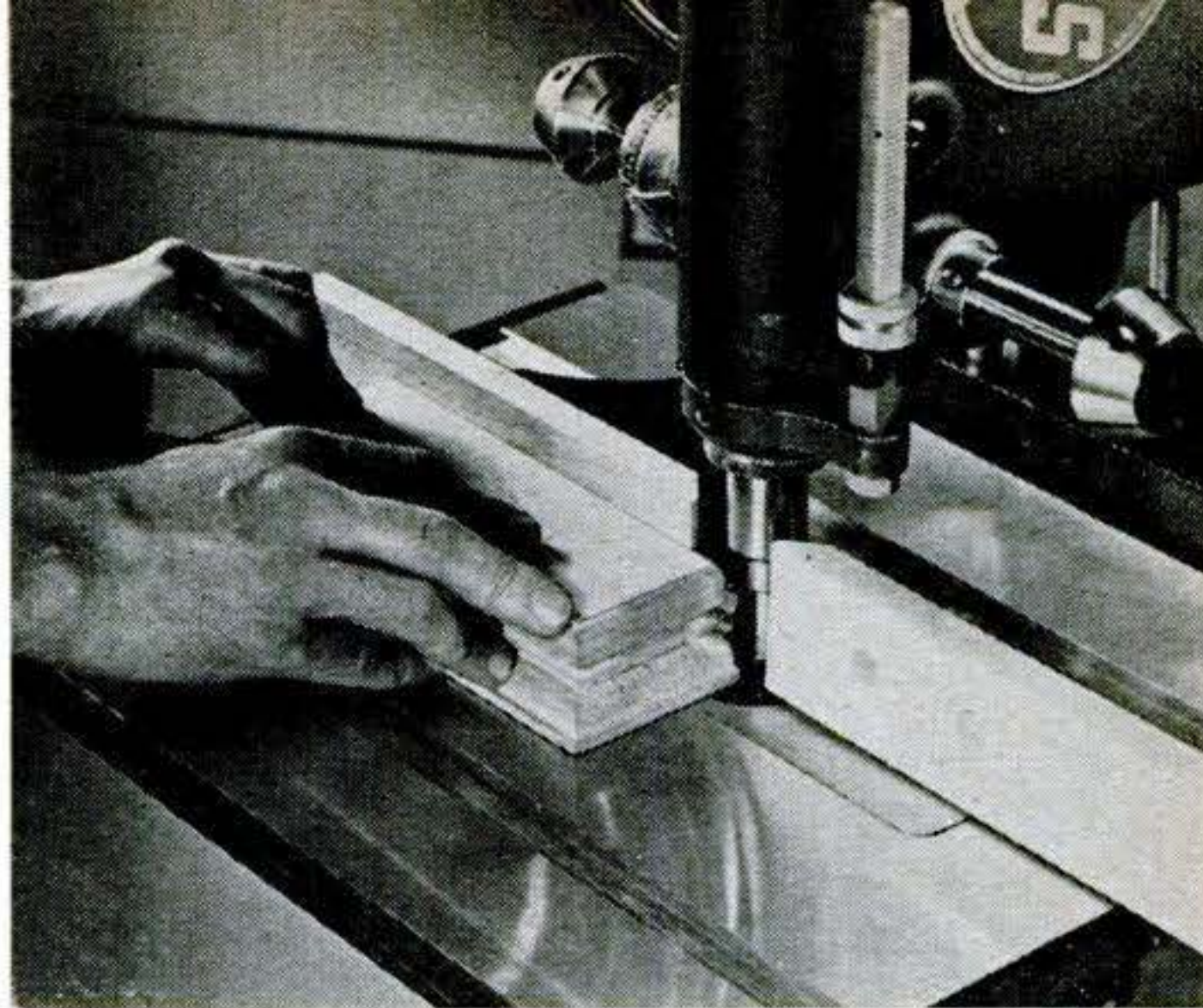
With special fence and attachments, tool can be used to shape, as shown above, or joint, rabbet, and mortise. Different-sized table inserts permit various tools to fit through table.
