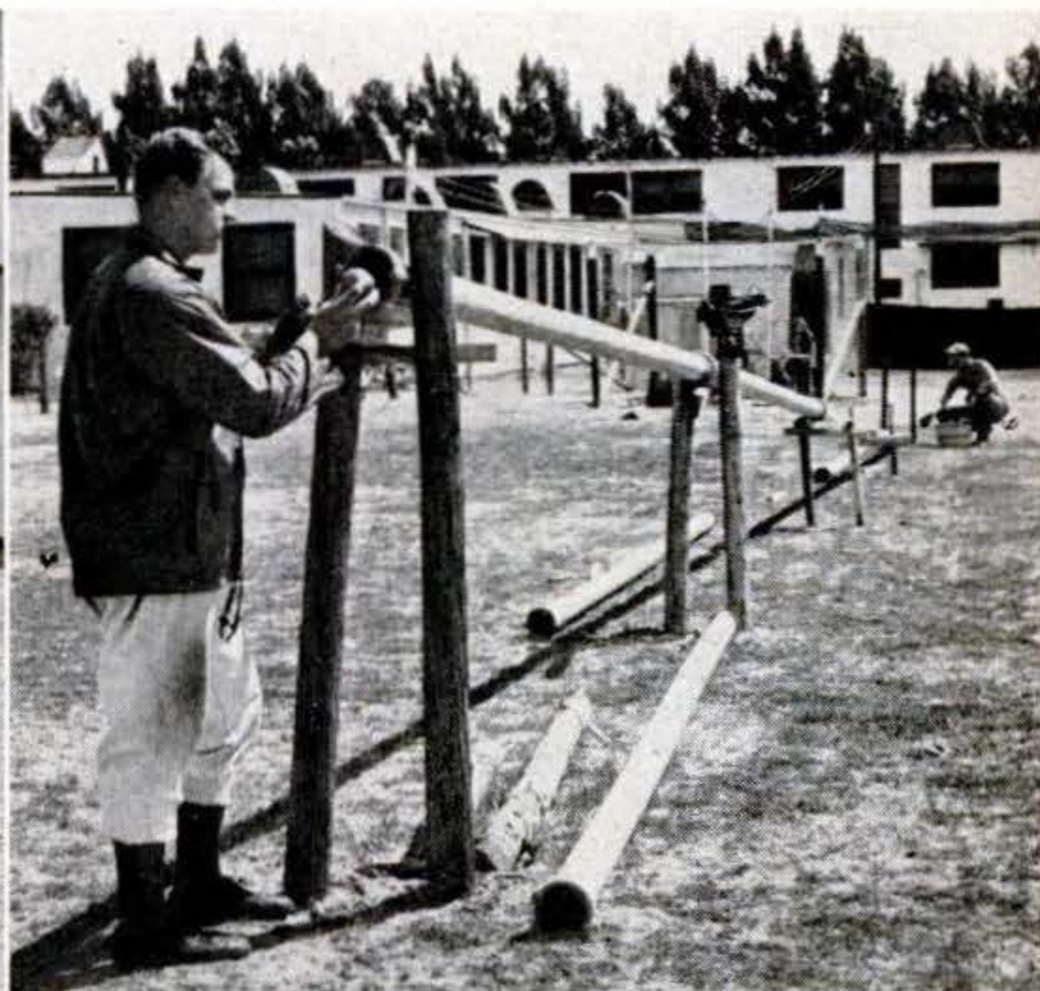
Gravity system for returning balls from outfield saves work for fly-chasers. Attendant gathers balls and drops them into pipeline back to pitching machine aimed high for long range.
