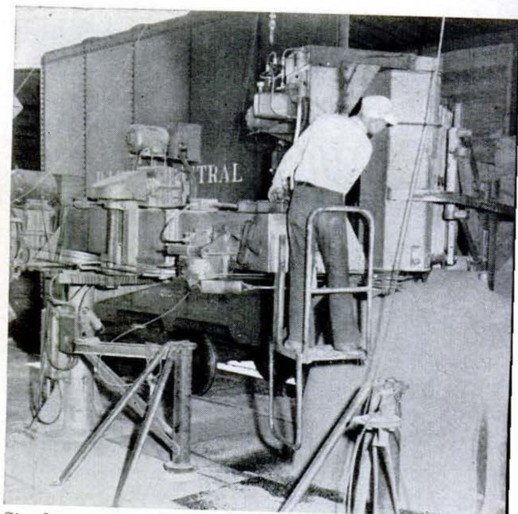
Single operator, riding arm on platform, need only aim scoop toward desired part of car. After this, its extend-dig-retract cycle is automatic. It is made by Stephens-Adamson Co., Los Angeles.
