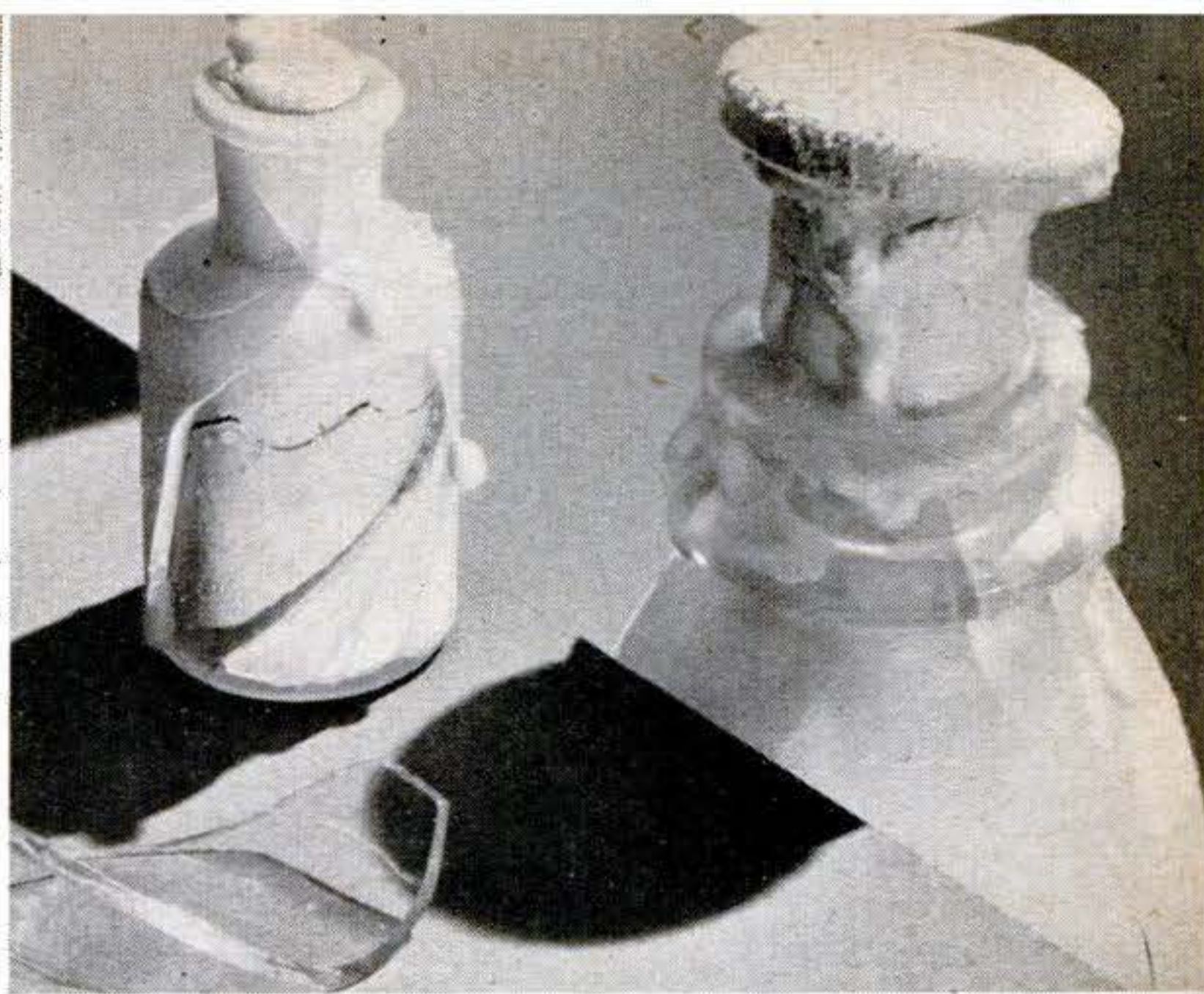
Expanding as it freezes , gallium cracks bottle at left and exudes from its neck, just like frozen milk in bottle at right. Rubber syringe bulbs make unbreakable containers for shipping.
