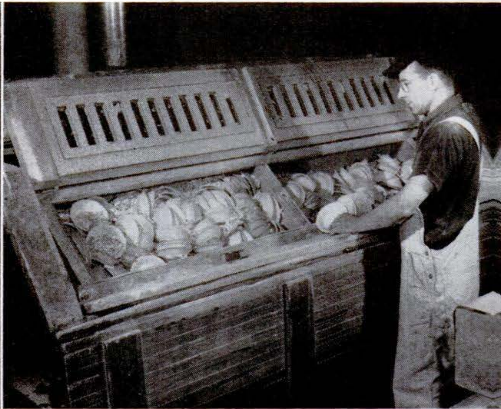
17 Biscuits, as fired pieces are called, are so tough that they can be smoothed down by tumbling them in long motor-driven drums partially filled with broken pieces of china.
