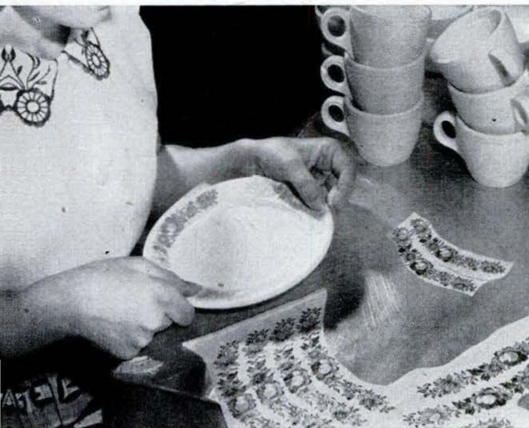
18 Underglaze decoration. Decorations using metallic oxides that can stand high heat can be applied before piece is glazed. These are printed on with lithographic transfers.
