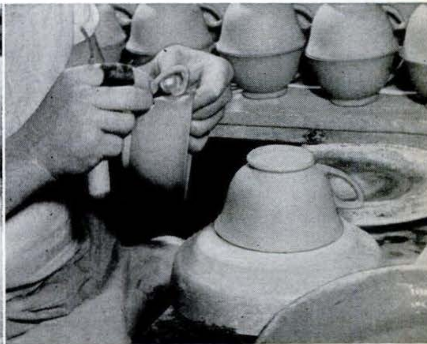
9 Handles for cups are cast separately and, after being trimmed by hand with a knife to fit the double curves of the cup, are cemented in place with liquid body mixture.
