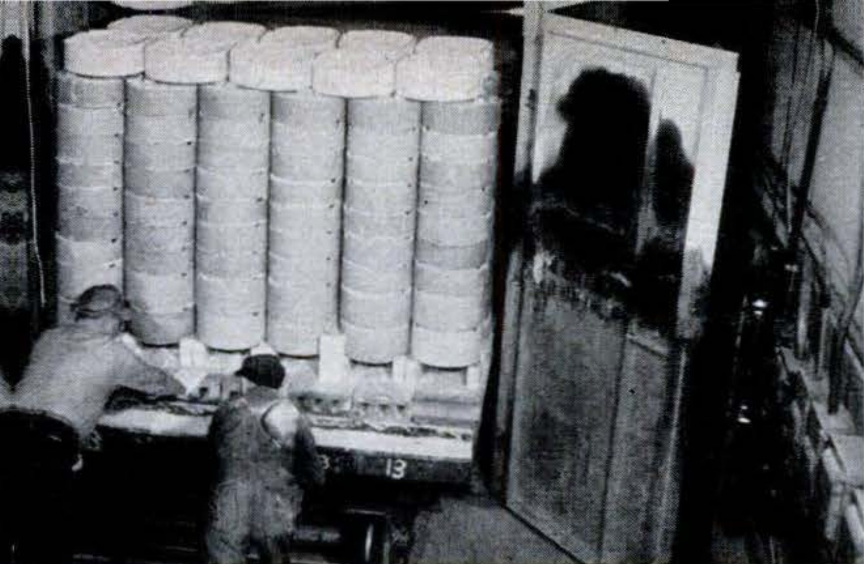
14 Into the tunnel kiln for 65 hrs. of firing. As cars progress through kiln, ware is subjected to rising temperatures until about 2,200° F. is reached. Then it is cooled.
