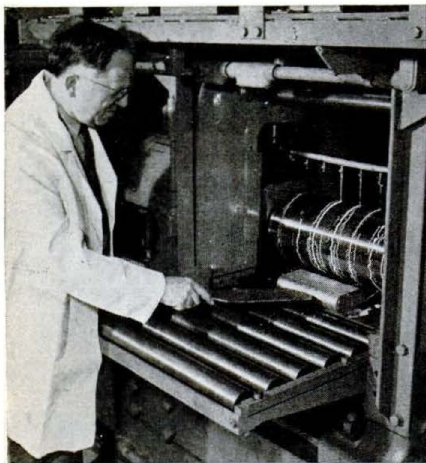
3 When an ingot has been properly heat-soaked, it's pushed in for its first pass through the baby rolling mill. A 50-hp. motor runs mill, which can make sheet only .01 in. thick.
