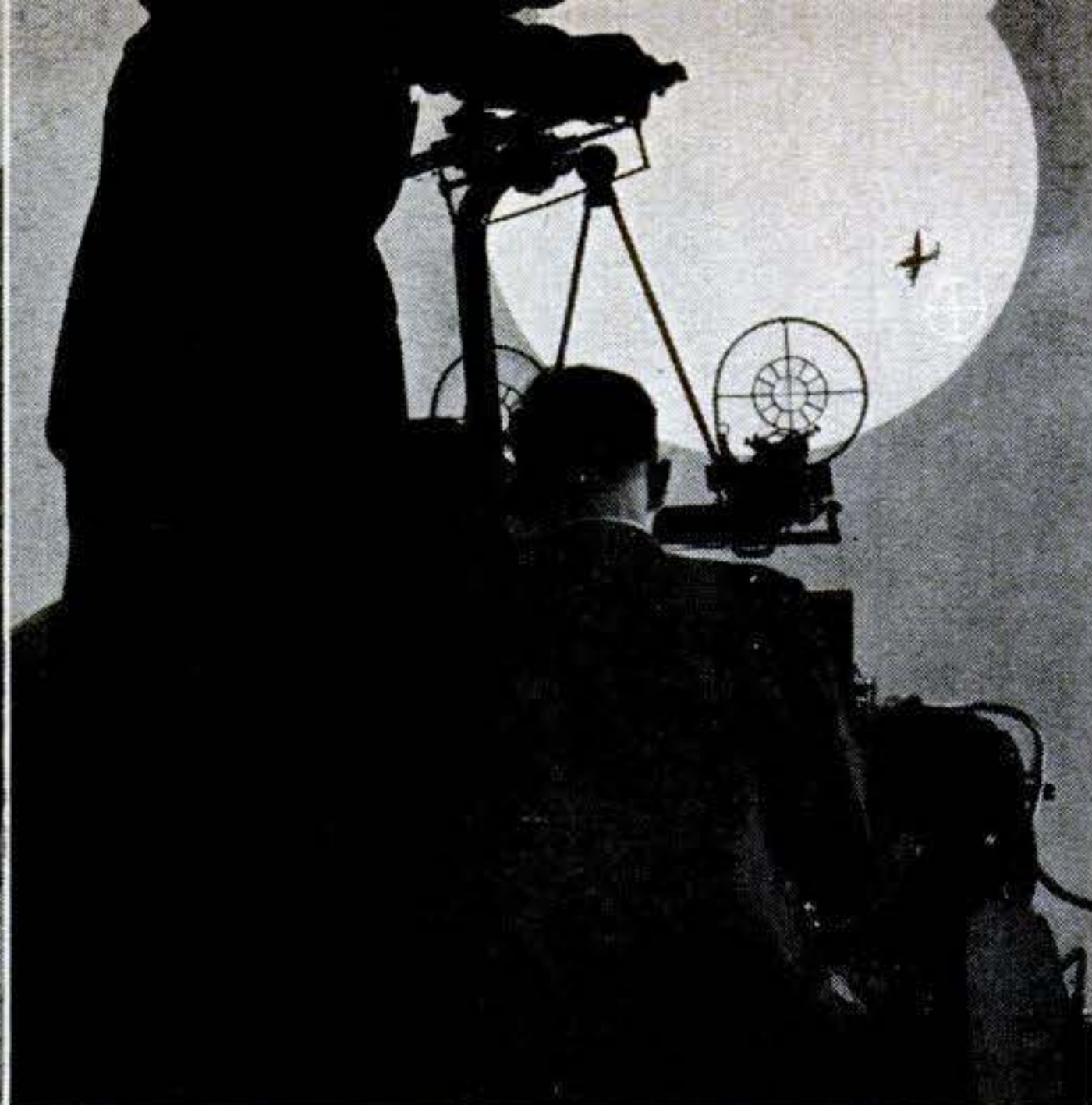
Inside dome , students follow movie target with dummy gun. Gun's sights, also projected onto dome, show instructor how close students are to yellow spot (invisible), correct point of aim.
