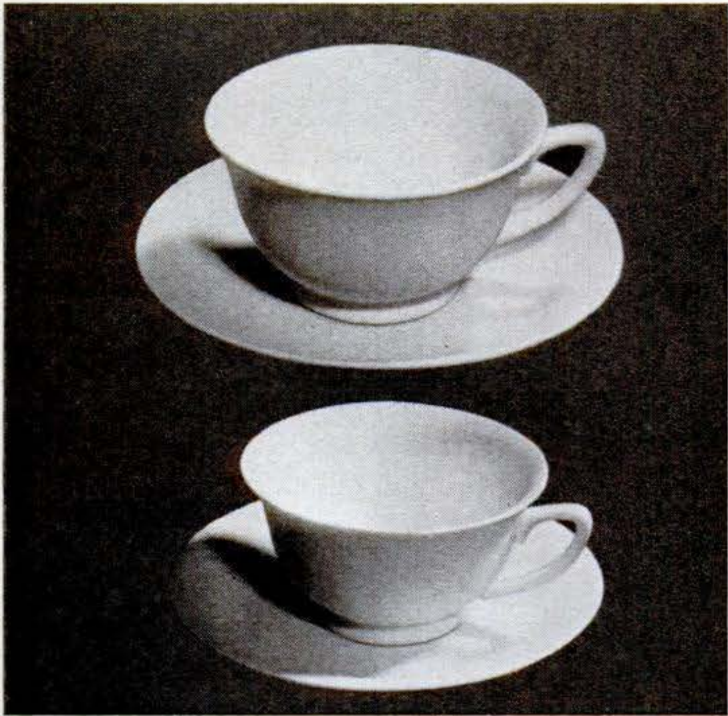
16 Shrinkage. The cup at the top is still in the clay state before firing. The cup at the bottom has been fired. Shrinkage from molding through firing totals 12½ percent.
