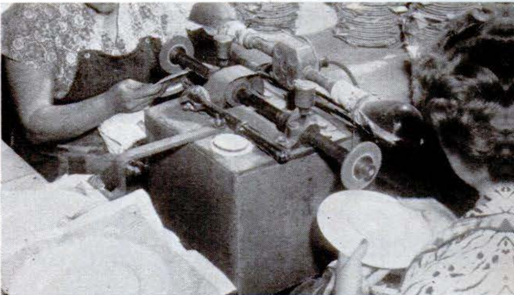
21 Finishing. Any slight imperfections in the glaze, such as marks caused by the pins used to support the plates in saggers during glaze firing, are removed by grinding.
