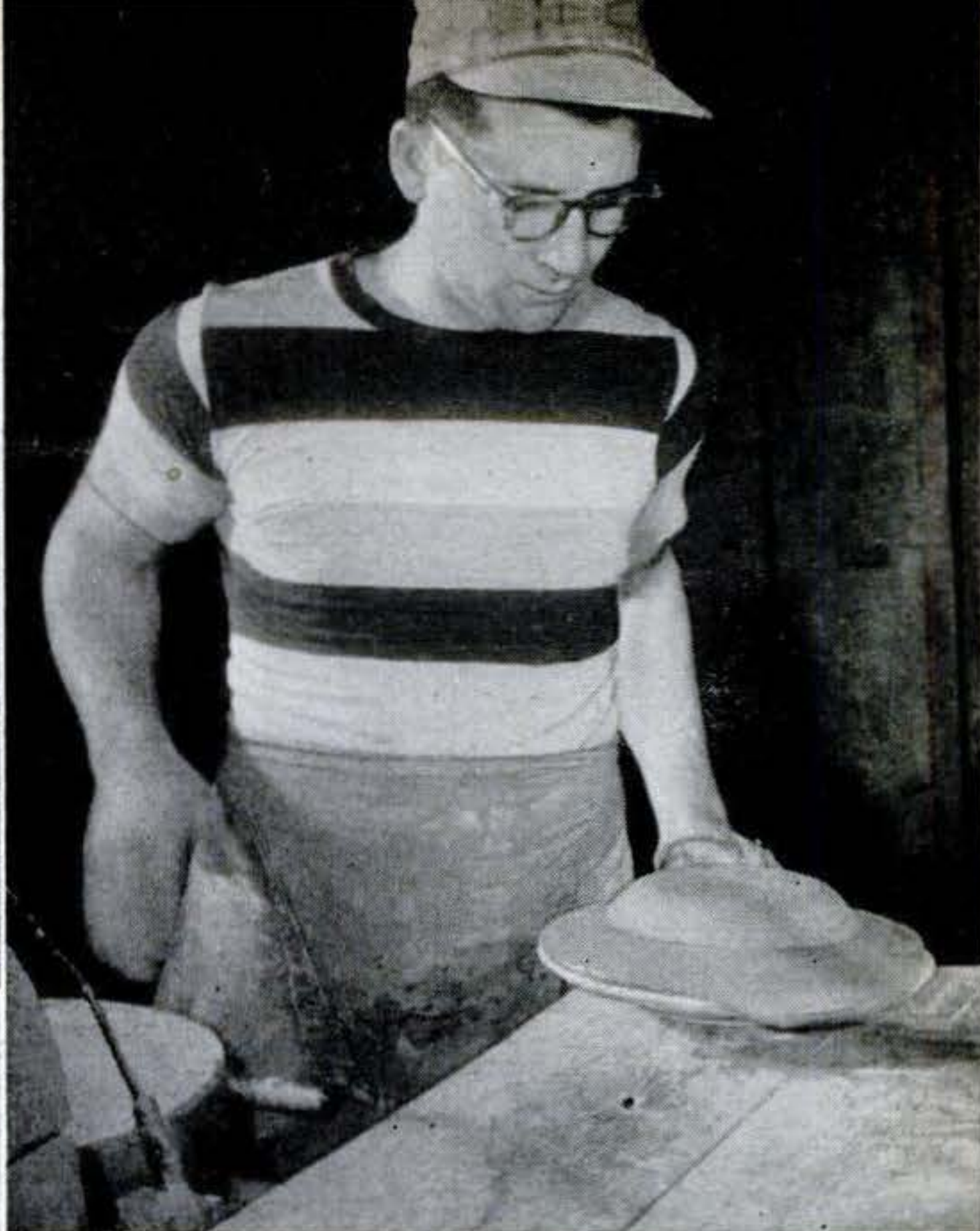
into a flat pancake or bat. The worker then picks up the bat, raises it up high, and slaps it down hard on a plaster-of-Paris mold of the particular piece to be formed.
