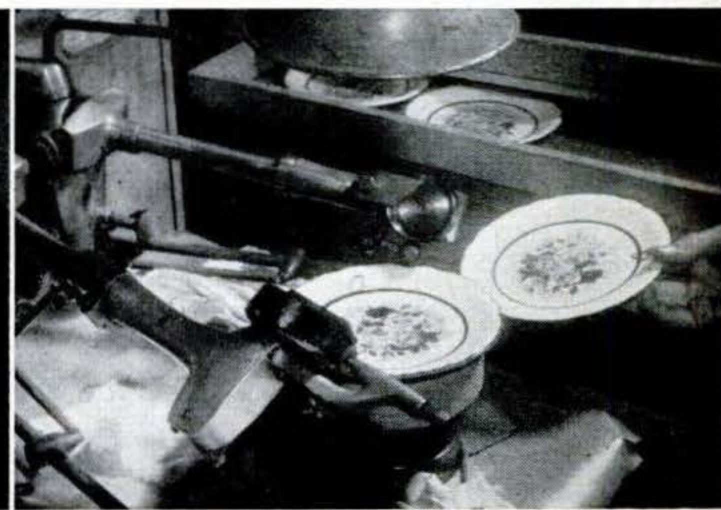
23 Gold edging and stripes are applied by machine. After firing, the gold is burnished to a high luster by hand with a burnishing stick made up of tiny glass fibers.
