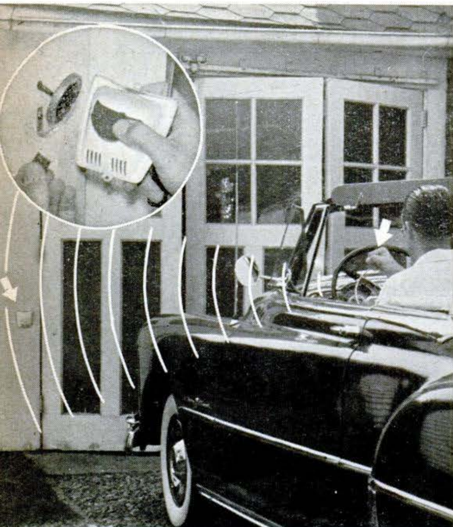
Automatic garage doors can be honked open with this sound-operated switch. Mike is cushioned on rubber, enclosed in a watertight hood.
