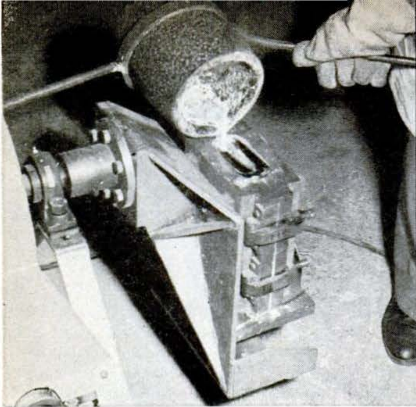
1 Molten metal is poured into a mold during the process used to make aluminum sheeting at the Kaiser Co.'s miniature mill, where alloys are tested before being run through big mill.
