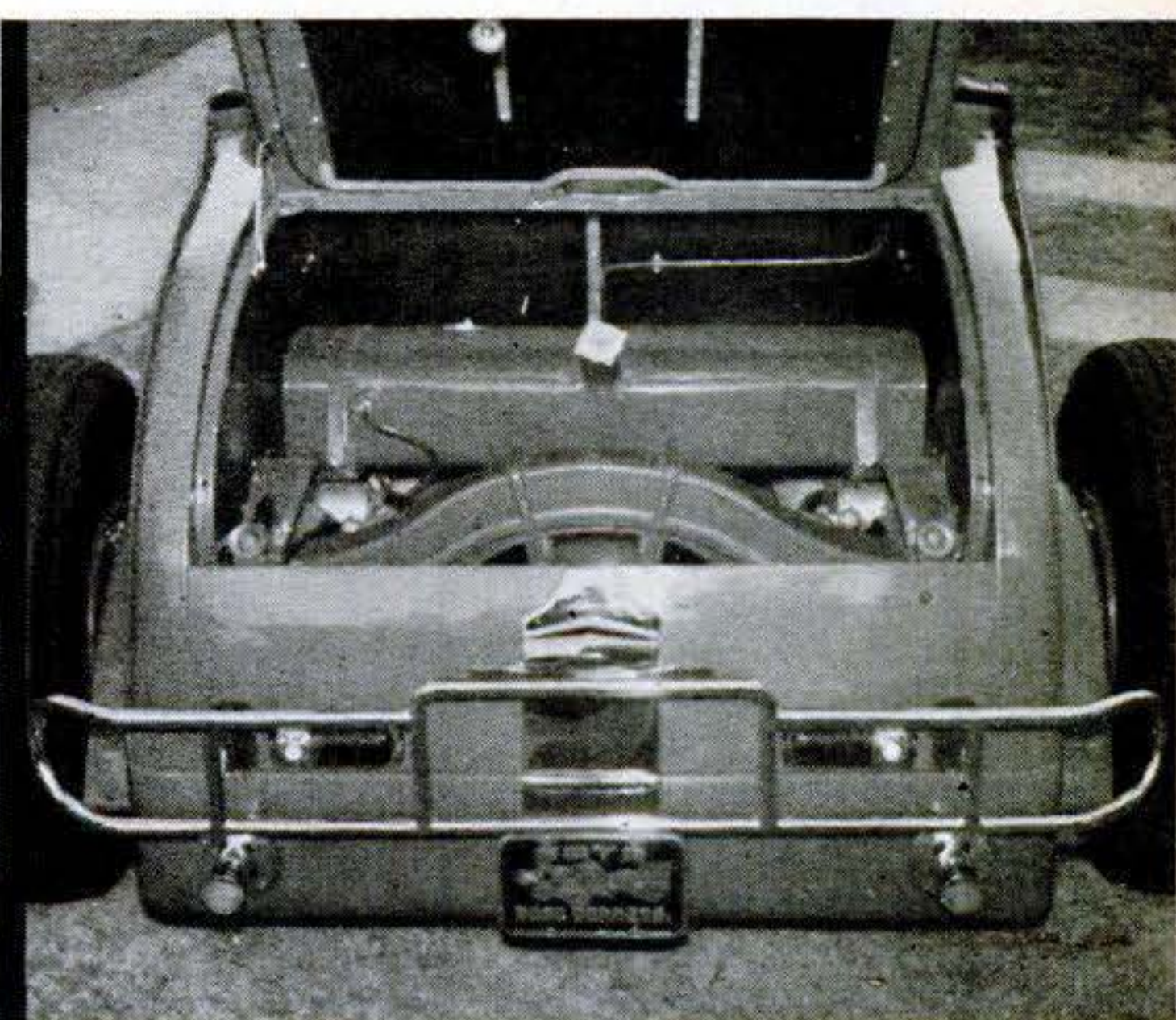
Rear end boasts two sets of shock absorbers, a pair of Houdaille needle-adjusted Fords and two tube-type Gabriels mounted at 45° angle to control body sway. Gas tank is '28 Chevy.
