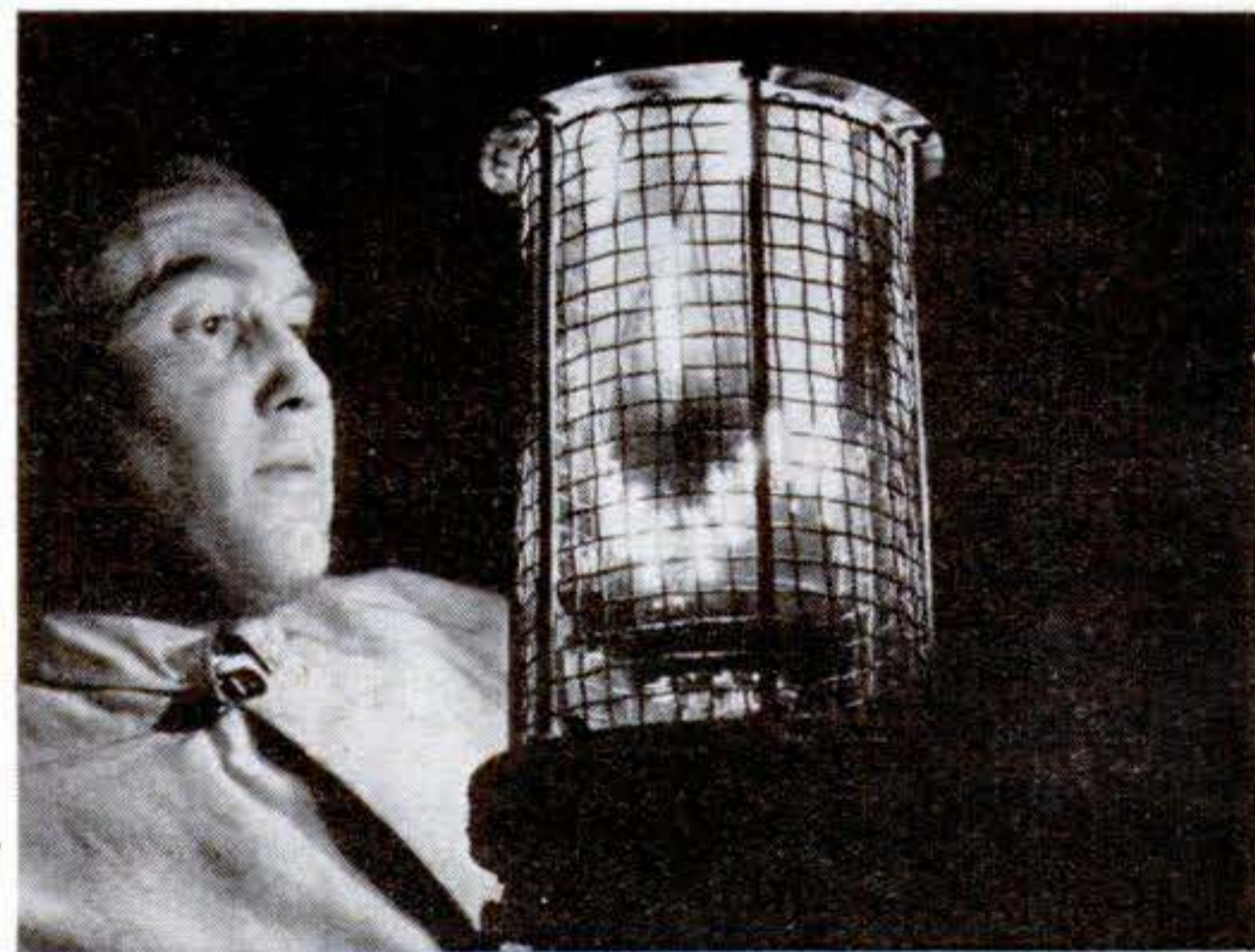
Within this quartz jacket , gas-turbine combustion is under study. Boeing engineer observes how and where burning occurs. Research is resulting in lower fuel consumption, higher power.
