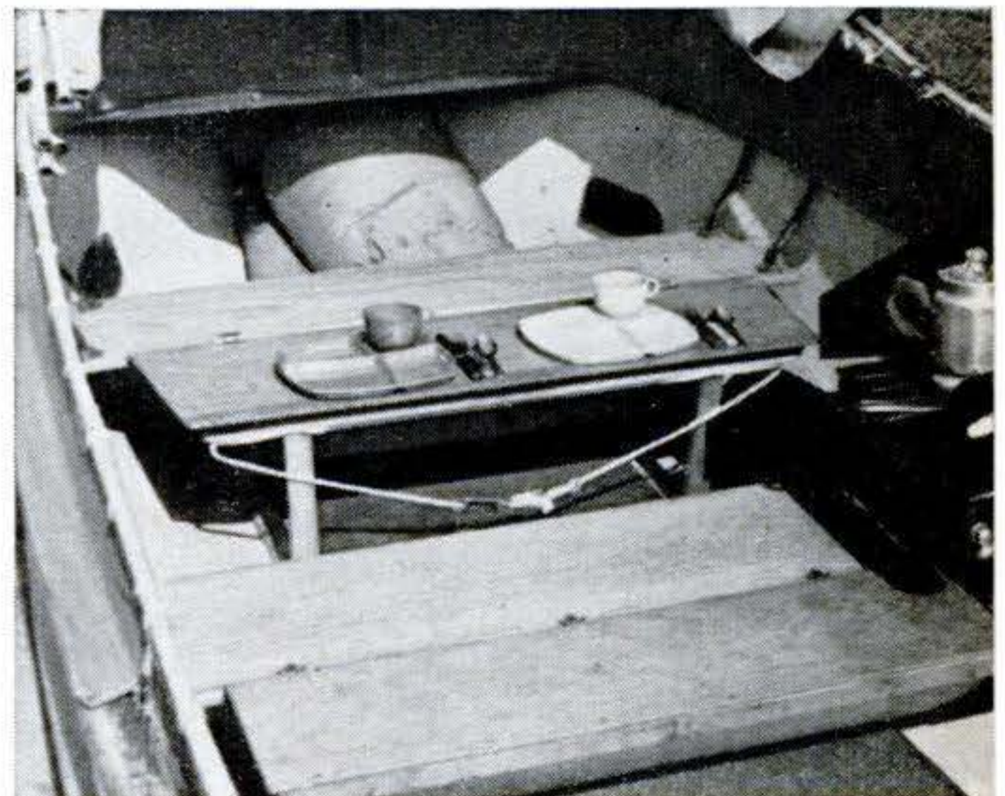
Legs hinged to top ribs of head and footrest convert them to tables for cooking and eating aboard. Bed roll is stowed forward.
