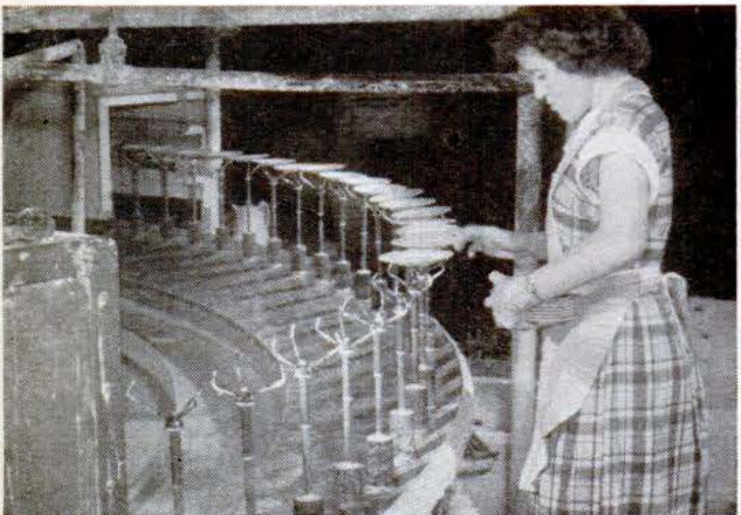
20 Machine glazing. Some pieces can be machine glazed. Dishes are rotated automatically while battery of spray guns spreads on the liquid glaze. This glaze also is fired.
