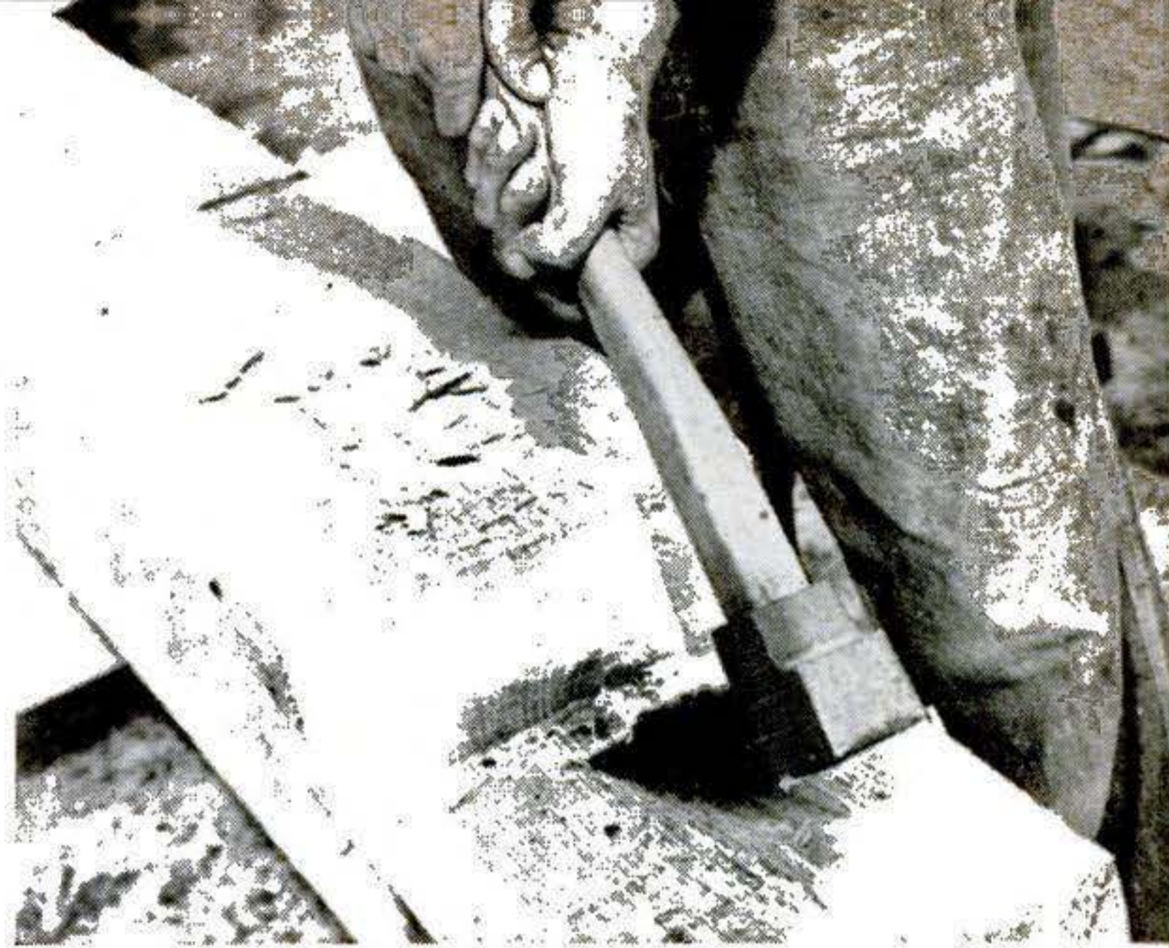
In the hands of an expert, the adze is a versatile tool, and can cut a chip the size of a man's fist, or slice a shaving as thin as paper. Cutting blade must be kept razor sharp.
