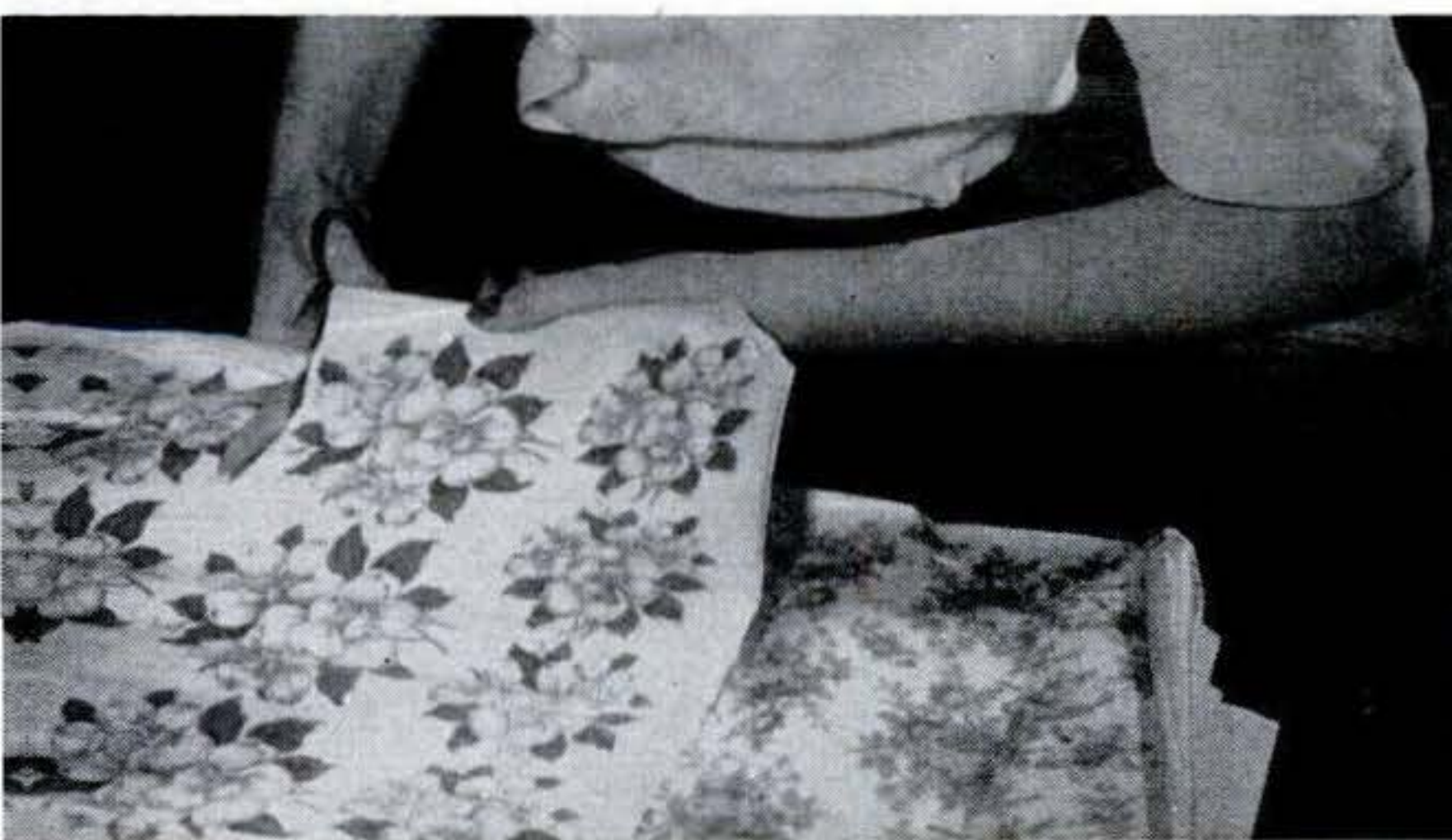
22 Overglaze decoration. Decorations using metallic oxides that cannot stand high temperatures are applied over the glaze and fired separately. Decalcomanias do the trick.
