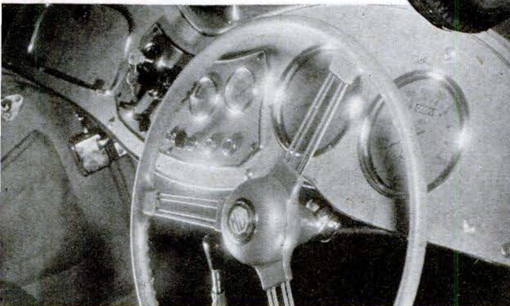
Telescoping steering wheel , shown retracted above and extended at right, permits tailoring car to driver. Car, shown here with right-hand drive, is now available with left-hand drive.
