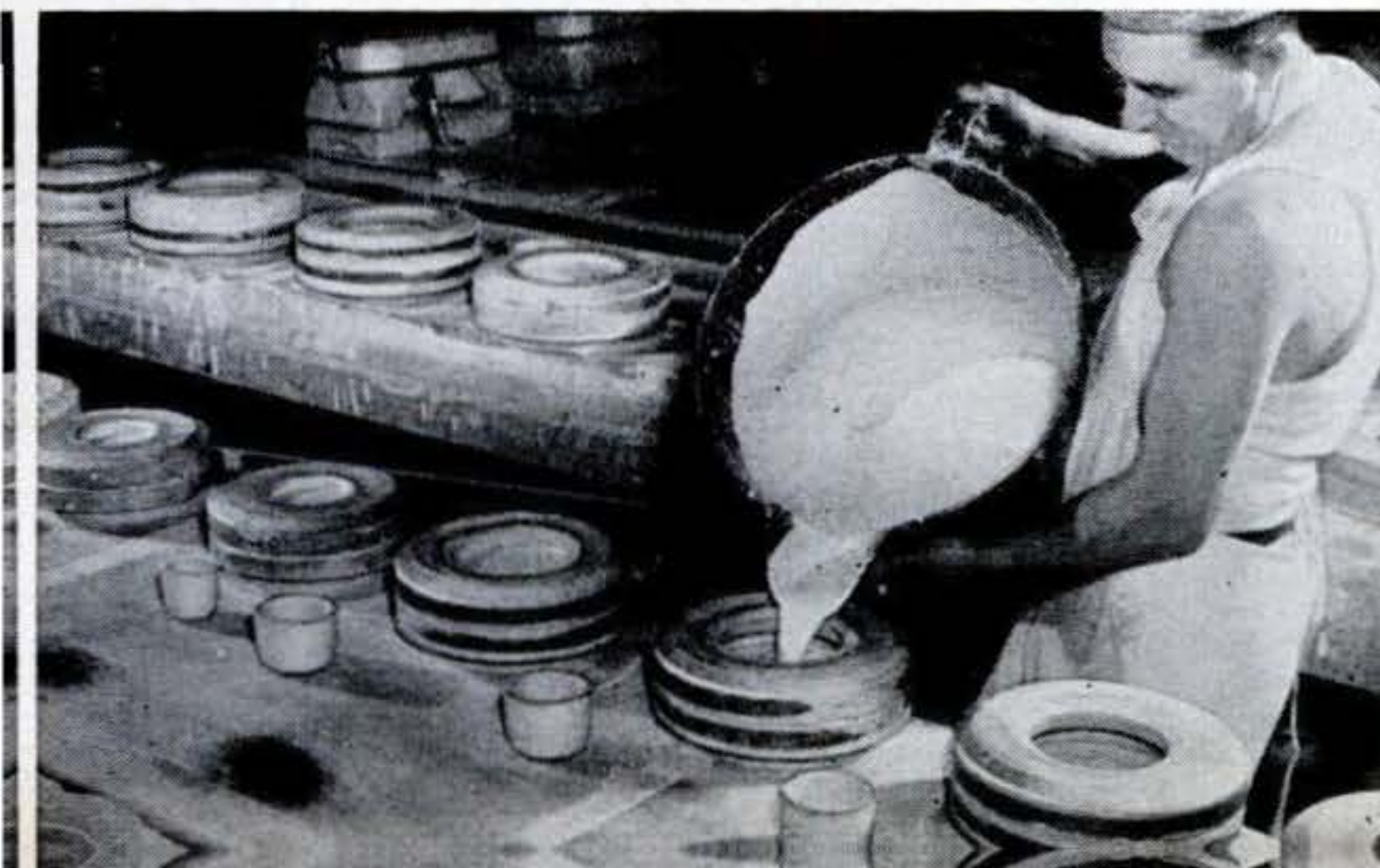
10 Molds used in jiggering and casting have comparatively short lives. As a result, the casting of replacement molds in plaster-of-Paris master molds keeps the molders busy.
