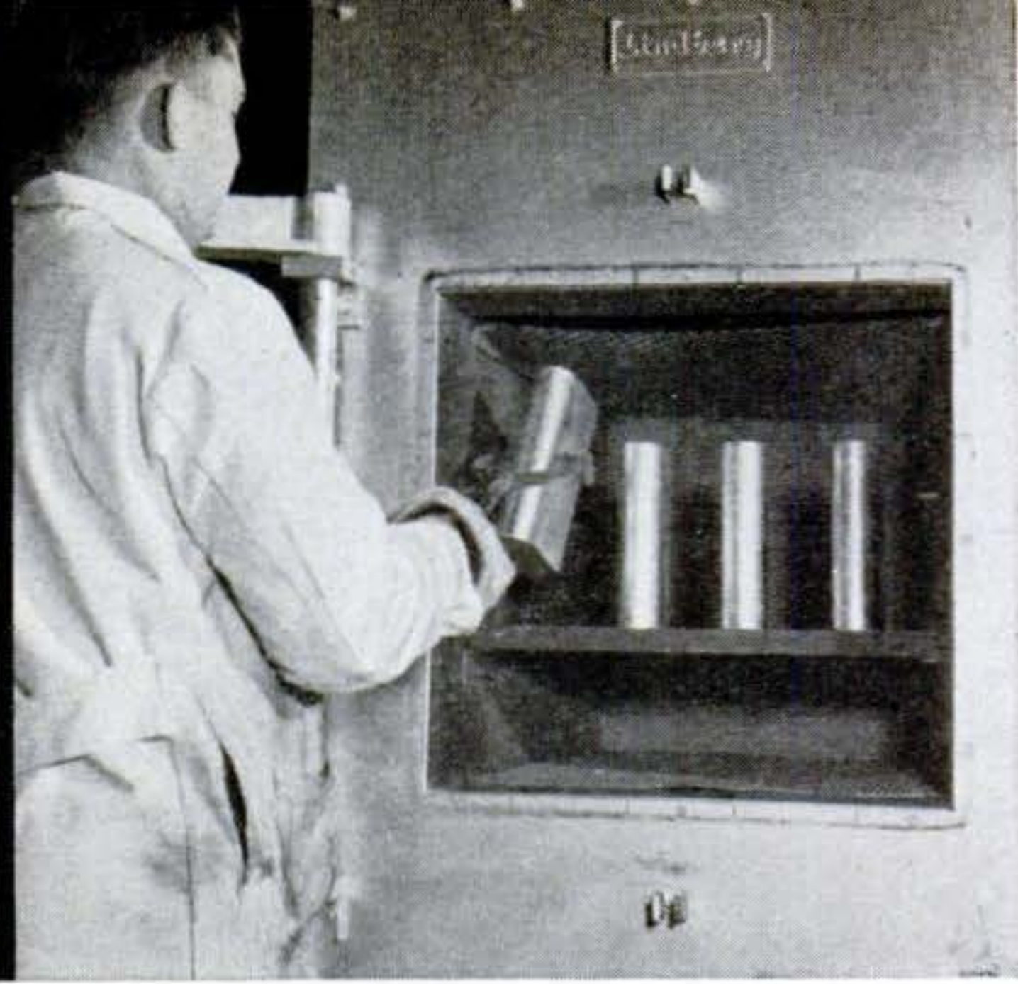
2 After a 23-lb. ingot is removed from its book-shaped mold, it is placed in an electric furnace with other ingots for a heat-soaking treatment to bring them to rolling temperature.
