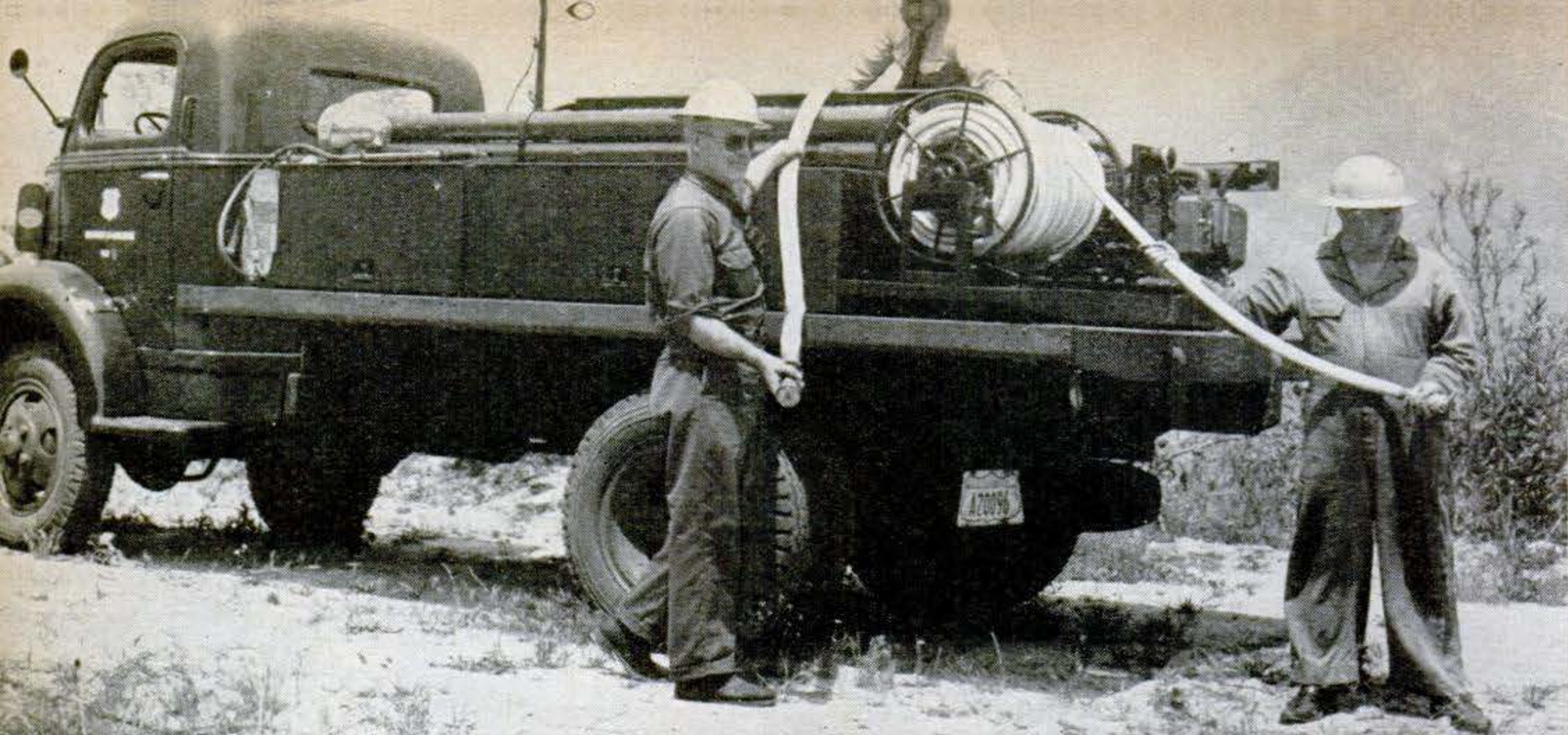
Standard Ford 1½-ton truck is converted to fire fighting by bolting slip-on unit to truck bed. Only other connection between pumper unit and truck is siren cable. Pump units can be changed
