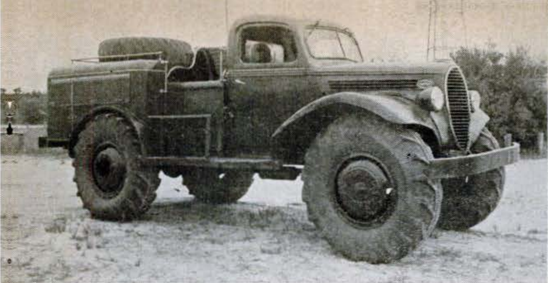
For Florida swamp fires, Forest Service uses this high-wheeled marsh buggy. It has water tank, hose, hand tools, and seats for fire fighters.
