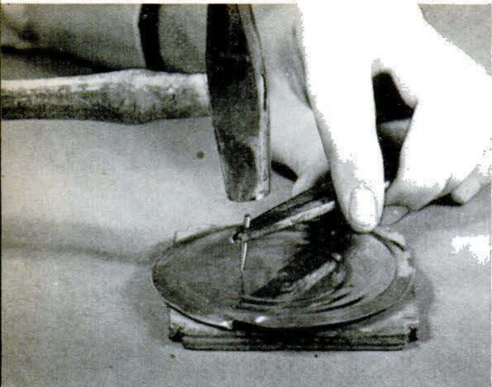
Gas orifice is punched with a sharp phonograph needle in tin-can stock or sheet brass.
