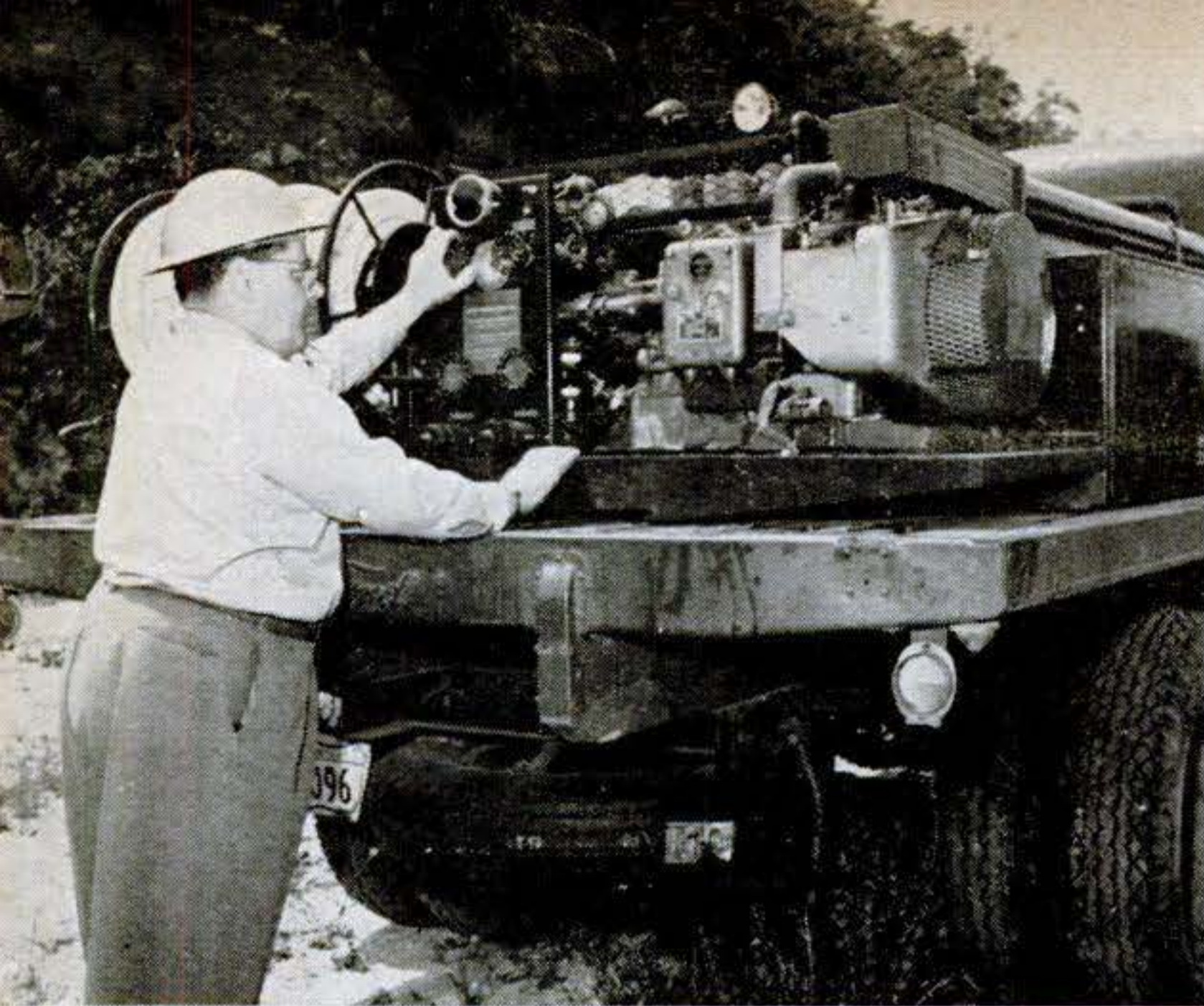
Close-up shows 10-hp. pumper unit mounted on 1½-ton truck. It delivers 30 gallons of water per minute from 300-gal. tank at 250-lb. pressure. Pair of 6-volt batteries furnish juice.
