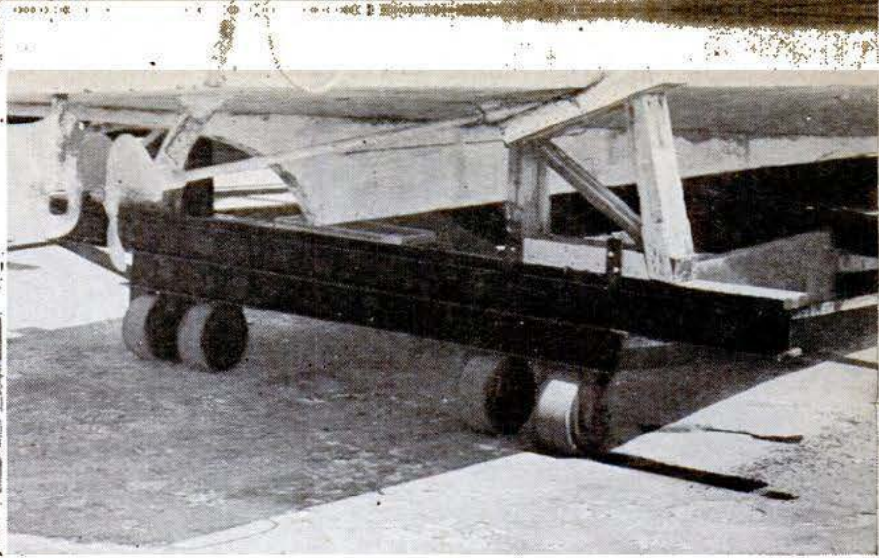
Close-up view shows how boat rests on steel dolly, braced by sliding chocks. This end of dolly has wheels. Other end has stumpy legs, lifted from ground when tractor tows dolly.
