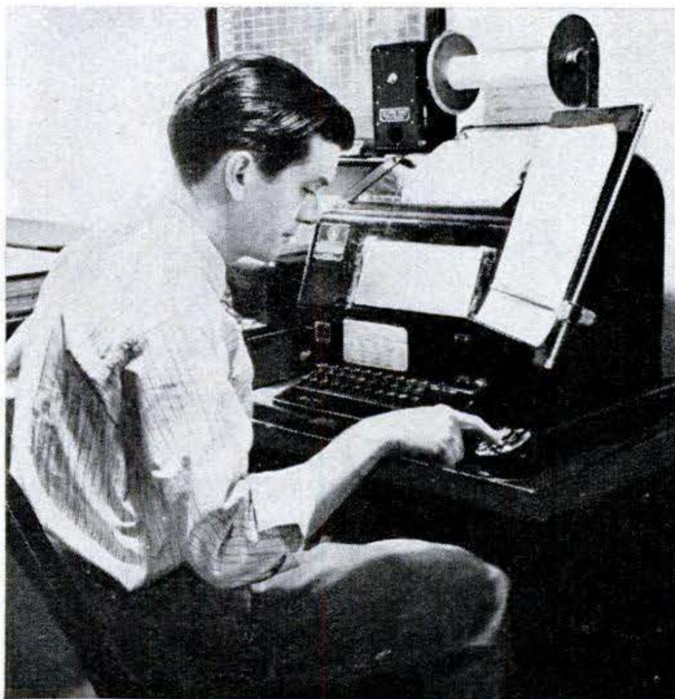
Dispatcher in home office skyscraper uses this dial system to transmit orders and get information at stations in New Douglas, Effingham, and Dennison, Ill., and North Salem, Ind.
