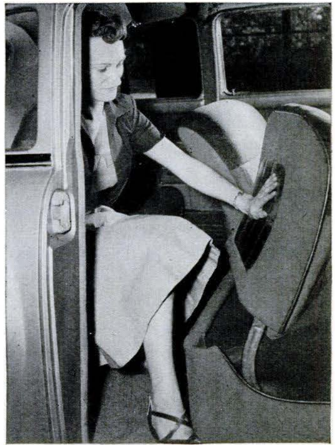
Ample entryway is provided for rear-seat passengers in two-door sedans. Body paneling is Fibreglas-padded to reduce road noise. Except in "200" series, seat cushions are foam rubber.
