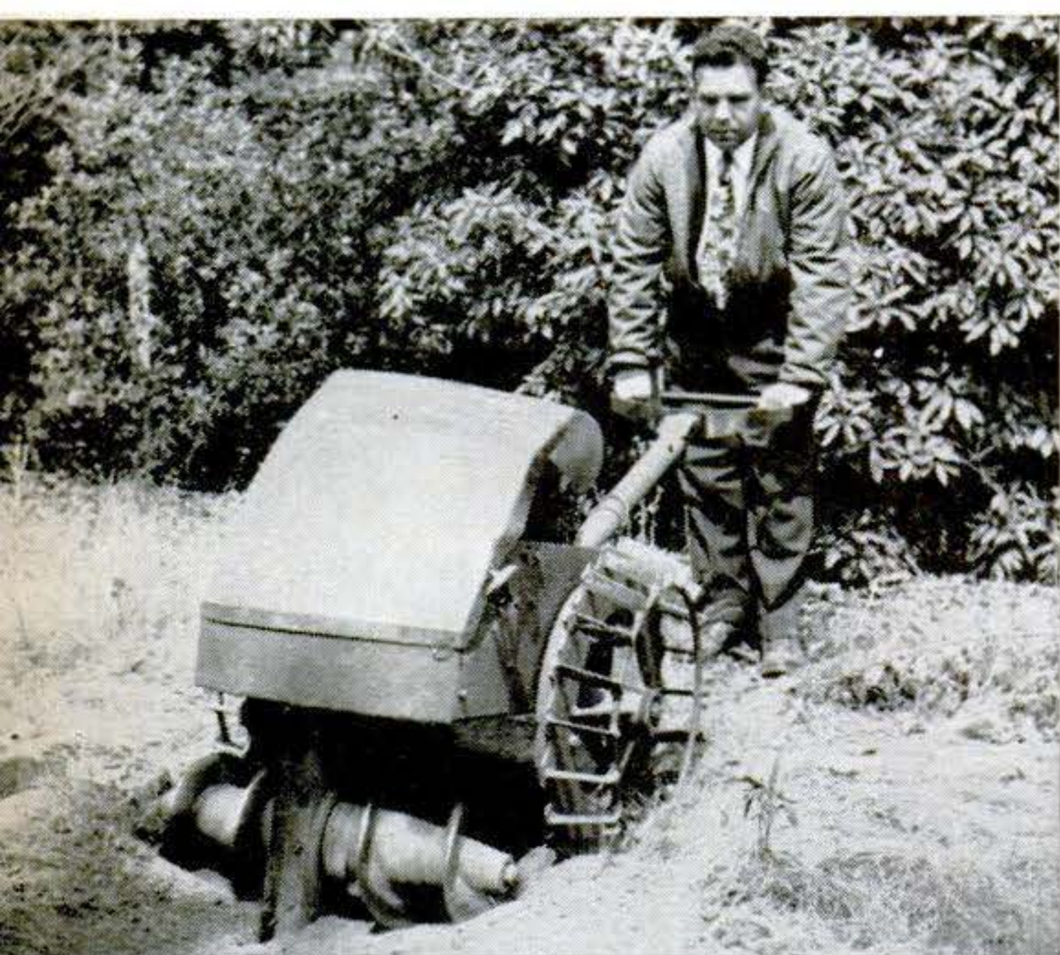
Rotary trencher is cross between plow and baby bulldozer. Opposed spirals peel off thin layers of soil and build ridges on each side. Machine cuts 18-in. trail at a walking pace.
