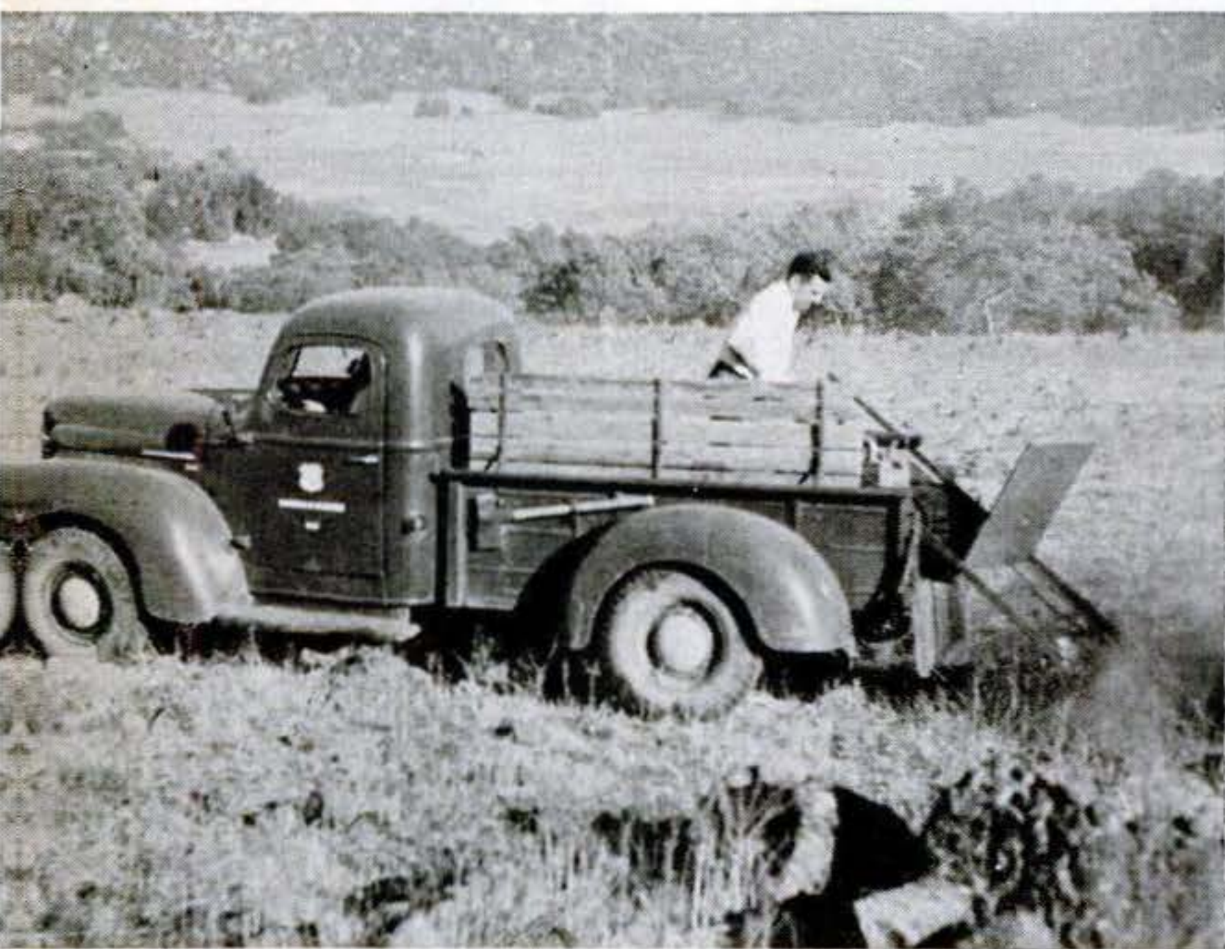
Clearing mine fields in wartime suggested development of this flail. It's used in Western lava beds where cover, though scanty, spreads a fire.
