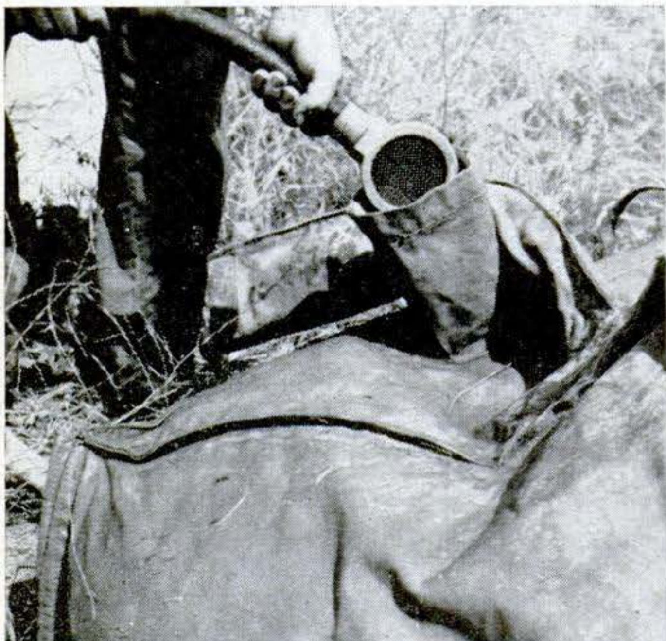
Any water remaining in tank after use is sucked through strainer back into pumper truck's tanks. Strainer is also used when drawing water from lake or stream, prevents clogging of hose.
