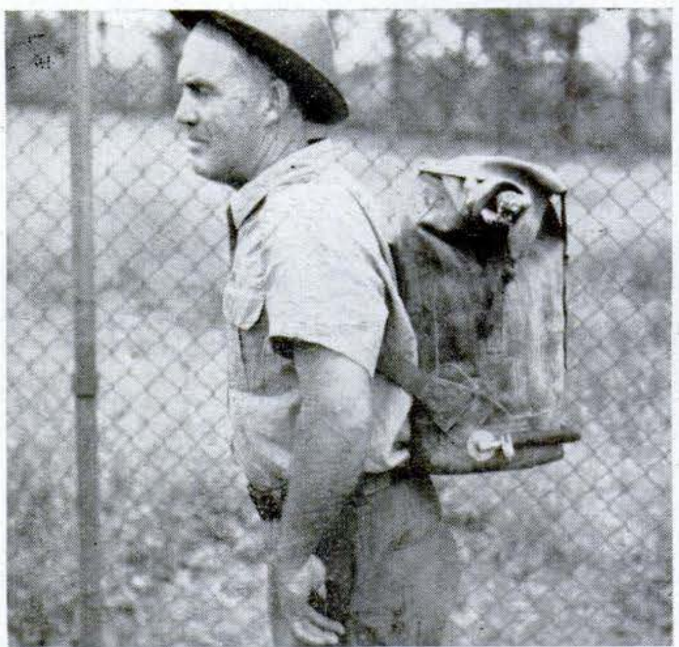
Forest Service engineers are constantly looking for new fire-fighting tools. This experimental model is a collapsible rubber back-pack bag that carries five gallons of water plus hand pump.
