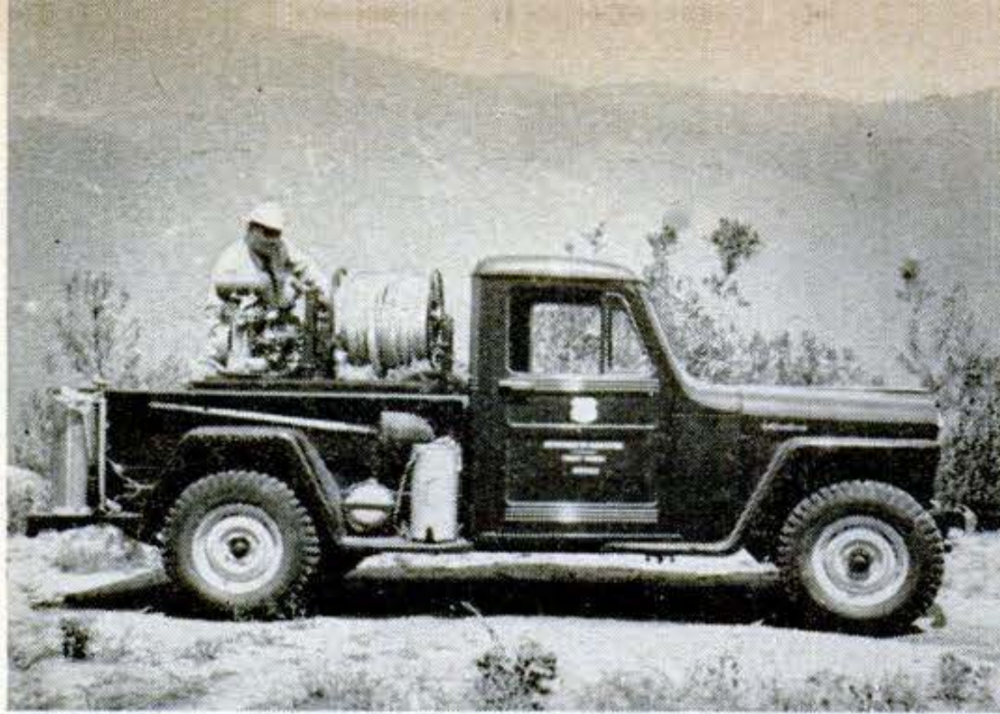
One-ton Willys carries 160 gal. of water in three compartments. Single-cylinder, four-cycle engine develops six hp., pumps 18 gal. per minute at 250-lb. pressure.
