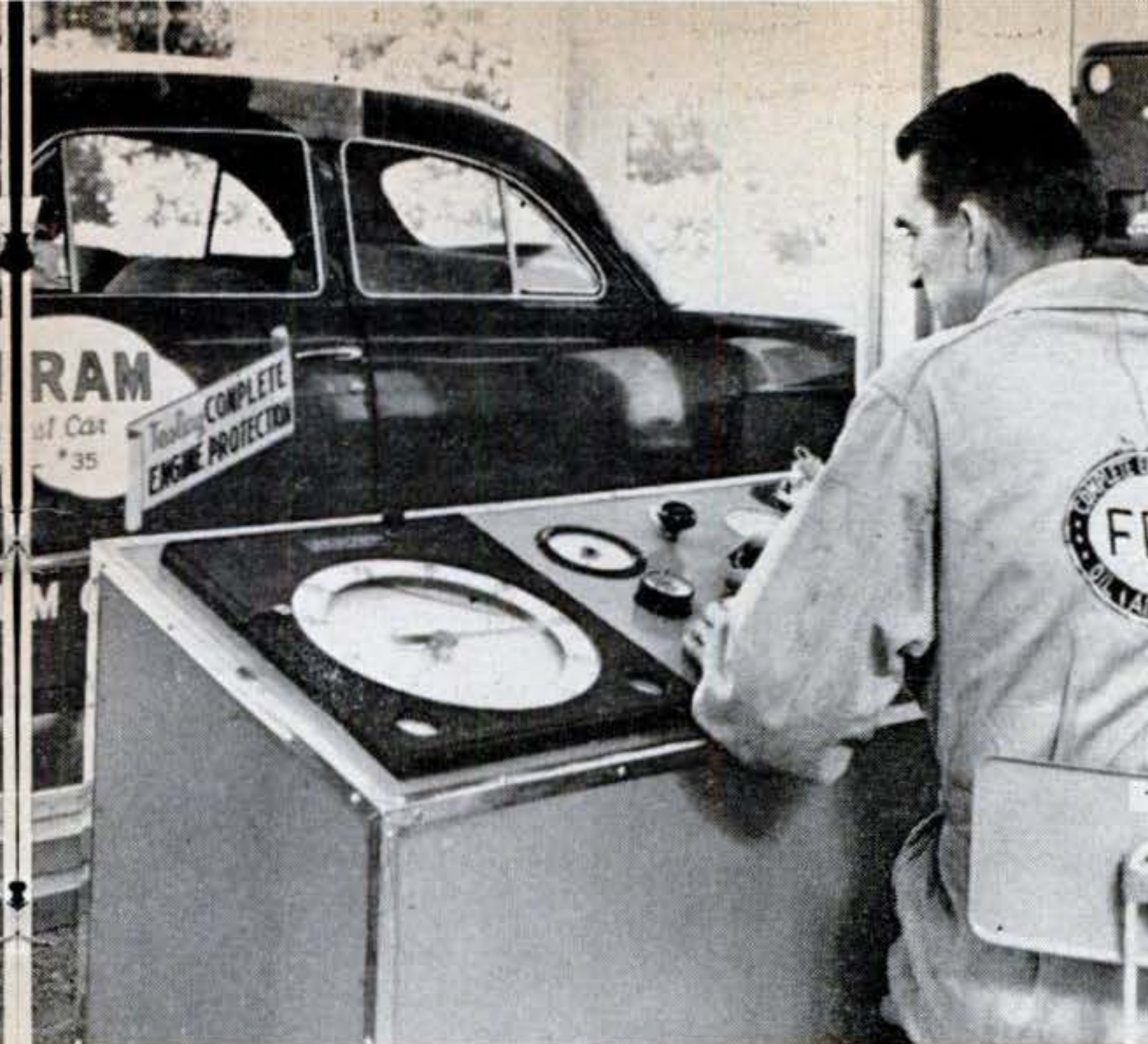
Throttle, ignition controls are "remoted" to laboratory panel that supplies progressive data on car. Ford is equipped with racing-type tires. Rollers wore out regular tires too fast.
