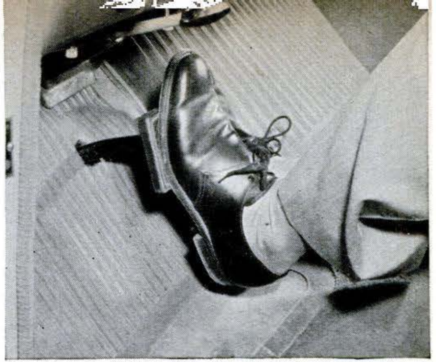
By moving brake pedal to the left , designers make it available to either right or left foot. Wilbur Shaw commented, "With practice, the left foot is bound to become the braking foot."
