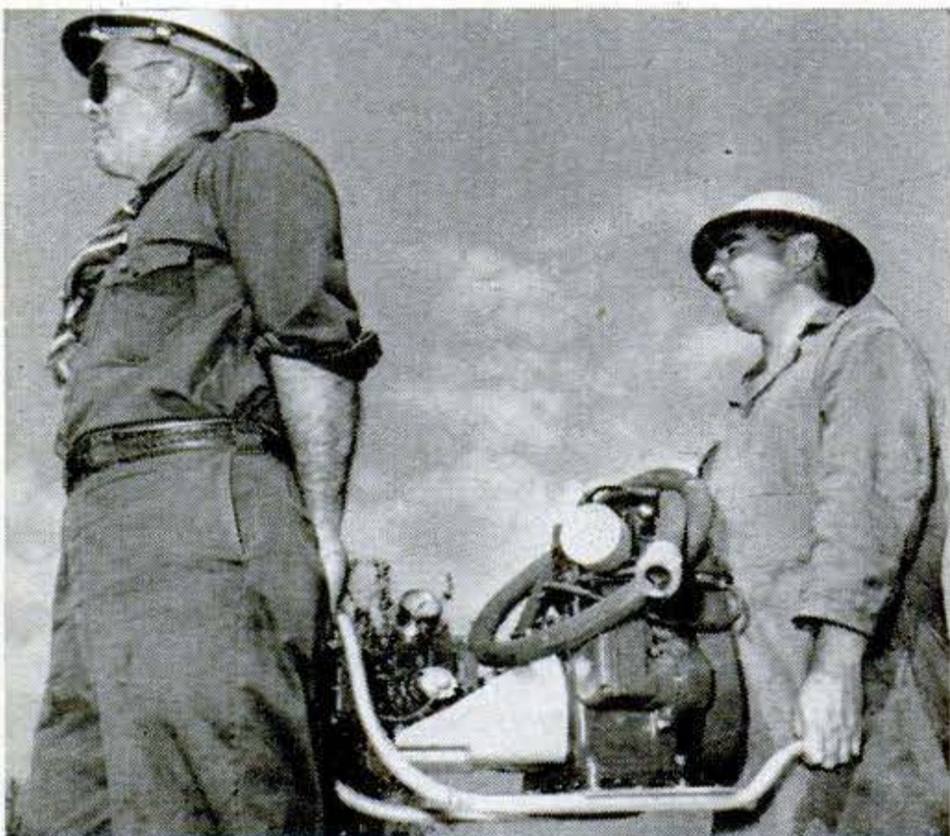
When no other power is available, small one-cylinder engine mounted on skids can pump from stream or act as booster on long hose line. Two men can easily carry the 94-lb., 6-hp. outfit.
