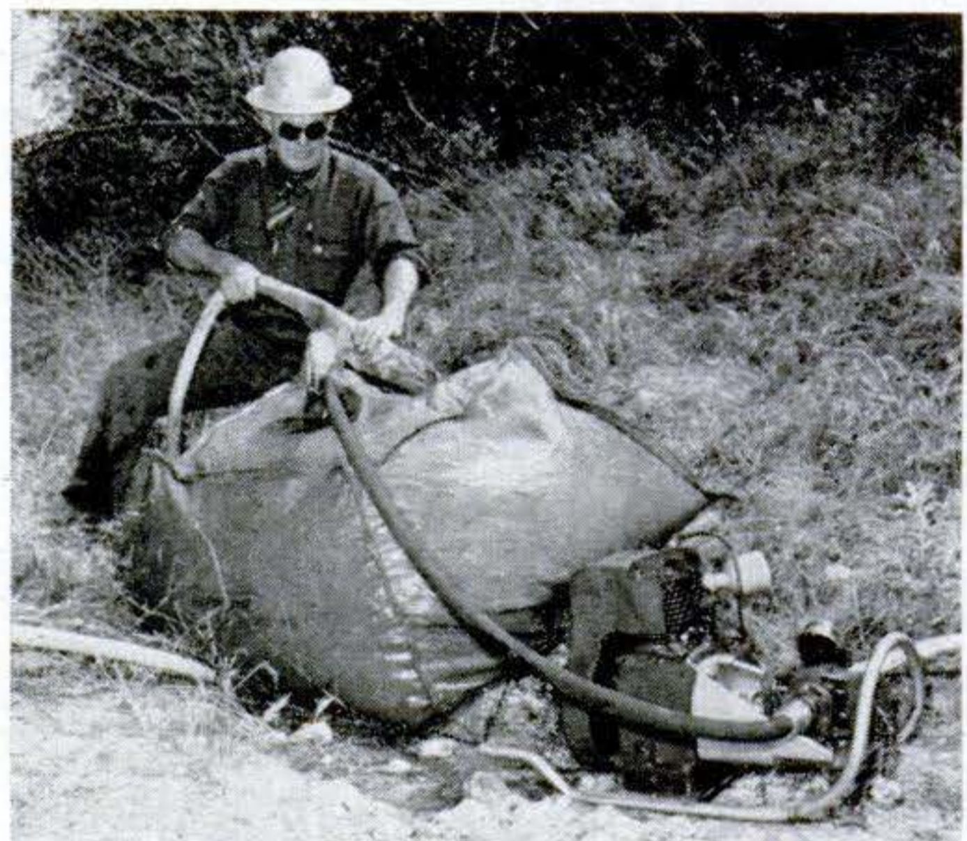
Auxiliary canvas tanks are being tried by Forest Service in three sizes—150, 300, and 600 gal. This is 300-gal. tank, treated for mildew. Tank hugs ground, can be used on hills.
