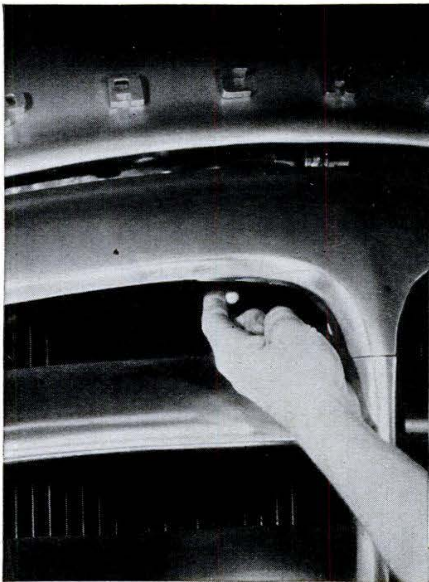
Hood-release lever on the '51 Packard is inside grille because of breakage trouble with cable from driving compartment. It sacrifices engine-compartment theft protection, however.
