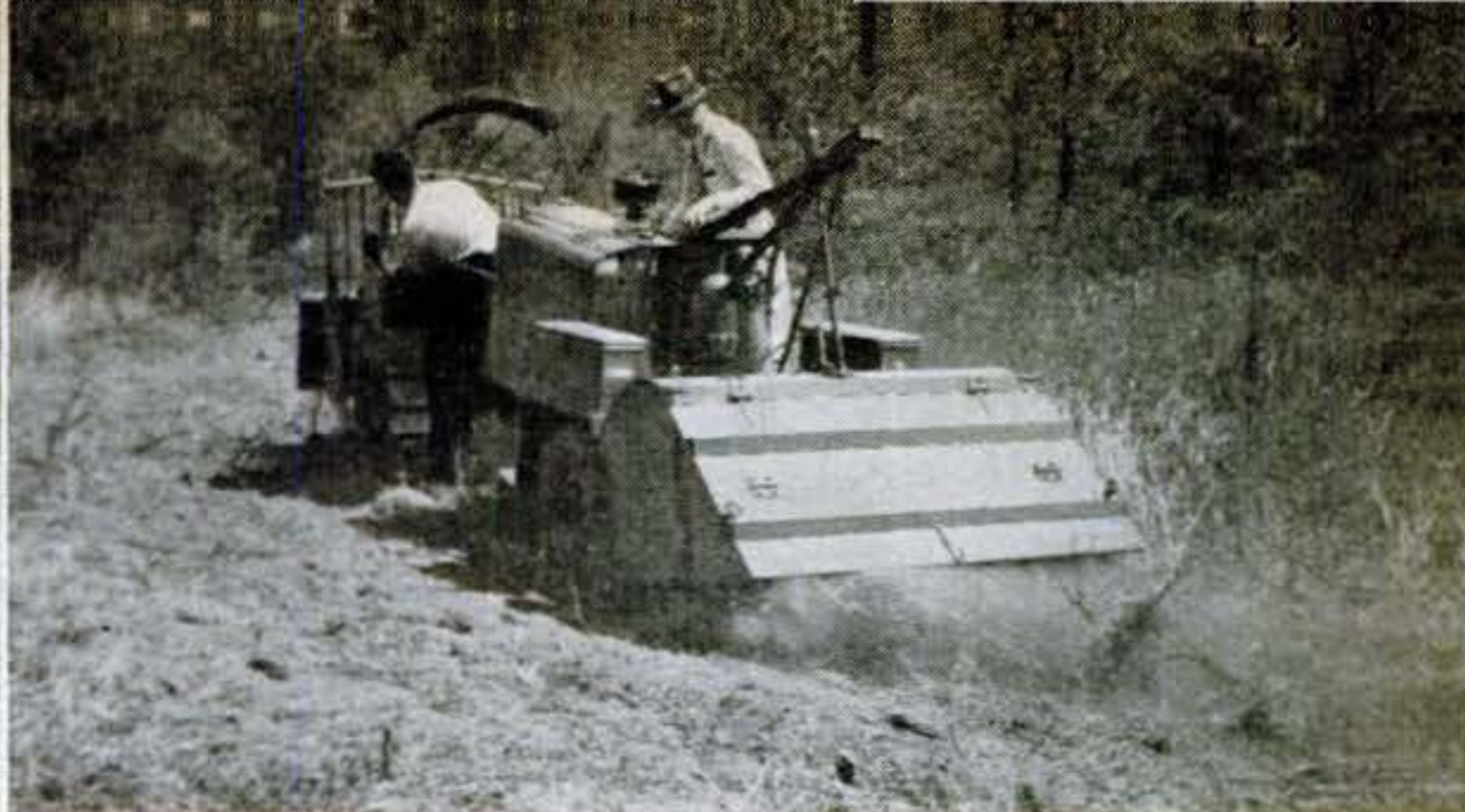
"Pulvimixer" has four-foot rotor with curved blades that break up and bury surface growth and litter. Pulled by tractor, it goes 2-3 m.p.h.
