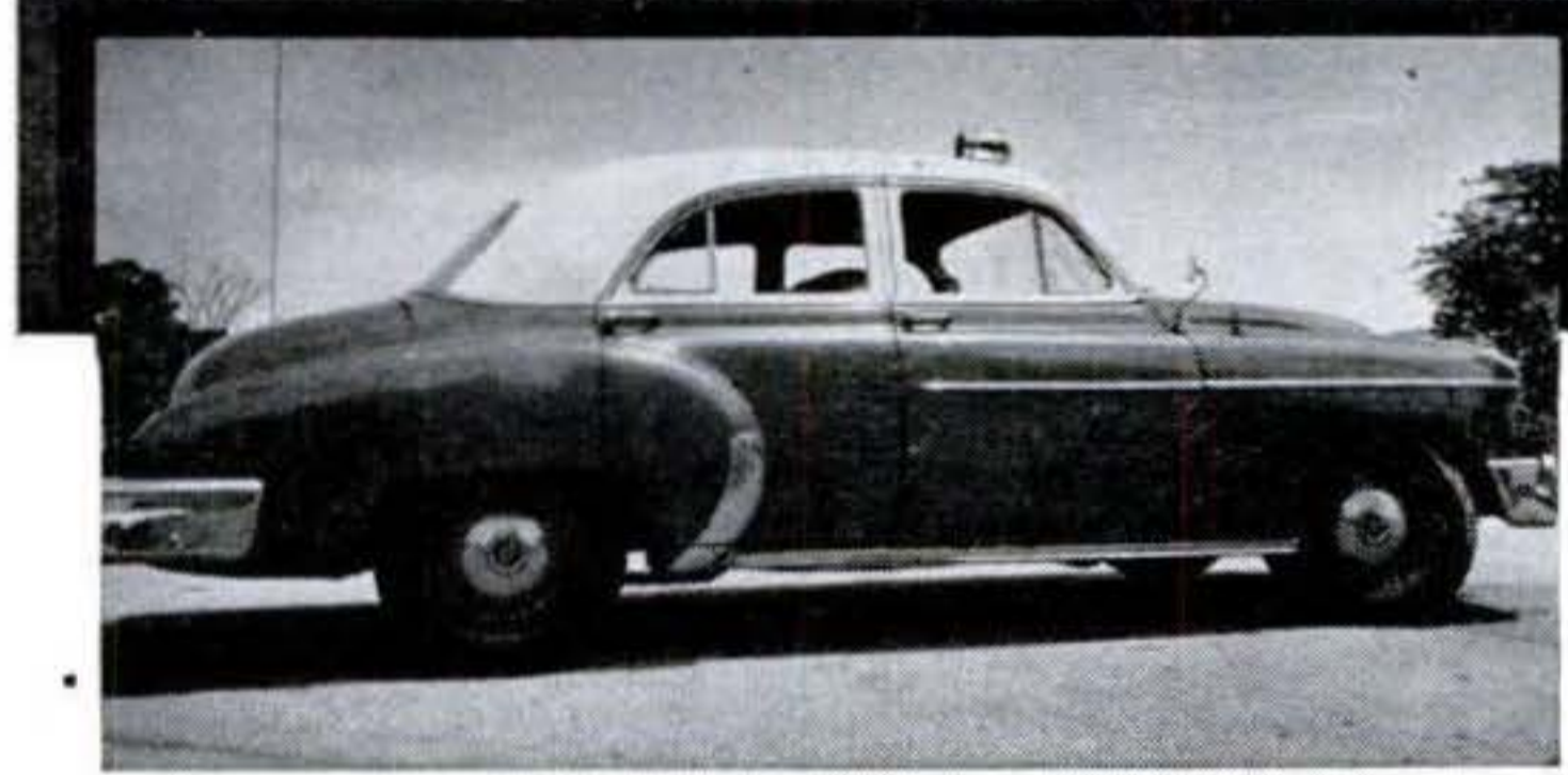
Two-minute conversion turns car into ambulance. Inventor, at wheel, gets instructions over radio telephone. Note oxygen tank near dash. At left, roof spotlight and whip antenna are only hint of car's double purpose.
