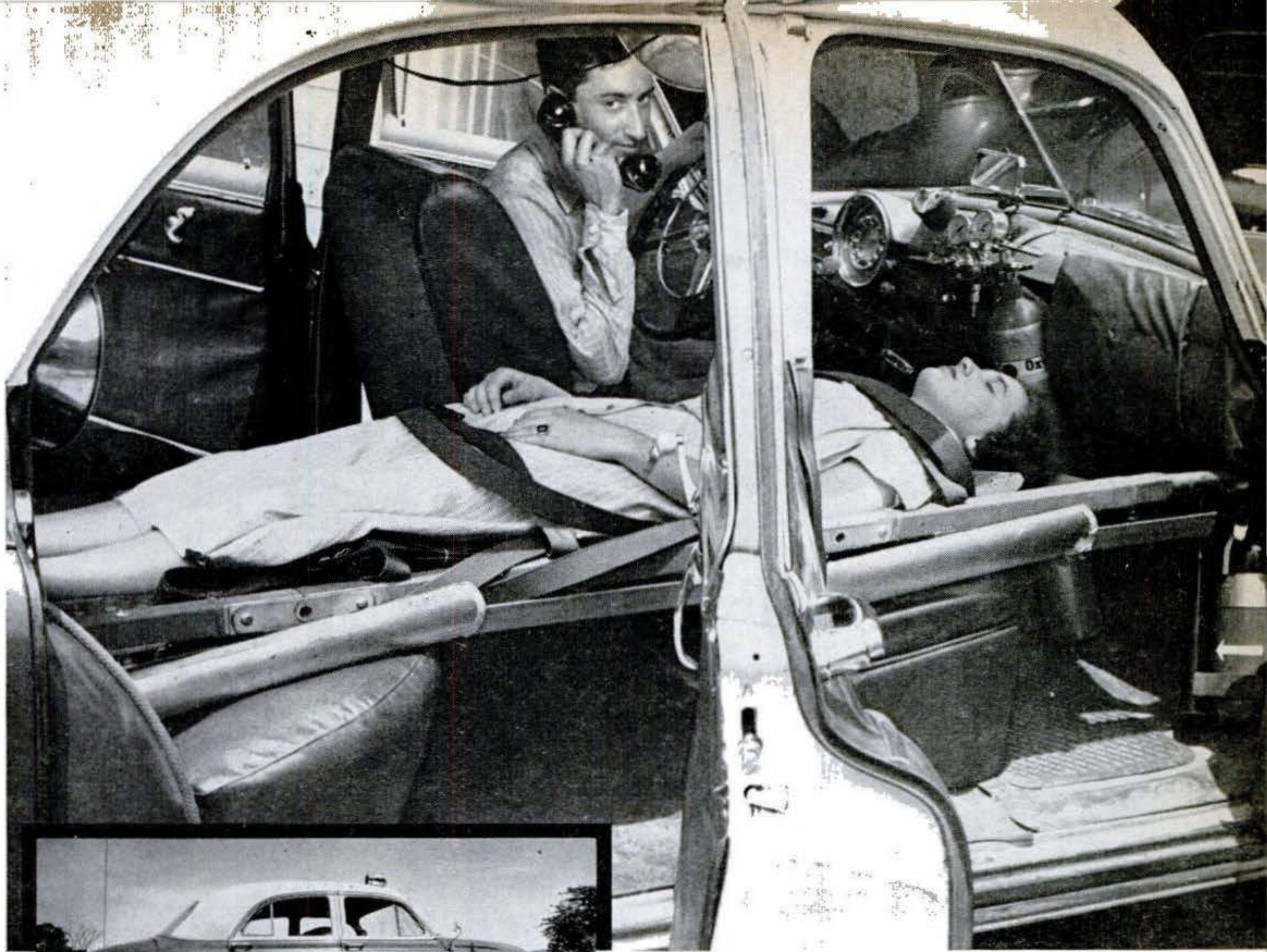
Two-minute conversion turns car into ambulance. Inventor, at wheel, gets instructions over radio telephone. Note oxygen tank near dash. At left, roof spotlight and whip antenna are only hint of car's double purpose.
