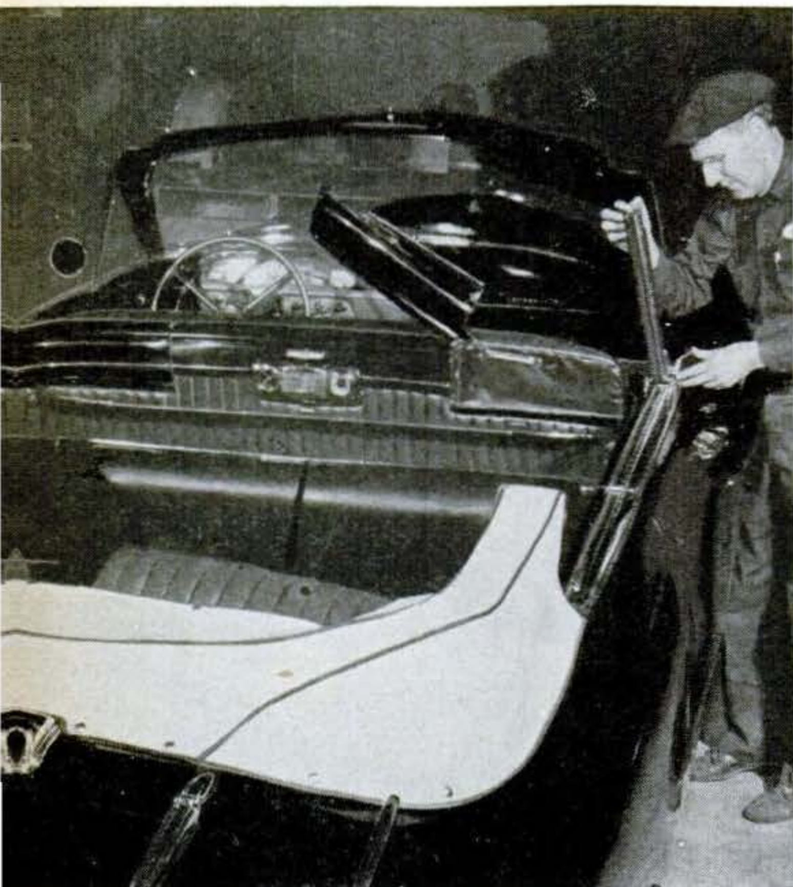
Pillar support for convertible's top folds sideways into partition and then is covered by hinged cap. Convertible is only one of the 10 cars without an extra radio for rear-seat passengers.
