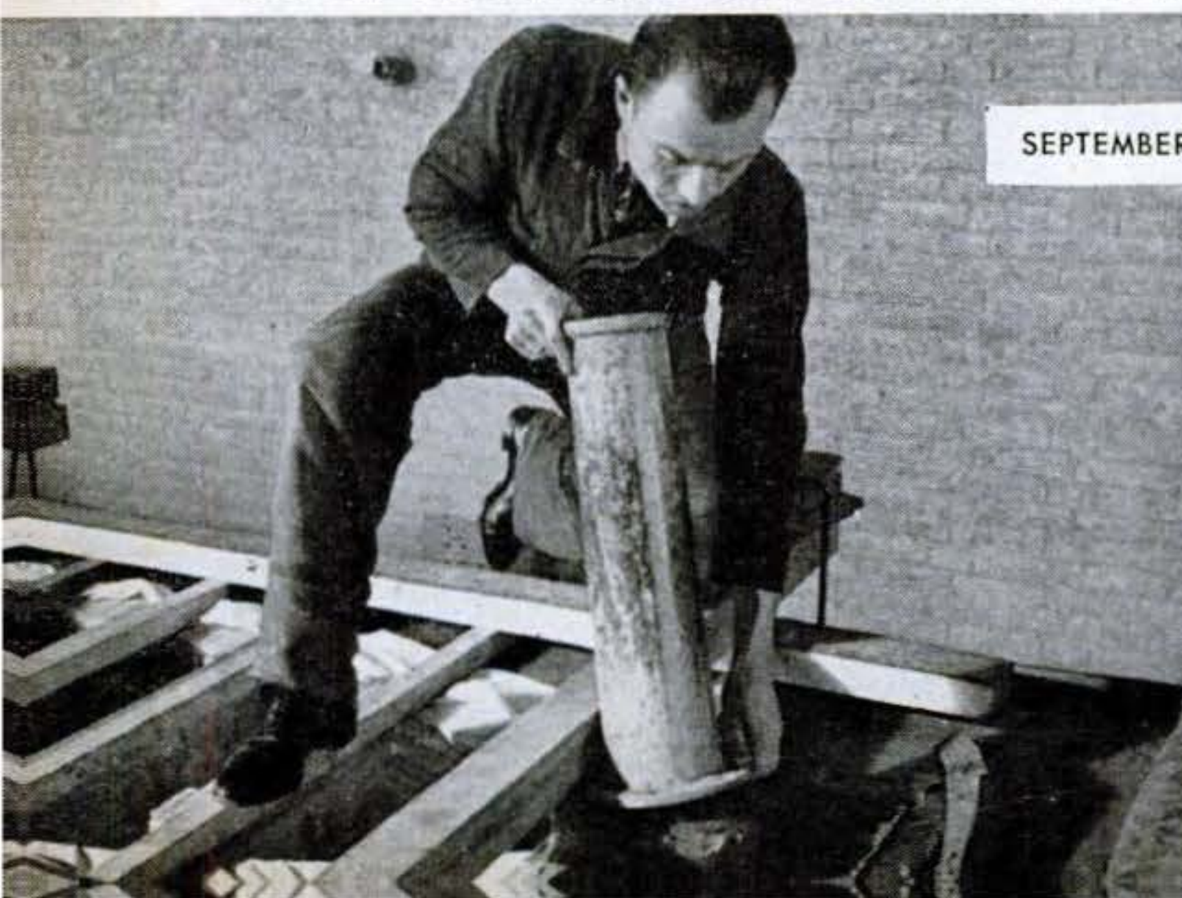
5 AN AIR VENT is placed at front of gap between molds. This permits the escape of air that will be displaced as molten paraffin flows into the narrow space from the opposite end.
