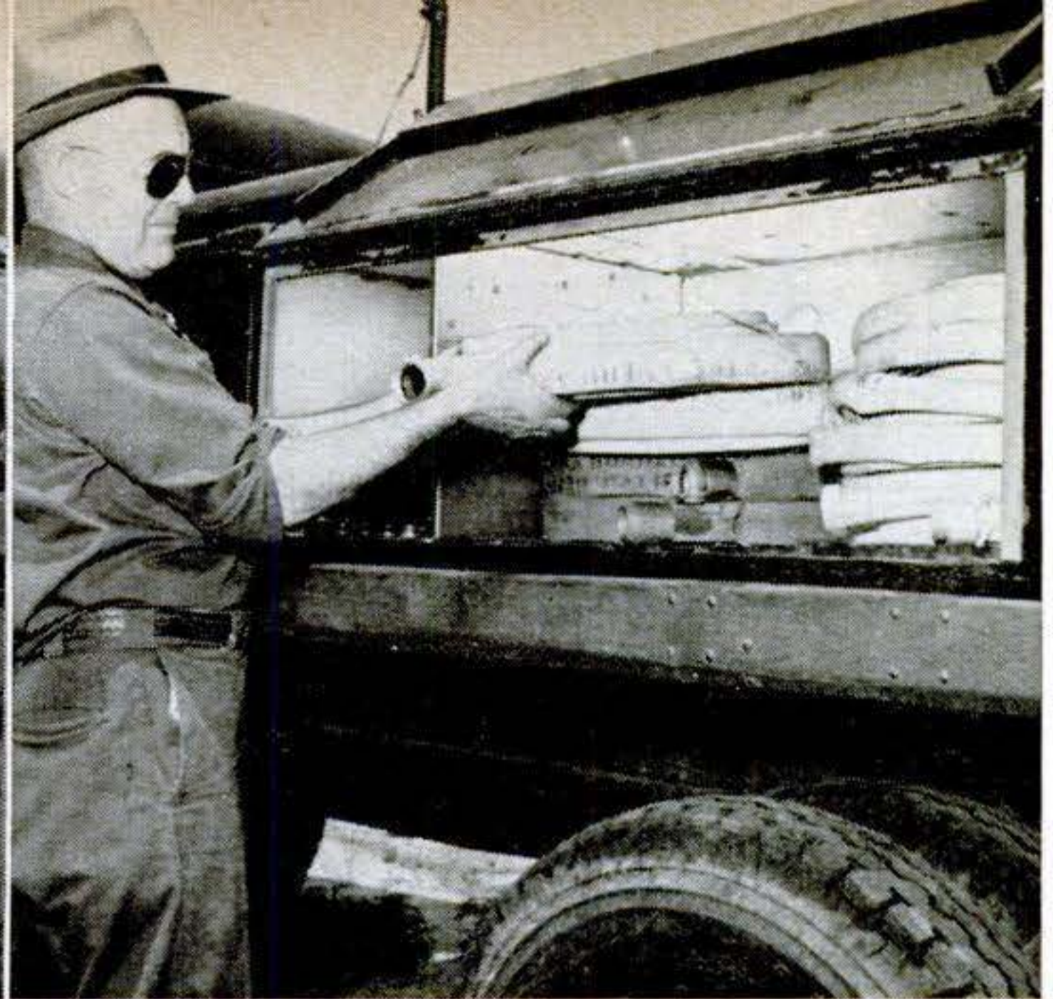
Extra lengths of hose are neatly stowed in lockers on side. Similar compartment carries hand tools, including axes, shovels, McClouds, Pulaskis, brush hooks, wire cutter, pinch bar.
