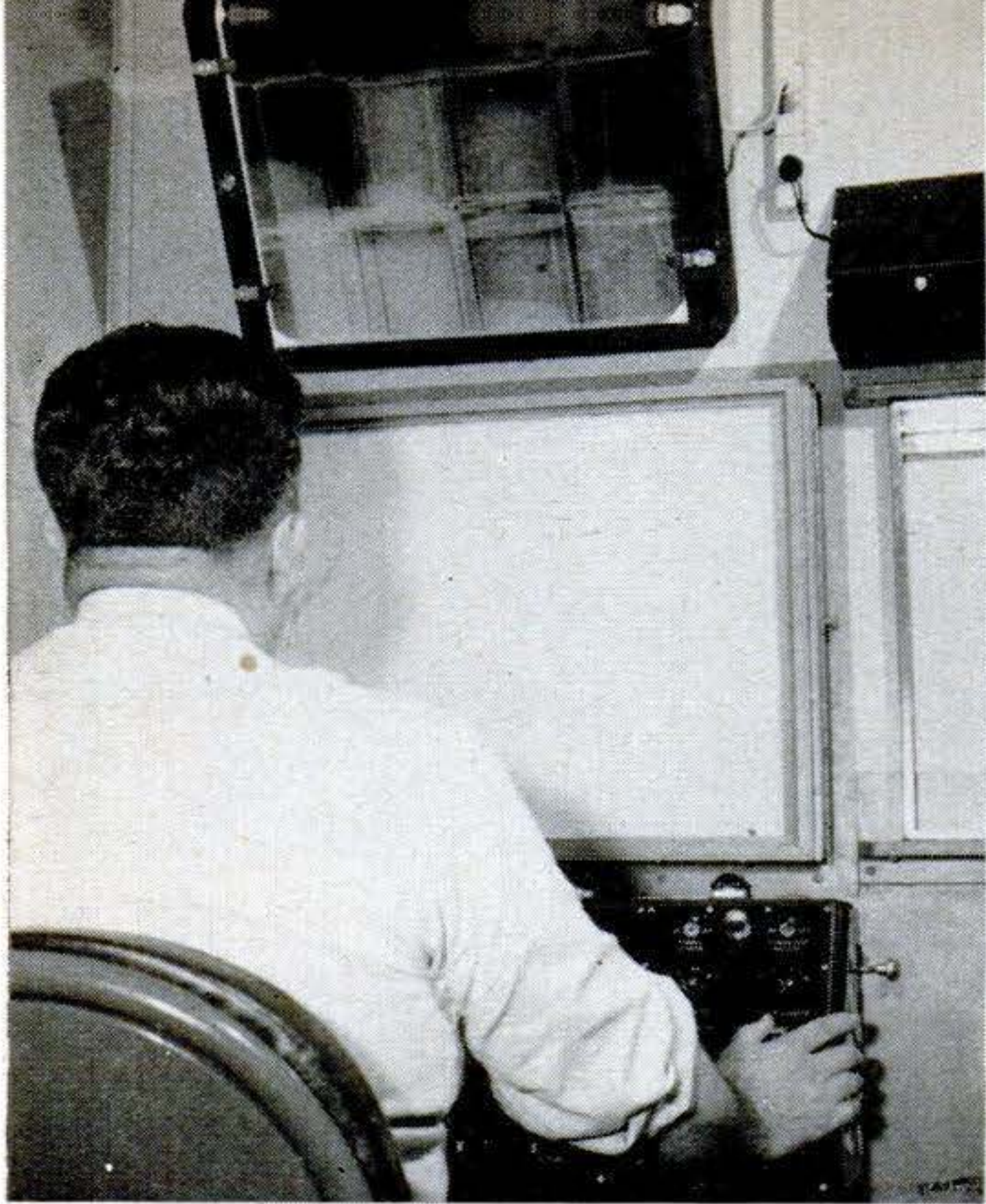
Screen in front of inspector, left, gives him X-ray view of carton of canned goods placed on roller platform, above. To help spot defects, sample film above screen shows typical faults.
