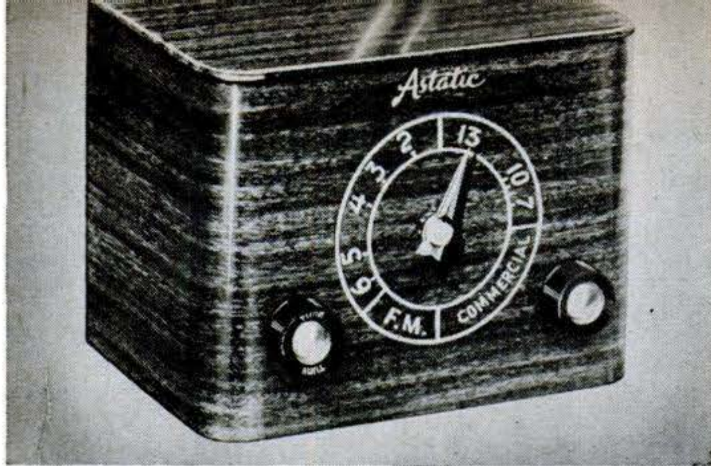
Tunable boosters like this generally give most amplification but must be tuned to match set.
