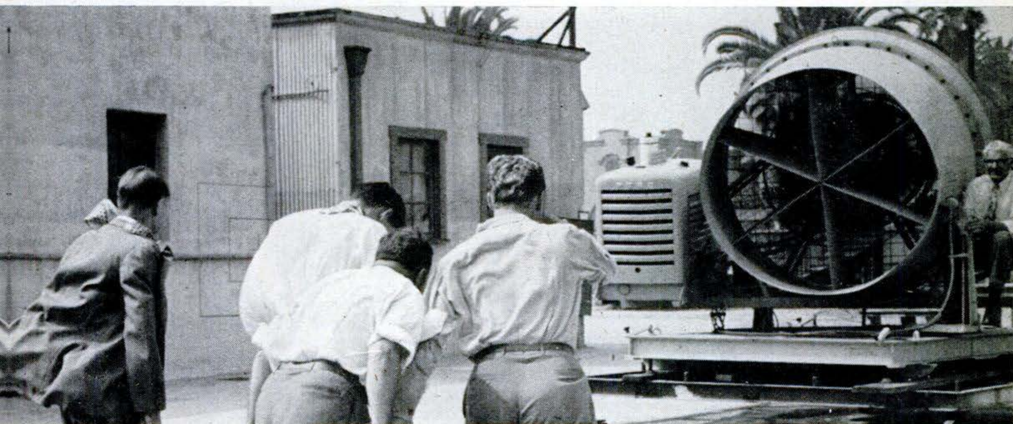
Four men try to buffet gale from new machine that can blow up a 200-mile hurricane. When throttle of its 145-hp. industrial engine is wide
