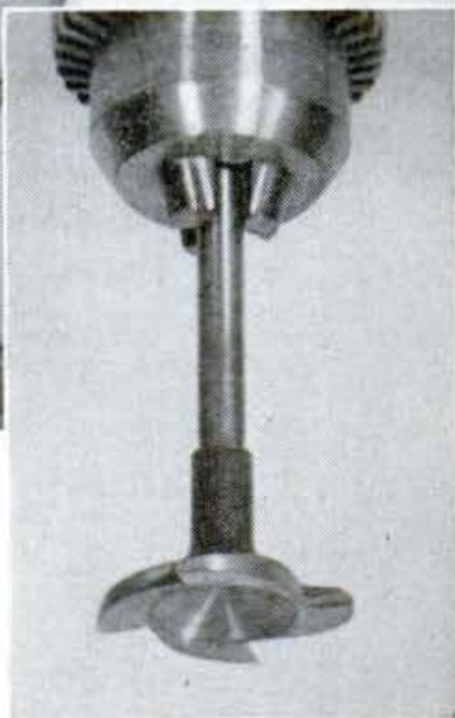
Rotary planer can be made from any valve. One with hollow head provides ready-made chip clearance. Edges must be sharp to rim.
