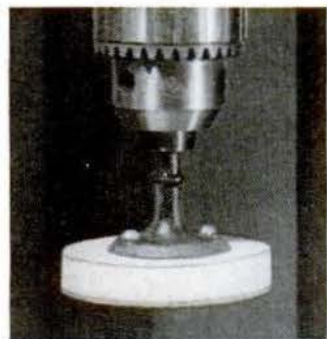
Sander pad snaps onto valve with keyhole slots filed in head. Cement sponge rubber to pad; attach abrasive paper with rubber cement.
