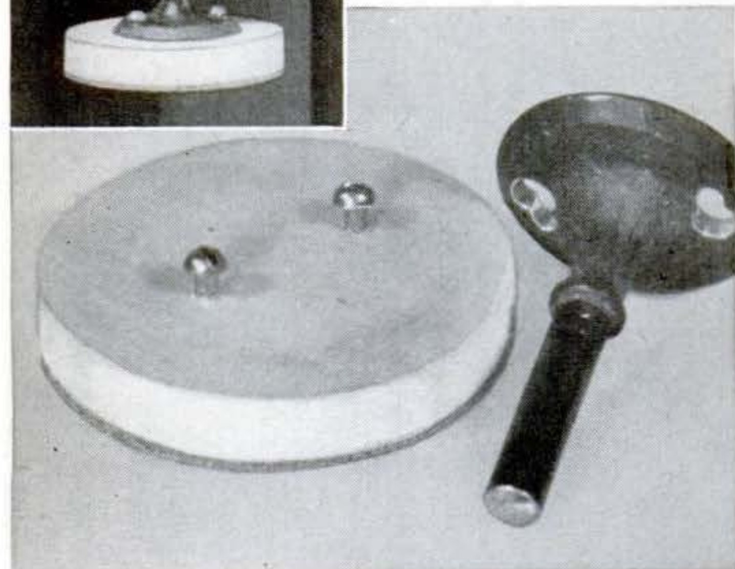
Sander pad snaps onto valve with keyhole slots filed in head. Cement sponge rubber to pad; attach abrasive paper with rubber cement.
