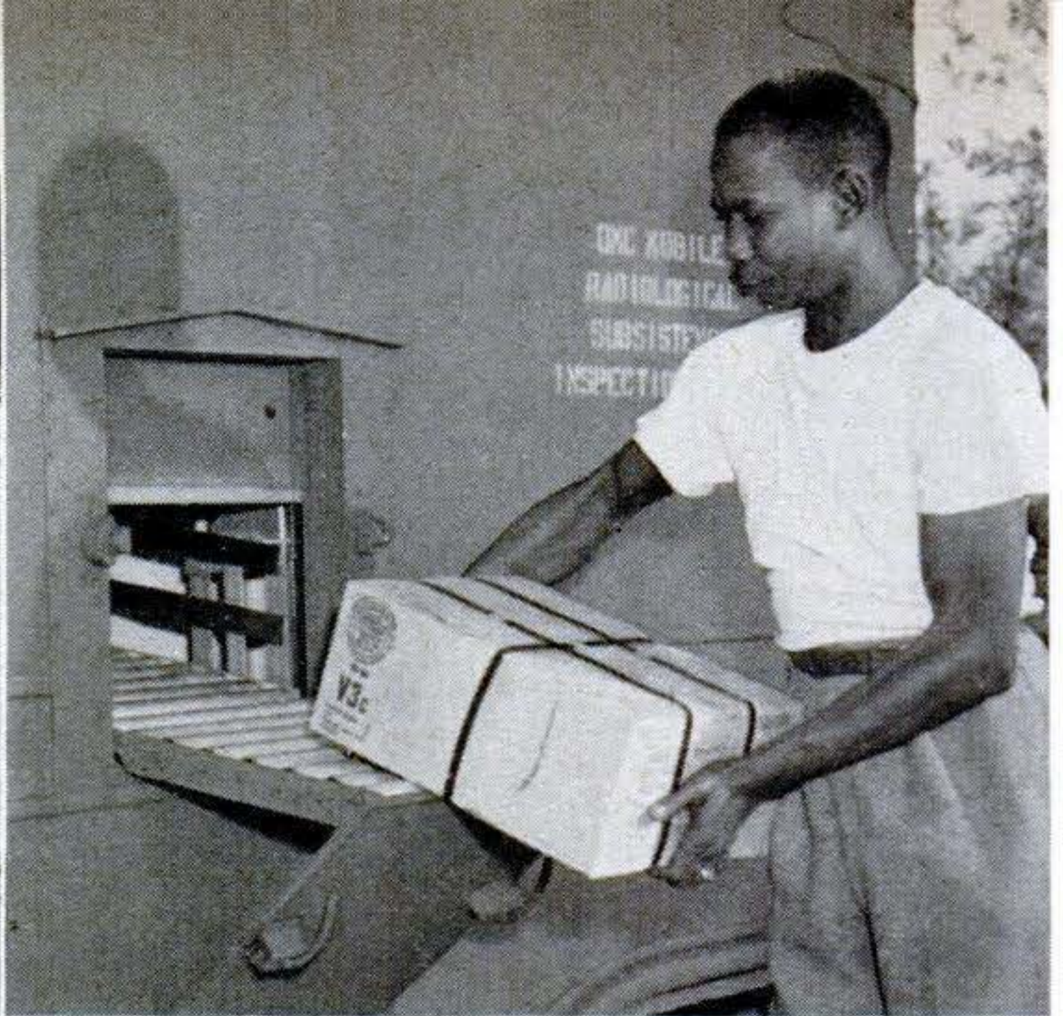
Screen in front of inspector, left, gives him X-ray view of carton of canned goods placed on roller platform, above. To help spot defects, sample film above screen shows typical faults.
