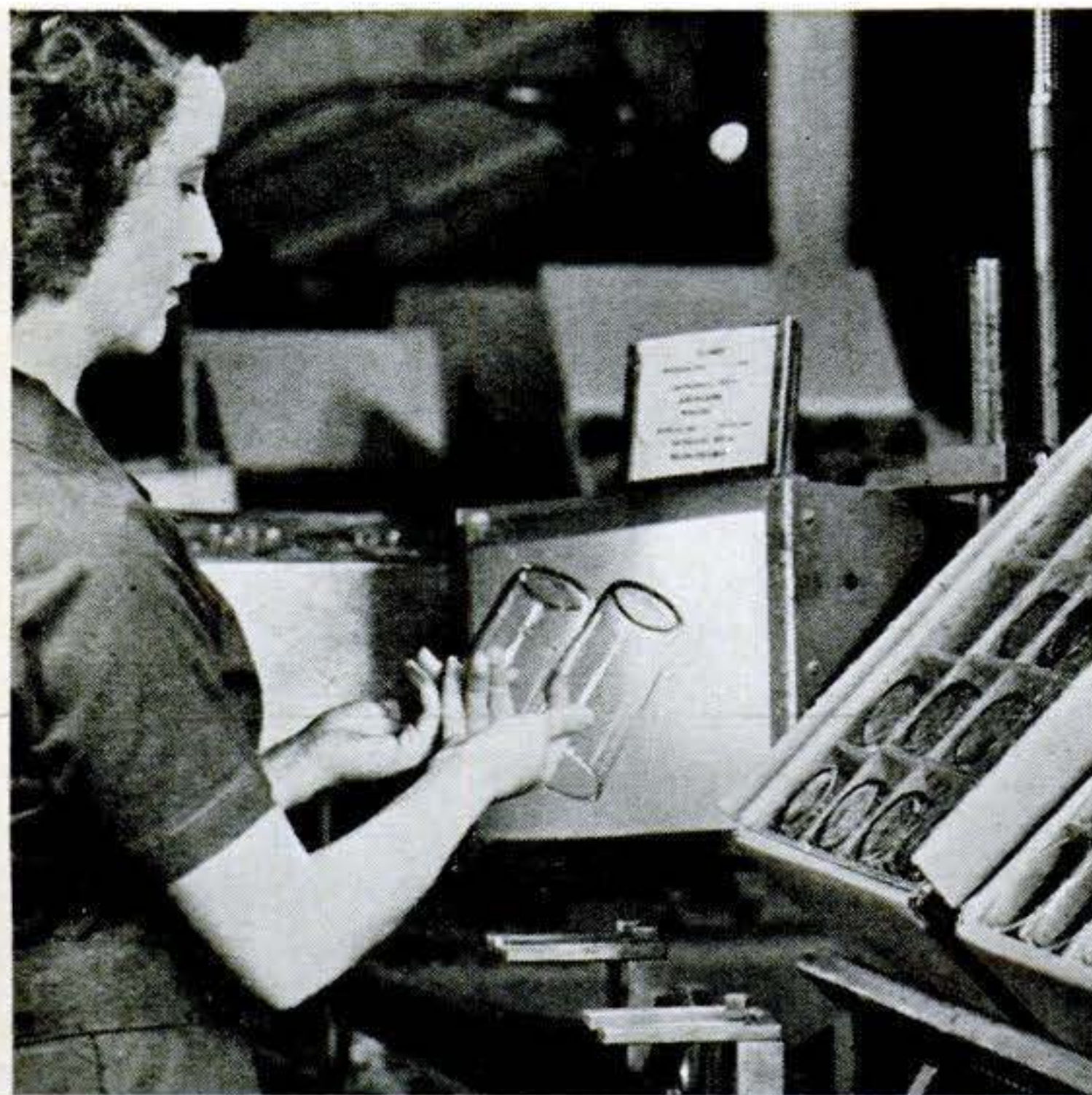
4 After annealing, glasses are carefully inspected in front of the screen of a polariscope. Polarized light from polariscope reveals any stresses that might cause breakage.
