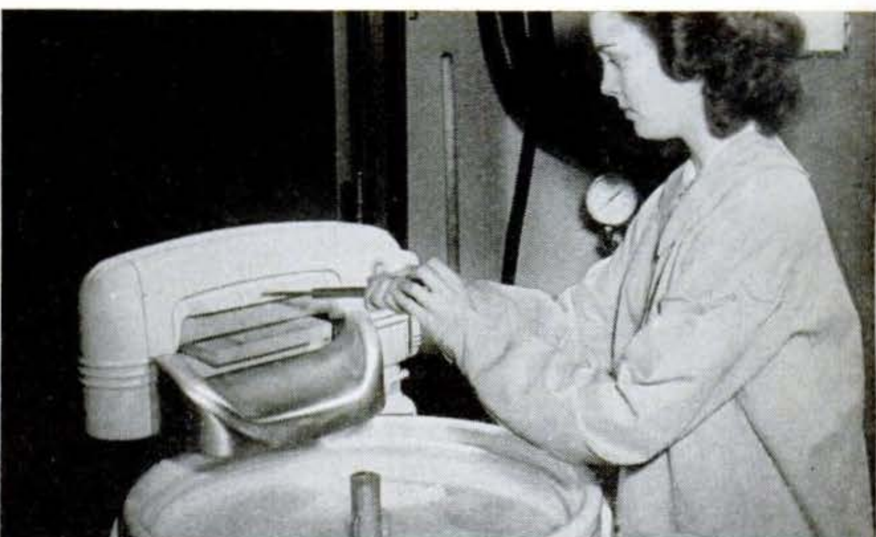
Washing-machine wringer is tested by pressing on safety release with a spring gauge. Rollers must snap open at a push of no more than 20 lb. or wringer is not held to be safe for use.
