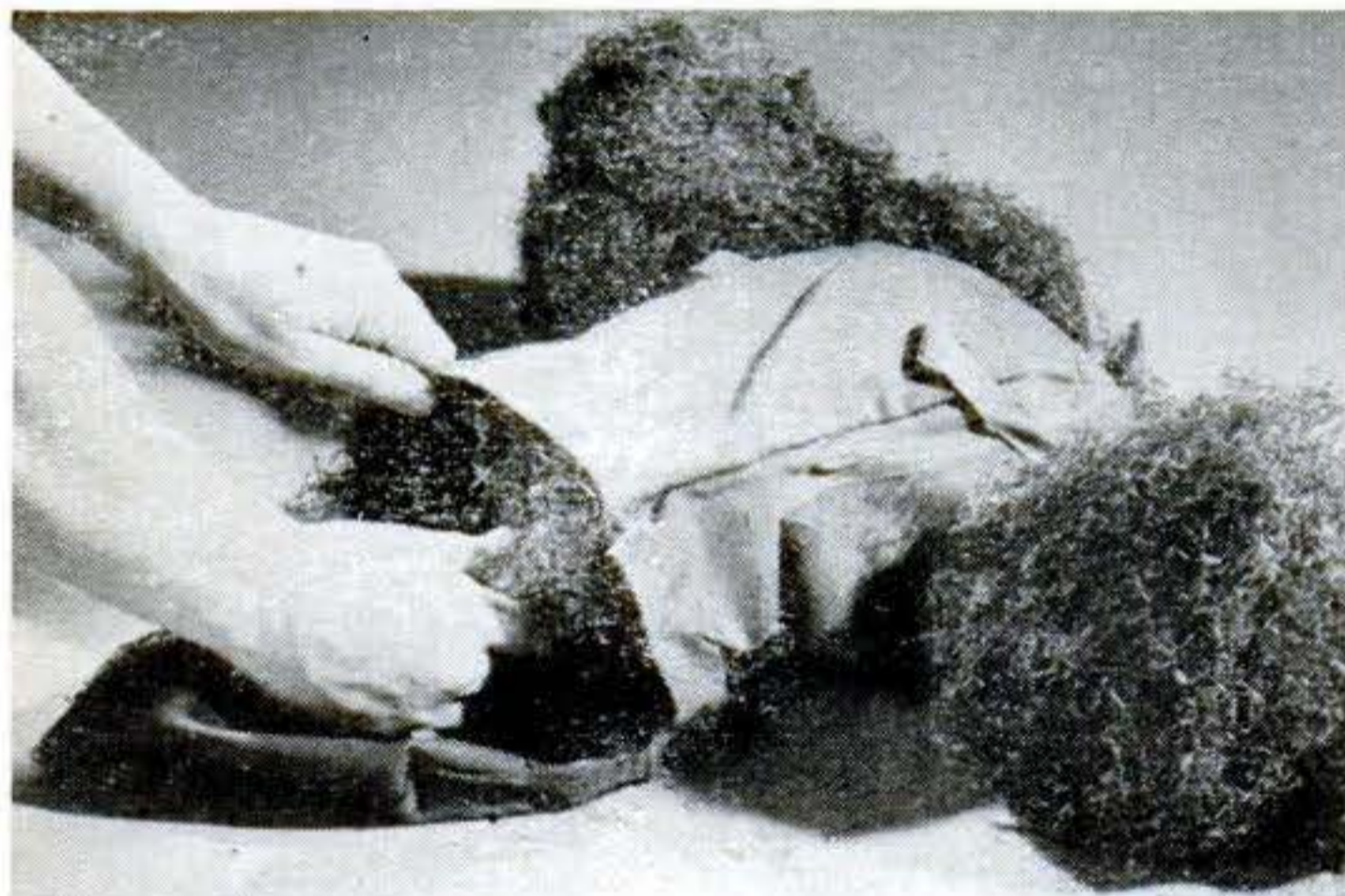
Stuff the bag tightly with upholstery moss. Don't remove any of the tie straps or the car-
