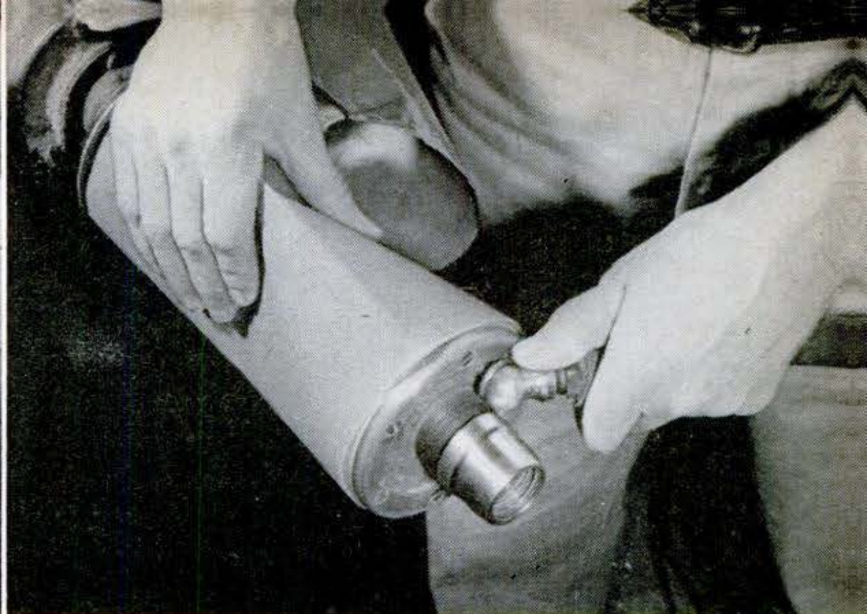
13 "Balloon" sanders get their name from the fact that their spindles are not solid, but are rubber cylinders that can be inflated to provide just the right amount of cushion.
