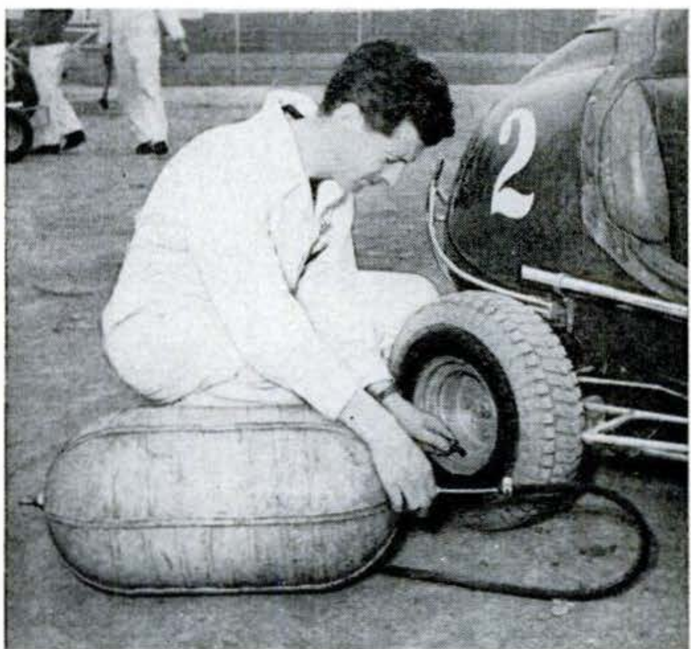
Pit mechanic, fixing flat, inflates tire by attaching bottle of compressed air with hose. Bottle once carried oxygen in B-29 bomber. Welded wheel guard prevents hooking in turn jams.
