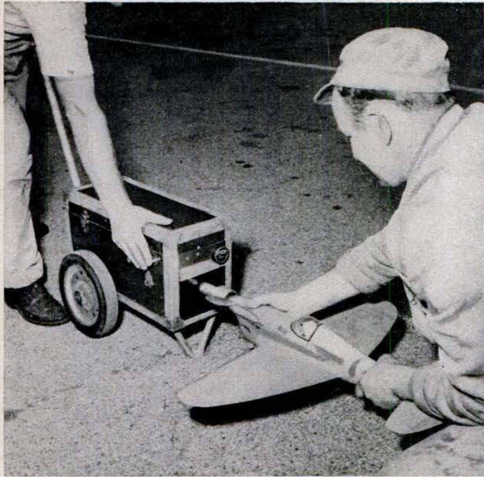
Motors that balk at starting when prop is spun by hand get an assist from cart holding auto battery and starter motor. Rubber-hose fitting grips spinner and whirls model engine to life.
