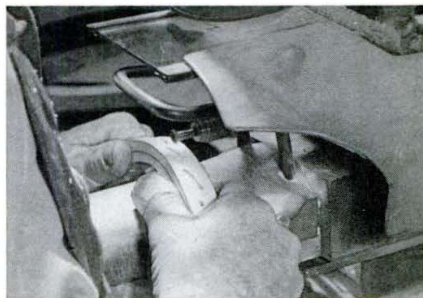
9 After holes are drilled, grooves are routed from hole to hole on outside of the upper end and sides of the bow. These grooves will protect the strings from injury.
