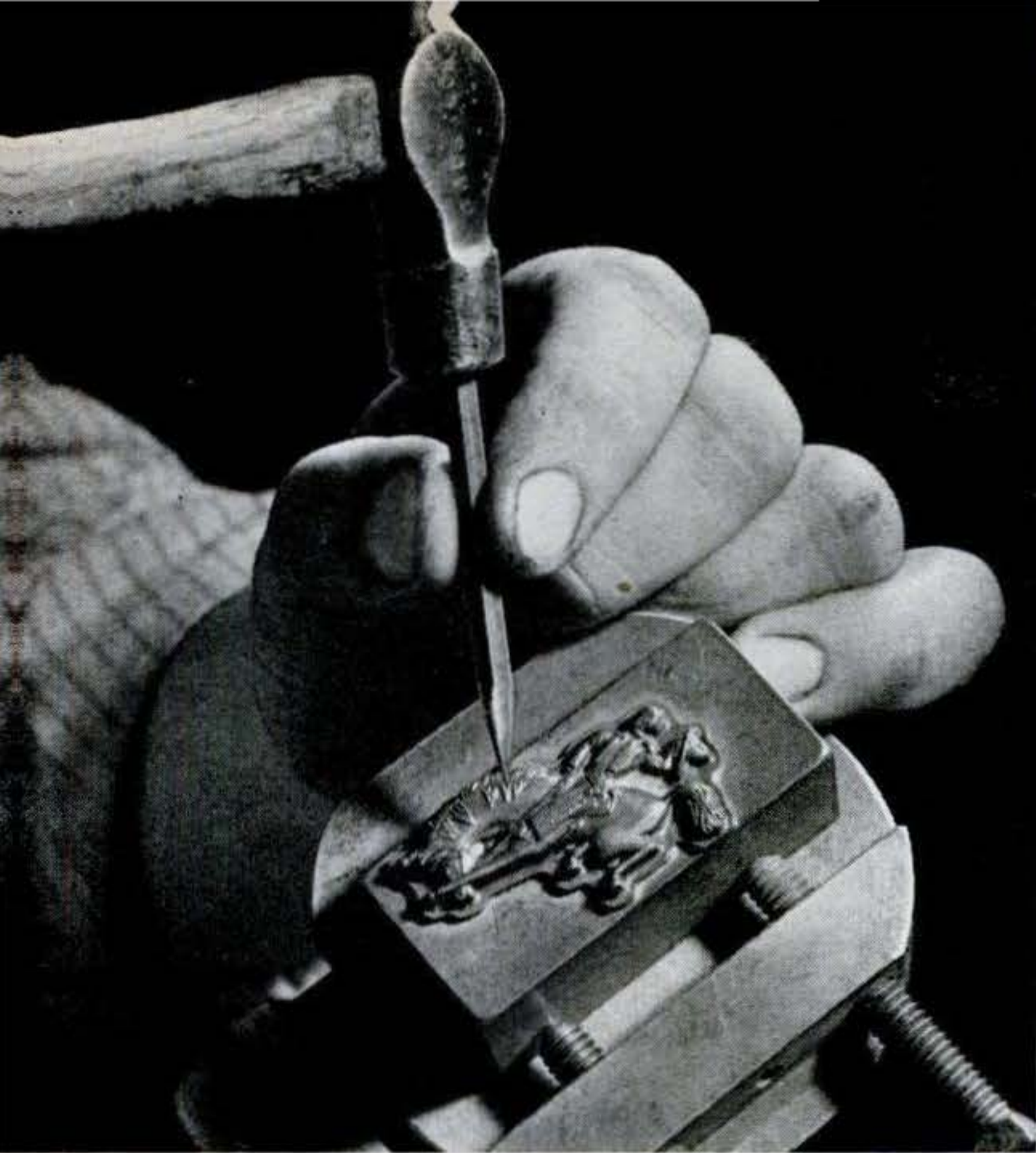
Engraver tools minute details, such as horse's mane, into steel pattern. Tool points are specially ground for many miniatures. Finished pattern, called a "hob," is then hardened.
