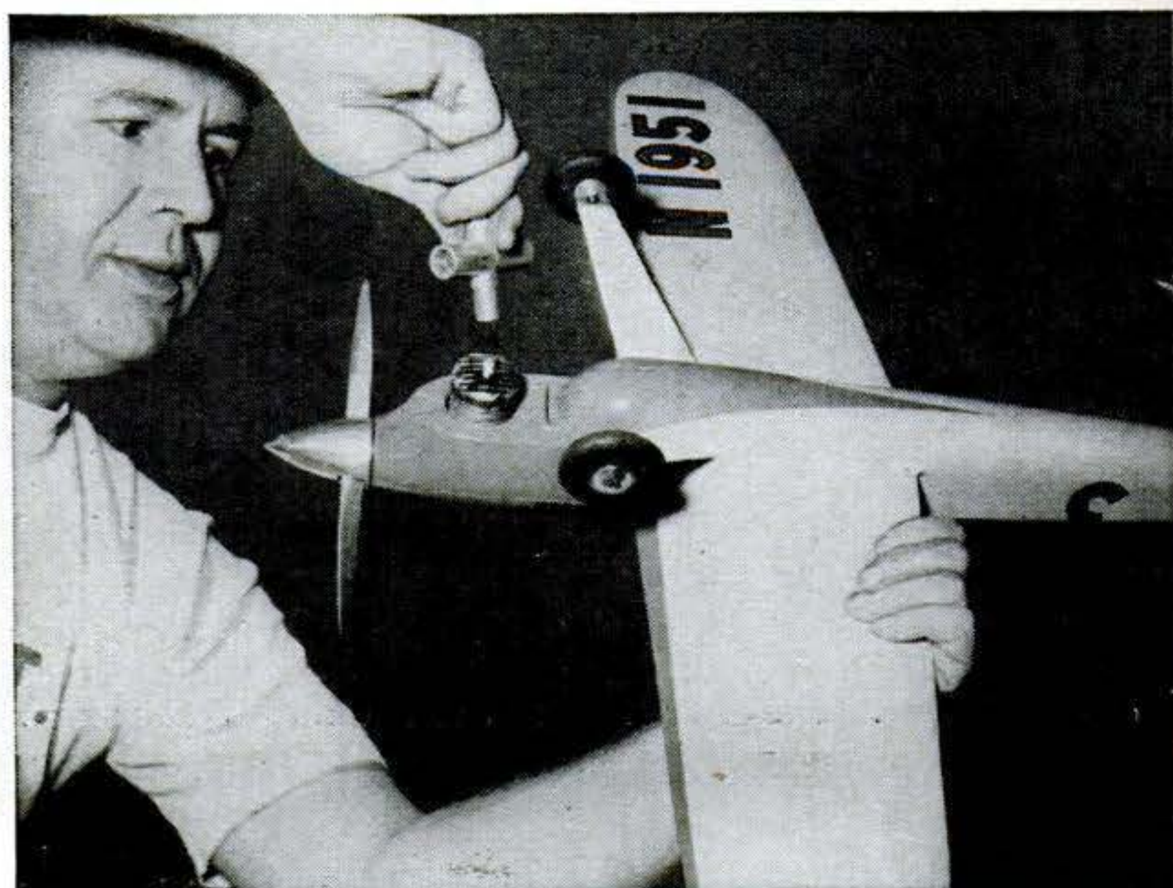
Glow plug is tightened with spark-plug wrench. End of cylinder, projecting through bottom of plane, will be covered by streamlined fairing when model plane has been readied for race.
