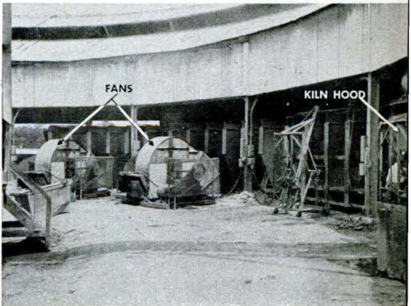
Traveling kilns (beneath roof) heat bricks 21 hours at 2,000°F. to harden them. Leftover hot air, blown through flues, dries and preheats bricks that await firing elsewhere in circle.
