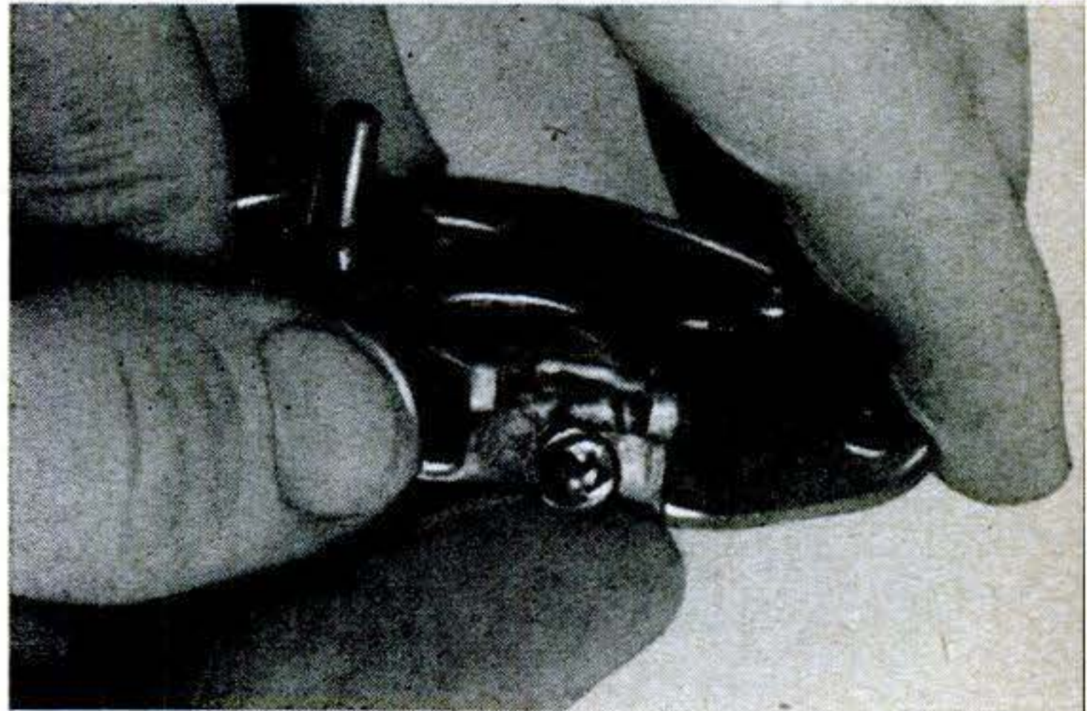
Hardened grease may lock breaker-plate ball bearing. Wash clean with thinner and then lubricate lightly with petroleum jelly.
