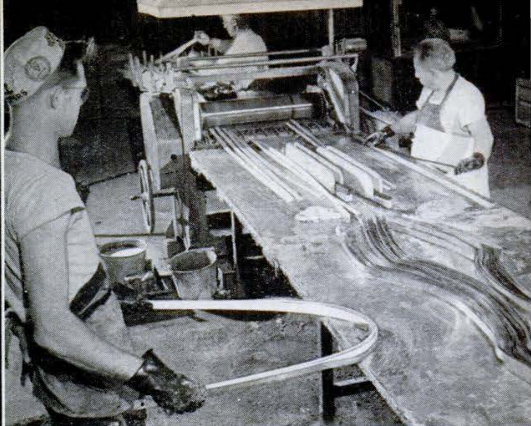
2 After being carefully selected for color and grain, the strips are coated with glue. Then the proper number, together with fiber strips, are bowed inside a metal strap.
