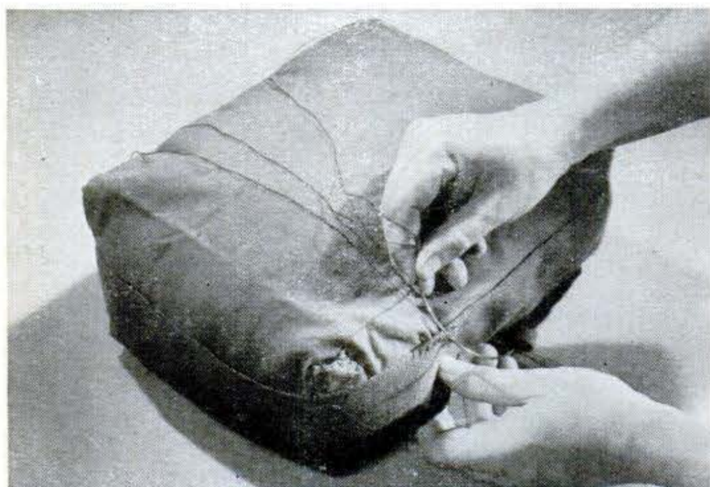
Sew the bag with heavy thread. A curved upholsterer's needle makes the job easier. Cut off
