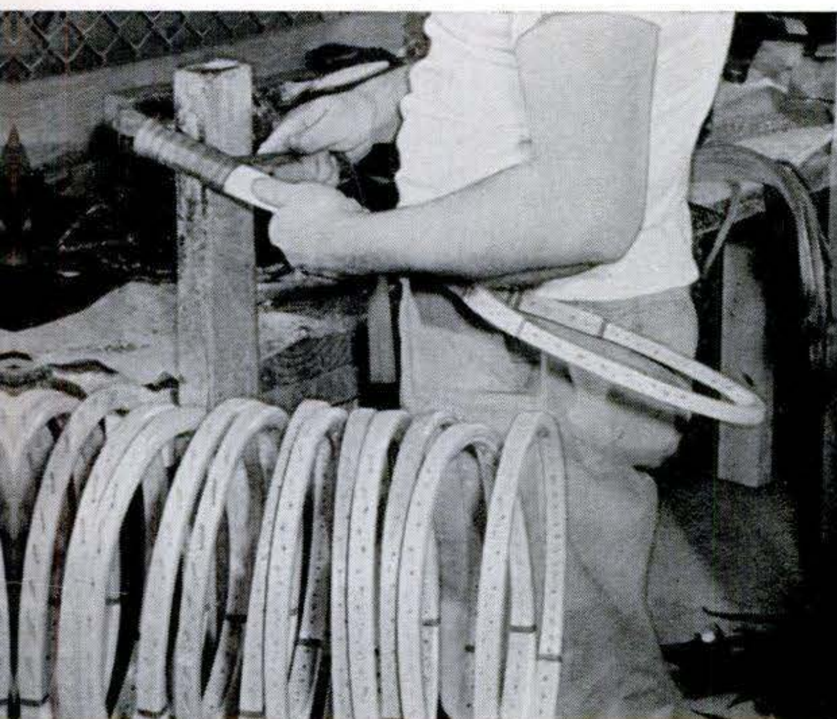
16 After the decorative bindings and decalcomania labels have been applied, a cap is put on the butt of the handle and the leather grip is glued and wrapped into place.
