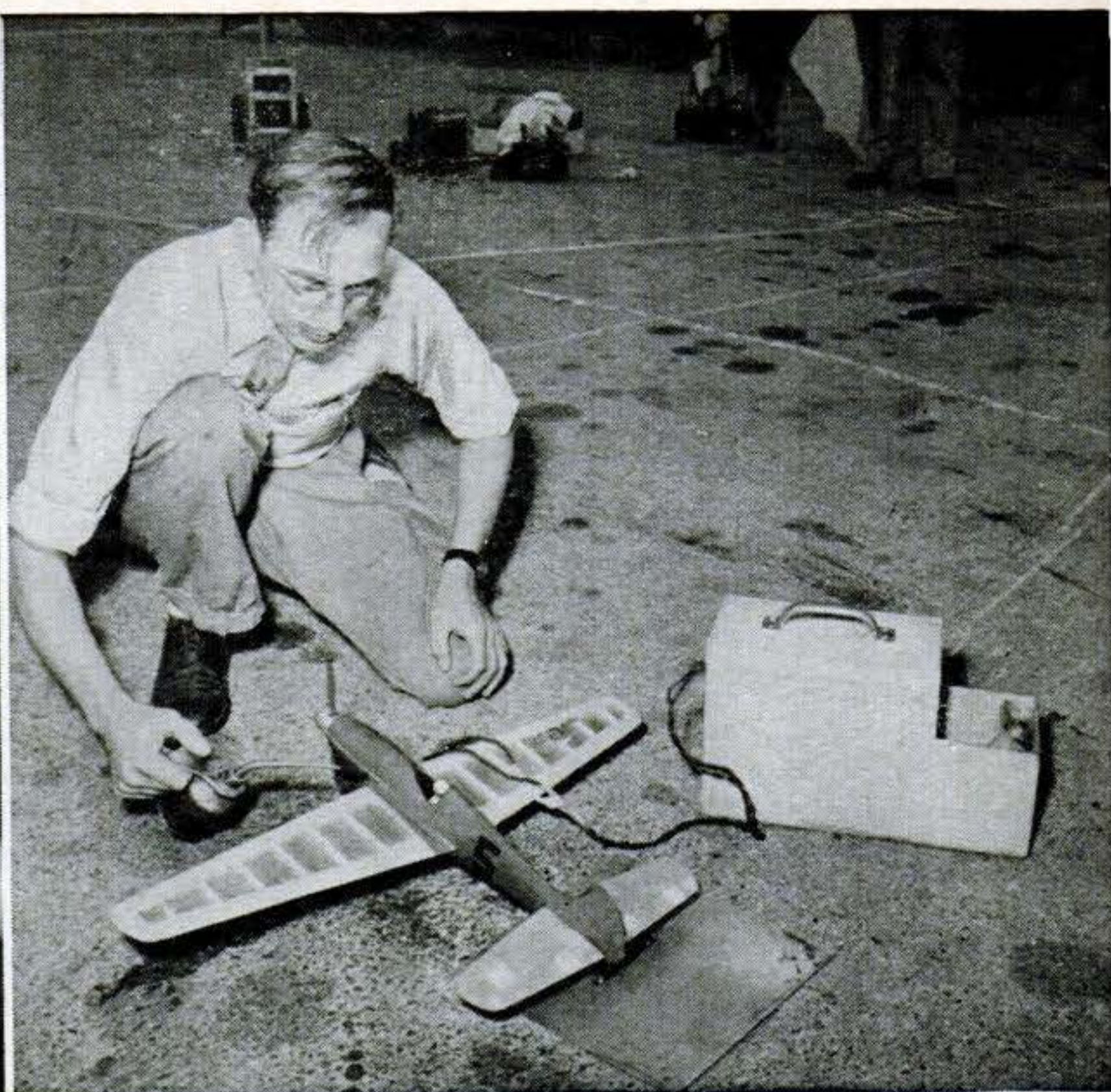
Flight box beside plane being fueled is owner's portable service station. Usual contents include tools, spare parts, fuel, and dry cell, hooked up as shown to heat engine's glow plug.
