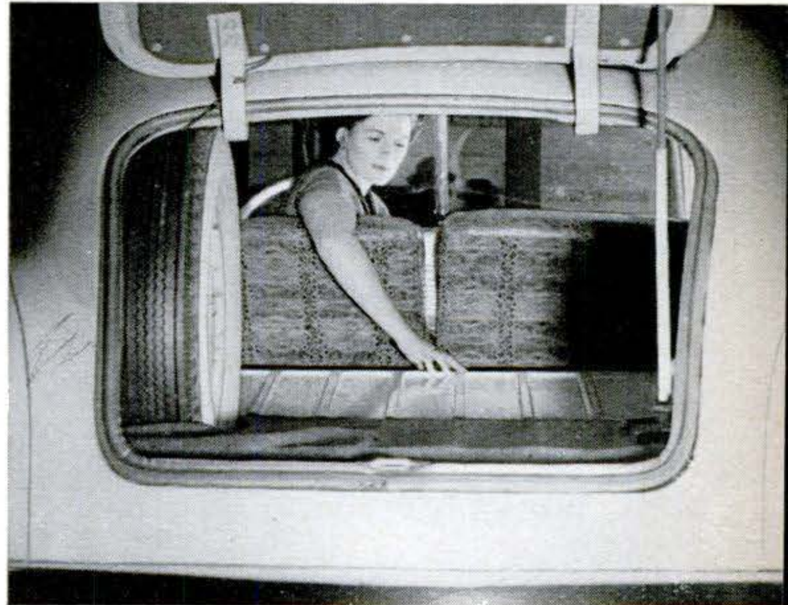
This picture was shot through the back of a de luxe Henry J, which has a rear-opening trunk lid. Back of rear seat is locked down. This model has a divided front seat and special trim.
