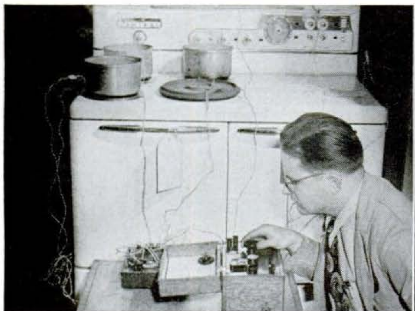
Cooking range is checked for fire hazards by thermocouples attached to 20 points on stove. With oven and burners on, tester notes whether temperature anywhere exceeds the safety limit.
