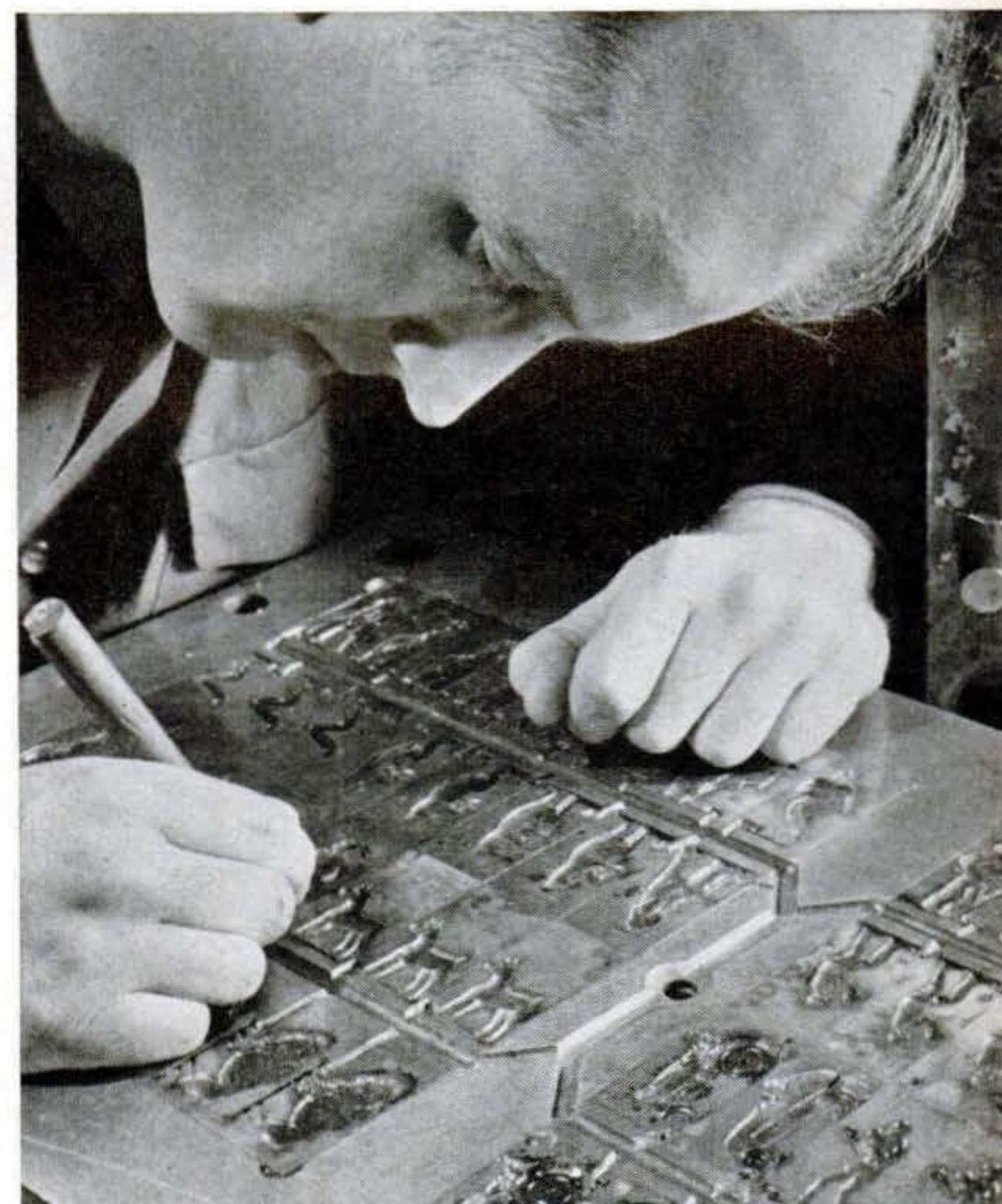
Polisher uses diamond-burnishing compound to remove any flaws or impurities from cavities just before they go to the molding machine. Care here avoids production stoppages later.
