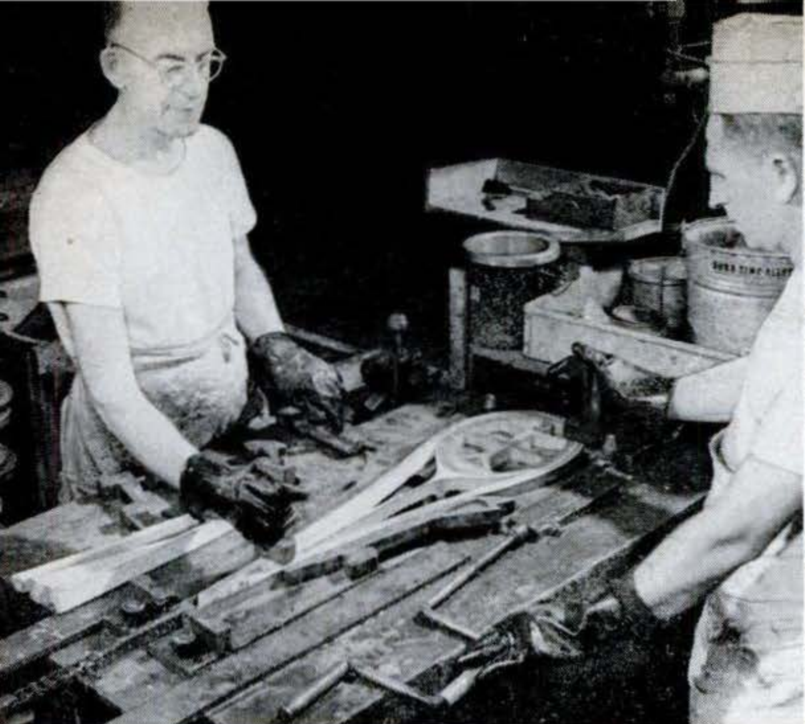
3 Strap and strips then go to bending machine. Straps are placed around a metal core, and ends are attached to a hydraulic plunger. Then other wood parts are put in place.
