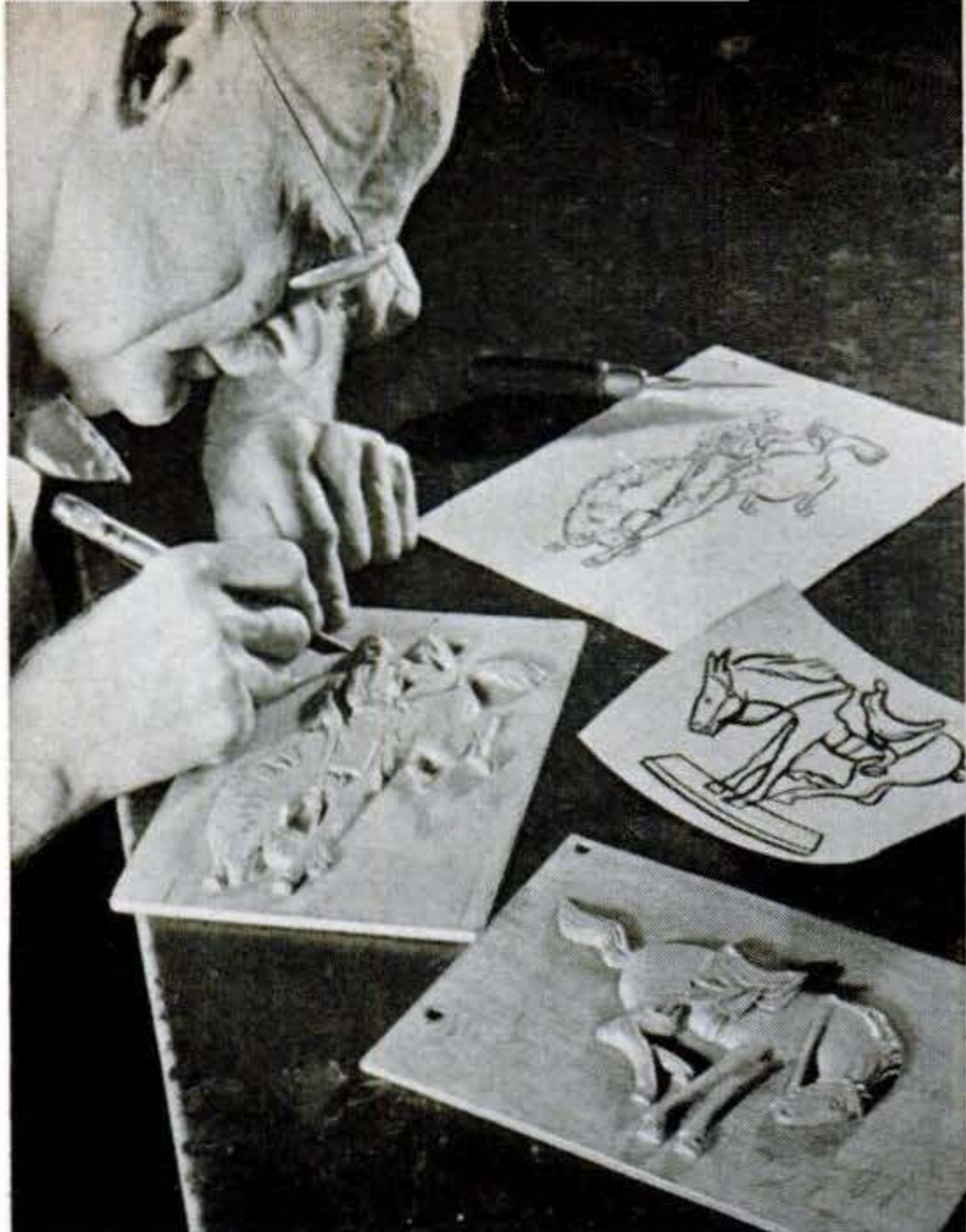
Modelmaker Cloy D. Niver, guided by artist's sketch for a premium, carves whitewood pattern four times the size of future plastic figure. Often he adds intricate touches of his own.
