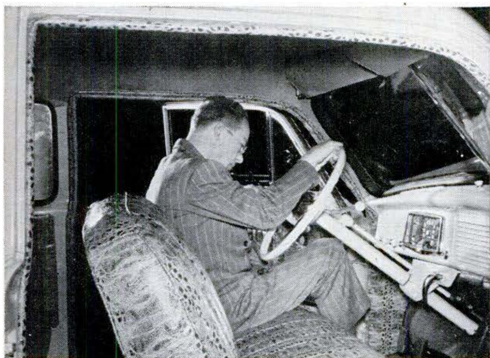
The Henry J's entrance room was a bit better than the Rambler's—40¼ by 27. Both had the disadvantage found in all two-door sedans—a tight squeeze getting into the back seat.
