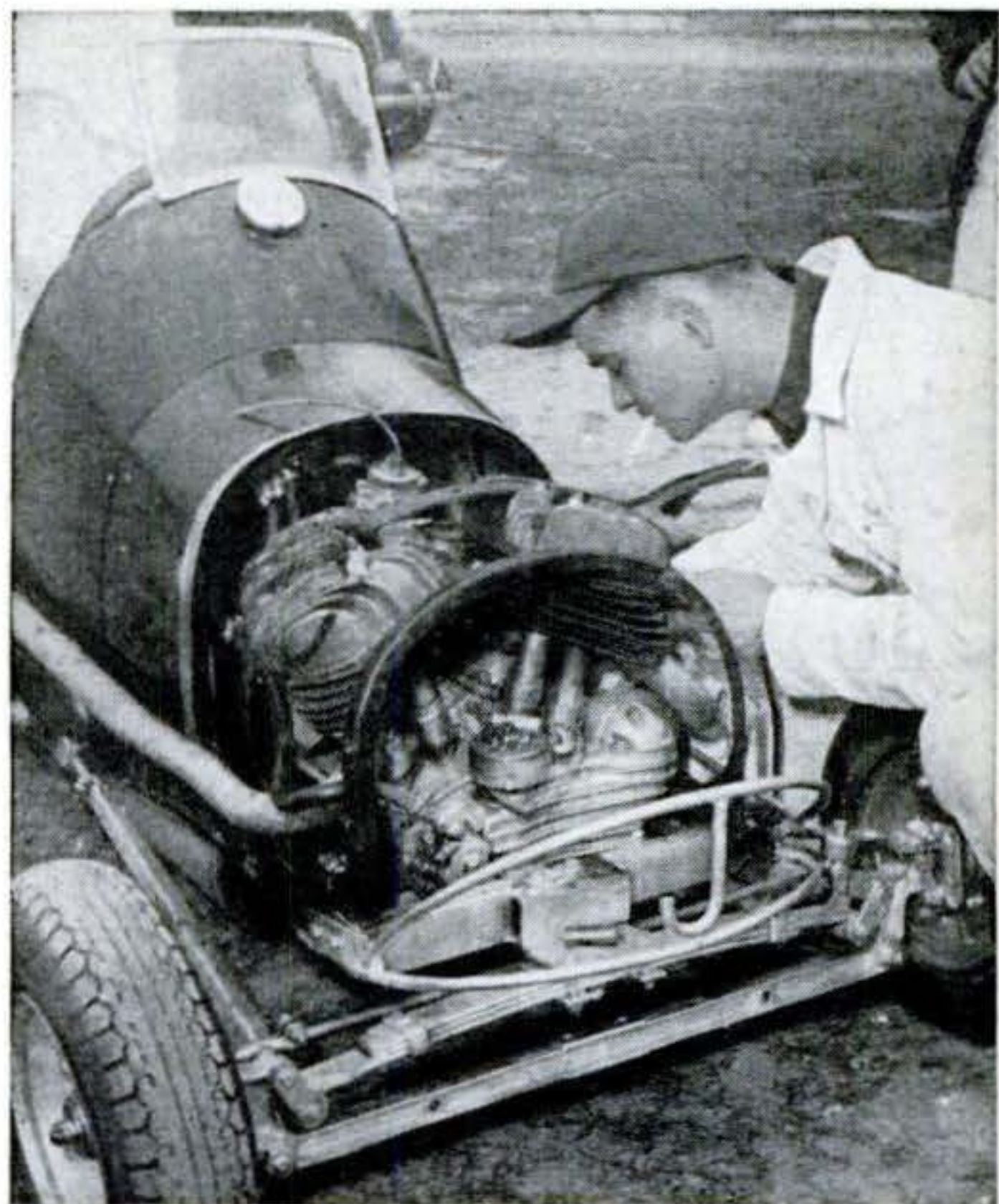
Motorcycle engines serve as power plants for three-quarter midgets. This tiny racer has front-mounted twin Harley, of 45-cu.-in. displacement, driving car through rear wheels.
