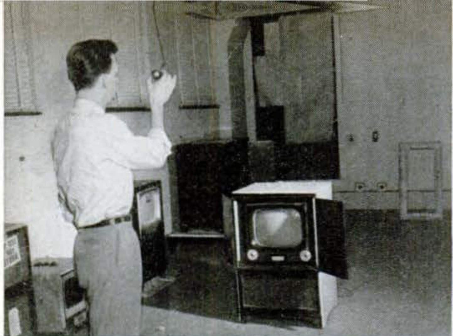
Glass or plastic safety mask on TV set is tested for shatter-resistance by letting a 2-inch steel ball, hung from the ceiling, swing against it three times from 51 inches away.
