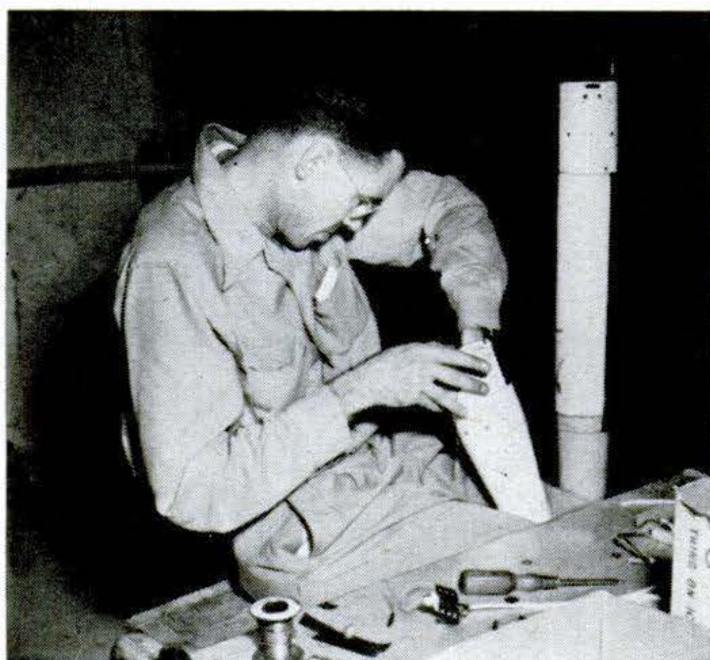
Parachute is packed carefully into nose section. Powder charge explodes nose from engine, and another charge blows 'chute out to bring recording instruments down safely.
