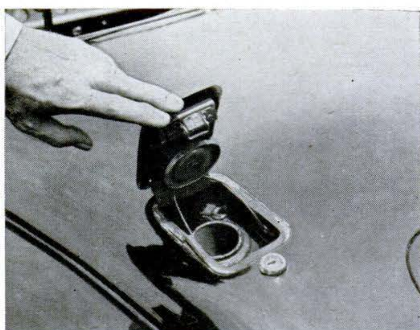
Like all sports cars, the Jag is full of items like this integral gas-tank lock cap. But the car badly needs a couple of air vents to cool the feet. It will do an honest 125 m.p.h.
