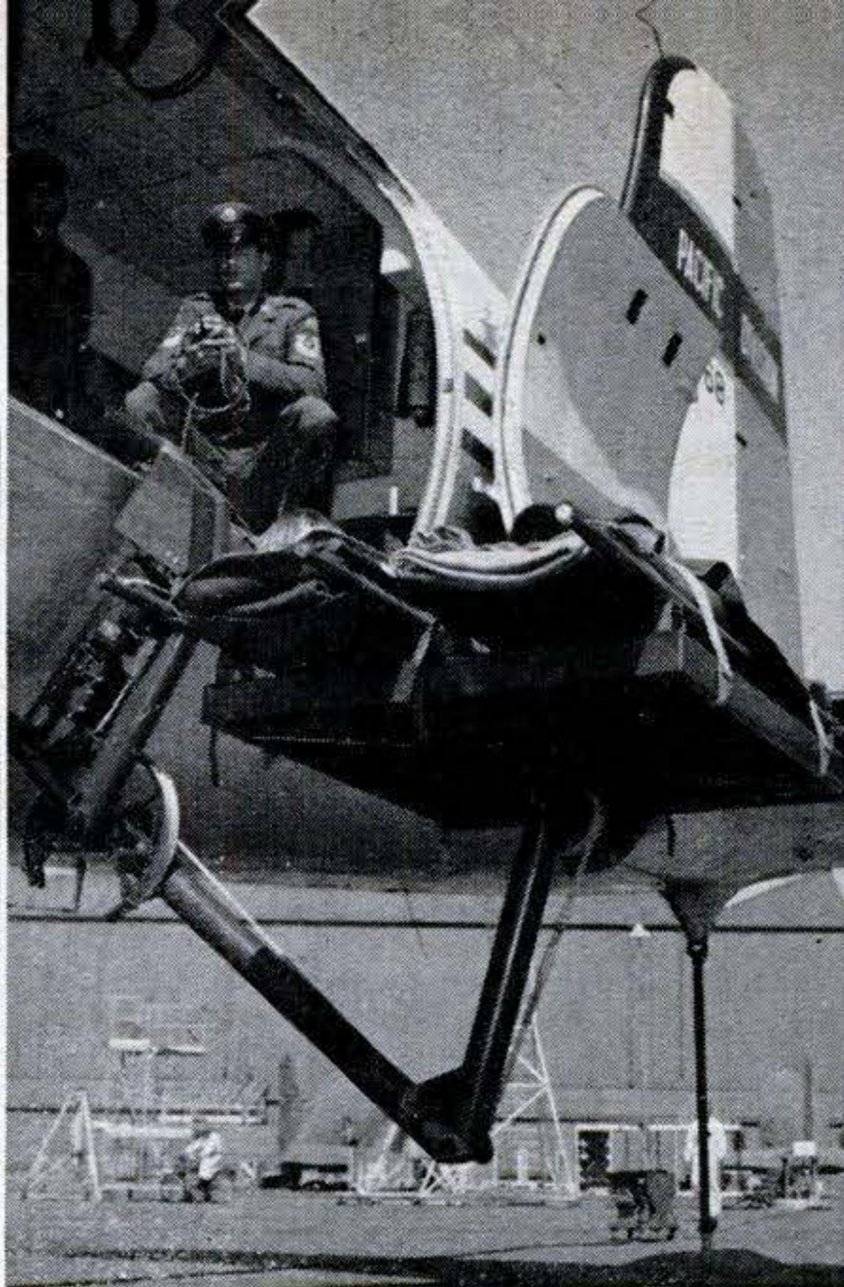
Patients move smoothly and are kept in a perfectly level position as they ride up into plane.
