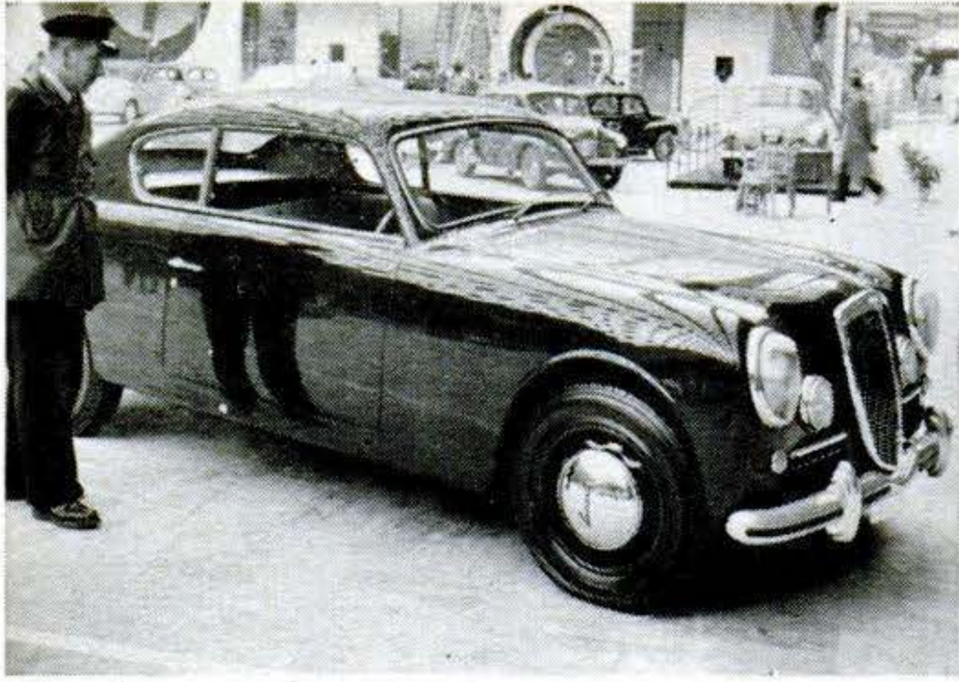
The Lancia Aurelia Gran Turismo is a two-door coupe for two or three passengers. Its six-cylinder engine puts out 75 hp. Only 55 inches high, it has a wheelbase of 112½ inches.
