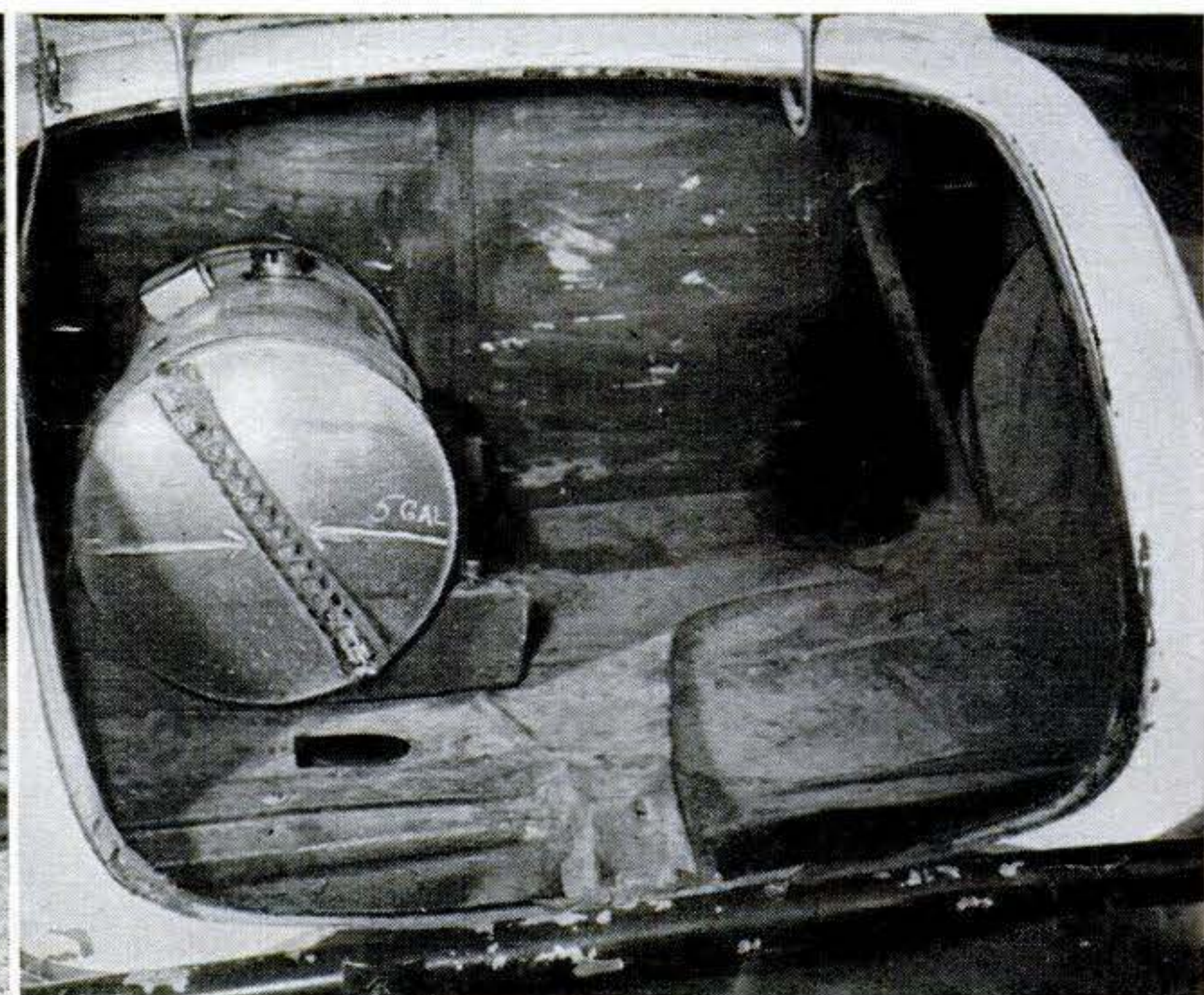
Gasoline tank is in trunk. In front of tank is a metal firewall to protect driver. Zeke mixes his own gas, uses lots of Ethyl. He gets four to five miles a gallon.
