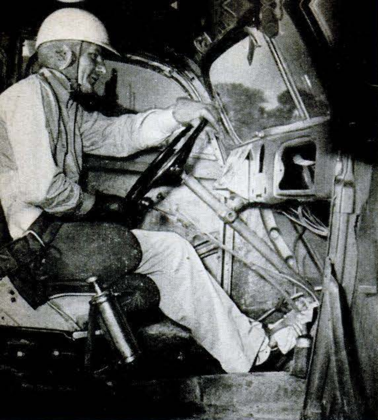
Champion driver in New York area is Johnny Zeke, 30, a believer in safety belt (under elbow) and caution. Pump near seat builds up air pressure in gas tank to aid starting.
