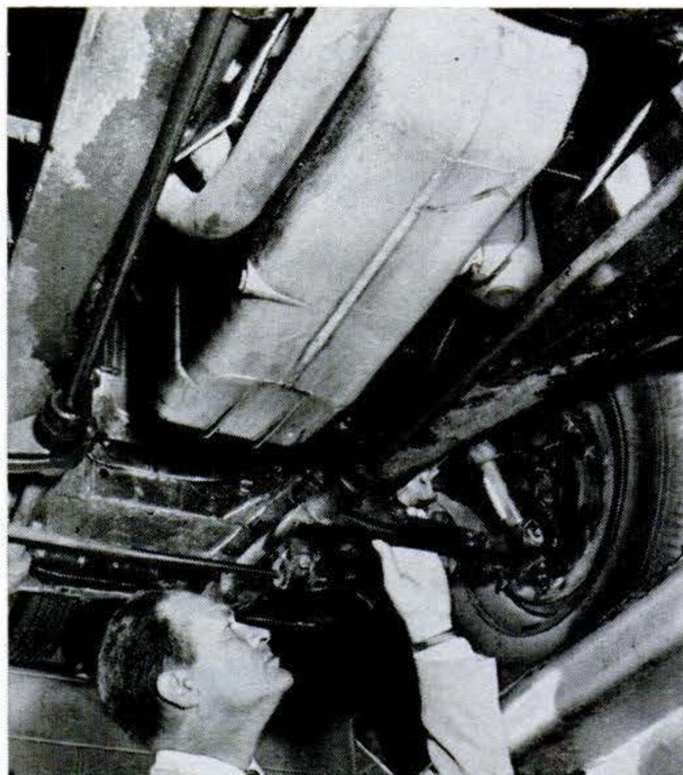
I liked the Jag's underpinnings best. Its stabilizing transfer torsion bar between the front wheels is just now being adopted for racing cars. The ground clearance is 7 1/8 inches.
