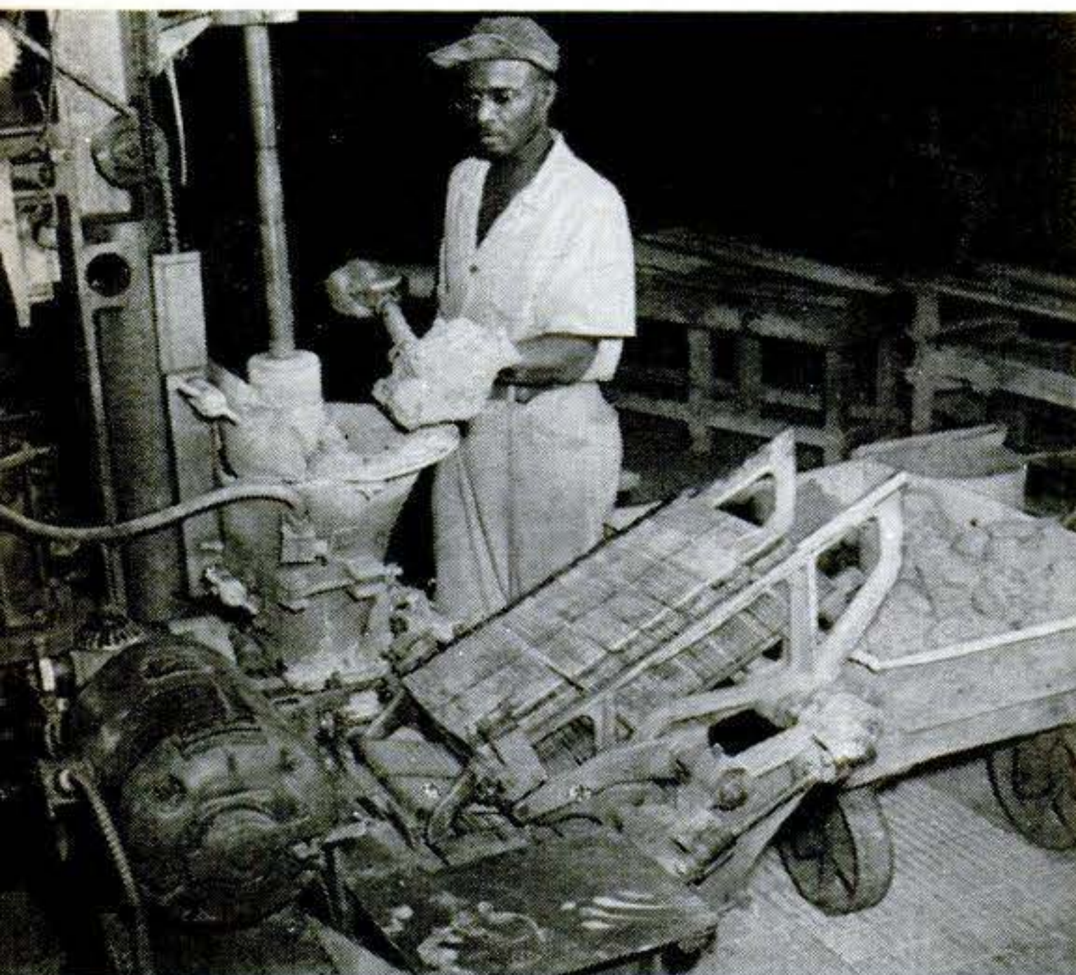
Pasting machines , which apply the active materials to the cast grids, also are completely automatic. Photo above shows active material and cast grids being fed into a machine.
