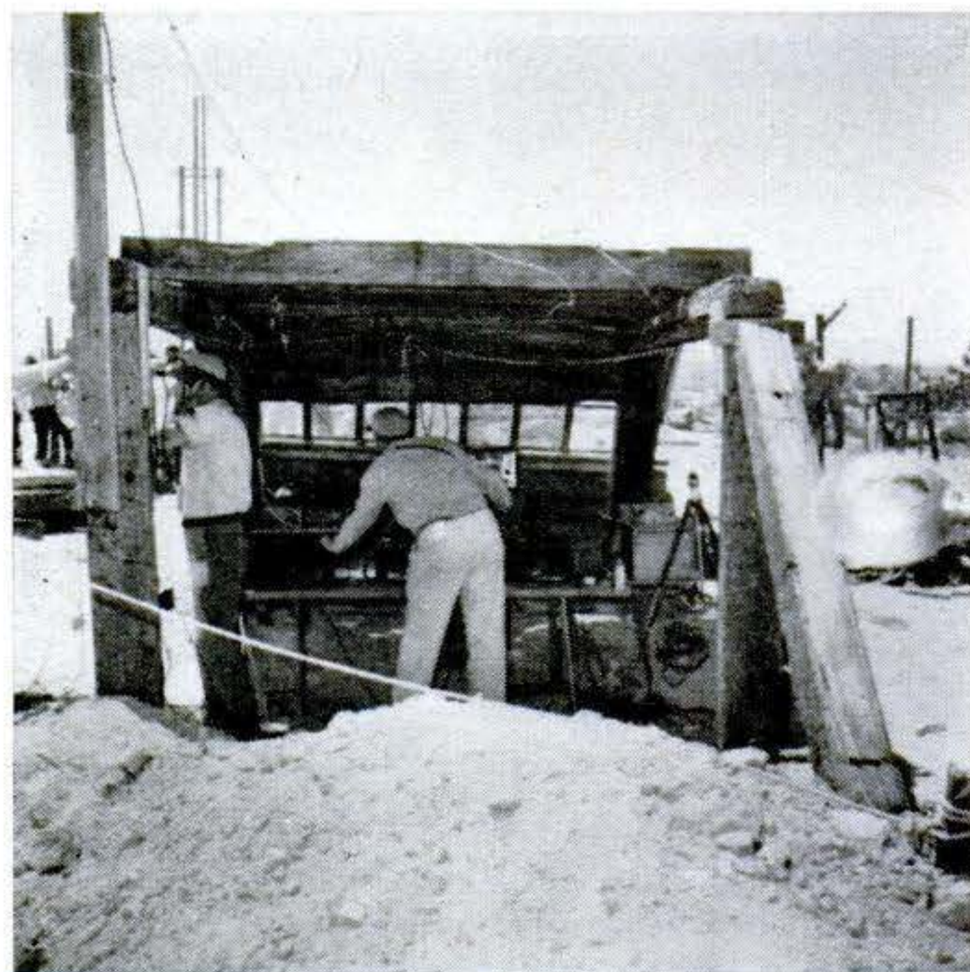
Test crew is protected by shelter built from old bridge timbers and bulletproof glass. Panel connects warning siren, distant trackers, loudspeakers and firing circuit.
