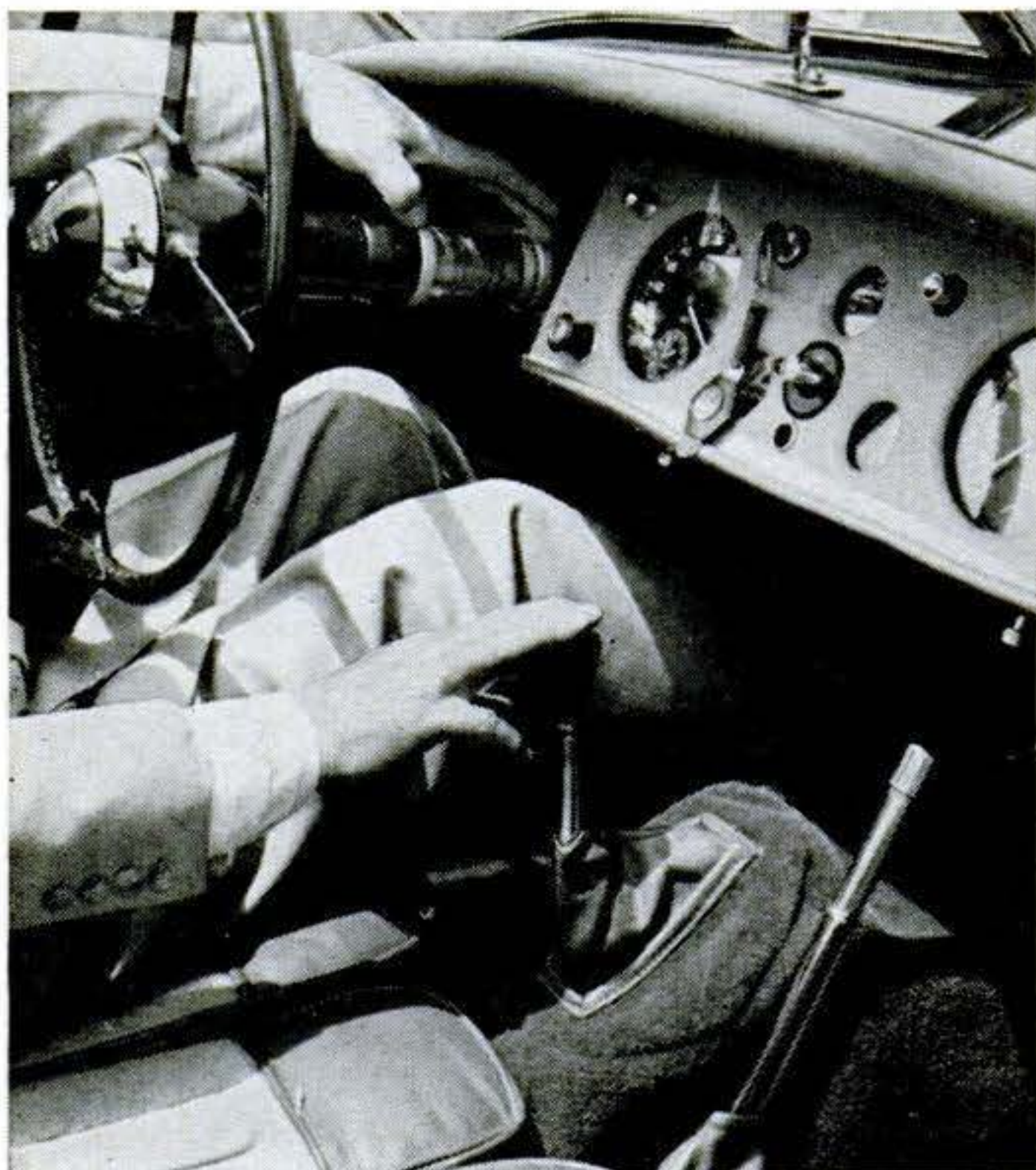
Like the Nash-Healey, the Jaguar has a pencil-length gearshift lever, an adjustable steering wheel and a floor tunnel of acceptable height. The car has four forward speeds.
