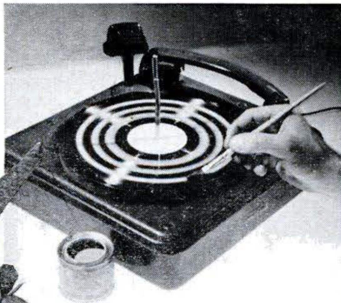
You can add color to the "pot" by painting stripes on it this way. Hold dipped brush against record as it spins.
