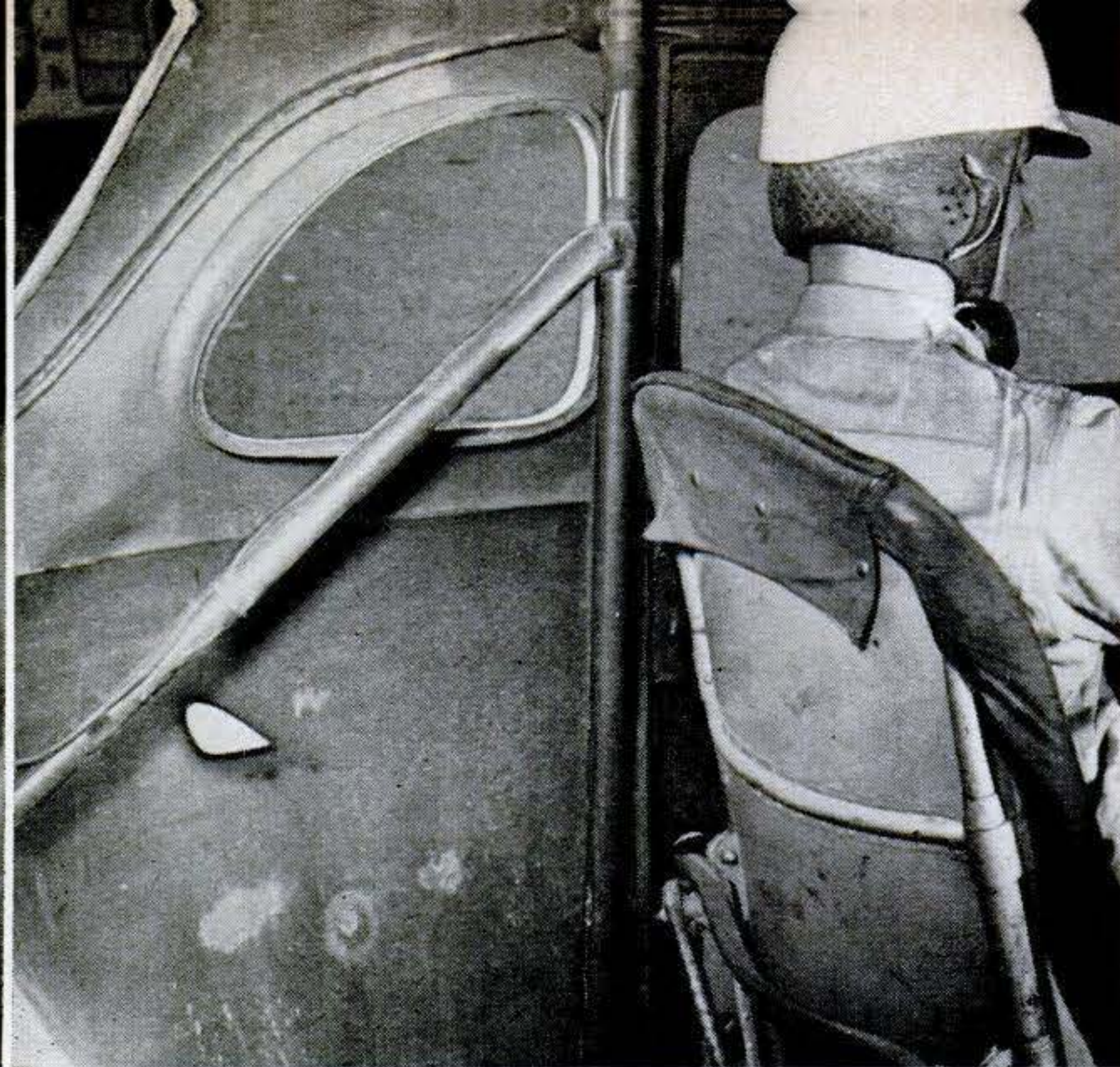
Rollover bars (steel framework behind Zeke) hold up roof in turnover. Helmet is plastic, lined with foam rubber. Zeke thinks bars, belt, helmet should be used by highway drivers.
