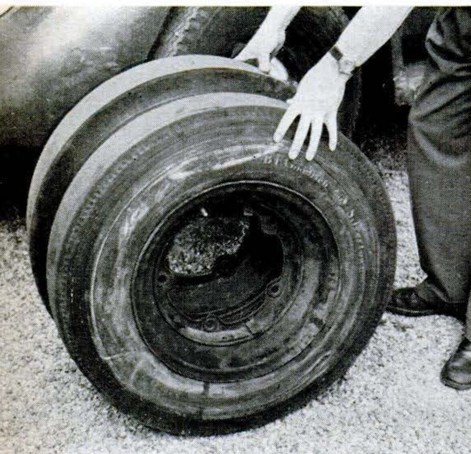
The tire for his left rear wheel (foreground) is smaller than tire for right wheel (behind it). Differential action is eliminated, and right (outside) wheel travels longer distance.
