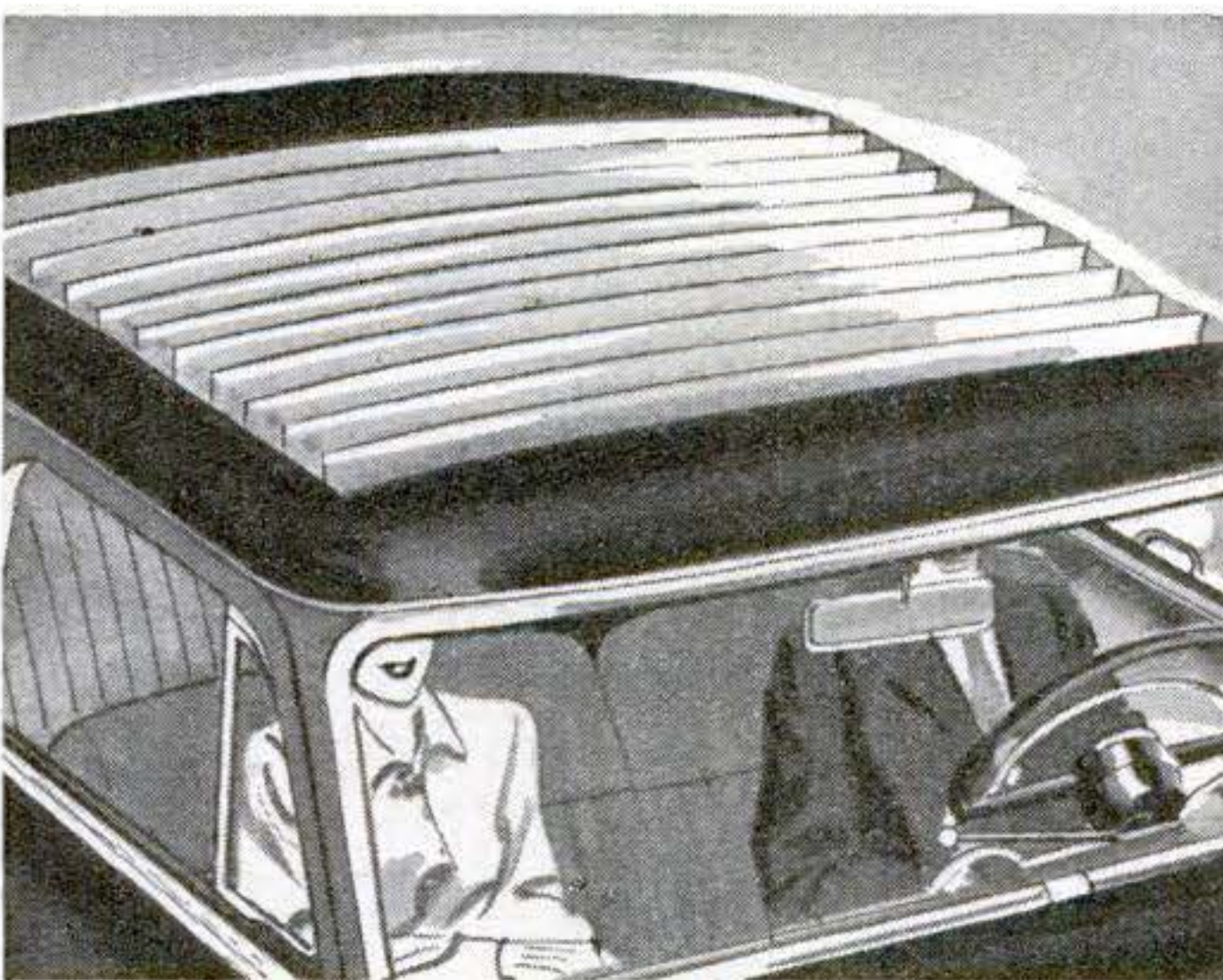
A VENETIAN-BLIND AUTO TOP for controlling sunshine, air and visibility. Waterproof when shut, it would be operated by a crank on the dashboard.— Irving Surdam, Winsted, Conn.
