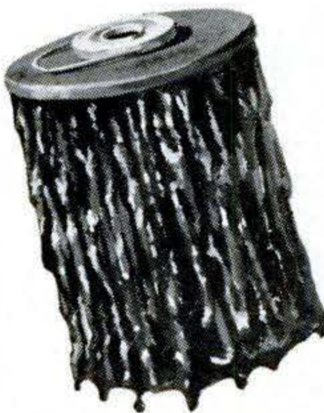
REPLACE CLOGGED OIL FILTER
