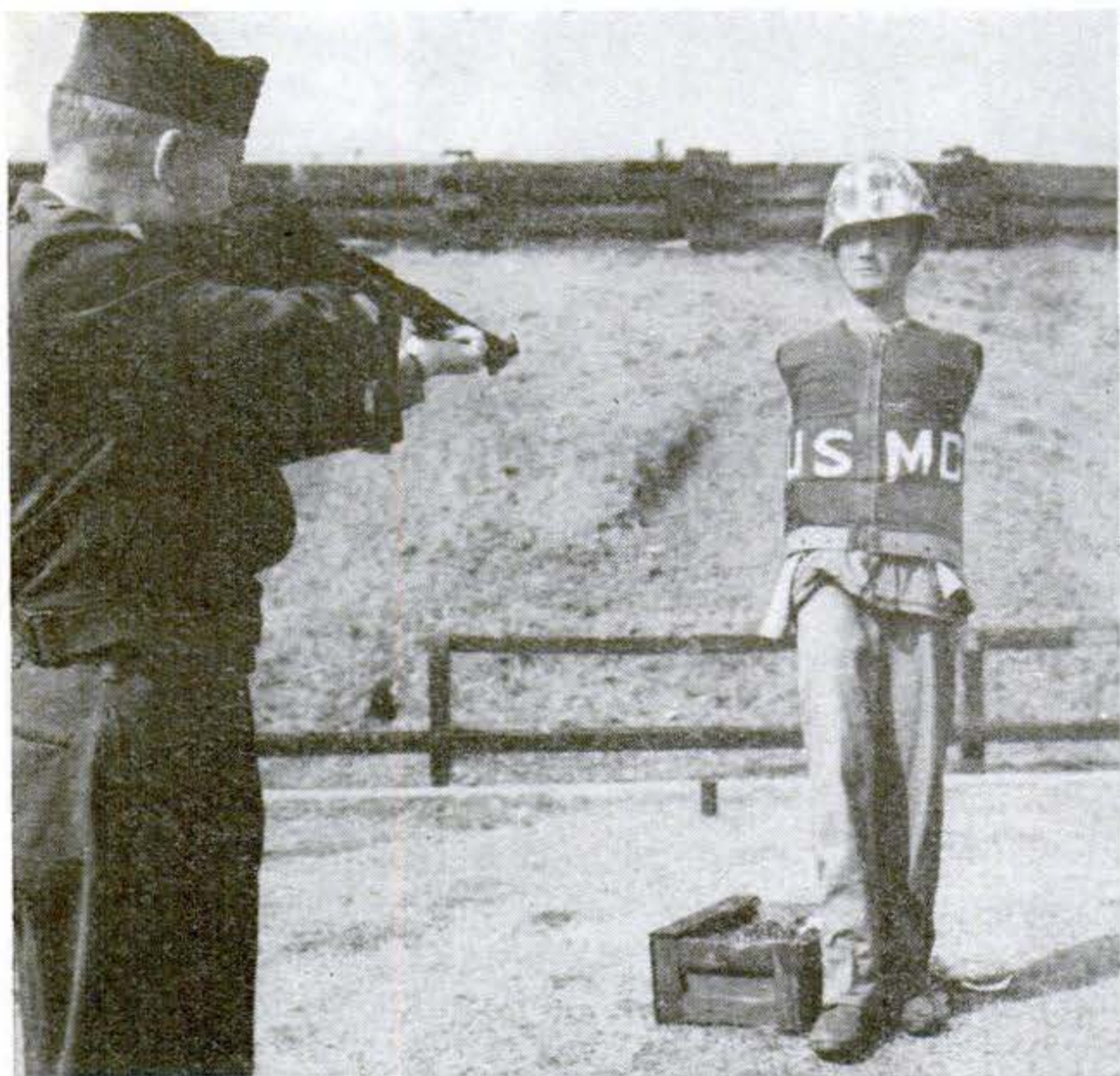
HOW NEW ARMOR STOPS BULLETS: Demonstrator at left above fires .45-cal. submachine gun point-blank at dummy wearing Marine Corps armored vest. Photo at right shows
